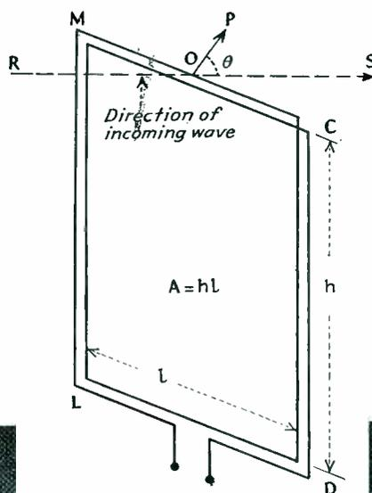
Fig. 1 (above)—Loop diagram for which equation (1) is derived.
