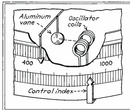
Arrangement of pick-up coils and aluminum vane
