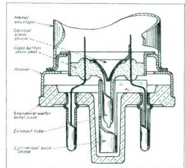
Base construction of the new RCA single-ended pentodes is shown in this cross-section diagram. It also shows shield cone and cylinders for reducing inter-electrode capacitance.
