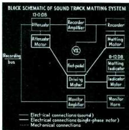
Fig. 3—Block diagram showing the functional arrangement of equipment for sound track matting system
