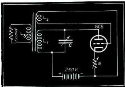
Fig. 1—Circuit of sine-wave oscillator using negative feedback
