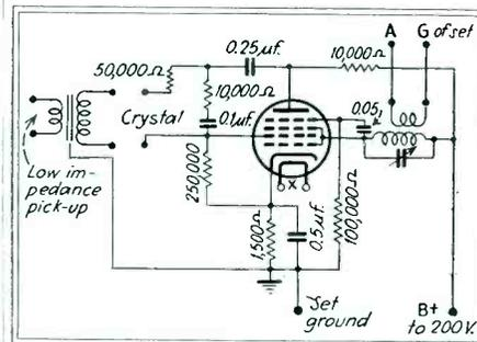
Fig. 1—Basic circuit of phonograph oscillator
