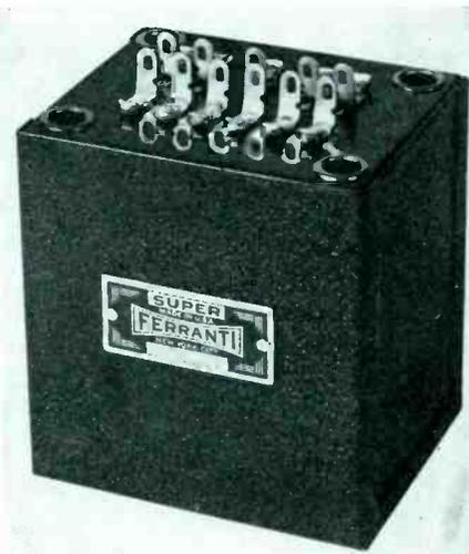
ohms; secondary 15,000/60,000 ohms; operating level —80 to +20 db; primary unbalanced 4 ma.; primary current per leg 50 ma.; operation is from a line to a single or push-pull grid and the weight of the unit is 2 lbs.
