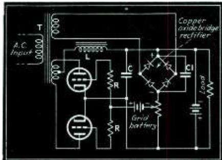
Fig. 2—Full-wave self regulated rectifier circuit
