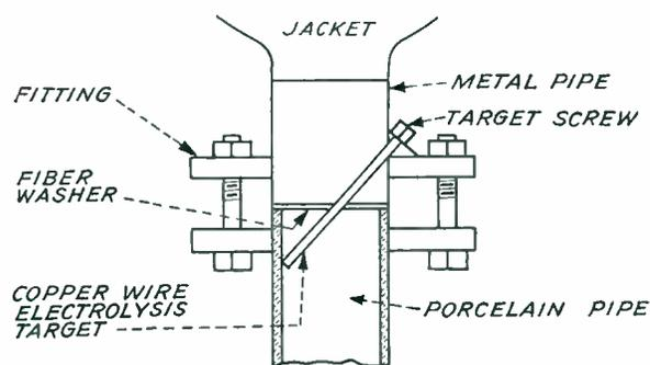
Fig. 5—Drawing showing how targets work
