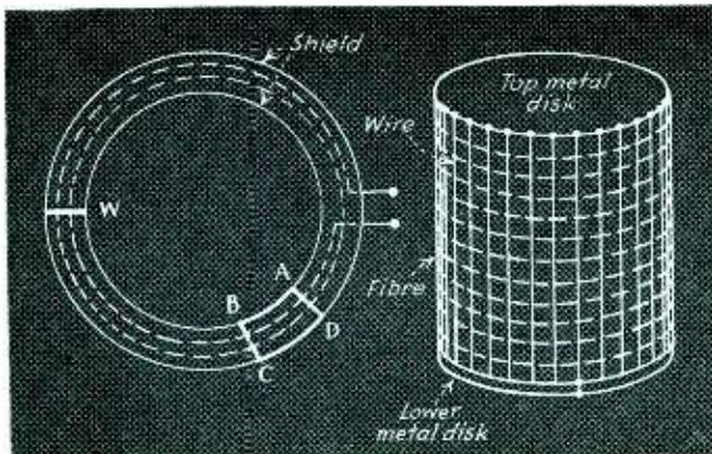
Fig. 4A (left)—Electrostatic shield in which loop winding is enclosed in metallic tube.
