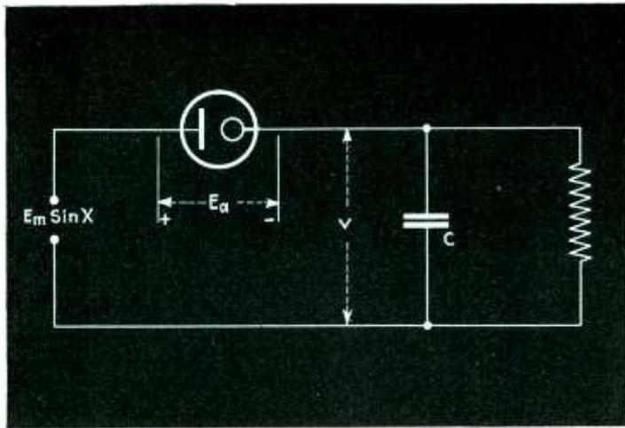
Fig. 6—Gas tube rectifier circuit having resistive and capacitive plate loading
