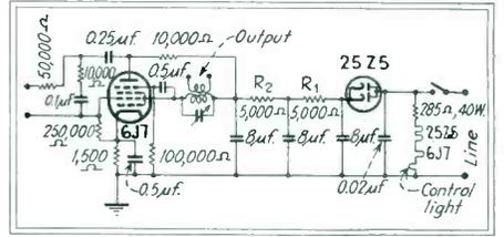
Fig. 2—A-c d-c version of circuit
