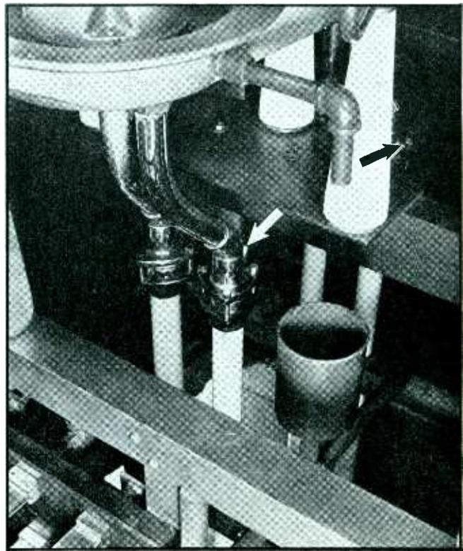
Fig. 2—Method of attaching the pipe to the water jackets. Note electrolysis target
