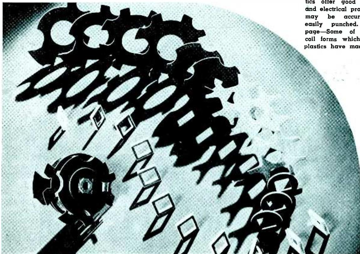
**Punchability.** Laminated plastics offer good mechanical and electrical properties and may be accurately and easily punched. Opposite page—Some of the many coil forms which laminated plastics have made possible
