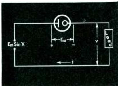
Fig. 1, above—Fundamental half-wave rectifier circuit using gaseous rectifier for which analysis is carried out
