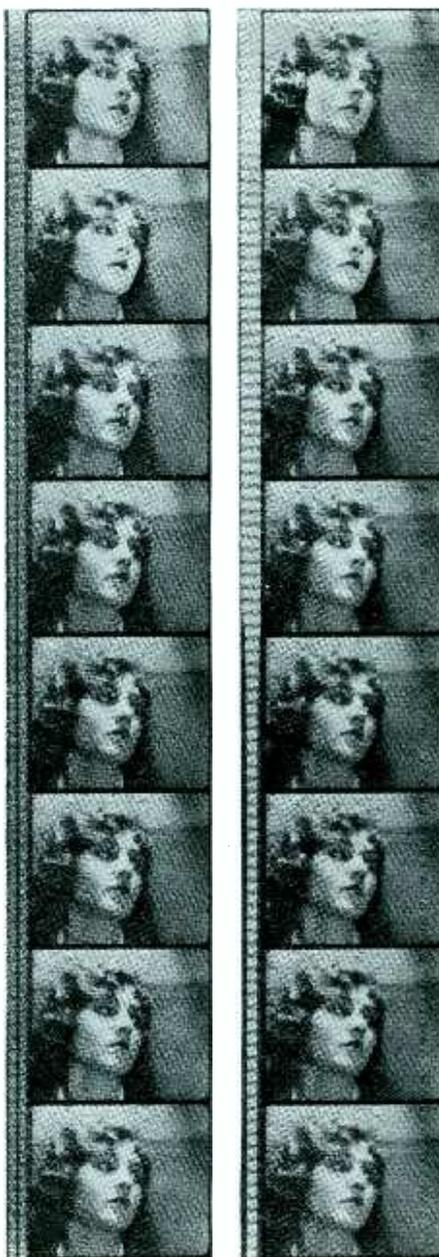
Fig. 1—Left. Single variable density double squeeze, showing transition from full width track to double squeeze track. Fig. 2—Right. Single variable density squeeze, showing change from full to squeeze track
