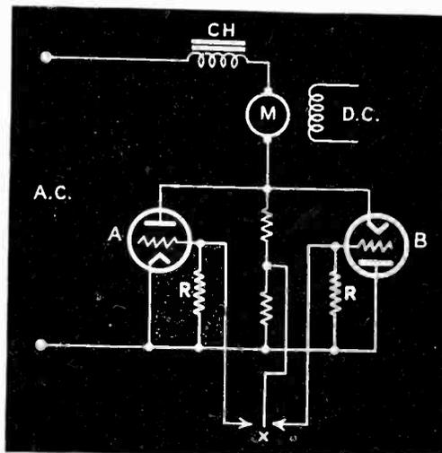
Fig. 1—Circuit for obtaining reversal and speed control of motors from thyatron tubes
