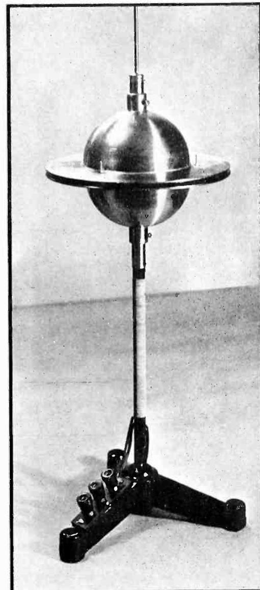
of single tube transmitters. The larger transmitter is equipped with an RCA 834 and has a power output of about 25 watts at 1.5 meters. The smaller spherical tank oscillator is excited by an acorn tube (RCA 955) in the region of 75-85 cms. An extension of the grid side of the central tube provides an antenna.
