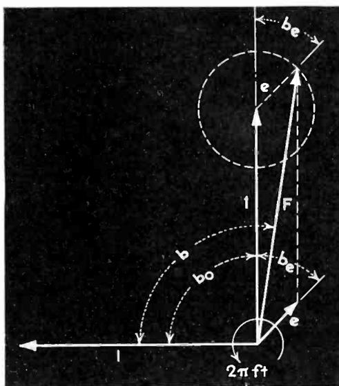
Vector addition of main signal (one) and echo (e) to show effects of amplitude and phase distortion (Wheeler)
