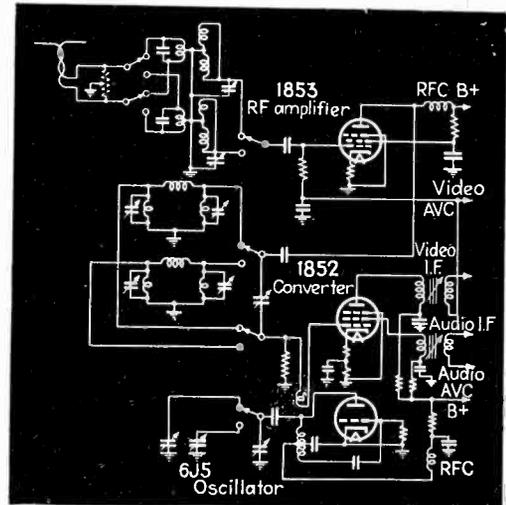
Two channels of the 7-channel television r-f switching system (Lyman)
