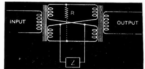
Fig. 3—Adaptation of circuit for distortion measurement
