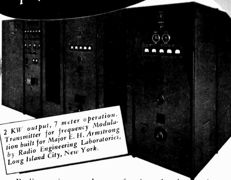
2 KW output, 7 meter operation. Transmitter for frequency Modulation built for Major E. H. Armstrong by Radio Engineering Laboratories, Long Island City, New York.
