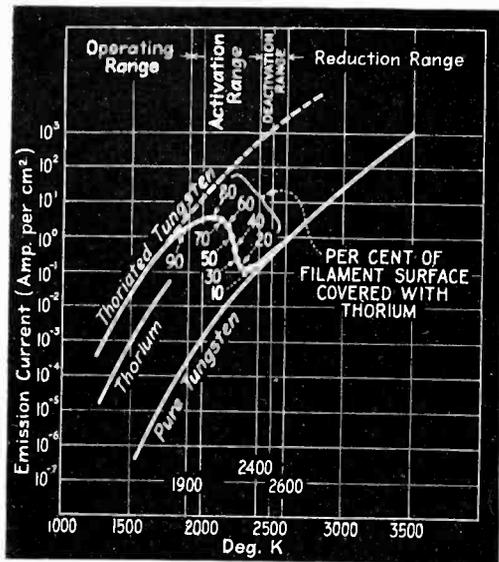
Fig. 1—Graphical plot showing relation between temperature and emission of a thoriated tungsten filament, together with the percentage of surface covered by thorium
