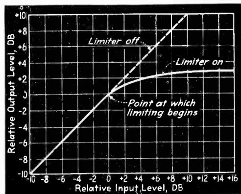
Fig. 2—Input-output characteristics of limiter circuit
