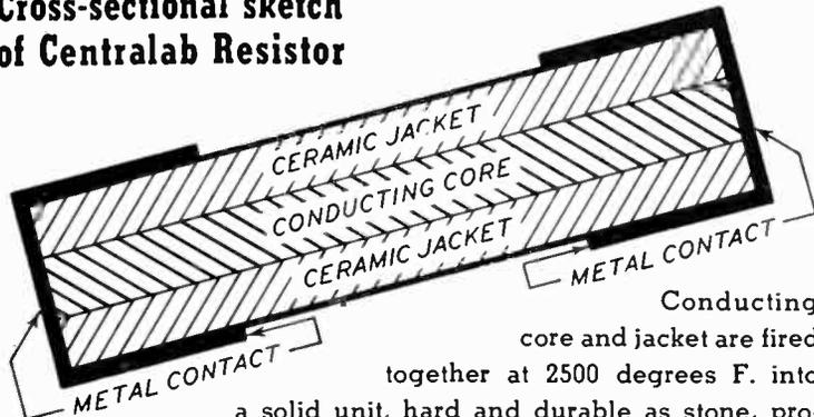
Conducting core and jacket are fired together at 2500 degrees F. into a solid unit, hard and durable as stone, providing mechanical strength and protection against humidity. Copper contact to the resistance material at the extreme ends only provides uniform resistance and load distribution over ENTIRE length. End contacts do not short circuit part of the resistance as in other types.
