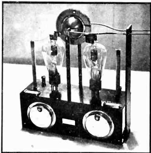
Fig. 8—Push-pull oscillator using RCA 834 tubes
