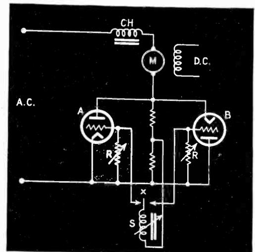
Fig. 2—Motor reversal and speed control of d-c motors are possible with this circuit
