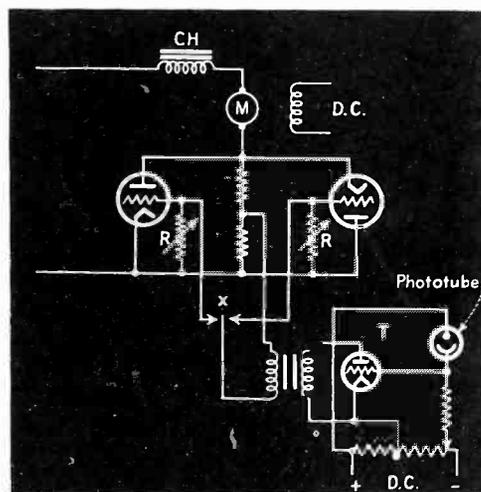
Fig. 4—Use of phototube to control value of inductance for speed control using circuit of Fig. 2
