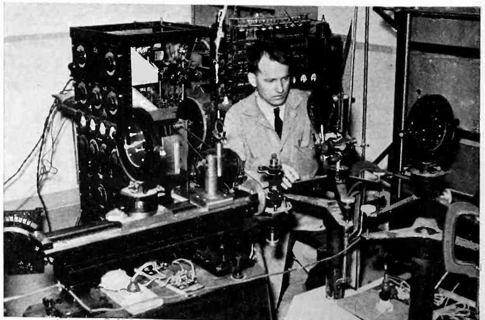
A new method of measuring the speed of light, which is completely automatic, has been devised by W. C. Anderson of Harvard, shown here with his apparatus. The limit of accuracy at present is two and one-half miles per second
