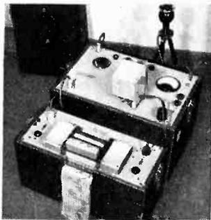
The RA-281 Recording Frequency Analyzer is the first complete, practical acoustic testing equipment for the development laboratory, providing for overall noise measurements and continuous analysis, either by meter indication or automatically recorded graphic record.
