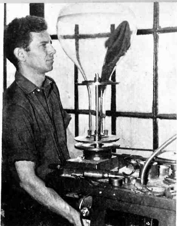
These pictures, taken at the Allen B. Du-Mont Laboratories, Passaic, N. J., show steps in cathode-ray tube manufacture. First, the fluorescent screen is applied and then trimmed on a vertical lathe as shown above. The colloidal graphite shield is then applied and the mount assembly is inserted and sealed in place
