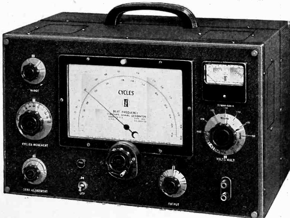
The CR-6 has two logarithmic frequency ranges 10-20,000 cps and 10-50,000 cps. Max. output 5 watts. Level constant  $\pm 0.5$  db over 20 KC range.
