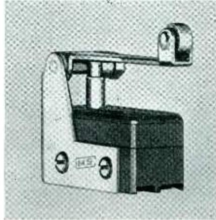
which rests on the plunger of the switch. A case hardened roller is mounted on the end of the lever arm. An 0.008 inch movement at the end of the lever arm moves the switch plunger 0.001 inch and a pressure of 2 ounces at the end of the arm will exert a pressure of 16 ounces at the actuator point. Minor adjustments can be made by slightly bending the lever arm.
