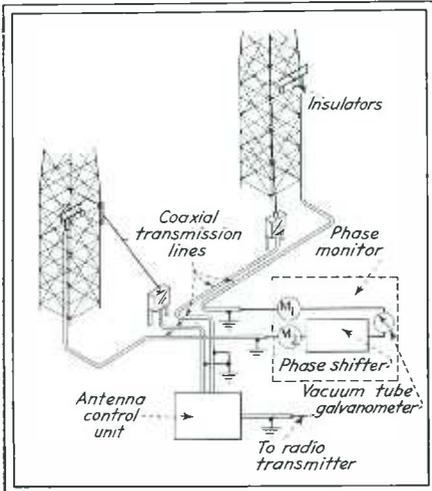
Block diagram of method of directly measuring antenna currents by means of a phase monitor
