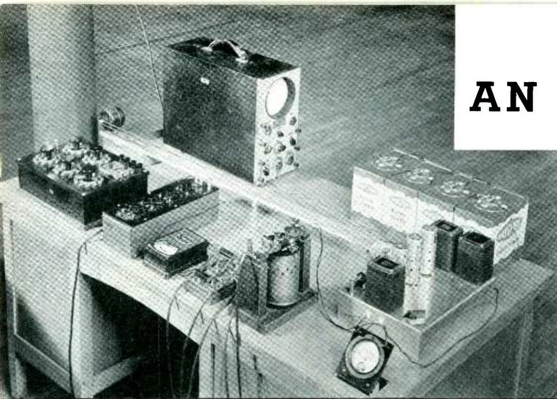
The experimental model with which it is possible to estimate the value of a resistance to six significant figures
