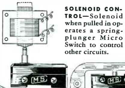
**SOLENOID CONTROL**—Solenoid when pulled in operates a spring-plunger Micro Switch to control other circuits.
