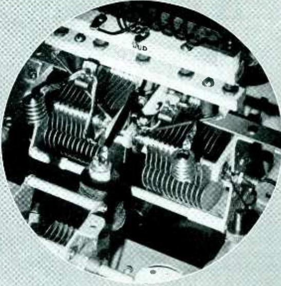
Here is a BUD Junior Transmitting Condenser (No. JC-1569) as installed in a special amplifier designed to operate from 2 to 32 megacycles. This particular unit was selected because it has the valuable Maximum-to-Minimum Capacity ratio of OVER 22-to-1 in addition to many other outstanding BUD features including Center-of-Rod Rotor Contact, Ceramic Insulated Tie Rods, Fitted Cone Bearings, Alsimag 196 Stator Insulation, and many others.
