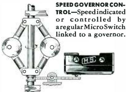
**SPEED GOVERNOR CONTROL**—Speed indicated or controlled by a regular Micro Switch linked to a governor.
