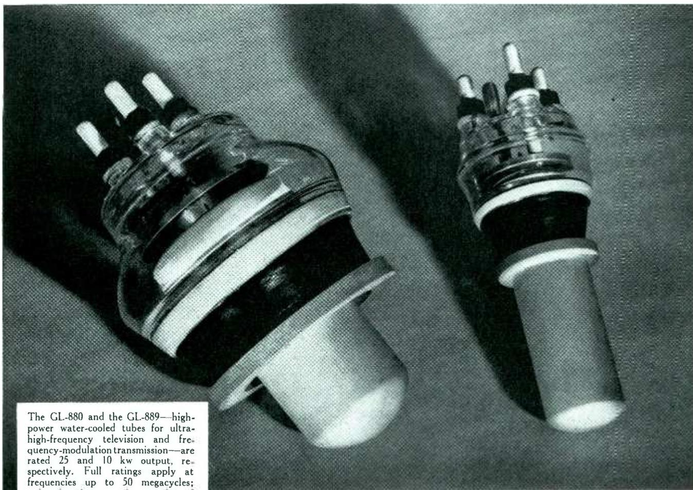
The GL-880 and the GL-889—high-power water-cooled tubes for ultra-high-frequency television and frequency-modulation transmission—are rated 25 and 10 kw output, respectively. Full ratings apply at frequencies up to 50 megacycles; reduced ratings permit operation of these tubes at well over 100 megacycles.
