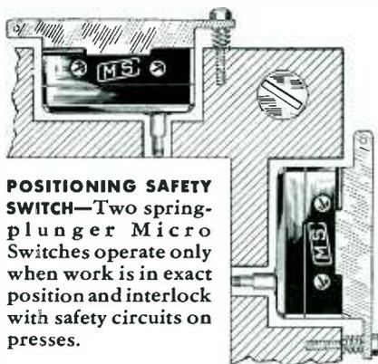
**POSITIONING SAFETY SWITCH**—Two spring-plunger Micro Switches operate only when work is in exact position and interlock with safety circuits on presses.
