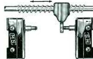
**SCREW LIMIT**—Screw operated carriage at each end of travel actuates a spring-plunger Micro Switch which reverses or stops motor drive.
