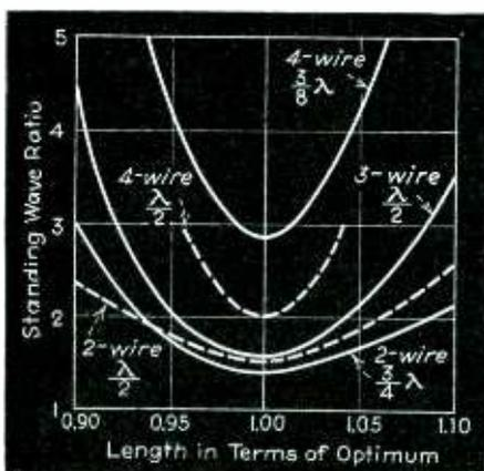
Fig. 3—The length of the antenna becomes more critical as the number of wires is increased. Also, the standing wave ratio increases
