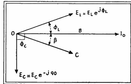
Fig. 2—Vector diagram of circuit in Fig. 1
