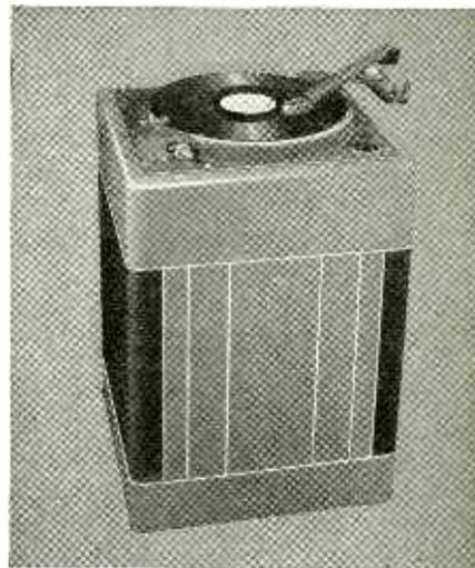
Here is a turntable designed for practical operating conditions in broadcasting stations where from two to five different makes of recordings are used daily. In place of the ordinary tone controls this Presto turntable is equipped with a compensating network accurately calibrated to reproduce the full range of NBC-ORTHACOUSTIC, WORLD, A.M.P. and R.C.A. transcriptions, COLUMBIA, DECCA and R.C.A.-VICTOR phonograph records.
