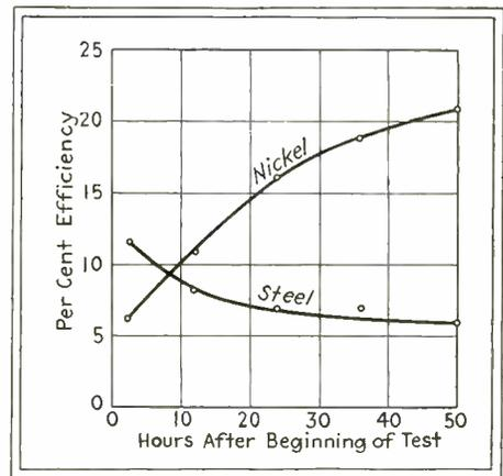
Comparison of nickel and steel condenser surfaces over a short period
