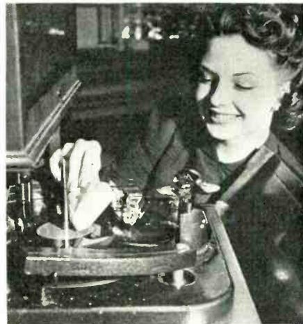
Replacing the old-time phonograph needle in this radio-phonograph combination is a photocell which is used to obtain greater fidelity of reproduction. A rounded jewel, which replaces the phonograph needle, has a tiny mirror mounted on it and this mirror reflects light from a lamp into the photocell. The vibrations of the mirror and jewel are converted into a pulsating light beam and thence into a varying current
