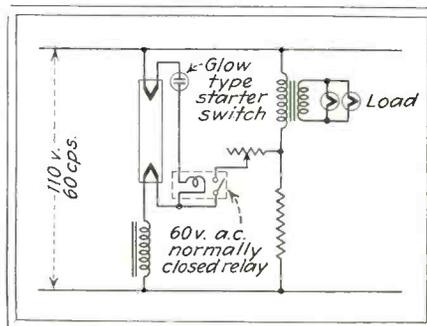
Fig. 2—Circuit using a relay for automatic starting
