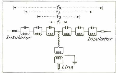
Fig. 2 — Tuned antenna system applied to several frequencies
