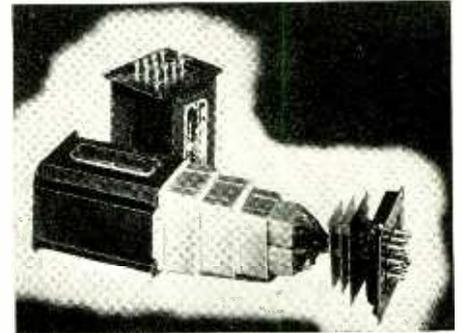
minus 1 db 30 to 20,000 cps. Shielding, 90 db. Type P205 has a primary the same as P204 and a secondary of 100,000 ohms to P.P. grids. Frequency response is  $\pm 1$  db 30 to 20,000 cps. Shielding, 90 db. Transformers in this group are annealed after complete construction to remove all bending and shearing strains brought about during manufacture.
