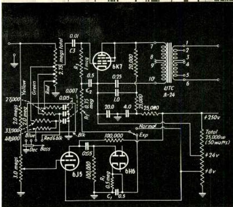
Fig. 1—Circuit diagram of the expander using a type 6K7 tube connected as a triode. The operate time is 0.385 second and the release time is 0.635 second
