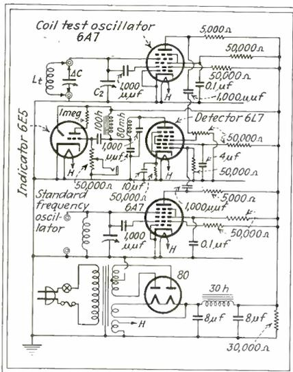
Circuit diagram of instrument for measuring inductance at radio frequencies
