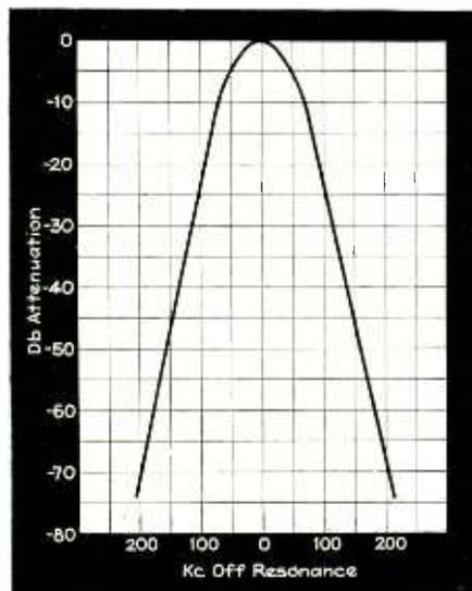
Fig. 5—Overall selectivity characteristic measured below input required for limiter action
