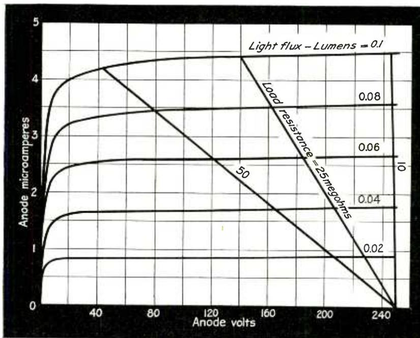
Fig. 3—Anode current characteristic for various values of light flux. Note that the anode current is independent of anode voltage over a wide range
