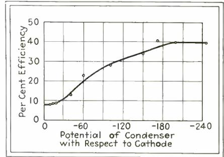
Curve showing effect of maintaining mercury condenser at a negative potential
