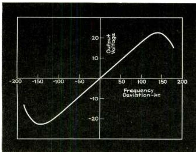
Fig. 7 — Frequency detector (discriminator) characteristic designed for 75 kc deviation each side of the central frequency
