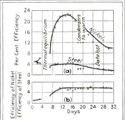
Comparison of nickel and steel condensers over a testing period of 32 days
