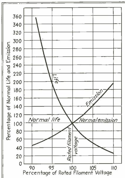
Curves showing effect of filament voltage on life and emission of tubes
