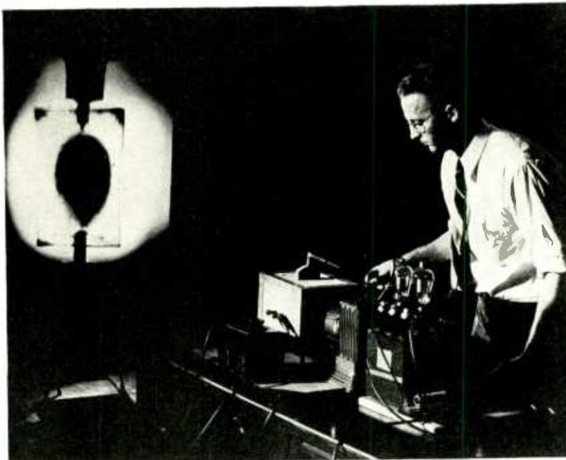
Dr. L. J. Berberich, Westinghouse research engineer, projects an image of electrons entering a salt crystal. The heart-shaped cloud effect is formed by electrons entering the crystal which has been heated to a temperature of 1200° F. The electrons reveal their presence as a reddish mass, as their vibrations absorb all but the red and violet colors of white light passed through the crystal
