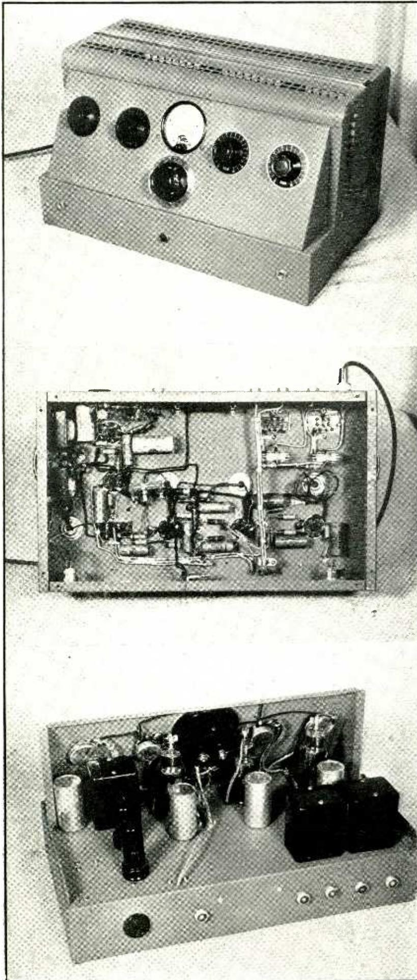
**A** MOST necessary part of all television pick up equipment is the sound equipment. In the signal generator here described the output amplifier and power supply are included in the bottom chassis in the right hand cabinet. The output amplifier employs four 6L6 tubes in push-pull parallel fed by a phase inverter tube on the same chassis.
