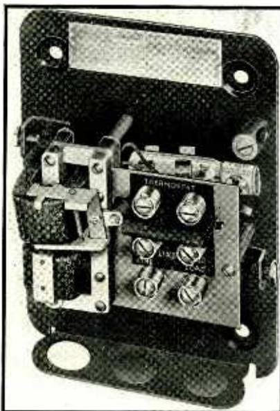
The transformer relay, which avoids the armature and pole-face construction by employing the repulsion between two transformer coils to actuate the mercury contact tube
