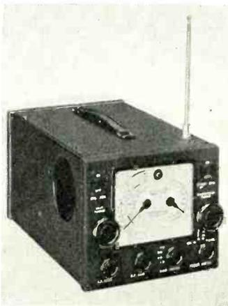
tubes which provide one r-f and two i-f stages, mixer, detector and avc, two audio stages, beat oscillator, automatic noise limiter, and line rectifier. The tuning range is continuous from 542 kc, to 30.5 Mc in four steps and electrical band-spreading is provided for all parts of this range. Sensitivity averages better than 2 microvolts in all ranges. Operation is from any 110 volt a-c or d-c line or from batteries. It is available from Hall-crafter's Inc., 2611 S. Indiana Ave., Chicago.
