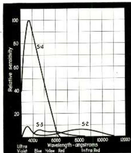
Fig. 1—The new photosurface S-4 compared with previously available surfaces S-2 and S-3
