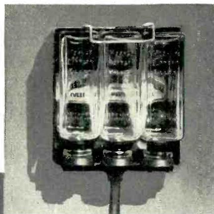
Photograph shows "Lucite" parts. Dis-tilled water flows from the reservoirs through the multiple-hole rubber tubing to the six-prong "Lucite" connector, and then to each of the three "Lucite" hydraulic control plugs which connect directly with the battery cells.
