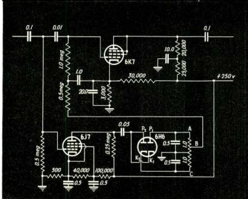
Fig. 3—Diagram of circuit used for both expansion and compression. Potentiometer is connected to both diodes of a 6H6 tube, which rectifies both positive and negative portions of the control signal
