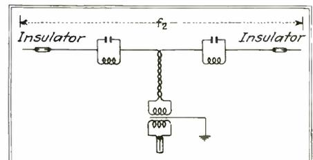
Fig. 1—Basic tuned antenna system devised by Mr. Morgan
