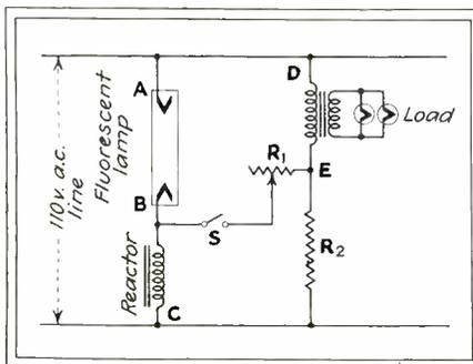
Fig. 1—Simple voltage stabilizer using a fluorescent lamp
