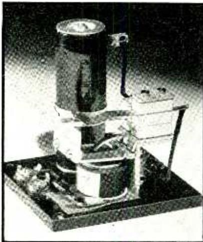
Specially designed to discharge filter condensers in transmitting equipment power supplies, this relay uses ceramic insulation
