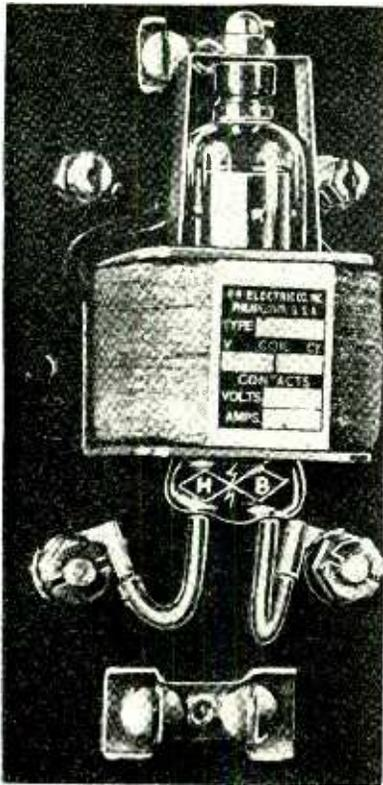
The plunger type of mercury contact relay may be operated at angles as great as 45° from the vertical
