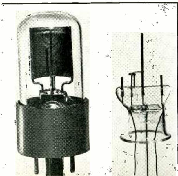
The material used in the cathode surface of a new phototube is highly sensitive in the ultra-violet region and has negligible response in the red and infrared regions. The new cathode is ten times as sensitive to daylight as the best previously available surfaces
