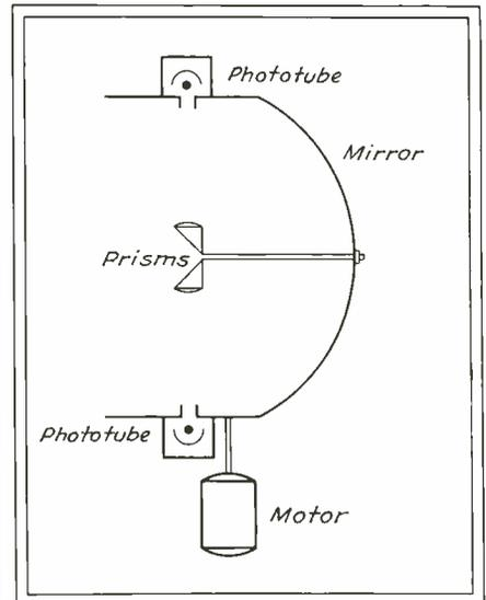
Alternative system for use with reflector telescope
