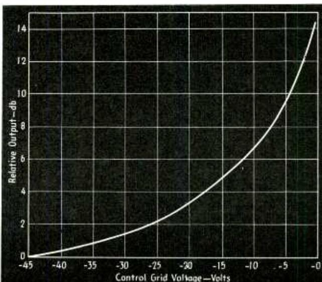
Fig. 2 — Relative output of triode-connected 6K7 ( $G_2$  and  $G_3$  connected to plate) amplifier with  $E_f = 6.3$  v and  $E_p = 250$  v
