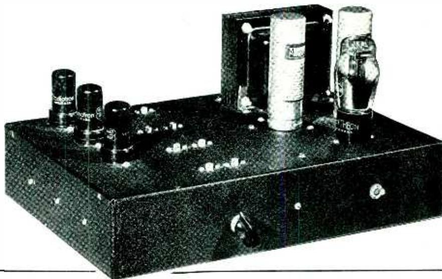
A description of a straightforward three stage r-f "booster" amplifier capable of an overall gain of from 20 to 1000 times, depending on the video signal bandwidth required. Useful in raising the sensitivity of television receivers in areas of low signal strength, or in overcoming transmission line losses
