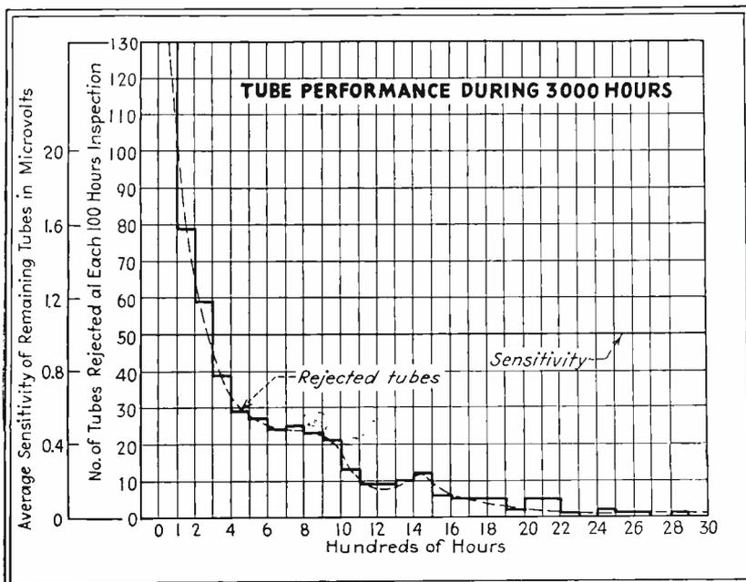
Graph showing the number of tubes rejected after each hour of operation in aircraft receiving equipment. Emission was maintained throughout, as indicated by curve marked sensitivity
