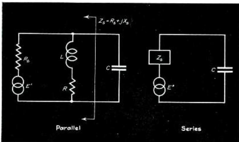
Fig. 3.—Parallel-to-series transformation of a triode amplifier output circuit network
