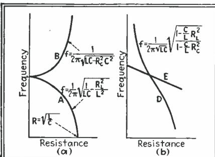
Fig. 2—Frequency of resistance-tuned oscillator. Curve A:  $R_c = 0$ ,  $R_L$  varied from 0 to  $\sqrt{L/C}$ . Curve B:  $R_L = 0$ ,  $R_c$  varied from 0 to  $\sqrt{L/C}$ . Curve D:  $R_L + R_c = k\sqrt{L/C}$ ,  $R_L$  varied from 0 to  $k$ . Curve E:  $R_L + R_c \approx k/2$ ,  $R_L$  varied from 0 to  $k/2$
