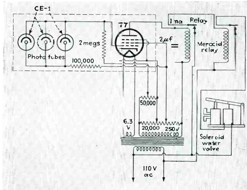
Circuit diagram of the infrared sensitive photoelectric relay. The three phototubes connected in parallel are mounted within a Pyrex glass cylinder. (Below) The ore moves from right to left on the pan conveyor. The water spray (A) is mounted away from the phototubes (B) to permit the ore to reach it before the water flows
