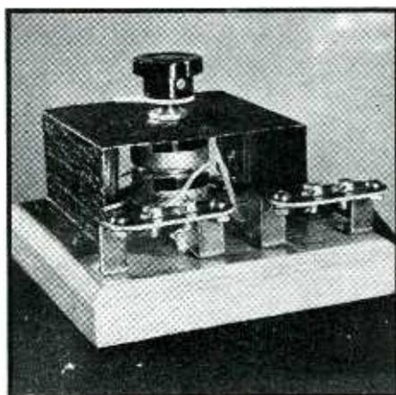
Fig. 4—Laboratory model of the circuit of Fig. 3. At 1000 cps a phase shift of about 174 degrees can be obtained
