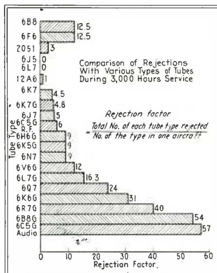
Rejection factor of a variety of tubes used in aircraft equipment. Tubes for audio service gave the most trouble
