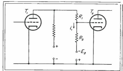
Fig. 11—A possible, but not too convenient solution of coupling two stages of a d-c amplifier, requiring a regulated supply
