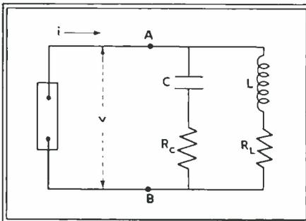
Fig. 1—Circuit of simplified ideal oscillator
