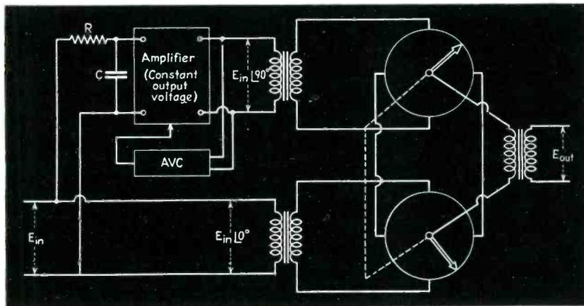
Fig. 10—Circuit of a 360-degree phase shifter which is independent of frequency
