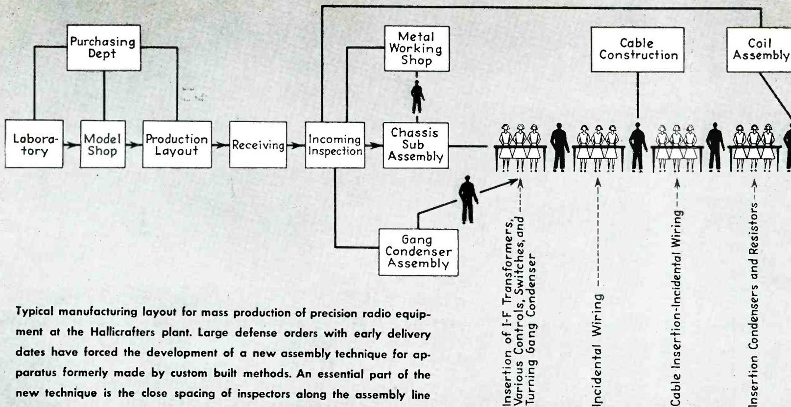
Typical manufacturing layout for mass production of precision radio equipment at the Hallicrafters plant. Large defense orders with early delivery dates have forced the development of a new assembly technique for apparatus formerly made by custom built methods. An essential part of the new technique is the close spacing of inspectors along the assembly line
