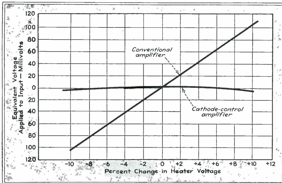
Fig. 5—Manner in which changes in heater voltage affect the equivalent input voltage applied to a conventional amplifier and to the cathode control amplifier described in this article
