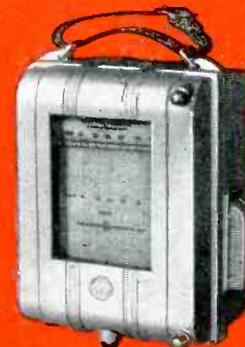
D-c recording milliammeter (Type CF-2)
