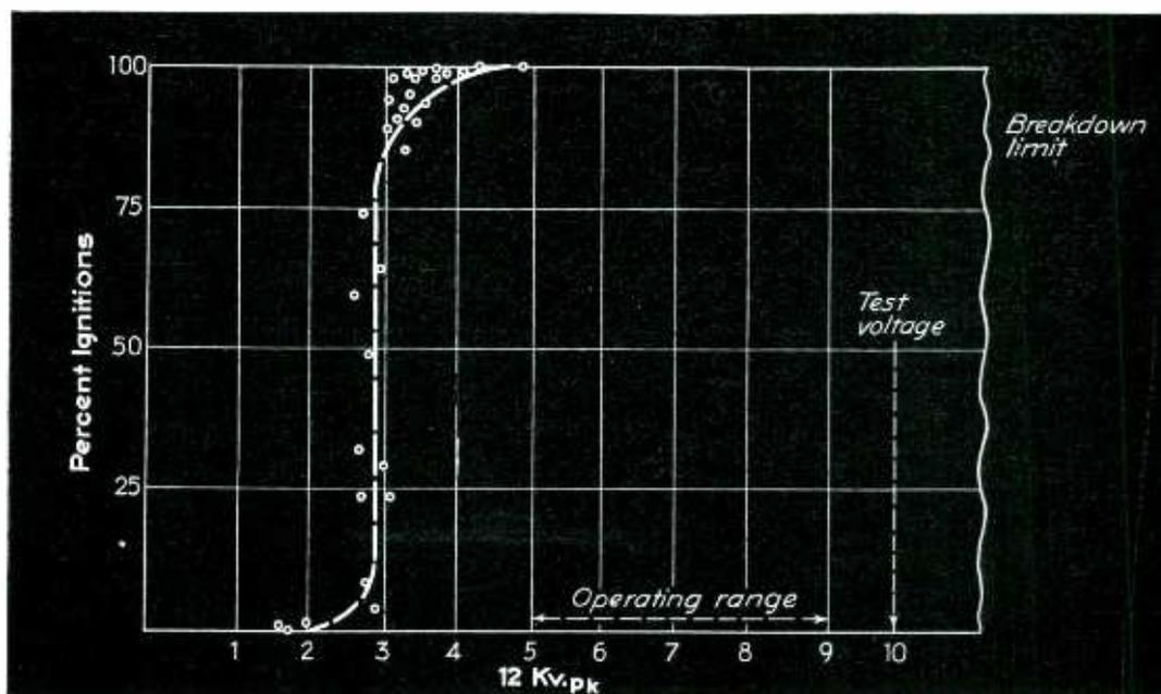
Fig. 3—Ignition characteristics of the dip-in starter electrode. Ignition occurs for voltages above 3,000 or 4,000 volts
