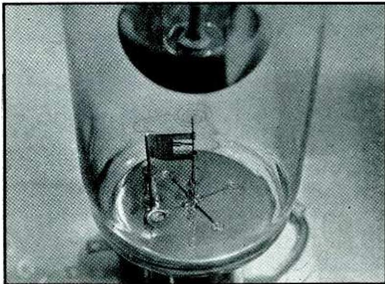
Fig. 4—View of pool cathode with floating starter assembly
