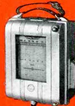
D-c recording milliammeter (Type CF-2)
