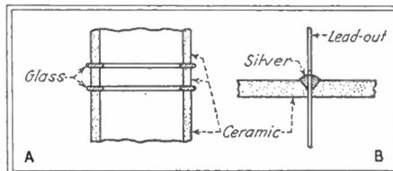
Fig. 2—Illustrations of glass-ceramic and silver-ceramic vacuum tight joints
