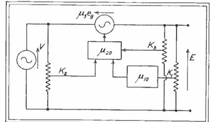
Fig. 10—Block diagram illustrating that the use of a feedback amplifier reduces variations in a regulated power supply
