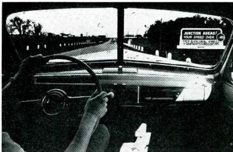
When a car approaches this automatic sign a photoelectric speed measurement circuit informs the driver of his speed
