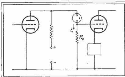
Fig. 12—By replacing the resistor,  $R_1$  of Fig. 11 by a gaseous discharge tube, improved operation of the d-c amplifier is possible using a single voltage supply
