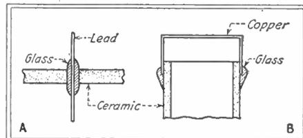
Fig. 1—Glass is used to seal the joints between a metal wire or cap and the ceramic
