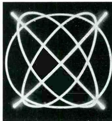
Fig. 13—Composite Lissajous figures showing constant input voltage and changing output voltage of the circuit of Fig. 10
