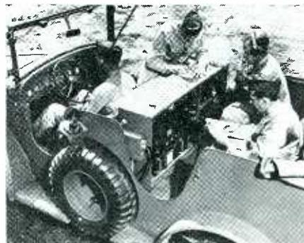
A radio equipped command car at Fort Monmouth, N. J. shown in communication with headquarters. This car has equipment for both key and voice radio communication
