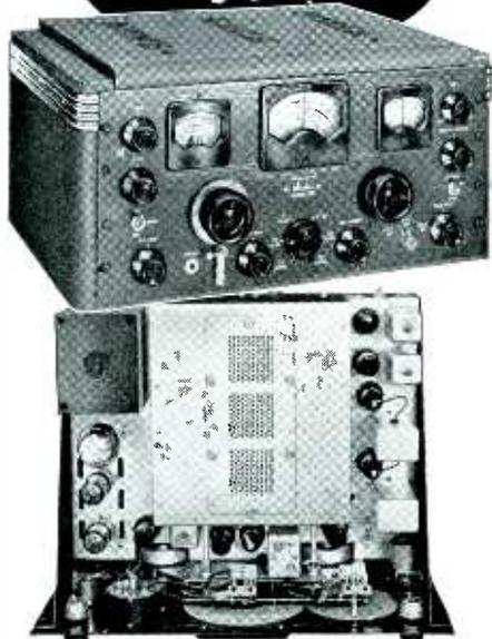
Try a Hallicrafters Super Skyrider, Model SX-28 and know the difference! — in operation, performance and stability. This 15 tube, 6 band communications receiver delivers dependable results, even under adverse operating conditions. Covers 550kc. to 42mc. The controls are arranged to give effortless tuning.
