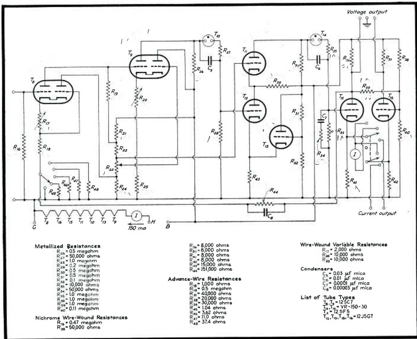
Fig. 1—Schematic wiring diagram of the complete d-c amplifier
