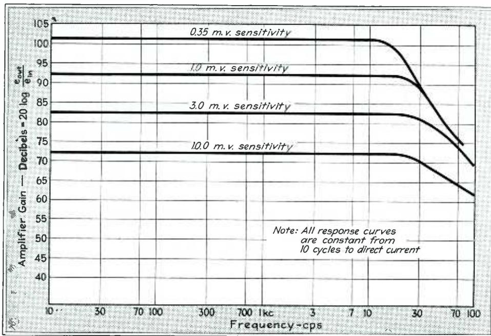
Fig. 3—Frequency response characteristics of the d-c amplifier for various settings of the gain control
