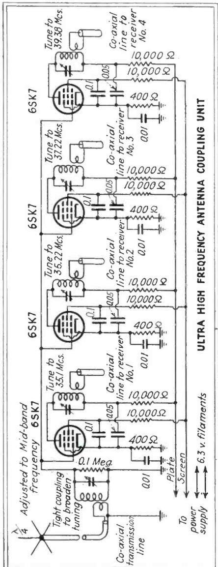
Circuit diagram of antenna coupling unit
