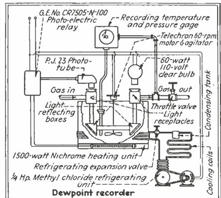
Diagram illustrating the equipment in which the photoelectric dew-point recorder is used
