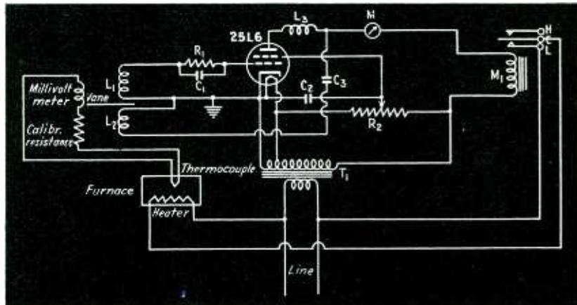
Schematic wiring diagram of the electronic pyrometer control unit
