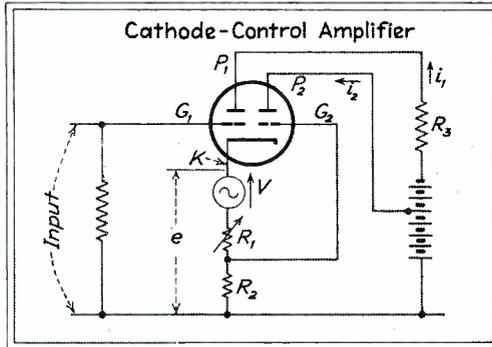
Fig. 7—Fundamental circuit of cathode control amplifier
