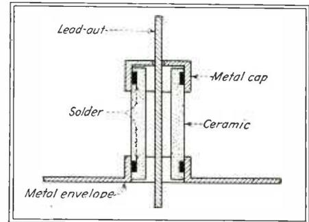
Fig. 4—A metal-ceramic-solder joint made without metallizing the ceramic
