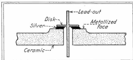
Fig. 3—A silver-ceramic joint making use of a metallized ceramic surface
