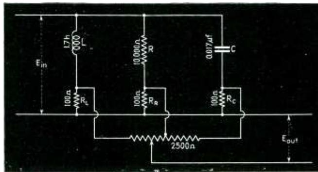
Fig. 7 — Three-arm phase shifter in which the input and output have common leads. The output voltage is about one percent of the input voltage
