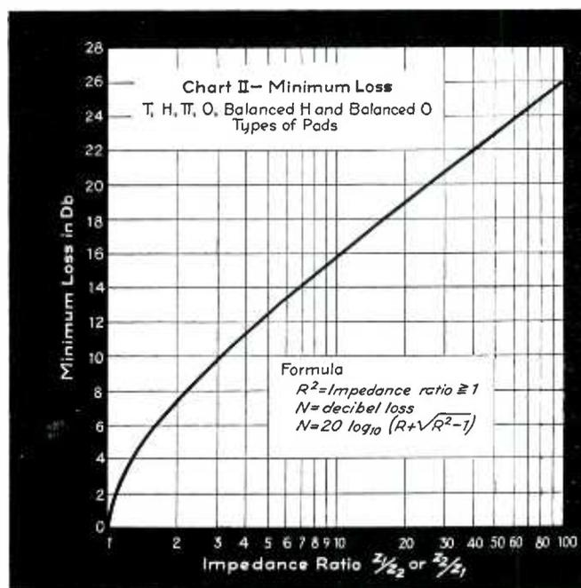
The minimum loss of any pad inserted in a circuit is given in decibels for impedance ratios,  $Z_1/Z_2$ , of from 1 to 100. The range may be extended for values of from  $Z_1/Z_2 = 0.01$  to  $Z_1/Z_2 = 1.0$  by forming the ratio  $Z_2/Z_1$  which will be greater than unity
