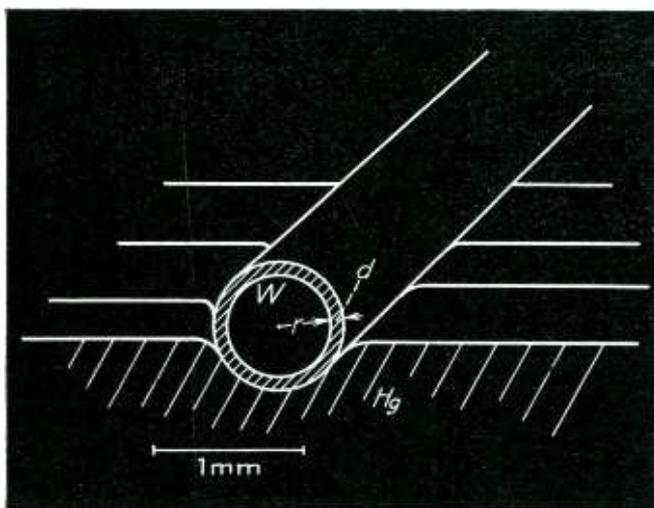
Fig. 1—Cross section of igniter element in mercury pool, showing the meniscus which is formed at the edge of the starter electrode
