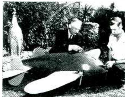
A strange looking radio controlled aerial weapon developed by a Mare Island Navy Yard engineer has aroused the interest of Army officials at Vallejo, Calif. The winged torpedo shown above operates on the principle of the gyroscope and is designed to fly at an altitude of 30,000 feet, carrying a load of bombs. John Hodgdon, the inventor, is shown at the left, with Bob Polson, who built the working model shown
