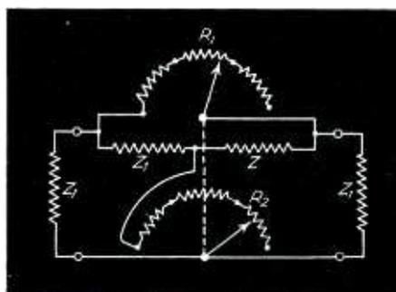
Simple voltage dividing network having given input impedance and specified loss. design data for which is worked out as Problem I
