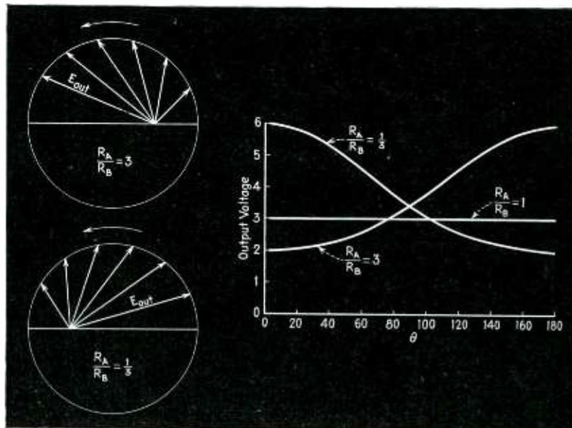
Fig. 2—Diagrams showing how the circuit of Fig. 1 can be made to produce varying output voltages for varying phase angles
