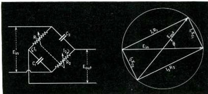
Fig. 3—Double-reactance bridge phase shifter and its vector diagram. Note that the output voltage is equal to the input voltage
