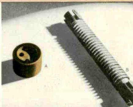
A — Connector plug — sawed, turned, and drilled.
