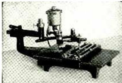
For lettering panels of steel, aluminum, brass, or bakelite, or for marking finished apparatus.
