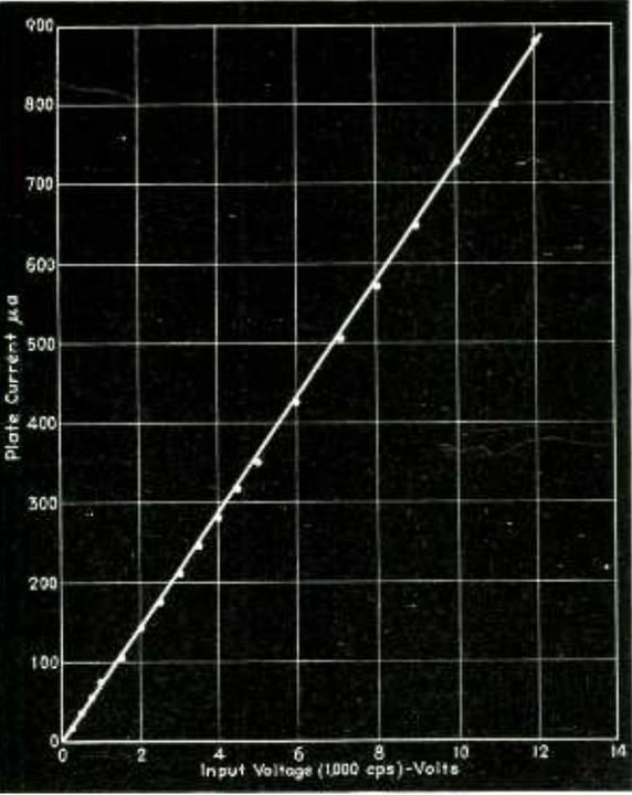
Fig. 4—Input-output characteristics of the combined circuits of Fig. 2 and Fig. 3, illustrating that a linear relationship is accurately attained
