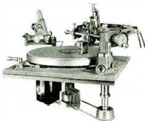
**VARIABLE CUTTING PITCH:** The buttress thread feed screw is driven by a belt and two step pulleys beneath the table giving accurate cutting pitch adjustments of 96, 112, 120, 128 or 136 lines an inch. Changing the cutting pitch is a matter of seconds. A hand crank and ratchet on the feed screw spirals starting and runout grooves up to 1/4" apart.
