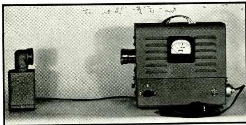
Fig. 3—Completed photoflash synchronizer tester, with light source at left
