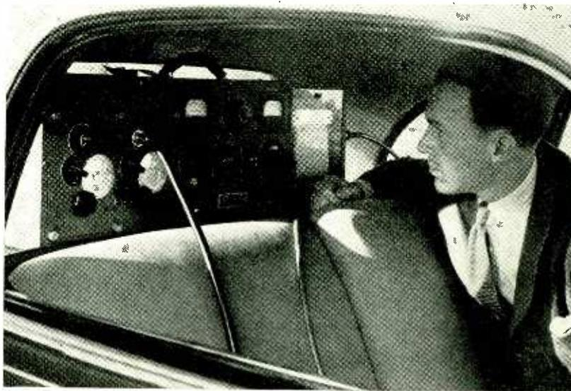
Fig. 1—The field intensity recorder is shown installed in an automobile. The recording mechanism is at the far right
