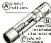
are especially designed to protect small motors, magnets, solenoids, and other equipment having high inductive and capacitive surges. Also the dependable fuse for intermittent duty circuits, vibrators, control circuits, etc., where frequent cycles would soon crystallize or break a simple fuse element. Slo-Blo blows but holds awhile.
