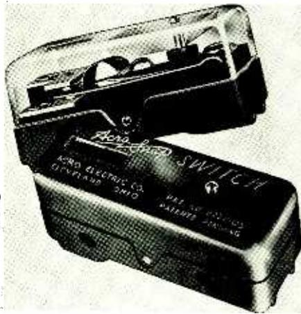
The unique design of the ACROSNAP SWITCH with its rolling spring to snap the blade from one position to the other permits actuation with a very slight flexure of the blade.
