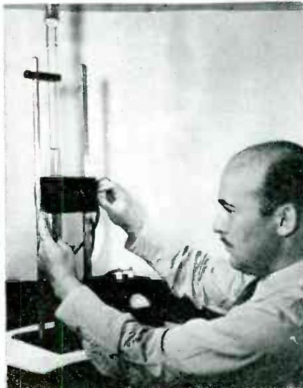
Dr. A. A. Bates of Westinghouse demonstrates P. R. Kalischer's device that quickly determines grain size of metallic powders having particles as small as 1/25,000 inch. Mixed with a liquid in a long glass tube, the particles intercept a light beam directed into a phototube as they settle. The rate at which the solution clears up, indicated by anode current change through a milliammeter, gives comparative data
