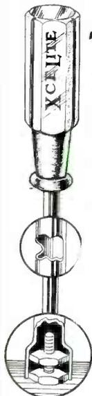
• One of the handiest tools ever designed for electrical and radio work—especially panel assembly jobs. The nut is readily tightened or loosened without damage to the panel. On telephone or power switchboard, the hollow shaft readily slips over the long protruding bolts or studs and the socket firmly engages the nut. Shock-proof handle; precision machined shafts and sockets. Five sizes, from 5/16" to 5/8" (nut sizes). Full details on request.
