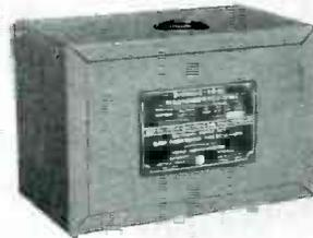
Power Supply using rechargeable non-spill storage battery for operation of "Walkie-talkie" radio equipment. Input Voltage, 4 Volts; Output, Numerous voltages supplying filament and plate requirements of equipment. Width, 3 1/2"; Length, 6 1/2"; Height, 4 3/4".
