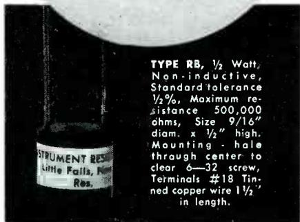
**TYPE RB**, 1/2 Watt, Non-inductive, Standard tolerance 1/2%, Maximum resistance 500,000 ohms, Size 9/16" diam. x 1/2" high. Mounting - hole through center to clear 6-32 screw. Terminals #18 Tinned copper wire 1/2" in length.
