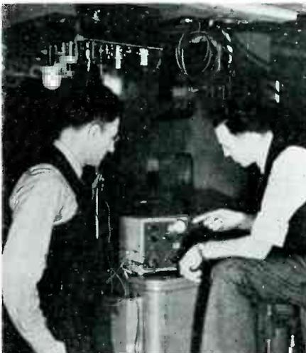
A G-E photoelectric color register control installed on a press in the plant of New York's Neo Gravure Printing Company is checked for synchronization by means of a cathode-ray oscilloscope
