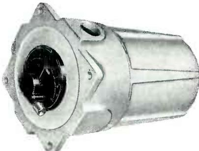
The illustration shows a Type TD1C explosion-proof time delay relay which is laid out for panel board mounting with the setting knob and dial projecting. Within this housing it is possible to mount either Type TD1C or TD1 with a small relay. The latter construction would be used where it is desired to control the timer from remote located momentary start button.
