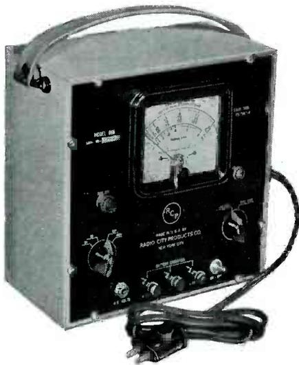
operation through appropriate terminal connections and a throw-over supply switch. Readings are made quickly and easily. The instrument is equipped with a  $4\frac{1}{2}$ -inch rectangular meter having a movement of 0-200 microamps. Ranges are 0-3-6-30-150 volts. Tubes used are type 6K6GT, 6X5GT, 6H6 and VR105-30. The latter is a voltage regulator, eliminating errors due to line voltage fluctuations.
