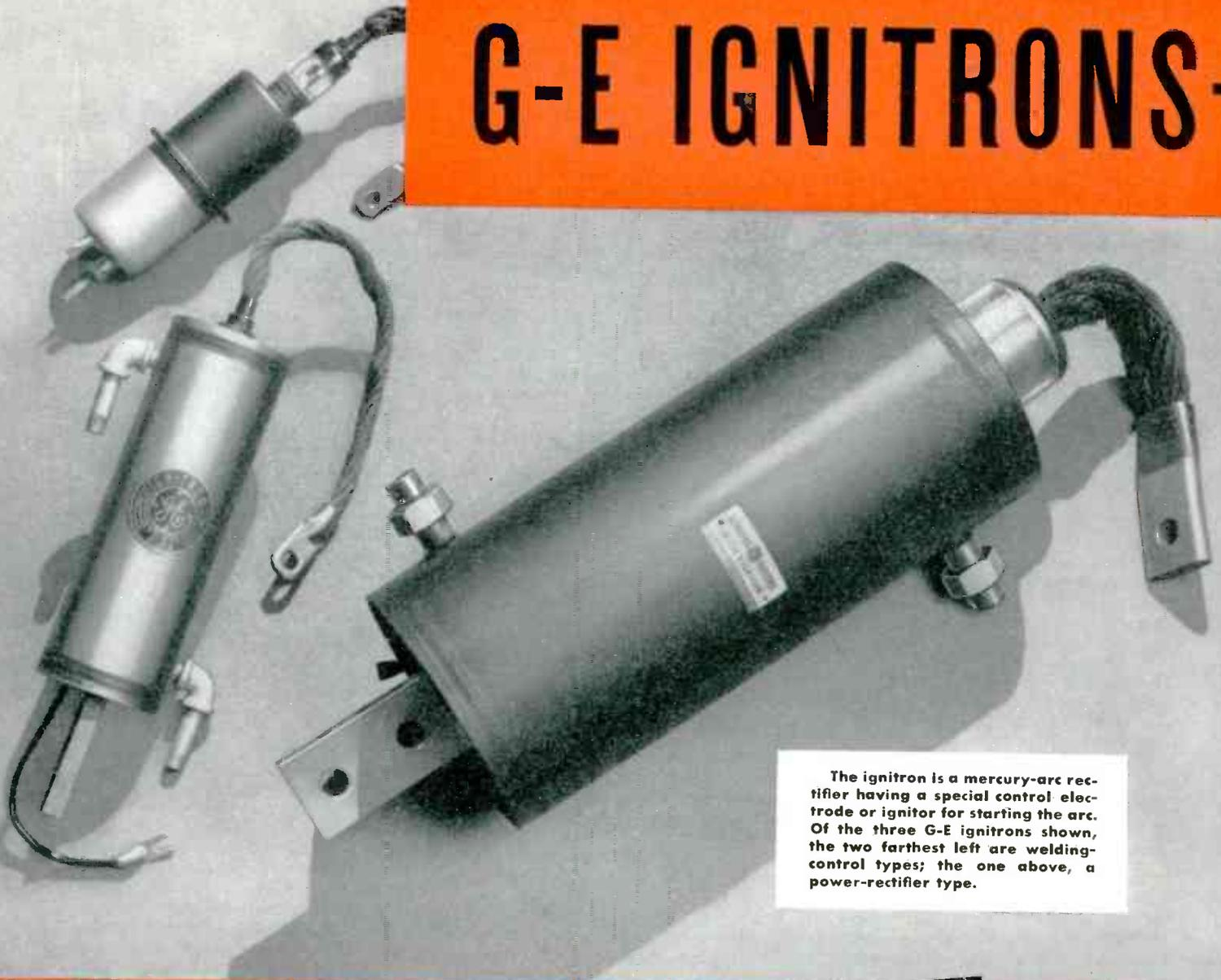
The ignitron is a mercury-arc rectifier having a special control electrode or ignitor for starting the arc. Of the three G-E ignitrons shown, the two farthest left are welding-control types; the one above, a power-rectifier type.
