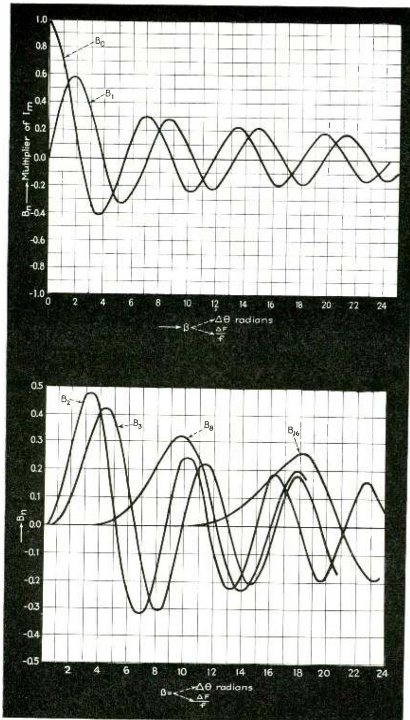
Fig. 5—Curves for the Bessel multiplier,  $B_n$ , plotted against deviation produced by modulating agency. The amplitude of the assigned carrier frequency,  $F$  is  $B_n I_m$ ; of frequency  $F \pm nf$  is  $B_n I_m$ ; where  $f$  is the modulation frequency and  $I_m$  is the amplitude of the carrier
