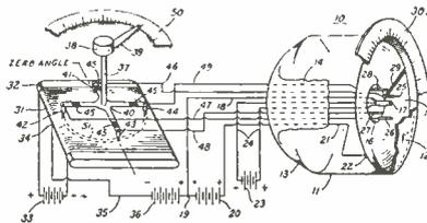
with connections between stator and control electrodes, electrons constrained into beams, and means for indicating on anode position of rotor of transmitter as it moves. A. A. Stuart, Bendix, Dec. 30, 1940. No. 2,283,103.
