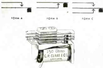
gauge silver, rated 1 amp, 50 watts; or 18 gauge palladium, rated 2 amps, 100 watts, can be furnished. All metal parts of the relay are specially plated to withstand a 200 hour salt spray test, and each relay is given a 1000 volt a-c insulation breakdown test.
