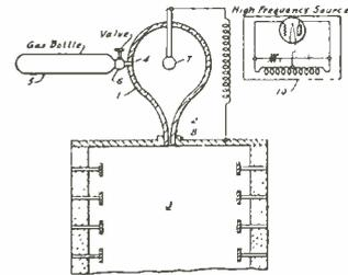
suming device, an electrode in said chamber, an electrode adjacent said outlet and a source of high frequency power connected to said electrodes for producing a high frequency discharge through said outlet. J. Slepian. WE&M Co. June 14, 1940. No. 2,285,622.
