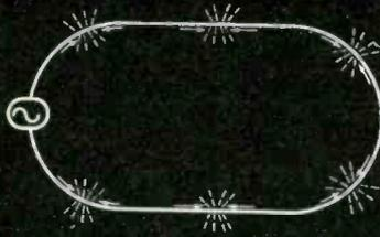
**FIG. 6** (Above center) At high frequencies, charges pile up at points on the conductor because of the finite time it takes the magnetic field to build up. The field may not have time to establish itself all around the circuit before the generated current changes its direction of flow
