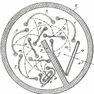
traveling to emissive inner surface, and a collector electrode for secondary electrons supported within enclosed space behind the marginal portions of the plate. J. A. Rajchman, RCA. July 28, 1939. No. 2,285,126. See also No. 2,285,848 to van den Bosch, Vacuum-Science Products, Ltd. on an electron multiplier tube.
