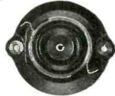
**4. By filing smooth** the corners of the ring inserts before they were inserted in the mold, internal strains were relieved, thus eliminating some of the cracking difficulty. This combination of material "C" with the redesigned metal inserts proved satisfactory mechanically, but the material lacked the required dielectric strength.
