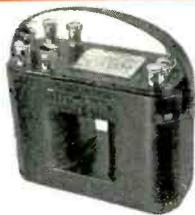
Portable potential and current transformers, of which the PV-130 and the PC-137 are examples, extend the range of measurement on portable a-c instruments.
