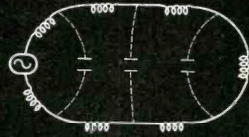
**FIG. 7** (Above) At high frequencies, even a simple circuit may act as though it is made up of many series impedances and shunt admittances
