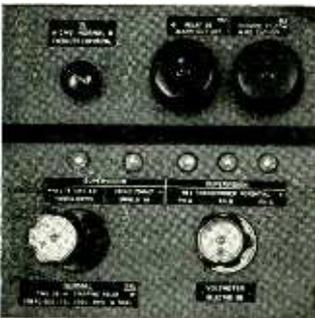
(Above) SWITCHES AND CONTROLS clearly identified with clean-cut lettering and calibrations routed into sheets of Engraving Lamicoid.
