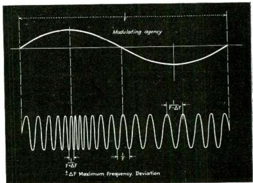
Fig. 4—Frequency modulated current showing extreme modulation conditions of the carrier for a complete modulation cycle. above
