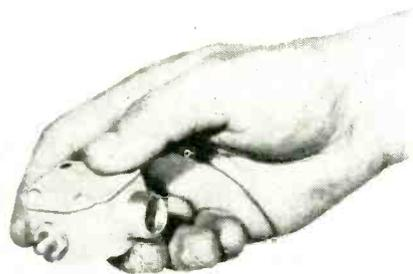
is available in three contact arrangements: single-circuit, normally open or normally closed; and single-pole, double-throw. Each form can be furnished with a contact air gap of 0.010, 0.020, or 0.030 inch. The switch weighs 0.13 lb and meets all U. S. Army Air Force stipulations.
