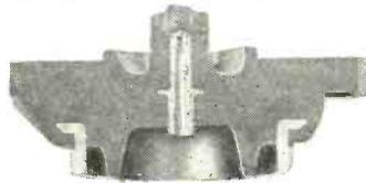
**6. Despite this improvement,** two types of cracks still occurred. One was a radial crack on the face of the ring originating at the small round center insert. Another was located in the recess of the base of the tower. The recommendation that preheating time be increased and that plasticity be changed from flow 100 at 330 lb. per sq. in. to flow 100 at 500 lb. per sq. in. resulted in definite improvement.
