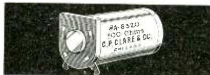
The small coil is equipped with a front spool head having a flat side. This locks the entire coil in place against the heelpiece, preventing it from turning or becoming loose. The screw holding the coil in the heelpiece is equipped with a split type lockwasher. The coil is carefully wound to exact turns on precision machines. Coils can be supplied impregnated
