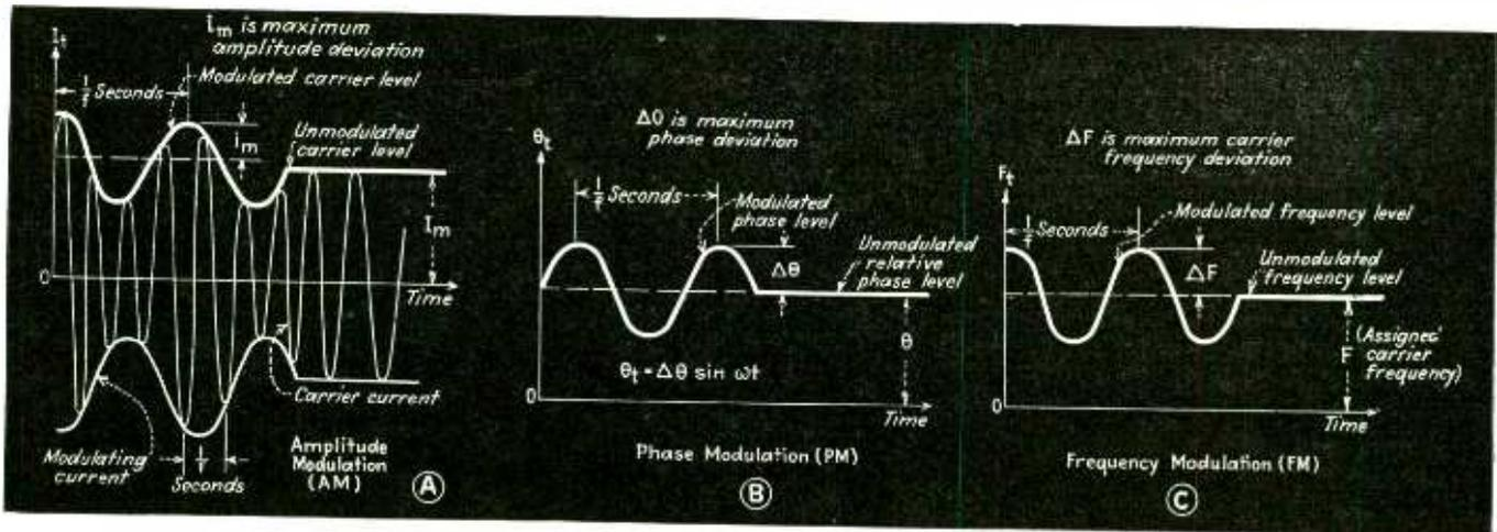
Fig. 1—Graphs illustrating the variations which take place, on a time plot, for amplitude modulation, (A), phase modulation, (B), and frequency modulation, (C). The variable factor is indicated by the ordinate in each case
