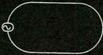
**FIG. 5** (Above) An elemental electrical circuit. At low frequencies it is assumed that flow of current through the wire, and a field about the wire, is established instantaneously—but this is not true at centimeter wave frequencies
