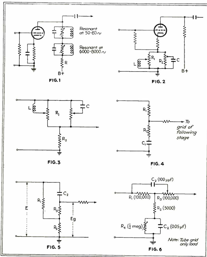
Conventional high and low frequency "boost" circuits are shown in Figs. 1, 2 and 3. Development of an improved circuit is shown in Figs. 4 and 5, with the final version appearing in Fig. 6
