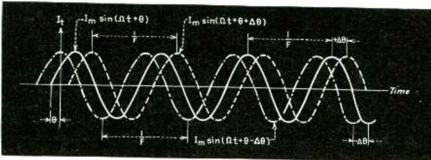
Fig. 3—Unmodulated carrier wave (solid line) with modulated carrier (broken lines) for phase modulation. The frequency of modulated and unmodulated carrier is unchanged. An instantaneous change in frequency occurs (not shown) when carrier is changed from unmodulated to modulated state, or vice versa
