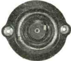
**5. It was thereupon decided** to revert to material "B." However, in order to obtain the necessary mechanical strength, the metal inserts were again redesigned to offer less resistance to the shrinkage of the plastic material. In addition, a circumferential slot was turned in the ring insert to a proper depth which made it possible to machine the part after molding without exposing sharp corners. This corrected all cracking due to machining operations.
