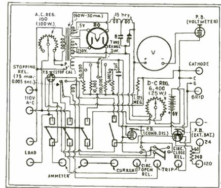
Fig. 1—Tester timing unit
