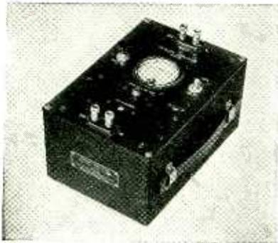
A highly stable amplifier giving gains of exactly 10 and 100 times. Operated by self-contained batteries. Through the use of special circuits the gain is independent of battery voltage, circuit constants and tubes within 2% from 10 to 100,000 cycles. Particularly useful with our Model 300 Electronic Voltmeter to increase its sensitivity, permitting voltage measurements down to 30 microvolts. Send for Bulletin 7.
