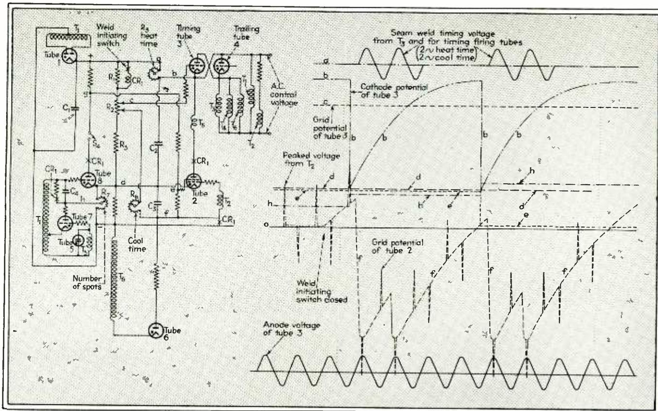
Fig. 1—Schematic circuit diagram and waveforms showing operation of spot, seam and pulsation welding control
