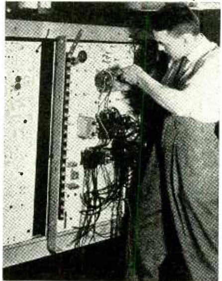
Drilling of holes, mounting of parts, installation and check of wiring on resistance welding panels is facilitated at G-E by pasting templates to the back of the panels before such work starts. Template paper is oil-resistant and all lines are drawn with special non-conducting ink so the templates can be left in place to simplify service later
