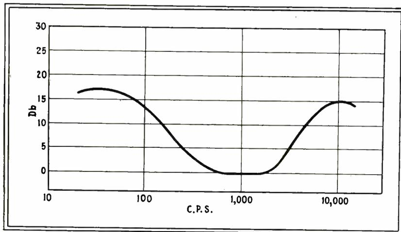
Fig. 7—Characteristics of the improved circuit with controls set for maximum high and low frequency boost
