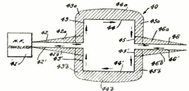
radiant conductor, energy transfer to transmission line at a point such that if energy were supplied thereat current would circulate about periphery in the same sense at all points, whereby radiant action of system is substantially uniform in all directions about periphery and has everywhere a polarization substantially parallel to the plane. A. Alford, IT & R Mfg. Corp. Apr. 26, 1939. No. 2,283,897.
