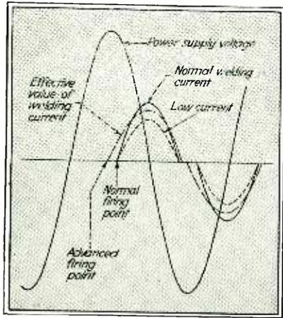
Fig. 4 — Waveform sketch showing basic operating principle of compensating and regulating controls for maintaining constant welding current
