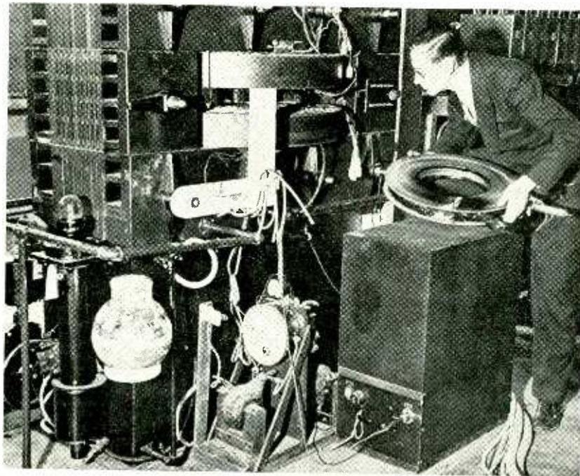
New scientific machine, 20-million volt betatron, that is a super x-ray, atom-smasher and the source of more radium-like radiations. Prof. Kerst, inventor and designer, is shown preparing to place the doughnut vacuum tube between poles of the electro-magnet (left). The vacuum tube whirls electrons to a speed within one-tenth of one percent that of light (186,000 miles per second)
