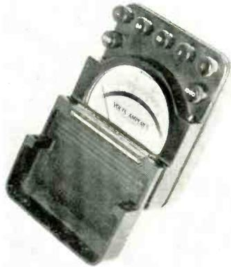
accurate readings. P-14 embodies a variety of single, and multi-ranges providing for the measurement of a-c volts, amps and milliamps; d-c volts, amps, milliamps, and micro-amps. Ranges and combinations of ranges have been chosen to meet the needs of test men, laboratory technicians and research engineers. Combinations of four current and three voltage ranges are available. The molded cases are fully insulated and magnetically shielded from stray field influence.
