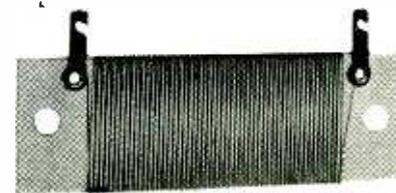
TYPE JN—mica card, standard tolerance 1%, maximum resistance—100,000 ohms, size 1" wide x 3/4" long x 1/16" thick. Mounting by insulated holes to clear 6/32 screw. Terminals: hot tinned copper lug.
