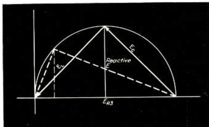
Fig. 2—Vector diagram of feedback voltage. Dotted lines show conditions for too small a value of  $C_s$ .
