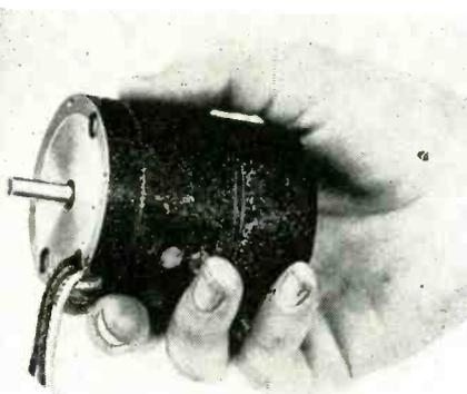
housing is 2.306 ins; overall length, not including the shaft extension, is 2 1/8 ins; it weighs 1 lb and 3 oz; the shaft diameter is 0.250 ins; the shaft extension is 0.766 ins. The motor is equipped with ball bearings and is reversible (3 leads).
