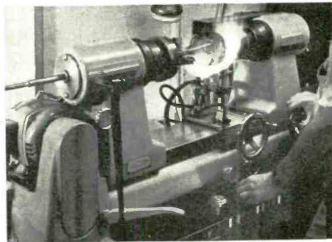
*Glass bulbs are annealed after tube is fully assembled. This operation relieves stress and strain in the glass itself which may have been induced during manufacture.*
