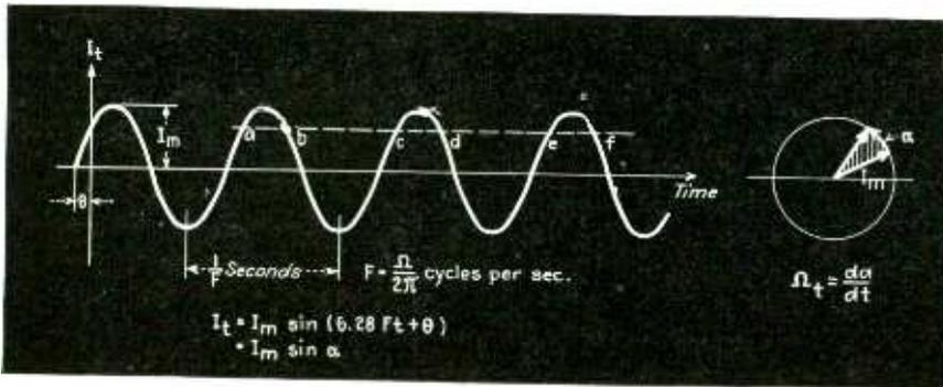
Fig. 2—Wave train of typical carrier current. Since frequency and phase modulation methods are unaffected by changes in amplitude, PM and FM may be separated from AM, by clipping the wave at points such as ab, cd, ef, and so on
