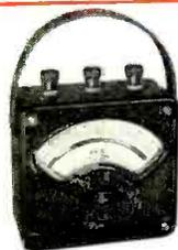
This portable P-4 instrument with ¾% accuracy meets a wide range of requirements. A-c and d-c models available.
