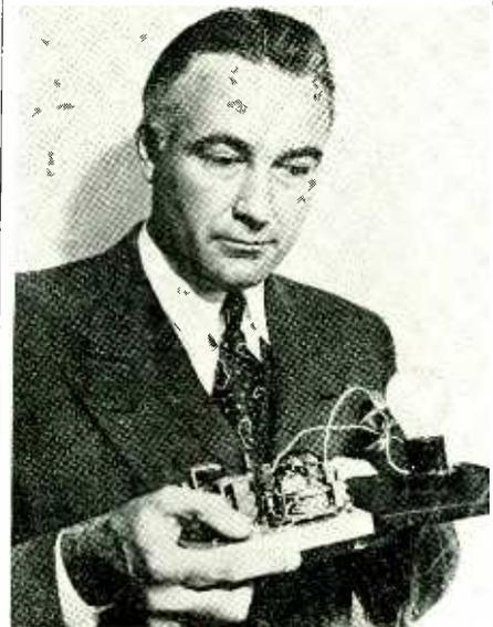
In the event of a blackout this device, invented by William Sprague of Los Angeles, turns out all lights and sounds an alarm. All that is necessary to operate the device is a short interruption of service from the local power company. The momentary interruption starts the device working. The same method will turn the lights back on when the "all clear" signal is given
