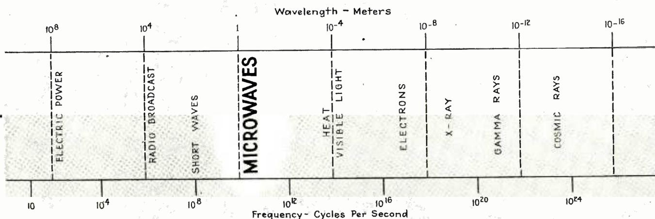
FIG. 1 - The electromagnetic spectrum. The region considered in this article is labeled "microwaves"
