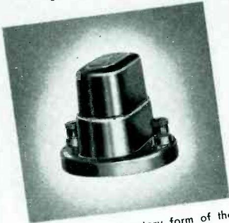
The portable laboratory form of the International Standard, with practically no errors due to temperature changes or hysteresis effects.
