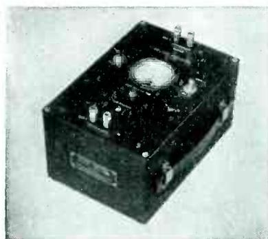
A highly stable amplifier giving gains of exactly 10 and 100 times. Operated by self-contained batteries. Through the use of special circuits the gain is independent of battery voltage, circuit constants and tubes within 2% from 10 to 100,000 cycles. Particularly useful with our Model 300 Electronic Voltmeter to increase its sensitivity, permitting voltage measurements down to 30 microvolts. Send for Bulletin 7.
