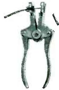
also be used as a wire cutter. All that is necessary to operate the tool is to press the handle.
