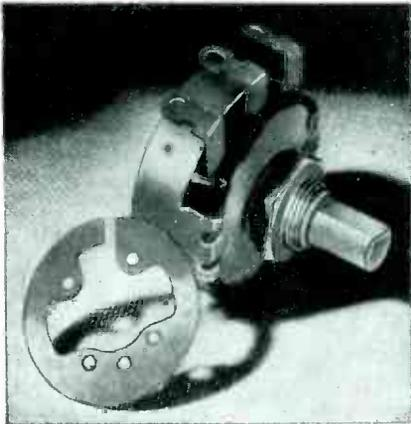
composition, and to stabilize its temperature and humidity characteristics; so that the controls have accurate resistance values even after continuous usage under adverse conditions. Another feature is that the controls may be used in place of wire-wound units for relatively low resistance values.
