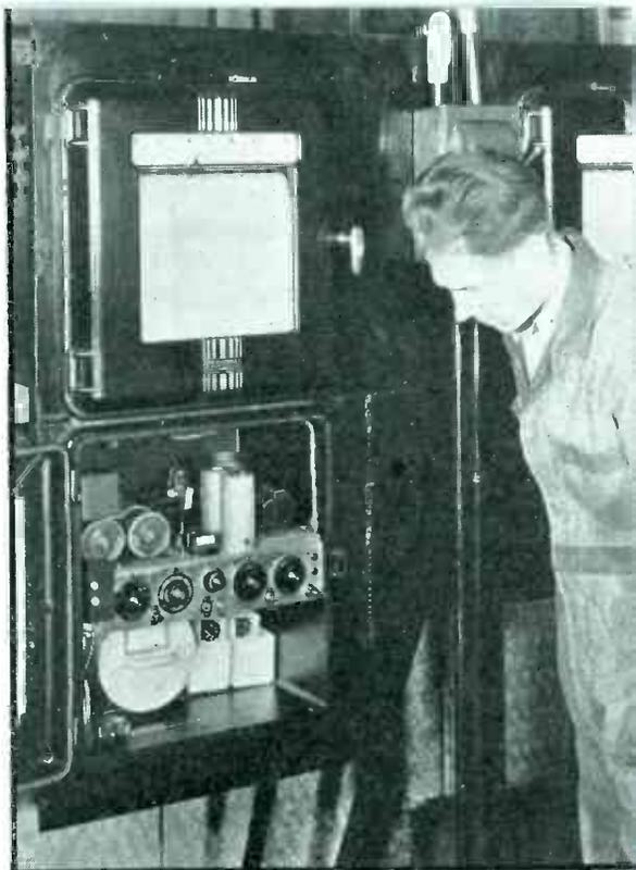
Fig. 9—The Leeds & Northrup Speedomax which converts the potentiometer unbalance voltage to a.c. by means of an a-c driven carbon microphone which is then amplified to drive the balancing motor
