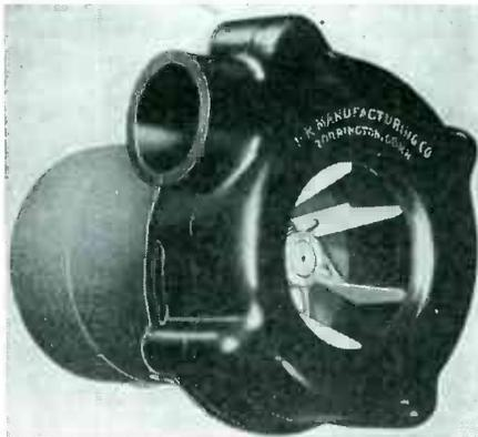
at an angle of 90 deg. Output is rated at 60 cfm at 7500 rpm. The unit has Universal mounting (with motor plate for any small motor) and is assembled with four 10/32 screws which may be used as bracket supports for various methods of mounting.
