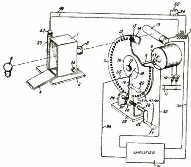
means whereby a record disk may be detachably mounted thereon, means for amplifying the output impulses of said device, a stylus arranged adjacent to said conducting disk, and means for applying said amplified impulses between said conducting disk and said stylus to mark said record disk. W. K. Kearsley, GEC. No. 2,296,676.
