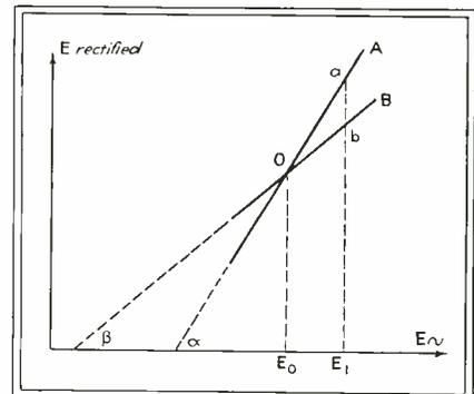
Fig. 2—The voltage output from the regulator is proportional to the difference of slopes of the two rectifiers and to the deviation from standard voltage, and can be used as a corrective means
