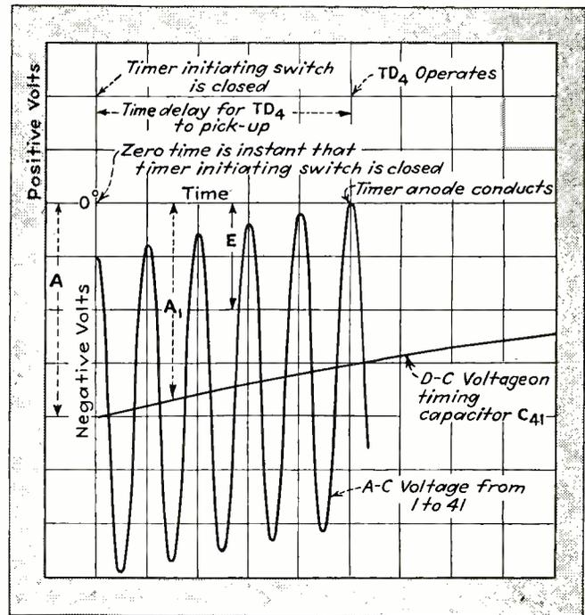
Fig. 4—Grid voltage characteristic of typical timer circuit. When the sum of the d-c voltage and the instantaneous a-c voltage equals zero the thyatron timing tube will fire
