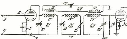
lagging phase angle approaching 90 deg. and whereby currents in input and output differ in phase by approximately 180 deg. and the voltages induced in the output cancel. W. R. de Cola, Belmont Radio. No. 2,293,384.
