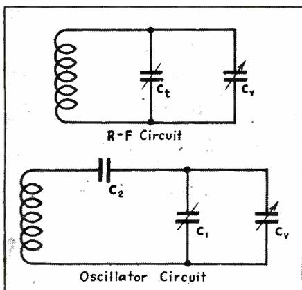
Fig. 1—Radio-frequency amplifier and oscillator circuits in which are the trimmer and padder condensers whose relations are outlined in this short-cut to the tracking problem
