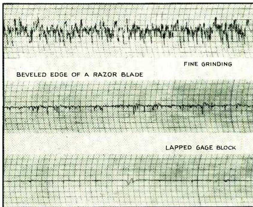
Fig. 5—Typical roughness charts. Vertical scale—2 micro-inches per small division; horizontal scale—500 micro-inches per small division
