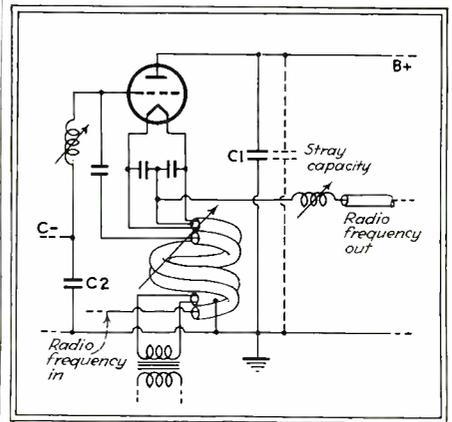
Fig. 2—Improved form of power amplifier circuit developed for use in frequency modulated transmitters
