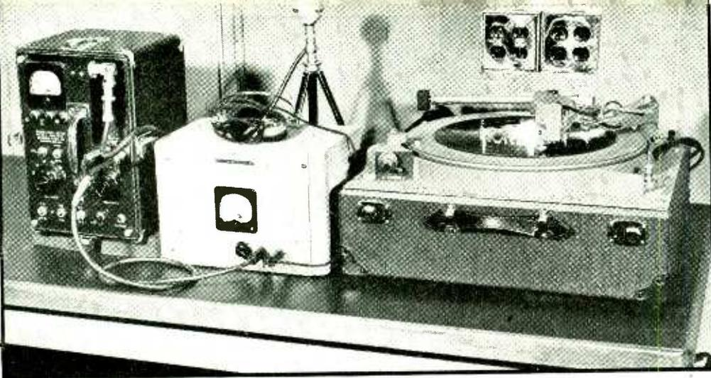
Field equipment consists of a microphone, two stages of a sound level meter used as a pre-amplifier, a single-ended recording amplifier incorporating feedback and an instantaneous disc recording mechanism with a modified cutting head
