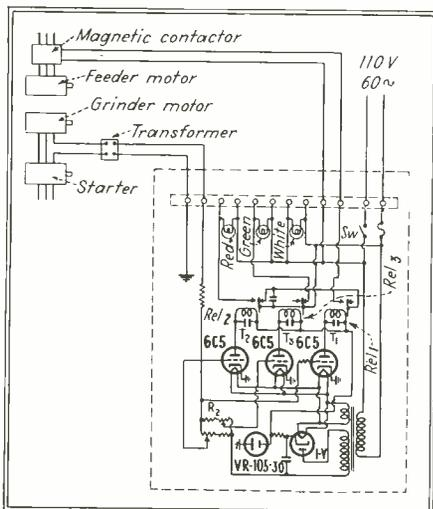
Circuit of automatic control for grinding machine feed motors
