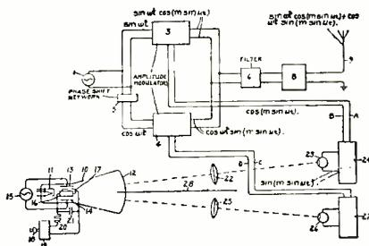
wave which is a simple sinusoidal function of the instantaneous value of the signalling voltage, and modulating the carrier wave in accordance with the auxiliary wave. Hans Roder, GE. No. 2,294,209.
