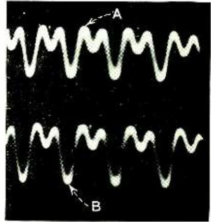
Fig. 9—Comparison of cutter output voltage waveform and playback output voltage waveform
