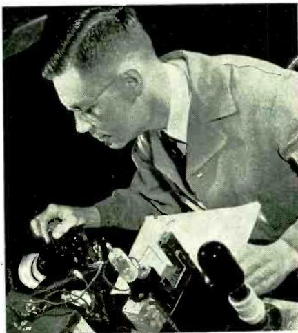
Dr. N. C. Beese, Westinghouse research engineer, is shown measuring the amount of fatigue of a piece of fluorescent glass when exposed to constant and continued ultraviolet radiations. Research on the fatigue phenomenon showed that the molecules responsible for fluorescence get "tired" and lose an appreciable amount of their activity when excited for long periods of time, but regain their strength after suitable rest periods in the dark
