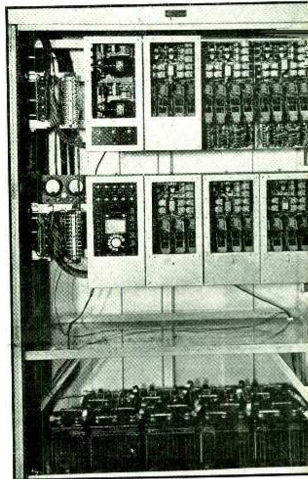
American Teletimer Corporation equipment measures and records the time for the leading horse at various points around a racetrack. Modulated light-beams are cut as the animal passes, stopping a rotary switch and relay mechanism in the equipment room
