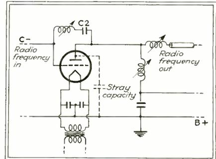
Fig. 1—Usual type of circuit employed in radio frequency power amplifiers
