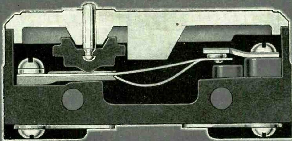
This sectional view of the Micro Switch shows assembly of features described below
