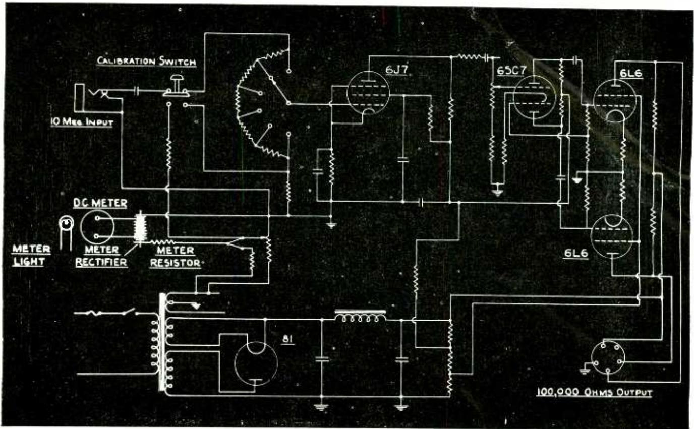
Fig. 4—Resistance-capacity, three-stage amplifier for use between Rochelle salt crystal and oscillograph. Amplifier gain is approximately 100,000
