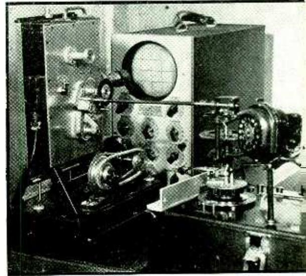
Laboratory equipment comprises a special playback pickup pictured elsewhere, an equalizer and turntable, the sound level meter again used as a pre-amplifier and the sound analyzer, moving film camera and DuMont oscilloscope shown here
