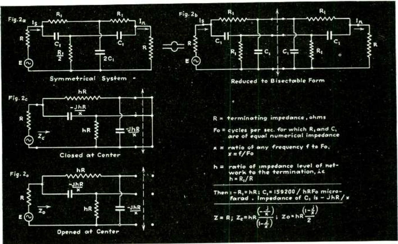
A special method of evaluating the transmission characteristics of four-terminal networks which possess electrical and structural symmetry. This method saves considerable labor and time compared to conventional solutions
