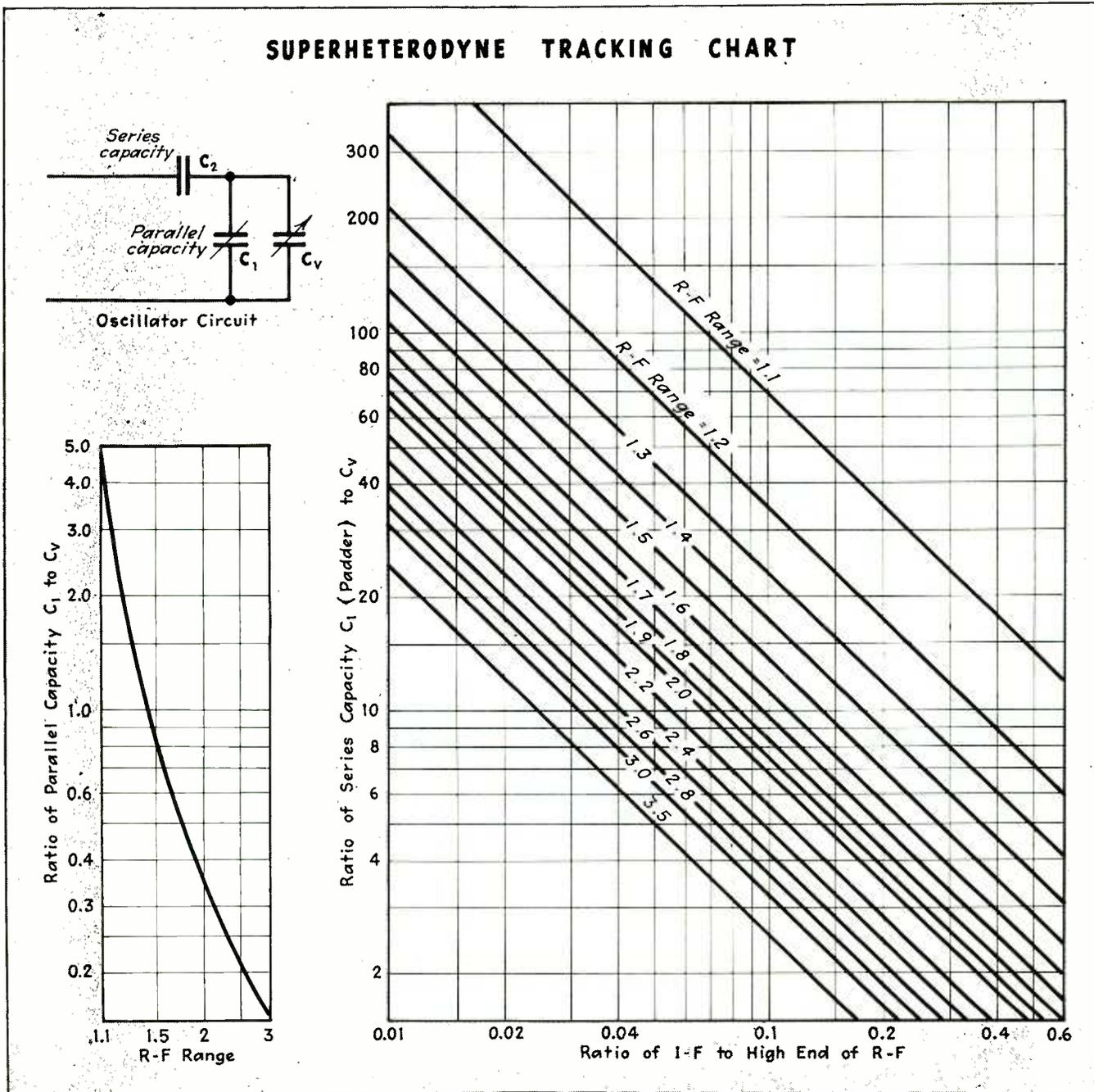
Fig. 2—Design chart for determining series and shunt capacitances for tuned circuits in single control superheterodyne receivers
