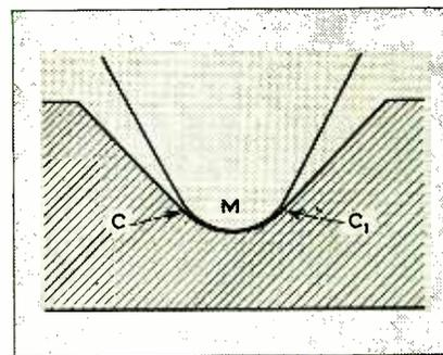
Fig. 6—When playing back lacquer-coated discs the system will have a resonant frequency dependent upon the stylus point mass  $M$  and the elasticity at points  $C$  and  $C_1$
