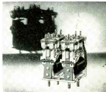
double throw contacts, maximum (non-inductive) rating of 5 amps per contact, weight 7 ounces, size  $1\frac{1}{8} \times 1\frac{1}{8} \times 2$  inches. They meet every Army, Navy or CAA specifications.
