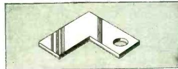
The stationary contact is a flat inlay of 99.95% fine silver. This construction assures ample over-load capacity and maximum heat dissipation.
