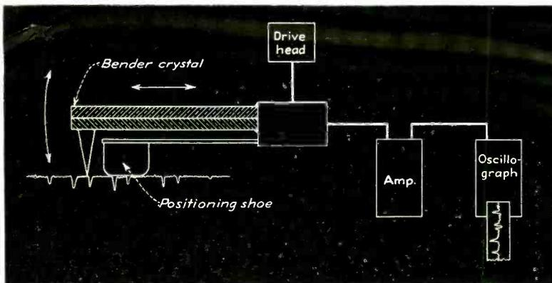
Fig. 3—Block diagram of the surface analyzer showing method by which tracer point follows indentations in surface to be measured
