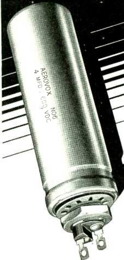
● Something new has been added to this long-popular Aerovox "10" series Hyvol capacitor. Note the double terminals—spaced on the stepped bakelite threaded terminal post. This means the can of this handy inverted-screw-mounting capacitor is now insulated or "floating". No longer is an insulator washer required when non-grounded mounting on a metal chassis is desired.
