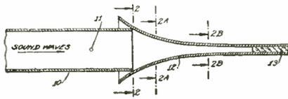
whereby sound waves applied at input opening are increased in particle velocity during progression through horn, and sound absorbing means at the throat of horn to absorb the energy of increased particle velocity waves. F. E. Terman, Int. Standard Electric. No. 2, 293,181.
