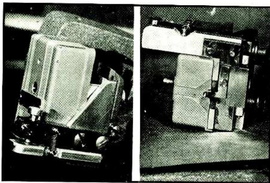
Fig. 1—Two views of a commercial cutting head with advance-ball attachment added to insure uniformity of depth-of-cut
