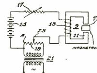
an alternating current of a predetermined frequency through said electromagnet, and gradually reducing the amplitude of alternating current to condition said electromagnet for operation at a predetermined point on its hysteresis loop characteristic. R. E. Braden, RCA. No. 2,296,764.
