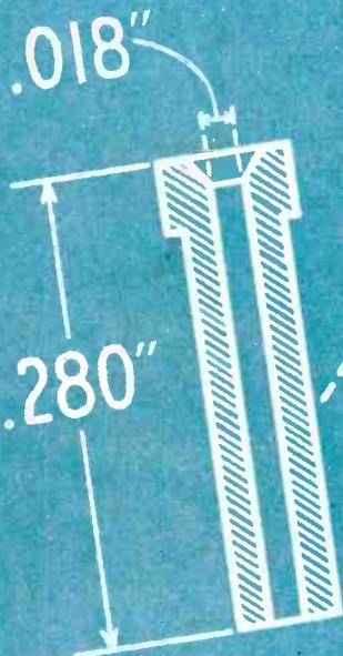
This will give you an idea of what can be done by custom molders. It is a communications part of Lumarith. It is .280" long. It comes out completely formed with a true .018" hole through the center. No finishing necessary. Rate of production: 100,000 a day. Formerly took 3 months.
