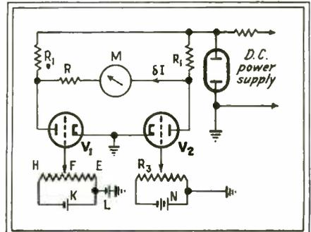
FIG. 2—Simplified circuit of equipment used for experimental verification of theoretical results and for calibrating the meter
