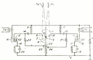
anode-cathode paths of said phototube by introducing into the grid circuit of each amplifying tube a controlled voltage derived from the currents generated in said phototubes opposite in phase but corresponding in magnitude to the crosstalk voltage normally present in said grid circuit. W. J. Alberseim, WECO. No. 2,295,536.
