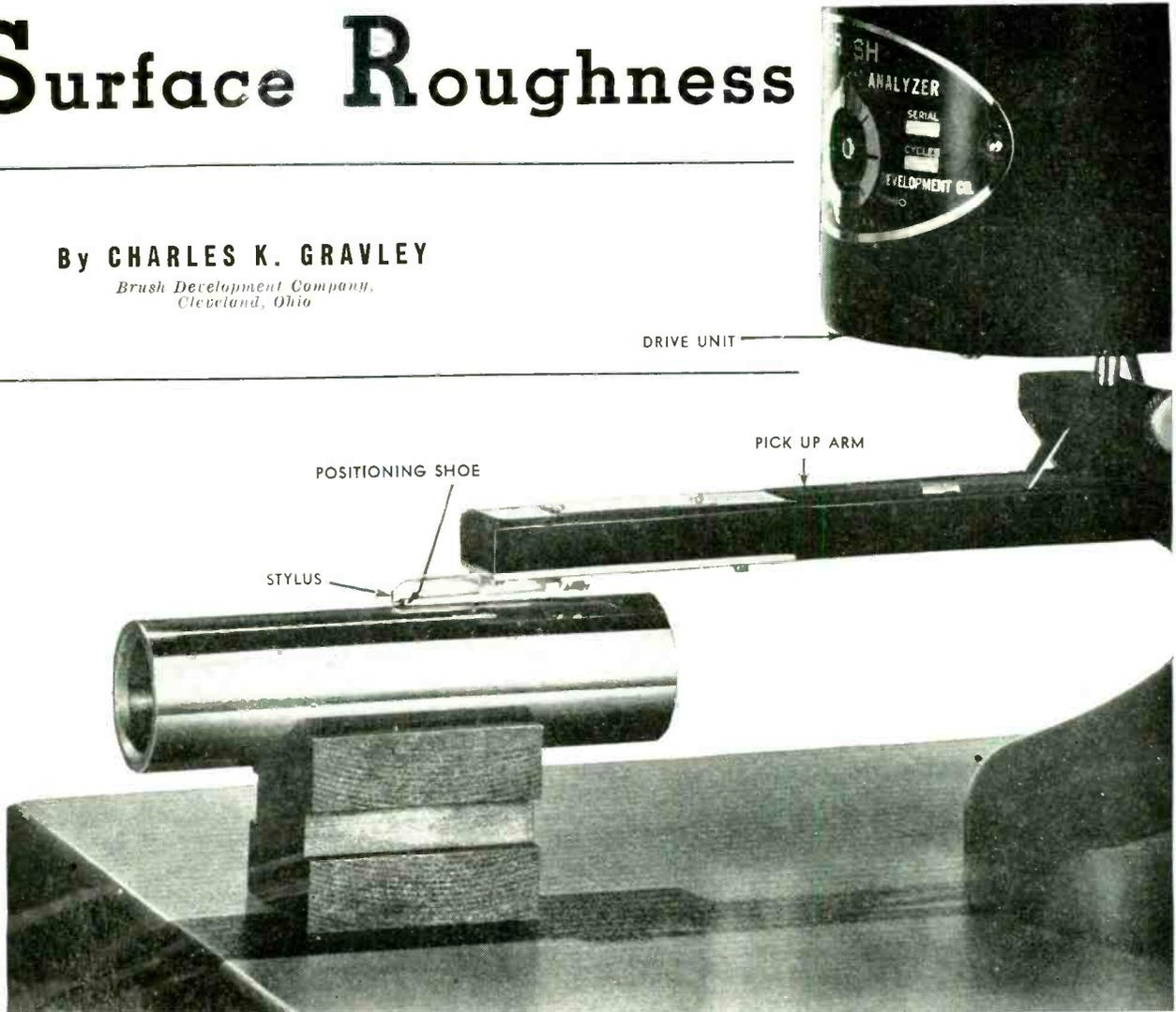
Fig. 2—Closeup of the pickup arm with positioning shoe and tracer point
