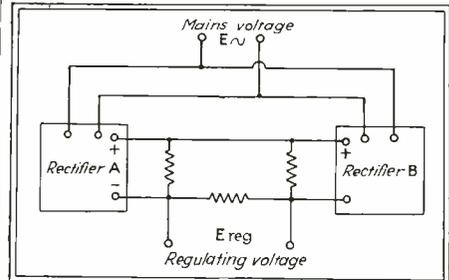
Fig. 1—Block diagram of voltage regulator consisting of two rectifiers operated in opposition
