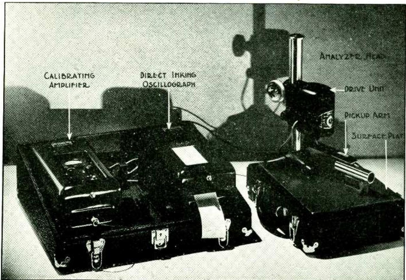
Fig. 1—A complete setup for measuring surface roughness composed of a hill-and-dale pickup, a means for moving the pickup over the surface and amplifier with oscillograph
