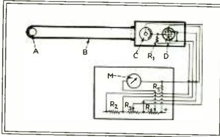
Fig. 1 — Diagram of field strength meter. (A) Discharge vessel. (B) Insulating tube, 1 in. in diameter, 2 ft. in length; (C) Phototube; (D) Amplifier tube; (M) Meter 0.25 milliamperes. (R<sub>1</sub>) 10 megohm resistor. (R<sub>2</sub>) 10,000 ohm resistor; (R<sub>3</sub>) 10,000 ohm resistor; (R<sub>4</sub>) 10,000 ohm resistor; (R<sub>5</sub>) 2,000 ohm resistor
