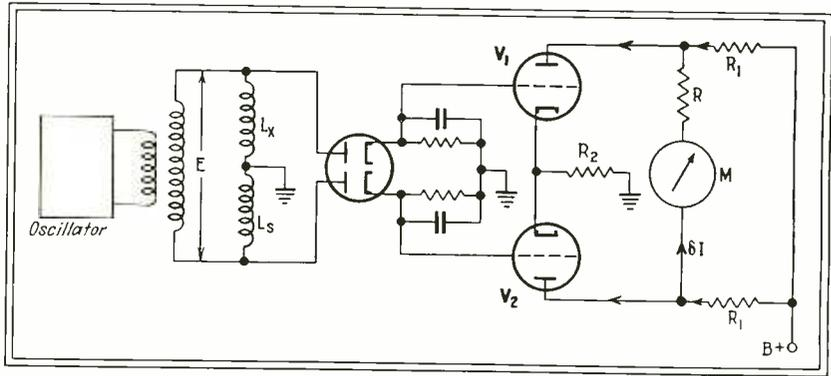
FIG. 1—Simplified circuit diagram of impedance testing bridge
