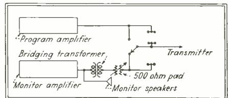
**Scheme permitting rapid substitution of a monitor amplifier for a program amplifier in the event the latter fails**
