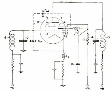
to neutralize a substantial part of this input conductance. W. H. Aldous, Hazeltine. No. 2,294,328.
