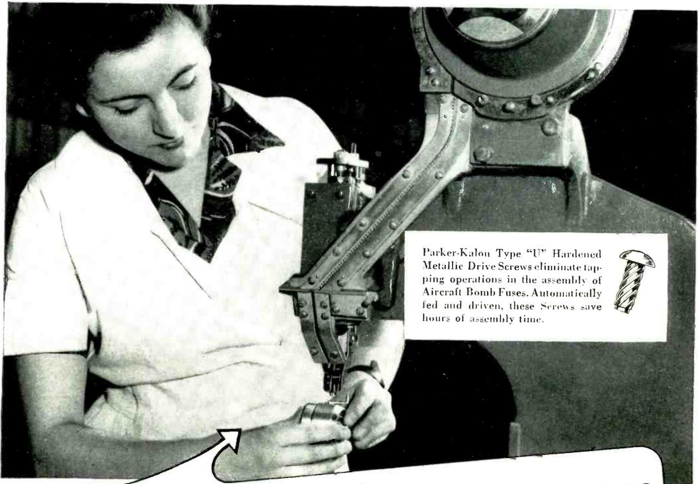
Parker-Kalon Type "U" Hardened Metallic Drive Screws eliminate tapping operations in the assembly of Aircraft Bomb Fuses. Automatically fed and driven, these Screws save hours of assembly time.
