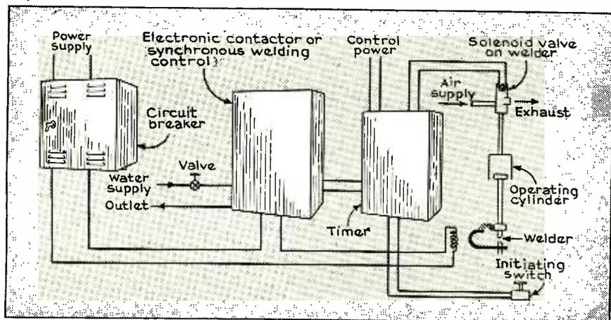
Fig. 1—Complete setup for resistance welding, illustrating a typical arrangement of electrical and mechanical as well as electronic controls
