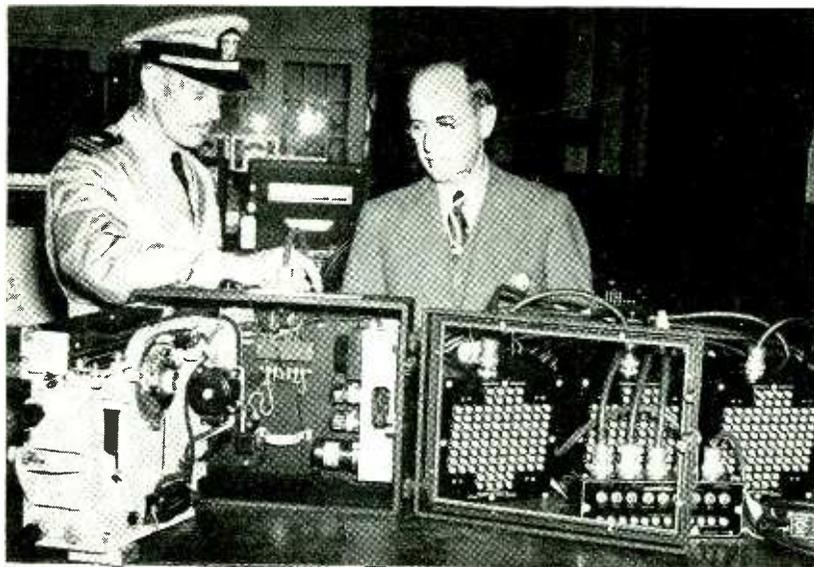
Lieut. William C. Clay, U. S. N. and E. B. Evleth, vice president and general manager of the Brown Instrument Co. inspect the newly developed Flight Recorder. This instrument automatically records as many as 144 different readings every three to four minutes and provides a complete and accurate record of an airplane's performance while permitting the test pilot to concentrate on flying the plane
