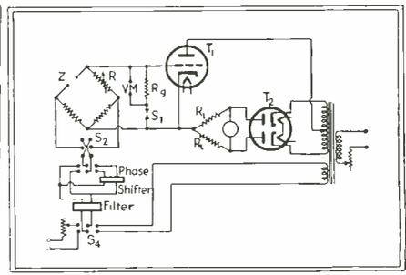
Fig. 2—Schematic wiring diagram of the complete phase bridge showing the electronic detector and supplementary impedance bridge required in making the measurement
