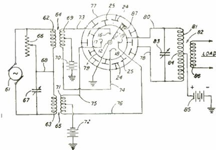
phase current as to produce a revolving electrostatic field and restrict the electrons emitted into a narrow beam, alternate anodes being connected together and to a source of high potential to form an output circuit, whereby, upon said beam rotating in sequence upon anodes, an alternating current of the frequency desired may be set up in output circuit. A. A. Stuart, Jr. Bendix Aviation. No. 2,293,368.
