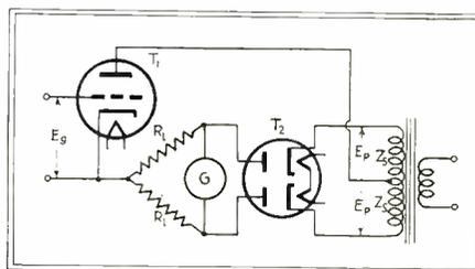
Fig. 1—Schematic wiring diagram of the essential elements of the electronic phase bridge
