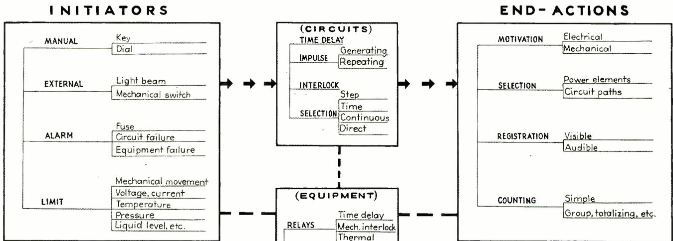
A remote control cycle may be started in many ways and one of the first concerns of the design engineer is selection of a suitable type of initiator, the most common of which are listed at the left. Work which may be done at the distant point is likewise varied, as suggested by the tabulation at the right, so the most desirable end-action must simultaneously be chosen
