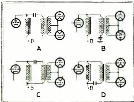
is used to feed d.c. to the first tube and a condenser is used to keep the d.c. out of the push-pull input transformer primary. Does it make any difference which of the four connections is used?
