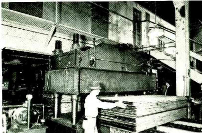
One of two presses utilizing radio frequency power to speed up plywood bonding in Albany Plylock's western plant. Radio frequency generators and associated equipment are located in the balcony immediately above the press. The control panel just barely visible behind and to the right of the press permits both presses to be operated at maximum efficiency from a central point
