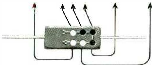
The Types J and K condensers, molded in Bakelite, are identified by the standard R.M.A. 6 dot color code, read in the direction of the molded arrow to indicate 3 significant figures, decimal multiplier, tolerance, and rated voltage, as shown in the table above. The unit pictured has a capacity of 500 MMF  $\pm$  2%, with a voltage rating of 500.
