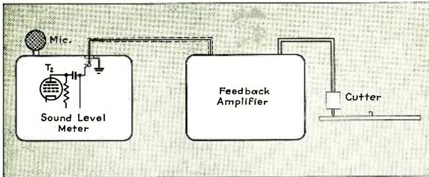
Fig. 5—Block diagram of field recording setup, showing position of auxiliary jack in sound level meter permitting two stages to be used as a pre-amplifier
