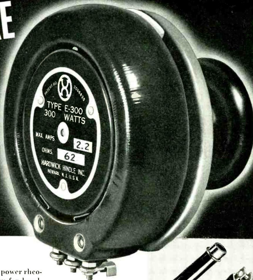
Exclusive features of this compact power rheostat assure you 25% more capacity for handling possible overloads,—and consequently more heat dissipation—less temperature rise without taking up more space. The deeper winding form gives more wire, more surface area.
