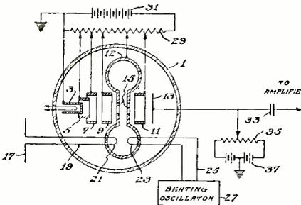
electrode between cavity and collector biased independently of the cavity and collector, the hollow electrode having the purpose of returning electrons to the cavity and for adjusting their phase so that the returning electrons produce uhf waves within cavity. E. G. Linder, RCA. No. 2,293,151.
