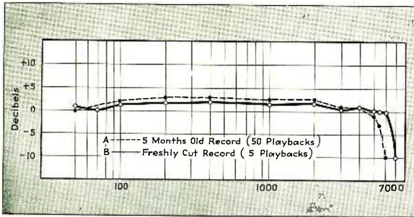
Fig. 8—Overall response characteristics of playback system. Calibration is, in part, a function of the type of disc used
