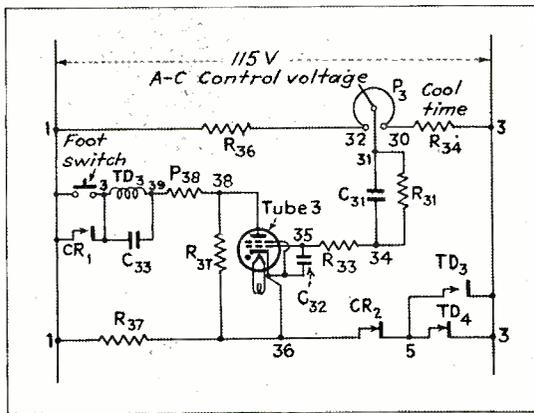
Fig. 5—Elementary diagram of cool timer circuit. It resembles the circuit of Fig. 3 but a-c supply leads are reversed to secure required polarity conditions
