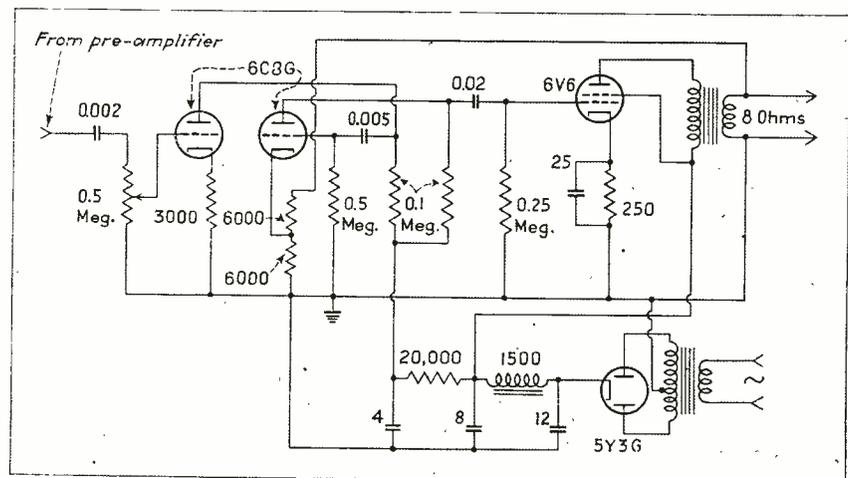
Fig. 4—Circuit diagram of single-ended recording amplifier incorporating feedback. Two stages of a sound level meter are used as a pre-amplifier
