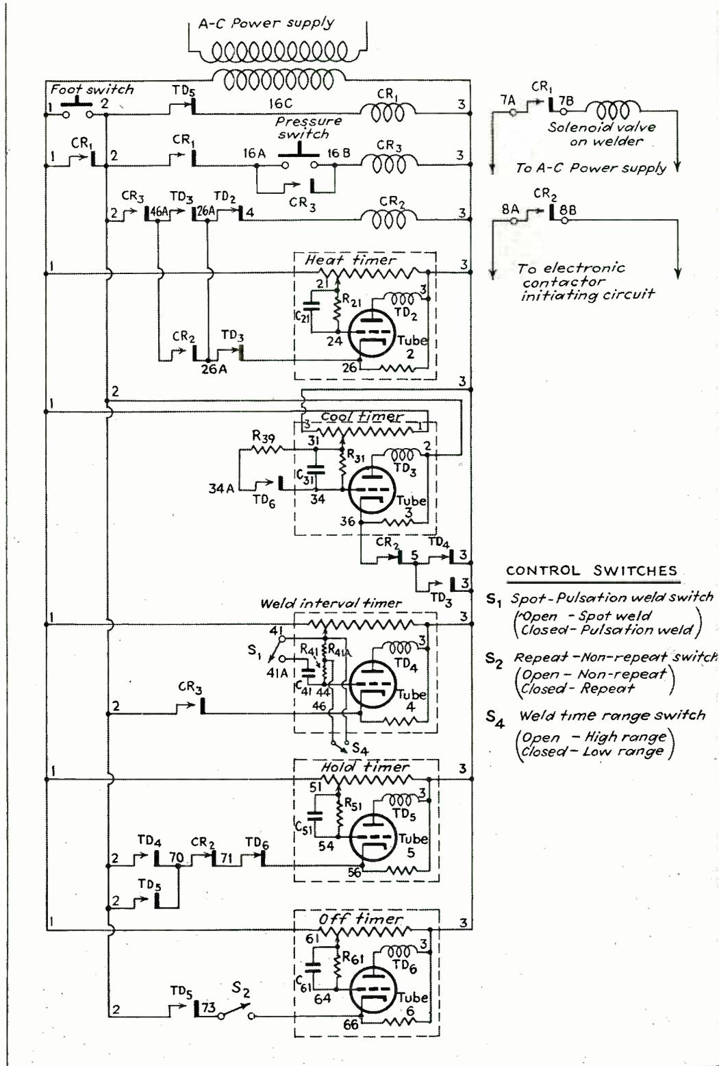
Fig. 2—Elementary diagram of a 5A type automatic electronic weld timer designed for use with welding power control units of the non-synchronous electronic contactor variety. Circuits included by the dashed lines are shown in simplified form
