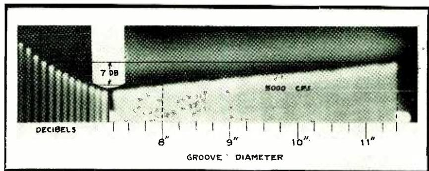
Fig. 10—Oscillographically plotted curve of system's translation loss at 5000 cps. An error of almost 7 db would result if the high frequency range was plotted at the beginning instead of at the end of a record cut from the inside out. A method of minimizing this error is outlined in the text
