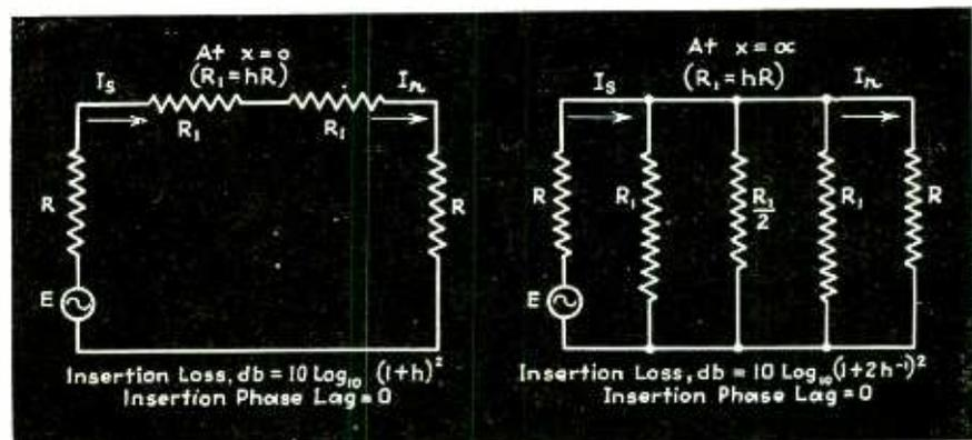
Fig. 4—Equivalent circuit of Wien bridge at zero and infinite frequencies
