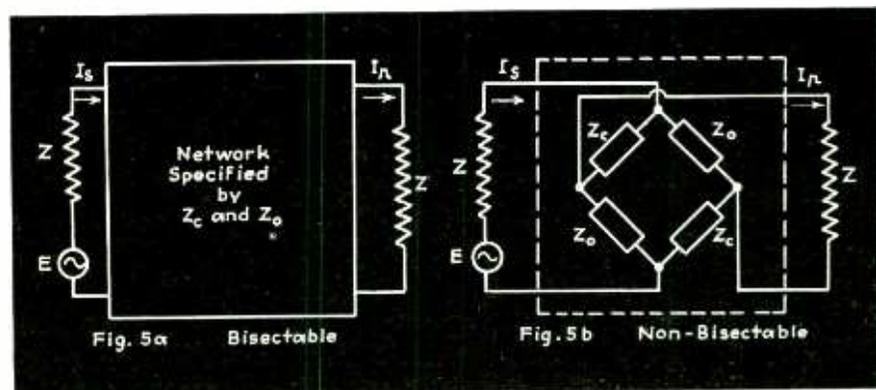
Fig. 5—Method of replacing a bisectable network by a non-bisectable bridge
