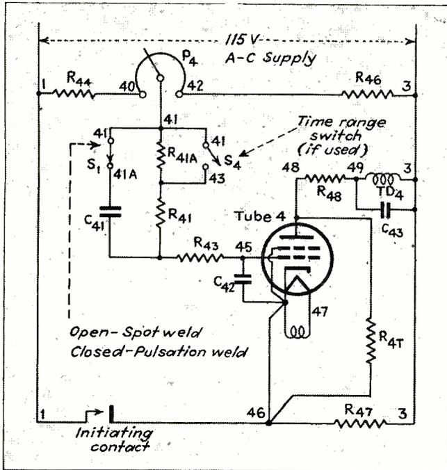
Fig. 3—Simplified diagram of a typical thyatron tube timer circuit. It is the basis of design for all the individual timing units shown within the dashed lines of Fig. 2 except the cool timer
