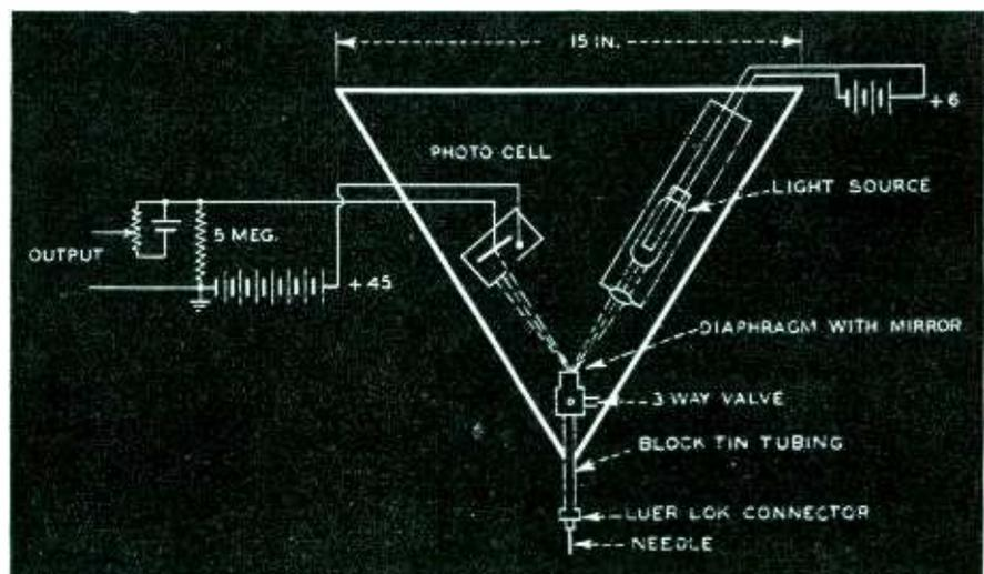
Fig. 7—Circuit of a device for making an accurate record of the pressure changes in the cardiovascular systems of animals such as the dog and turtle
