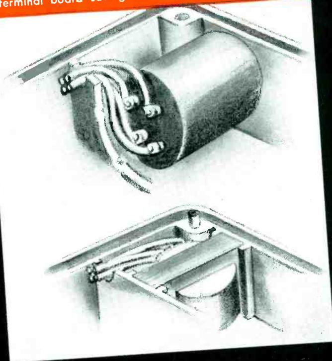
One UTC design eliminated a threaded shank, lockwasher and nut by changing to a spun-over shoulder on the shank. Saving . . . 150,000 lockwashers and nuts . . . 150,000 threading operations.
