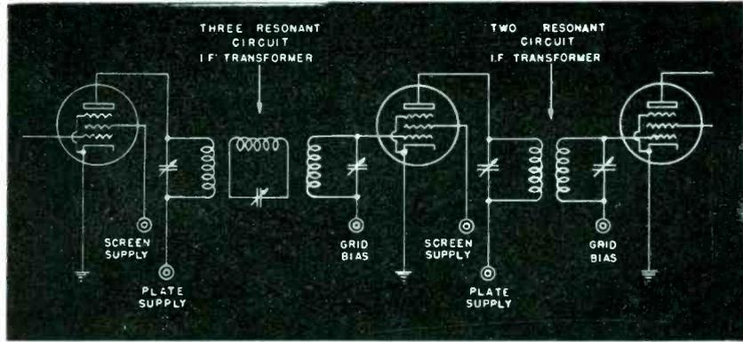
Fig. 1—Schematic wiring diagram of two stage amplifier containing a three resonant circuit network and complementary two circuit network for providing uniform response in the pass band
