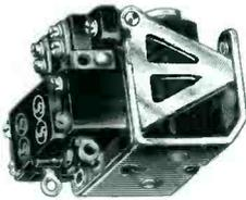
double make, double break contacts, 50 grams; contact capacity at 30 volts d.c., 20 amps (inrush 100 amps); 200-hour salt spray test; pickup, at 20 deg. C., 5 volts (0.36 watt); nominal coil voltage, 14 volts d.c.; coil wattage at 14 volts d.c. at 20 deg., 2.8 watts; temperature range, -40 to +90 deg. C. Dimensions are  $1\frac{1}{2} \times 1\frac{1}{8} \times 1\frac{1}{4}$  inches high, weight 5 ounces.
