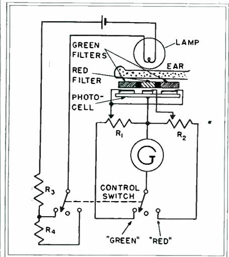
Fig. 1—Schematic wiring diagram for multiple scale oximeter, which, when used multiple scale, permits direct readings to be made of oxygen saturation of the blood
