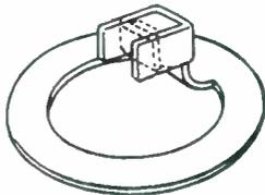
pierced hole in the shielding. The tongues on the bonding ring are then formed around the shielding pigtail and soldered. Since the unit is made of soft copper, all excess lengths of tongue may be cut away. The soldered connection is protected by insulation material (such as plastic tube or friction tape) to prevent any stray wires of the shielding braid from rupturing the insulation of other wires and causing a short circuit.
