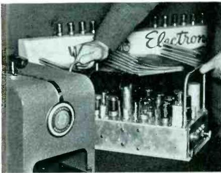
This permits easier and more accurate tuning, and reduces the effects of car vibration on tuning adjustments. Receiver battery drain has been reduced 35 percent and a material improvement made in the effective communication range.
