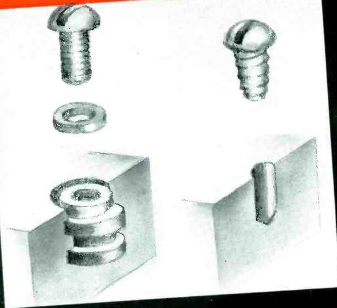
In die cast structures, covers and nameplates were held on by screws. A UTC design modification added a round projection in the casting, which is spur over to hold the plate or cover. Saving: over 2,000,000 screws and lockwashers . . . over 2,000,000 tapping operations.
