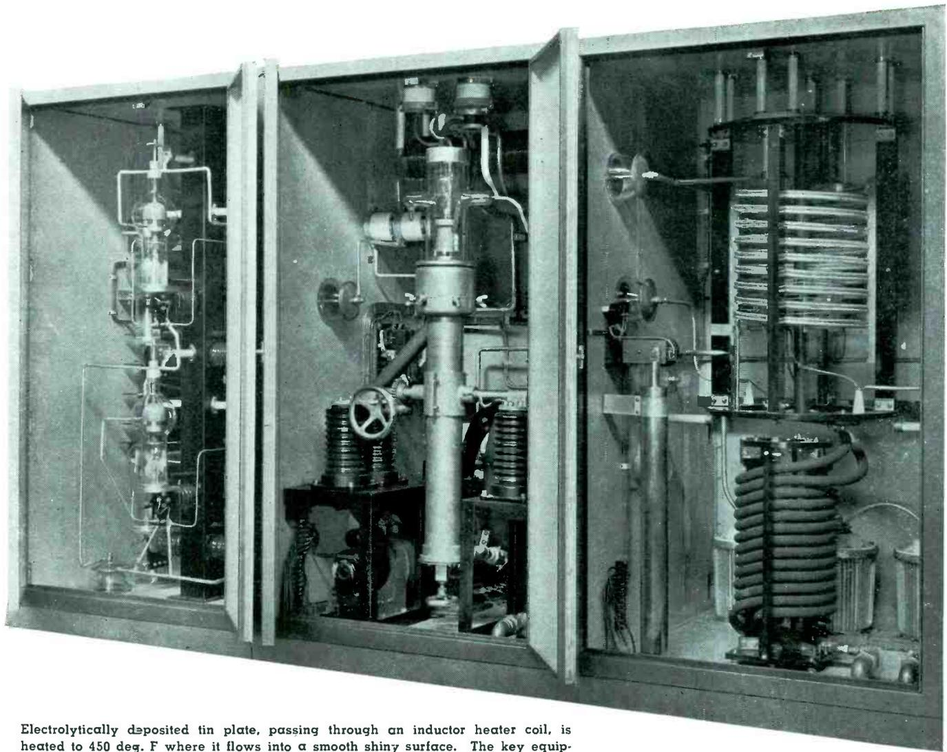
Electrolytically deposited tin plate, passing through an inductor heater coil, is heated to 450 deg. F where it flows into a smooth shiny surface. The key equipment behind the inductor coils is shown above. This three cubicle unit contains electronic rectifier, oscillator tube and oscillator circuit. The d-c power at 17,000 v is fed to the plates of the 100 kw oscillator tube where it is converted into high frequency alternating current, changing direction 400,000 times per second
