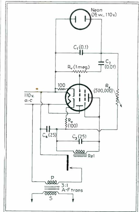
Fig. 5—"Relaxation" type timer using high vacuum tube
