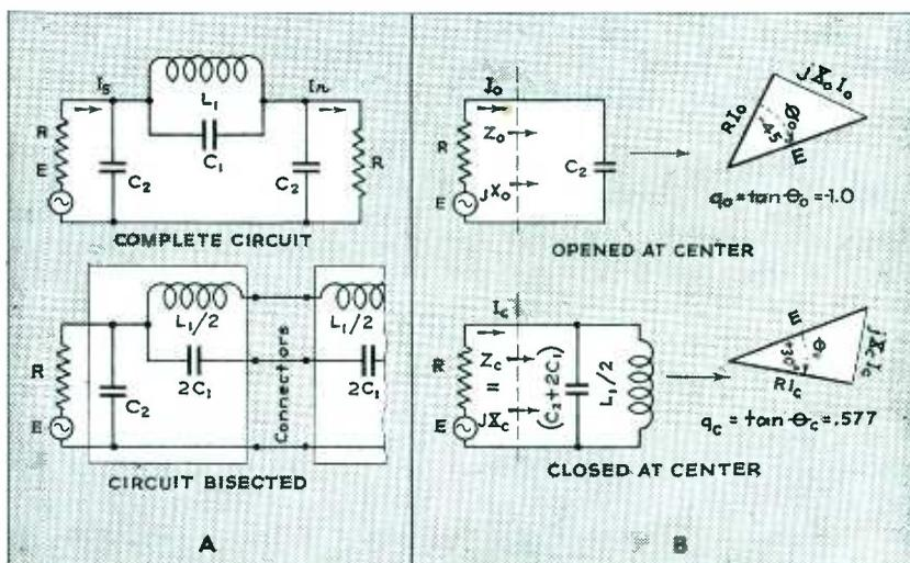
Fig. 1—Bisectable reactance networks with equal resistance terminations
