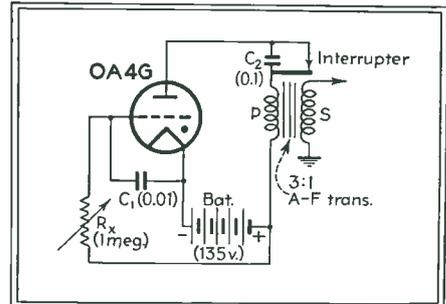
Fig. 1—Simple pulse-generating circuit
