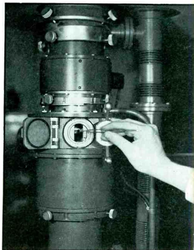
electrons incident on it. It is furthermore obvious that glass lenses cannot serve to focus the electrons. This is accomplished instead by strong axially symmetric magnetic fields formed by suitably designed iron-encased coils carrying electric current. Otherwise the electron microscope closely resembles the light microscope in plan.
