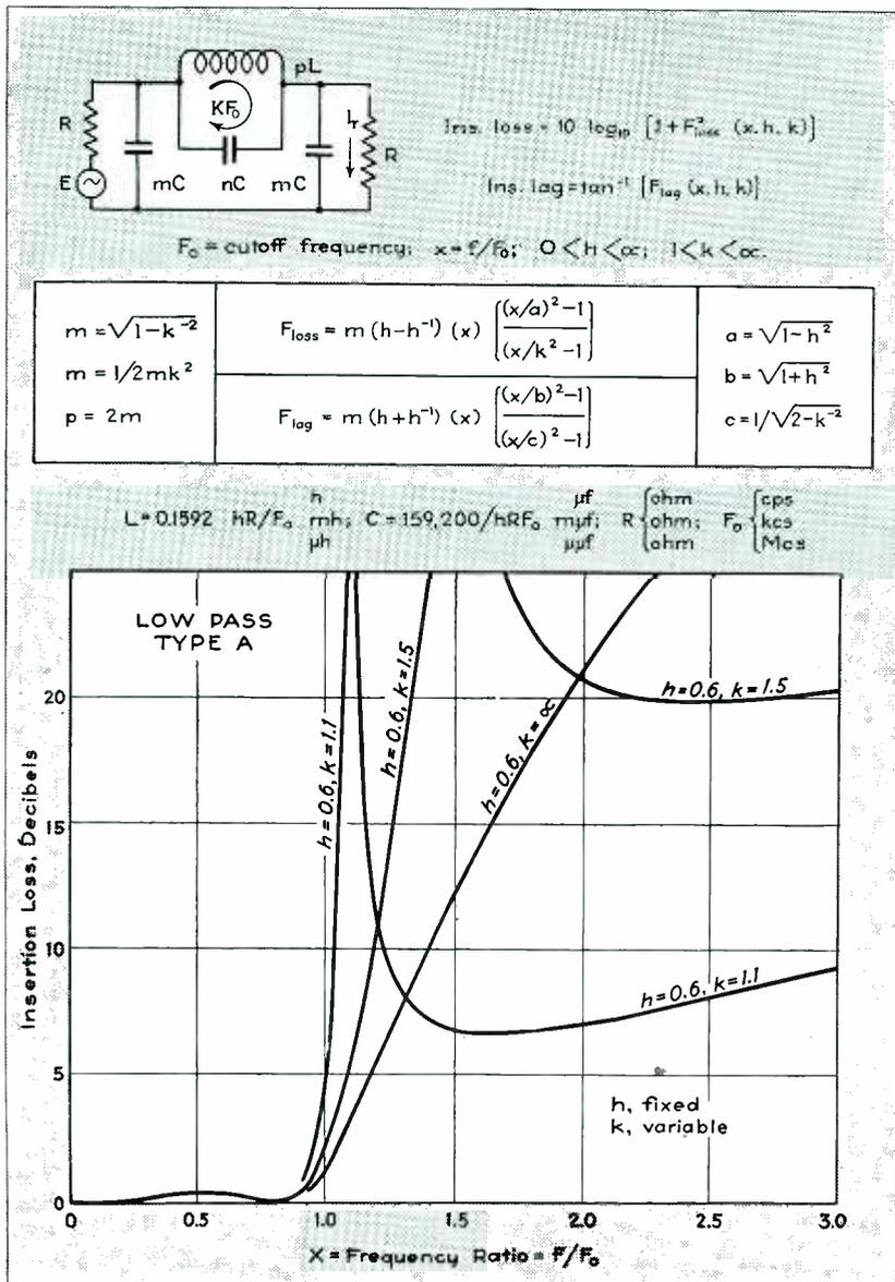
The ratio  $f/F_0$  will be here given the designation  $x$  customarily applied to the abscissa in curve plotting.
