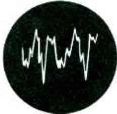
E-392 cycles per second as produced by a single reed of an accordion. Complex wave form is the result of reed being driven to a high amplitude, producing many harmonics or overtones.
