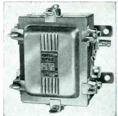
corners are gas welded inside and out. The unit is closed by a simple eyebolt and wing nut arrangement of clamping design which protects the rubber gasket from excessive pressure caused by forcing the wing nuts too tight.
