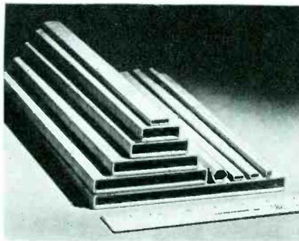
inches square inside with a tolerance of approximately 0.002 inches. The tubes have square corners and straight side walls and are available in continuous lengths in high dielectric kraft, fish paper, red rope, acetate, or combination wound. Shapes which may be had are square, round, or rectangular. The tubing and cores may be used for coil forms as well as other uses.
