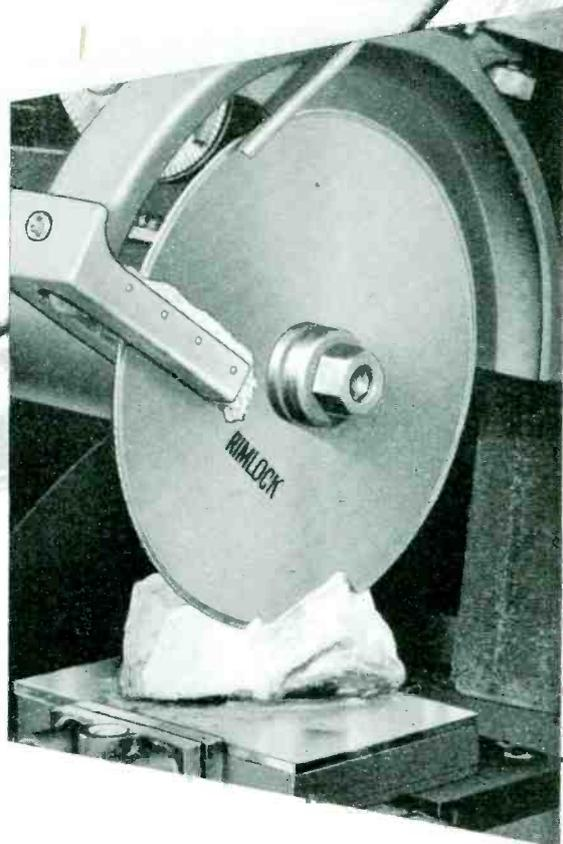
Rimlocks are long lived cutters, too—over 700 quartz wafers, averaging 4 sq. inches of surface area each, have been cut with a single blade.
