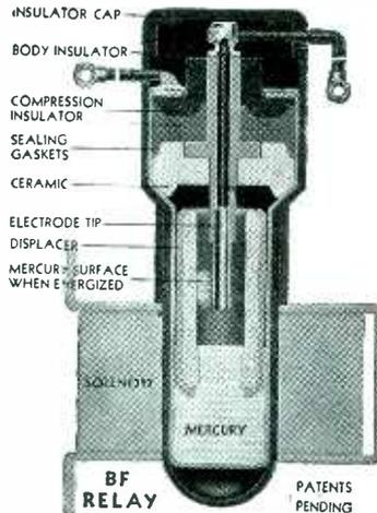
Available in 10-, 30- and 75-amp sizes, the relays are factory-adjusted to fast or slow opening or closing or both; set to normal open or closed, as desired. The relays can be built in any size or kind, including time delays.
