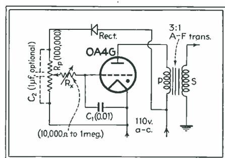
Fig. 3—Pulse generator operated from a-c line
