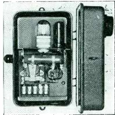
those of a SPDT switch, for either normally closed or normally open operation. This provides for action either when the light beam is broken or when it is made. The operating range of Type A15 is 20 feet with light source L30, and 40 feet with light source L60. (Type A25 is supplied with light source L30 for 50 foot operation, and with light source L60 for 100 foot operation).
