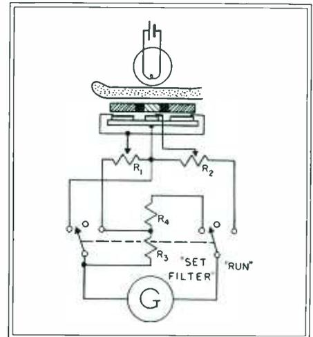
Fig. 3—Circuit diagram of single scale oximeter, with automatic adjustment for ear thickness
