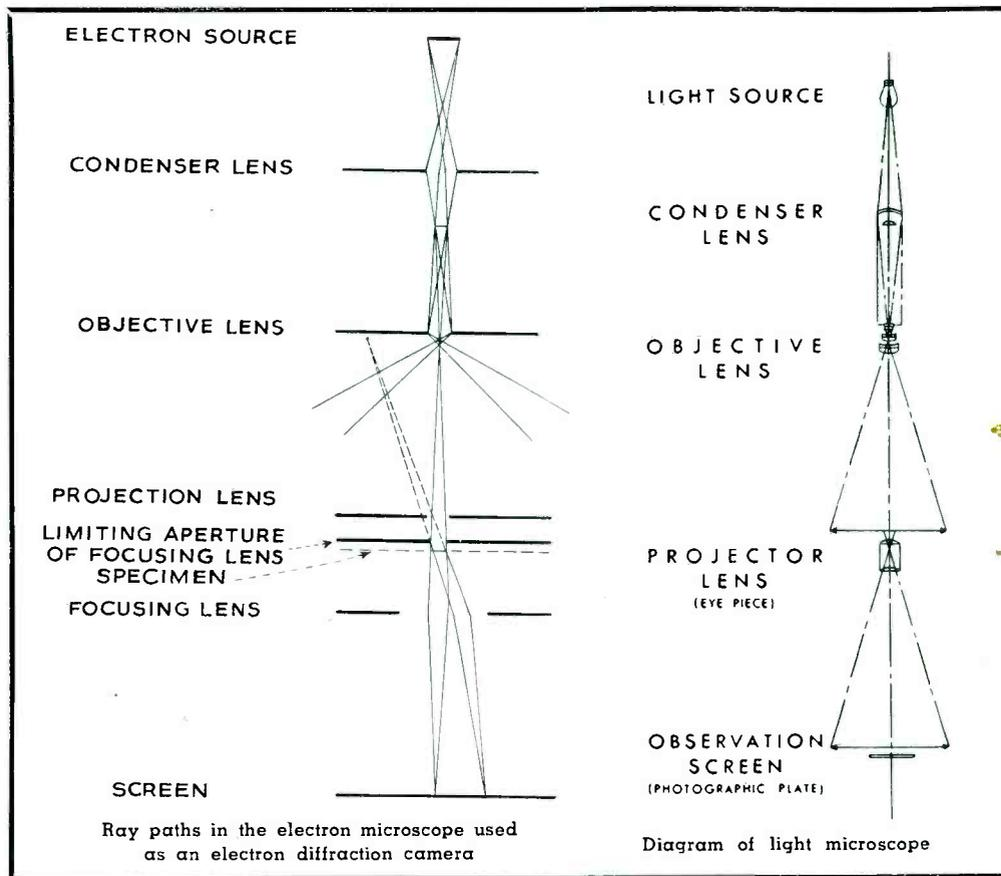
Ray paths in the electron microscope used as an electron diffraction camera
