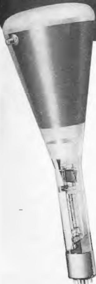
★ Hour after hour, day-in day-out, DuMont cathode-ray tubes check Clarostat controls coming off the production line. The single-dot trace meandering diagonally across the screen in response to resistance vs. rotation, provides "all the answers" at a glance for inspectors and engineers alike.
