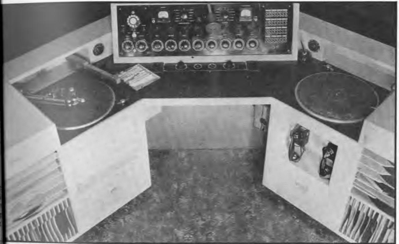
Master control console in transmitter room, using many unique switching circuits designed and built by KTKC engineers
