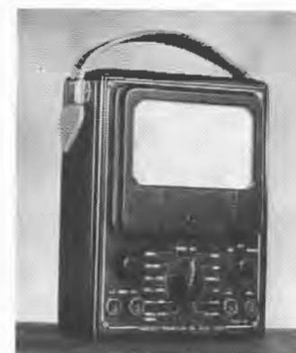
are obtained on the 100-ma scale. Shunts and matched pair metalized voltage multipliers are rated as within 1 percent accuracy. The rectifier is a copper oxide type. Overall dimensions are 7 x 5½ x 3 inches, and the instrument is supplied complete, with self-contained battery supply.
