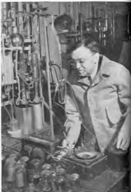
Dr. Harvey C. Rentschler conducting an experiment in which oxygen gas is being dissolved in a strip of zirconium metal enclosed in the glass tube suspended directly in front of him
