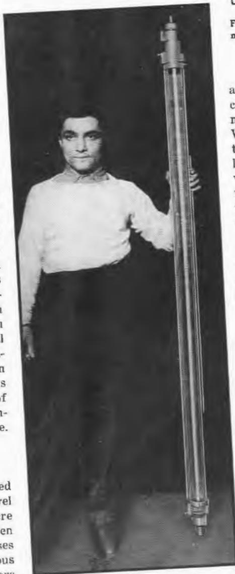
High-pressure mercury vapor tube 5 feet long, with rated input power of 4.5 kw. for use in a blueprint machine
