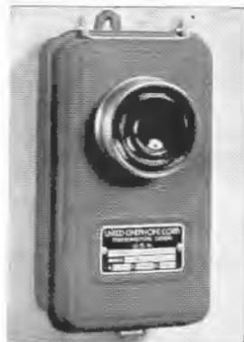
is designed for applications requiring high sensitivity. Model 72 operates on a minimum of 4 ft. candles, while Models 74 and 76 are rated at 1/2 ft. candles. Contact capacity of all four units is rated at 3 amps. For additional cost infra-red filters are available, as well as a non-inductive microswitch for mounting on the sensitive relay to increase the contact capacity to 10 amps.
