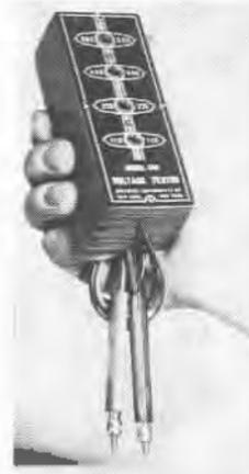
pointed prods across the line or part in question. It utilizes less than a milliamperere of current, requires no accessories and is a general "bang-around" type of instrument. It is 5 inches high, 1 1/2 inches wide and is 3/4 inches deep. Weight, approximately 2 lbs.
