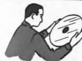
3. A non-warping, non-chipping fibre piece is cut to exact measurements and inserted in the center hole. This is another of Audio's original and unique developments.
