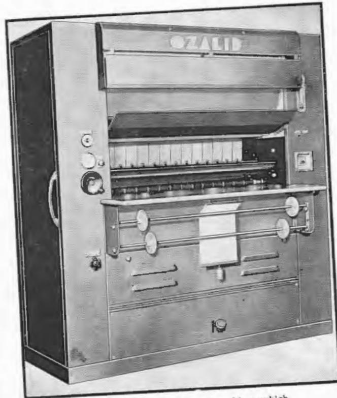
High-speed photo-printing machine which uses a high-pressure mercury vapor tube
