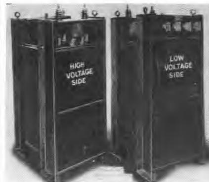
The unit is also light and compact and requires no headroom. It is constructed throughout with class B, heatproof insulation consisting of fiber glass, mica, asbestos and porcelain. The transformers are available up to 500 kva; in voltages to 4800 volts, single phase, three phase, and Scott connected 3 to 2, or 2 to 3 phase, in one unit.
