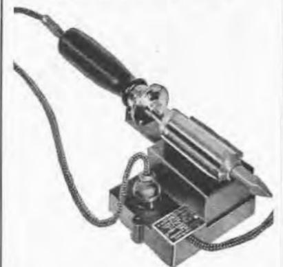
This is a thermostatically controlled device for the regulation of the temperature of an electric soldering iron. When placed on and connected to this stand, iron may be maintained at working temperature or through adjustment on bottom of stand at low or warm temperatures.
