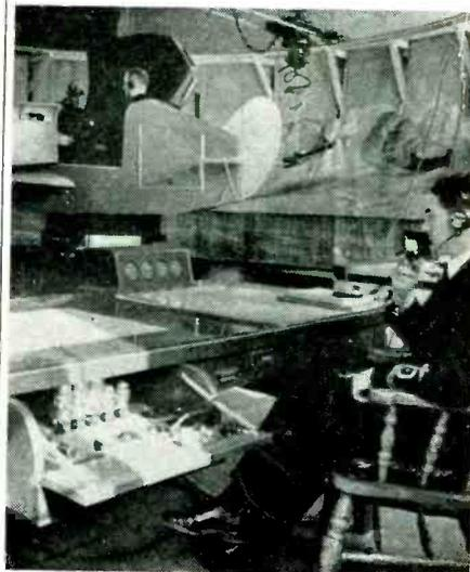
A Link trainer in action at a Royal Naval Air Station. The desk contains an electronic amplifier that the instructor uses to communicate with students during blind flying training
