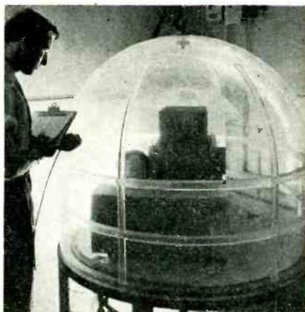
RCA Victor engineers made this transparent altitude chamber for aircraft radio equipment tests from the Plexiglas nose cone of a bomber. It permits measurements and observation by many engineers from all directions
