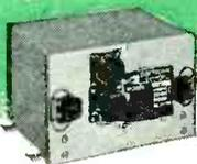
Here is a low-powered E-L Power Supply (Model S-1361). Its output power is 10 watts to DC; AC to DC; AC to AC. Input voltage is 24 volts DC, and output voltage is 350 volts DC at 25 ma. It weighs only 5 pounds.
