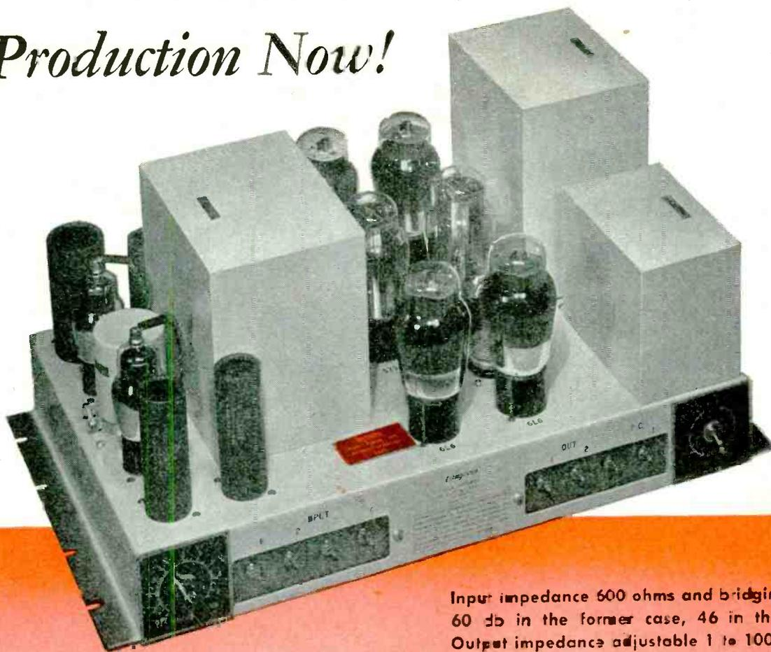
Input impedance 600 ohms and bridging. Gain 60 db in the former case, 46 in the latter. Output impedance adjustable 1 to 1000 ohms.
