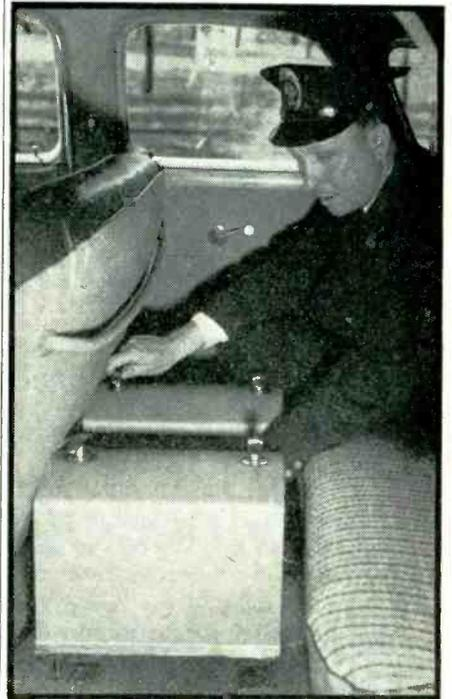
Transmitter and receiver units mounted behind driver's seat in squad car. Cable connectors permit quick removal of units
