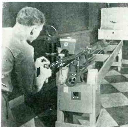
Student pilots in the U. S. Navy get gunnery practice with this lightbeam gun. An optical gunsight, similar to the one used in fighter planes, is used to spot the target. The gun shoots a lightbeam at the model plane and the score is recorded by a phototube
