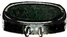
The Leitz Photo-Electric Colorimeter uses a Luxtron\* photocell, of which Leitz literature says: "... possesses exceptionally stable and uniform characteristics. Its high sensitivity in the range of short wave lengths of the spectrum is a definite advantage in many colorimetric determinations..."
