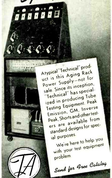
Atypical "Technical" product is this Aging Rack Power Supply—not for sale. Since its inception, "Technical" has specialized in producing Tube Testing Equipment. Peak Emission, GM, Inverse Peak, Shorts and other testers are available from standard designs for special purposes.
