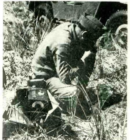
This walkie-talkie wears a wool felt overcoat to cushion it against bumps and shocks. A zipper permits access to the controls for operation in the field. Wool felt is also used inside to protect the parts from vibration
