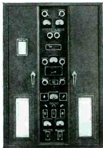
Control Cabinet Assembly. Consists of transmitter remote control unit, loud speaker and two fixed frequency airport receivers.
