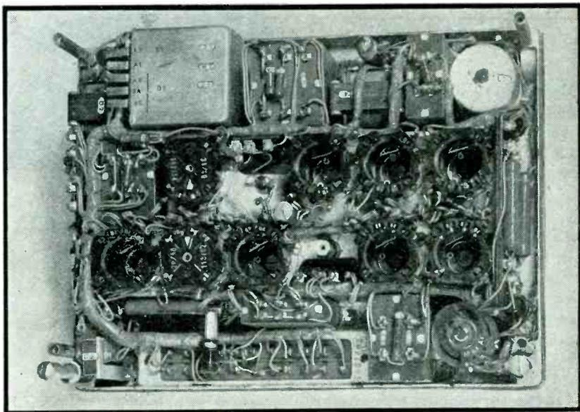
FIG. 4—Intercom amplifier, shown with tubes removed
