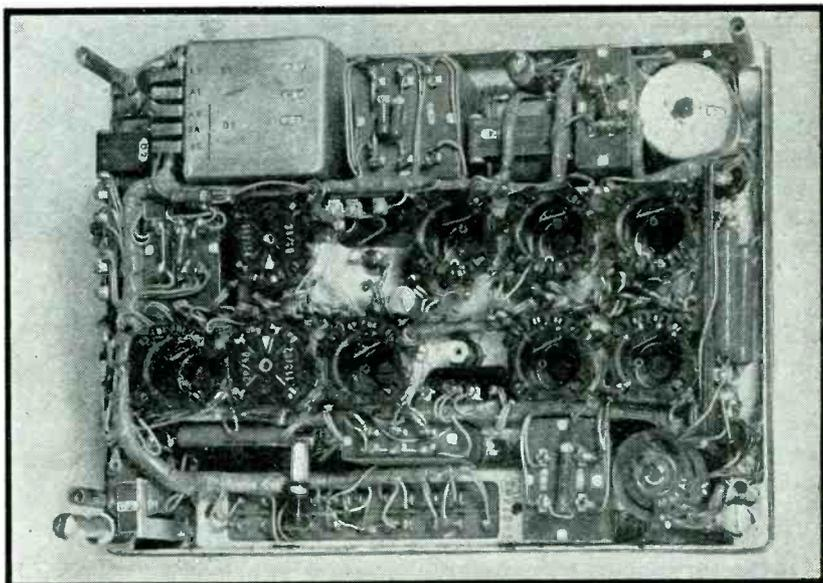
FIG. 4—Intercom amplifier, shown with tubes removed
