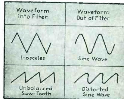
FIG. 8—A graphic illustration of saw-tooth wave transformation by use of RC filters designed for wide-range operation. This indicates the importance of keeping the input waveform isosceles in shape
