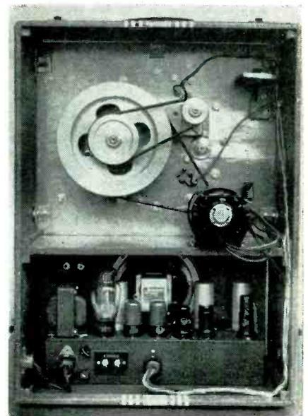
Rear view of the cellophane tape recorder shows the electronic equipment and speaker, at the bottom of the case, and the motor drive mechanism that feeds the tape through the machine
