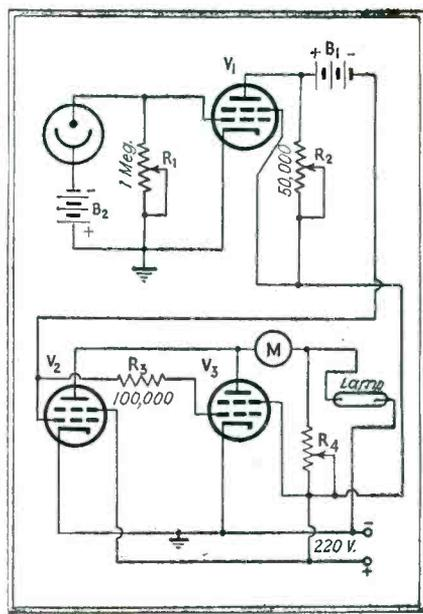
Circuit of electronic method of obtaining constant illumination. Variation of light causes the phototube and amplifier to change the current through the lamp instantaneously
