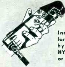
Indent connections on larger cable are made with hydraulic or pneumatic HYPRESSES, either portable or bench type.
