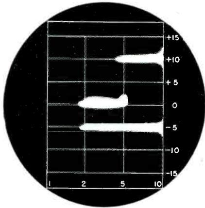
This vertical separation indicator shows a pilot the vertical distance between his plane and others within a fixed radius. A rough indication of the horizontal separation is also provided by the scale
