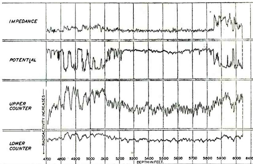
FIG. 1—Comparison of gamma-ray (two lower curves) and electrical logs made in an uncased well
