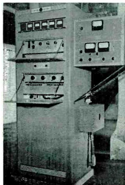
The 25-watt General Electric 337-Mc i-m relay transmitter. Equipment extending from the right side includes frequency and modulation monitors and remote control apparatus
