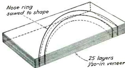
FIG. 1—Curved wood aircraft parts such as nose rings are formed by sawing the required shapes from a thick slab of plywood as shown.
