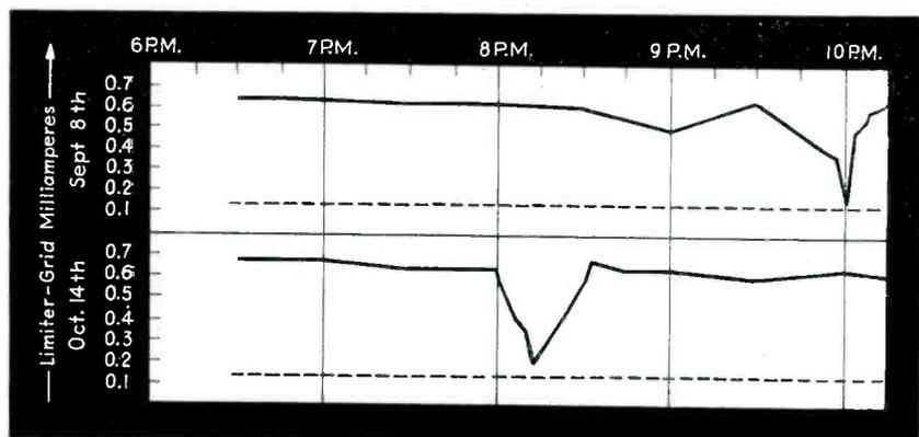
Graphs showing effect of tropospheric fading on two occasions during 1943. Eastern War Time is indicated. Dotted lines indicate limiter-grid no-signal current
