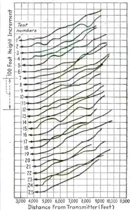
Fig. 1—Flight paths of 25 blind landings. Each curve represents a separate approach and all curves extend through contact
