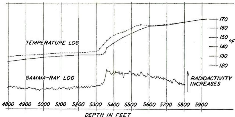
FIG. 4—Comparison of temperature log and gamma-ray curve in a well containing activated cement
