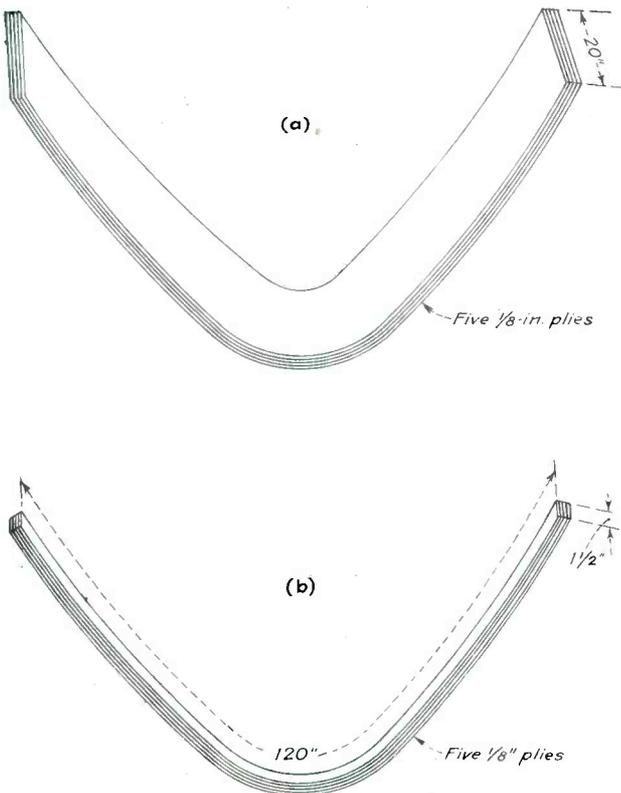
FIG. 5 (left)—Sketch showing makeup of the fuselage ring section shown in Fig. 4. A wide piece of curved-laminated board (a) is formed, and sections (b) are then sawed to required width
