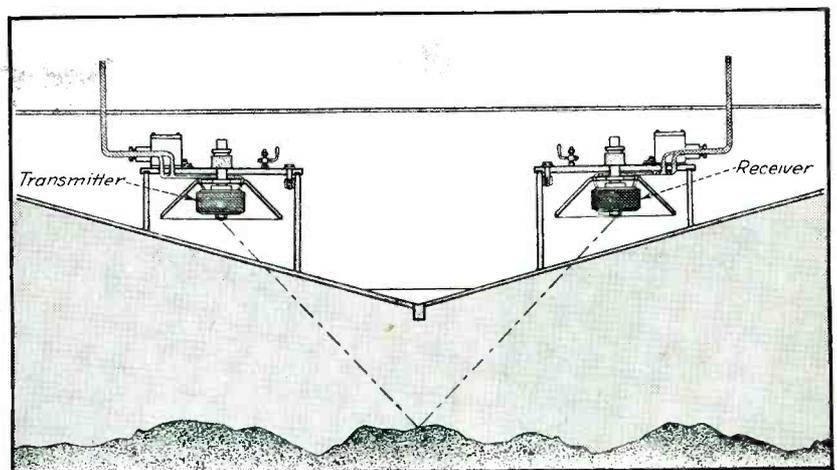
Echo sounding is one important application of supersonic waves. A typical arrangement in a boat is shown here; the transmitter mounted against the hull inside the ship sends supersonic waves down to the ocean bottom, and the receiver picks up the reflected waves. Electronic equipment plots depth on moving tape as ship moves. (From "Precision Echo Sounding and Surveying")
