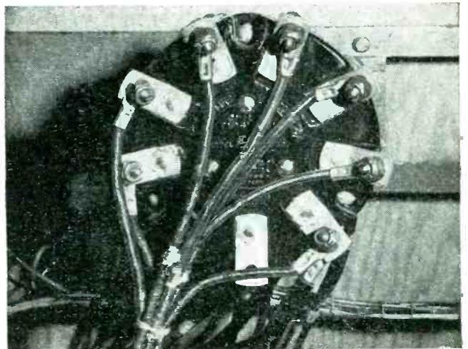
Indent connections are used on rotary switches of all sizes; Burndy Indent connectors being available for all wire sizes from #29 up through the larger cable sizes.
