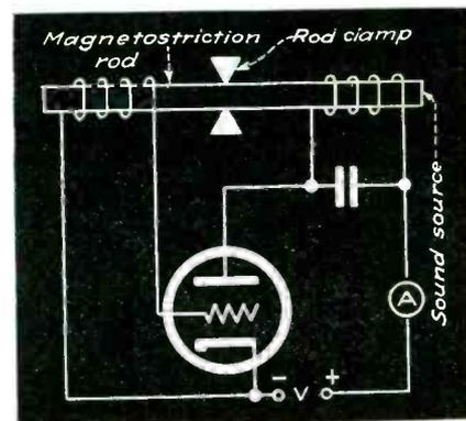
FIG. 3—Magnetostriction generator circuit for producing supersonic waves
