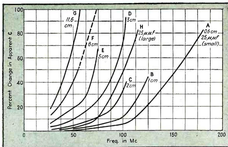
**FIG. 2—Percent changes in apparent capacitance with frequency for a midget 25- $\mu\text{mf}$  capacitor (A) and a 25- $\mu\text{mf}$  unit with physical dimensions twice as large (B). These curves are based on data in Table III. Curves A to G show percent changes in apparent capacitance with frequency for a 25- $\mu\text{mf}$  midget capacitor used with leads from 0.6 to 11.6 cm long, as given in Table IV**
