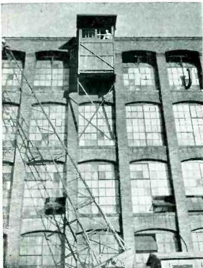
To test radio apparatus under high centrifugal and tangential forces, such as are encountered by equipment used in the crow's nest of a ship, Westinghouse engineers use this pivoted 50-foot steel mast. It swings 45 deg both sides of vertical, making a round trip every six seconds. A 35-hp variable-speed motor with an oil-well reduction-gear and crank supplies the power
