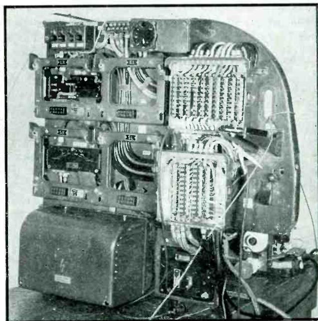
FIG. 2—Panel with the plug-in units removed
