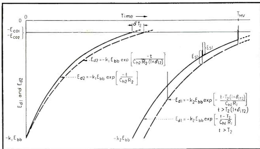
Fig. 3.2—Synchronizing voltage supplied to only one tube. Since  $T_{MV}$  must remain constant, the ratio  $T_2/T_1$  will vary with changes in the characteristics of the uncontrolled section. It is not necessary that  $k_1E_{bb} = k_2E_{bb}$  as it does in this figure
