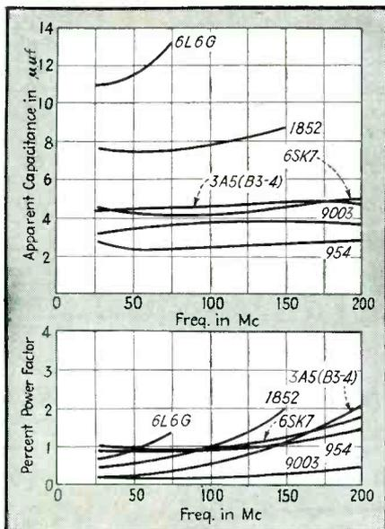
FIG. 4—Curves showing power factor in percent and apparent capacitance for six types of vacuum tubes in Table VI
