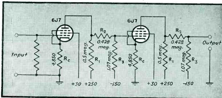
Fig. 3—A two-stage d-c amplifier using pentode tubes
