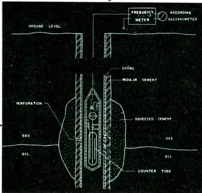
Gamma-ray counter used to detect squeezed cement
