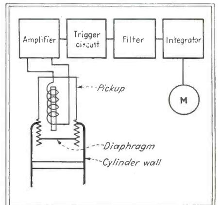
Fig. 2—Cross-section view of pressure-operated pickup in engine cylinder and block diagram of electronic stages in the direct reading octane rating indicator
