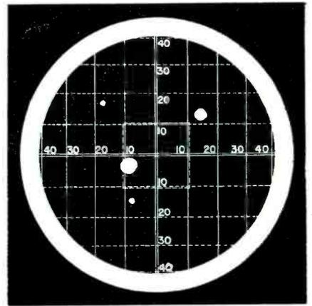
Horizontal separation indicator for aircraft. The dots indicate the relative position of nearby planes, while the size of the dots shows approximate distance from the observer
