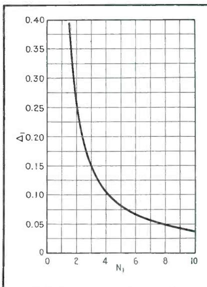
Fig. 4.6—Curve of  $\Delta_1 = \exp [-(N_1-1)/f_s C_{h1} R_1] - \exp [-N_1/f_s C_{h1} R_1]$  vs.  $N_1$  using the maximizing values of  $N_1/f_s C_{h1} R_1$  as given in Fig. 4.7
