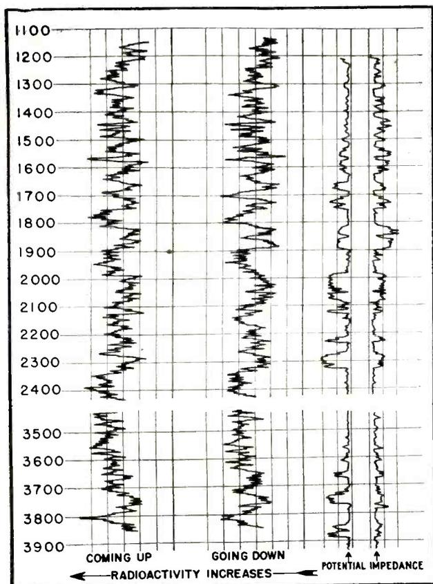
FIG. 2—Comparison of electrical logs in an uncased well with gamma-ray logs made in same well after casing
