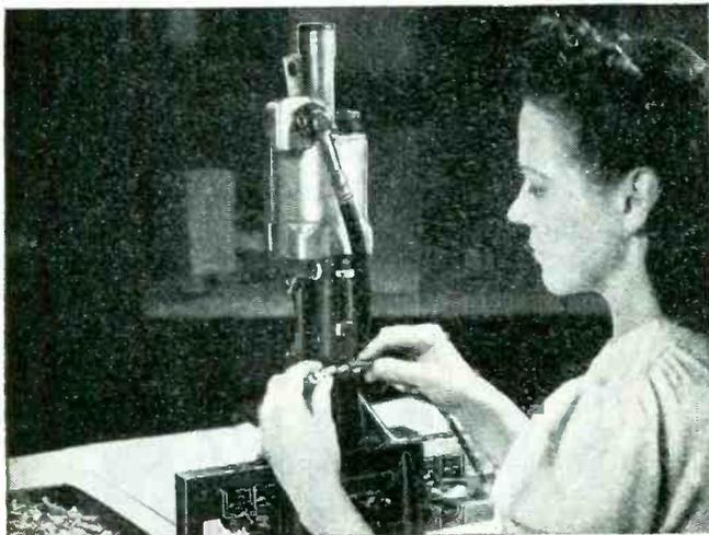
This automatic Burndy HYPRESS indents connectors as fast as the operator can press the trigger. Used extensively by aircraft and electrical manufacturers producing harnesses or leads in large quantities.
