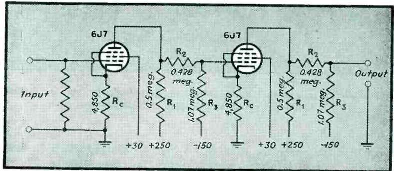
Fig. 3—A two-stage d-c amplifier using pentode tubes
