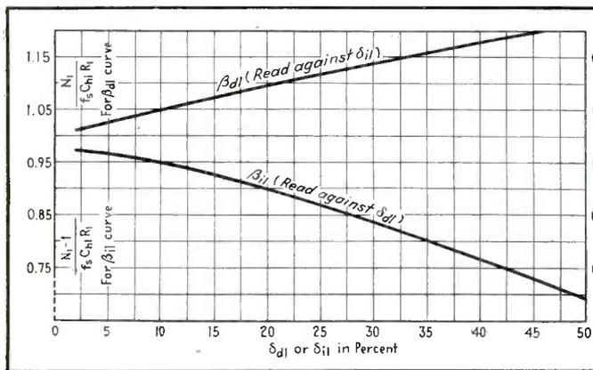
Fig. 4.1—Value of  $N_1/I_c C_{h1}R_1$  that maximizes  $\beta_{d1}$  or  $\beta_{i1}$  as a function of  $\delta_{d1}$  and  $\delta_{i1}$ . Multiply the ordinate by  $N_1/(N_1-1)$  to obtain  $N_1/I_c C_{h1}R_1$  for the  $\beta_{i1}$  curve
