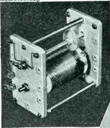
B & W offers a wealth of experience backed with highly specialized facilities for the production of special rotary coils. Above is a typical unit made to exacting war equipment specifications.
