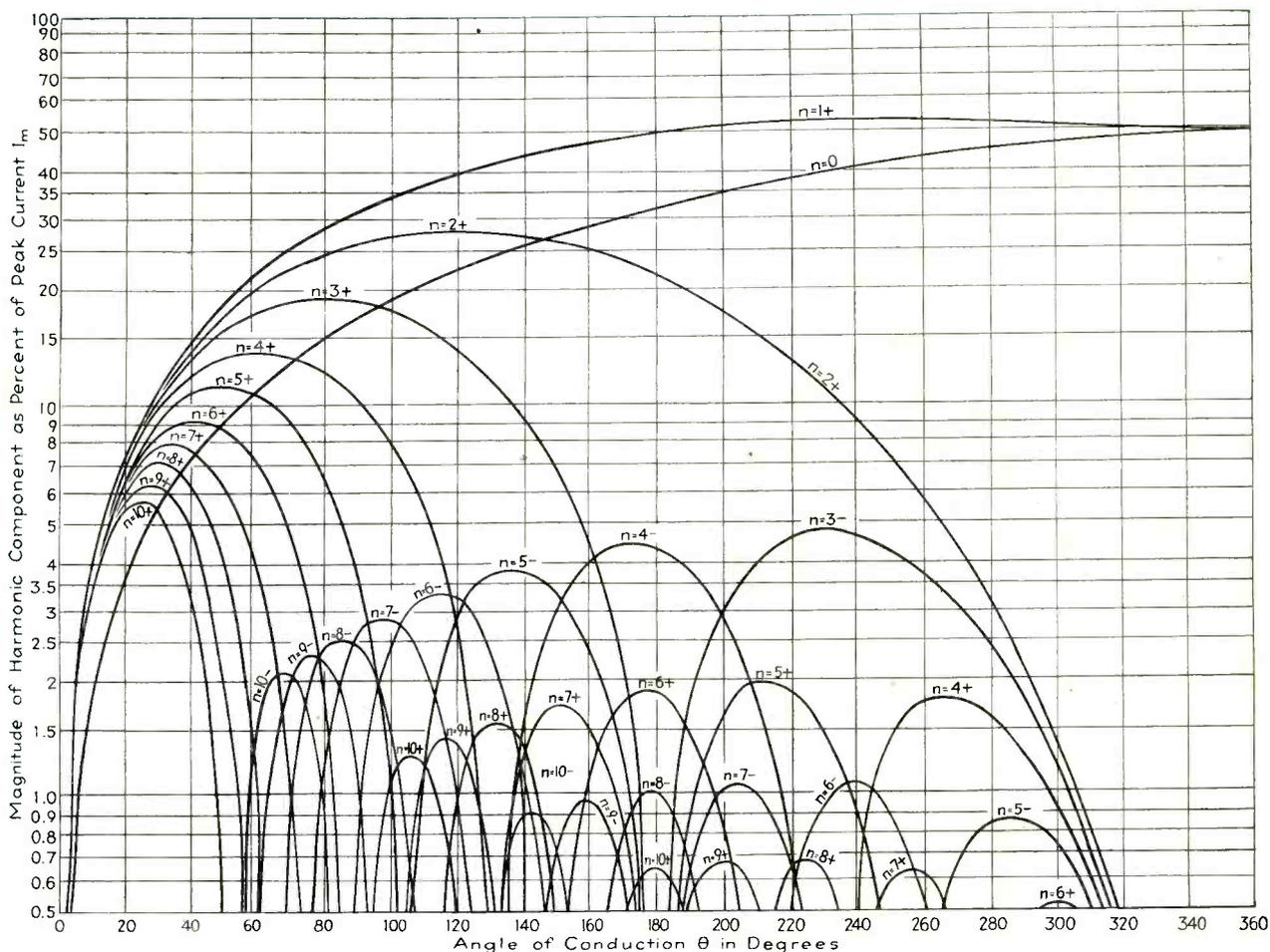
FIG. 2—Graph illustrating the magnitude and phase of the first ten harmonics of an overbiased amplifier. The harmonic amplitudes are expressed in percentages of the peak current, for various conducting angles in degrees
