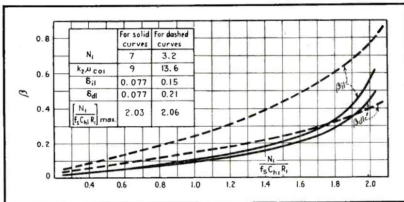
Fig. 4.4—Percentage variation permissible in the amplitude of the synchronizing pulse as a function of  $N_1/f_s C_{h1} R_1$  for the MV's designed in Examples III and IV
