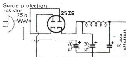
Two forms of voltage-doubling circuits using condenser networks having common negative leads. One is for two half-wave rectifiers, and the other for double-diode rectifiers like the 25Z5
