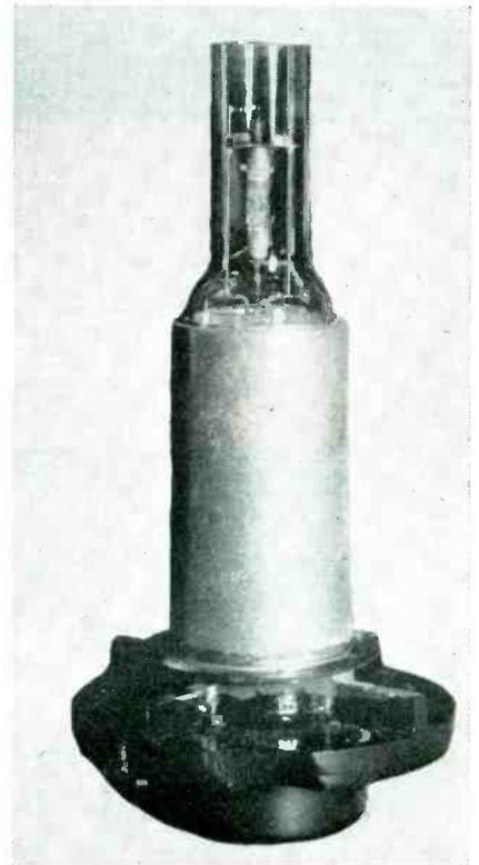
Mercury vapor lamp assembly as used in a typical motion picture printer at Paramount Pictures, Inc. for making release prints
