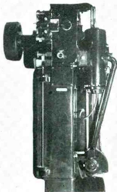
This motion picture printing machine contains a mercury vapor lamp at upper right and a motor blower for illumination control at lower right. The cylindrical pipe connects the two units
