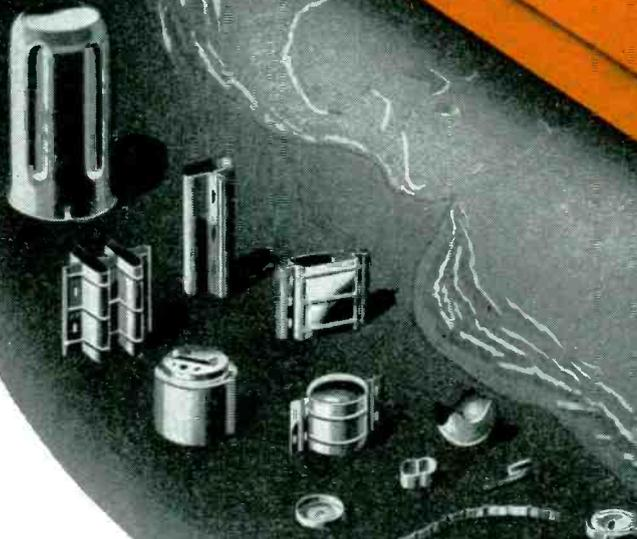
Typical electronic tube parts you'll find in GOAT boxes that have been stamped, drawn and formed on GOAT machines, dies and presses.
