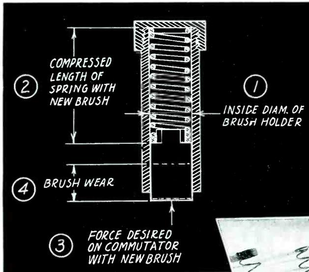
Instrument Specialties engineers have devised a simplified design procedure for determining the best brush spring to do a specific job; based upon only four brush-holder design details:
