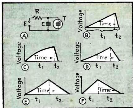
FIG. 1—Characteristics of a typical relaxation oscillator consisting of a potential source  $E$ , a limiting resistor  $R$ , a capacitance  $C$ , and a gaseous discharge tube  $T$ . The curves illustrate various charging,  $t_1$ , and discharging,  $t_2$ , conditions
