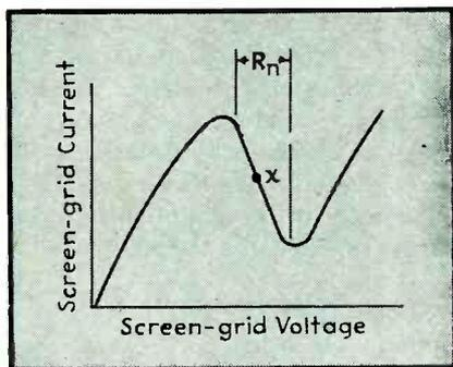
FIG. 3—Typical negative resistance curve of transitron oscillator.  $R_n$  is the negative resistance portion of the screen characteristic, where an increase in screen voltage gives a decrease in screen current
