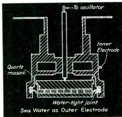
FIG. 2—Langevin quartz supersonic source for underwater signalling
