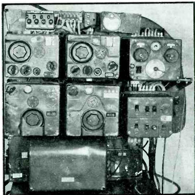
FIG. 1—The FUG-10 panel with all units in place
