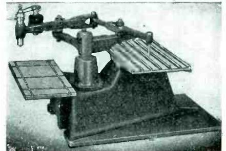
It can also be used to drill a series of holes, profile small parts, etch glass or to cut an even channel for wiring on panels. Model Nos. 100 and 200 are priced at \$850 and \$600 respectively.
