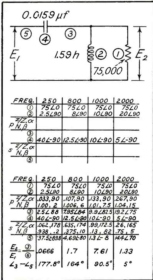
FIG. 3—Circuit for Example II in text, and tabulated solution for four different frequencies. Impedances are numbered in the order of their appearance in the solution
