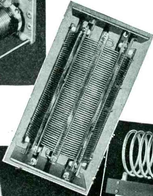
20" long, and wound with #8 solid wire, this B & W Air Inductor carries a conservative continuous rating of 7.5 amps. Aside from special bracing, however, it is simply a "grown up" version of B & W Junior Coils of amateur radio fame.
