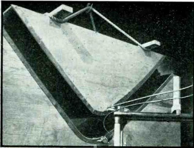
FIG. 8—Photograph of the male and female forms used to make fuselage ring section, with r-f connections in place
