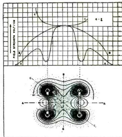
**Fig. 3—Field strength between two circular plates of different size**
