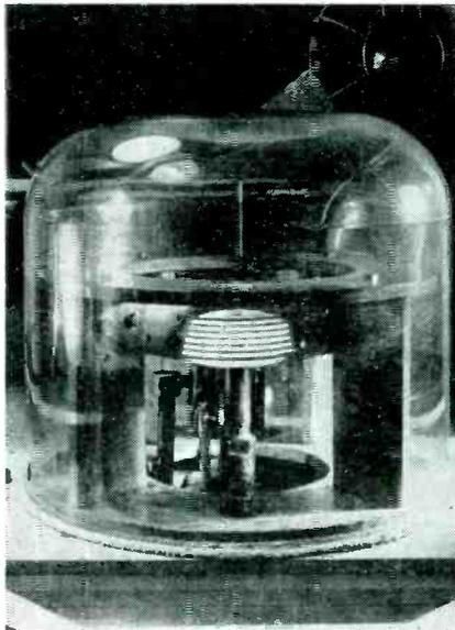
A red hot rock bit for drilling oil wells is hardened in an experimental induction furnace. Tungsten carbide, held in place by an adhesive coating, is deposited on the teeth of the bit under the high heat
