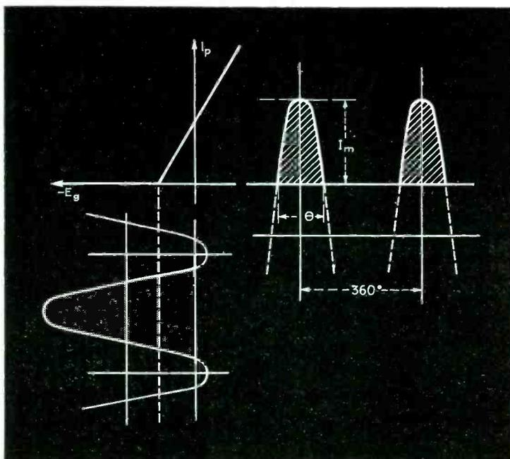
FIG. 1—Diagram illustrating the idealized linear amplifier characteristics on which the main graph in Fig. 2 is based
