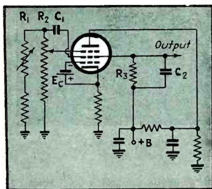
FIG. 2—Basic transitron oscillator circuit.  $R_1$  is the frequency adjustment,  $R_2$  the feedback adjustment, and  $C_1$  the feedback capacitor;  $R_3$  and  $C_2$  are screen grid resonant circuit components.  $E_0$  is the grid bias used to produce sine waves
