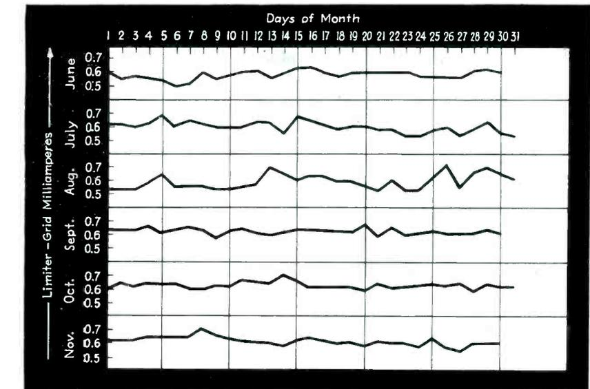
Graphs showing signal received at Clingman's Peak from the 25-watt, 337-Mc 1-m relay transmitter W4XGG at the Winston-Salem studios. Readings were all taken in 1943. Limiter-grid current of 0.5 ma indicates 100  $\mu$ v input
