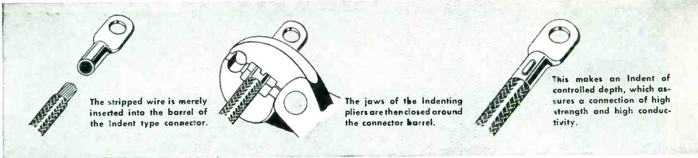
The stripped wire is merely inserted into the barrel of the Indent type connector.
