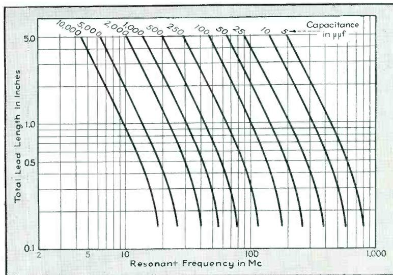
The chart gives lead lengths and capacitance values for series resonance at any frequency from 5 to 800 Mc, for postage-stamp mica by-pass capacitors with No. 20 tinned copper leads
