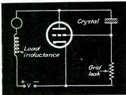
FIG. 1—Simple circuit for driving a quartz crystal serving as a supersonic source of sound
