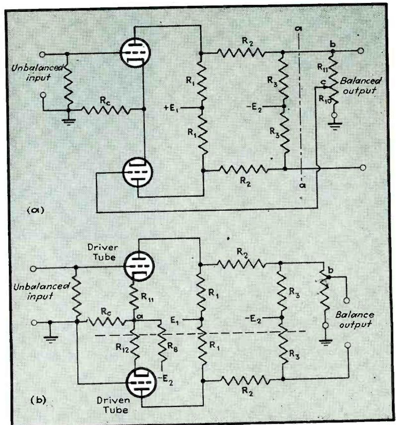
Fig. 6—Two types of d-c phase inverters. The tubes can be either triodes or pentodes in the circuit at (a)
