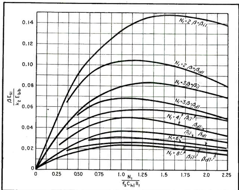
Fig. 4.3—Increase and decrease permissible in the amplitude of the synchronizing pulse for various orders of division as a function of  $N_1/f_s C_M R_1$ . These curves are applicable only in the special case of  $\delta_{s1} = \delta_{i1} = 1/(2N - 1)$
