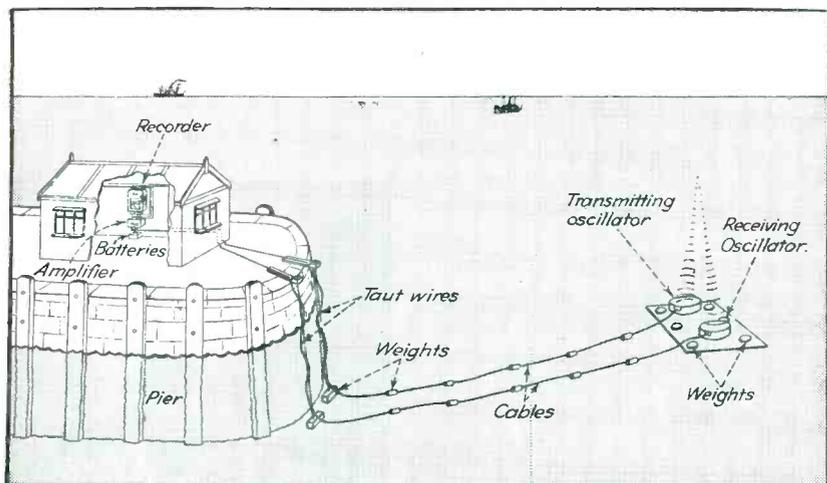
This schematic diagram of a harbor tide-recorder is an interesting practical supersonic application. (From "Precision Echo Sounding and Surveying", by Lt. Commander D. H. Macmillan, Henry Hughes & Son, Ltd, 59, Fenchurch St., E.C. 3, London). Both oscillators are on ocean bottom
