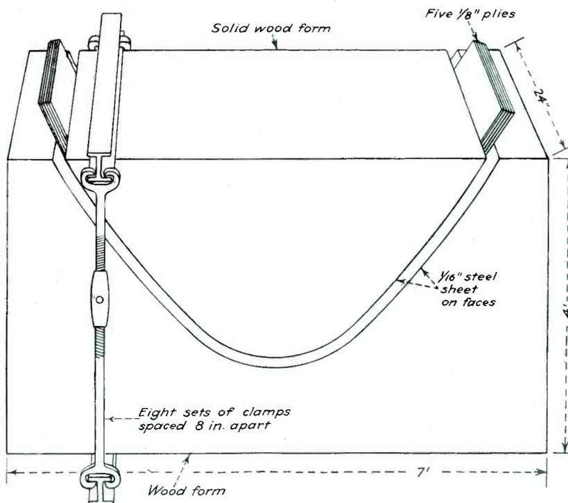
FIG. 7—Arrangement of male and female forms for making the laminated section shown in Fig. 5. Pressure is applied by means of a large number of hand-clamps. Radio-frequency heating is applied by utilizing the steel face plates of the forms as electrodes
