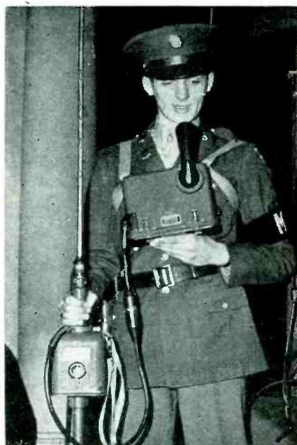
Originally designed for cavalymen, with the bottom of the antenna fitting into a saddle boot, this guidon radio is also used by other troops on the ground or on the bumper of an army vehicle
