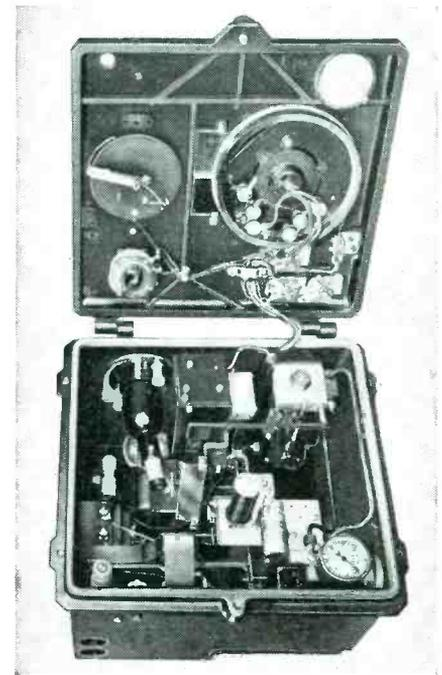
able "dead zone", high sensitivity and adjustment to very low sensitivity, no mechanical connection between galvanometer and pneumatic circuit, and simple load error adjustment.
