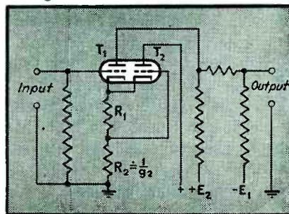
FIG. 8—The basic Miller circuit which improves the drift problem of the input stage of the d-c amplifier. If  $g_2$  is the transconductance of  $T_2$ , then  $R_2$  is nearly equal to  $1/g_2$ .
