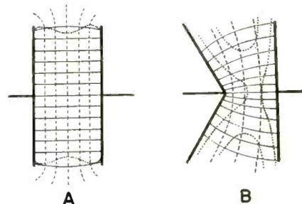
Fig. 1—Homogenous and nonhomogeneous fields. Force lines are shown solid, equipotential lines dashed, and iso-field strength lines dotted
