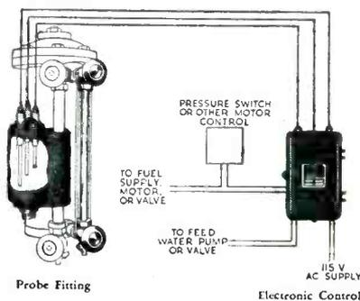
Typical FIREEYE Installation For Automatic Boiler Feedwater Control And Low-Level Safeguard
