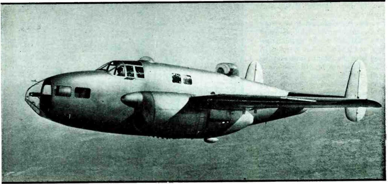
The Fairchild AT-21 Gunner Crew Trainer, a "plastic plywood" plane of the type referred to in this article. The only metal used in its construction is in the engines, the engine supports, instruments and certain other equipment, supports and controls
