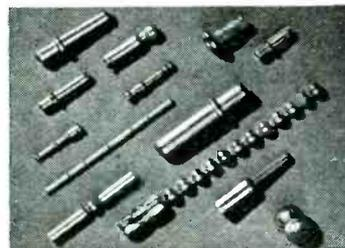
*These are typical "Multi-Swage" products. This process will turn out large volume speedily while maintaining close tolerances accurately.*
