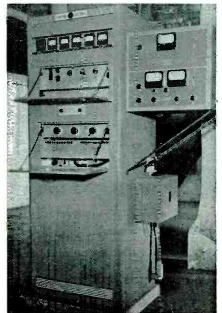
The 25-watt General Electric 337-Mc i-m relay transmitter. Equipment extending from the right side includes frequency and modulation monitors and remote control apparatus
