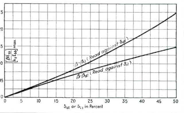
Fig. 4.2—Maximum number of volts increase and decrease permissible in the amplitude of the synchronizing pulse vs.  $\delta_{d1}$  and  $\delta_{i1}$ . The maximizing values of Fig. 4.1 were used
