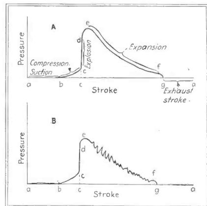
Fig. 1-(A)—Curve of an Otto cycle for an ideal gasoline engine. (B)—The portion of the curve during the expansion period (from *e* to *f*) actually contains high-frequency oscillations of about 6,500 cps
