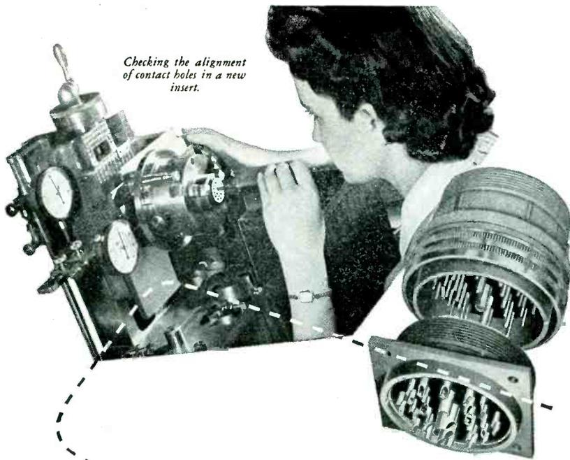
Checking the alignment of contact holes in a new insert.
