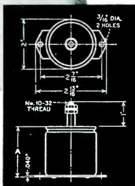
Type 1860 (see photo and above drawing) has suitably plated brass terminal mounted in mica insulating plate. Dimension A is from 2 to 3 1/2"
