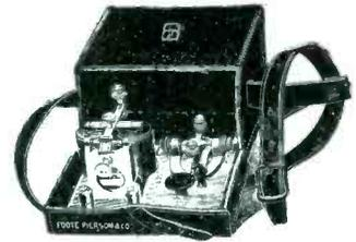
Main line telegraph combination set as supplied to the Signal Corps in 1898
