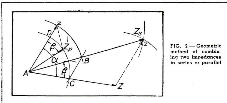
FIG. 2 — Geometric method of combining two impedances in series or parallel
