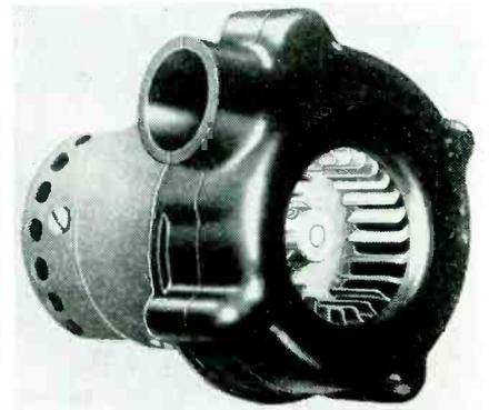
Running at 7200 rpm, the blower circulates 22 cu ft per min continuously. The motor is designed for use in ambient temperatures up to 80 deg C. Overall length of the unit is 4 1/2 in.; weight 19 1/2 oz.
