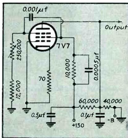
FIG. 5—Practical transitron oscillator circuit for production of sawtooth waves between 7 and 26 kc
