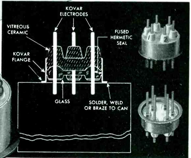
**H**ERMETIC transformer or capacitor seals of Kovar and glass may be made in a wide size range and with single or multiple electrodes. Electrodes may be solid or tubular.
