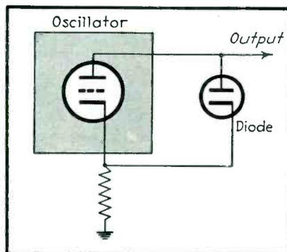
FIG. 6—Automatic amplitude control of this transitron oscillator is used to compensate for a falling off in output voltage
