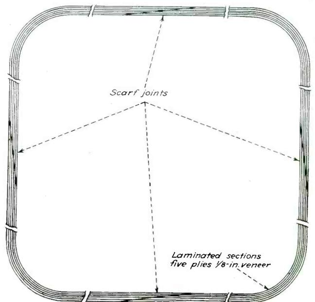
as shown in Fig. 3 would have greater strength, would be lighter and, once the fixtures were developed, would be cheaper to make. Since these parts are made in tens or even hundreds of thousands, the work necessary to develop a production setup would be amply justified. Several radio cabinet manufacturers have already investigated this field.
