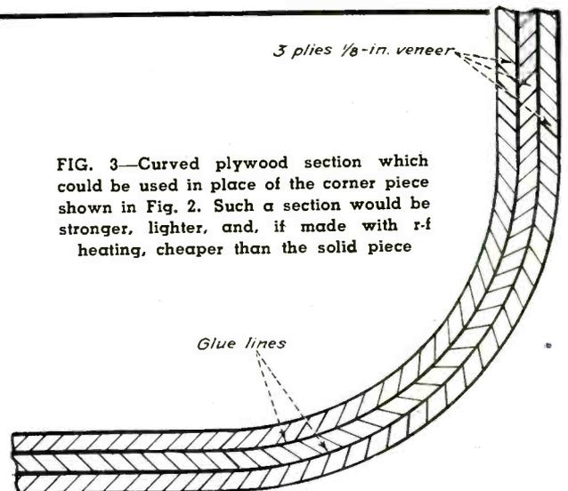
FIG. 3—Curved plywood section which could be used in place of the corner piece shown in Fig. 2. Such a section would be stronger, lighter, and, if made with r-f heating, cheaper than the solid piece
