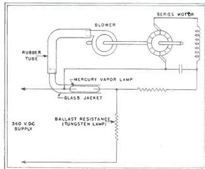
Circuit for maintaining constant illumination by blowing more air around a mercury vapor lamp when the line voltage rises and less air when it decreases
