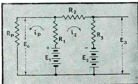
Fig. 1—Basic bridge circuit, and bridge version used for interstage coupling
