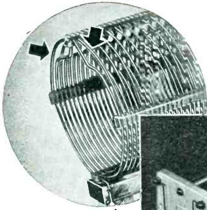
Indents are a special optional feature of B & W "Air Wound" construction on small, closely wound coils. Windings on either side of every turn of wire are indented, thus making tapping quick and easy, anywhere on the inductor.
