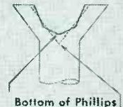
Bottom of Phillips Recess is nearly flat... NOT tapered to a sharp point.
