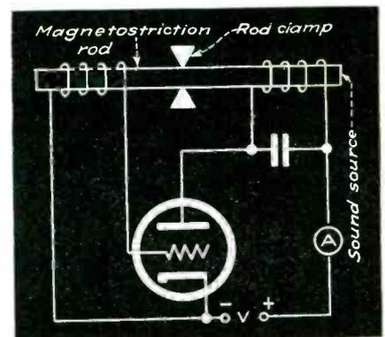
FIG. 3—Magnetostriction generator circuit for producing supersonic waves
