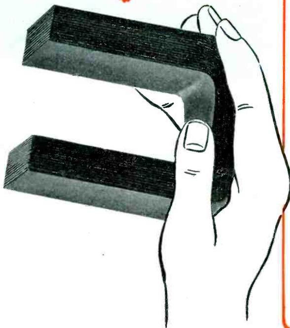
Now you can eliminate the time-consuming operation of stacking hundreds of tissue-thin core laminations by hand for High-Frequency Communications Equipment. Pre-assembled Type C HIPERSIL cores are delivered to you in just TWO ready-to-assemble pieces per loop: Westinghouse winds a thin strip of HIPERSIL to form, bonds it, then cuts it in two.
