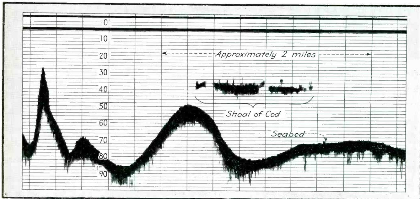
Example of supersonic depth record obtained on a ship. Such objects as fish above the ocean bottom give indications also, making the equipment of great value to deep-sea fishing boats
