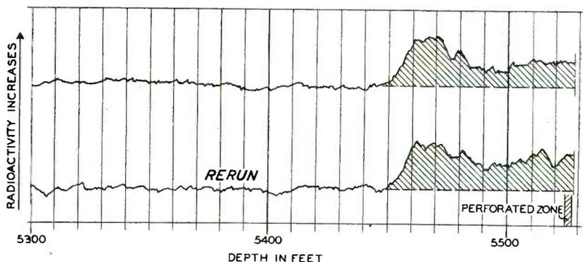
FIG. 5—Gamma-ray curves obtained when using radioactive "squeezed cement." The extent the cement traveled is clearly shown
