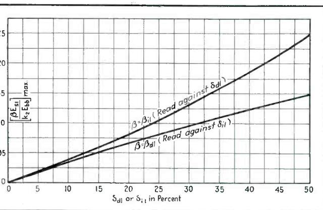
Fig. 4.2—Maximum number of volts increase and decrease permissible in the amplitude of the synchronizing pulse vs.  $\delta_{d1}$  and  $\delta_{i1}$ . The maximizing values of Fig. 4.1 were used
