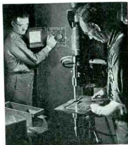
Spot-welding two .062-inch thick pieces of aluminum with 48,000 amperes of current. The ignitron welding control in the background allows the current to flow for eight cycles in this application and permits adjustment for spot-welding various other thicknesses of metal
