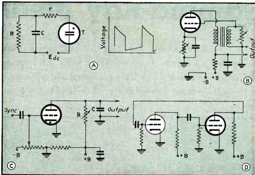
A—Direct voltage produces ionization in *T*, charging *C* through *r*. Voltage across *C* builds up, with an accompanying decrease across *T*, until ionization can no longer be sustained and *C* is discharged through *R*, after which the circuit conditions are returned to their initial state, and the sequence repeats
