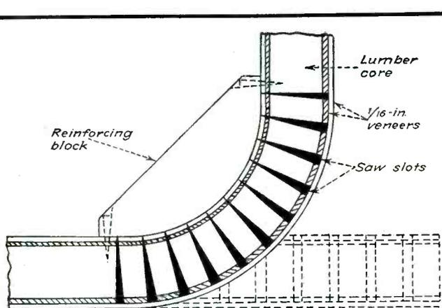
FIG. 2—Corner of a table model radio set made by the process of slotting, steaming and bending as now used
