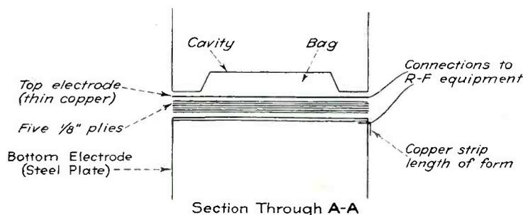
Fig. 11—Sketch of the arrangement used to obtain "flexible" pressure on one side of the laminated assembly. A rubber bag which occupies a cavity in the upper form is inflated to 75 psi after the clamps are applied. Using a thin copper sheet for the upper electrode gives an approximation of "fluid" pressure
