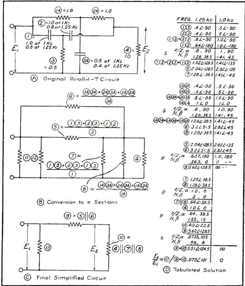
FIG. 4—Original circuit and steps in simplifying it for Example III in text, with complete tabulated solution for two different frequencies. An orderly compilation of data minimizes changes of mistakes and permits checking any part of the work quickly. Impedances are numbered for the same reason
