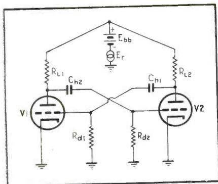
Fig. 4.5—Ripple voltage in the plate power supply is coupled directly into the grid circuit of each tube in the MV
