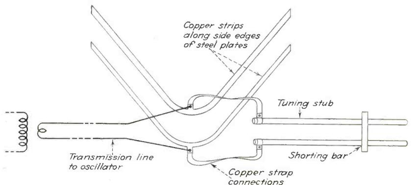
Fig. 10—Schematic illustration of the r-f connections used to feed the forms shown in Fig. 8 and Fig. 9. A tuning stub is used to parallel tune the load
