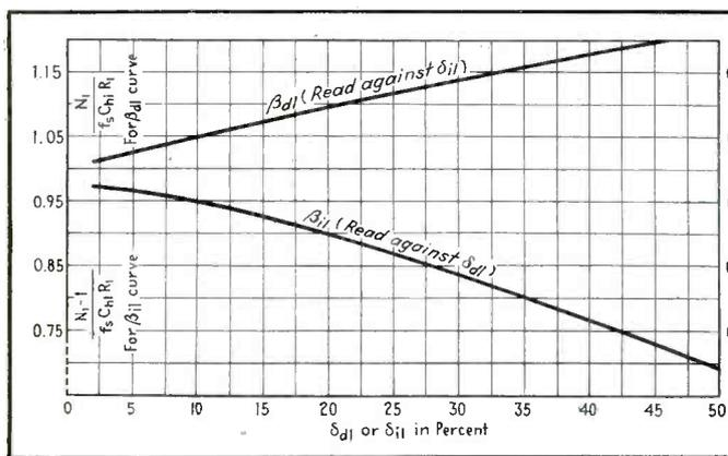
Fig. 4.1—Value of  $N_1/I_c C_{h1}R_1$  that maximizes  $\beta_{d1}$  or  $\beta_{i1}$  as a function of  $\delta_{i1}$  and  $\delta_{d1}$ . Multiply the ordinate by  $N_1/(N_1-1)$  to obtain  $N_1/I_c C_{h1}R_1$  for the  $\beta_{i1}$  curve
