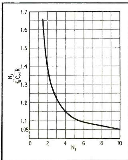
Fig. 4.7—The value of  $N_1/I_2 C_{n1} R_1$  given by this curve maximizes the increase in the exponential grid voltage between the  $(N_1-1)$ th and the  $N_1$ th synchronizing pulses
