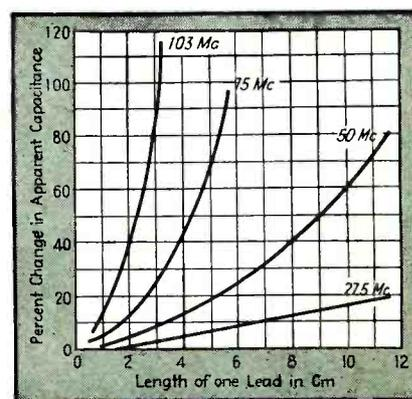
**FIG. 3—Curves for four frequencies of Table IV, showing percent change in apparent capacitance for different capacitor length leads**
