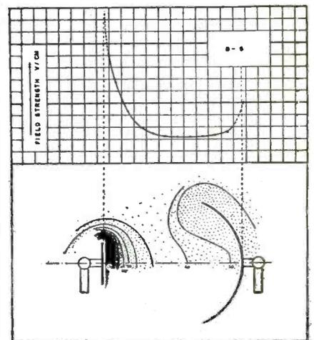
Fig. 5—A cylindrically curved electrode produces this field form
