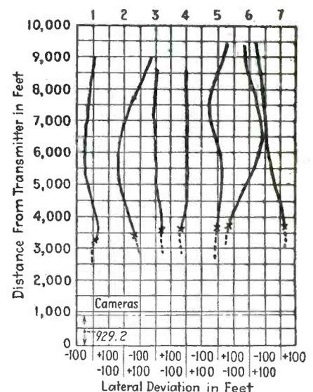
Fig. 2—Several curves of approach paths, showing lateral deviation from the runway centerline. Points marked X indicate contact of the plane to ground and dotted portions of the curves represent taxiing paths after contact
