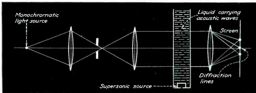
FIG. 5—Arrangement for obtaining diffraction patterns from light that has passed through a liquid carrying supersonic waves
