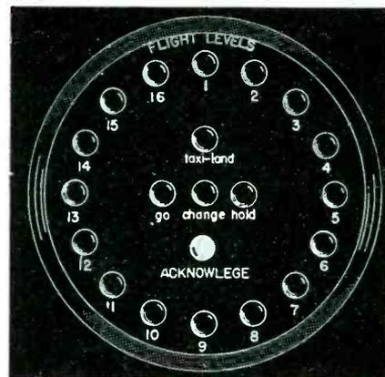
The traffic clearance indicator contains a number of lamps around its circumference to indicate the various flight levels on which the plane is directed to fly by the ground station. The indicators in the center of the dial authorize movement of the plane on the ground as well as landings and take-offs
