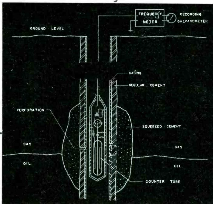
Gamma-ray counter used to detect squeezed cement
