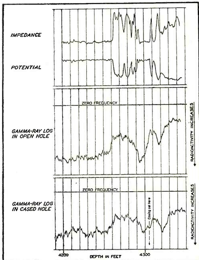
FIG. 3—Detailed logs made in a producing section of a well, electrically, and electronically in open and cased holes
