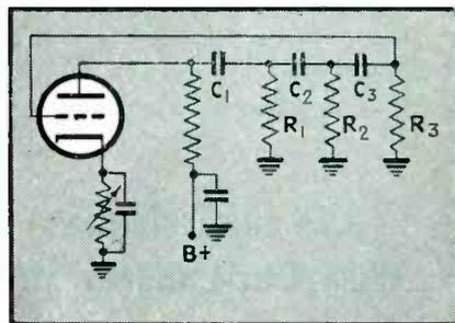
FIG. 7—Usual method of operation of this phase shift oscillator over a frequency range is to make  $C_1$ ,  $C_2$ , and  $C_3$  variable and ganged, while  $R_1$ ,  $R_2$ , and  $R_3$  are switched in steps to change ranges
