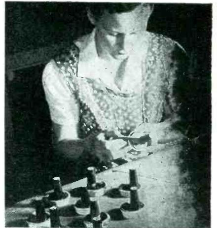
Checking dimensions of Prestite insulator used for terminal posts on capacitors for aircraft equipment to prevent flashover at high altitudes. The insulator, a Westinghouse product, holds up at altitudes of 60,000 feet and resists temperature changes from 234 deg. above zero to 15 deg. below. The insulating material is a mixture of clay, feldspar, and flint and can be solder-sealed to metal shield cans
