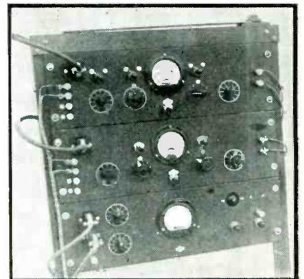
Electronic surface equipment used in conjunction with gamma-ray detector employing two counter tubes
