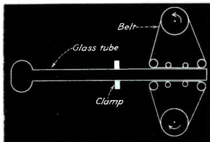
FIG. 4—Holtzmann's ultrasonic generator using two moving belts
