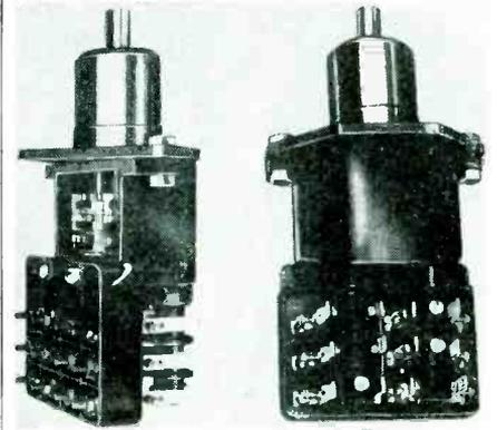
struction providing easily accessible terminals. Contacts are double break, self cleaning due to wiping action, and of silver. Rated for voltage up to 550 ac or dc.
