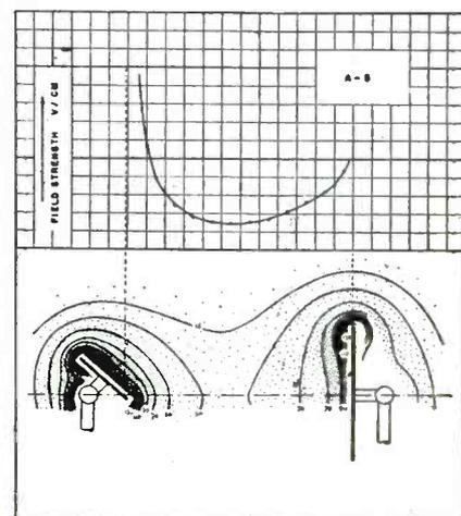
Fig. 4—Effect of change in position of one of the electrodes of Fig. 3
