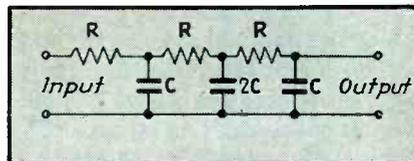
FIG. 4—Low-pass filter for converting isosceles waves of 10 to 20 kc to sine waves.  $R = 50,000$  and  $C = 0.001 \mu f$
