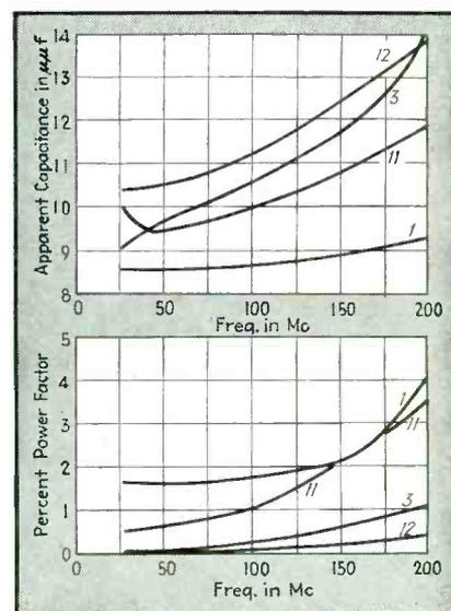
FIG. 1—Curves showing how power factor and apparent capacitance change with frequency for four of the small capacitors for which VHF data is given in Table II
