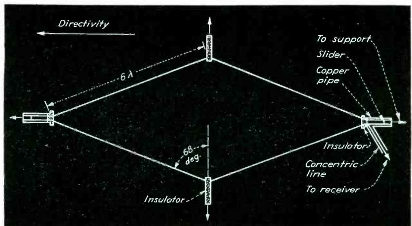
Rhombic receiving antenna. Theoretical signal gain is 11.5 db, theoretical directivity gain 15.8 db
