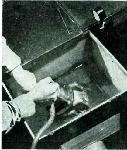
The waterproof design was evolved through use of a labyrinth-type seal having appropriate traps and drains.
