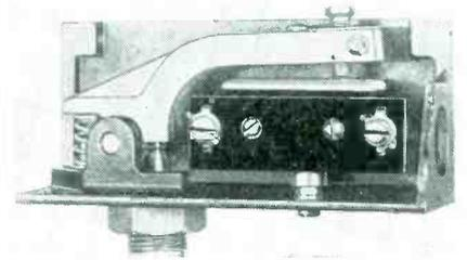
Locking-screw locks temperature setting. Terminal plate has large screw terminals. Snap-action micro-switch eliminates contact troubles. Range 0-1400 deg F. Adjustable range 200-300 deg F. Dimensions are 5½ by 1¾ by 3 in.
