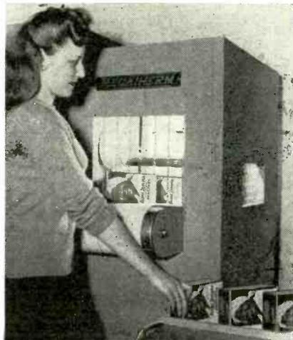
A continuous belt has been added to this Megatherm electronic heating unit, made by Federal Tel. & Radio Corp., for conveying packages of food products between metal plates for dielectric heating to provide sterilization
