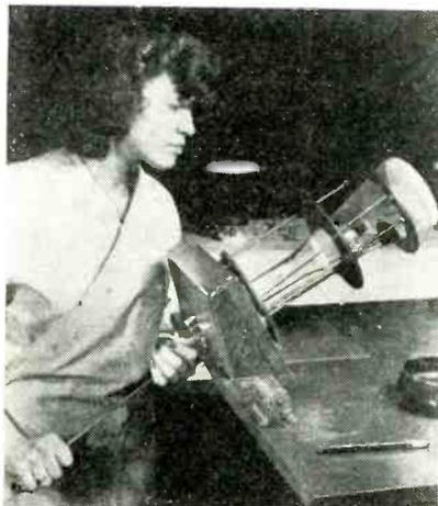
Glass bulbs for cathode-ray tubes are rotated in this jig at a constant speed while the operator moves a brush containing Aquadag up and down the vertical axis of the tube. The unit is in use at the Dobbs Ferry, N. Y. plant of North American Philips Co., Inc.
