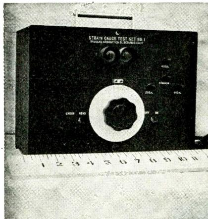
Electronic test set for calibrating strain gages during manufacture. The dial adjusts a potentiometer to balance a bridge circuit and is calibrated in percent tolerance
