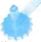
In two quick steps, this little part is made. The head and the shank with projection are upset from Alcoa Aluminum wire in a rivet header. A blanking operation shapes the head, and the part is ready for heat treating.
