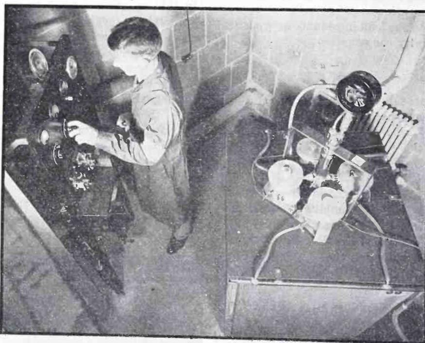
At the right are four evacuable powder cameras in position around the x-ray tube of an x-ray diffraction unit. High-voltage equipment is under the table, enclosed by metal screening. The operator is adjusting the intensity of the x-ray beam. This unit was built in Socony-Vacuum Laboratories about six years ago, but complete and versatile commercial equipment is now available
