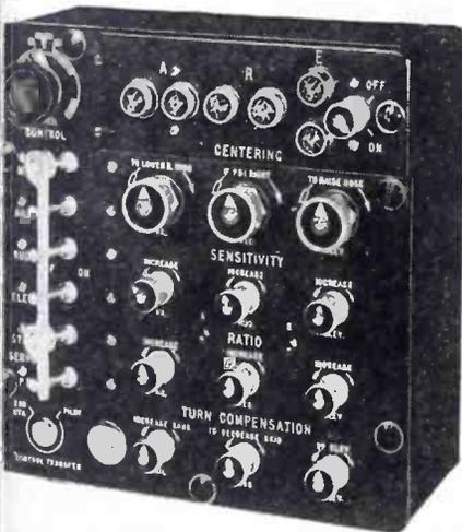
autopilot control panel, mounted within convenient reach of the pilot. With the autopilot in control at any given altitude, the plane can be maneuvered by finger-tip adjustment of the turn-control and elevator knobs or by similar remotely located knobs near the bombardier
