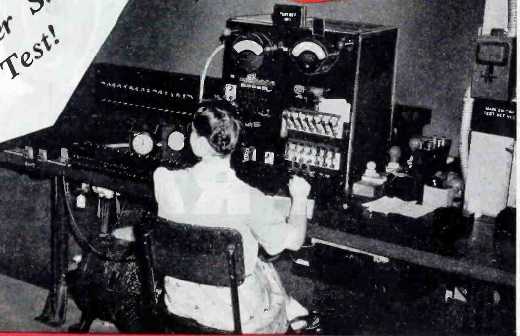
The above photograph shows Heinemann Circuit Breakers on the final time test. Breakers are manufactured with time delays closely matched to customer's specification. Each breaker is tested on at least three points of its time delay curve to insure that the time delay stays within the curve limits specified.
