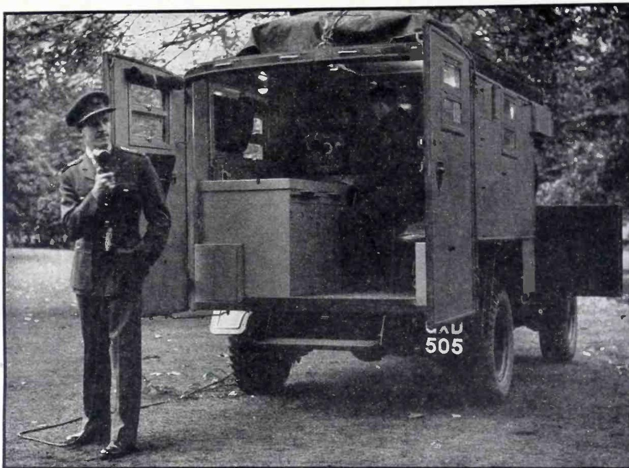
Recording equipment developed by the British Broadcasting Corp. for use at the front is often housed in trucks of this type, which include living facilities, 200 yards of microphone cable, a shortwave receiver and a three-channel mixer
