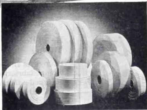
Fiberglas tapes are available in tight and medium weaves, in all widths commonly required for insulating electrical products, in thicknesses of .003", .005", .007", .010" and .015".
