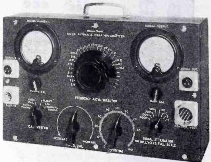
ing the low frequencies, however, the full accuracy of the analyzer is not realized below 5.5 cps.
