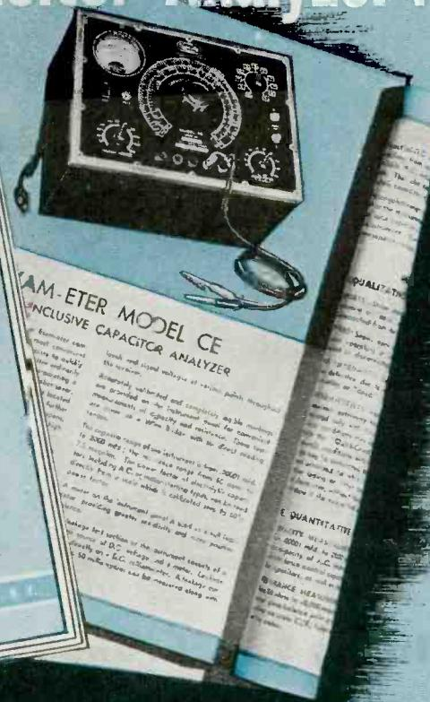
**T**HE SOLAR MODEL CE Capacitor Examiner speedily locates common defects in capacitors without disconnecting condensers—often eliminating further tests. This saving of time and labor is accomplished by the unique Solar "QUICK-CHECK" feature.
