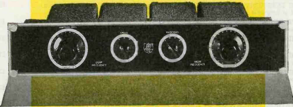
**BAX** . . . THE UNIVERSAL EQUALIZER FOR BROADCAST AND RECORDING SERVICE. PROVIDES ADJUSTABLE EQUALIZATION AT 25, 50, OR 100 CYCLES FOR LOW END, AND AT 4000, 6000, 8000, OR 10,000 CYCLES AT HIGH END. CALIBRATED CONTROLS READ DIRECTLY IN DB EQUALIZATION AND FREQUENCY SETTING. THE INSERTION LOSS EFFECTED BY THE EQUALIZER IS COMPENSATED THROUGH SPECIAL COMPENSATING PADS, SO THAT IT IS CONSTANT REGARDLESS OF SETTING. RAPID CHANGE IN TONE COLOR CAN BE OBTAINED WITH NEGLIGIBLE CHANGE IN VOLUME.
