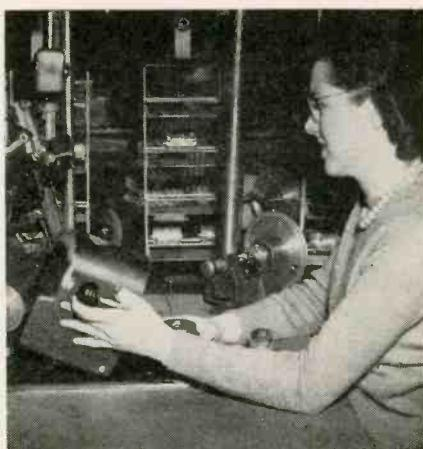
Timing of shell fuses is compared electronically to the ticking of a master electric clock at the Eclipse-Machine division of Bendix Aviation Corp. Called a dynamic regulator, the device plays an important part in production of anti-aircraft shells.
