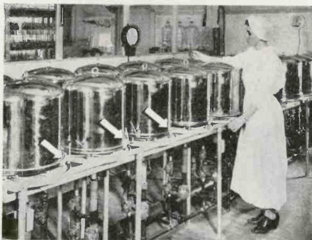
Plasma reduction units depend on THERMOSWITCHES for accurate regulation.
