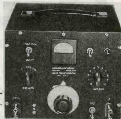
calibrated dial indicates the percentage difference between the unknown and the standard. The comparison bridge is supplied with three frequencies of 60, 1,000 and 10,000 cycles. Components being compared to a similar standard range are: capacitors 25  $\mu\text{f}$  to 20  $\mu\text{f}$ ; inductors 5 microhenries to 500 henries, resistors from 10 ohms to 5 megohms. The instrument measures 10 x 7½ x 8½ in.
