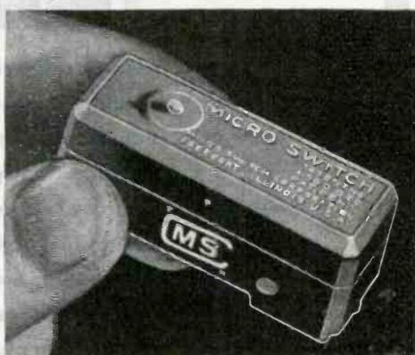
The basic Micro Switch is a thumb-size, feather-light, plastic enclosed, precision, snap-acting switch. Underwriters' listed and rated at 1200 V.A. at 125 to 460 volts a-c. Capacity on d-c depends on load characteristics. Accurate reproducibility of performance is maintained over millions of operations. Basic switches of different characteristics are combined with various actuators and metal housings to meet a wide range of requirements.
