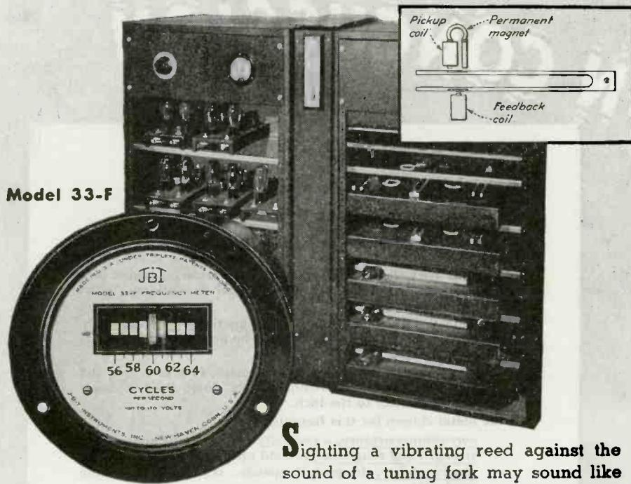
**S**ighting a vibrating reed against the sound of a tuning fork may sound like double talk . . . but that is essentially the principle in the exacting process of J-B-T Frequency Meter calibration.
