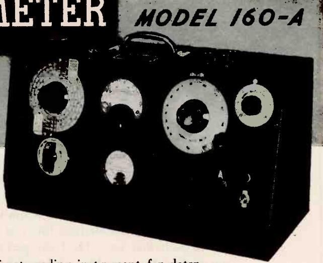
A dependable direct-reading instrument for determining the Q or the ratio of reactance to resistance, of coils. Used in design and production engineering of Radio and Electronic equipment. Condensers and other components readily measurable.
