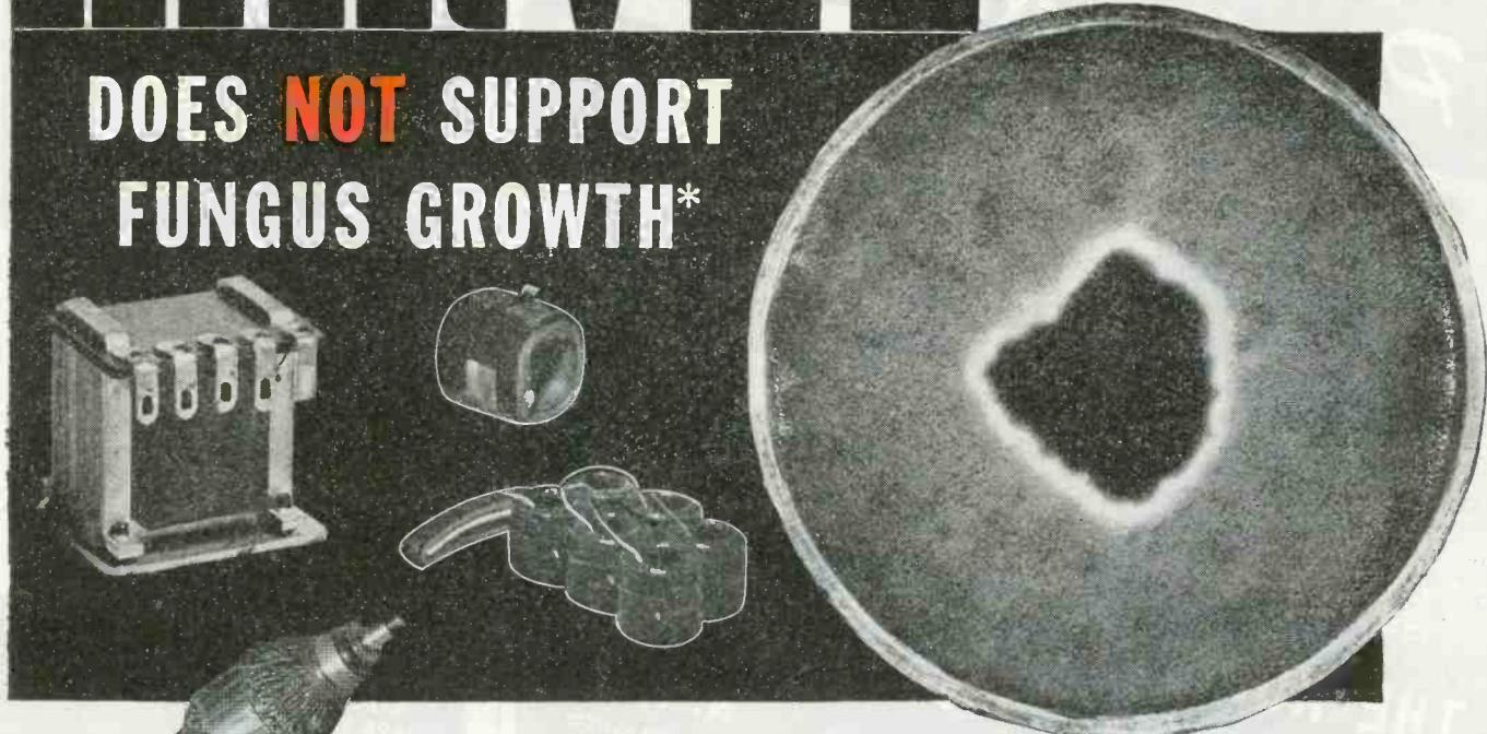
Photograph illustrates the fungus resistance of Harvel 612-C Baking Varnish. Note that the fungus culture of *chaetomium globosum* has not attacked the sample film of Harvel 612-C.
