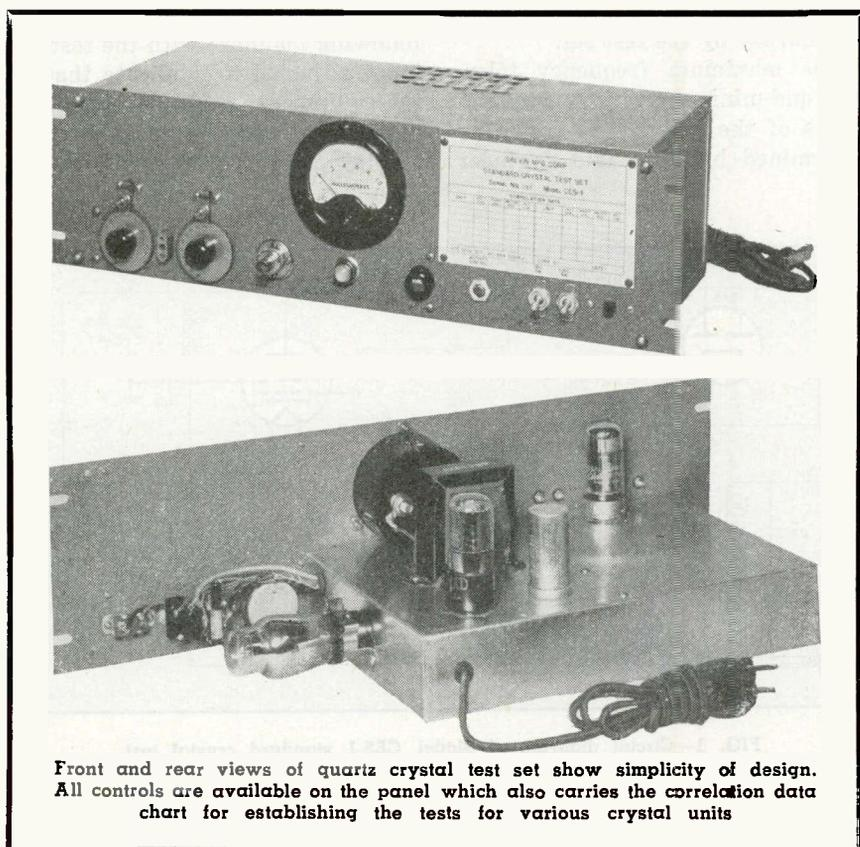
Front and rear views of quartz crystal test set show simplicity of design. All controls are available on the panel which also carries the correlation data chart for establishing the tests for various crystal units
