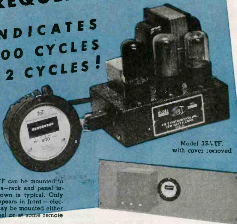
Model 33-VTF can be mounted in several ways—rack and panel installation shown is typical. Only the meter appears in front—electronic unit may be mounted either on same panel or at some remote location.
