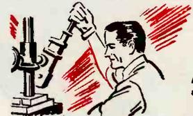
**AND FORM** . . . pressure of about 100 psi is applied and shape cooled briefly in mold.
