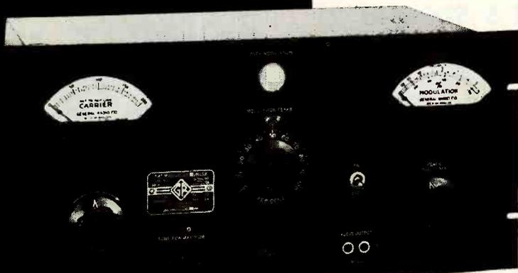
TYPE 1931-A AMPLITUDE MODULATION MONITOR
