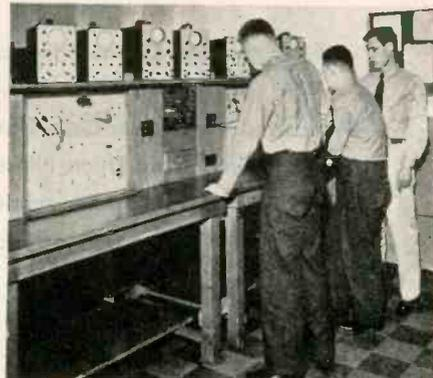
**Breadboard layouts are used to familiarize students with basic circuit operation before they service and operate standard Naval gear**
