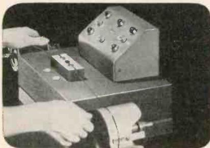
Equally important, Essex Magnet Wire is spot checked each day by means of this mercury-bath test. Pin-hole breaks and film continuity are thus determined—enabling production engineers to maintain constant control of the variables which often cause poor insulating films.
