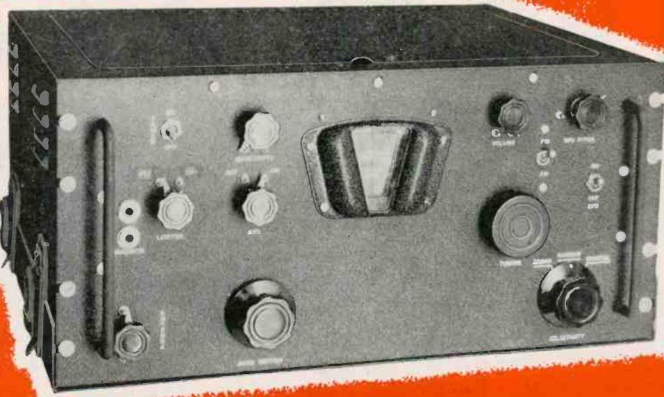
It is apparent that everyone wants to know what sort of general purpose receiver we are going to have for communications after the war . . . Alive to the problem, Press Wireless, Inc. has developed a receiver which is capable of both AM and FM reception.
