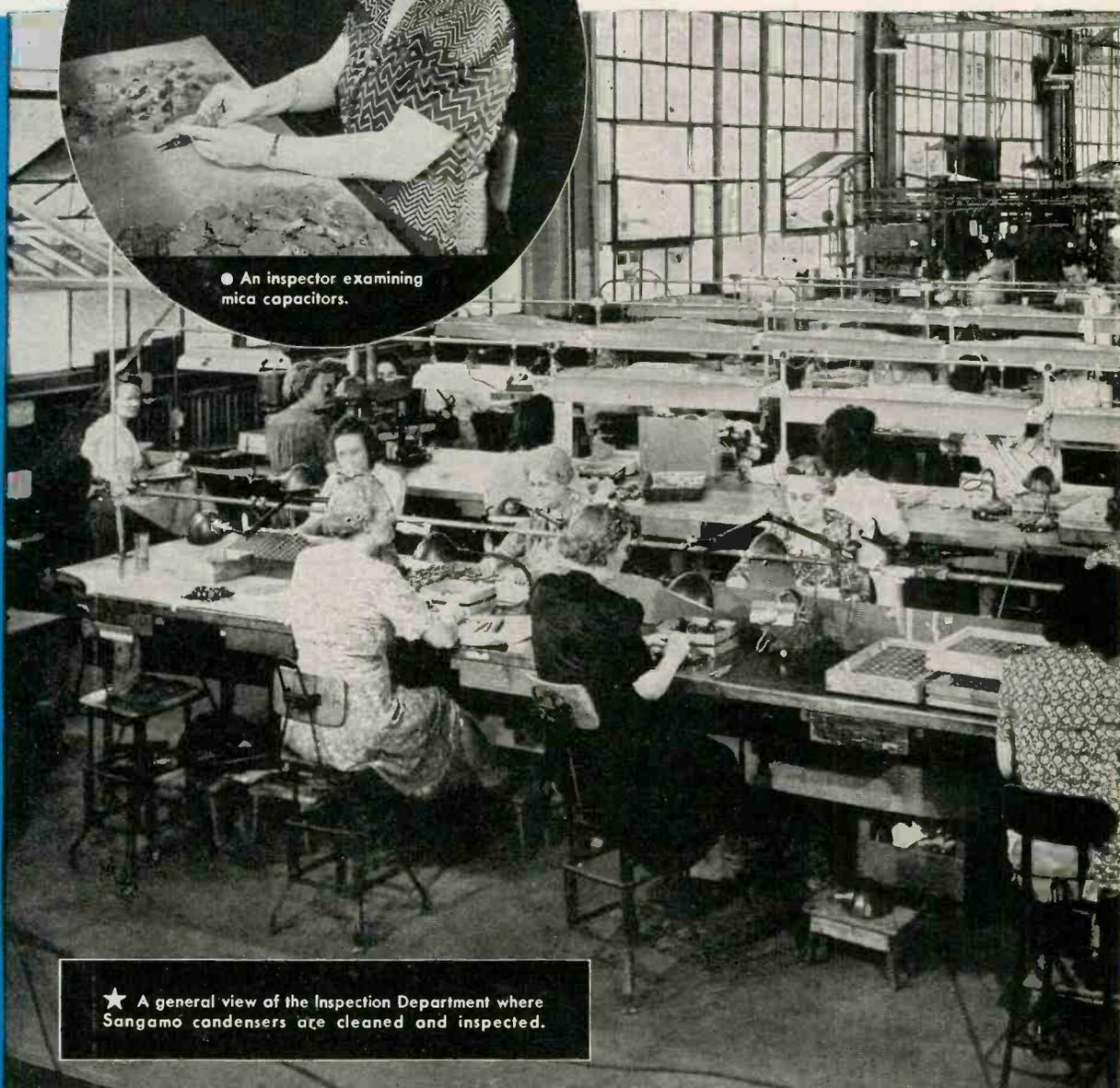
★ A general view of the Inspection Department where Sangamo condensers are cleaned and inspected.
