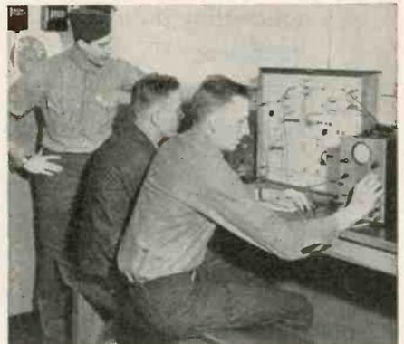
Students use test equipment to study circuit operation. In this instance they are observing wave shapes throughout a d-c amplifier
