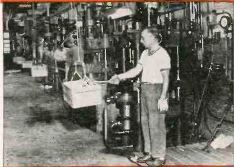
One of several batteries of precision presses for injection and compression molding Mykroy. Here are produced a large percentage of all malded mica ceramic parts required for the war effort.
