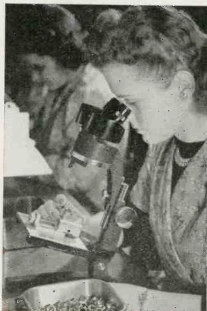
Vital bearings for a Mark XIV Gyro Compass being inspected with a Spencer Stereoscopic Microscope.
