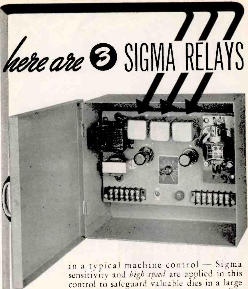
in a typical machine control — Sigma sensitivity and *high speed* are applied in this control to safeguard valuable dies in a large press. Continuing press cycles are possible only as each formed piece is ejected and monitored by the control.
