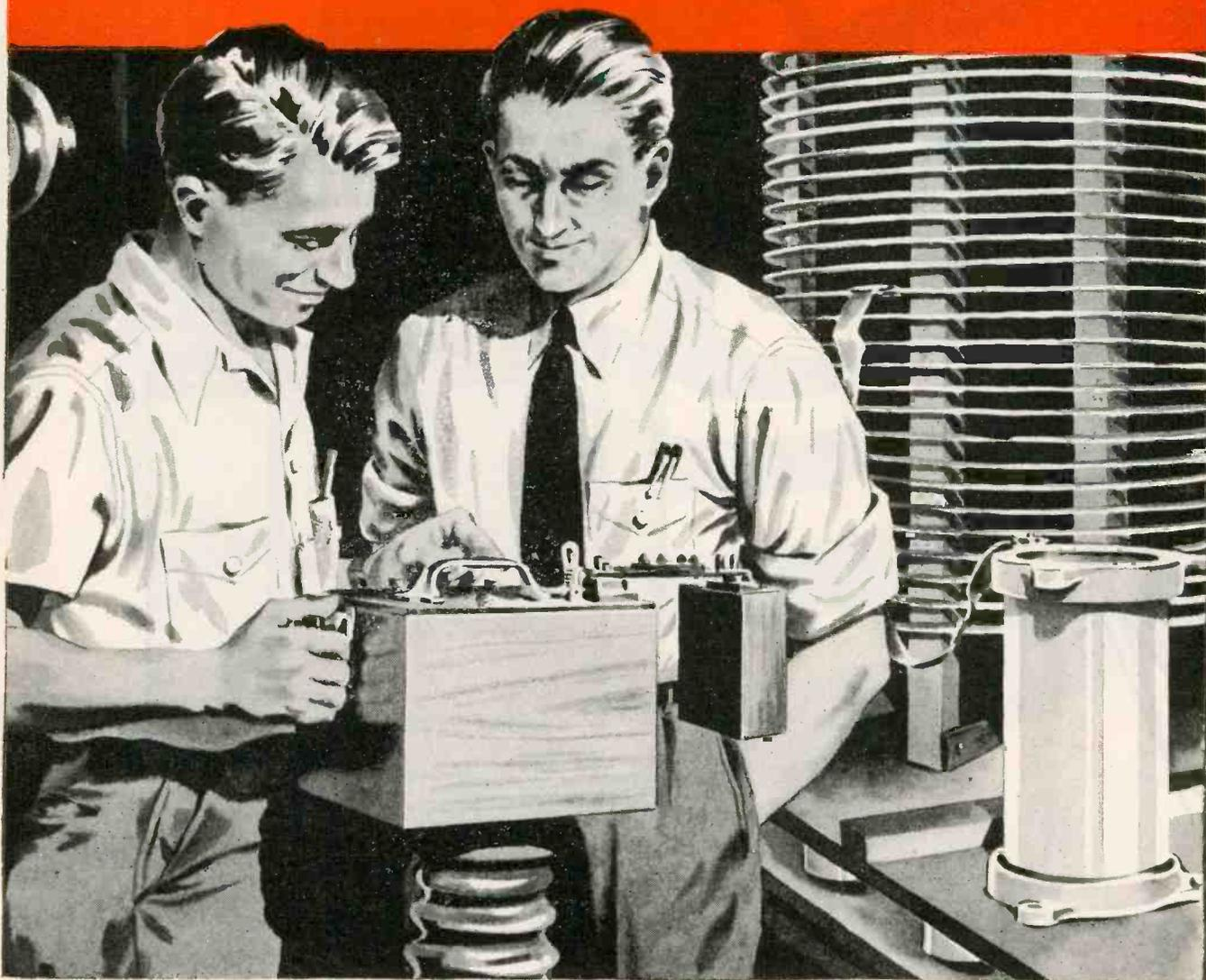
Here this Cornell-Dubilier series 50 capacitor is checked to make sure that the current and frequency ratings are correct.
