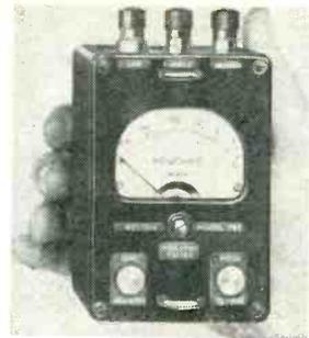
switch automatically disconnects the battery circuit when the instrument is not in use. Ferrules in the panel permit attachment to a lineman's belt or shoulder strap. The unit measures  $5\frac{1}{2} \times 3\frac{1}{4} \times 4\frac{1}{2}$  in. and is manufactured by Weston Electrical Instrument Corp., 617 Frelinghuysen Ave., Newark 5, N. J.
