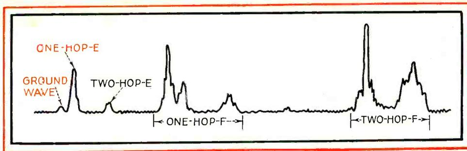
FIG. 8—Typical ground-wave and sky-wave pulse sequence as observed on the Loran oscilloscope. Signals to the right of the one-hop-E are disregarded by the navigator
