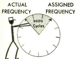
**ZERO HOUR:** Starting up after a shut-down, transmitter may be 3000 cycles above or below assigned frequency. *Frequency Watchman* goes to work.
