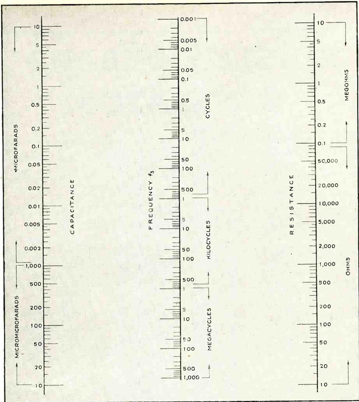
FIG. 2—Resistance-capacitance filter chart based on the relation  $f_3 = 1/2\pi RC$ , where  $f_3$  is the frequency at which the filter provides an attenuation of 3 db. To find the reactance of a capacitor, place ruler on known capacitance and frequency values and read the reactance value on the resistance scale
