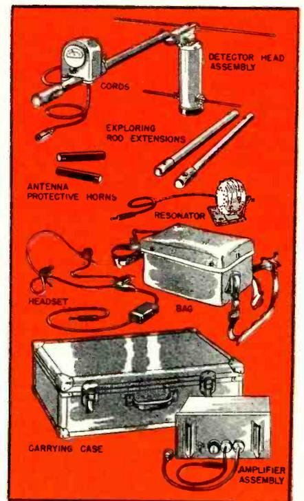
FIG. 1—Main components of detector set AN/PRS-1
