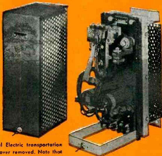
General Electric transportation relay cover removed. Note that only one DZUS fastener is necessary
