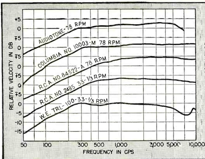
FIG. 2—Measured velocity-frequency characteristic of several test records
