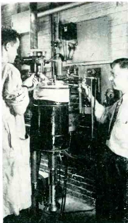
In the fabrication of the 2,000,000-volt x-ray tube made by Machlett Laboratories, each Kovar and glass ring assembly is sealed by induction heating supplemented by a gas flame. When the section is finished, the column is lowered through the floor so that the work surface is always in position to receive the Kovar-glass seal
