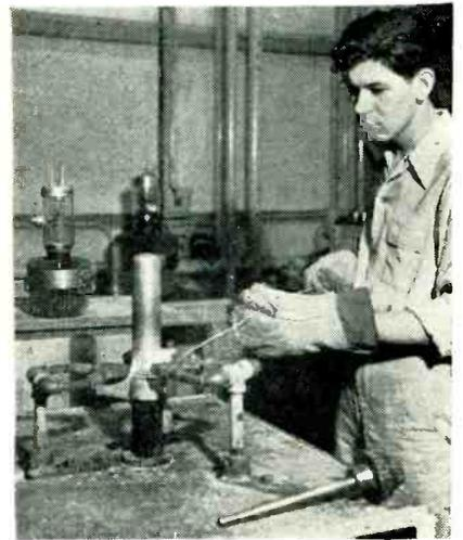
FIG. 3—Anodes for small air-cooled transmitting tubes are brazed with a smaller number of burners
