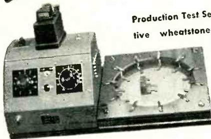
Production Test Set to test varistors. A sensi-
