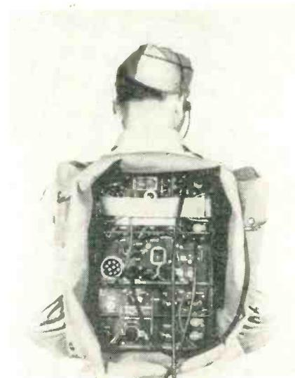
Twenty pounds of transmitter-receiver in the single case of model SCR 694. At the right is the battery pocket, jumper-connected. With cover in place, the set is watertight enough to float without damage
