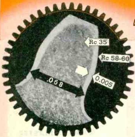
Thin case contour hardening of gear teeth with controlled depth of hardness has been made possible by the use of MEGATHERM induction heat.
