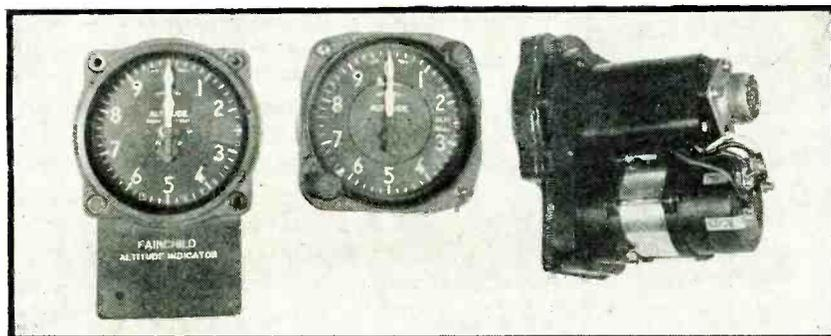
Front and rear views of repeater used on ground, with standard altimeter (center) shown for comparison
