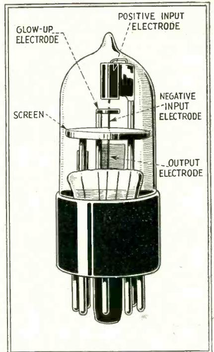
Fig. 1—Addition of a screen disk to separate input and output electrodes, and a glow-up electrode to maintain a pilot discharge produces a high-speed, sensitive relay amplifier tube
