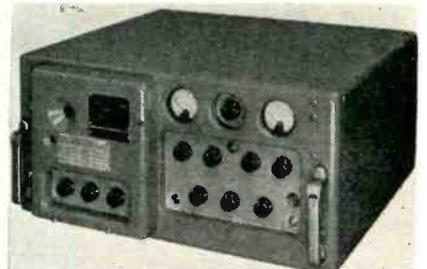
the wrist) the panel section from the cabinet. Design of the interior mechanism utilizes a drawer slide which does away with the necessity of removing the receiver from the cabinet. With the receiver pulled out on this drawer slide, the
