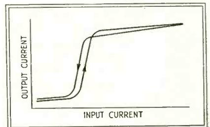
Fig. 2—Relative input-output characteristic of the Teleion indicates how, at a critical point on the characteristic, a small decrement in the input produces a large change in the output
