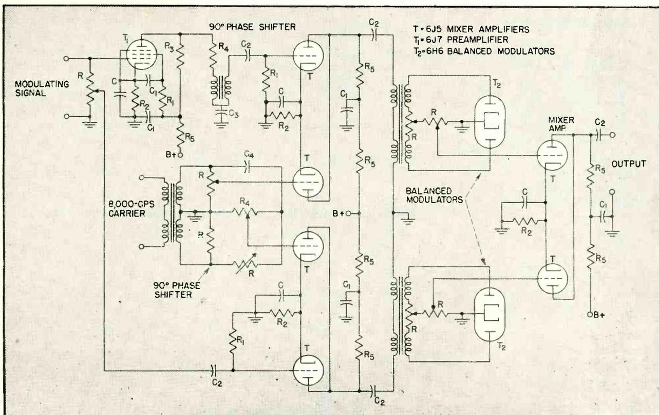
FIG. 6—Circuit of experimental single-sideband generator
