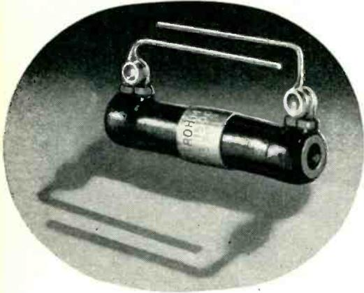
Lectrohm's method of manufacture has established an enviable reputation as providing a most dependable, lasting performance at rated resistances of any resistors made. They're solid—consistent performance—no variance over long hard usage. Resistance wire is silver soldered to the solder lugs by special process (not by torch method of brazing) for perfect electrical bond always. Wire and lugs are completely embedded in high temperature vitreous enamel. Write for complete data.
