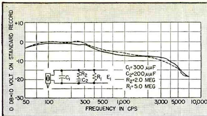
FIG. 6—Solid line is response of PN pickup cartridge with compensating network; dash line is Audiotone record response adjusted to N.A.B. Standard
