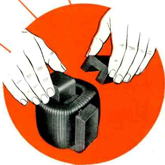
Hipersil Type "C" Cores come ready assembled, in two segments per loop. They eliminate tedious time-consuming "stacking" of separate laminations . . . permit quick, economical assembly with coils and stamped metal bases by means of steel straps. Cast mountings and assembly bolts can be dispensed with.
