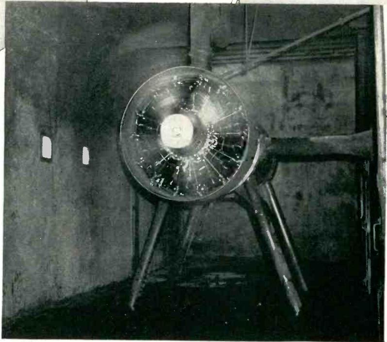
A Wright Cyclone engine running on the test stand. Electrical resistance strain gages affixed to various component parts and wired to the remote oscillographic equipment, serve to indicate stress and load under actual operating conditions.
