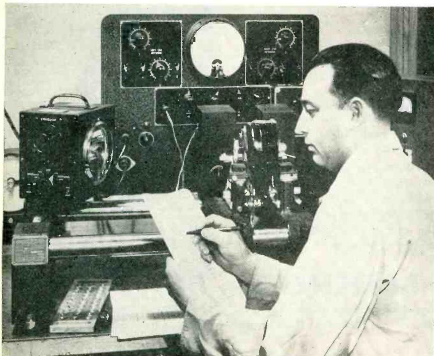
sight equipment in the laboratory of the Victor Adding Machine Company, using a General Radio Strobotac and a Gisholt Dynetric Balancer.
