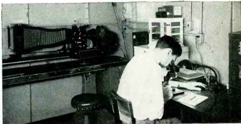
**S**PECTROSCOPIC analysis, accurate to 0.001%, tells exactly the chemical composition of Mallery contact materials. Tungsten, Elkonite\*, Elkonium\*, silver, platinum and combinations of these metals are checked for correct grain size by Mallery photomicrographs. X-ray examination determines whether contacts and backings are firmly bonded. Life tests check the durability in service of Mallery Contacts and Contact Assemblies.
