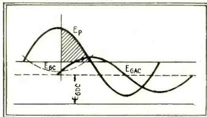
Fig. 2—Phase-angle firing control is used in the arc-furnace regulator. Variations in  $E_{GDC}$  cause  $E_{GAC}$  to intersect the  $E_{GC}$  curve at different points, instituting conduction for the remainder of the half-cycle. Motor power is represented by the shaded area
