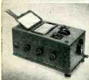
**The New U. S.-Made Midget "Megger" Tester**—In many ways the most remarkable "Megger" instrument ever built. Weighs only 3 lbs—will fit an overcoat pocket or tool kit. Reads up to 50 megohms. Generates 500 volts and is always ready for use anywhere because of the hand crank. Bulletin 1785-E.
