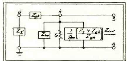
Fig. 4—Generalized equivalent output circuit of cathode follower
