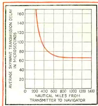
FIG. 7—The additional time of transmission of the "one-hop-E" sky wave, relative to the ground wave, over various distances. This delay is applied as a correction when using sky-wave signals with ground-wave charts
