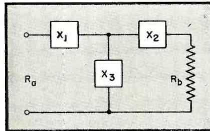
FIG. 6—Three-element T network
