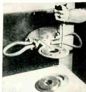
tronic heating equipment to aid them in immediately adapting the unit to any specific application in a minimum of time. The sets consist of master coils and removable inserts in diameter sizes ranging from 1/8 in. to 3 in., and of any desired thicknesses so that the coils are capable of heating axial bands of various widths to produce many heat patterns. Blank inserts are available to allow the user to cut the
