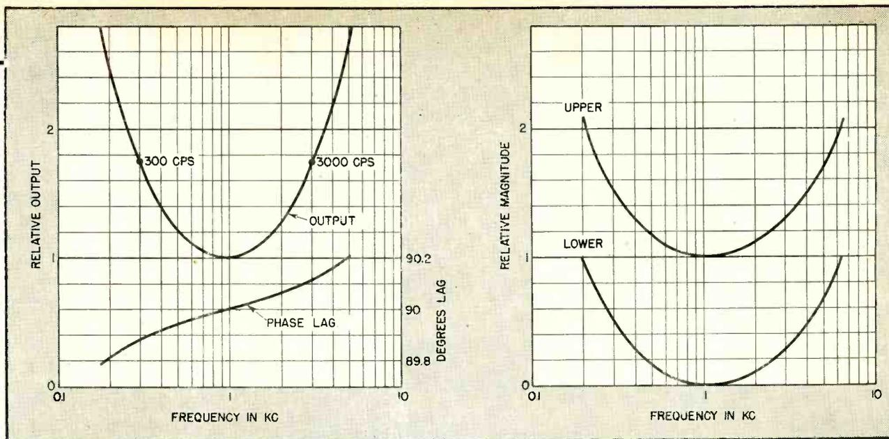
FIG. 3—Calculated amplitude and phase response of phase shifter with  $R = 100,000$  ohms,  $C = 2.34$  microfarads, and  $L = M = 0.012$  henry
