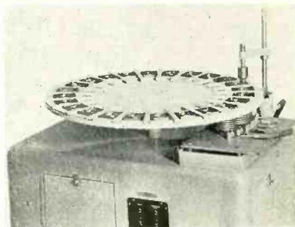
Used in the brazing of metal assemblies, this twenty-four-station circular indexing carrier permits the completion of one piece each twelve seconds. The operator merely loads the stations as they come around empty, ejection being performed by the vertically-operating mechanism which follows the three water-cooled induction coils. The carrier can be applied to any "S" Corrugated Quenched Gap Co. electronic generator rated between 5 and 100 kw
