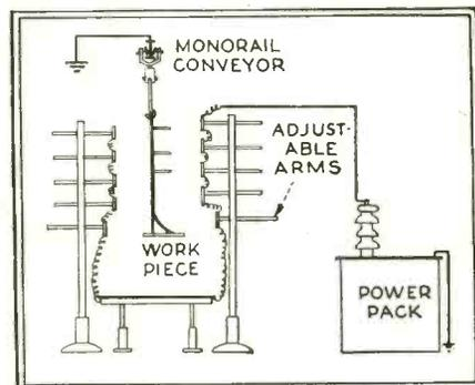
For production of electrostatic field in paint-spraying operation, an adjustable arrangement like this accommodates various sizes of articles. For detearing, the polarity of the field is reversed
