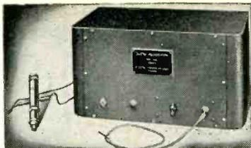
Indicates in linear response, on screen of cathode ray oscillograph, the pressure-time-curve of any internal combustion engine, pump, airline, or other pressure system where pressure measurements are desired. Static—also dynamic pressure up to 100,000 R.P.M.
