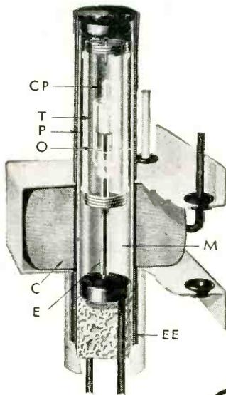
Contacts and break-offs are as quick as a wink because Adlake Plunger-type Relays (models for A.C. or D.C.) use fast-moving, liquid metal mercury . . . positive in action; silent and chatterless; will not burn, pit, or stick.
