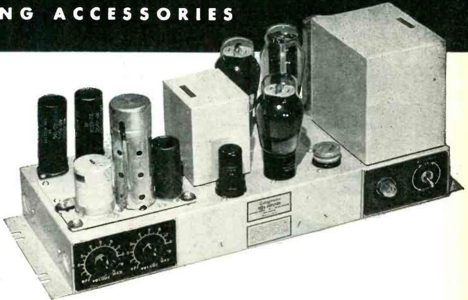
**TYPE 108-B** two-stage Amplifier provides transformer input impedances for either 30 or 250 ohms with nominal output impedance 500 or 8 ohms. Variable gain 65/105 db. with electronic volume control. Frequency response better than  $\pm 1$  db. 30/16,000 c.p.s. Power output +43 V.U. (20 watts) with less than 5% RMS harmonic content. Noise level full gain 56 db. below full output.
