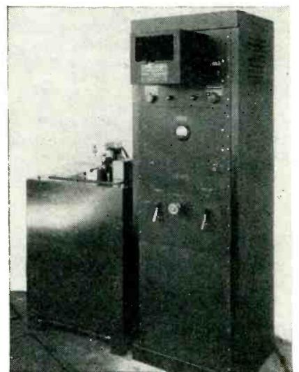
Parts to be balanced are mounted for test on the seismically suspended platform at left. The electronic equipment in the cabinet at right includes a cathode-ray tube indicator and a phototube tachometer.
