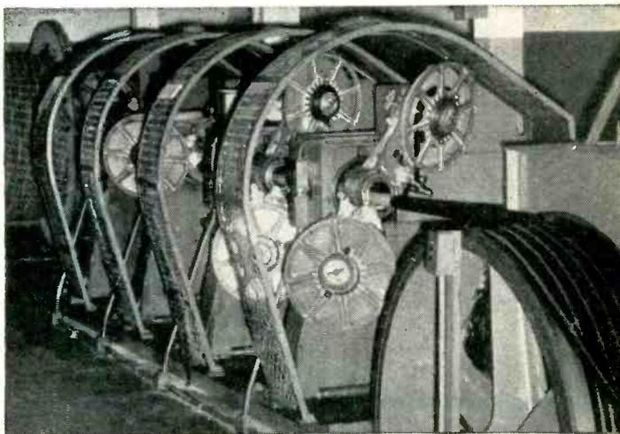
*Cable wrapping machine in the plant of Collyer Insulated Wire Co., Inc., utilizes Empire straight-cut cable tape in the manufacture of their heavy-duty cable.*
