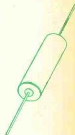
"L" Type Powder used in cores for permeability tuning.
