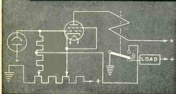
A typical vacuum tube application. A slight increase in plate current closes the relay, thus increasing negative bias on the amplifier tube so that plate current through the relay coil immediately decreases to a point close to the release value for the relay. Thus, any slight decrease in light falling on the photo cell will reduce plate current sufficiently to return relay contacts to normal position.
