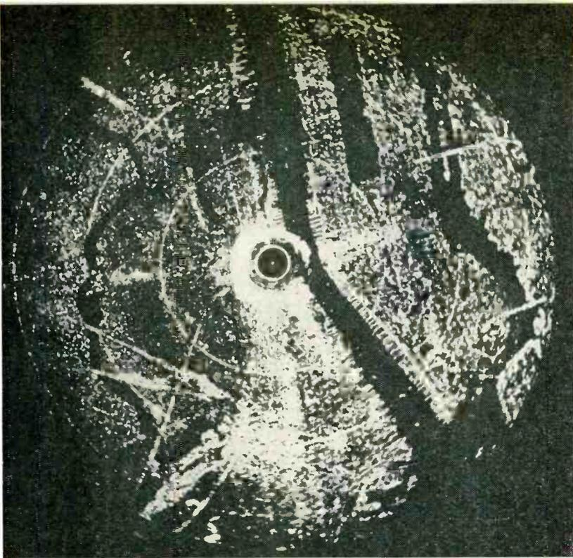
The radar equipment which produced this PPI picture of Manhattan Island and nearby New Jersey (looking north) was still under development at the war's end. The resolution of the individual docks along the Hudson River, bridges, islands, ships, and even railroad tracks (diagonal lines lower left) is made possible by the use of a wavelength shorter than 3 cm
