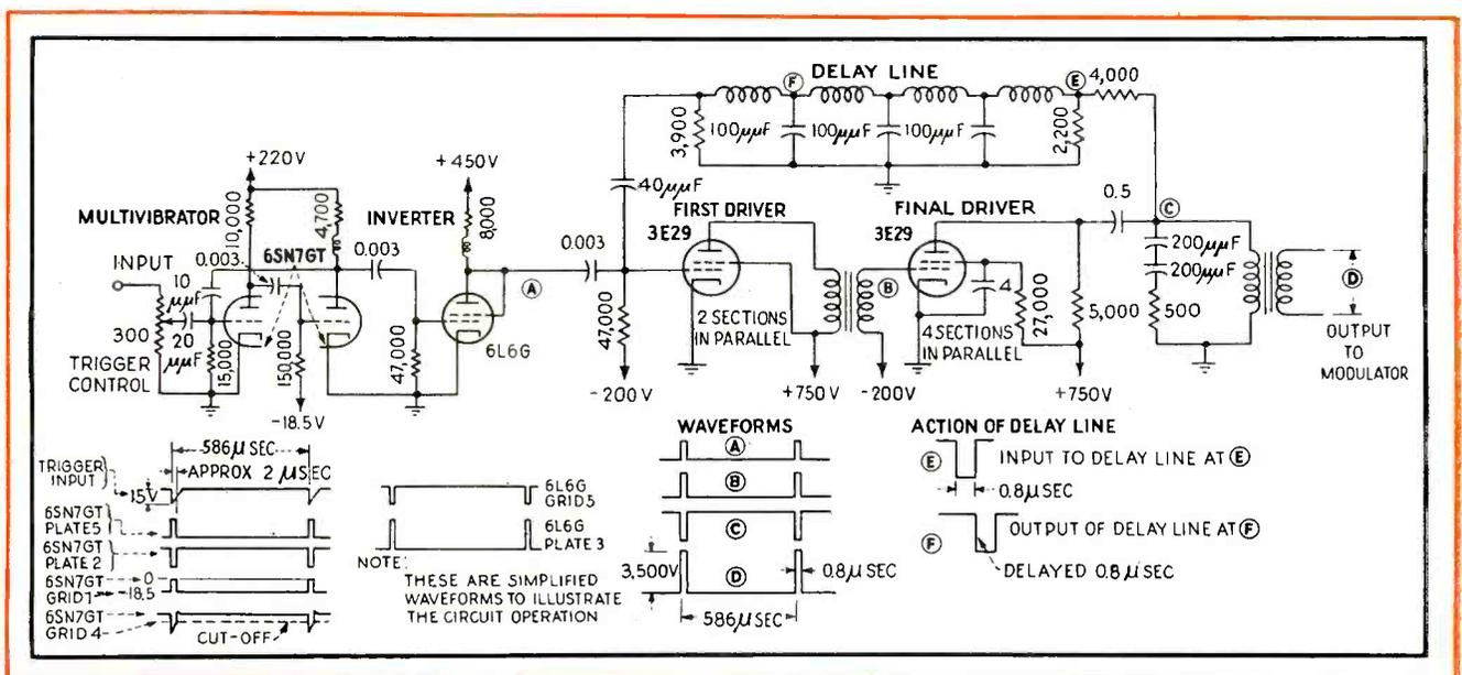
FIG. 4—Simplified schematic of the driver unit, which creates 0.8-microsecond pulses of 3500-volt amplitude for driving the modulator tubes
