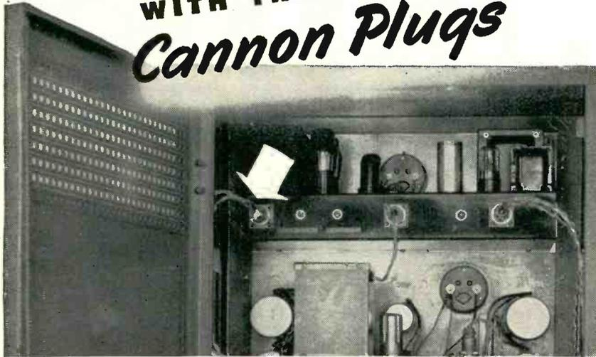
This is the Waugh Metal Analyzer (above and below). It gives an instantaneous indication of the hardness, grain structure and other properties of ferrous materials on which it is used. It performs this scientific feat by means of magnetic analysis and employs many precise electric circuits in its hook-up. These circuits are connected and test units are plugged in through various Cannon Connectors—indicated in the rear view of the open cabinet. Both plug and receptacle types are shown.
