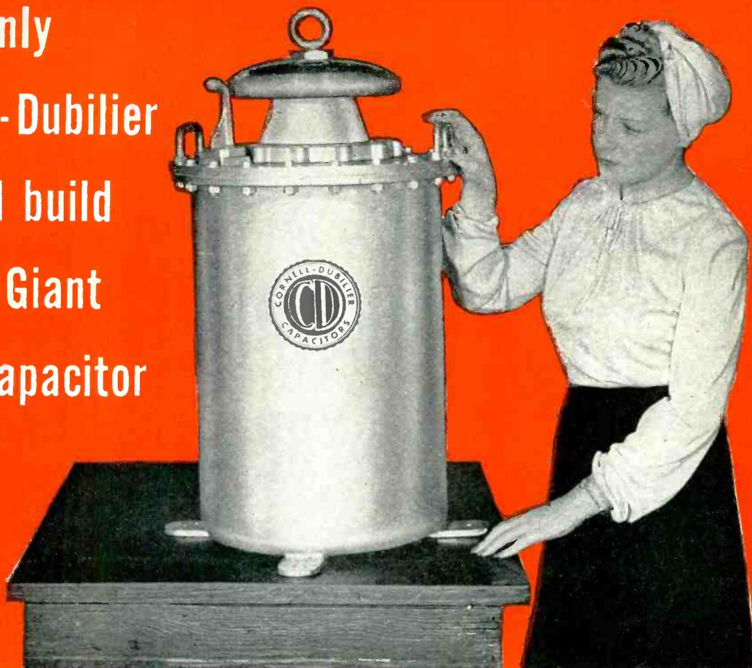
When an unusual problem in capacitors arises, engineers think first of C-D. A case in point is this giant mica tank capacitor for a transoceanic transmitter. It is now in use and combines space - saving design with the capacity of much larger units.
