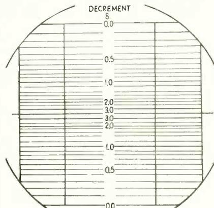
Fig. 2—Scale for measuring decrement directly
