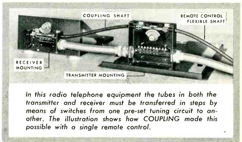
In this radio telephone equipment the tubes in both the transmitter and receiver must be transferred in steps by means of switches from one pre-set tuning circuit to another. The illustration shows how COUPLING made this possible with a single remote control.
