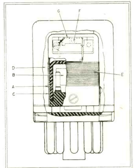
Cutaway view of the crystal oven for aircraft radio equipment that anticipates temperature changes
