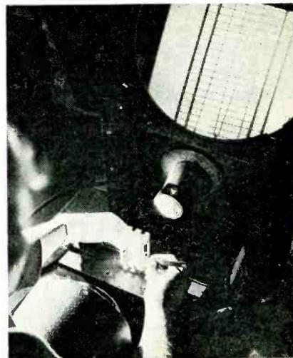
The 813 transmitting tube has two grids which must be perfectly aligned. At North American Philips, light is projected on the tube mount and then focussed on a ground-glass plate. The 20-to-1 enlargement produced shows whether or not one grid is exactly behind the other.
