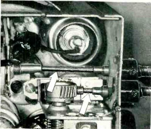
COUPLING the external remote control shafts to the tuning elements, as in this radio receiver, damps vibration, thus preventing vibration-created noise from being communicated to the sensitive receiving circuit. It also eliminates any need for precise mounting and alignment of the tuning elements and gives complete freedom in their location.
