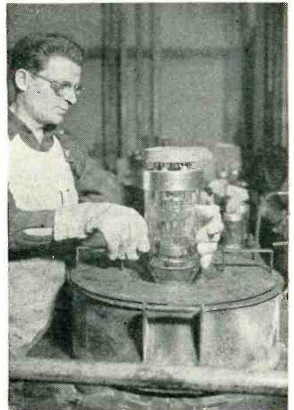
FIG. 5—A weight on top of the tube maintains constant pressure to force the anode into the radiator
