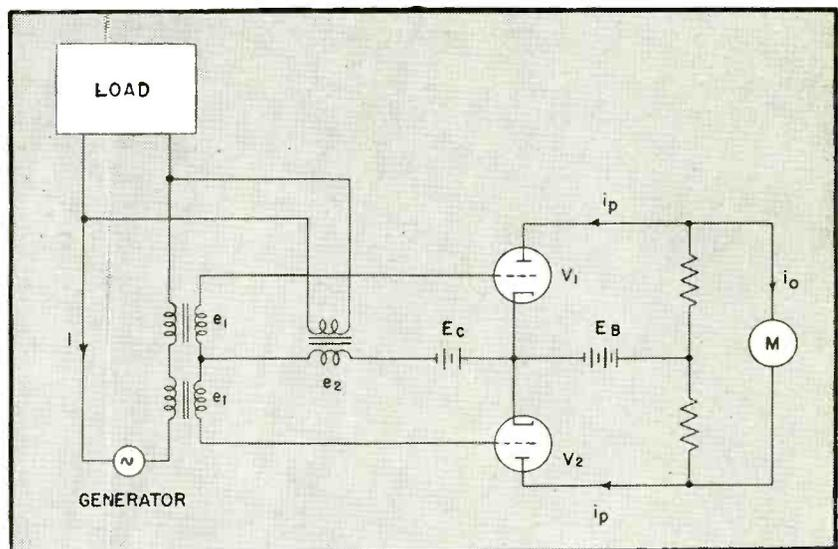
FIG. 1.—Original electronic wattmeter circuit of Peterson, using transformers to compare the phase angle between potential and current
