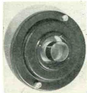
clamping ring that is in turn held down by two machine screws. By loosening the screws holding the pressure ring, a small lateral movement of the spider is permitted by which the voice coil can be re-centered concentrically around the pole-piece and within the gap.
