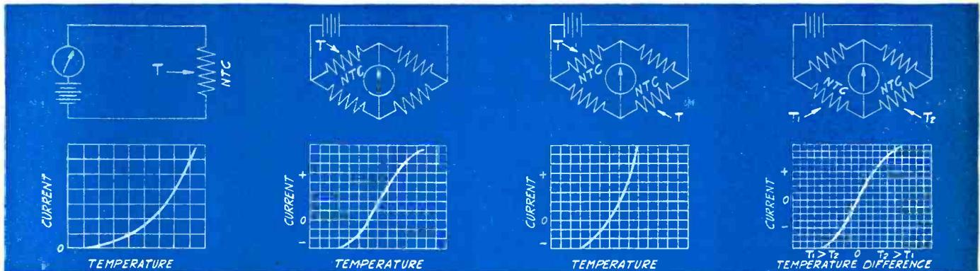
This simple series circuit of voltage source, instrument and NTC unit has been utilized to indicate engine coolant temperature, etc. It provides sufficient accuracy for many applications despite scale crowding at the bottom.
