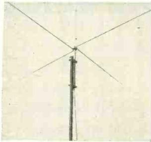
when the antenna is used with transmitters there is no standing wave on the line, thus reducing line losses and voltage flashover, and freedom from reflections is obtained; the band-width is good for f-m because it is not less than 400-kc wide for a standing wave ratio of 1.2 to 1, and by careful selection of transmission-line impedance, may be made as wide as 1 mc; the antenna may be used with any 70-ohm coaxial cable, solid dielectric or beaded, up to 3/4-in diameter.
