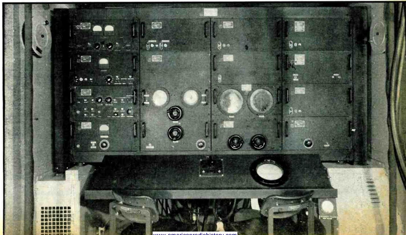
signal, the other proportional to the elevation component. These control voltages operate an amplidyne control system which orients the antenna so that the error signal is a minimum. Manual positioning is also possible through the use of an artificial error signal, produced within the equipment and controlled by knobs set by the operator to the desired values of azimuth and elevation.
