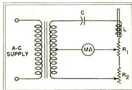
Circuit of simple coil testing unit capable of detecting a single shorted turn of 40-gage copper wire. The coil is placed over projecting core of inductor  $L$ .
