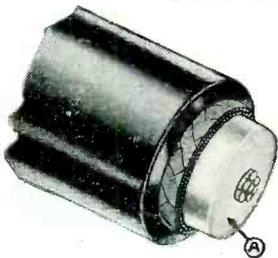
Cross-section (4 2/3 times actual size) of coaxial cable used in television transmission by Allen B. DuMont Laboratories, Passaic, N. J. Polythene's non-polarity is an additional advantage here, since the current sometimes changes direction at 100 million cycles per second. (A) Polythene insulation.
