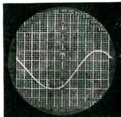
Sine-wave trace obtained on the screen of the cathode-ray tube of the Electro-dynascope
