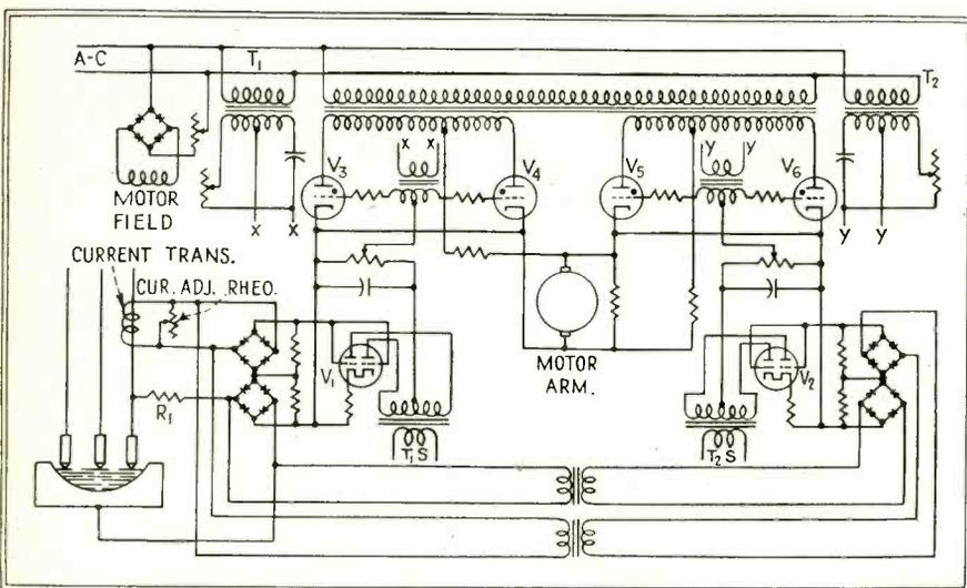
Fig. 1—Circuit of the electronic arc-furnace regulator. Tubes  $V_1$  and  $V_2$  regulate the firing of thyratrons  $V_3$ ,  $V_4$ ,  $V_5$ , and  $V_6$ , each pair of which is related to one direction of electrode-motor rotation
