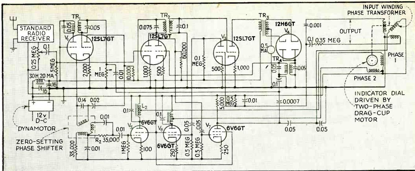
FIG. 2—Schematic diagram of chassis used on ground to convert output signals of receiver into currents suitable for driving an indicator that repeats accurately the readings of the instrument on the plane
