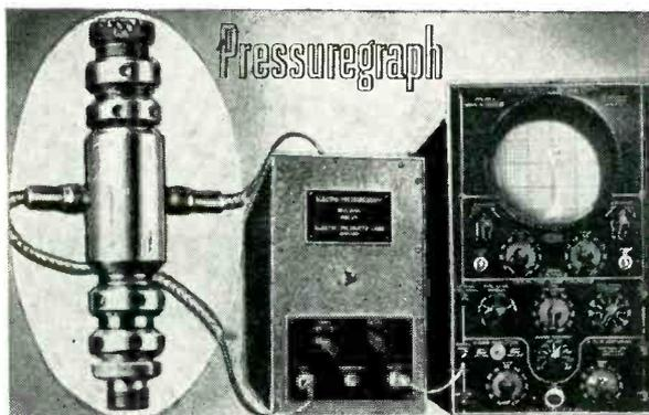
Indicates in linear response, on screen of cathode ray oscillograph (or on string oscillograph for photographic recording), the pressure-time-curve of any internal combustion engine, pump, airline, or other pressure system where pressure measurements are desired. Covers wide range of engine speeds and pressures up to 10,000 p. s. i. Screws into cylinder and can be calibrated using static pressures. Vibration-proof. Accurate, dependable for frequent engine tuning.
