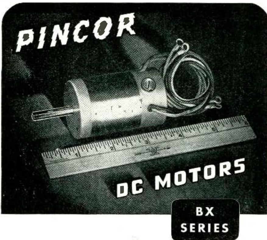
Pincor BX motors, in their classification, meet the varied requirements of manufacturers who demand light weight, compact motors for efficient and dependable application. Pincor BX motors are direct drive, ball bearings, high speed units wound for continuous or intermittent duty. Shunt, series or split series windings are for operation on 12 to 24 volt battery systems currently used and may be easily modified to meet your product demand.
