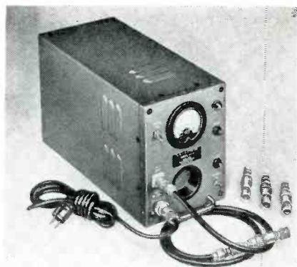
50-ohm load of wide-band constant-impedance design, series thermocouples near the transmitter end and a d-c millivoltmeter. The blower is powered by a 115-v, a-c or d-c 60 cps motor which need not be operated below 50 w r-f input.
