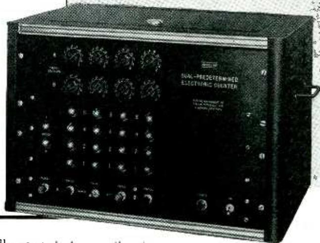
For processes requiring a rapidly repeated operation to occur after a predetermined number of counts!
