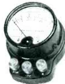
Dual Range 0-3 Amp. and 0-15 Amp. full scale for use on any frequency from 25 to 500 cycles. The ideal instrument for all commercial, industrial, experimental, home, radio, motor and general repair shop testing. Comes complete with a genuine leather, plush-lined carrying case and a pair of test leads. A very convenient pocket sized meter priced at less than 50% of manufactures list.
