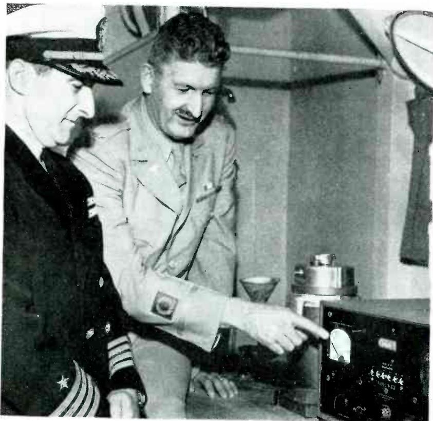
Radioactivity of seawater caused by atomic bomb test at Bikini will be measured by this electronic equipment. Geiger counter output is amplified and used to operate an indicating meter. Col. S. Warren, Radiological Safety Advisor to Joint Task Force One, shows Capt. A. C. Thorington what the indications will mean in terms of personnel safety
