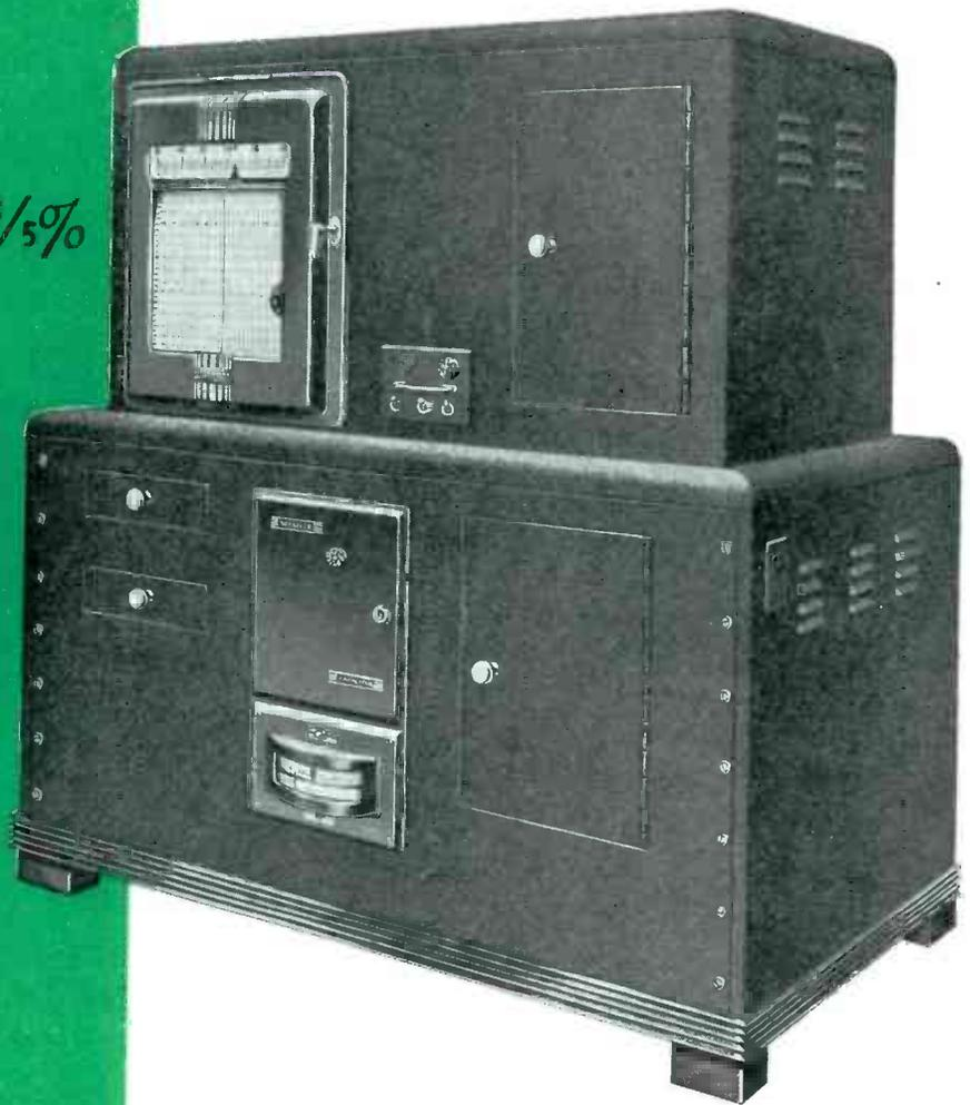
**THE SYLVANIA DILATOMETER** measures expansion and contraction by the concentric quartz tube principle... providing the extreme accuracy characteristic of this method.
