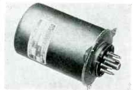
provide protection against adverse atmospheric conditions such as moisture, dust, and corrosion. Relay coil and contact connections are totally enclosed within the metal housing and are brought to the prongs of a standard octal-plug base. Plug-in relays are available in contact combinations to double-pole, double-throw with a-c contact ratings (at commercial frequencies) of 4 amperes from 0 to 115 volts and d-c
