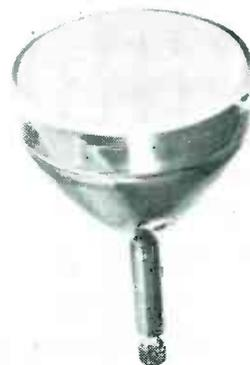
plays electromagnetic focusing and deflection. Face of the tube is 10 inches in diameter.
