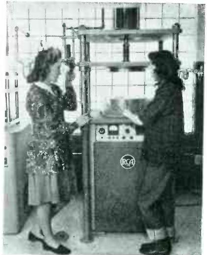
Seam-sealing with an electronic generator at the Lombard, Ill. plant of DuPage Plastics Company. When the upper electrode is lowered, strips of Vinylite are joined in airtight seams
