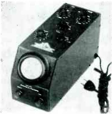
and within minus 6 db to 200 kc. With maximum gain, vertical and horizontal deflection sensitivities of about 0.1 volt rms per inch are obtained. Input resistance is 0.5 megohms and shunt capacitance is 36 microfarads. The self-contained power supply operates on 105 to 125 volts, 50 to 60 cps with a power consumption of 23 watts under normal operating conditions. The unit measures 6 3/4 x 3 3/4 x 10 inches and weighs only 5 1/2 pounds.
