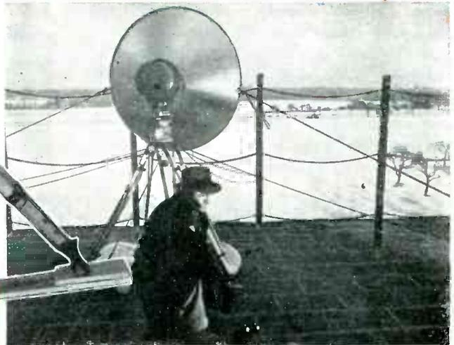
**ON LOCATION**—The microwave transmitter relays the signals picked up by field cameras to the studio—recently used with excellent results to transmit scenes of the U.N. Conference at Hunter College to Radio City.
