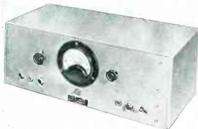
the range of 10 to 20,000 cps with an overall accuracy of better than 1 percent. The addition of a stroboscopic lamp allows its use as an electronic tachometer. Pulses of practically any wave form up to 50 micro-seconds duration can also be measured. External recorders or meters can be used for graphical or remote indications.
