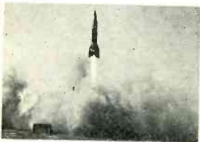
A V-2 rocket taking off from White Sands Proving Ground, New Mexico. It could easily carry a man up a hundred miles since the maximum 6-G acceleration is below that at which pilots black out, but getting down safely is another problem
