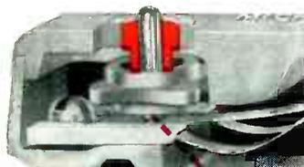
This accurate repeatability of operation at a precise point is due to special construction which involves three specific features. The stainless steel plunger pin, instead of being guided by a hole in the plastic cover, moves in a carefully fitted bronze guide imbedded in the cover. The pin and the guide are carefully ground to close tolerances assuring absolutely straight travel of the actuating plunger. Note illustration.
