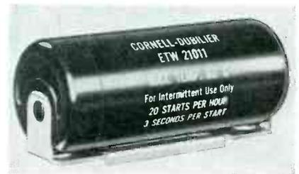
starting capacitor which is designed for mounting in a clip-type bracket. The capacitor is enclosed in a plastic case. Capacitance range is 25 to 450 microfarads.
