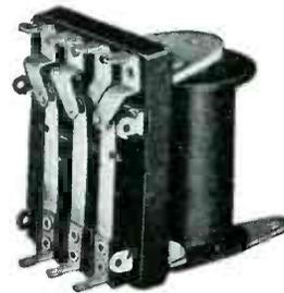
be selected for any d-c voltage between 0.5 and 150 volts, and any a-c voltage between 3 and 500 volts. The approximate dimensions are 2 x 1 7/8 x 1 1/4 inches. The weight is approximately 4 ounces. Additional information may be obtained in Bulletin 1646.
