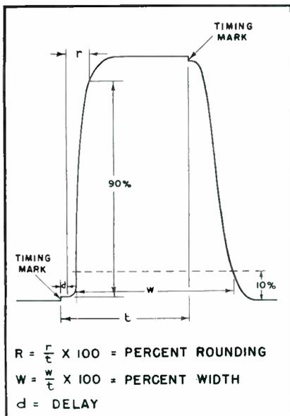
FIG. 2—Typical output pulse with the percent rounding and percent width defined. The delay between the timing mark and the initiation of the output pulse occurs in the amplifier and other circuits
