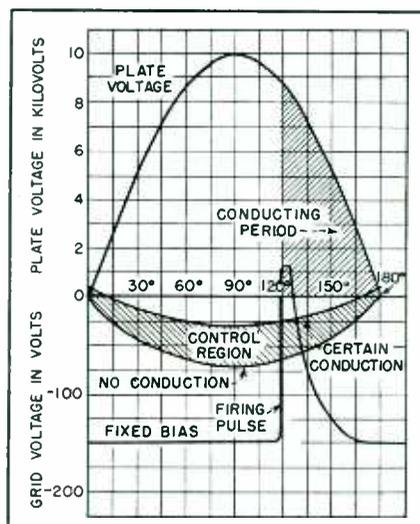
FIG. 2—Operating curves for a typical thyatron
