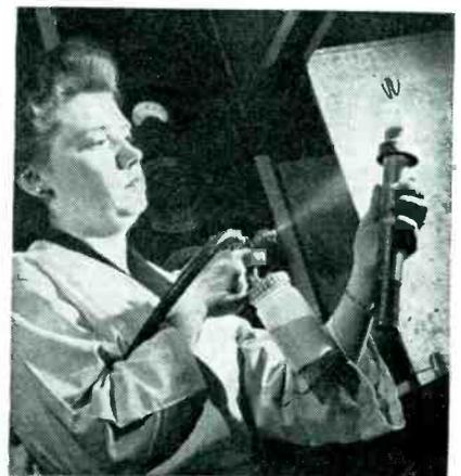
For making large and complex glass-to-metal seals, engineers at Westinghouse Lamp Division have developed a method in which the metal Kovar is heated in a temperature-controlled oven, then cooled and sprayed as shown above with powdered glass suspended in liquid. A second heating fuses the glass into a film to which the glass tube envelope can be sealed in the ordinary manner
