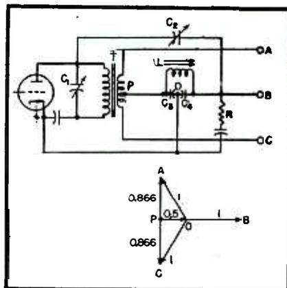
FIG. 7—The phase-splitting circuit described in the text and a vector representation of phase relations at various points in the circuit
