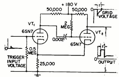
**CATHODE-COUPLED ONE-SHOT MULTIVIBRATOR**—Circuit values are adjusted so that  $VT_1$  is cut off when  $VT_2$  is conducting. The trigger signal interrupts this stable condition, but after the period  $t$ , the circuit automatically returns to the stable condition. If the grid return of  $VT_2$  is made to cathode instead of to +180 volts, a somewhat longer period is obtained. This circuit has the advantage that the triggering circuit is isolated from the multivibrator circuit by  $VT_1$
