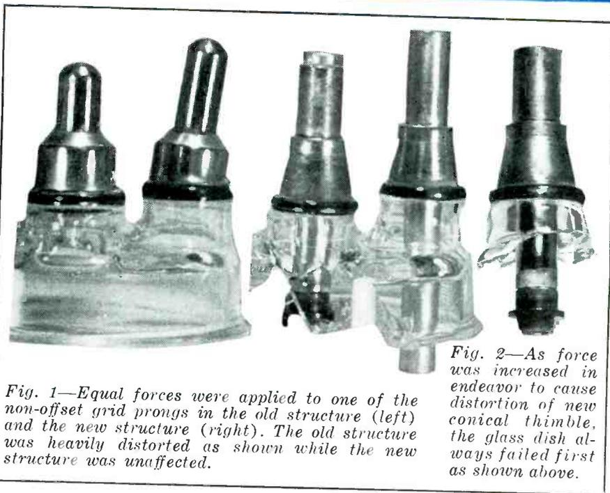
Fig. 1—Equal forces were applied to one of the non-offset grid prongs in the old structure (left) and the new structure (right). The old structure was heavily distorted as shown while the new structure was unaffected.
