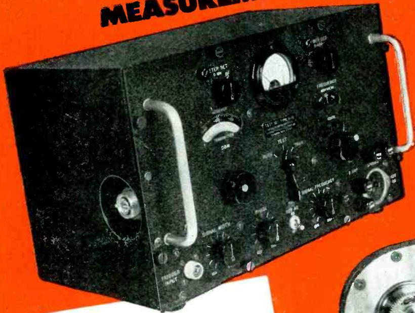
A.R.C. 24,000 Mc. wavemeter and attenuator, built to highest precision standards through unique split-plate method of construction.
