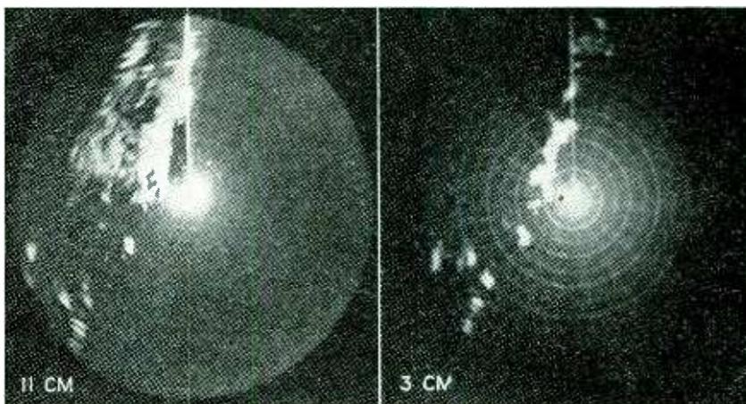
FIG. 5—Summer line squall as it appears on scope of 11-cm radar and 3-cm radar. Range marks are 5 nautical miles apart on both patterns
