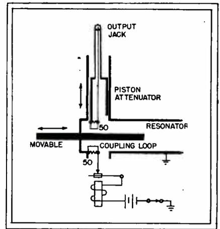
Circuit of simple microwave signal generator
