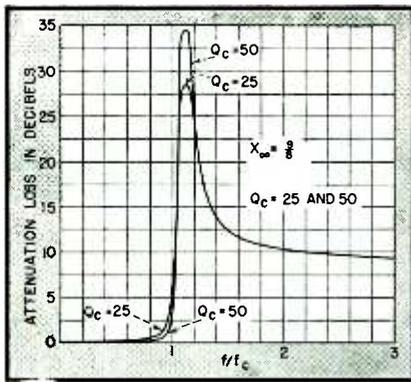
FIG. 3—Attenuation curve of network for two values of  $Q$ ;  $m = 0.458$
