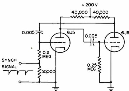
**SYNCH INPUT TO ONE GRID**—This circuit tends to favor the odd submultiples of the synchronizing frequency when a sine-wave synchronizing signal is used. When pulses are used, synchronization occurs more readily with negative pulses
