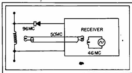
Fig. 1—Simple converter for prewar 1-m receivers. The line couples the original oscillator to the new mixer
