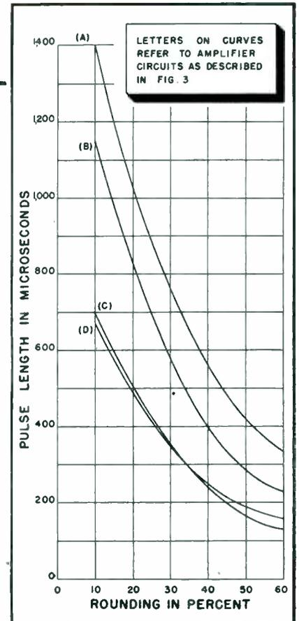
FIG. 4—As a circuit rounds the output shape of a square-wave input pulse, the length of the pulse must be increased or else the output amplitude will decrease
