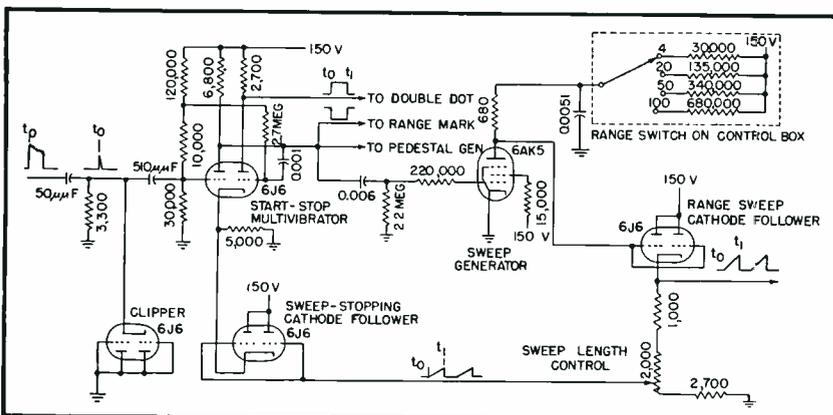
FIG. 4—Diagram of range sweep circuit
