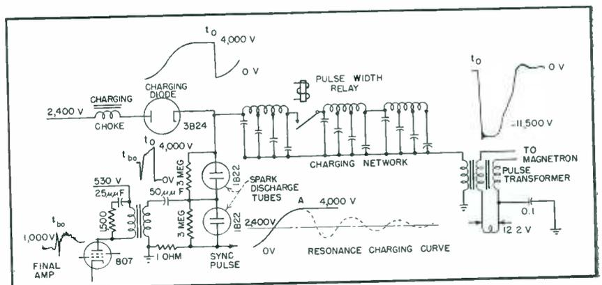
FIG. 2—Modulator circuit, showing how spark discharge tubes are used in connection with a charging network to energize the magnetron
