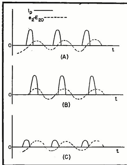
FIG. 2—Variation of plate-current pulse due to phase difference of oscillator and incoming signal
