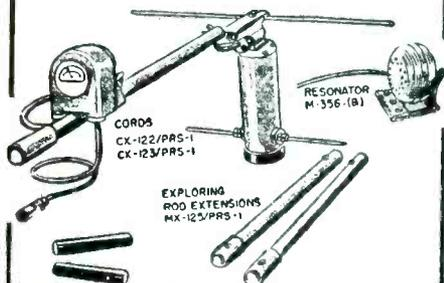
These are used for detecting Metallic and Non-metallic materials by indicating either aurally, visually, or both.
