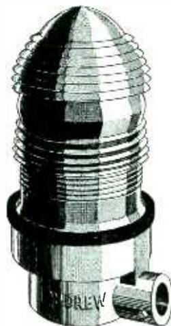
**OBSTRUCTION LIGHT.** Type 661 is a 100-watt unit fitted with a red fresnel lens to concentrate the light in a nearly horizontal direction. Used in pairs at  $\frac{1}{3}$  and  $\frac{2}{3}$  levels on radio towers for aircraft warning.
