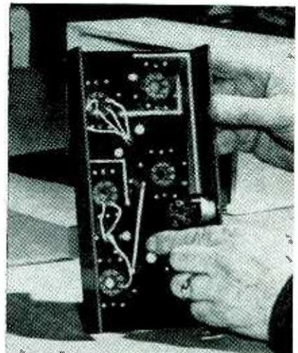
By using a cutout mask as a stencil, sand blasting the plastic chassis to cut the wiring channels, and spraying molten metal into the channels, radio receivers are being turned out at the Buffalo plant of Promette Radio and Television
