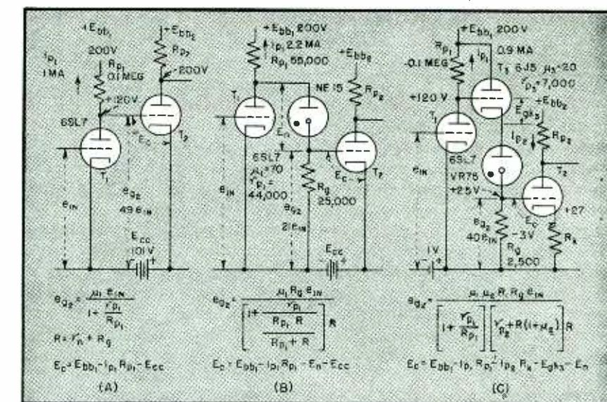
FIG. 1—Conventional d-c amplifier circuit and two methods of using gas tubes for coupling between stages. Typical values for the networks are given
