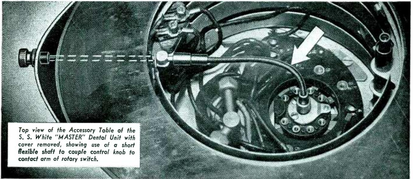
Top view of the Accessory Table of the S. S. White "MASTER" Dental Unit with cover removed, showing use of a short flexible shaft to couple control knob to contact arm of rotary switch.
