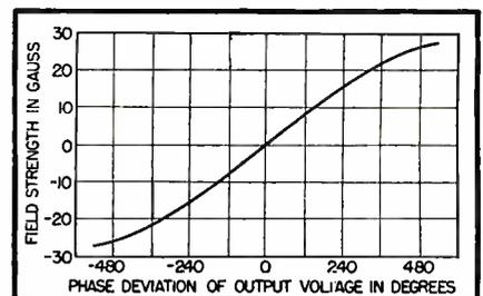
FIG. 5—Phase deviation of the output voltage with respect to field strength of the modulating coil in gauss
