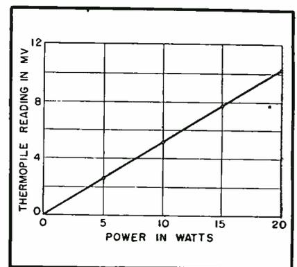
FIG. 2—Typical calibration curve for the air-flow wattmeter
