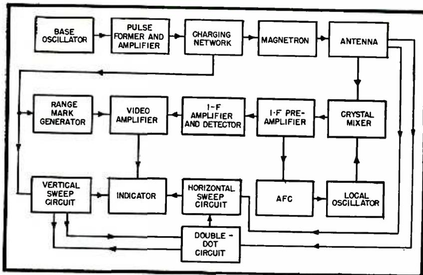
FIG. 3—Block diagram of complete APS-4 radar system. Two indicators are used on some planes
