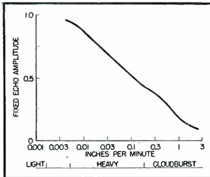
FIG. 6—Attenuation of 3-cm waves for simulated rain falling on radome at various rates
