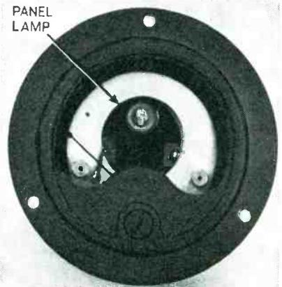
FIG. 1—Close-up of panel instrument with scale removed to show panel lamp mounted inside the case
