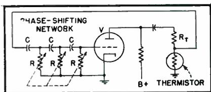
FIG. 1—Basic circuit of phase-shift oscillator
