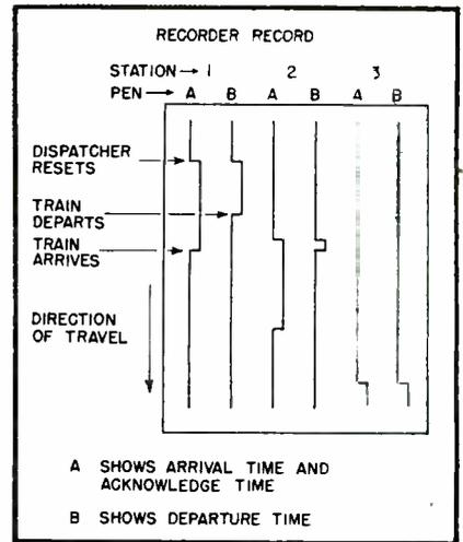
FIG. 5—Typical record of what is indicated by recording pens
