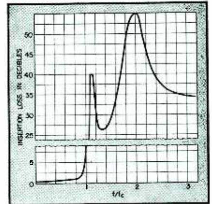
FIG. 7—Insertion loss of a composite filter consisting of two single  $m$ -derived sections in cascade having the values  $m = 0.458$  and  $0.866$  and  $Q$ 's of 50 and 25 respectively
