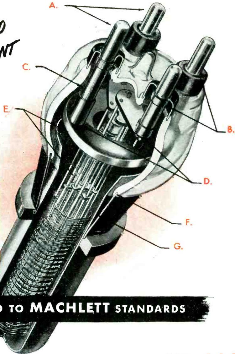
Sectional view of the ML-889-A, showing features typical of Machlett external anode tube construction.
