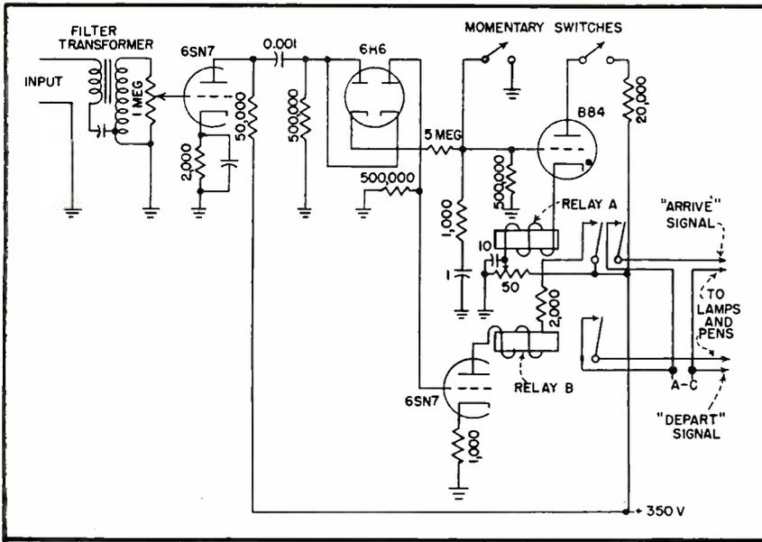
FIG. 3—The original indicating unit, showing just one of three identical channels
