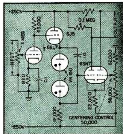
FIG. 3—Circuit of direct-coupled amplifier for an oscilloscope. The novel coupling system provides a response flat within one db to ten kilocycles
