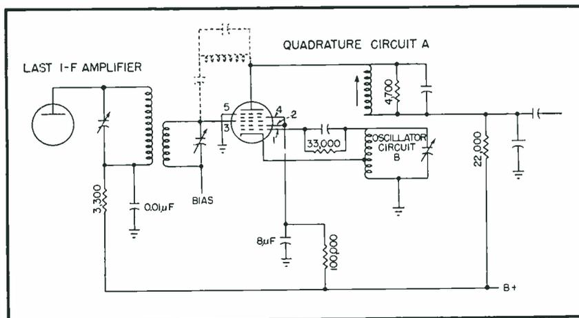
FIG. 1—Basic circuit of the f-m detector
