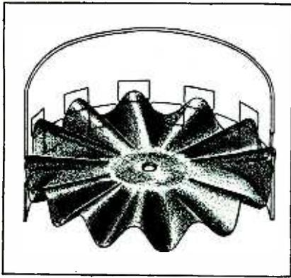
FIG. 3—Pictorial representation of the shape of the electron disc in the Phasitron tube. In this position, minimum current is collected at perforated anode No. 1
