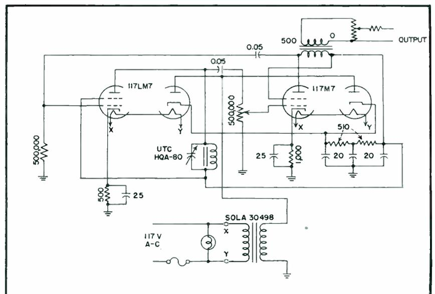
FIG. 2—Multivibrator-type audio oscillator circuit. One of these oscillators is used at each remote point
