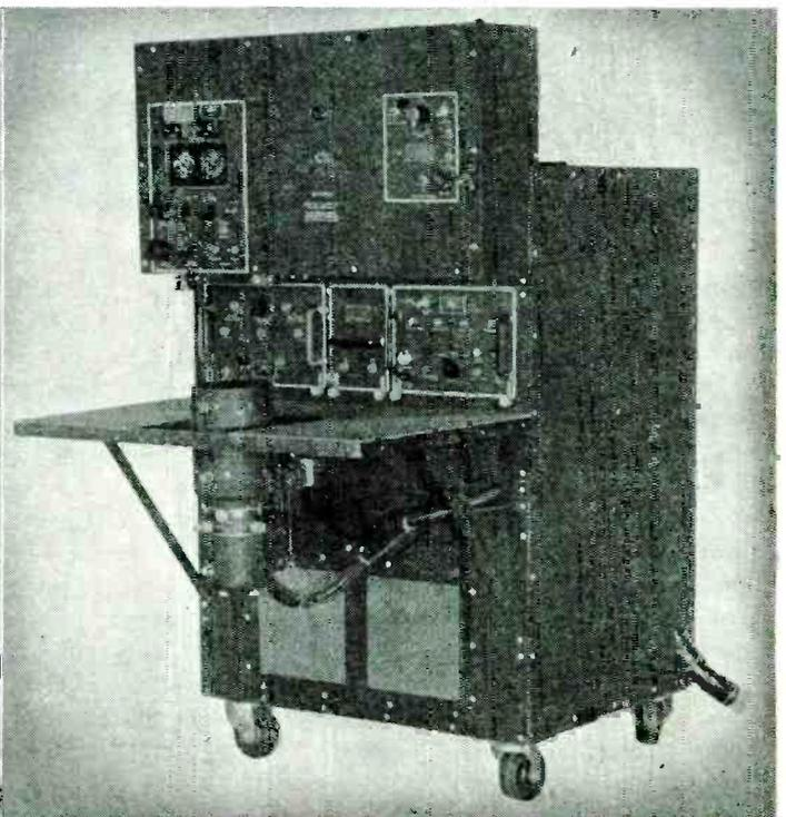
FIG. 4—Three-centimeter aircraft radar set mounted in weather station console designed by Signal Corps Engineering Labs and Air Materiel Command for storm detection
