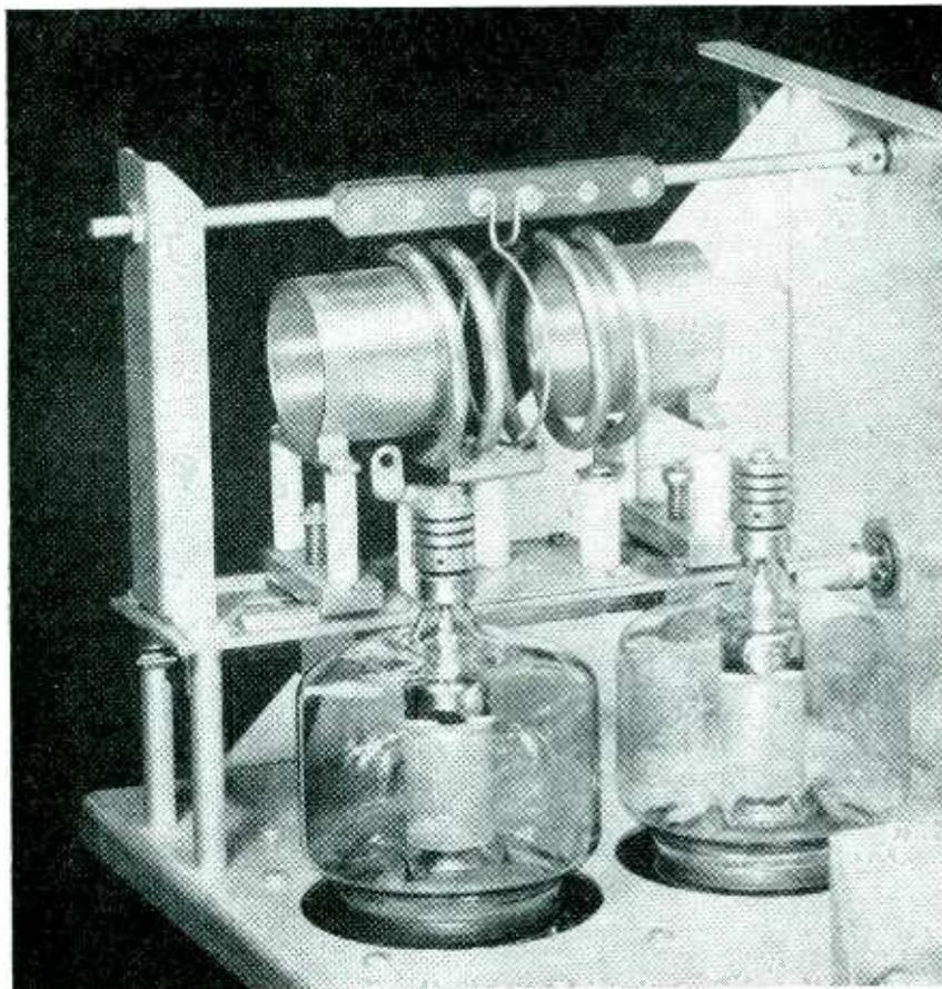
FIG. 8—Output stage of the 250-watt Phasitron f-m transmitter, showing the inductance-tuning arrangement consisting of two movable metallic cylinders in the plate circuit of the final amplifier. The output coil is shown between the two sections of the split tank coil
