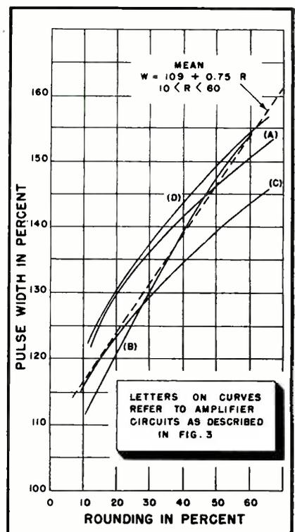
FIG. 6—Output pulse percent width as a function of percent rounding
