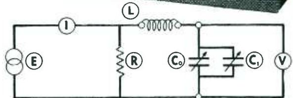
SIMPLIFIED LAYOUT AND SCHEMATIC OF THE 160-A Q-METER
