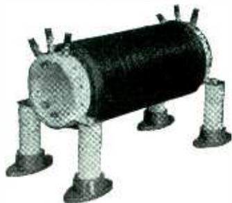
**LIGHTING FILTER.** The ANDREW Model 1803 lighting filter serves to connect the 60-cycle lighting voltage across the base insulator of a series excited tower without detuning the tower. Three windings provide for operation of code beacon and obstruction lights. Mica insulated by-pass condensers of ample current rating included. Also offered in weatherproof steel housing.
