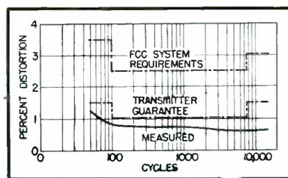
Graphical presentation of audio harmonic distortion versus frequency with respect to FCC requirements, transmitter guarantee and actual performance on the preproduction model
