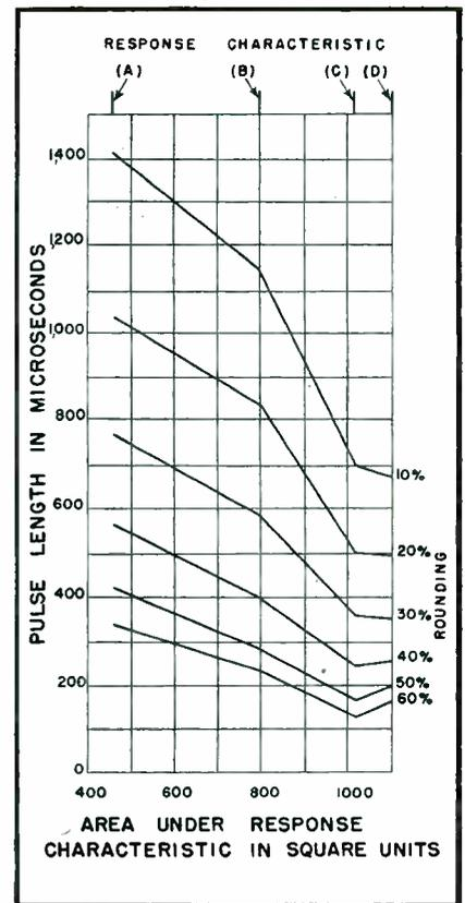
FIG. 8—Minimum pulse length expressed in terms of the area under response characteristic for several amplifiers at different percent rounding
