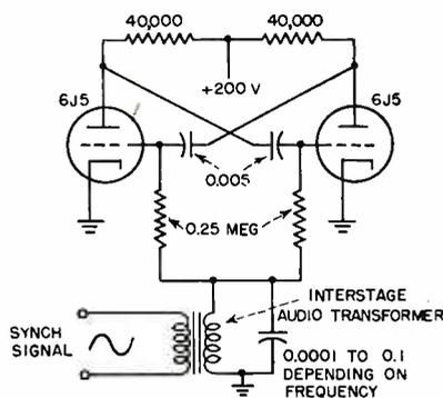
**SYNCH INPUT TO BOTH GRIDS**—Method of injecting synchronizing signal on both grids with the same phase. This circuit tends to favor even submultiples of the synchronizing frequency and should not be used when frequency ratio is one to one
