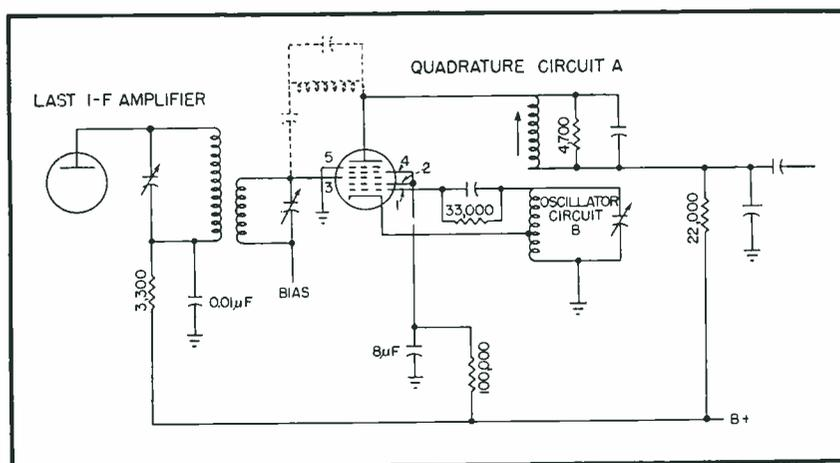
FIG. 1—Basic circuit of the f-m detector
