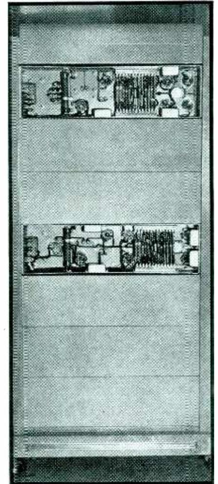
Audio signals having frequencies identified with fixed points along the rail lines are transmitted over wayside wires to a distant dispatcher. They pass through selective filters, amplifiers, trigger tubes and relays to signal lamps and pens which indicate and record time of arrival and departure
