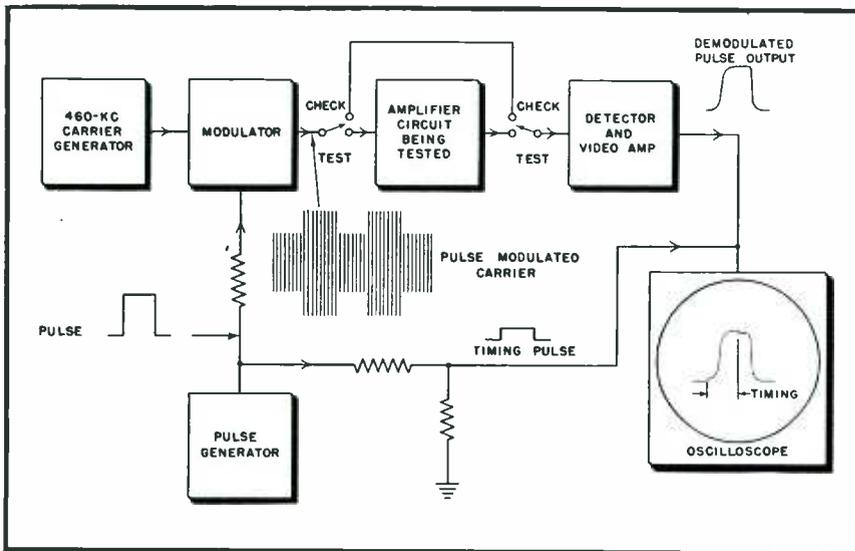
FIG. 1—Block diagram of the test equipment used in determining the response of amplifiers to pulsed signals. The pulse generator also supplies timing markers to the oscilloscope
