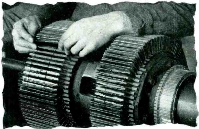
Irv-O-Slot provides the electrical protection necessary for top-quality slot insulation. Moreover, it possesses the mechanical strength required to withstand punishment received during motor assembly and operation. A complete range of varnished fabrics duplexed to selected rag and fish papers allows wide selection. All the base fabrics secure their high dielectric strength from uniform coatings of Irvington-formulated insulating varnishes.
