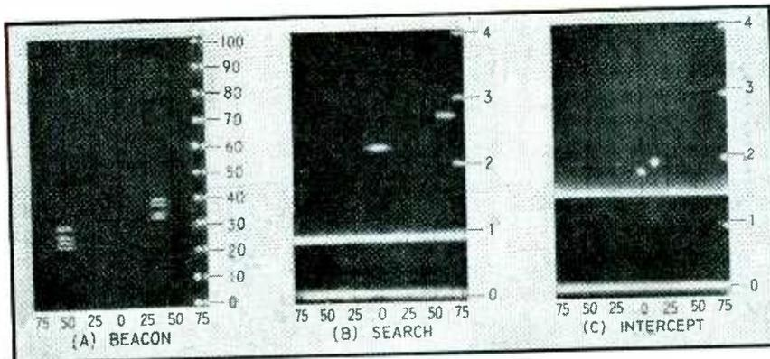
FIG. 1—Examples of indicator displays. Type-B scan is employed, with slant range to target shown along vertical axis. Bearing of target with respect to longitudinal axis of airplane is shown on horizontal scale. Circuits required are more compact than for ppi. With practice an operator can interpret the displays quite accurately
