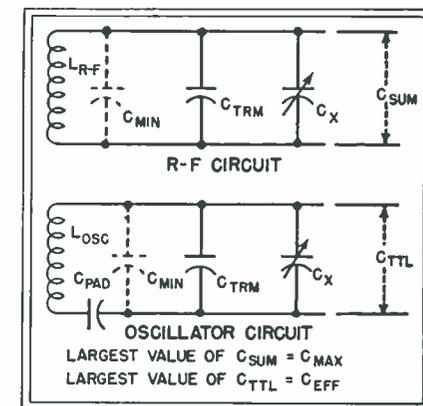
Fig. 1—Resonant circuits of oscillator and r-f input
