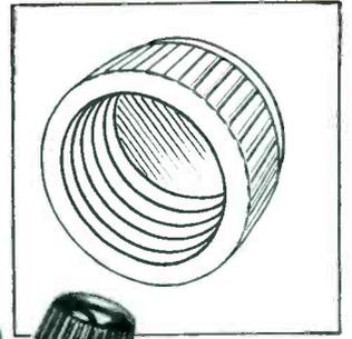
Tolerances of .001" must be held in the Molded threads of this piece, whose inside diameter is only 5/16 inch.
