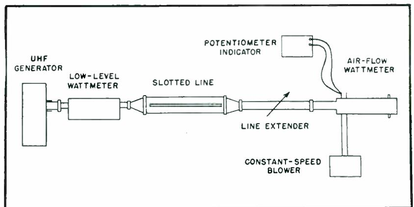
FIG. 3—Arrangement used for observing behavior of the wattmeter. It was found that it extracts very little power from a transmission line
