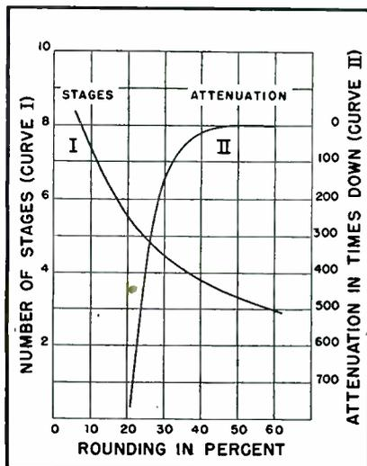
FIG. 7—Curves showing the number of stages needed and attenuation as a function of percent rounding for single-tuned amplifiers
