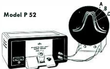
For rapid alignment of I.F. coils of frequencies from 85 kc to 11 mc. Operator adjusts test trace (B) to fall between traces of limit coils (A and C), set up to production specifications. Defective coils immediately detected. All error is eliminated as circuit changes or line voltage
