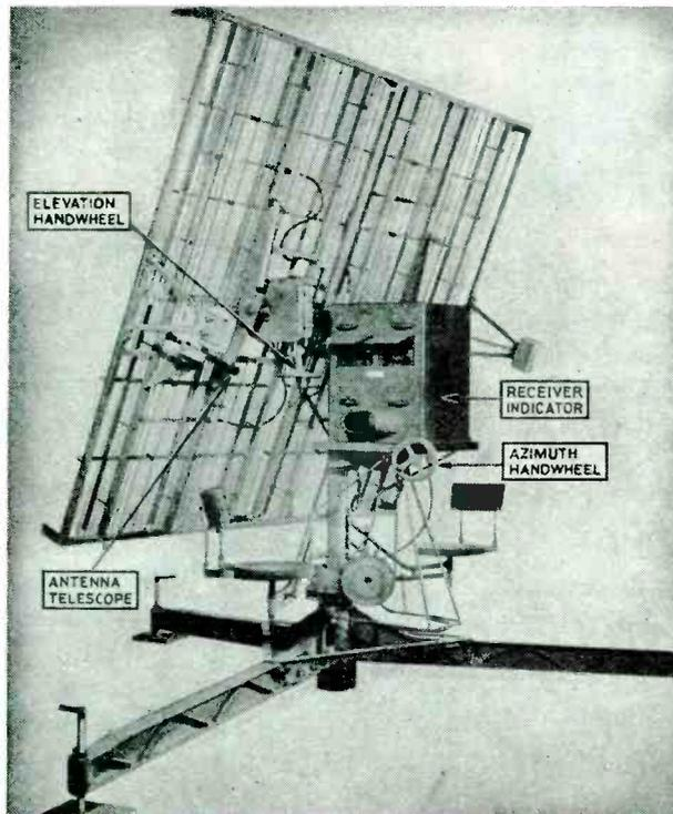
FIG. 3—This direction-finding receiver became standard equipment in the Air Weather Service for tracking balloon-borne radiosondes through clouds and darkness as well as in clear weather
