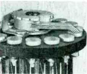
Quadruple-leaf, phosphor-bronze switches with wiping contact. Contact surfaces ground flat. Contact resistance only 0.002 ohm. Cam-type positive detent mechanism. Entire unit shielded behind panel.
