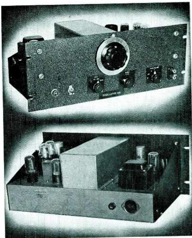
Front and rear views of stable low-frequency oscillator. Tuning dial in center of panel controls a three-gang potentiometer having special inverse square law taper to give a linear scale
