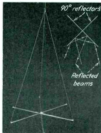
FIG. 2—Dipole target for 200-mc radar, and diagram showing how a target reflects incident beams back to their source
