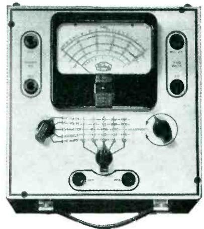
current range of the instrument is chosen by the setting of appropriate knobs. A separate knob is provided for three ohmmeter ranges
