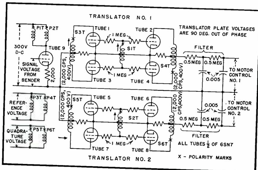
FIG. 4—Translator circuit converts phase signals from bender circuit into direct current signals for motor control
