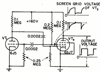
**MULTIVIBRATOR WITH CATHODE-COUPLED OUTPUT**—This circuit is useful because it has a low-impedance output and a steep wave front on the output signal. The addition of  $R_k$  affects the free-running frequency only slightly.
