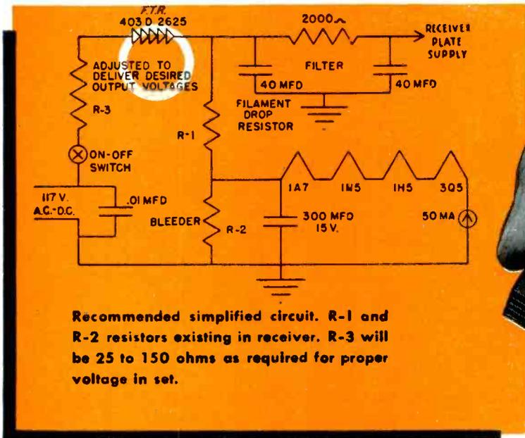
Recommended simplified circuit. R-1 and R-2 resistors existing in receiver. R-3 will be 25 to 150 ohms as required for proper voltage in set.
