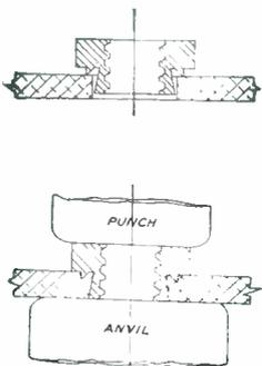
PEM Self-Clinching Fasteners solve assembly problems involving steel, aluminum, copper, or brass sheet. Because no special tools are required, PEM Self-Clinching Fasteners save time, labor, and weight; mean faster, more simplified clinching. For complete information, write to *Penn Engineering and Manufacturing Corporation, Doylestown, Pennsylvania.*
