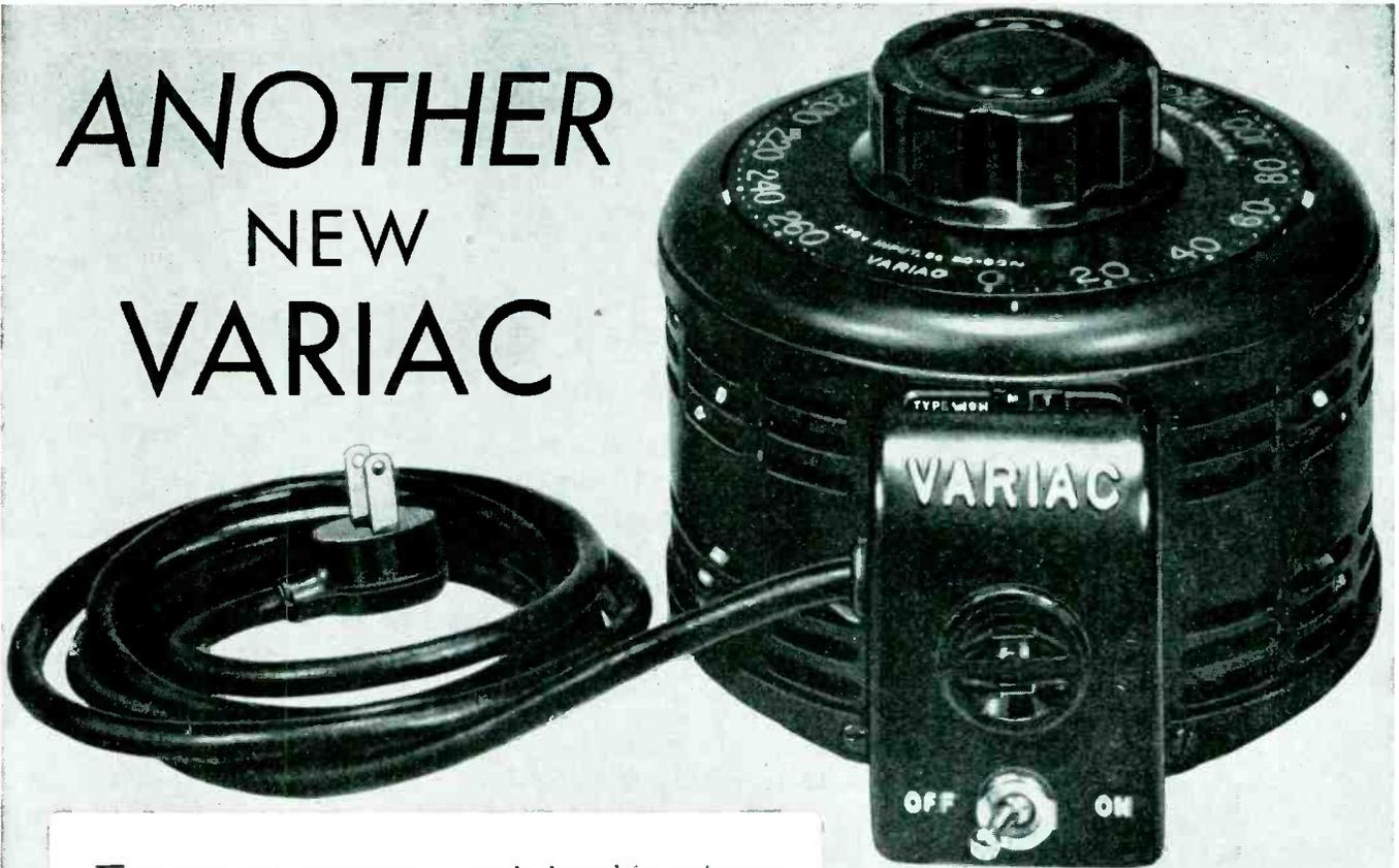
FOR some time there has been a steady demand for an intermediate size VARIAC . . . something between the new Type V-5 (old Type 200-C) with a 5 ampere rated output, and the Type 100 rated at 18 amperes. The new Type V-10 has been designed to supply this need. Its rated output is 10 amperes, with a maximum of 15. This maximum rating coincides with the capacity of outlets, plugs, cords and No. 14 circuits ordinarily found in the laboratory and in the home.
