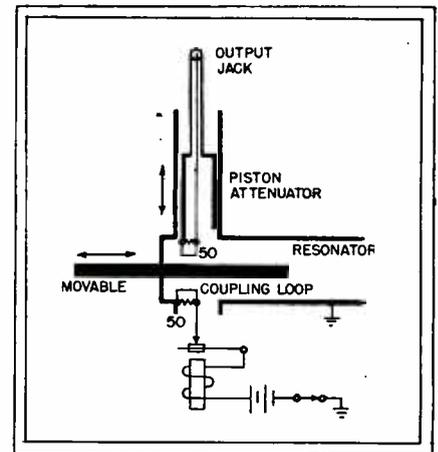
Circuit of simple microwave signal generator
