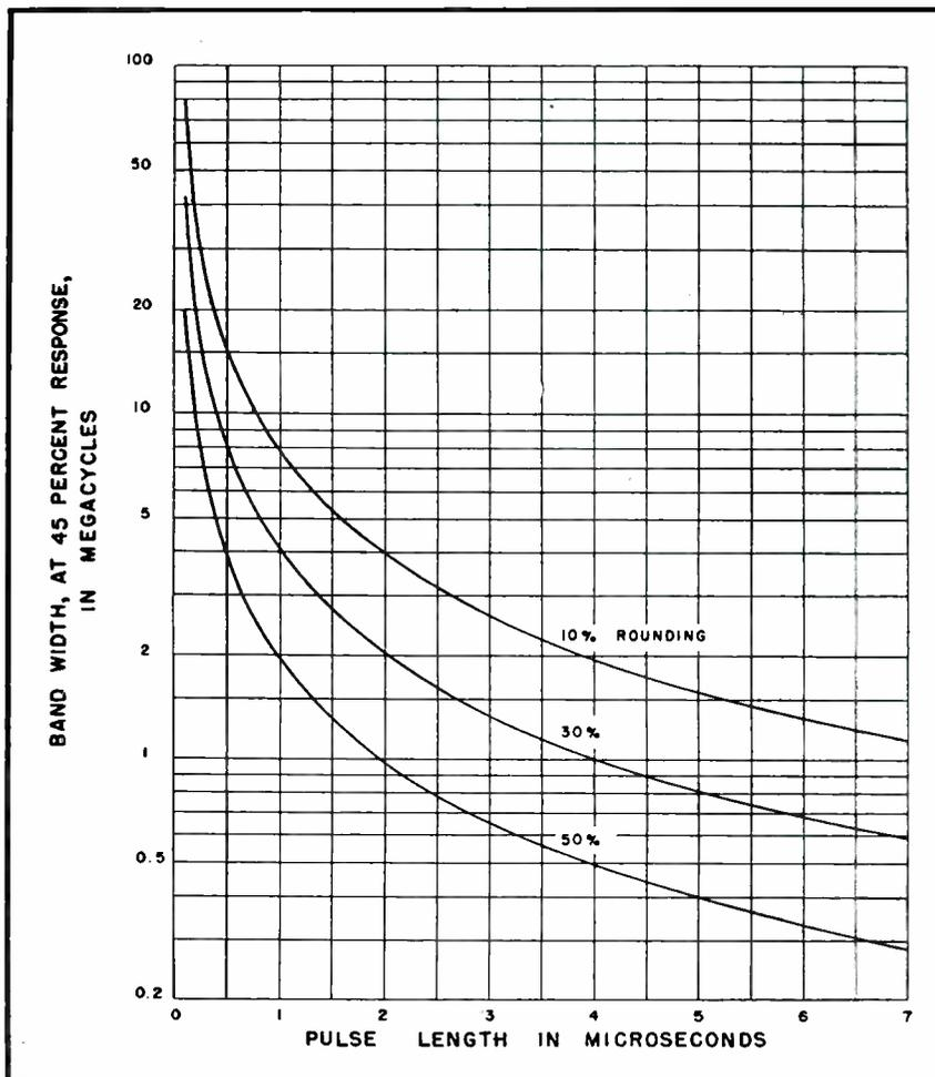
FIG. 11—Bandwidth required as a function of pulse length for three different percent rounding
