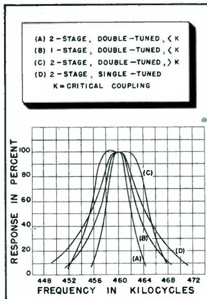
FIG. 3—Response characteristics of several amplifiers for steady-state or sine-wave amplification. The response to pulses is described in the text
