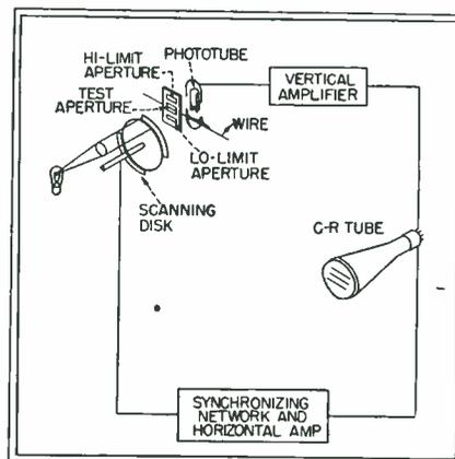
Essential units of the electronic micrometer for continuous examination of wire and strip thickness
