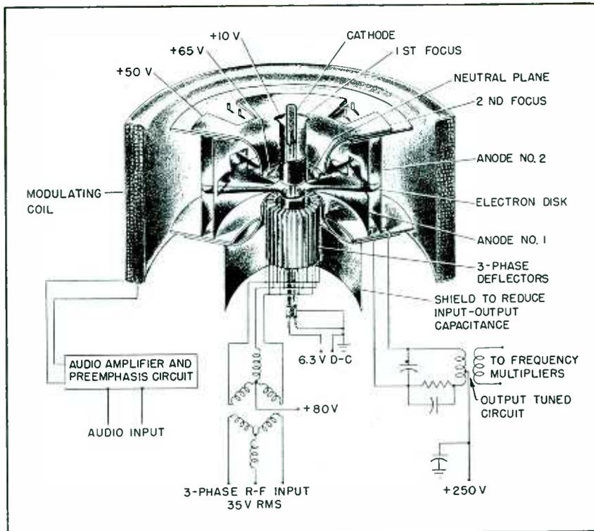
FIG. 2—Vertical section of the tube and modulator coil. Connection to a typical transmitter circuit is indicated
