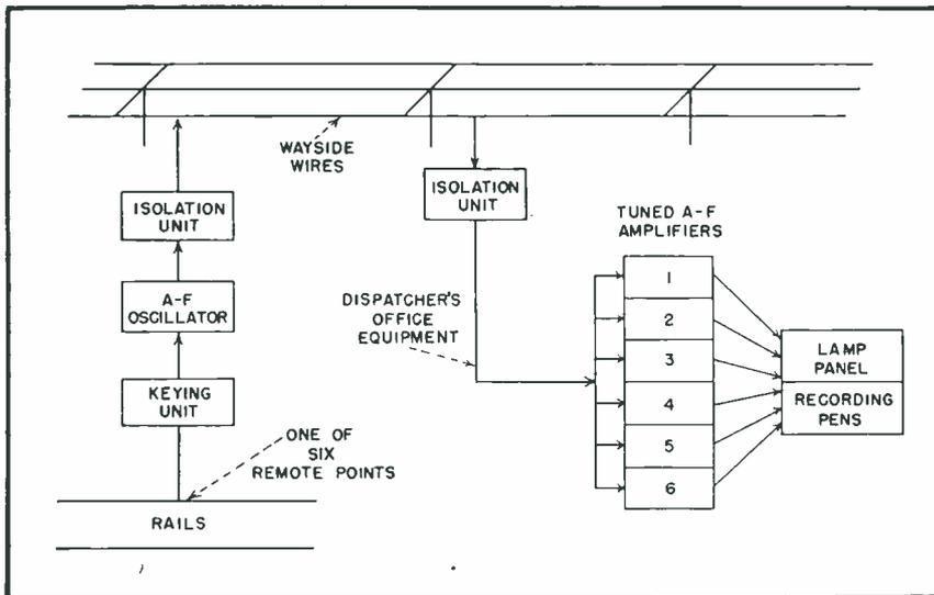
FIG. 1—Block diagram of the overall train-position indicator system installed in the vicinity of Bureau, Illinois
