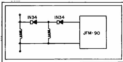
Fig. 2—Double converter for the JFM-90. The coils are ten turns of No. 16 wire on a 1/2-inch diameter form
