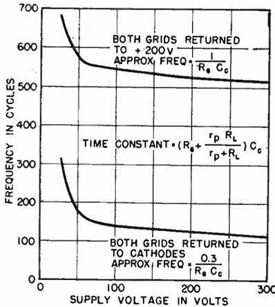
**EFFECT OF SUPPLY VOLTAGE ON FREQUENCY OF TYPICAL SYMMETRICAL MULTIVIBRATOR**—A multivibrator is relatively insensitive to changes in the supply voltage except when the supply voltage becomes quite low. The increase in frequency obtained by changing the grid returns from the cathodes to the plate supply lead is clearly shown. The amount of increase can be made greater by making the cathodes 2 or 3 volts positive
