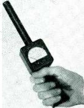
television, and electronic heating equipment operating at frequencies up to 1,500 megacycles. The probe element measures  $\frac{3}{8}$  inch in diameter and the overall length of probe and meter is 11 inches.
