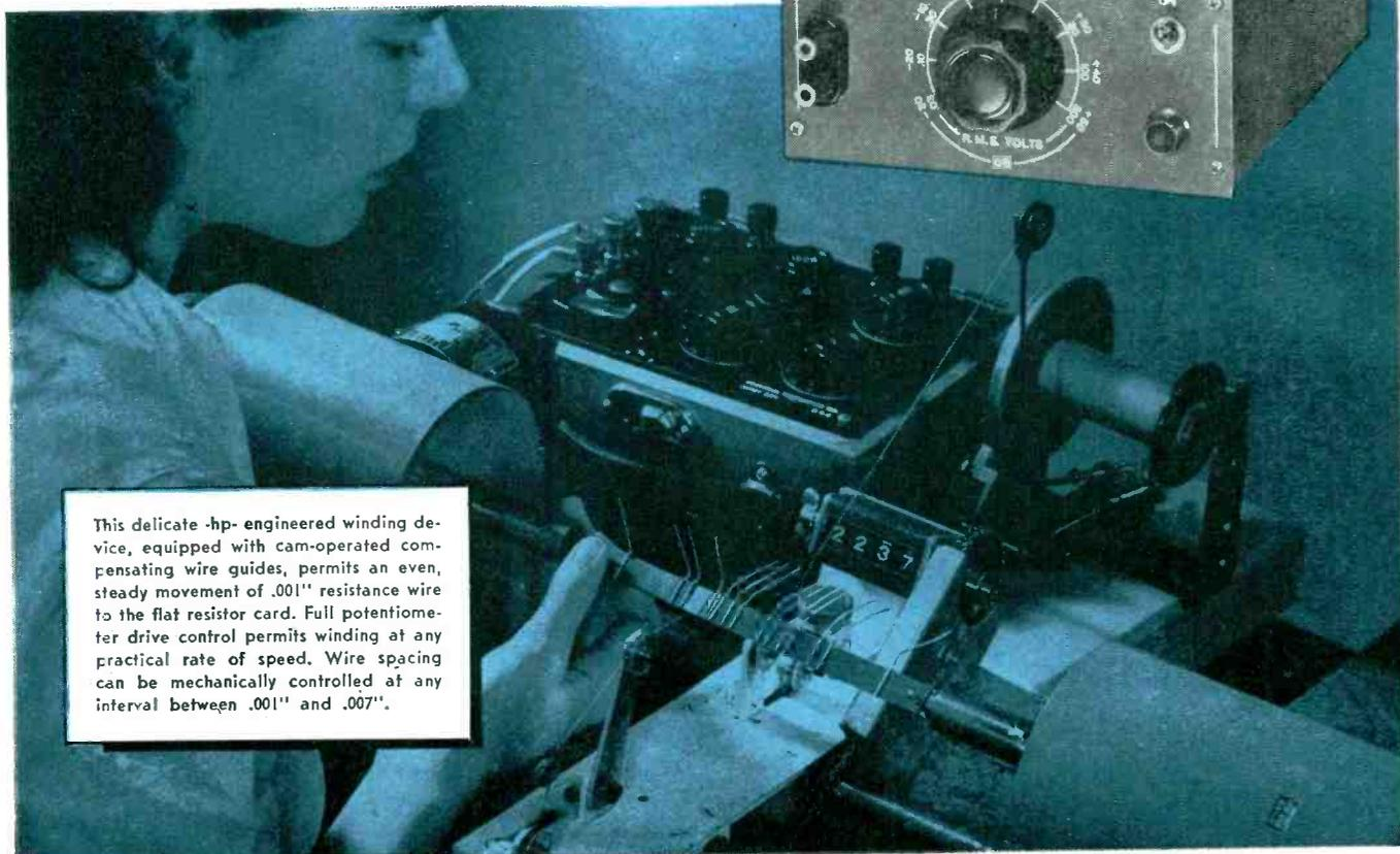
This delicate -hp- engineered winding device, equipped with cam-operated compensating wire guides, permits an even, steady movement of .001" resistance wire to the flat resistor card. Full potentiometer drive control permits winding at any practical rate of speed. Wire spacing can be mechanically controlled at any interval between .001" and .007".
