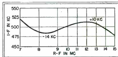
Fig. 2—Measured tracking error after alignment
