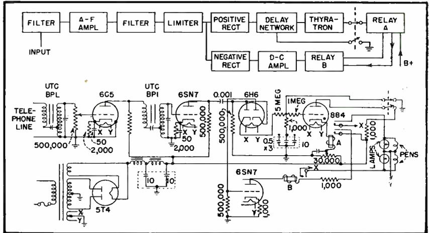
FIG. 4—The improved indicating unit, designed for increased selectivity and sensitivity
