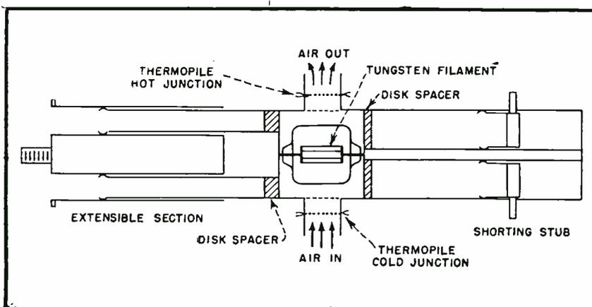
FIG. 1—Details of wattmeter unit. Disk spacers are made of insulating material having low dielectric loss at ultrahigh frequencies
