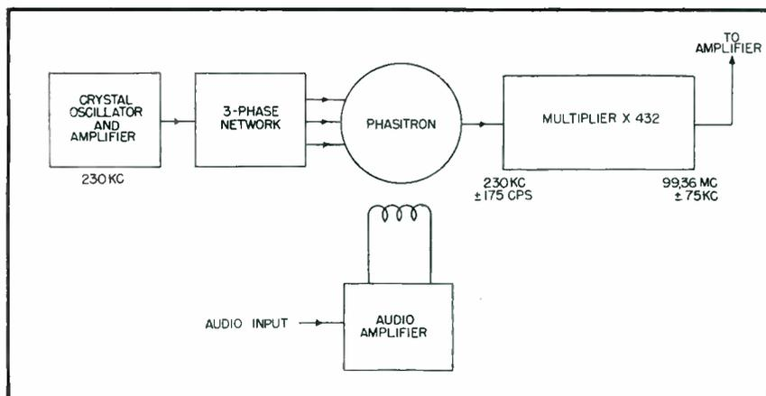
FIG. 1—Block diagram showing the use of the phasitron tube in an f-m transmitter
