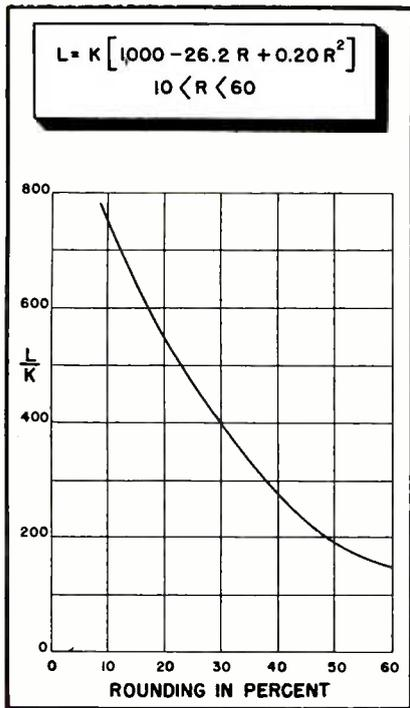
FIG. 5—Graphical representation of Eq. 5 showing percent rounding in relation to the quotient of pulse length divided by circuit response to sine waves
