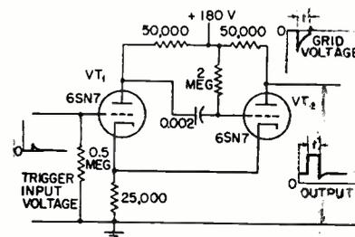
**CATHODE-COUPLED ONE-SHOT MULTIVIBRATOR**—Circuit values are adjusted so that  $VT_1$  is cut off when  $VT_2$  is conducting. The trigger signal interrupts this stable condition, but after the period  $t$ , the circuit automatically returns to the stable condition. If the grid return of  $VT_2$  is made to cathode instead of to +180 volts, a somewhat longer period is obtained. This circuit has the advantage that the triggering circuit is isolated from the multivibrator circuit by  $VT_1$
