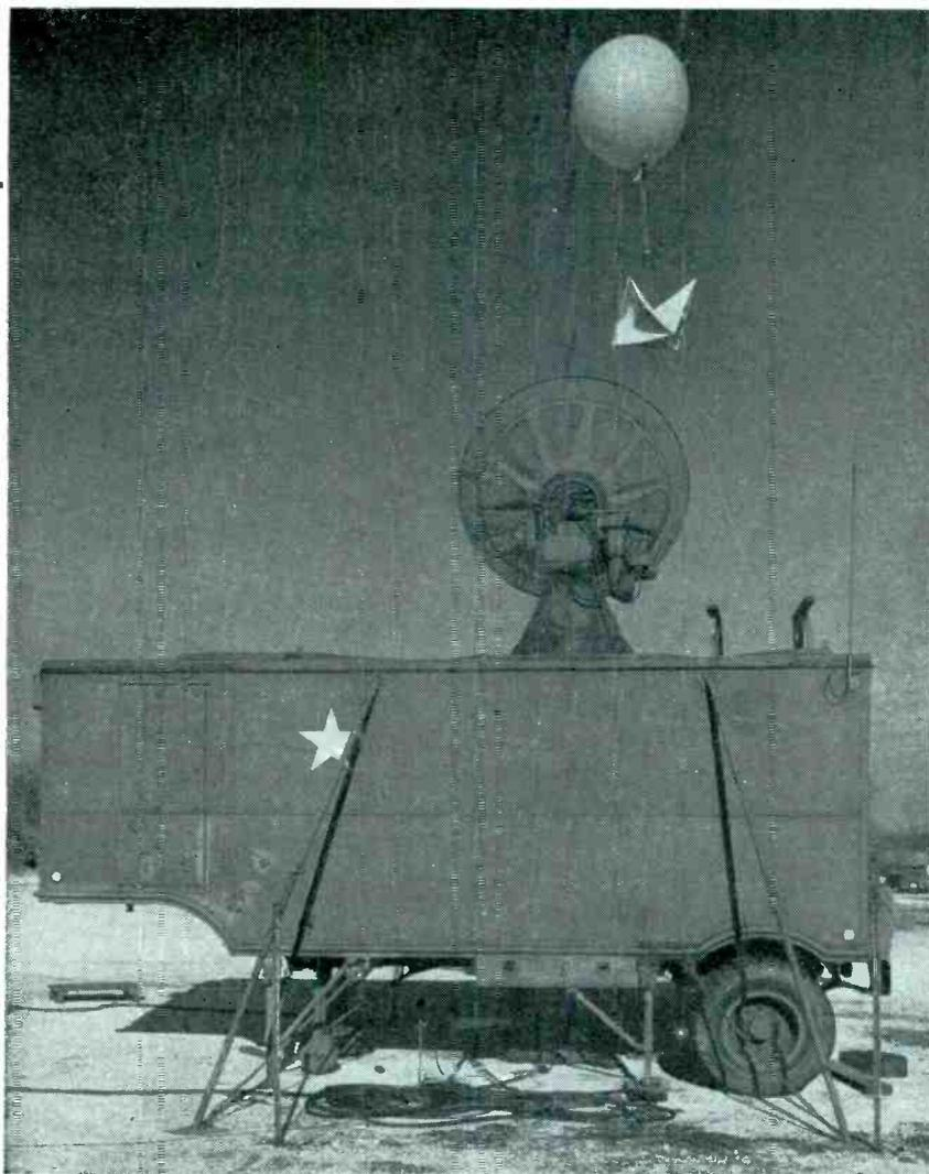
Two operators and this 11-cm radar can track a weather balloon through clouds and darkness to 100,000 yards range if the balloon carries a gable target like that shown aloft here
