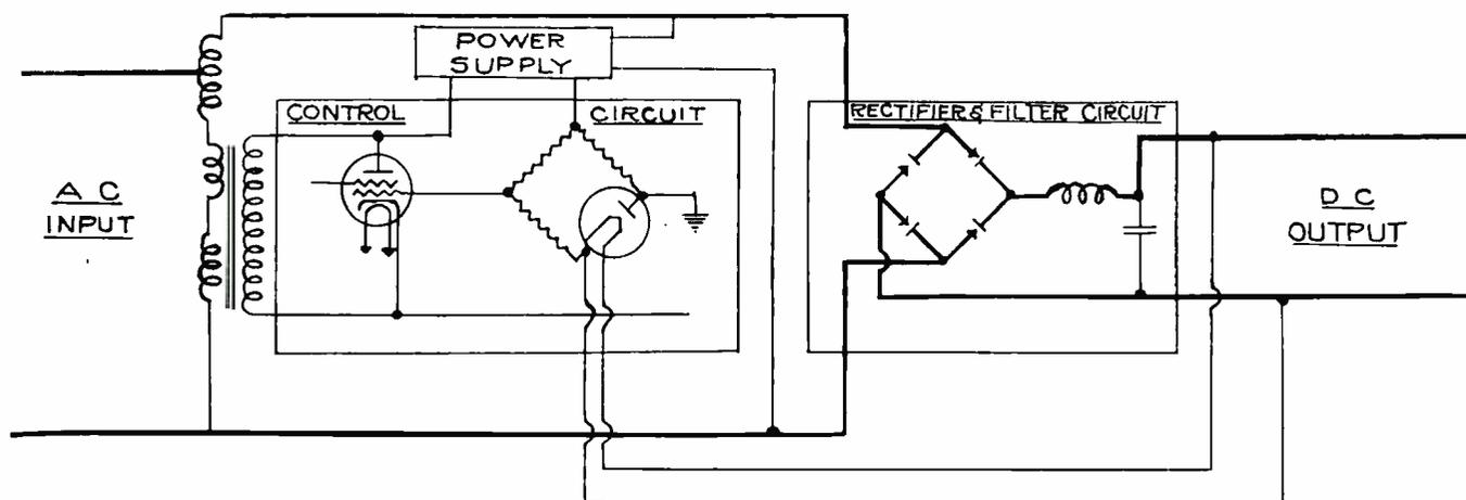
Based upon an adaptation of the principle of the Sorensen AC Regulator, the DC VOLTAGE REGULATED POWER-SUPPLY UNITS will maintain DC output voltage with an accuracy of plus or minus 0.5%. These units are available in 5, 10 and 15 ampere sizes at either 6 or 12 volts nominal output; the DC Regulators have the following general characteristics:
