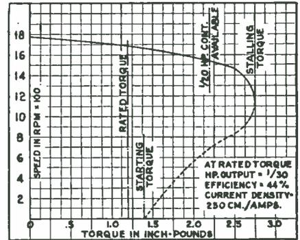
*Type ALP-191; 110 volt 60 cyc. single-phase Capacitor start & run; Motor Capacitor Value 4.25 Mfd. Curve # 235.*
