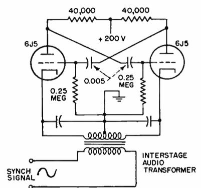
**SYNCH INPUT TO BOTH CATHODES**—Method of injecting the synchronizing signal so that it is out of phase on the cathodes. This circuit tends to favor odd submultiples of the synchronizing frequency applied through the transformer
