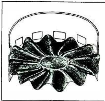
FIG. 4—Position of the electron disk for maximum current collected at anode No. 1 as a result of modulation by the magnetic coil
