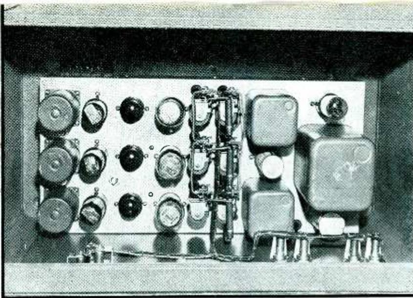
Interior of an early three-channel unit, one of two such units used by a dispatcher at Bureau, Illinois. The circuit for one of the channels is shown in Fig. 1
