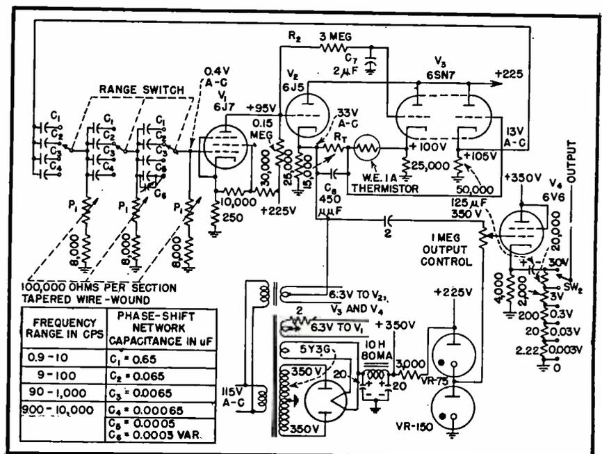
FIG. 2—Complete circuit of practical phase-shift oscillator
