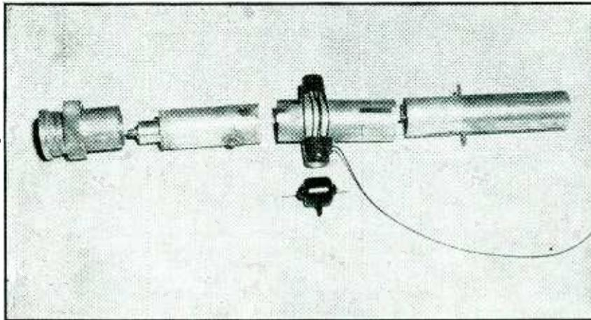
Dismantled sections of the wattmeter, arranged to correspond with the drawing of Fig. 1 and showing mechanical details
