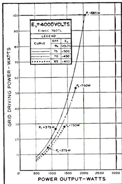
At frequencies below 40 mc, or as a Class-B modulator, the 750TL operates at high plate efficiencies, thus permitting r-f and a-f outputs of many times the plate dissipation rating.
