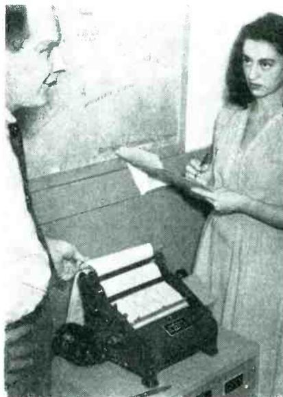
Facsimile receiver at Waltham recording a map of repeater station locations over Raytheon 4,000-mc relay circuit from transmitter in New York
