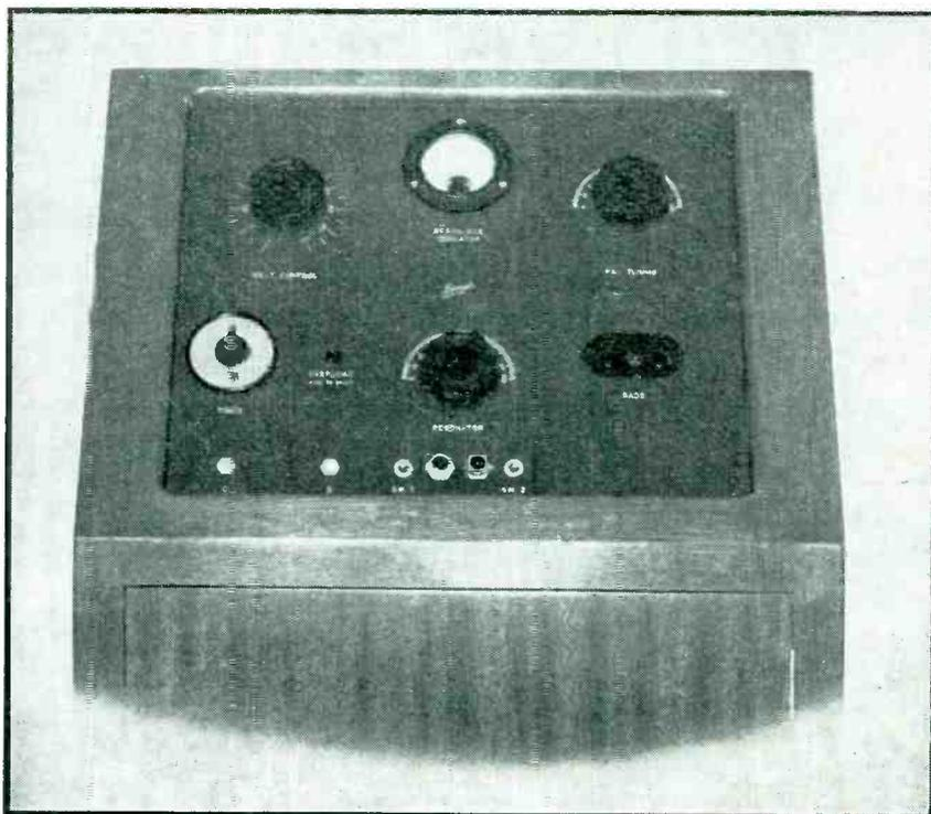
Front view of the upper portion of the diathermy cabinet, showing the control panel Underneath the r-f chassis. The crystal-stage components are separated by the chassis from the final amplifier plate circuit to avoid feedback
