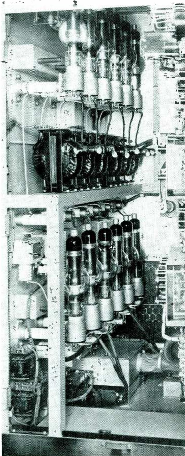
Dual thyatron rectifier bank used in 100-kw industrial r-f generator
