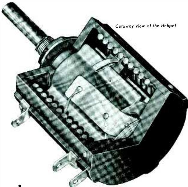
Cutaway view of the Helipot
