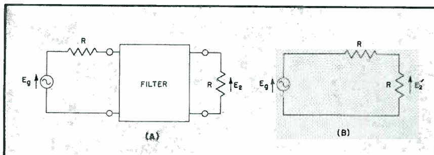
FIG. 1—Significance of insertion ratio, which is ratio of load voltages without filter to load voltage obtained with filter between source and load
