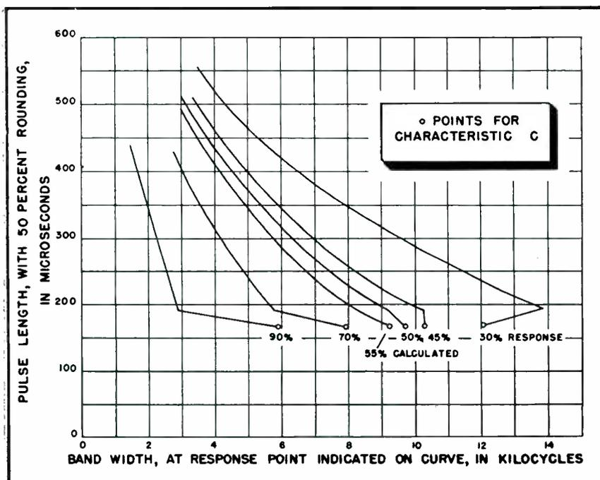
FIG. 9—Permissible pulse length as a function of bandwidth
