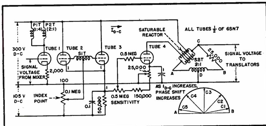
FIG. 3—Bender circuit introduces a phase shift so that drive direction is proportional to amplitude of stylus deflection
