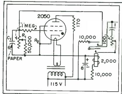
FIG. 1—Circuit of electronic timer that has a number of industrial applications
