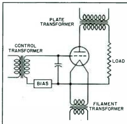
FIG. 1—Basic circuit of single-phase half-wave thyatron rectifier
