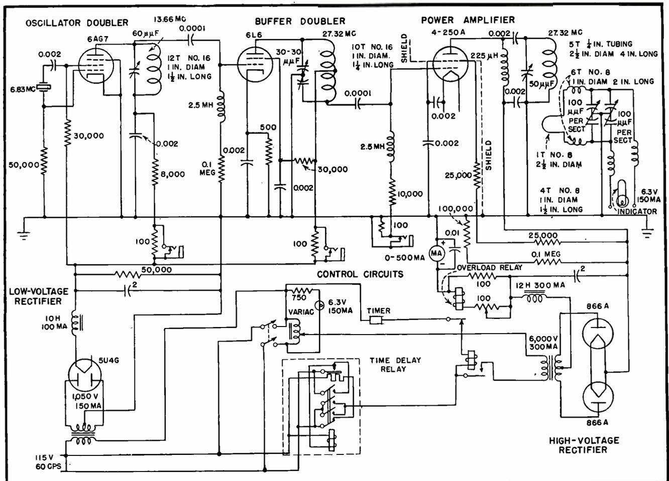
FIG. 2—Schematic circuit diagram of the three-stage r-f heater. Filament power supplies have been omitted. Power supply at the left serves the oscillator and buffer stages
