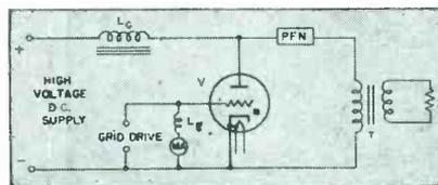
$L_g$  Grid Choke                      T Matching or Pulse
