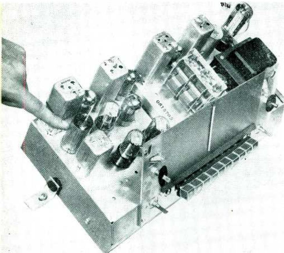
Receiver chassis utilizing the new f-m detector. The shield can at extreme left contains the step-down i-f transformer that feeds the FM 1000 tube; the oscillator and quadrature circuits are in the can below the tube
