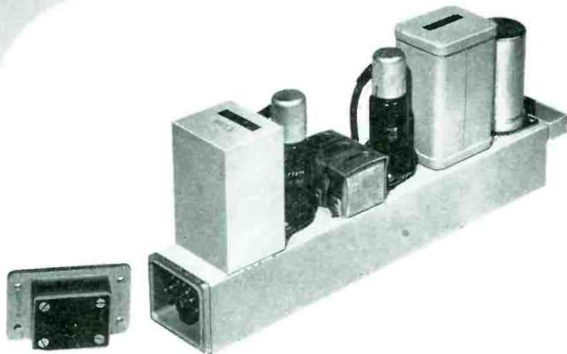
The Type 116-A has been designed for use as a microphone preliminary and as a booster amplifier—gain 36 db. Operates from source impedance of 150/600 ohms and into load impedance of 150/600 ohms, in accordance with RMA proposed standards.
