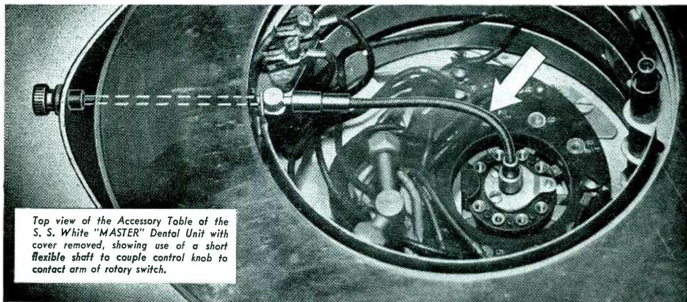
Top view of the Accessory Table of the S. S. White "MASTER" Dental Unit with cover removed, showing use of a short flexible shaft to couple control knob to contact arm of rotary switch.
