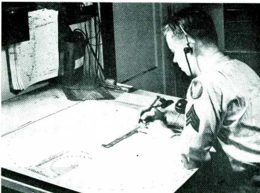
Plotting the horizontal track of an ascending weather balloon from radar indications
