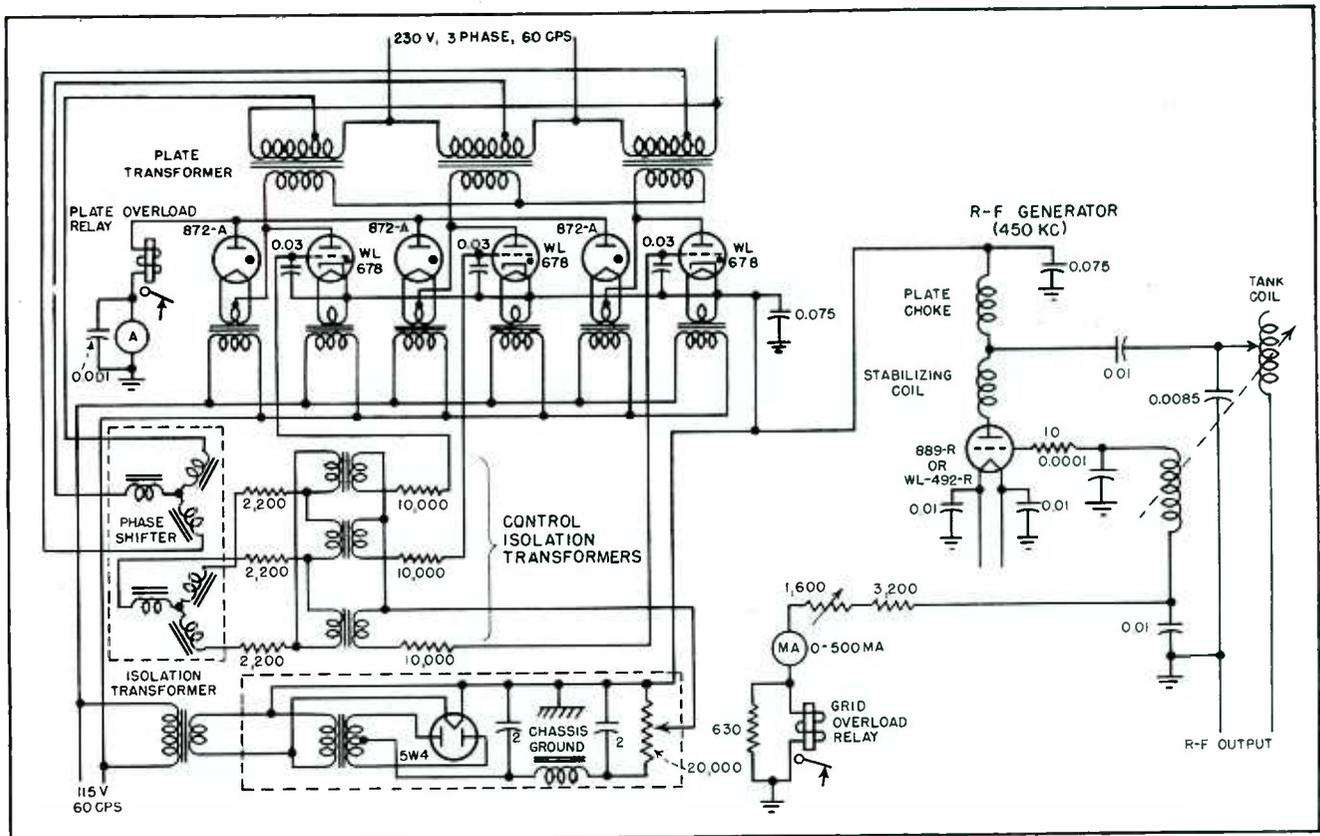
FIG. 3—Simplified schematic circuit diagram of grid-controlled rectifier as used with a 10-kw, 450-kc r-f generator
