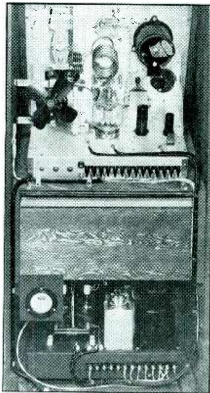
FIG. 1—Rear view of the diathermy unit with cover removed. Power supplies are at the bottom. The fan on the r-f unit draws air past the tube base and exhausts it through a hole in the rear
