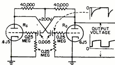
**SQUARE-WAVE MULTIVIBRATOR**—Addition of resistors  $R_C$  to the symmetrical circuit results in a plate-voltage waveform which is approximately a square wave. The frequency of oscillation is affected only slightly by the addition of these resistors
