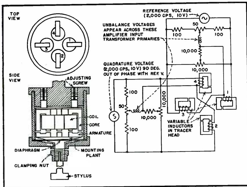
FIG. 2—Mechanical and electrical diagrams of tracer head, including its associated bridge circuit, indicate how stylus movement generates signals
