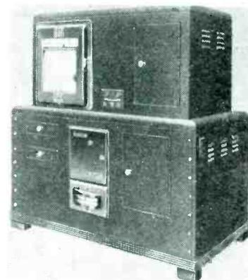
hour expansion and contraction cycles of samples, a new dilatometer accommodates temperatures up to 1,000 C held to within 1 C. Its oper-
