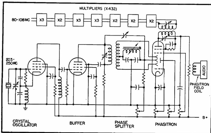
FIG. 6—Simplified block diagram of a crystal-controlled, phasitron-modulated broadcast transmitter. Audio modulation is introduced through the field coil that surrounds the new tube
