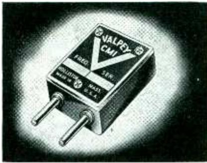
The CM1 and other VALPEY crystals offer the highest performance available for all Marine frequencies. The CM1 features Standard and GR pins with exact 3/4", .875" or .850" pin spacing. Sealed against salt water corrosion. Answers all manufacturer's specifications . . . ideal for replacements.
