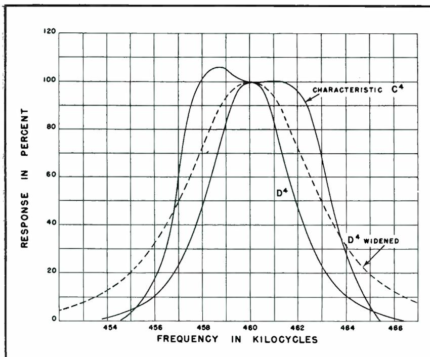
FIG. 10—Transmission characteristics of an 8-stage amplifier
