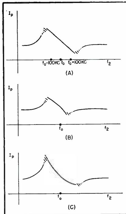
FIG. 3—Adjustment of the phasing circuit produces these curves of plate current plotted against frequency
