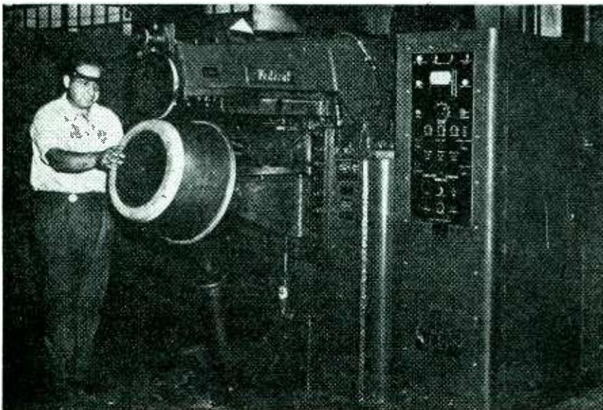
Roll spot welder, reported to be the world's largest, uses electronic rectifiers to charge 84 120- $\mu$ i capacitors that discharge into welding transformers. Westinghouse electronic controls permit 300 welds per minute on sheets of 0.032-inch aluminum
