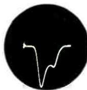
The HAR-CAM Visual Alignment Signal Generator instantly shows up the misalignment in the I-F circuit shown above.
