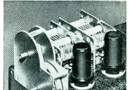
Converter using twin ganged tuning capacitors
