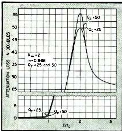
FIG. 4—Attenuation curve of network for two values of  $Q$ ;  $m = 0.866$
