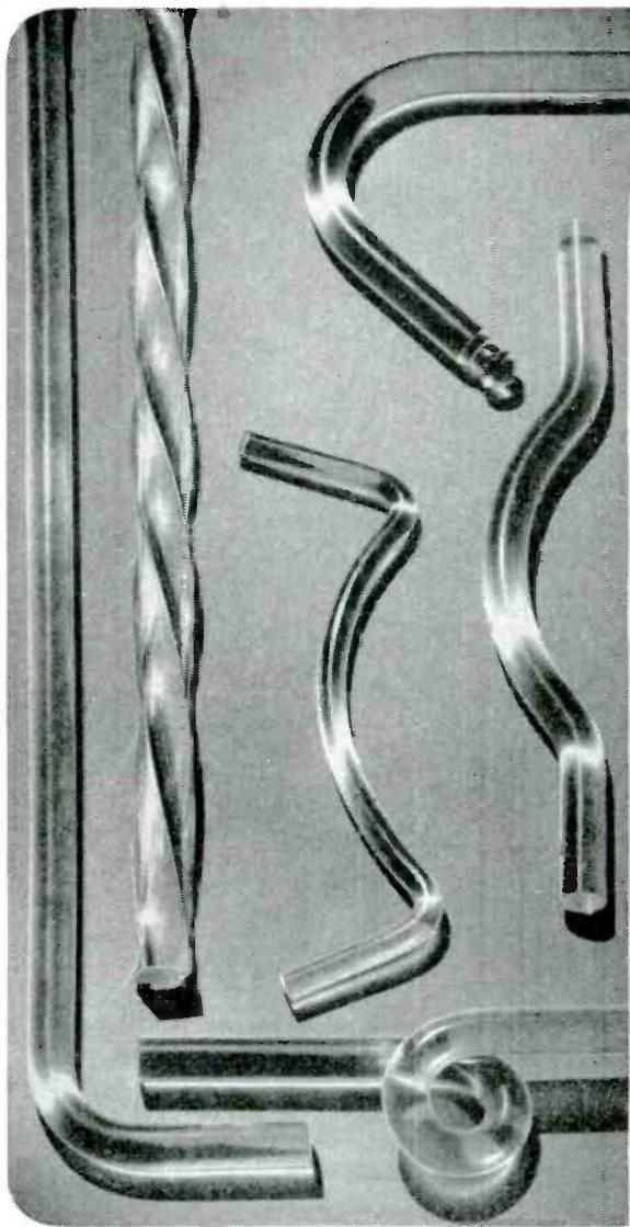
Plax crystal polished polystyrene rod can be heat formed without difficulty into many shapes and intricate bends. Correct forming techniques should be closely observed.
