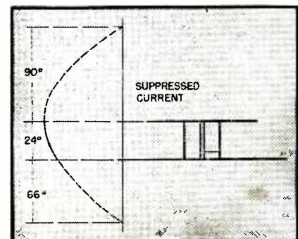
FIG. 3—Vertical distribution of antenna current
