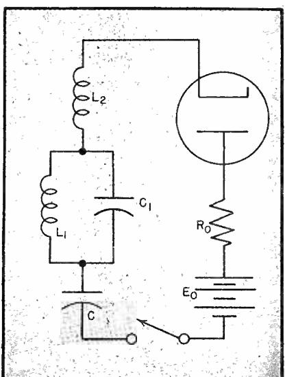
FIG. 8—A corrective network can be made entirely of reactive elements
