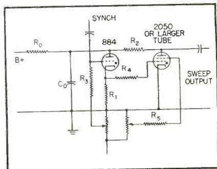
Sawtooth oscillator circuit combining advantages of 884 and 2050 to obtain rapid return trace of beam in c-r tube
