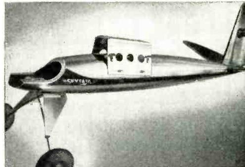
P-K binding head Type "Z" Screws fasten cabane to fuselage. Slots permit wing assembly to be moved back when model is changed over from "Class B" to "Class C", with heavier motor.
