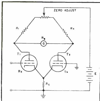
FIG. 1—Basic bridge-type vacuum-tube voltmeter circuit used with radiation pyrometer for flame radiation measurements
