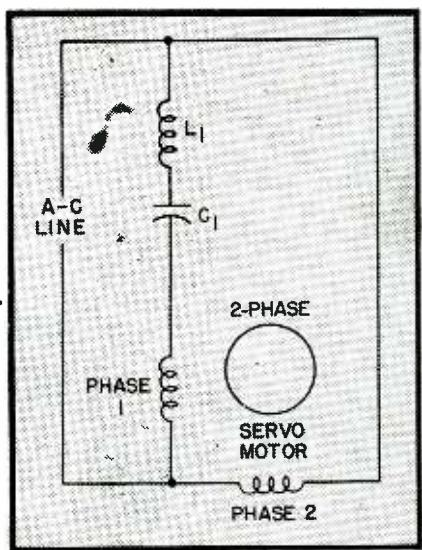
FIG. 2—The resonant circuit formed by  $L_1$  and  $C_1$  controls the current flowing through the motor winding of phase 1
