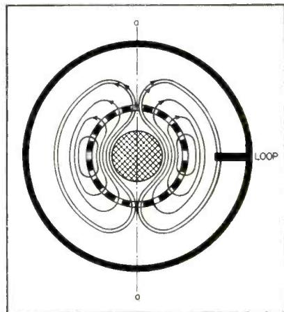
FIG. 2—Because the magnetic field links the squirrel cage, the size of the tube shell cavity does not appreciably affect the resonant frequency
