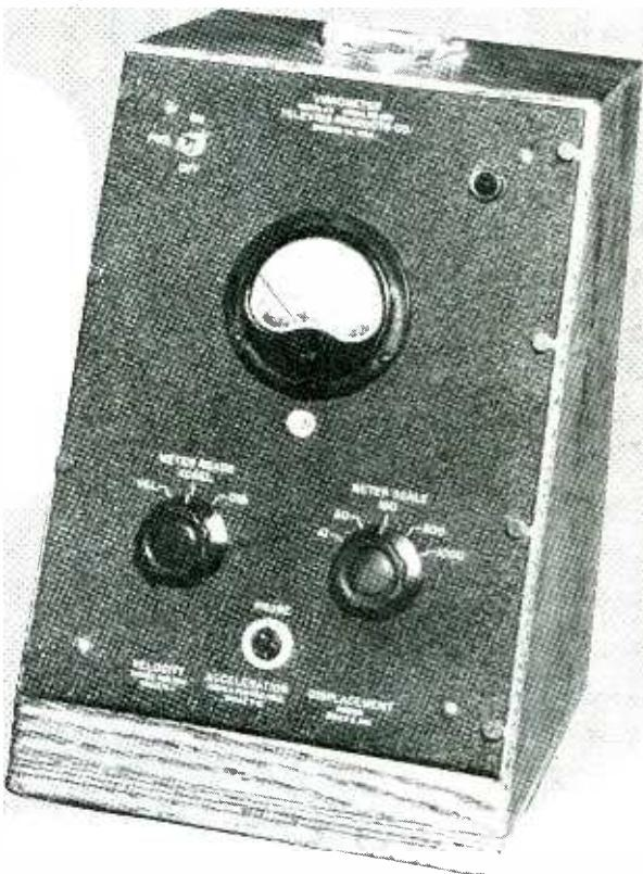
● The Televiso Model 11-B Vibrometer electronically measures the vibration characteristics of any moving surface instantly and accurately. Unnecessary wear, strain and noise no longer need be tolerated in industrial machinery, and in the integral parts of products.
