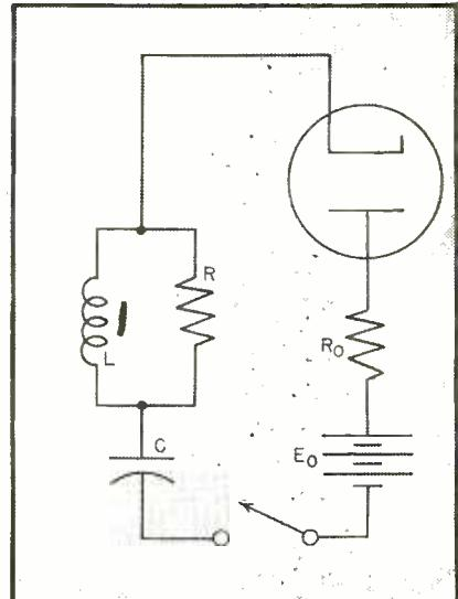
FIG. 2—A biased diode can be a part of the load through which constant current is passed
