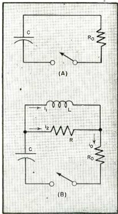
FIG. 1—(A) Exponential circuit, and (B) compensated circuit from which constant current can be obtained
