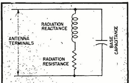
FIG. 4—Equivalent circuit of antenna as seen from its input
