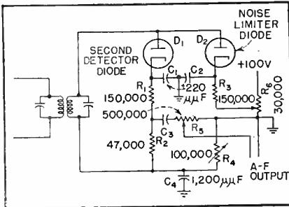
FIG. 7—Balanced-detector noise limiter
