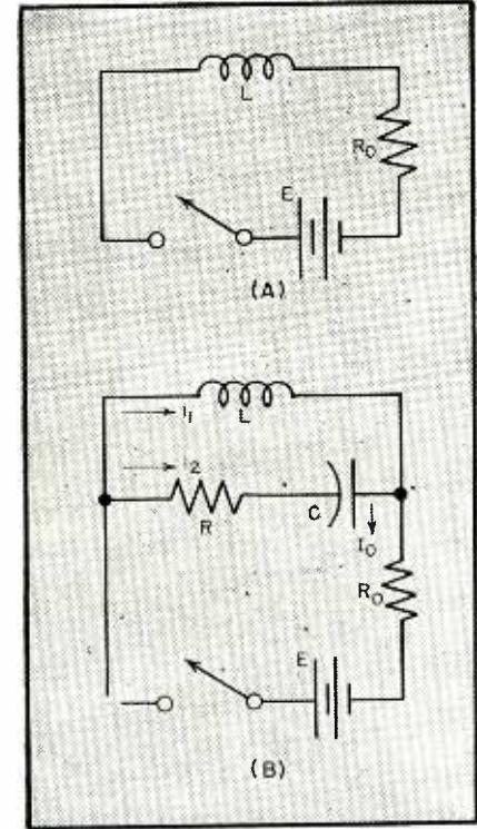
FIG. 4—(A) An inductor can replace the capacitor of Fig. 3. Corrective network (B) contains inductance
