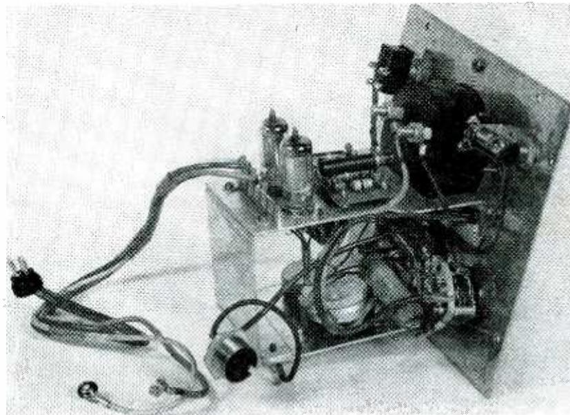
Chassis of vacuum-tube voltmeter used to measure output voltage of radiation pyrometer. Battery and pyrometer connections are at left
