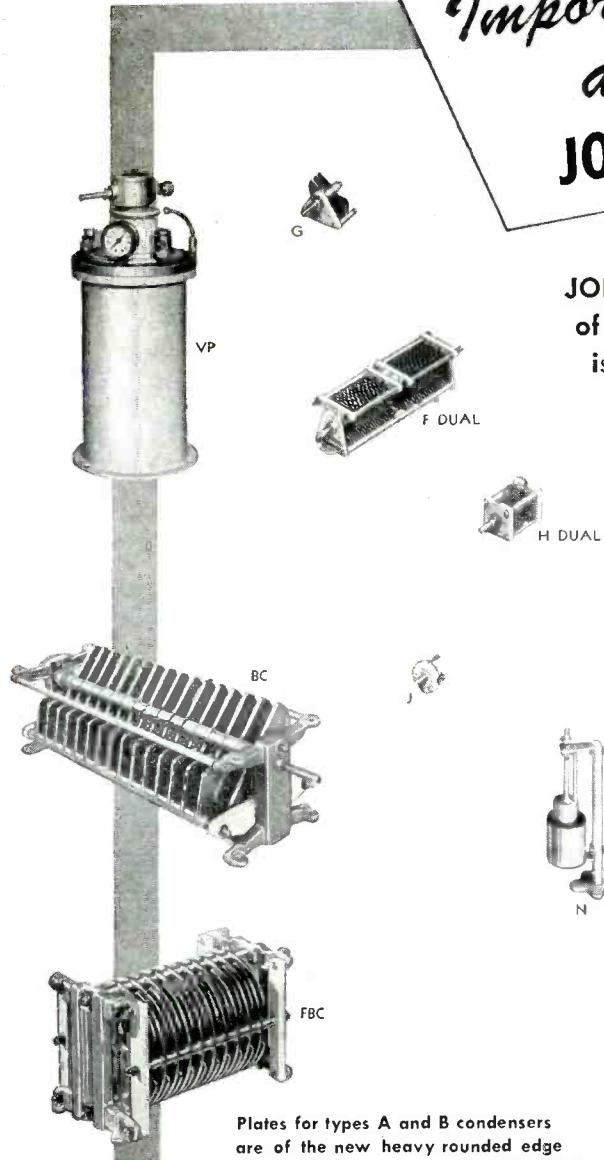
Plates for types A and B condensers are of the new heavy rounded edge design recently developed by JOHNSON engineers. Their higher breakdown voltage permits closer spacing, a shorter condenser, lower minimum, and less inductance at UHF. These features combined with new end frame design reduce weight to minimum, yet cost no more, in most cases less because of the saving in material.
