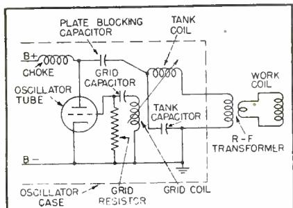
FIG. 1—Basic oscillator circuit, showing the variably coupled plate and grid coils. The r-f transformer is actually a part of the oscillator circuit but is located near the work
