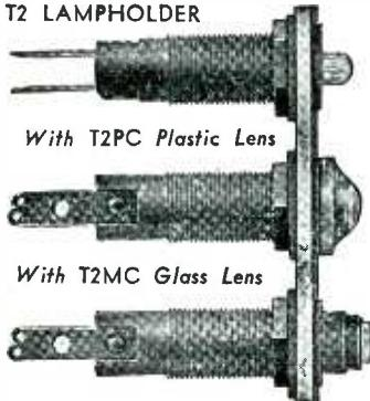
T2 lampholder, molded of bakelite, holding lip, dia. 11/16". Tip of lamp bulb protrudes sufficiently to be removed from front of panel without use of special tool.
