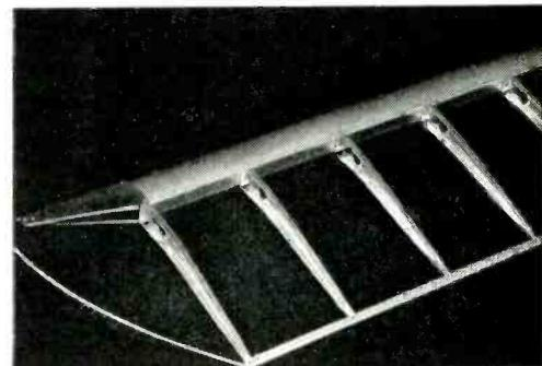
There are 15 P-K Self-tapping Type "Z" Screws in each wing structure, fastening spar, ribs, leading edge and tip securely together.
