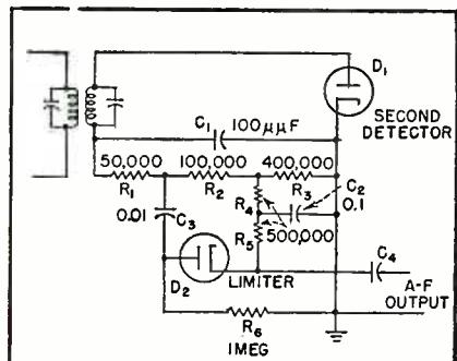
FIG. 5—Low-loss series limiter, requiring three more components than the simplest version in Fig. 1
