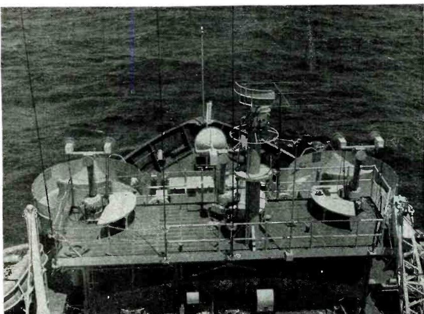
Bow of the USS Avery Island, showing radar platform from rear. Vertical whip antennas were used to monitor c-w transmissions on 5 to 15-mc from target ships
