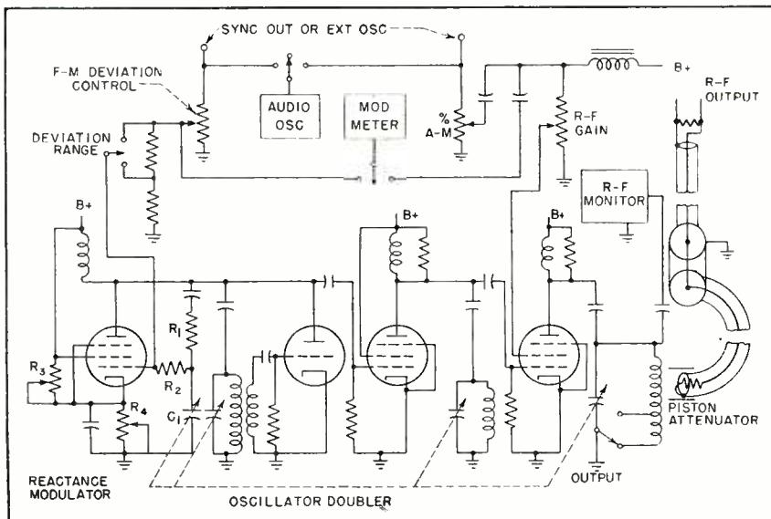
FIG. 8. Simplified diagram of the f-m signal generator
