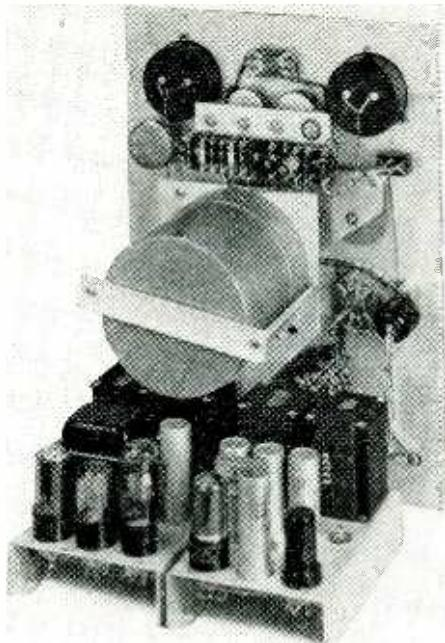
Front and rear views of the signal generator. Frequency deviation and percent of amplitude modulation are controlled by two potentiometers below the modulation meter switch. On the tuning dial, the vernier scale changes the frequency by about 26 kc on the low-frequency range and 52 kc on the high range. Choice of modulating frequency is provided by the dial at lower left and output from 0.0000001 to 0.2 volt is controlled by the attenuator dial at lower right.
