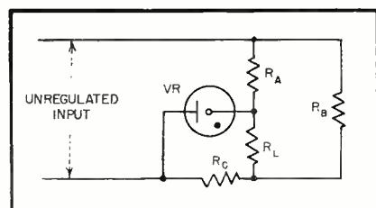
FIG. 6—Improved gaseous tube stabilizer circuit makes voltage across load resistance independent of input over a wide voltage range
