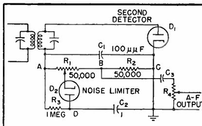
FIG. 11—Diode shunt-type noise limiter
