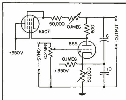
FIG. 3—Complete circuit of laboratory sweep generator whose output is linear
