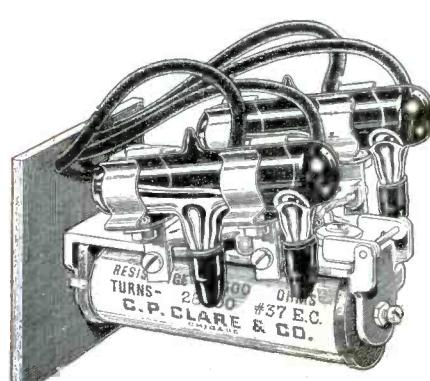
**Clare Mercury Contact Relay**—Shown above is a Clare Type "M2" Mercury contact relay with glass enclosed contacts. The mercury contact is mounted on a tilt table attached to the heelpiece of the relay. These relays must be mounted horizontally. Clare also provides Mercury contact relays with Bakelite enclosed contacts and with metal contacts.
