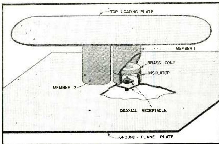
FIG. 1—Cutaway shows method of feeding antenna
