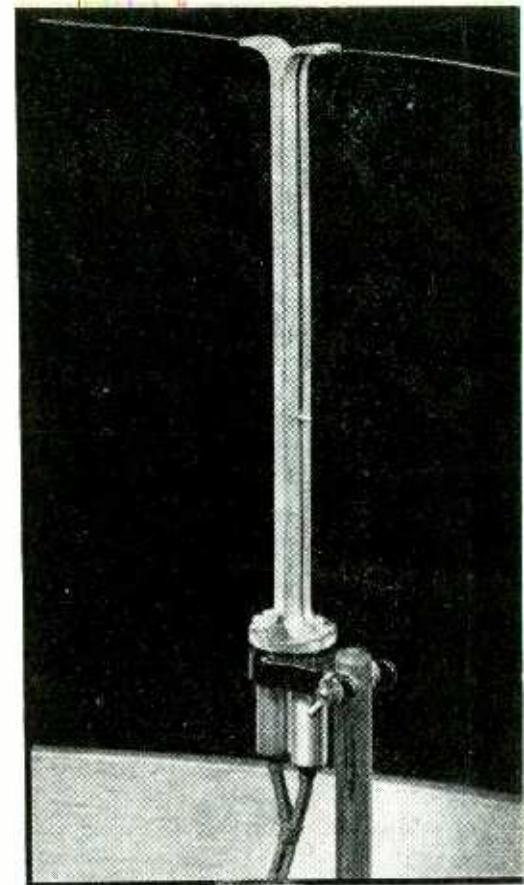
FIG. 5—Doublet antenna can be quickly tuned by sliding flexible tapes in two-wire transmission-line track
