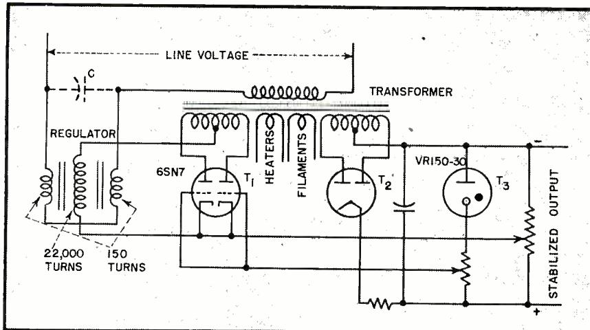
FIG. 8—Power-supply stabilizer, to regulate both filament and heater as well as high-voltage supply, uses controlled saturable reactor in power input circuit
