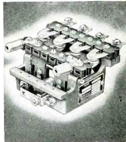
feature of the contact mechanism eliminates pigtail connections. Coils can be supplied to operate at voltages up to 230 volts, a-c or d-c. Typical power consumption of the coils is less than 3.5 watts on d-c, 8 watts on a-c.
