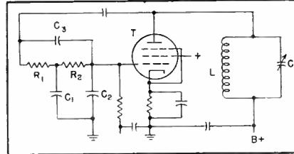
FIG. 6. In this constant-deviation network, the required inverse-square attenuation is obtained by the bridged-T phase-shifting network  $R_1$ ,  $R_2$ ,  $C_1$ ,  $C_2$ , and  $C_3$
