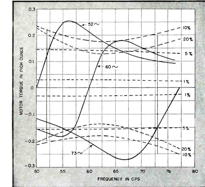
FIG. 8—Torque response curves of the control when set for resonance at frequencies of 52, 60, and 73 cycles. The solid lines indicate the resonant frequency constant; the dashed lines show the constant deviation in percent
