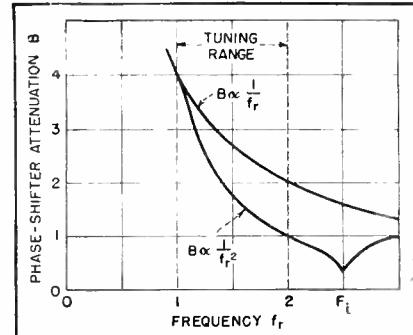
FIG. 7. Attenuation  $B \propto 1/f_r^2$ , produced by conventional two-element inductive reactance-tube phase shifter and attenuation  $B \propto 1/f_r$  required by an inductive reactance tube for constant deviation of a capacitance-tuned circuit
