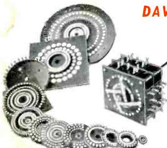
Featuring extremely low end uniform contact resistance and low noise level. Daven switches are supplied in varied combinations of decks, poles per deck and contacts per deck. Heavy duty, laminated, self-wiping arms need no lubrication; switch contacts and arms are of a special silver alloy (other metals to your specifications); bakelite or ceramic panels; break-before-make or make-before-break wiring.
