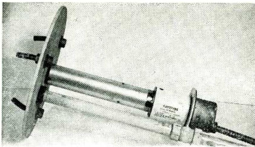
Radiation pyrometer (Leeds & Northrup Rayotube) used with bridge-type vacuum-tube voltmeter. Projecting lugs on heat shield at left engage wicket hole of furnace
