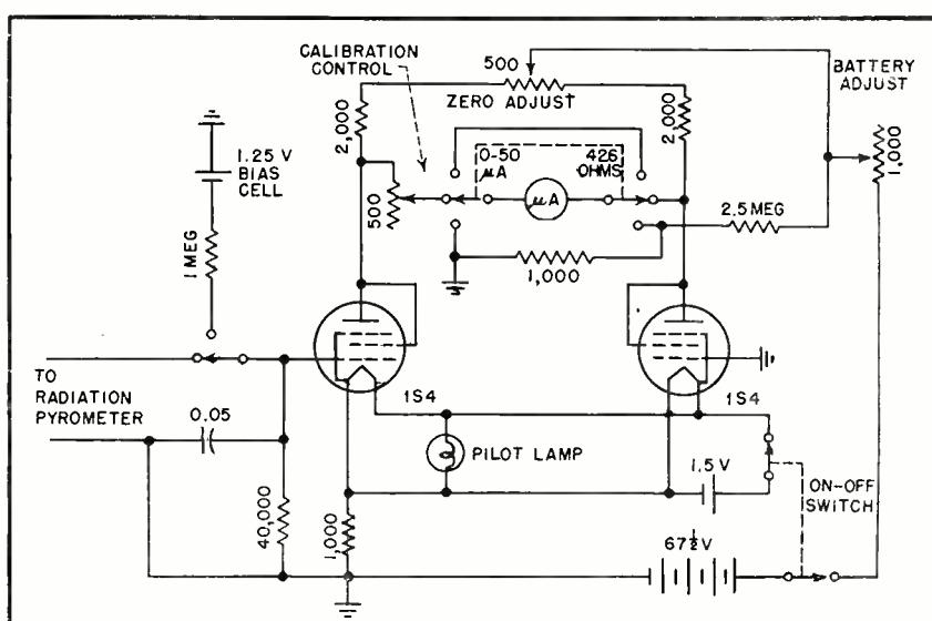
FIG. 3—Circuit of final instrument developed for flame radiation measurements
