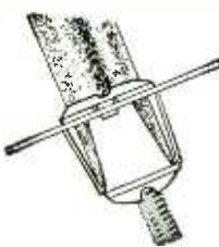
3. Snap the assembly into chassis, shield can or terminal board. Provides absolute security and rapid assembly.
