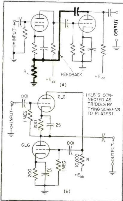
FIG. 1—By rearranging a two stage feed-back amplifier (A) the plate resistance of the second tube can serve as the cathode resistor in the stage of the first tube (B)
