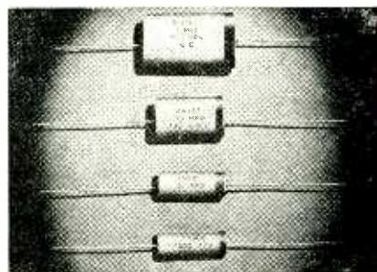
with Kraft paper and impregnated. Leads are securely anchored and the end-fill compound is not melted by a hot soldering iron. Capacitance values range from 0.001 to 0.1 microfarad in d-c rated voltages from 150 to 600 volts.
