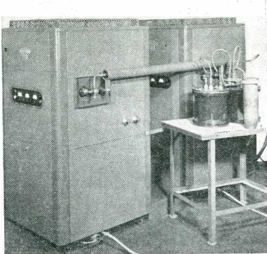
Side view of two heaters connected by a coaxial line to give double the power of a single unit in the common work coil. The two r-f transformers that feed the work coil rest on the table at the right
