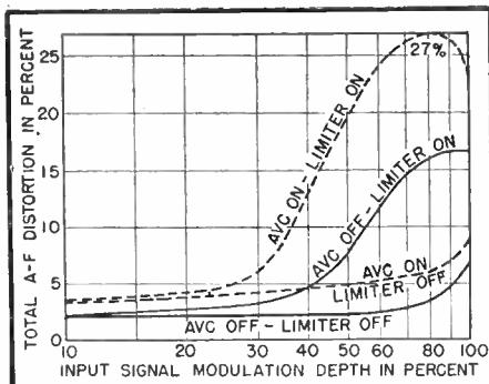
FIG. 3—Modulation distortion curves as measured at output of typical communications receiver using simple series limiter. The avc-off curves are substantially the same as for weak-signal avc-on operation. Signal input frequency is 4,000 kc, a-f output frequency is 1,000 cycles, and signal input level is 1,000 microvolts
