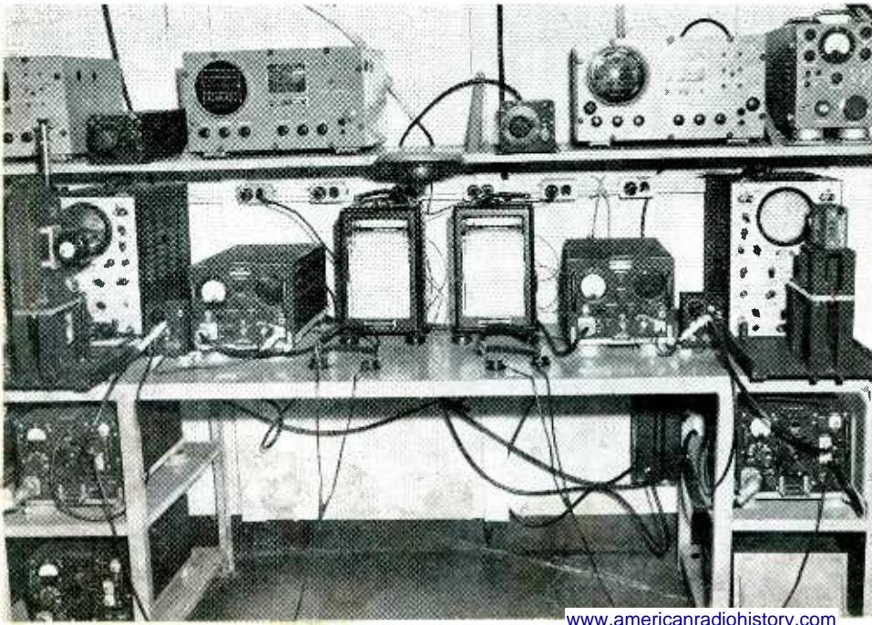
Two 3-cm radar equipments on Aomoe Island produced records of the disposition of the target array before, during and after each explosion. These records are of value in placing the time at which various ships sank, at times when smoke and spray prevented conventional photography.
