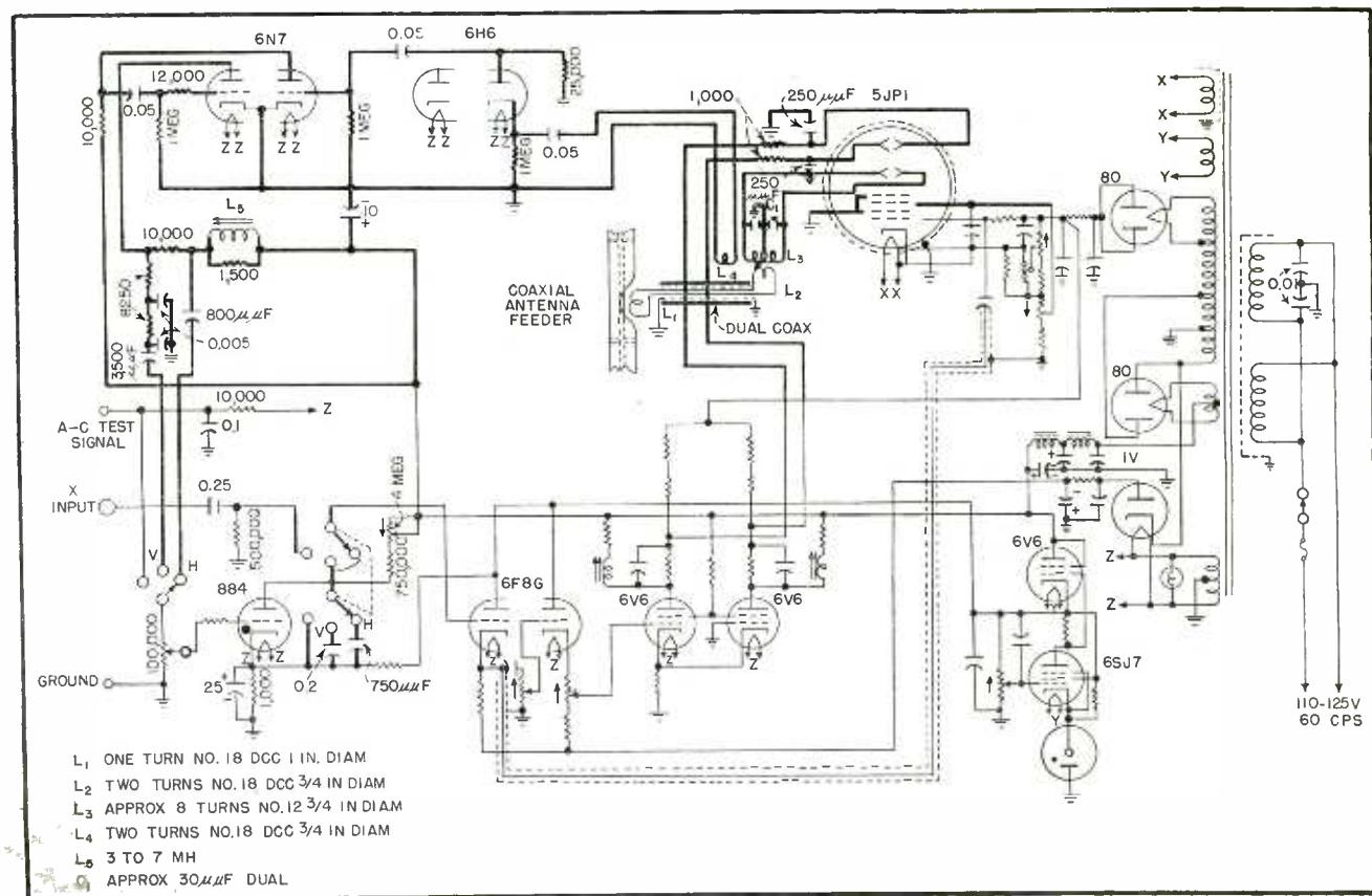
FIG. 1—Circuit modifications, shown in heavy lines, adapt standard oscilloscope for operation at television carrier frequencies
