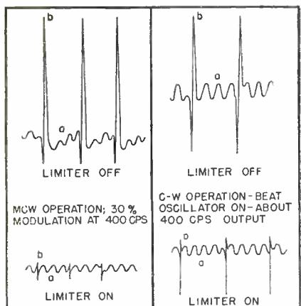
FIG. 2—Oscilloscope tracings of audio output of receiver, illustrating noise suppression of simple series limiter. Signal input to receiver is 80 microvolts, and avc is off
