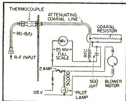
Complete circuit of the wattmeter for use from 20 to 1,500 megacycles
