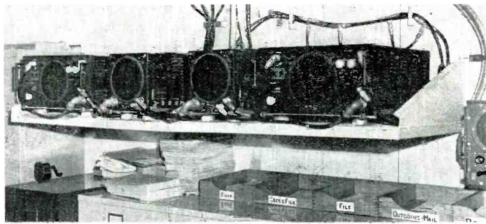
The Hobart camera, which took still pictures from television picture tube (in black case at left), at rate of one per second, processed them automatically, and projected positive image on screen (at right) two minutes later
