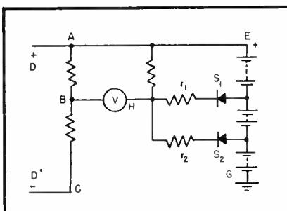
the dynode voltage is adjusted so as to maintain constant anode current in the presence of variations in incident light intensity, the relationship between the logarithm of light intensity and voltage will be
