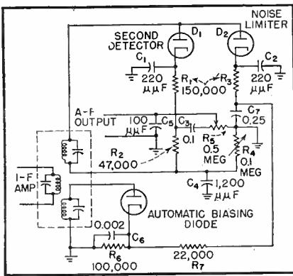
FIG. 8—Automatic balanced-detector noise limiter
