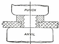
**IT'S THIS EASY!** Punch straight hole, insert fastener in sheet, and apply pressure to head of fastener.
