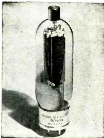
tube as a class A amplifier are: d-c plate, 1,500 volts; peak a-f grid, 150 volts; power output, 55 watts.
