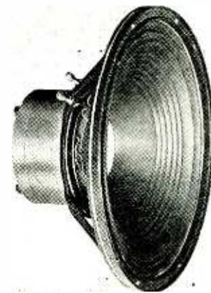
other in the line of dual speakers designed for good fidelity in home reception and reproduction. This model has a power rating of 18 watts and a 3-inch voice coil with an impedance of 10 ohms. Weight of the unit is 12 pounds.
