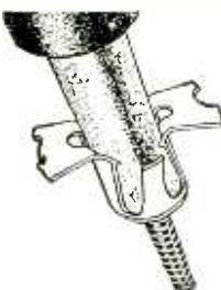
2. Provides support for the RF or IF coil tube. All coil tube length above chassis is usable electrically, as fastener does not extend above chassis.
