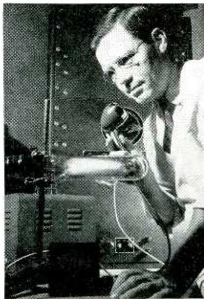
Norman C. Beese, research engineer at Westinghouse Lamp Division, demonstrates the caesium vapor lamp he designed for talking over an invisible infrared light beam
