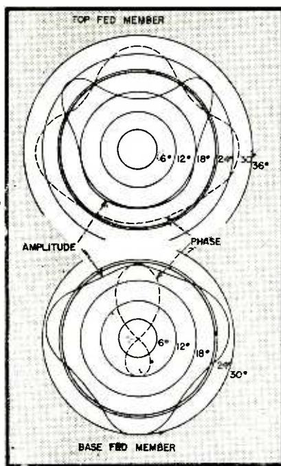
FIG. 2—Current distribution at base of antenna radiators
