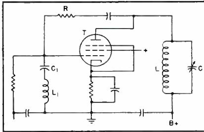
FIG. 5. Constant-deviation reactance-tube circuit. Phase shifter  $R$ ,  $C_1$ , and  $L_1$  produces an attenuation inversely proportional to the square of the frequency over the tuning range
