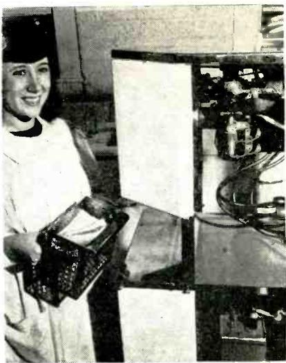
Food to be cooked in the Raytheon Radarange is placed in the ventilated "oven" and inserted in the cabinet where r-f is squirted into it from the horn antenna
