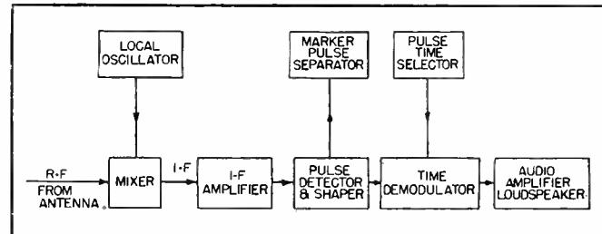
FIG. 2—In the receiver, pulses are separated and sorted to provide eight 9,000-cycle audio channels and/or audio, facsimile, and telegraph services
