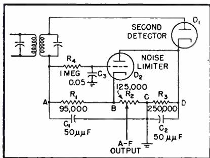
FIG. 10—Triode shunt-type noise limiter
