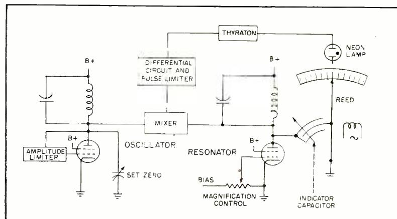
Fig. 1—Essential stages of the reactance comparator. Within its useful range, inductance can be checked against a standard with an accuracy better than one percent, and capacitance within 0.1 percent.
