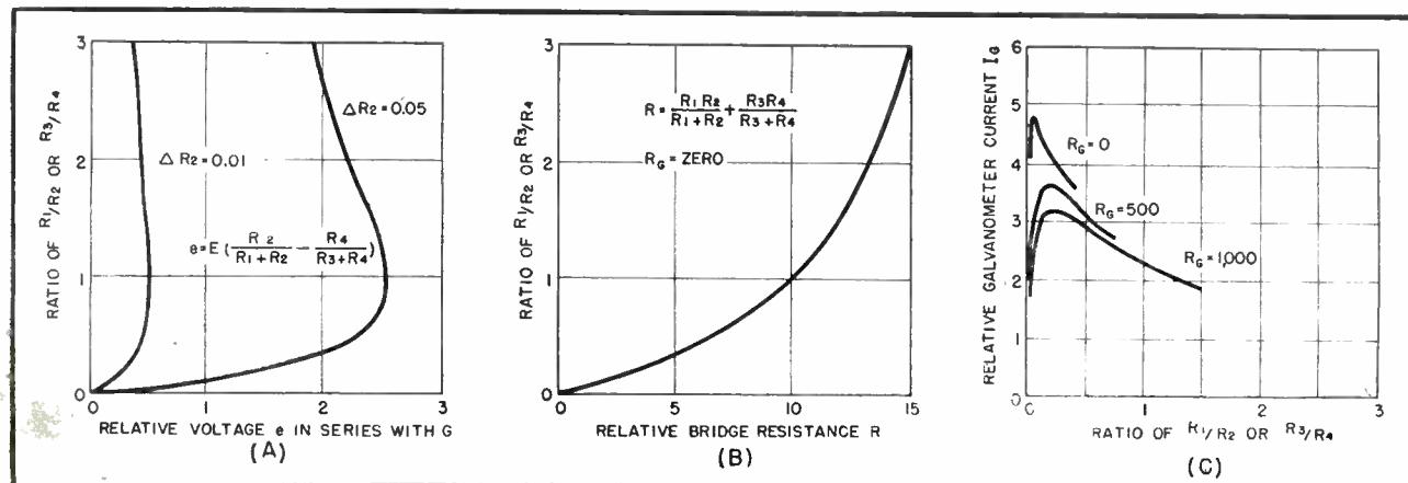
FIG. 2—Curves used in determining optimum values of circuit parameters for stable high-sensitivity vacuum-tube voltmeter
