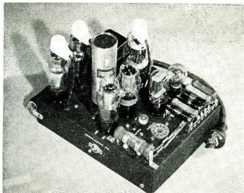
FIG. 7—Assembled power supply and control circuit of photometer
