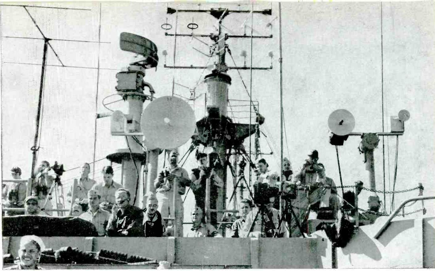
All set for the Baker Blast. Technical personnel aboard radar platform of USS Avery Island, a few minutes before the second atomic explosion. Note radar monitoring dishes, and intercept antennas on mast (top center)
