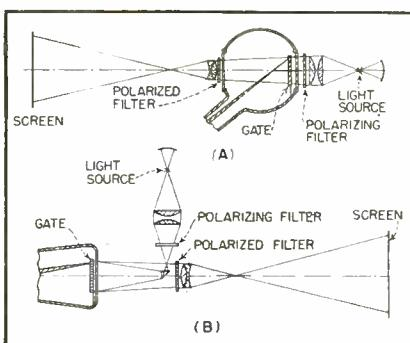
FIG. 1—Charge placed on gate by electronic scanning changes the angular rotation of the polarized light passing through the gate
