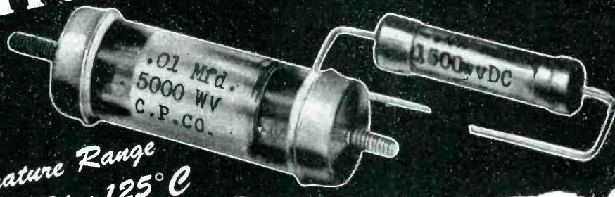
*Modern functionally designed capacitors. Metal ferrules are soldered to silver bands fused to each end of heavy-walled glass tubes. This vacuum tight assembly is fungus-proof and passes Signal Corps, Air Corps and Navy thermal cycle and immersion tests.*
