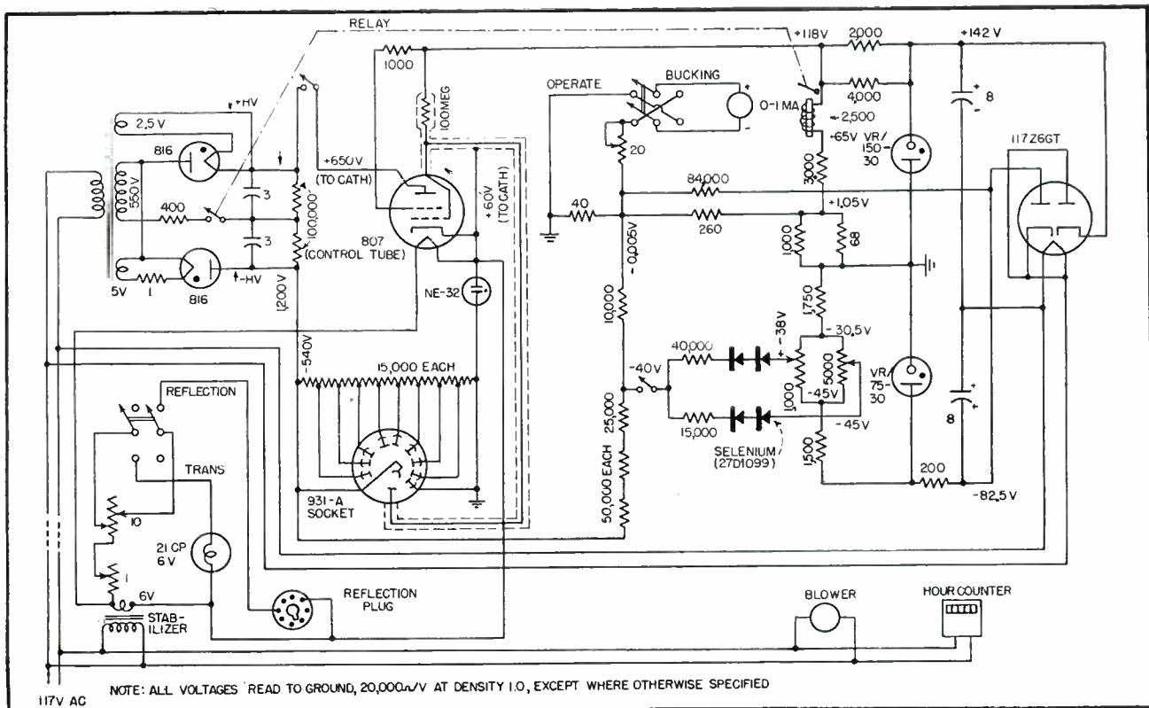
FIG. 4—Complete logarithmic multiplier phototube photometer circuit
