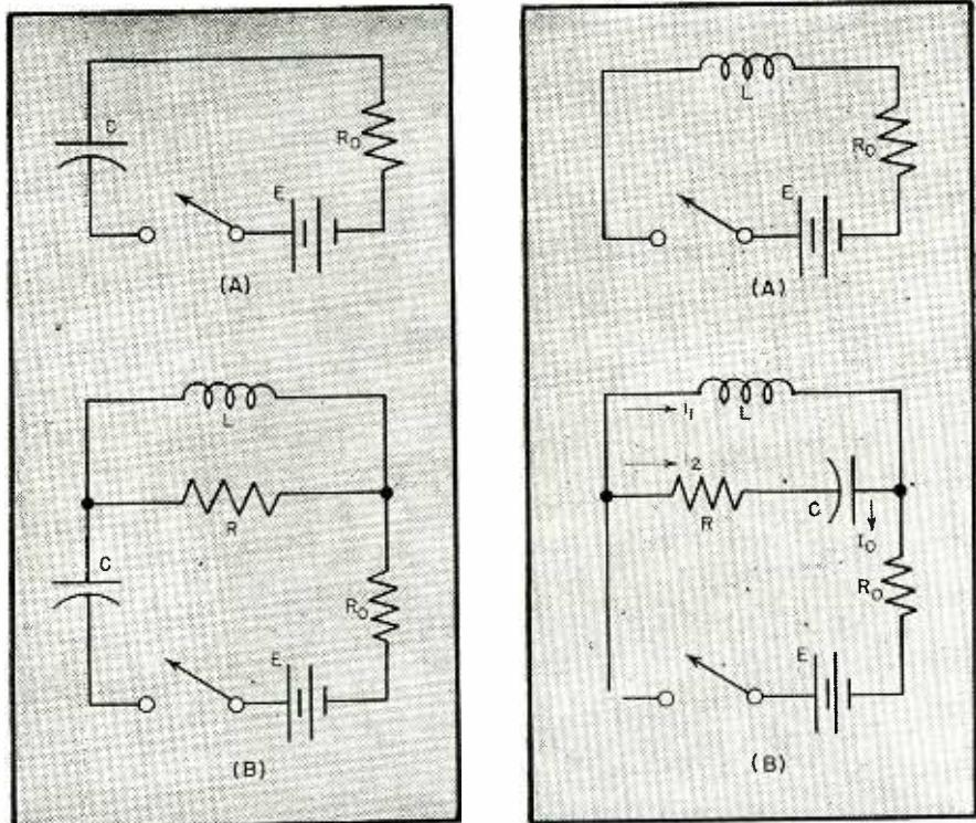
FIG. 3—Instead of discharging a capacitor, as in Fig. 1, the capacitor can be charged in the manner shown here
