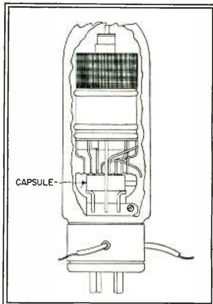
With a hydrogen generating capsule located inside 5C22 thyatron, greater life and higher pulse rates were possible
