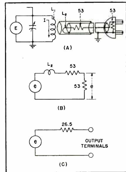
FIG. 10. Circuit (A) is the output system in which the D-shaped coil  $L_1$  is used. The equivalent circuit of the attenuator is shown at (B) and the equivalent circuit of the signal generator at (C).
