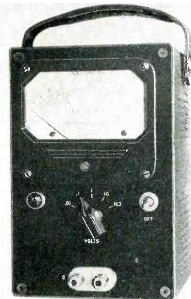
No. 1040 vacuum-tube voltmeter has a range from 0.001 to 100 volts with an accuracy of 2 percent for sinusoidal voltages. Frequency range is 10 to 200,000 cycles with 0.1 db variation. The power supply is contained in the metal cabinet.
