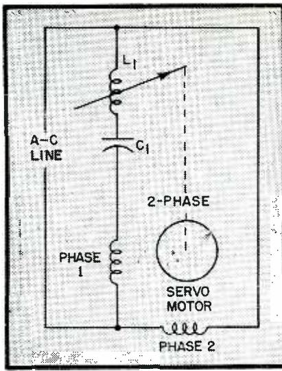
FIG. 3—Coupling the servo motor to  $L_1$  provides automatic tuning of the motor circuit to the line frequency
