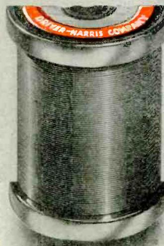
**ADVANCE\*** for winding precision resistors used in electric meters and laboratory testing devices. In finer sizes its negligible temperature co-efficient of resistance ( $\pm .00002$ ) combined with high resistivity makes it the most desired alloy for this use.
