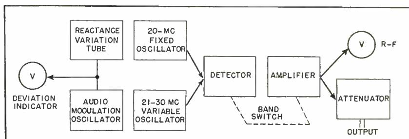
FIG. 1. Essential stages of f-m signal generator employing the heterodyne system
