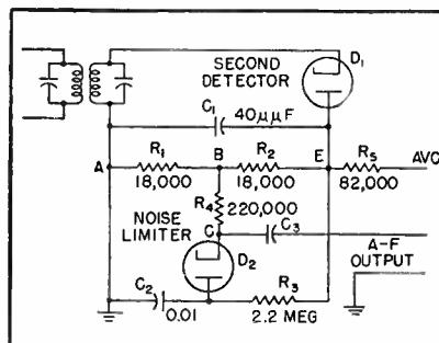
FIG. 12—Modified shunt noise limiter
