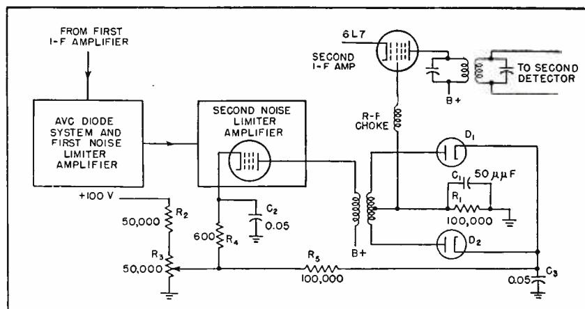
FIG. 13—Degenerative noise limiter, acting between first and second i-f stages
