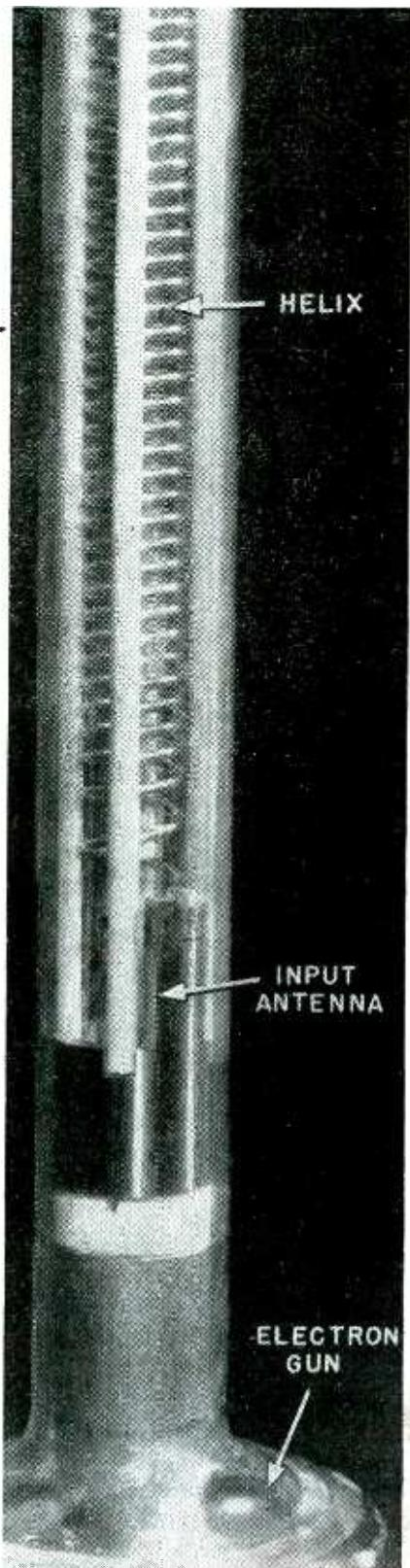
Tube provides nonresonant coupling between electron beam and traveling wave
