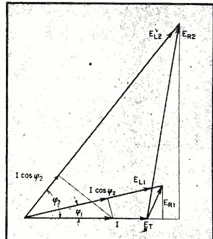
FIG. 9—Vector diagram shows that reactor absorbs the change in input voltage
