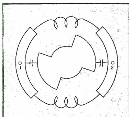
FIG. 2—Left—Schematic diagram of butterfly circuit indicates that high resonant impedance appears across points 1 and 2
