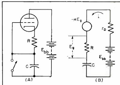
FIG. 2—(A) Simplified circuit of linear sweep generator (B) equivalent circuit of generator
