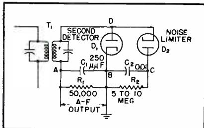
FIG. 9—Balancing-type noise limiter
