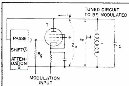
FIG. 4. Fundamental reactance-tube circuit
