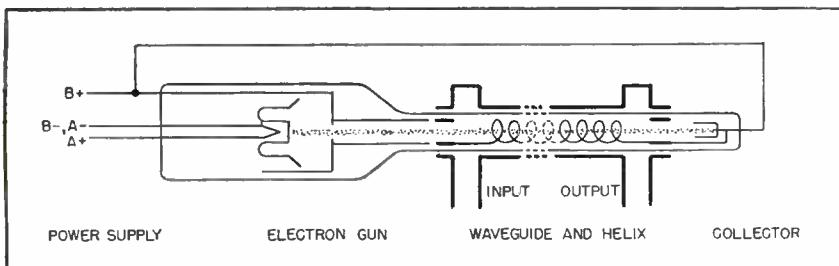
FIG. 2—Pictorial circuit shows how helix is coupled to waveguide at input and output ends. Guide extension along helix serves only as electrostatic shield
