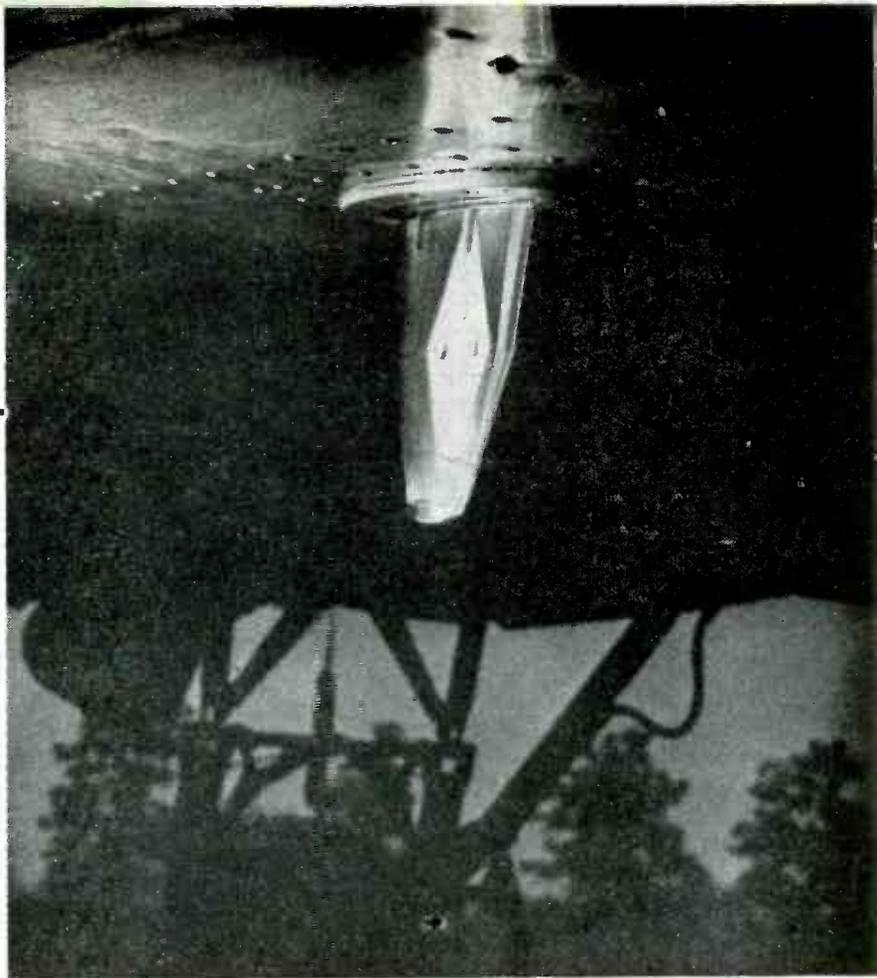
Experimental CAA installation of distance-measuring-equipment antenna on belly of DC-3. Though 1,000 mc was used for this radar interrogator-responder beacon in U. S. development work, PICA0 has requested a 40-mc band between 200 and 300 mc to make propagation characteristics correspond to those of other recommended radio aids
