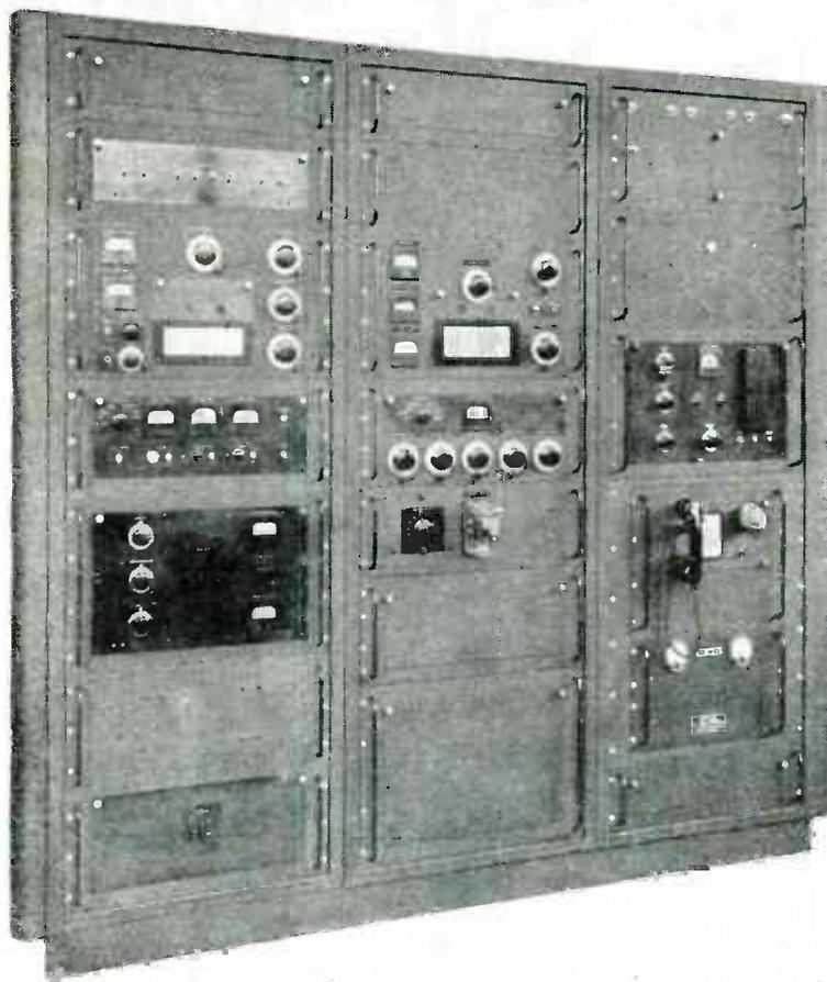
Basic vhf navigation equipment. Interchanging a single panel of this ground station unit will make it conform to PICA0 standards for the vhf omnidirectional radio range or either the equisignal or phase-comparison type of localizer for the instrument landing system
