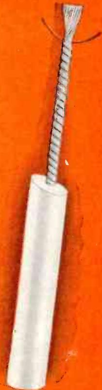
A section of the heating element used in Simmons Electronic Blanket, showing waterproof insulation and rayon core. Light wire is D-H 99 Alloy, dark wire copper.
