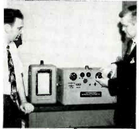
FIG. 2—Professor Klotz (left) and Professor Dole of Northwestern demonstrate the ultraviolet photometer developed by them for gas analysis
