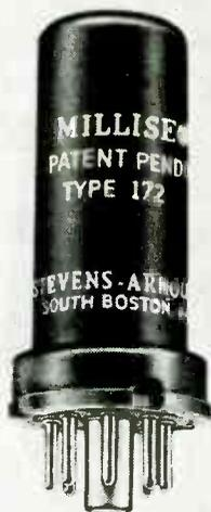
resistive loads has an operating time of one millisecond or less. Contact rating is 0.5 ampere at 110 volts. Because of its shock-absorbing mechanism, the relay can be used as a square-wave generator by applying a-c to the coil and d-c to the contacts. Catalog 105A gives complete details.
