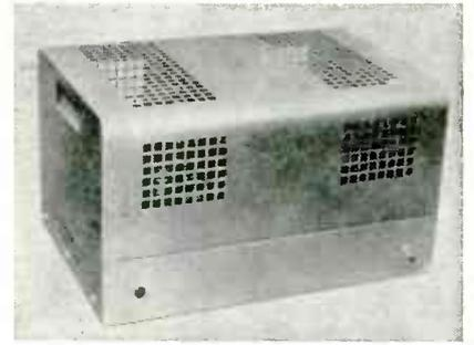
booster amplifiers, types G050 and G0125, capable of delivering 50 and 125 watts respectively use multi-stage inverse feedback to attain a flat response within 1 db from 20 to 20,000 cycles. Input impedance is 500,000 ohms with provision for balanced-line zero-level input for use on telephone lines. The self-contained power pack provides a regulated screen supply.
