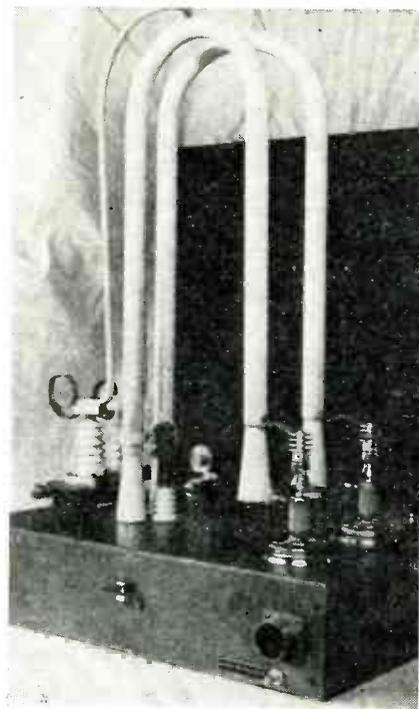
Power amplifier of f-m transmitter used at Bikini as the radio link for the telemetering system described
