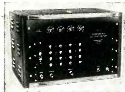
packaging control will function at rates of 15,000 per minute or higher if required. The unit utilizes four standard four-tube counter decades arranged to permit use of any predetermined number from 0 to 10,000.
