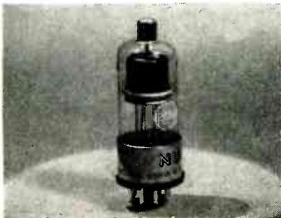
regulation of low-current power supply voltages up to 8 kilovolts, such as in pulse amplifiers, for high-impedance measurements, and in television equipment.
