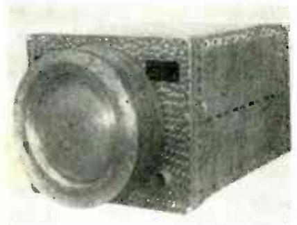
Pressure box containing the main chassis of the Farnsworth air-borne television transmitter. Excess heat from the chassis at low altitudes is passed to the radiating-fin assembly on one end
