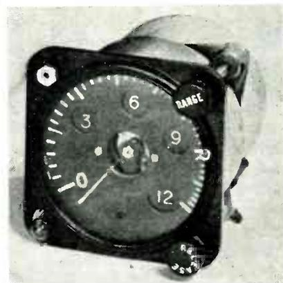
Dual-range indicator of experimental airborne radar distance-measuring equipment, to be used with instrument landing system and with vhf omnidirectional radio range to indicate distance from beacons
