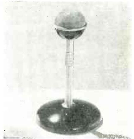
factured for home-recording, public-address, and amateur radio use. It provides flat response from 40 to 6,000 cycles with output level 50 db below 1 volt dyne per square centimeter open circuit. The microphone is supplied with cable, plug, and removable base.
