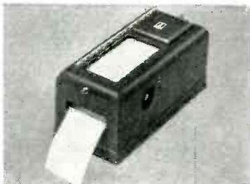
Brush Double-Channel Magnetic Oscillograph for use where two simultaneous recordings are desired—as in synchronizing problems. Three-speed paper drive, 5, 25, 125 mm per second. Chart paper 3 1/8" wide. Rugged construction.
