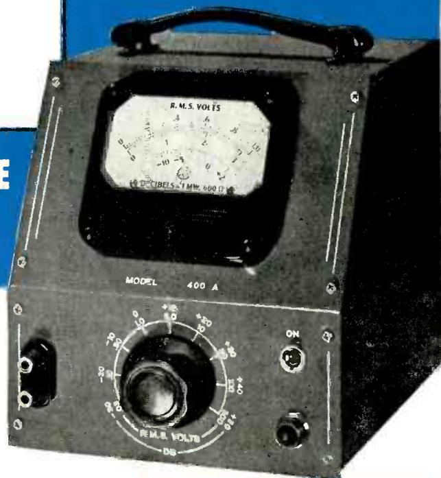
**Precise, Swift Measurements between .005 and 300 volts, 10 cps to 1 mc.**
