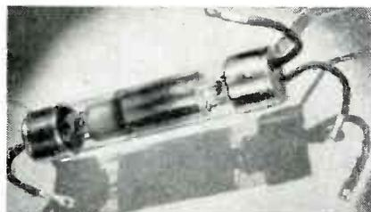
rent, 16 amperes; peak anode current, 96 amperes; peak inverse voltage, 620 volts; average arc drop, 7 volts; filament voltage, 2.5 volts.
