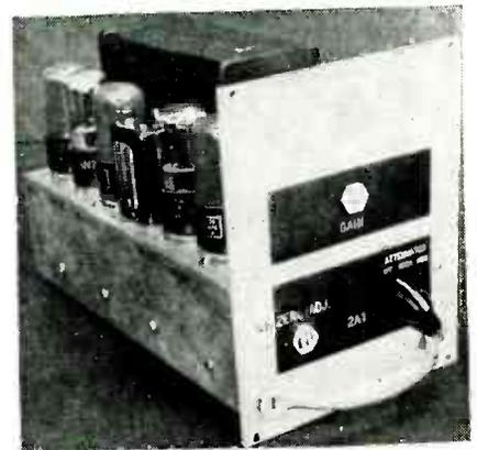
One channel of commutator unit at ground station. Low-pass pulse filter is at right rear on chassis
