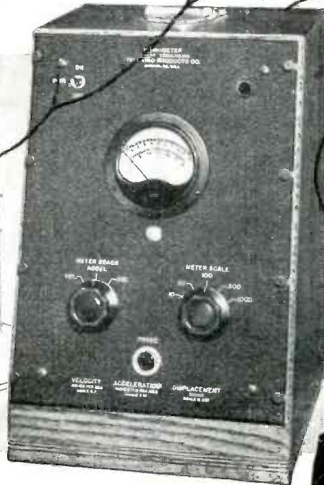
The new Televiso Model 11-B Vibrometer provides a fast, accurate and easily used method of maintaining proper vibration limits in any manufacturing process or test procedure.
