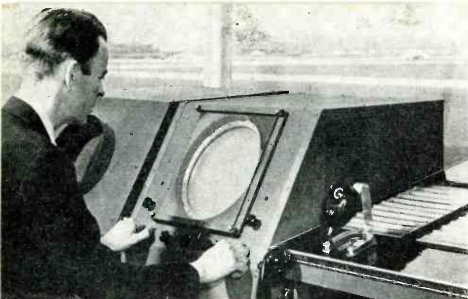
Experimental search radar installation at CAA control tower in Indianapolis. PICAQ encourages further development, to solve such problems as obtaining a sufficiently bright ppi presentation for reliable observation in a brightly illuminated control tower
