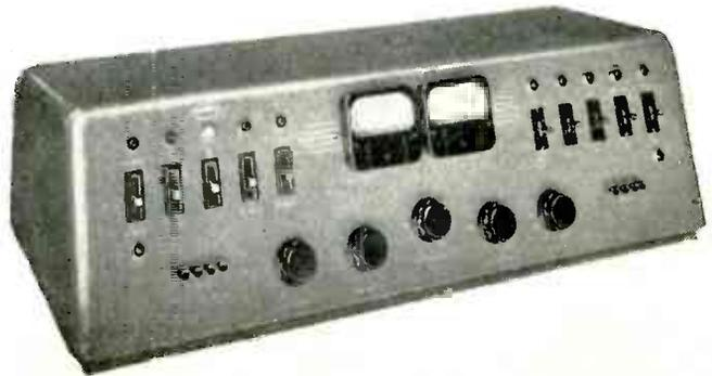
This handsome control console gives the engineer fully automatic control of all transmitter operations plus studio switching facilities for handling emergency programs originating at the transmitter. Controls audio and monitor switching; contains VU meter and remote antenna current meter. Finished in colors to match transmitter.
