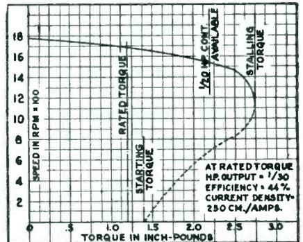
Type ALP-191: 110 volt 60 cyc. single-phase Capacitor start & run Motor Capacitor Value 4.25 Mfg. Curve #235.
