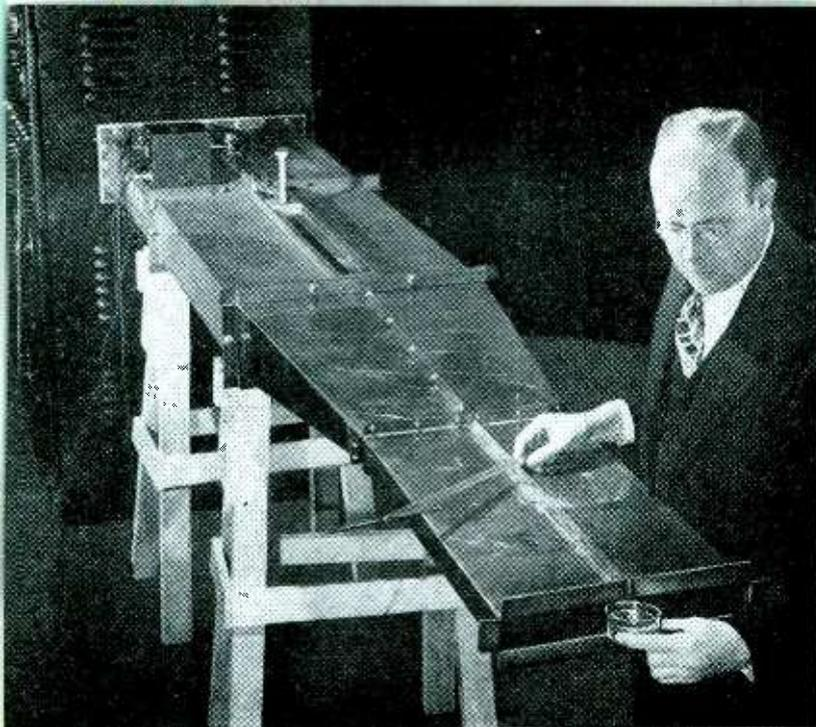
Experimental Westinghouse setup of microwave heating equipment. Liquid in container held near opening in waveguide is heated by r-f energy
