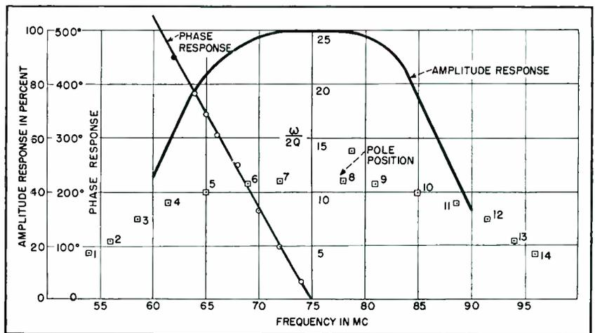
FIG. 8—Receiver i-f amplifier response curve
