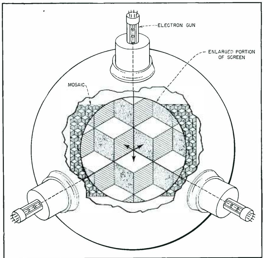
Cutaway drawing of back of Trichroscope shows how three guns paint three-colored picture on embossed mosaic on face of tube (seen here from behind). In experimental model, mosaic (not shown to scale) covers only portion of tube's face. Section of mosaic in center is shown much enlarged
