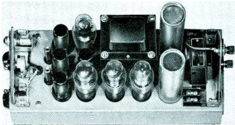
Chassis contains power supply and amplifier circuit of voltmeter; indicating instrument is mounted on cover
