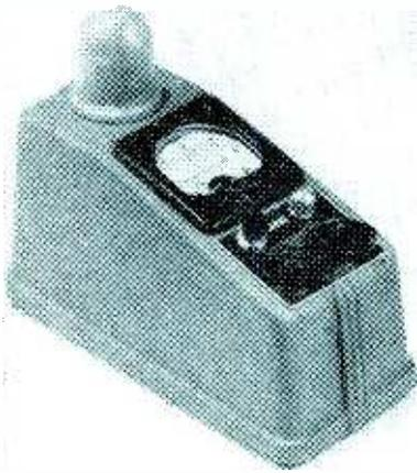
Accumulated effect of x-ray radiation is indicated directly in milliroentgens by this instrument; midscale indicates daily safe exposure. Figure 4 is the circuit
