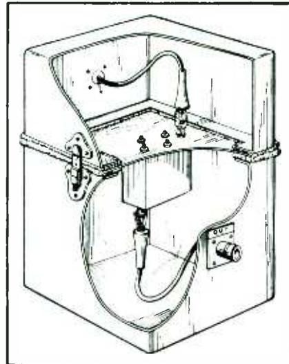
FIG. 2—Filter is mounted on plate inside shield box
