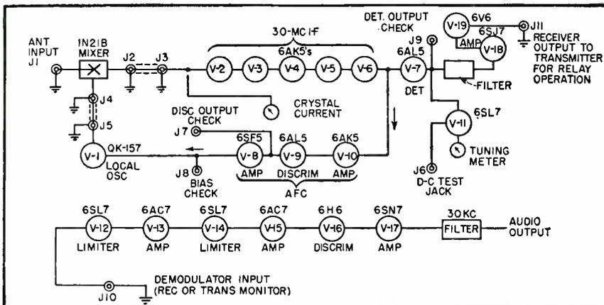
Block diagram of the microwave receiver. A klystron oscillator feeds a crystal mixer for conversion
