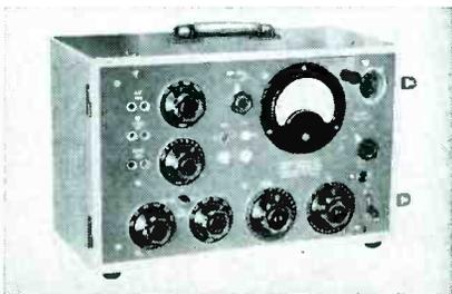
functions of an accurate vacuum-tube voltmeter, fixed-frequency audio oscillator with four settings, and precision attenuator. Designed for broadcasters, it measures gain up to 80 db and losses down to 60 db. The precision attenuator is flat to 20 kilocycles.
