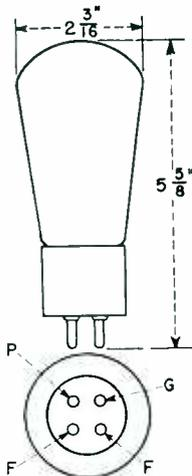
filament type, maximum ratings to 6 mc, basing 4AX.
