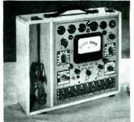
tube tester illustrated checks all tubes according to mutual conductance on a micromho scale that is also marked for "good" and "reject" values.
