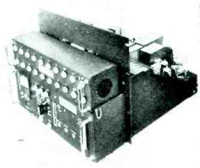
modulator unit delivers a positive pulse adjustable from 50 to 350 volts. Pulse current of 10 amperes has a duty cycle of 0.01. Width of the pulse can be varied between 1 and 25 microseconds. Repetition rate is variable between 500 and 2,500 times a second.
