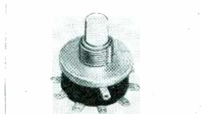
can be used in circuits passing up to 5 amperes, breaking up to 1 ampere at 110 volts. Featuring 360 degrees rotation in either direction, the switch can be moved from one position to another by turning through the least number of positions, as from position 1 to 10 without going through positions 1, 2, 3,
