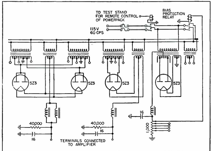
FIG. 3—Powerpack for a two-phase amplifier used in the tachometer production testing setup
