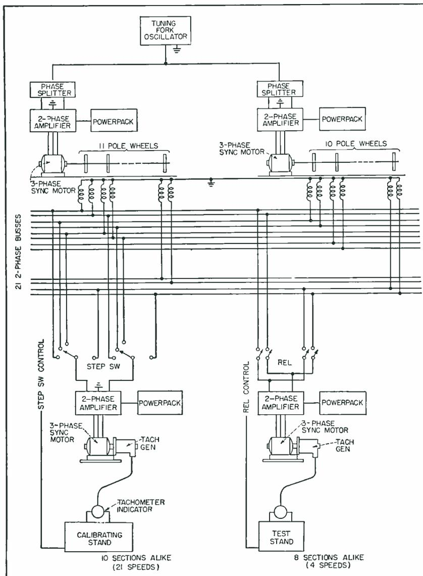
FIG. 1—Block diagram of the testing system
