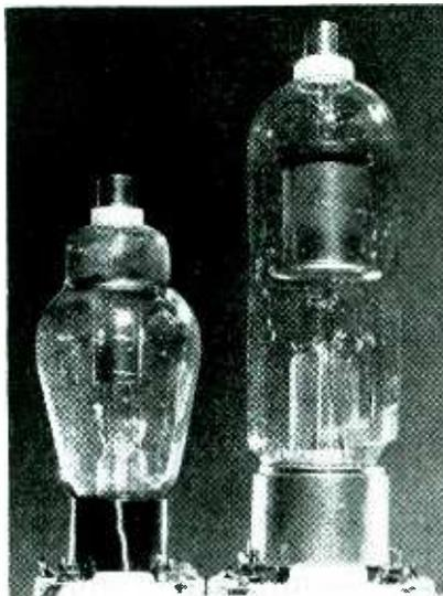
2.5 filament volts, peak inverse voltages as high as 10,000 volts, and a maximum average plate current of 0.25 ampere. The 872 has a 5-volt filament and carries a maximum peak inverse voltage rating of 10,000 volts and a maximum average current rating of 1.25 amperes.
