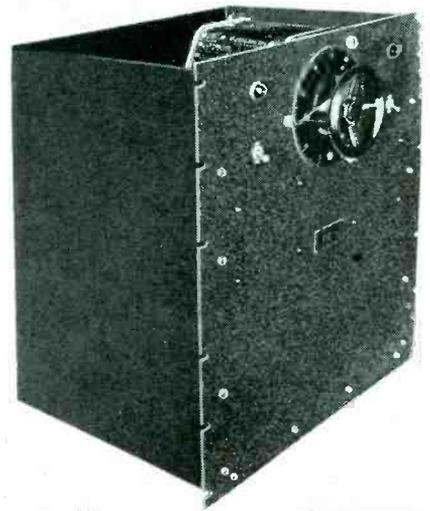
justed output voltage. The maximum d-c output current is 0.5 ampere. It operates from a 115-volt, single-phase, 50/60-cycle source. The power supply uses a full-wave bridge rectifier consisting of four type 866/866A tubes. A time-delay relay is provided which allows the filaments to be adequately heated before high voltage is applied. All major components are either potted or hermetically sealed.
