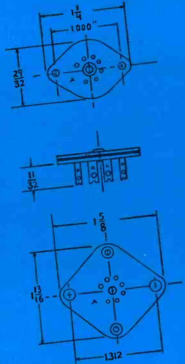
57 A 11 and 57 A 12 Miniature Laminated Sockets have spring type contacts that GRIP and hold the tube securely without the need for locking devices. These contacts, being longer and spaced wider apart, permit greater ease in soldering thus lower production costs. 57 A 12 is interchangeable with Octal Sockets of like mounting center enabling chassis design for use with either.
