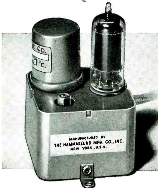
Connect up the FS-135-C in your receiver and you have a first-class frequency meter all set to go. You will have the satisfaction of knowing you are obeying F.C.C. rules and you'll get accurate signals every 100 KC's to mark the band edges or make any other checks you want.
