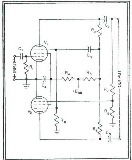
FIG. 1—Duplex feedback preserves balance of inverter
