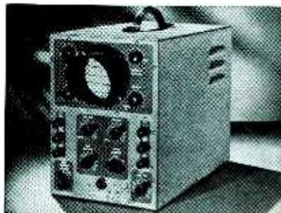
been designed for radio set servicing and general service applications. The new type 131 oscilloscope, weighing 18 pounds, is mounted in a cabinet measuring 10¾ in. high, 8½ in. wide and 13¾ in. deep. Signal frequency range from 15 to 40,000 cycles is provided with a five-range selection control and a fine frequency control. Visual study of wave form is provided by a 3-in. cathode-ray tube designed for 650-volt deflection plate operation.
