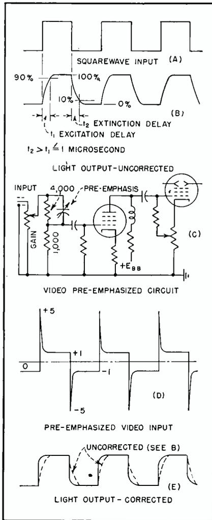
If a squarewave (A) is used to intensity-modulate a phosphor, the light output (B) from the phosphor will show finite rise and decay times. A compensating network (C) can be introduced into the intensity-modulating amplifier; it adds a large differentiated spike to the squarewave (D), with the result that the light output (E) closely duplicates the waveshape of the original input signal
