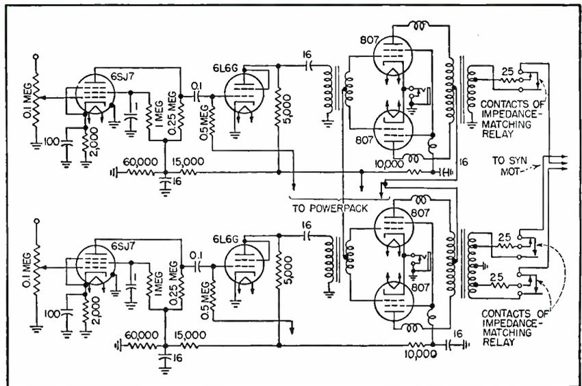
FIG. 2—Typical two-phase amplifier
