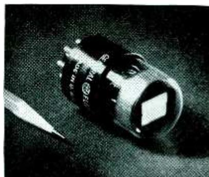
cent screen at the end of the tube, their shape depending upon the type of circuit used and its adjustment. Deviation from a proper tuning condition can be indicated to the extent of showing on which side of resonance the misalignment occurs.
