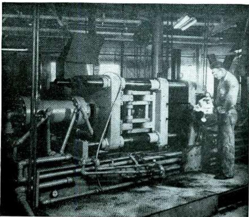
Diecasting machine for aluminum and zinc. Automatic control of the cooling period of the metal in the mold is obtained by a decay circuit
