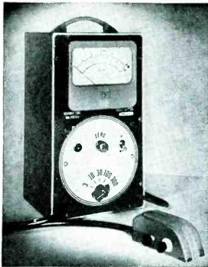
300 volts, 20 cycles to 200 megacycles. Input capacitance is less than 7  $\mu\text{p.f}$  at all frequencies.
