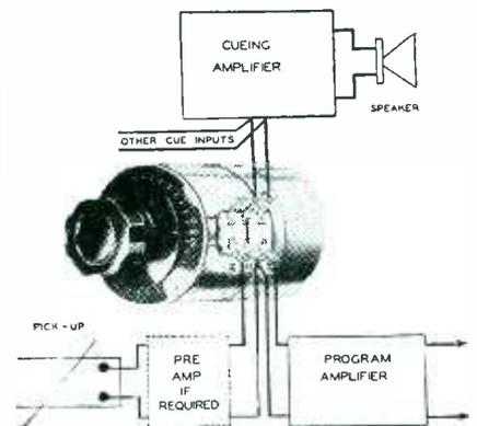
a cueing amplifier at the extreme attenuation position so that a program can be brought in smoothly without manipulation of additional cueing switches.
