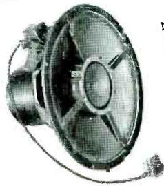
**MODEL JHP-52 COAXIAL (ST-601).** A 15-inch cone-type Coaxial like Model JAP-60 with efficiency approximately 4 db less. Furnished with H-F Range Control. Input impedance, 500-600 ohms. Power handling capacity in speech and music systems, 15 watts. List Price, \$65.00.
