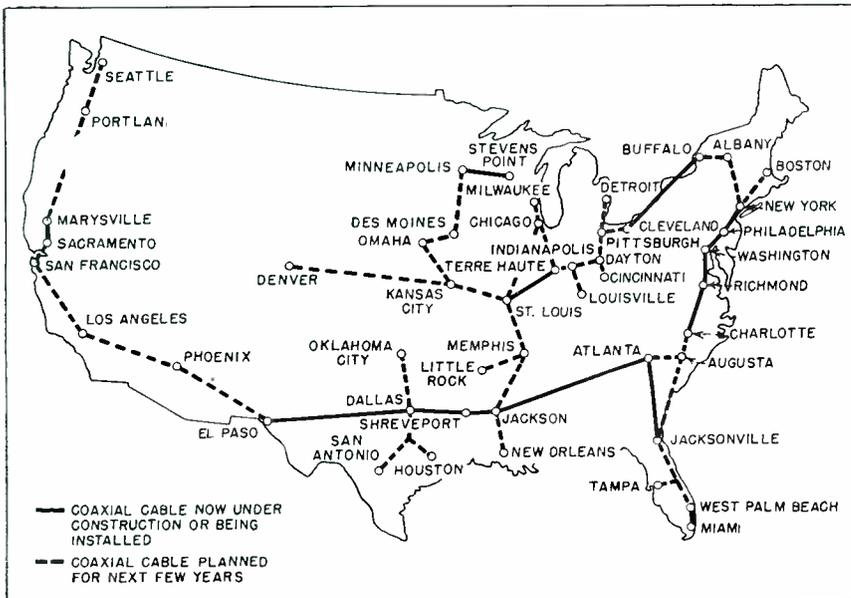
In addition to the New York to Washington coaxial cable in use since August by East Coast television broadcasters and available on an experimental basis in both directions, A T & T is installing cable facilities as shown on the map. Nationwide television network facilities will ultimately be provided by special repeaters on the coaxial lines, and by radio relay now undergoing trial operation between New York and Boston
