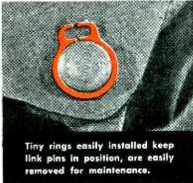
Tiny rings easily installed keep link pins in position, are easily removed for maintenance.
