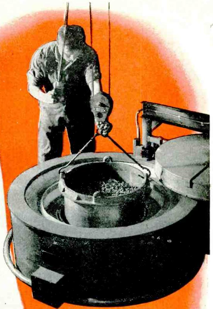
Precisely controlled heat treating in the Fomo Electric Furnace shown above is just one of the many procedures followed here at Accurate to guarantee uniformity in springs. Rigid adherence to your specifications lowers your ultimate spring costs... by making certain all your springs behave the way you want them to. Write for full details, today. ACCURATE SPRING MFG. CO., 3830 W. Lake St., Chicago 24, Illinois.
