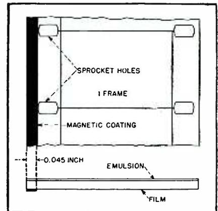
The magnetic coating can be applied to one edge of 16-mm film and the opposite edge left blank, coated with nonmagnetic material, or used as a second sound track for more intimate remarks to a select group
