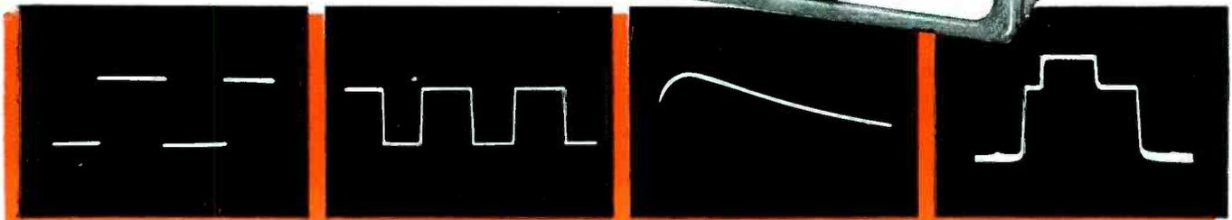
A 30-cycle square wave as seen on the WO-79A. There is no visible curvature. The frequency response of the instrument is flat down to 10 cycles.
