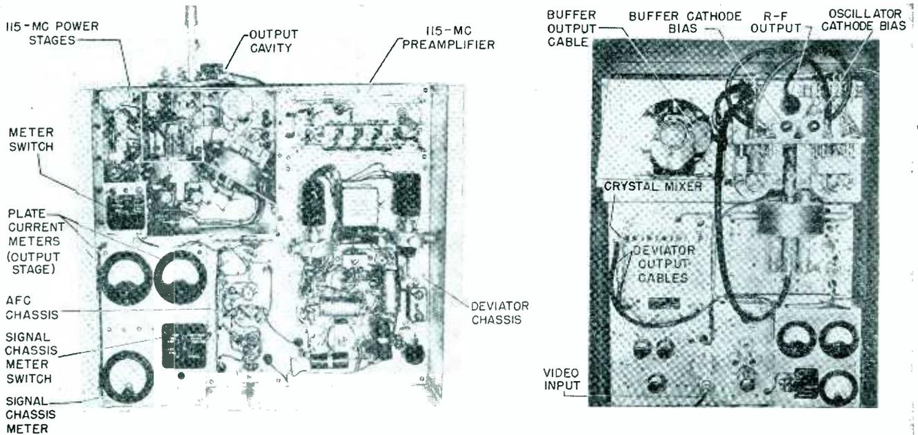
Front (left) and back views of a typical relay transmitter chassis
