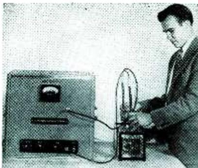
cal energy into electrical signals. Internal flaws produce measurable decreases in total transmission as indicated by a meter.
