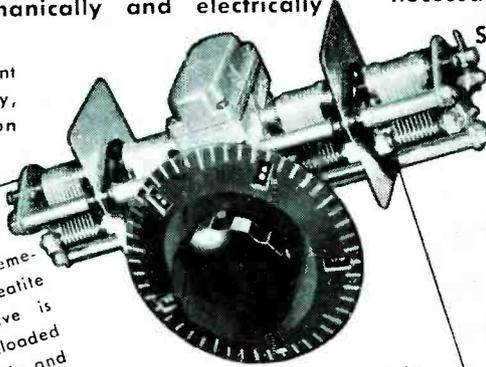
This PW Condenser is of extremely rigid construction with Steatite stator insulation. The drive is through an enclosed preloaded worm gear with 20 to 1 ratio and the rotor shaft is parallel to the panel. Plate shape is straight-line frequency when the frequency range is 2:1.
