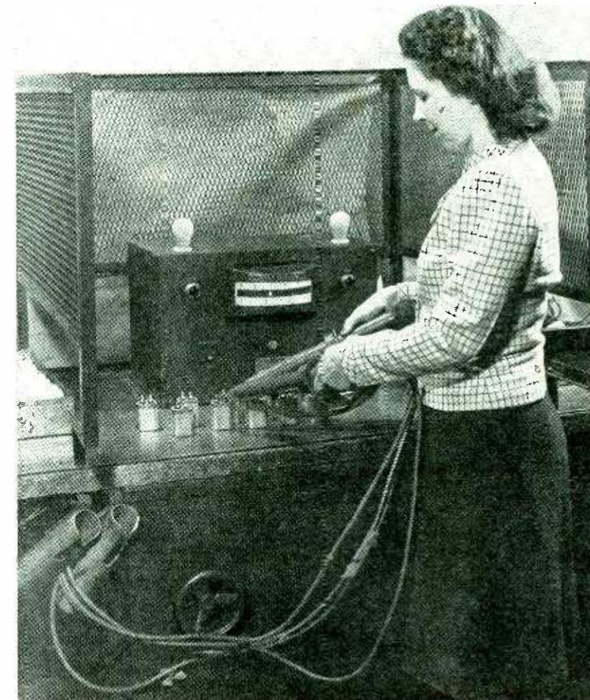
For voltage tests up to 5,000 volts, test prods handled by an operator can be safely used. Buttons on the handles of the prods control application and removal of test charge
