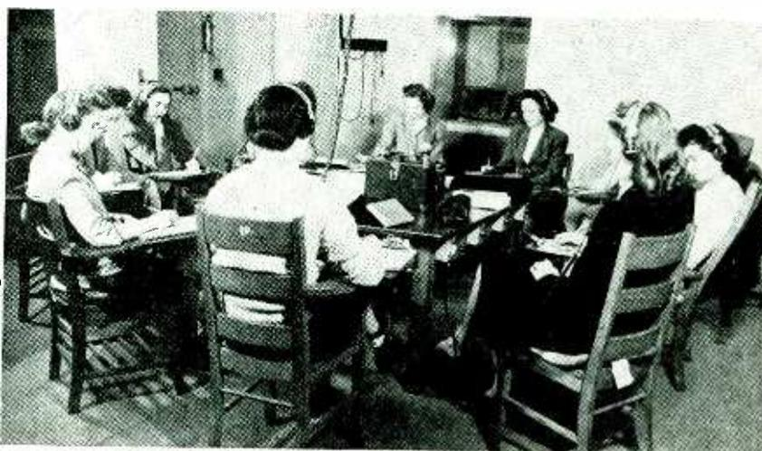
Listeners, developing data during articulation tests in which atmospheric static, such as that from lightning discharges, is artificially simulated under controlled laboratory conditions
