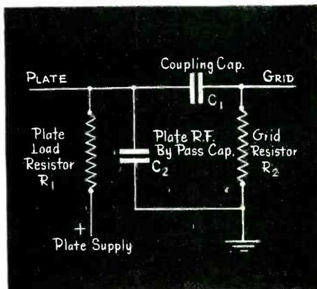
**4** Integral Ceramic Construction: Each *Couplate* is an integral assembly of "Hi-KAP" capacitors and resistors closely bonded to a steatite ceramic plate and mutually connected by means of metallic silver paths "printed" on the base plate. Think of what that means in terms of time and labor savings! Send for bulletin 943.
