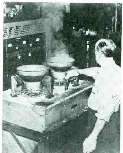
Necks of milk cans are now heated electronically without annealing the entire breast of the can and one man does the work of two formerly required in this and subsequent pickling operations
