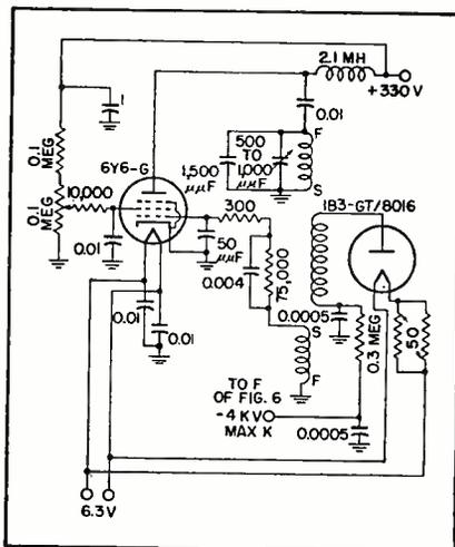
FIG. 9—R-f-operated high-voltage supply for the 7GP4
