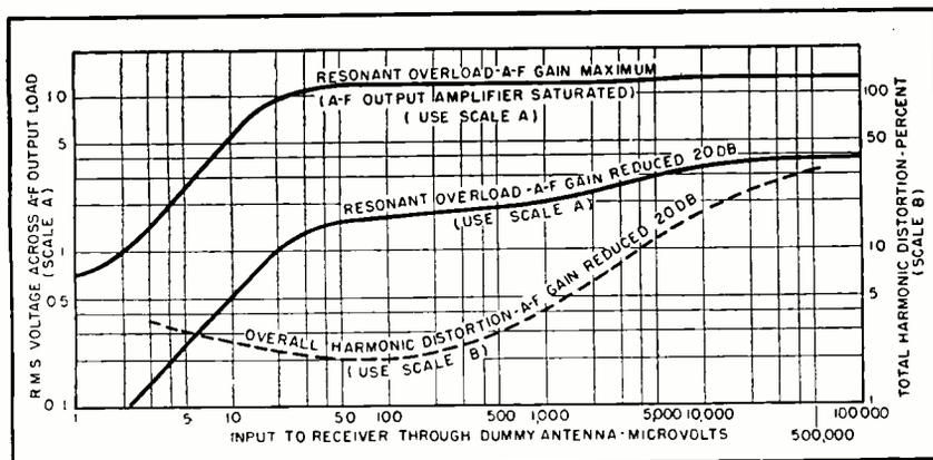
FIG. 2—Typical resonant overload and harmonic distortion characteristics of a-m receiver having undesirable i-f limiting. Carrier is modulated 30 percent at 1,000 cps
