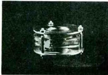
forced-air ventilation. Units are available for 500 and 1,000 micro-microfarads.
