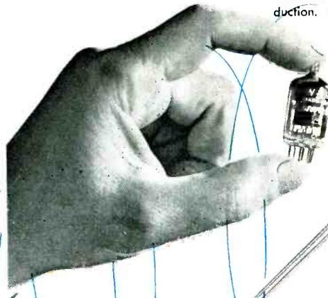
**1942.** This tiny 6AK5, operating in the vicinity of 400 mc, proved itself invaluable as an amplifier in radar receivers. Design specifications were supplied to other manufacturers by Western Electric to speed war production.
