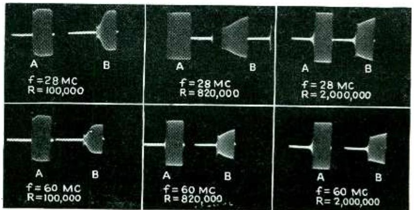
FIG. 6—Radio-frequency envelopes produced by switch under varying circuit conditions. Each left-hand picture (A), was obtained with the switch input connected to a low-impedance source, while at the right (B) it was connected to a 3,000-ohm source
