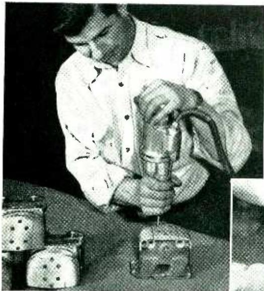
**NO WOBBLY STARTS** and slow driving to avoid skids here. Phillips Screws go in fast, set up tight and flush to hold cover of water jacket.
