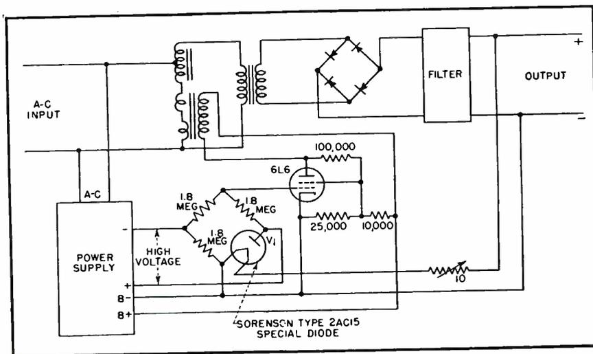
FIG. 4—Nobatron circuit, using dry-d.s.k. rectifier in conjunction with temperature-limited diode for regulating high values of direct current at low voltage
