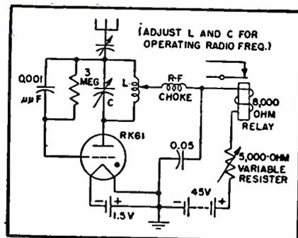
FIG. 1—Remotely controlled radio circuit uses subminiature tube
