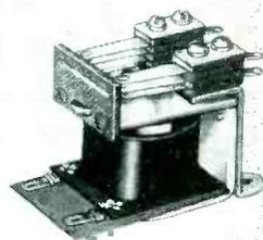
assembly, both of which are interchangeable. Contact combinations up to four-pole, double-throw and coils in ranges from 3 to 230 volts a-c and up to 110 volts d-c are available. Maximum contact current is 8 amperes.
