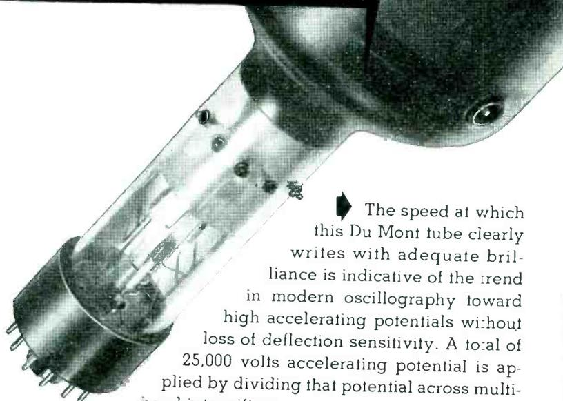
▶ The speed at which this Du Mont tube clearly writes with adequate brilliance is indicative of the trend in modern oscillography toward high accelerating potentials without loss of deflection sensitivity. A total of 25,000 volts accelerating potential is applied by dividing that potential across multi-band intensifiers.
