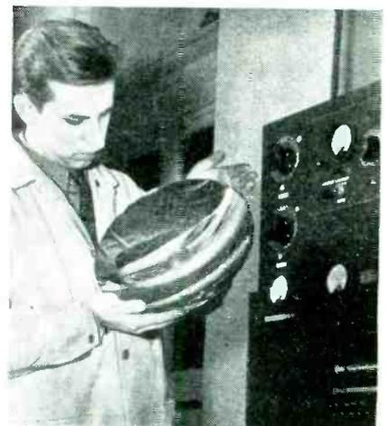
Spherical mirrors for projection television receivers are aluminized by evaporation in vacuum chambers
