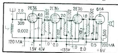
FIG. 6—Complete circuit of the receiver uses a square-law detector and three RC-coupled audio stages. Capacitance values are given in  $\mu\text{mf}$  and resistance in megohms except 6K4
