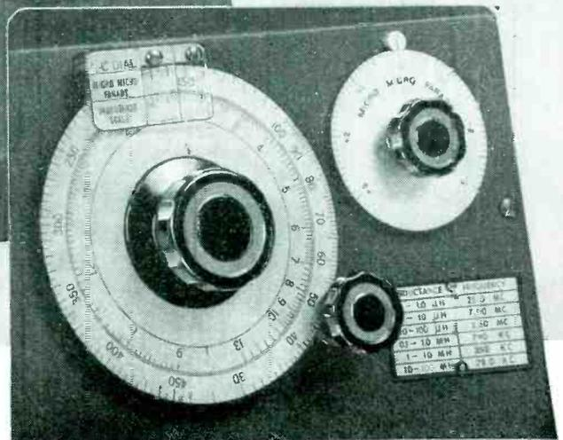
NEW INDUCTANCE SCALE ON Q-METER CAPACITOR DIAL NOW PERMITS DIRECT DETERMINATION OF EFFECTIVE INDUCTANCE VALUES BETWEEN 0.1 MICROHENRY AND 100 MILLIHENRIES.
