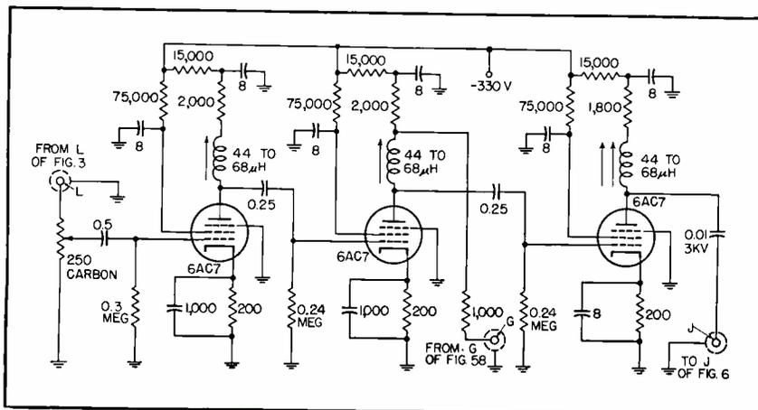
FIG. 4—Circuit of video line amplifier
