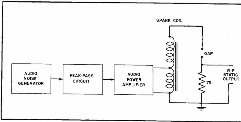
FIG. 2—Block diagram of the static generator
