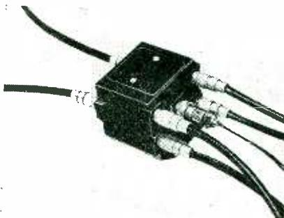
rate radar altimeters. The device is essentially a double-pole, double-throw coaxial switch.
