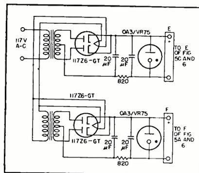
Fig. 10—Horizontal and vertical centering supplies
