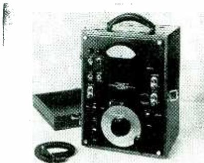
electrical and electroacoustic instrumentation is possible with the type 310-A Z-Angle Meter. Balance is accomplished by means of a single dial that reads directly in impedance and the phase angle is indicated on a direct-reading meter.
