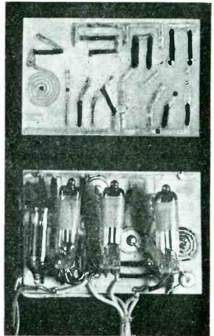
FIG. 4—Spiral coil, wiring, and resistors of the receiver on a steatite plate are shown at top of photo. The receiver at bottom needs only batteries and loudspeaker to be attached to the leads
