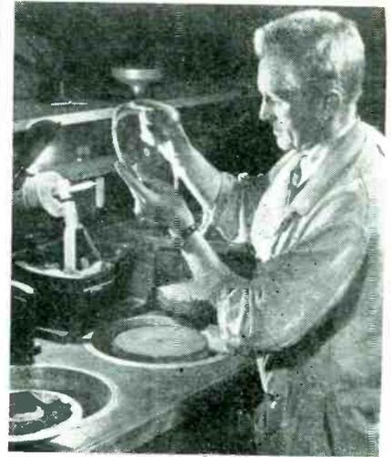
Glass correcting plates for optical systems were ground to shape by hand; they are now shaped by a dropping technique
