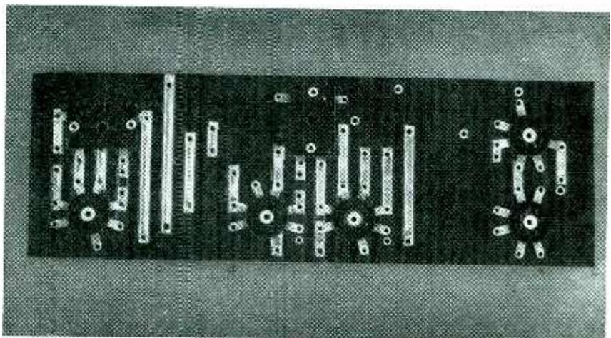
**FIG. 3**—Tube and transformer sockets in place. In this instance they are held in place by eyelets. In other developmental models use of female connectors permits them to be simply shoved down over deck pins
