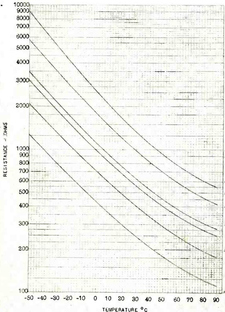
The steep negative curve of Globar Type F Resistors points up their sensitivity over a range from  $-50^{\circ}\text{C}$ . to  $100^{\circ}\text{C}$ . Actually this range can be extended beyond  $150^{\circ}\text{C}$ . This pronounced and important characteristic of Globar Type F Resistors makes them particularly useful for stabilizing circuits possessing a positive temperature coefficient of resistance.
