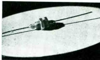
the capacitor, allowing either or both ends to be bent for point-to-point wiring. This type is available in the capacitance range from 7 to 1,500 micromicrofarads.
