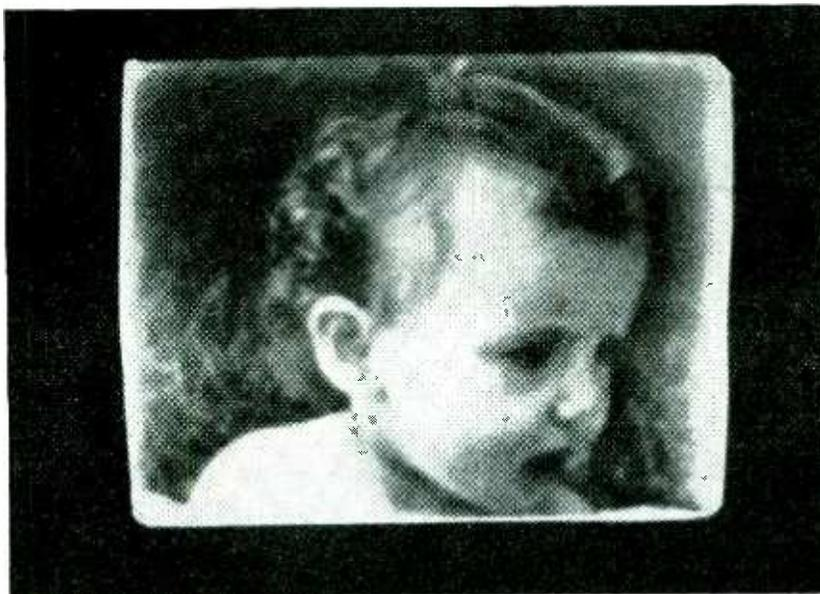
Capabilities of the system are illustrated by this same-size reproduction of a photograph taken of the screen of the 7GP4 kinescope
