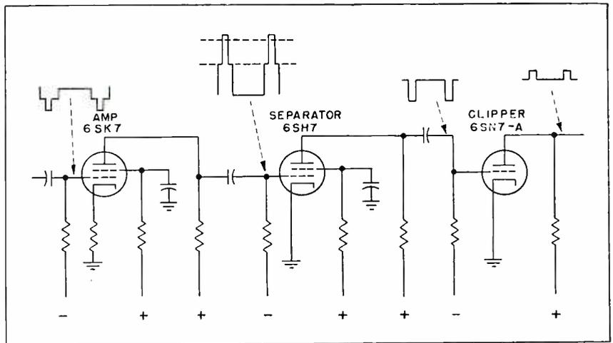
FIG. 5—The synchronizing chain, consisting of a polarity-reversing amplifier, amplitude separator, and clipper
