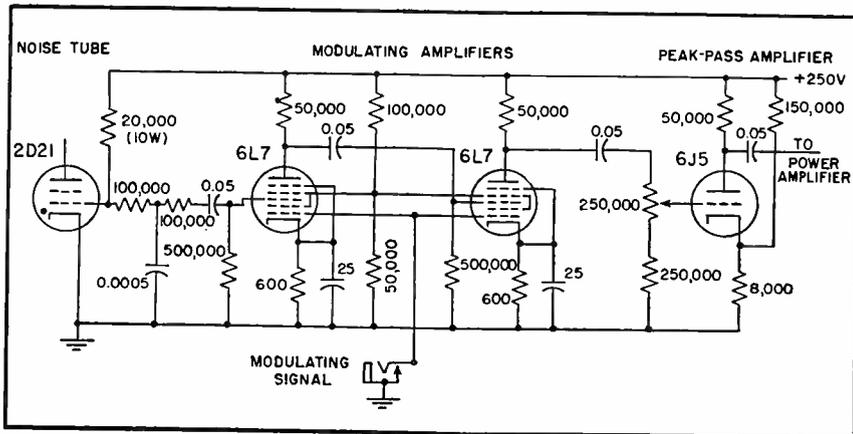
FIG. 3—Schematic diagram of the audio noise generator and peak-pass circuit
