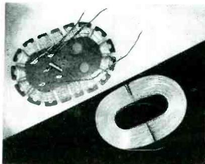
a Q of about 200. Owing to the thermoplastic properties of the insulation, the formed loop is merely heated, allowed to flow slightly and then hardens so that no other support is needed.
