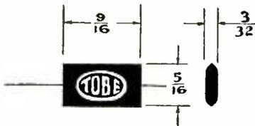
TO MEET REQUIREMENTS for miniature components for use in hearing aids, pocket radio receivers, airborne radio apparatus, and other devices in which economy of space is a primary factor:
