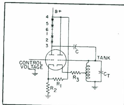
FIG. 3—Final circuit with the Varistor in the plate circuit. Values of  $R_1$  and  $R_2$  are 33,000 and 1,500 ohms respectively for a 6SN7 and 35,000 and 1,000 ohms for a 7F8. Numerals indicate Varistor terminals
