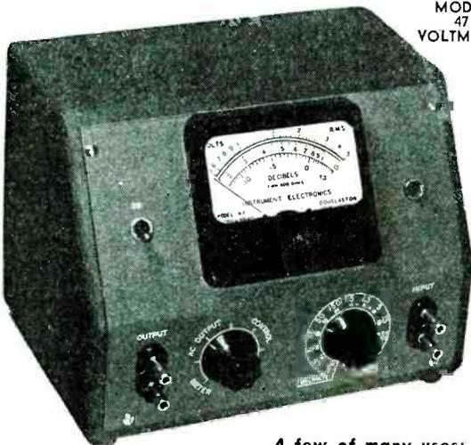
An extremely sensitive amplifier type instrument that serves simultaneously as a voltmeter and high gain amplifier.
