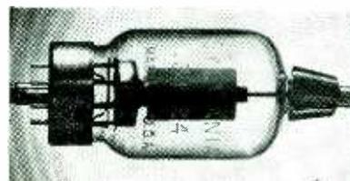
torily at frequencies up to 125 megacycles. Typical operating conditions follow: plate, 2,000 v; control grid, -300 v; screen grid, 375 v; plate current, 90 ma; full driving power, 4 watts; power output, 140 watts.
