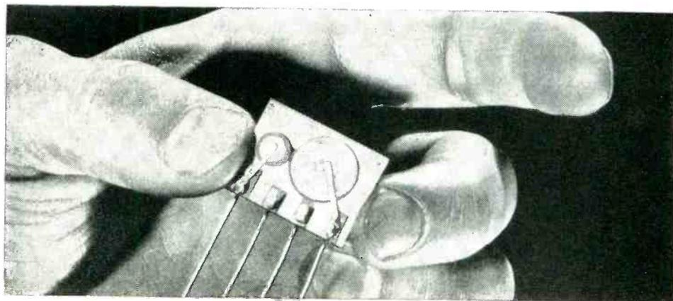
**2** For transmitters, power supply converters, X-ray equipment, etc., CRL's medium-duty power switches are now available. Efficient performance up to 20 megacycles.
