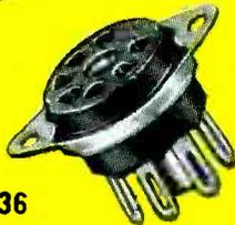
● Shield fits over and outside of retaining spring—no projecting fingers—retaining indentation on shield locks into ridge on base. A positive lock! Base is made of hardened carbon steel, supplying adequate spring retentivity on shield. The opening at the top of the shield permits speedy heat dissipation. Mounting holes coincide with those for miniature sockets as set up by RMA specifications.
