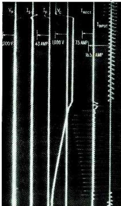
FIG. 2—Slow-speed oscillogram showing one complete cycle of welder operation. All scale values are peak. Frequency of input current curve at right is 60 cycles
