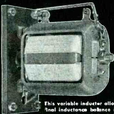
This variable inductor allows a final inductance balance independent of the resistive balance
