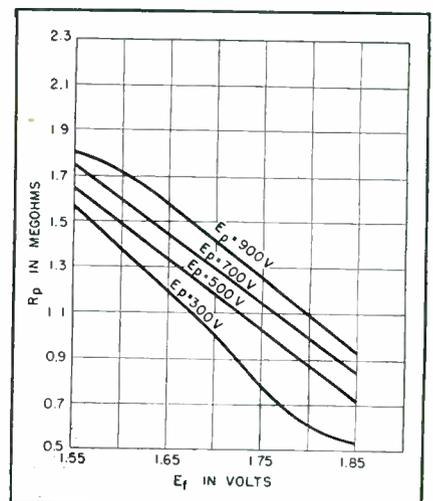
FIG. 2—Variation of plate resistance with filament voltage for Sorensen 2AC15 diode
