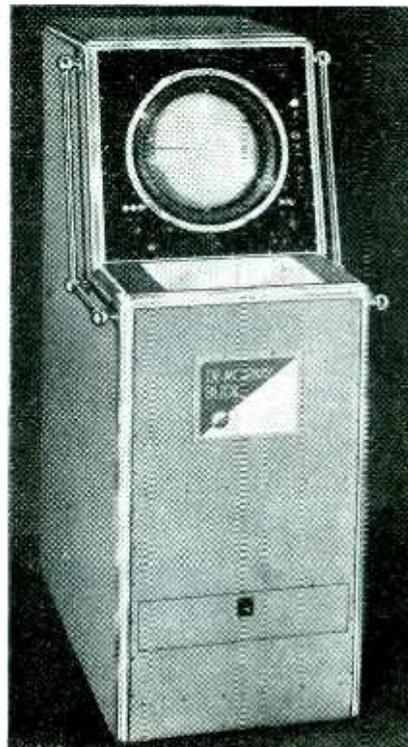
100 yards to 32 miles. It exceeds the specifications of the Coast Guard for class A equipment, operates in the band assigned by the Federal Communications Commission for marine navigation (approximately 9,300 megacycles) and has a peak pulse power output of 18 kilowatts. Microfilm copies of geodetic charts made on 70-mm color film are projected on a screen for comparison with indications on the 12-in radar screen.
