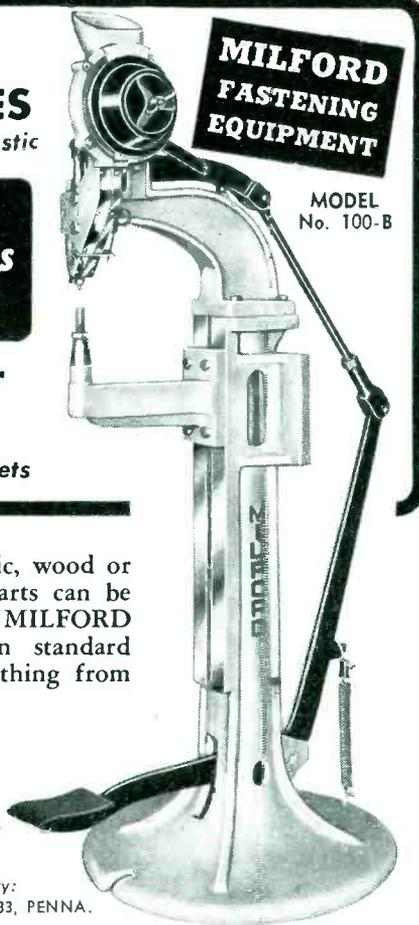
If your product — whether metal, fabric, wood or plastic — requires fastening and the parts can be brought to a machine, investigate MILFORD FASTENING EQUIPMENT. Fifteen standard models of rivet-setters to fasten everything from wrist watch bracelets to refrigerators.
