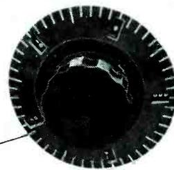
The PW-D micrometer dial can be read direct to one part in 500. It revolves ten times in covering the complete range and fits a  $\frac{3}{8}$ " diameter shaft.
