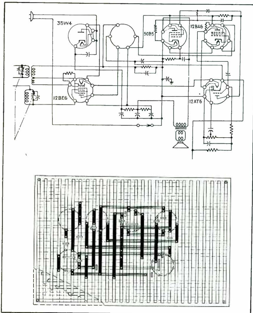
Electronic circuit, showing the manner in which a schematic may be converted into a stamped wiring deck layout by interconnecting and/or cutting conductors on obverse and reverse sides of the deck. Tube and transformer placement are indicated. Other component parts may be similarly shown
