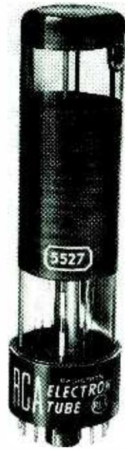
Two-inch iconoscope for the 250-line system
