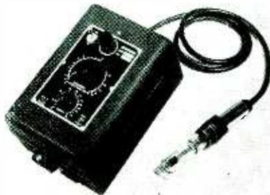
the bridge is off balance to sound a warning bell or other alarm. A conductivity cell in the boiler return line continuously checks return steam condensate for contamination from heating tanks or kettles.
