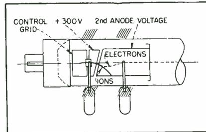
FIG. 10—An obliquely placed electrostatic lens deflects electrons and ions, so ions are trapped in electron gun.
