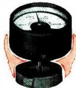
A tiny SILMANAL cylinder magnetized along a diameter is the heart of the G-E gauss meter. When the probe is placed in the field of a permanent magnet or a d-c electromagnet, the SILMANAL magnet on the shaft tends to line up with the flux. Flux density is measured by rotating the instrument until the pointer reaches its highest reading. This occurs when the probe-magnet flux is at right angles to the flux being investigated. The pointer when at zero scale position indicates flux direction.
