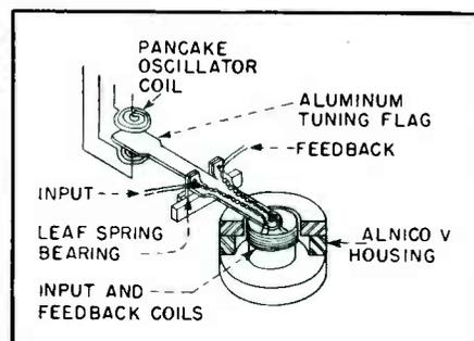
FIG. 3—Construction details of the galvanometer-type movement. The input and feedback coils are wound one above the other
