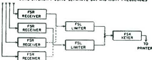
The FSR Receiver, the FSL Limiter and the FSK Keyer are the three units comprising this equipment and the use of multiple FSR's and FSL's makes possible space or frequency diversity or both.
