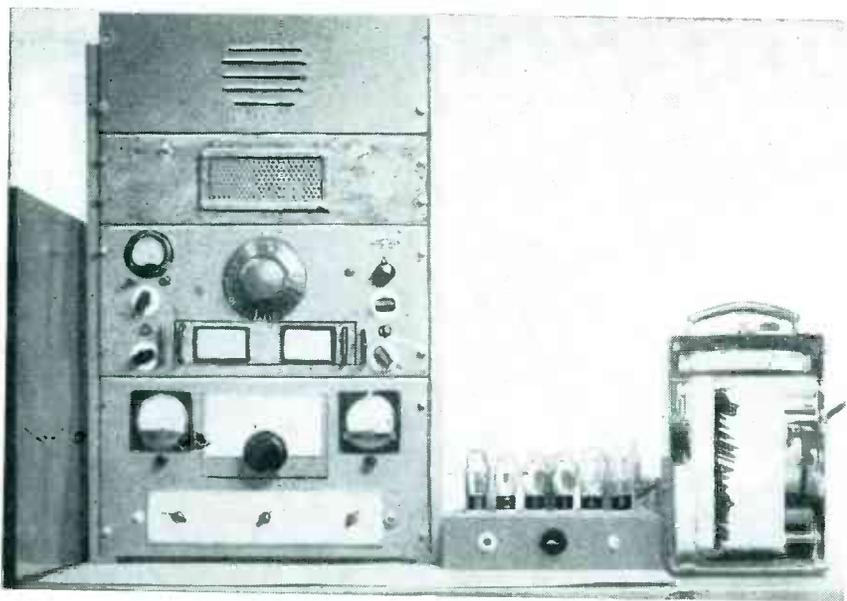
Receiving rack, cyclo chassis, and graphical recorder used at Ottawa frequency monitoring station for recording sky-wave signals from broadcast stations
