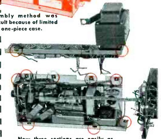
Now three sections are easily assembled separately, and quickly fastened together with SPEED NUTS into completed unit.
