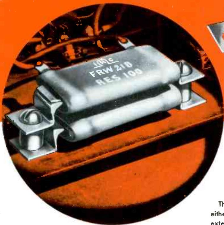
Designed to fulfill requirements of high wattage dissipation in limited-space applications, the IRC Type FRW Flat Wire Wound Resistor has a higher space-power ratio than standard tubular wire winds. For different operating conditions, IRC makes these compact resistors available in two coatings, the IRC "B Coat" or "C Coat."
