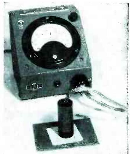
FIG. 1—Electronic micrometer measures change in coupling between probe coils caused by displacement of probe from metallic reference surface
