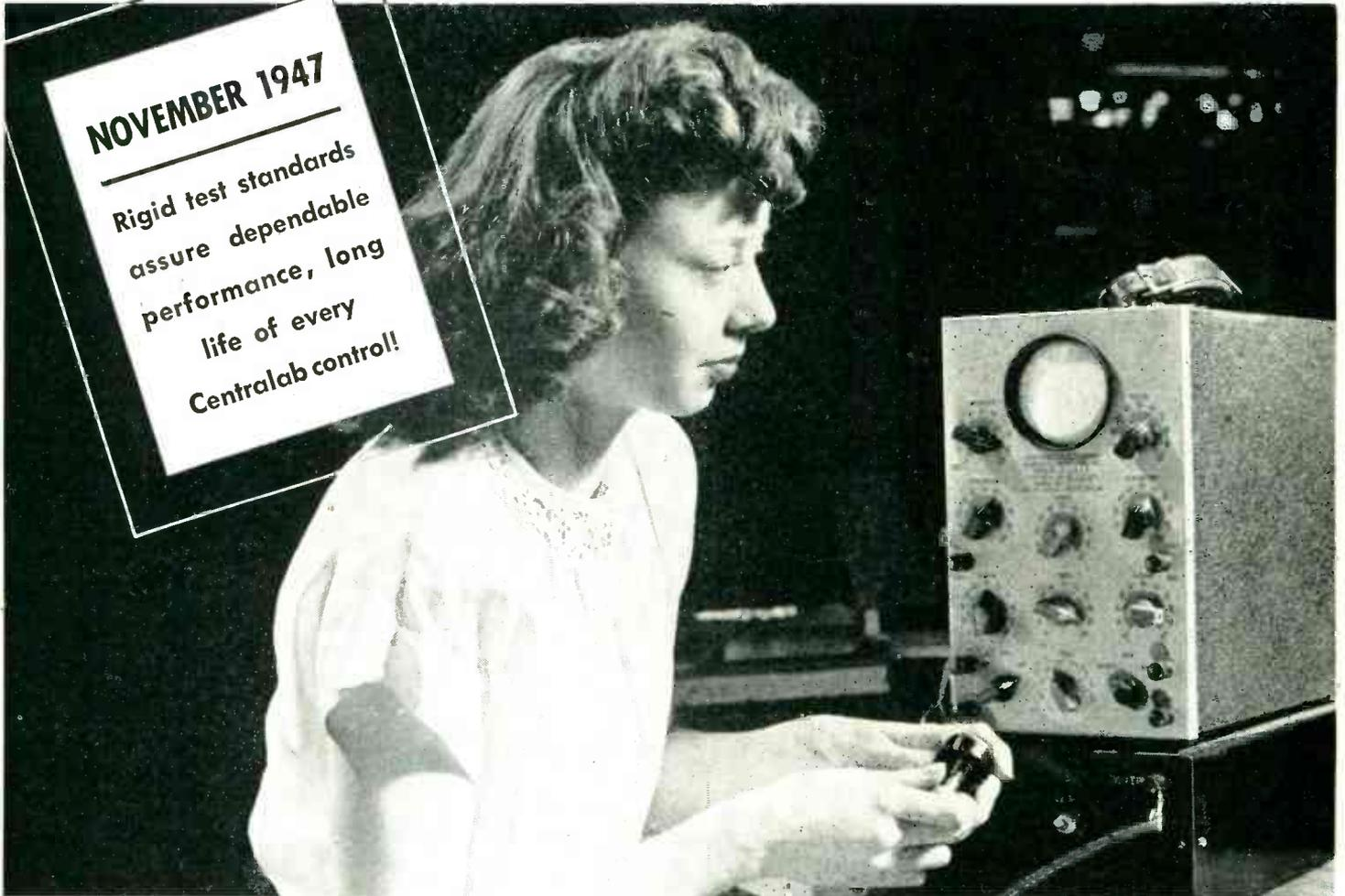
**1** 100% electrical test for continuity and "shorts" completes Centralab's program of tests for each control before it is shipped. This includes testing for resistance at various degrees of rotation, taper, noise, mechanical dimensions, etc. It's the
