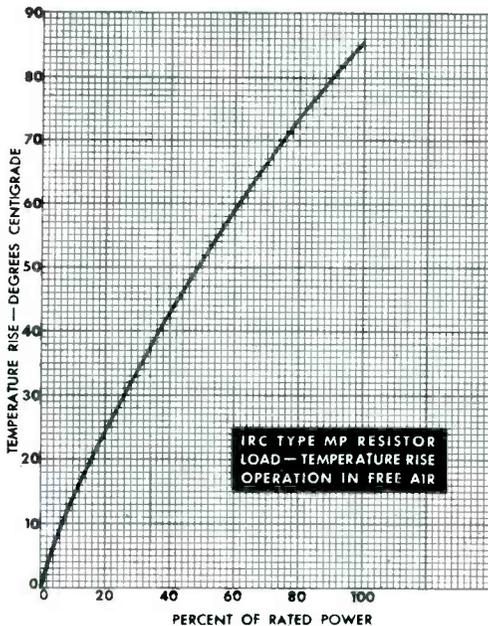
**DERATING.** Type MP Resistor power ratings are based on an ambient temperature of 20°C. When operated at any higher ambient, it is recommended that they be derated according to the following curve. For example, suppose an MPO Resistor is to be operated in an ambient temperature of 40°C. From the curve it is seen that the permissible load is 74% of the rated load. Since the MPO is normally rated at 30 watts, then at 40°C., it should not be loaded to more than 74% of 30 watts, or 22.2 watts.
