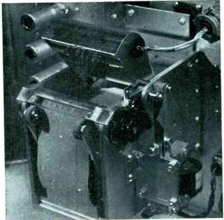
Six styluses projecting from the raised recorder head electrically mark the count on a 2.25-inch strip of Teledeltos paper. Strip is advanced in one-eighth inch steps by the ratchet wheel and magnet-actuated pawl on right of housing
