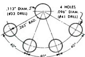
Recommended mounting template for Type SH Switch
