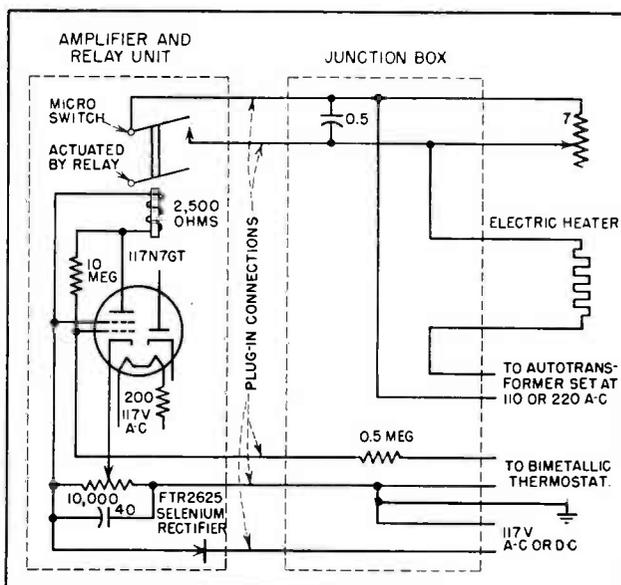
FIG. 2—Circuit of vacuum-tube relay having unique advantages for industrial control applications. Plug-in feature permits carrying standby unit in plant for quick replacement of entire amplifier unit in case of tube failure or other trouble
