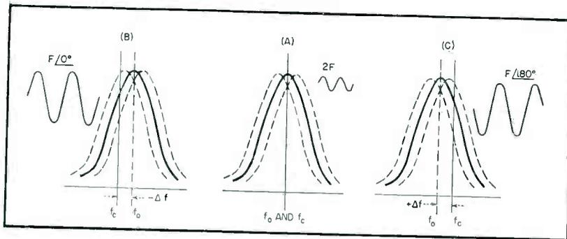
FIG. 1—Phase method of obtaining frequency drift sense
