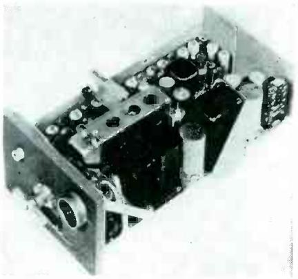
output is from 7 to 10 watts for a total transmitter drain of 20 amperes and a transmitter-receiver standby of 9.2 amperes. Full details of this equipment are available from the manufacturer.
