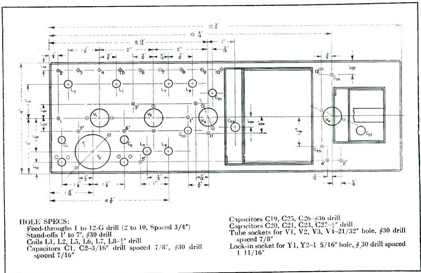
FIG. 3—Mechanical layout of chassis. Slight differences from layout shown in photos have been introduced to simplify construction. Relative location of tube sockets and resonators is critical
