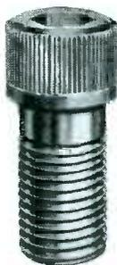
"Unbrako" Socket Head Cap Screws with the knurled head save assembly time because the knurling provides a slip-and-fumble-proof grip—though the fingers and head be ever so oily, therefore, they can be screwed in faster and farther before it becomes necessary to use a wrench. They can also be locked in place if heads are countersunk.
