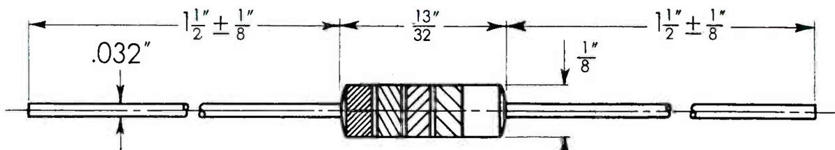
**POWER AND VOLTAGE RATING:** 1/2 watt (at 40°C. ambient)
