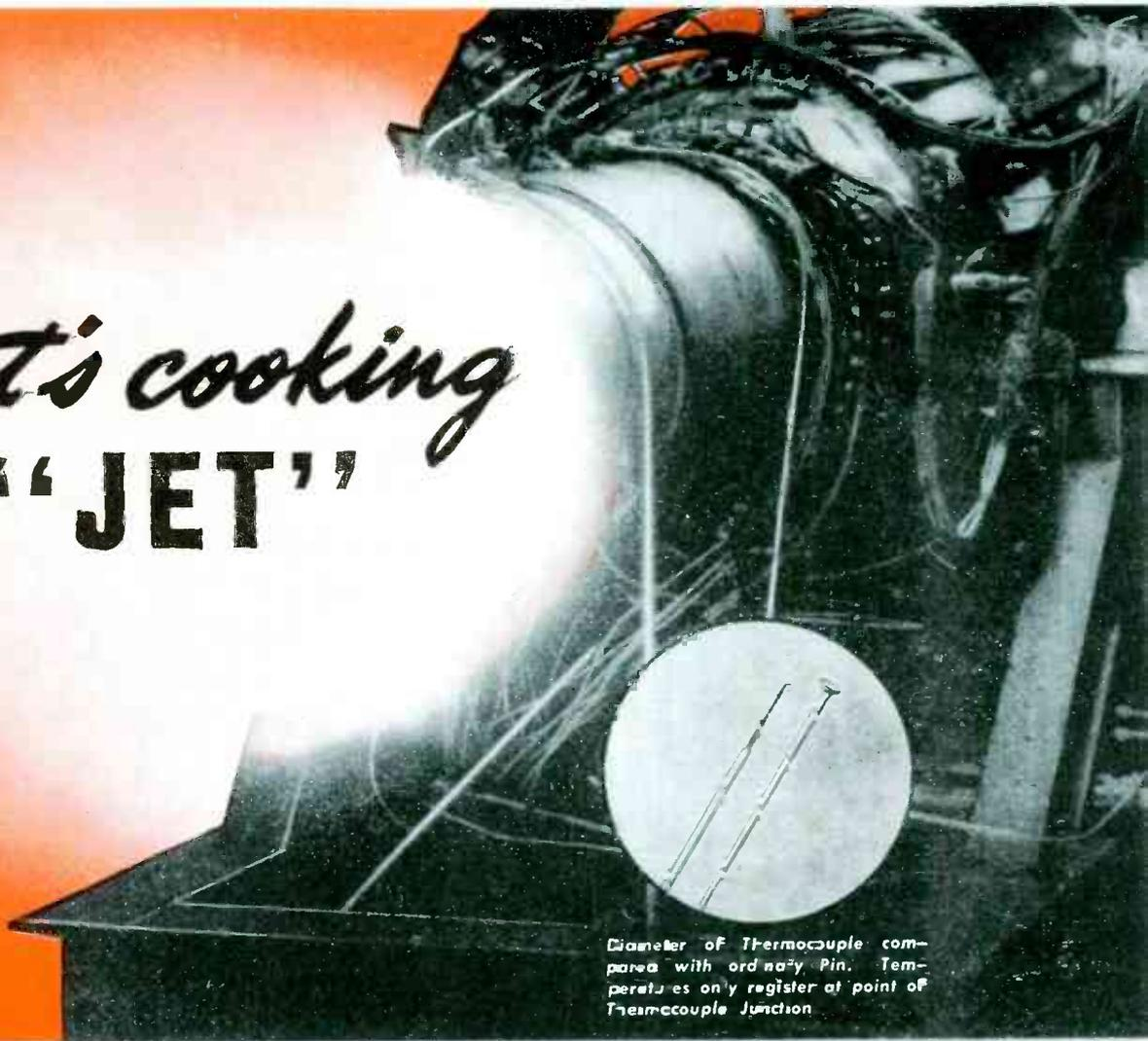
Diameter of Thermocouple compared with ordinary Pin. Temperatures only register at point of Thermocouple Junction
