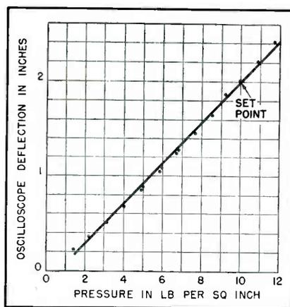
FIG. 4—Static calibration curve of pickup when using 0.02-inch thick steel diaphragm
