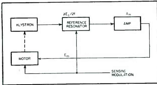
FIG. 3—A basic motor-operated automatic frequency control
