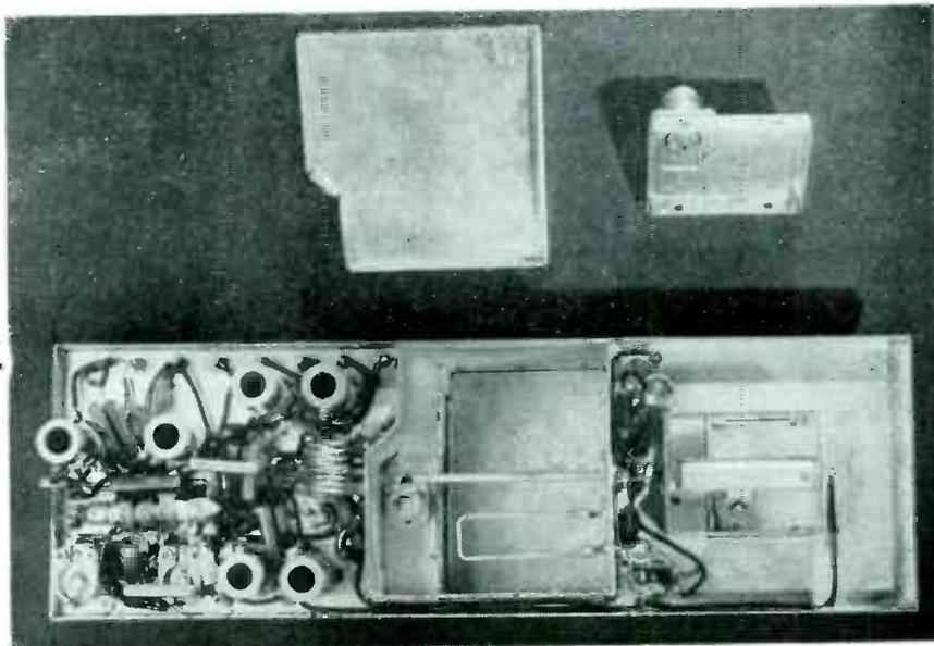
Bottom view, showing interior of resonators and coupling loops. Conventional coils are used up to 116 mc
