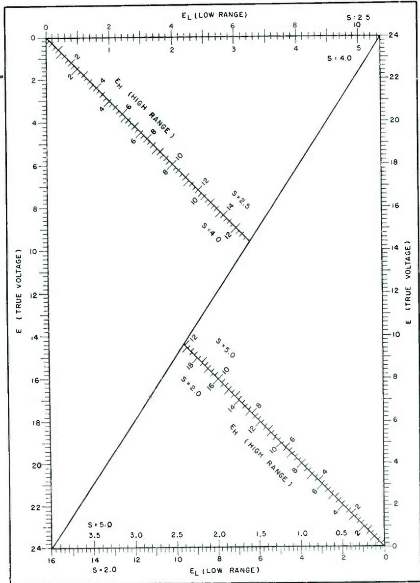
FIG. 2—Voltmeter loading nomograph. Take voltage readings on two ranges, divide higher range scale by lower to get  $S$  (either 2, 2.5, 4, or 5 on standard volt-ohm-millimeters), then place straightedge on measured values ( $E_L$  and  $E_H$ ) for  $S$  scale in question and read true voltage on adjoining  $E$  scale. If range of any scale is inadequate, multiply all scale values by 10, 100, or any other convenient factor
