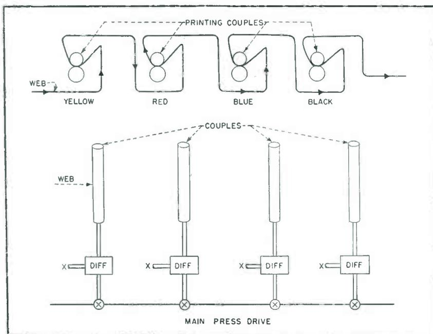
FIG 1.—Schematic views of mechanical arrangement of printing couples used in multicolor web. For register control, correction is applied to the differential systems at points marked X
