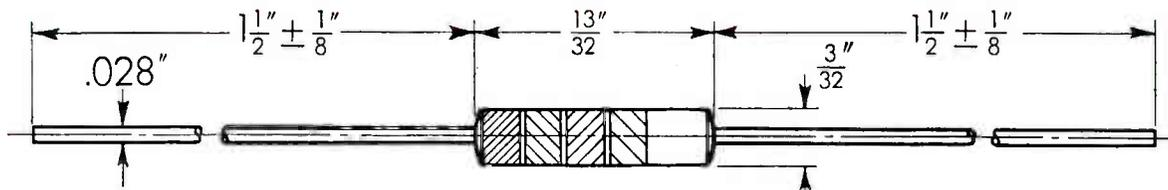
**POWER AND VOLTAGE RATING:** 1/3 watt (at 40°C. ambient)
