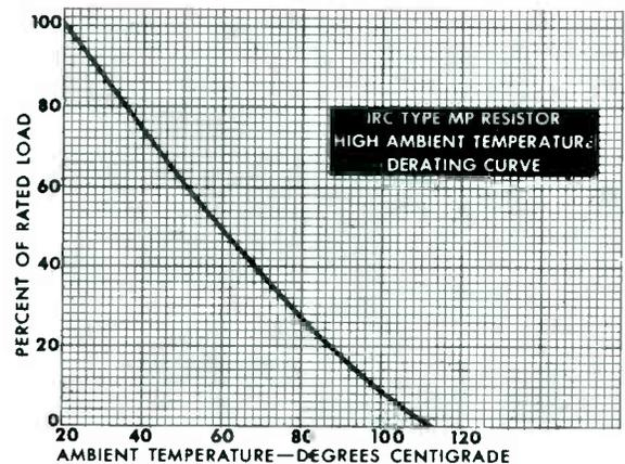
**TEMPERATURE COEFFICIENT.**  $-.005\%$  °C. for low resistance to  $-.07\%$  °C. for high resistance value.
