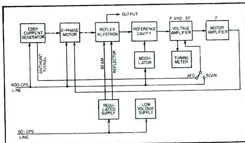
FIG. 9—Block diagram of an afc system with automatic scan
