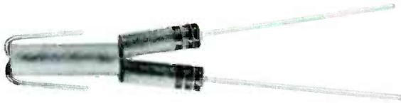
IRC Matched Pairs—two resistors matched in series or parallel to as close as 1% initial accuracy provide a dependable low cost solution to close tolerance requirements.
