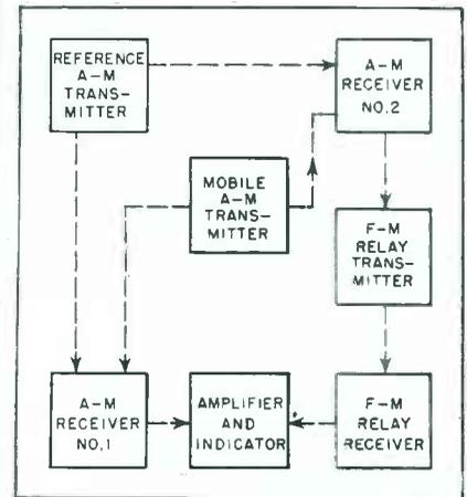
FIG. 1—Airline distance is measured with this setup
