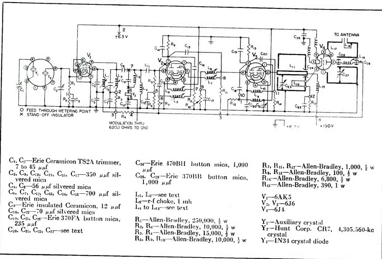
FIG. 2—Complete schematic of transmitter. Socket orientation and feed-through numbers correspond to mechanical layout of chassis, shown in the drawing at the right
