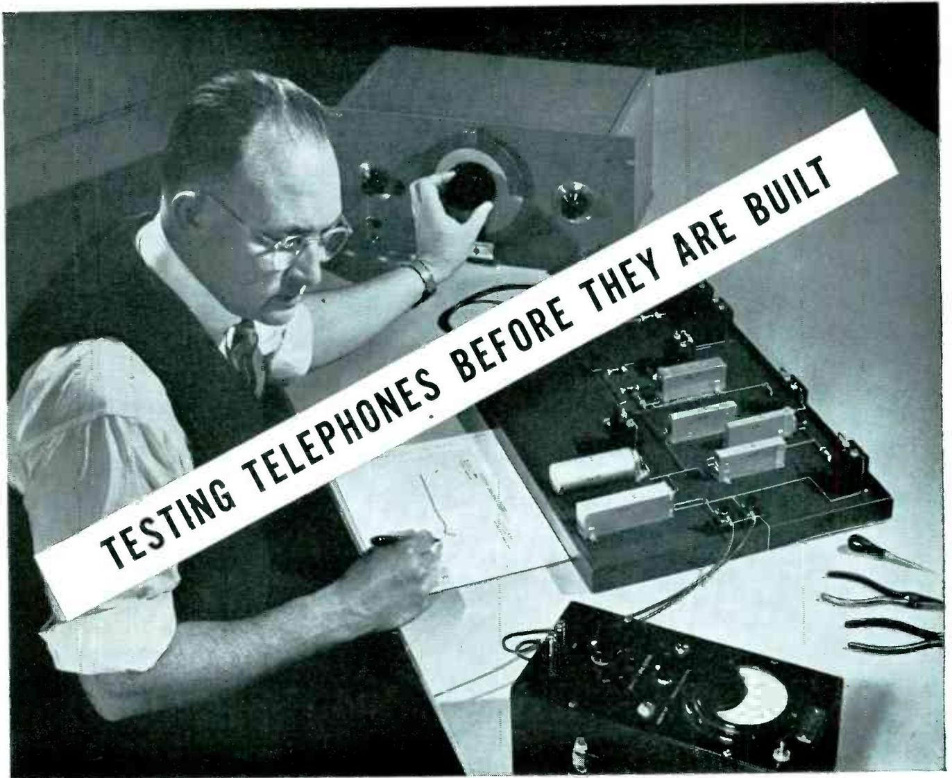
**A** TELEPHONE RECEIVER is a complex system of electrical and mechanical elements. Its coils, magnets, diaphragm and cap react on each other as they convert the electrical waves of your voice to sound waves. What is the best size for the holes in the ear cap? Will  $1/10000$ th inch greater thickness help a receiver diaphragm to carry your telephone voice more clearly? One way to find out is to build numerous experimental receivers and test them.
