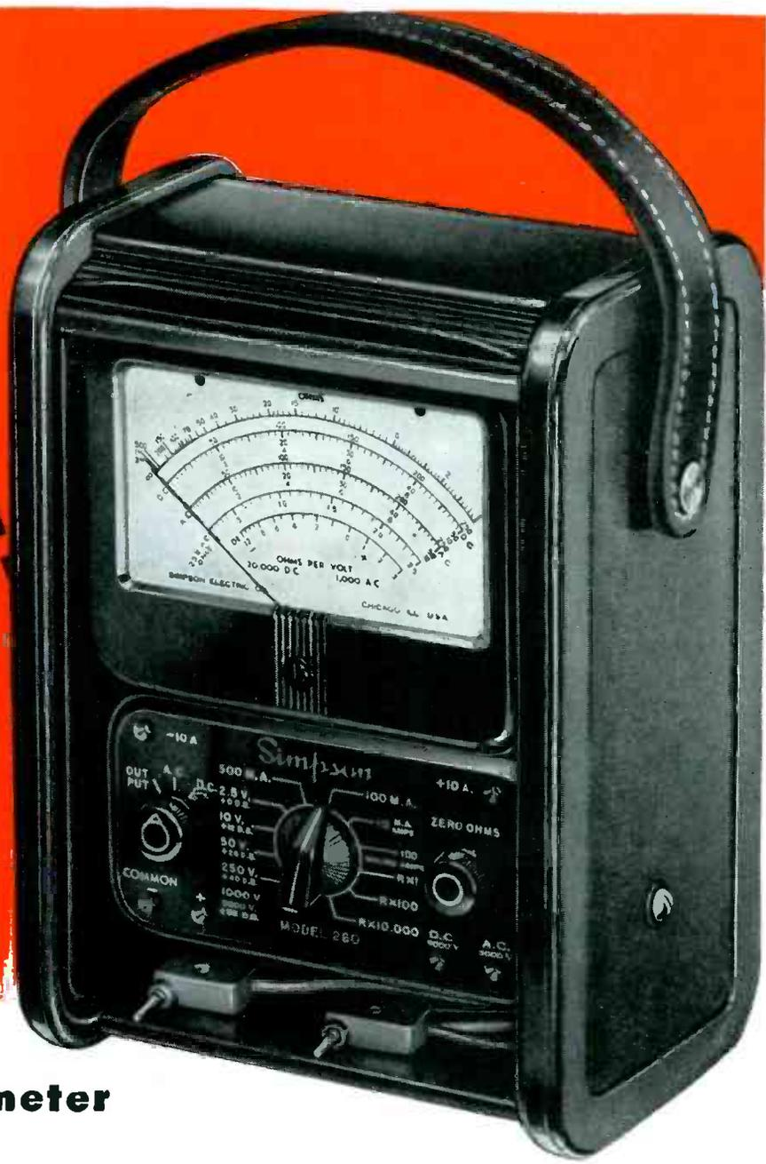
At 20,000 ohms per volt, this instrument is far more sensitive than any other instrument even approaching its price and quality. Unequaled for high sensitivity testing in radio and television servicing and in industrial applications.
