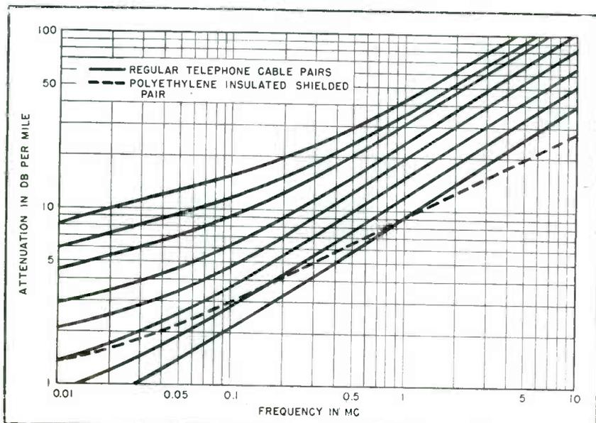
FIG. 1.—Transmission loss-frequency characteristics of regular telephone cable pairs as compared with the characteristic of a polyethylene-insulated shielded pair
