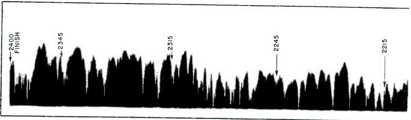
Example of strip chart obtained with sky-wave signal recording equipment at Strathburn, Ontario. Curve shows variation in input signal strength to receiver over period of several hours at night for signals of station WGY, Schenectady, N. Y.
