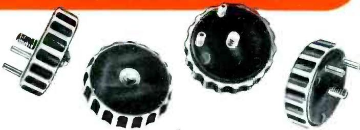
**RESISTANCE ELEMENT:** IRC Metallized coating, bonded to a phenolic strip, cured and stabilized at high temperature, in the same manner as IRC Type CS and D Controls. *Integral molding of this element with the phenolic base results in improved strength, more efficient heat dissipation, and increased resistance to humidity.*
