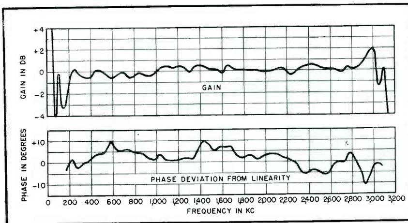
FIG. 7—Transmission and phase characteristics of the New York-Washington coaxial television circuit. Video bandwidth is limited to about 2.8 mc by the characteristics of the repeaters used
