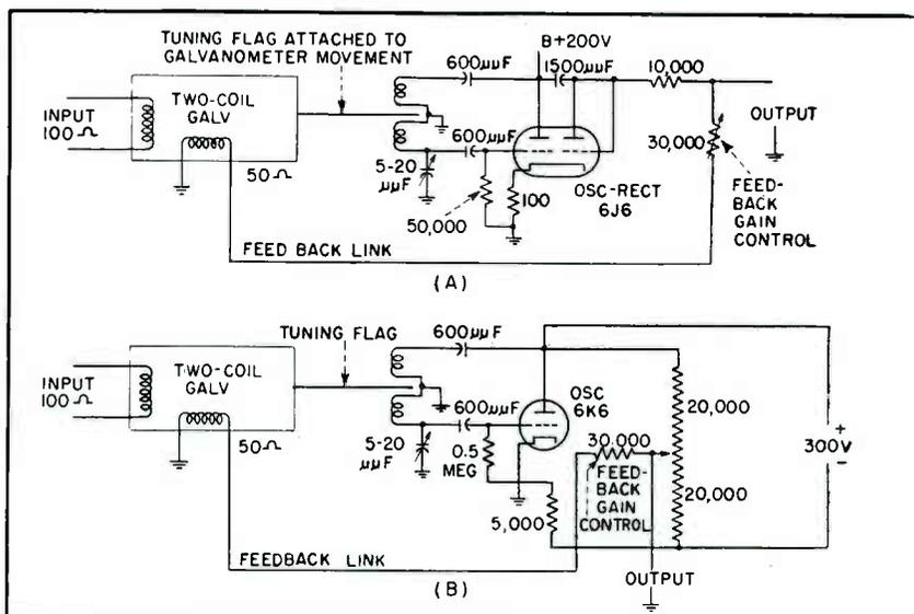
tween coils of a tuned-grid, tuned-plate oscillator. The motion of the metal flag loads and unloads the tank circuits with consequent variation in input voltage of the oscillator. With a reasonably sensitive galvanometer movement, such a conventional setup can easily provide voltage gains higher than  $10^6$ .
