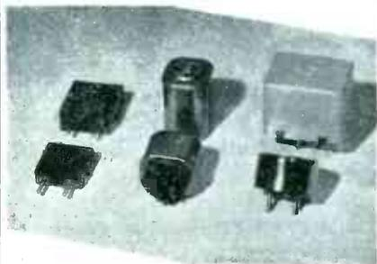
Plated quartz crystal oscillator and resonator bars mounted between resonant frequency pins and housed in metal holders—hermetic sealing and temperature control optional.
