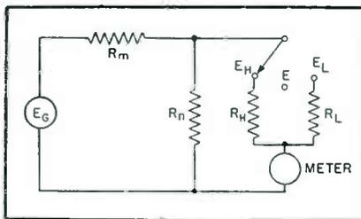
FIG. 1—Circuit of two-range voltmeter used as example
