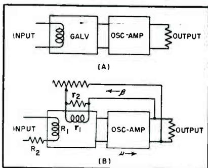
FIG 1—Basic principle of the electromechanical system is illustrated at (A). The method of adding feedback is shown at (B)
