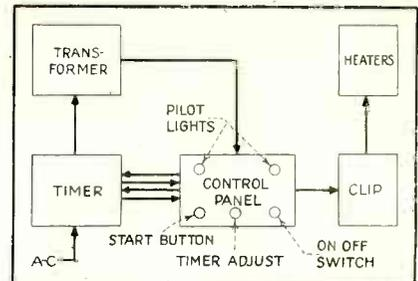
Block diagram of the electronically controlled permanent wave machine
