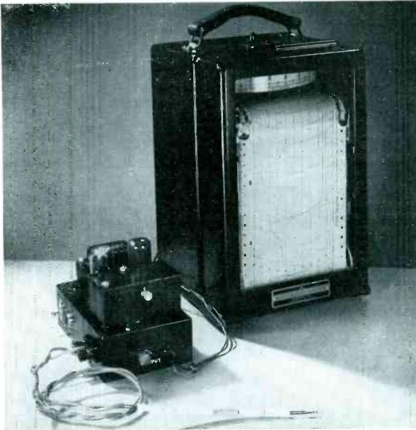
Small chassis at left contains the d-c amplifier and power supply used with the recorder and thermocouple (bottom) to measure transients in a thermal process
