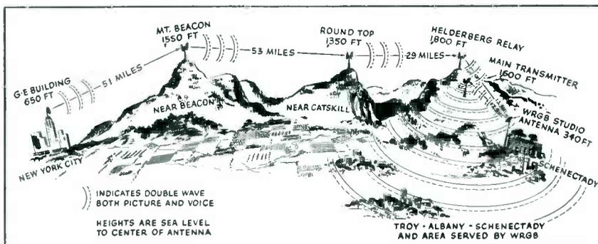
New York-Schenectady television relay using frequencies between 1,800 and 2,000 mc. The New York receiving point can pick up Washington, Philadelphia, or New York station programs, which are then relayed and rebroadcast from Schenectady
