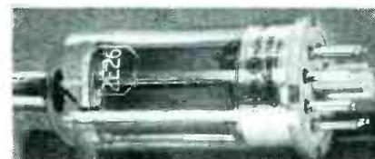
transmitters either as a driver or low-power output, the type GL-2E26 is a five-electrode beam power amplifier with 12.5 watts plate dissipation. Maximum ratings apply up to 125 megacycles.
