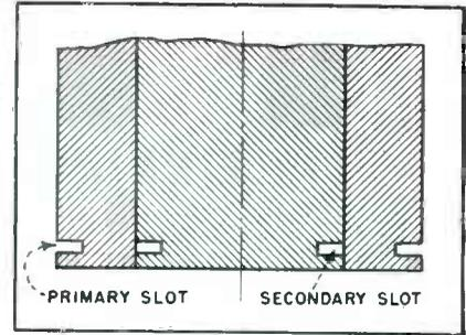
FIG. 2—Cross section of probe coil form
