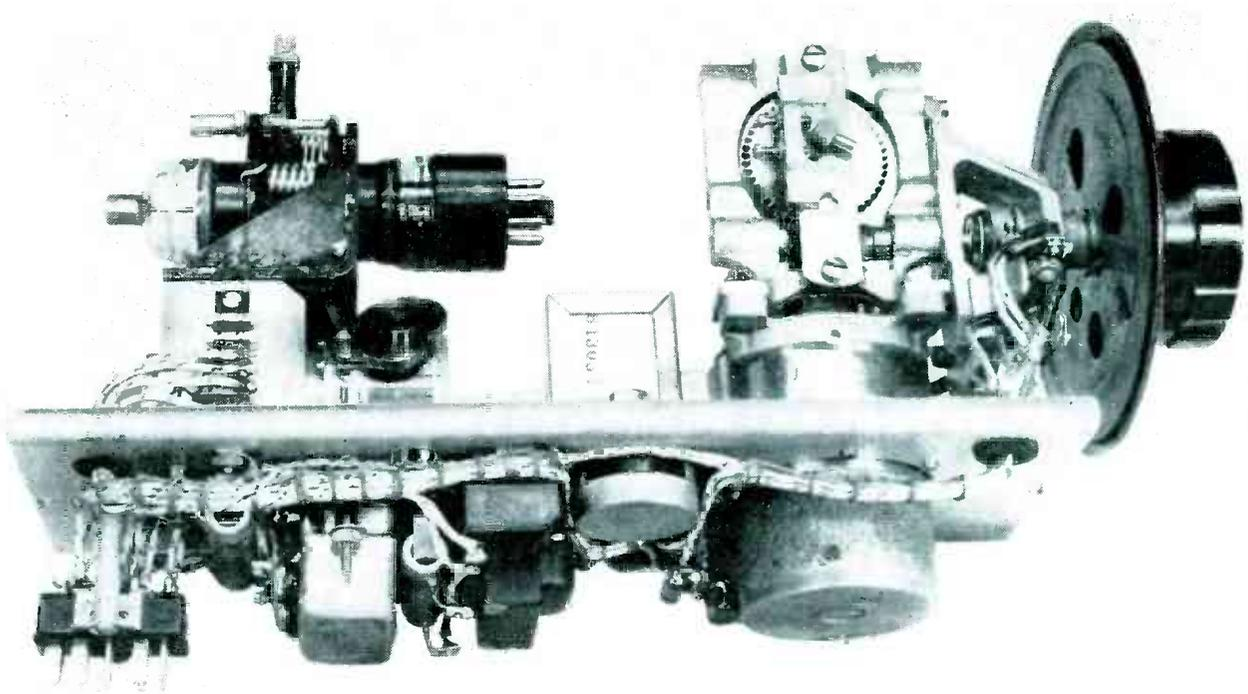
Microwave section of signal generator. Resonator and speaker-unit modulator are shown beneath the gear mechanism at right. Tuning motor with cam is above chassis at left
