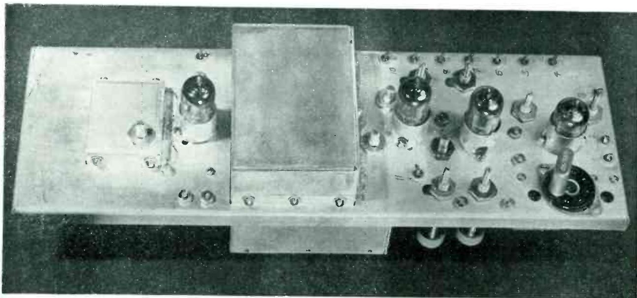
Top view of transmitter. Output of 4.3-mc crystal (lower right) is multiplied 108 times in three tubes to 465 mc. Final stage, a 6J4 triode (left), produces one-quarter watt output
