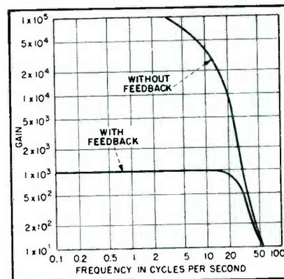
FIG. 5—Frequency characteristics of the electromechanical system with and without feedback
