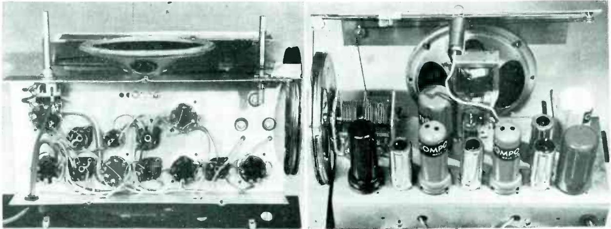
**P**HOTOGRAPHS here show how Cosmo Electronic Corp., New York City, achieves complete plug-in construction (except for the gang tuning capacitor) in their five-tube universal a-c/d-c superheterodyne radio receiver. Promotion will feature ease of servicing; any plug-in unit, including loudspeaker unit which screws to chassis but has plug-in connections, is to be available from dealers at price of \$1.85.
