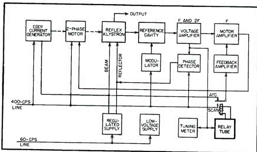
FIG. 7—Block diagram of a motor afc system connected for antihunting
