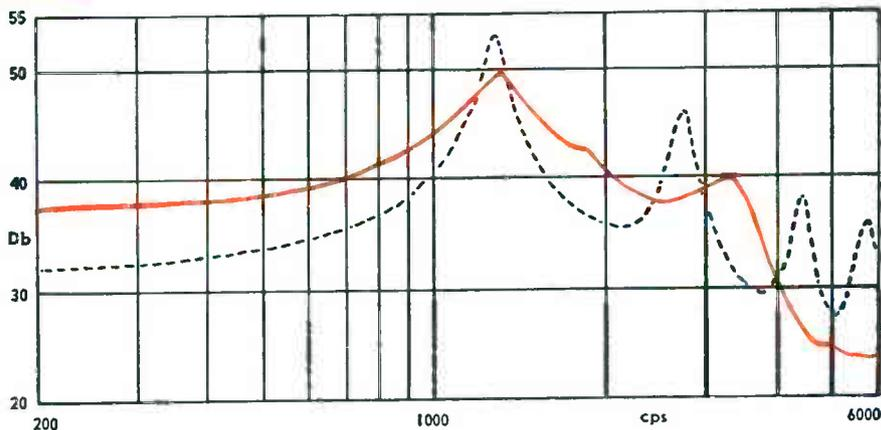
\*The curves shown are from our actual laboratory tests. The input to the receivers was held constant at 5 volts. The pressure output of the receiver was measured with a 2 cc cavity artificial ear with ear tip. 0 Db reference is 1 dyne/cm<sup>2</sup>.
