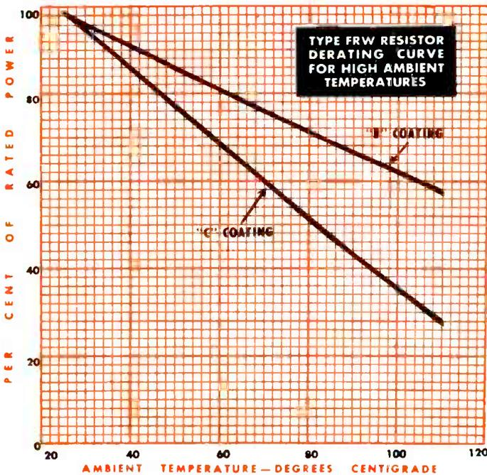
**DERATING.** If necessary to operate Type FRW Resistors in an ambient higher than 25° C., it is recommended that they be derated according to the Derating Curve for High Ambient Temperatures. For example, if the resistor is normally a 50-watt type and is to operate at 60° C. ambient, it should not be loaded to more than 82% of 50 watts, or 41 watts.
