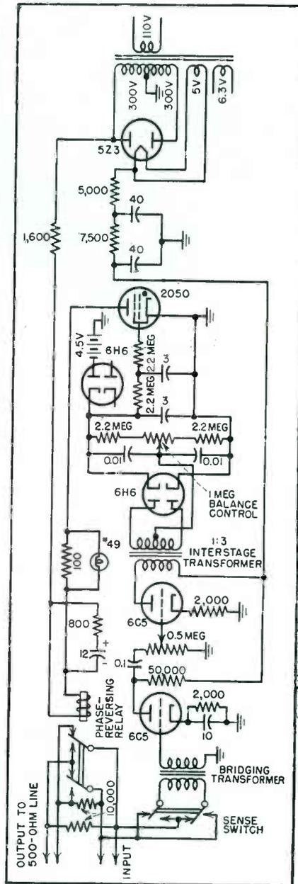
Automatic phase reversal of an audio signal is done by this circuit
