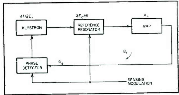
FIG. 4—A basic electronic automatic frequency control
