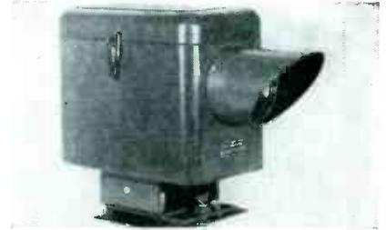
distances up to 1,000 ft. Its applications include traffic control, counting and limiting, and the like. The light source contains a lamp, transformer, and motor-driven slotted disk which modulates the light beam at about 900 cps. The relay, because of its tuned circuit, is responsive only at this frequency.
