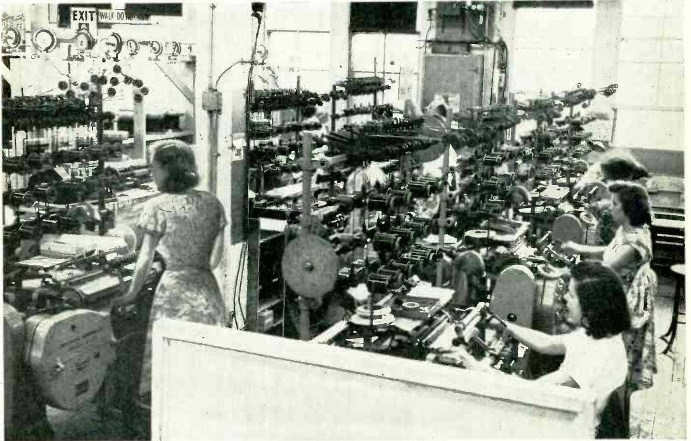
Transformer coils are wound, 14 at once on the same machine, at speeds up to 2500 rpm . . . on the No. 104 Universal Coil Winding Machines used by a company famous in the field of electronics.
