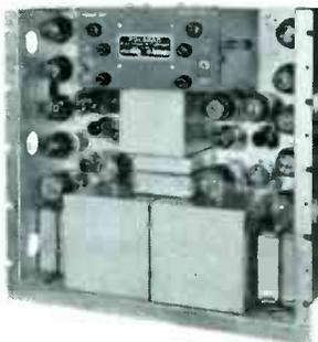
Each Power Unit has its own power switch, fuses, pilot light, and voltage control.
