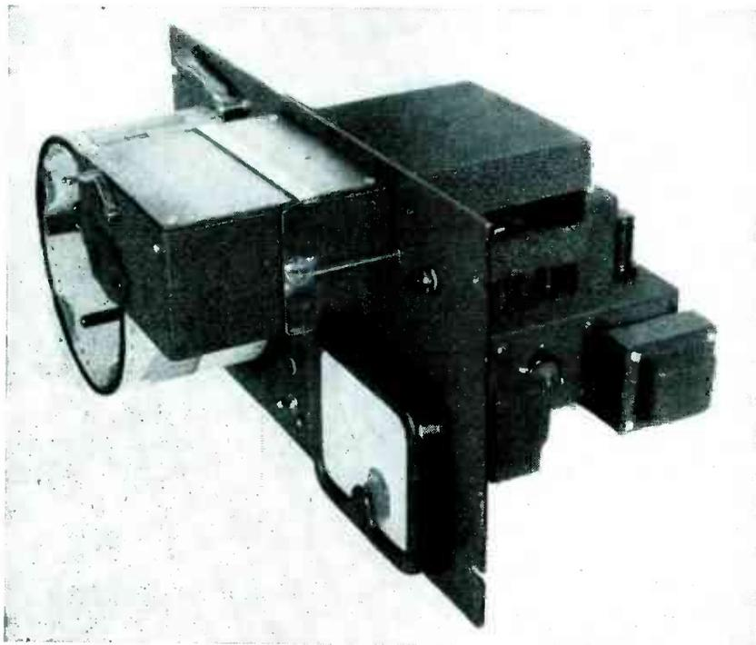
Electronic scanner unit used at Radio Standards Office in Ottawa for analysing sky-wave charts obtained with recording equipment. Logarithmic calibration chart is placed under pointer on table just above drum. Pointer is mechanically coupled to optical system
