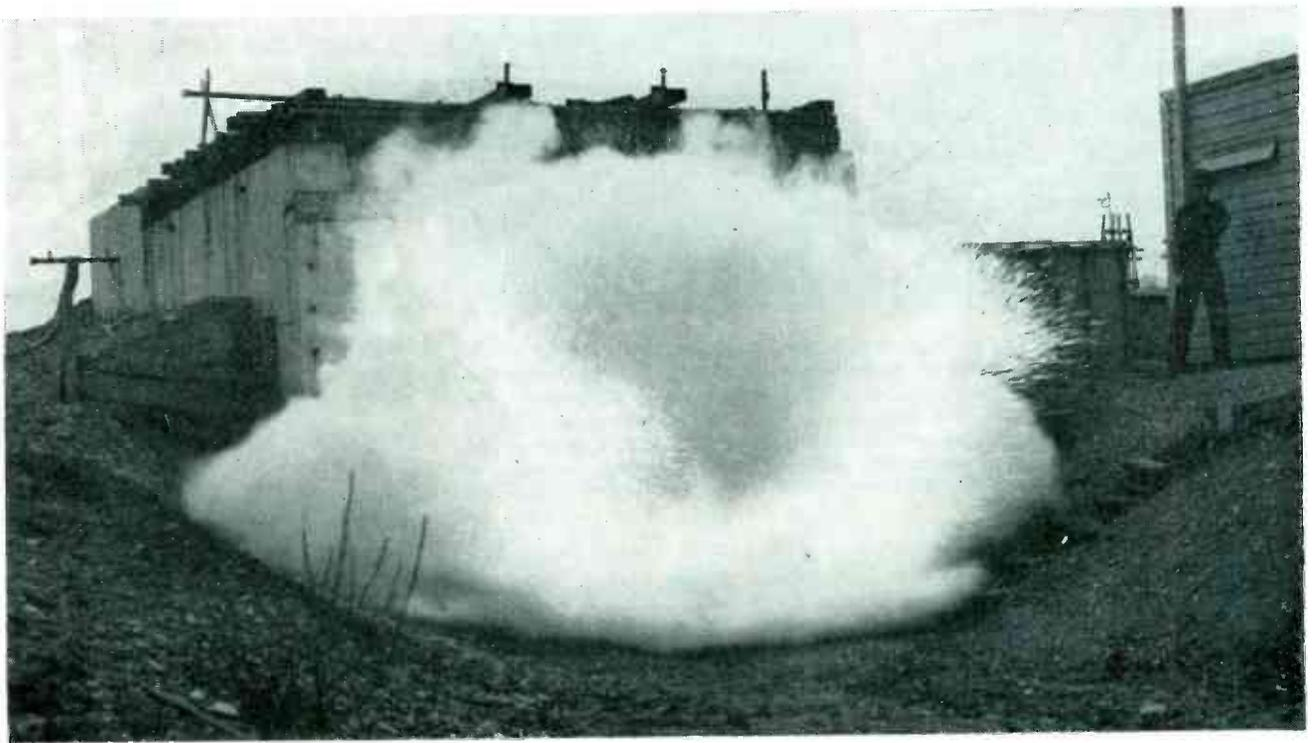
Explosion of magnesium powder in a heavy concrete test tunnel at the Factory Mutual Laboratories is typical of accidental explosions but is set off under controlled conditions so that pressures can be measured and recorded to determine safety of various industrial conditions. Other tests include explosions of cleaning fluids in enclosed spaces and explosions of black powder in pipes
