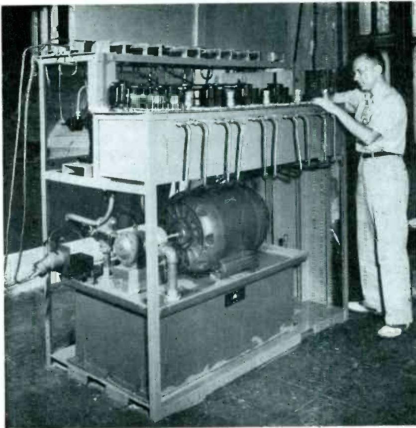
Complete setup of electronic and hydraulic units that connect to the printing press. Five 24-tube chassis are being immersed in oil inside the long steel box in which they normally operate
