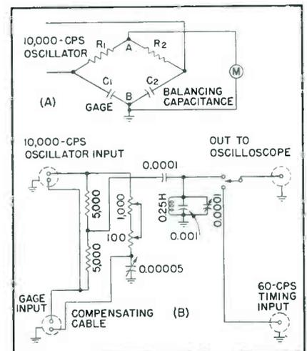
FIG. 2—Basic bridge circuit (A) used with gage, and final version (B) using tuned filter and compensating cable for limiting response to narrow band of frequencies around 10,000 cps
