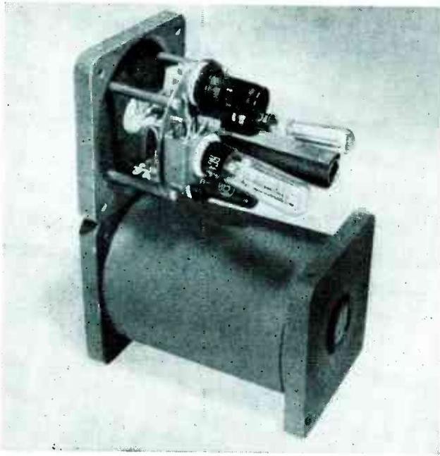
The pickup head and explosion-proof housing are mounted on the press. It contains two phototubes and two amplifier tubes so that if one set fails, the other set is switched into the circuit
