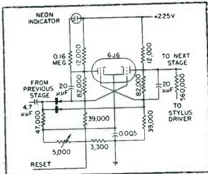
FIG. 2—Binary counter stages use this typical flip-flop circuit
