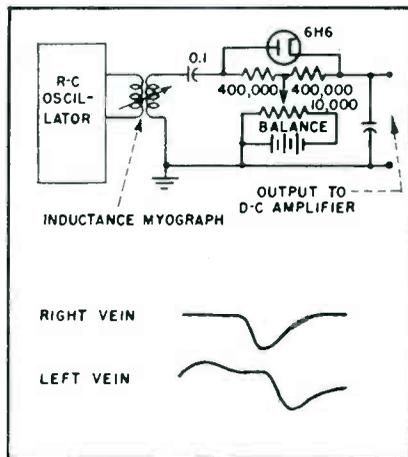
FIG. 2 — Two variable-inductance myographs, of the type shown in the schematic diagram, were used to make this record of fractionate contraction of the veins going to a turtle heart
