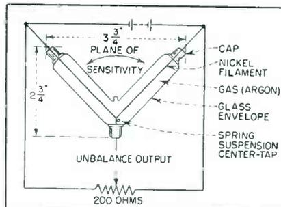
Convection vertical position sensing tube made by Eclipse-Pioneer Div. of Bendix changes resistance of its two arms when displaced in the plane through its legs
