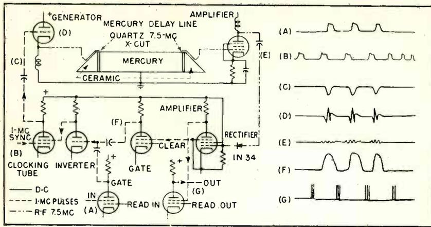
FIG. 2—Waveshapes at critical points throughout the recirculation mercury memory are shown at the right
