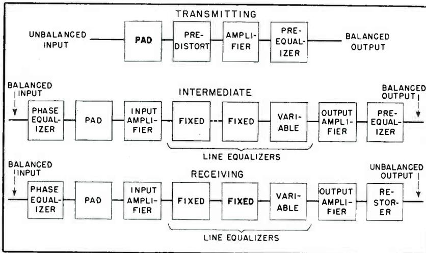
FIG. 3—Unbalanced-input transmitting amplifiers and unbalanced-output receiving amplifiers readily permit interconnection of broadcasters' equipment
