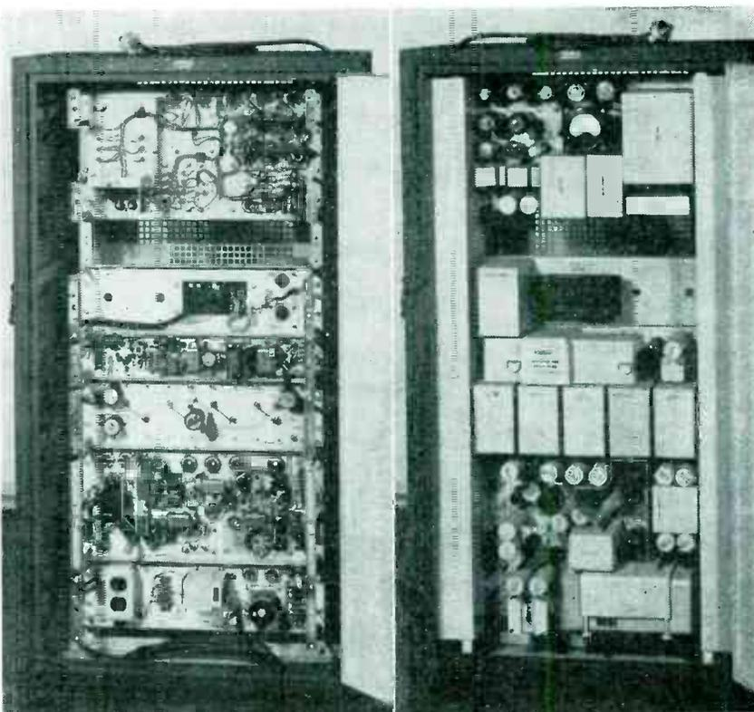
FIG. 2—Front and rear views of video amplifiers used in short haul circuits
