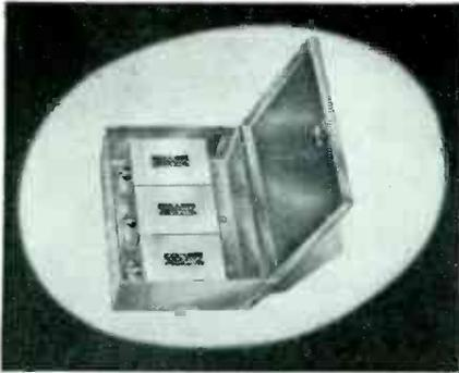
Solar Type EB series Elim-O-Stat radio interference filters are intended for heavy-duty service in 1, 2 and 3 phase circuits and equipment drawing from 5 to 200 amperes, 250V a-c/600V d-c. Voltage drop is negligible.
