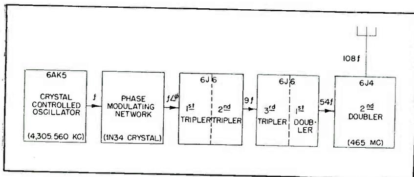
FIG. 1—Block diagram of transmitter. Tubes are conserved by operating three 6J6 triode sections as triplers. Phase modulation network produces 25-kc deviation
