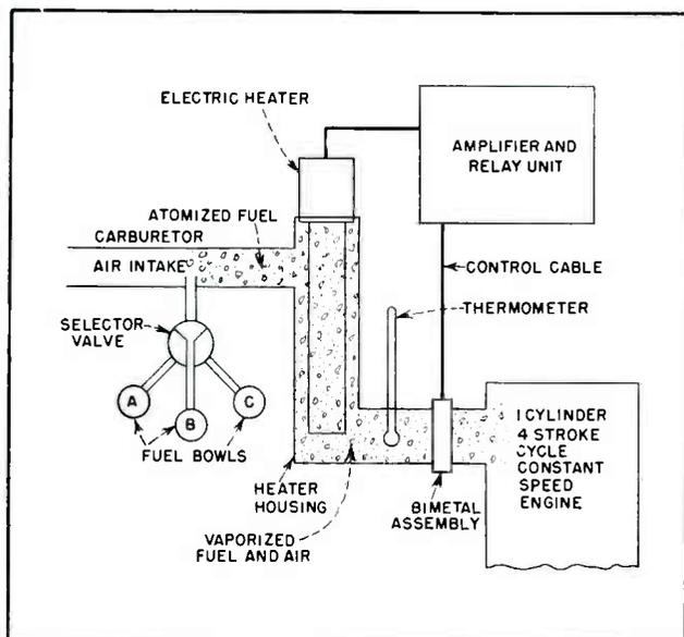
FIG. 1—Block diagram of knock-testing engine used for determination of octane ratings of various gasolines in refineries and petroleum-testing laboratories, showing location of bimetal assembly used with vacuum tube for temperature control
