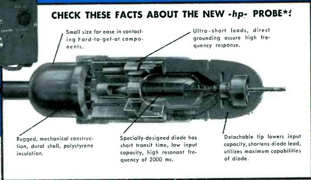
Small size for ease in contacting hard-to-get-at components.
