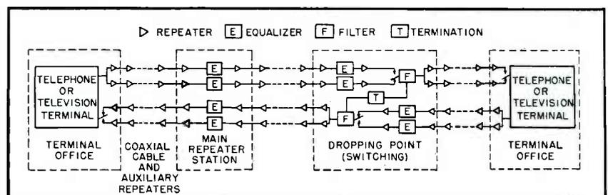
FIG. 6—An auxiliary parallel circuit in each direction is provided for emergency use in this layout of a typical coaxial system
