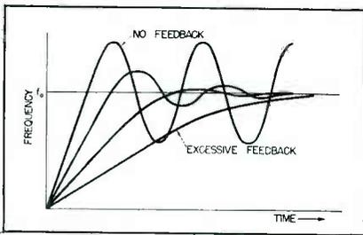
FIG. 5—Motor tuning time plotted against corrective feedback
