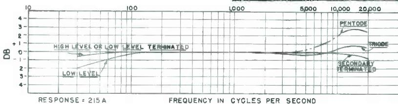
Low frequency response—(referred to 1000 cps) (High level + 26 vu, Low level - 15 vu.):
