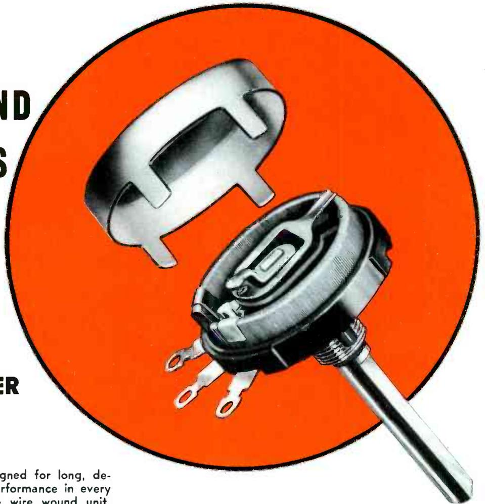
The IRC Type W Control is designed for long, dependable service and balanced performance in every characteristic. A 2 watt variable wire wound unit, this control provides maximum adaptability to most rheostat and potentiometer applications within its power rating. Its small 1 1/4" by 9/16" design features the exclusive IRC spiral spring connector, a long-wearing alloy contactor, and welded connections between resistance element wire and terminals.
