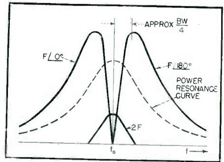
FIG. 2—Resonator-detector output
