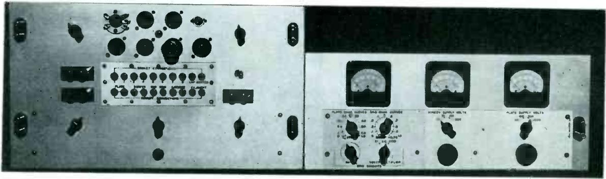
Front panels of equipment contain sockets for all types of tubes
