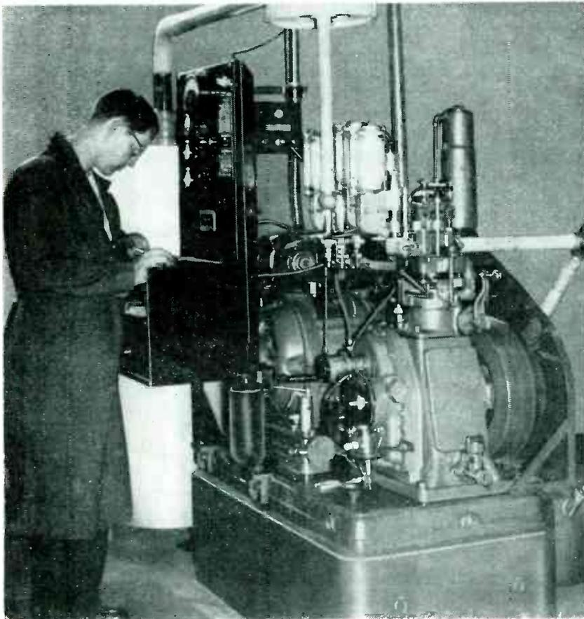
Knock-testing engine in Ethyl Corporation plant, using Malraison Mixture Thermostat for maintaining temperature of gas-air input mixture within 2 degrees of 300 F as indicated by mercury thermometer. Vacuum-tube relay housing is mounted behind control panel at eye level
