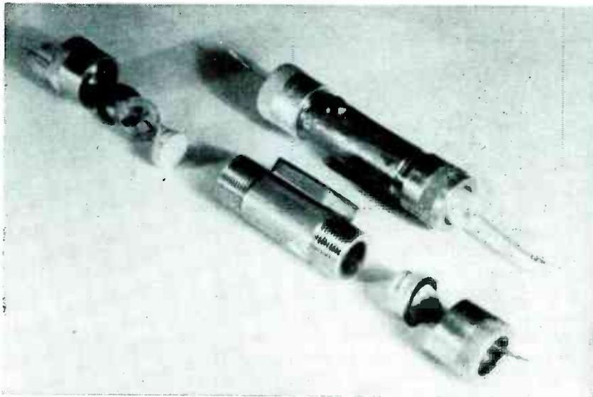
This 2-inch long mercury line introduces about 40 microseconds delay
