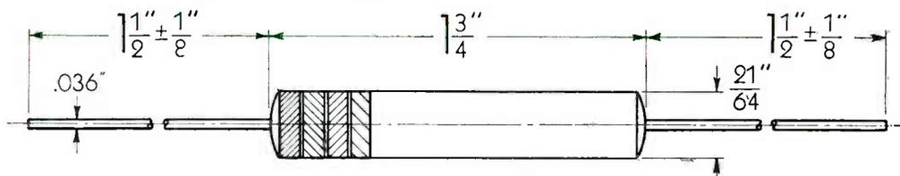
**POWER AND VOLTAGE RATING:** 2 watts (at 40°C. ambient)
