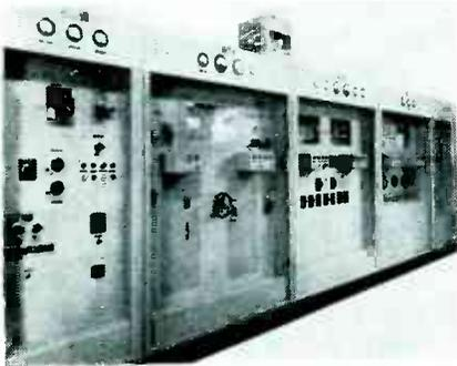
transmitter illustrated features front-panel continuous tuning over its entire frequency range from 2.85 to 22.5 mc.
