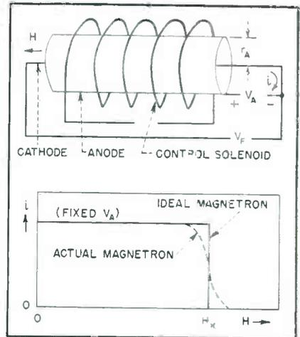
At the top is the basic magnetron connection; current in the solenoid produces a magnetic flux  $H$ . Below is the magnetron characteristic for a fixed anode-cathode potential, decreasing that potential moves the cutoff to the left, decreasing the heater current lowers the saturation current available at low magnetic flux
