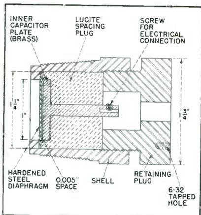
FIG. 1—Cross-section of capacitance-type pressure pickup. Sound waves act on steel diaphragm at left, causing capacitance between grounded diaphragm and insulated brass plate behind it to vary. Shell and retaining plug are turned from 1 3/4-inch hexagonal steel stock
