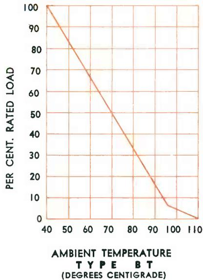
Ratings of Type BT are based on an ambient temperature of 40°C. Ambient conditions as well as voltage ratings and actual power requirements should be considered when determining the proper size of resistor for any application. When BT's are used at ambient temperatures exceeding 40°C., load should not exceed that indicated by the JAN-R Derating Curve reproduced here.
