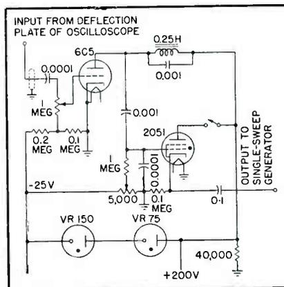
FIG. 5—Automatic tripper circuit for starting single-sweep generator when voltage on deflection plate of cathode-ray oscilloscope reaches about 5 percent of maximum
