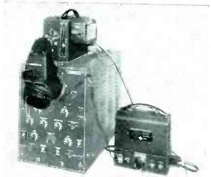
film records of the tube displays. Speed of the film is variable so as to allow recording of successive traces at the instant of their presentation. The film can be driven in conjunction with the sweep or the film itself can be used as the sweep, giving a continuous record.
