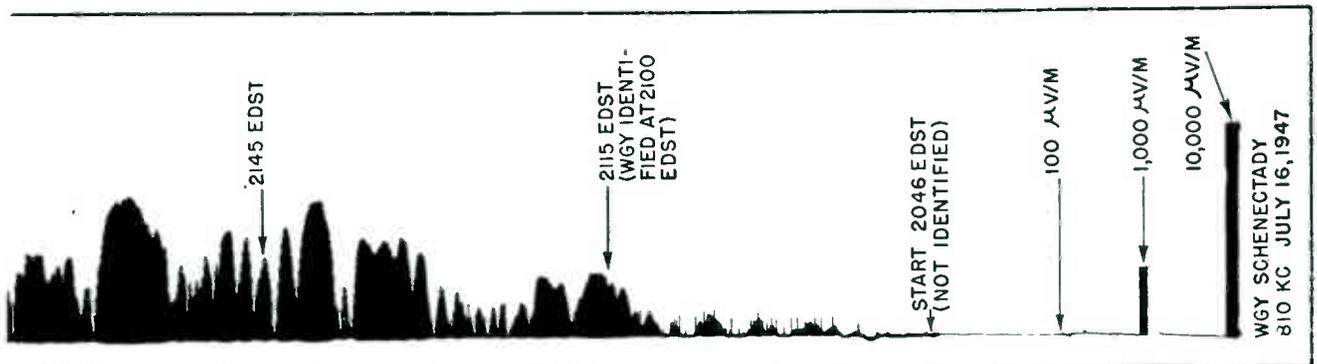
Analysis of above chart with photoelectric scanner showed that signal exceeded 6,100  $\mu\text{V}$  5% of the time, 5,300  $\mu\text{V}$  10%, 3,000  $\mu\text{V}$  30%, 1,700  $\mu\text{V}$  50%, 1,400  $\mu\text{V}$  60%, 820  $\mu\text{V}$  90%, and exceeded 700  $\mu\text{V}$  95% of the time
