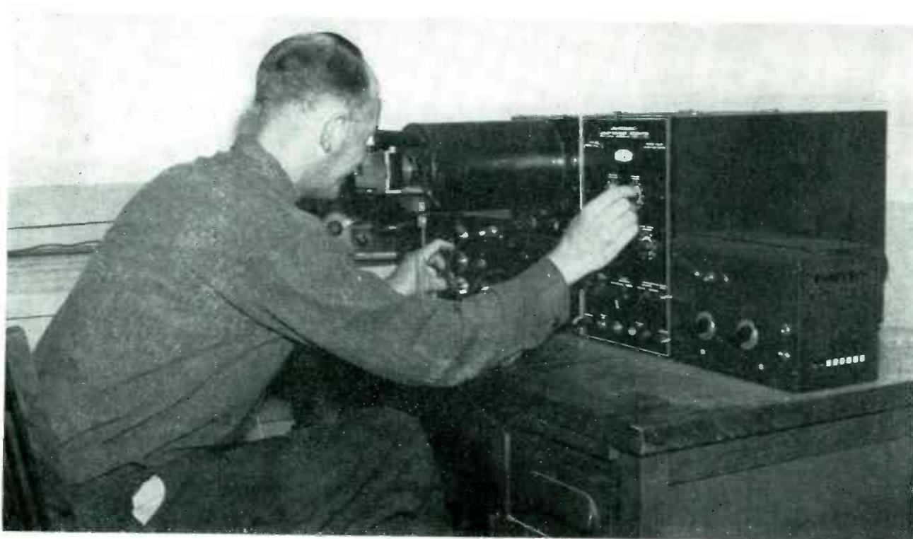
Explosion-pressure recorder setup for use with remotely located capacitance-type pressure pickup. Operator adjusts bridge control unit with left hand and single-sweep generator with right hand while viewing pattern on oscilloscope screen through peephole alongside camera on hood. Unit at right is sweep tripper control unit
