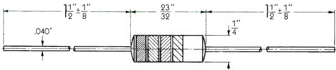
**POWER AND VOLTAGE RATING:** 1 watt (at 40°C. ambient)
