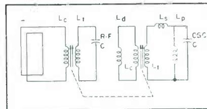
Method of neutralizing effect of loop antenna reactance on tracking of permeability-tuned receiver
