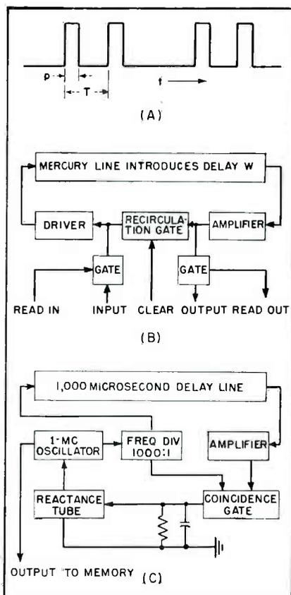
FIG. 1—For use with delay lines, information is in the form of pulse chains (A). These chains can be recirculated (B) through gates and the line so as to be stored as long as necessary. To compensate for temperature effects on the mercury lines, a timing oscillator (C) can be frequency controlled by an auxiliary line, the output being used to time pulses to the bank of mercury memories
