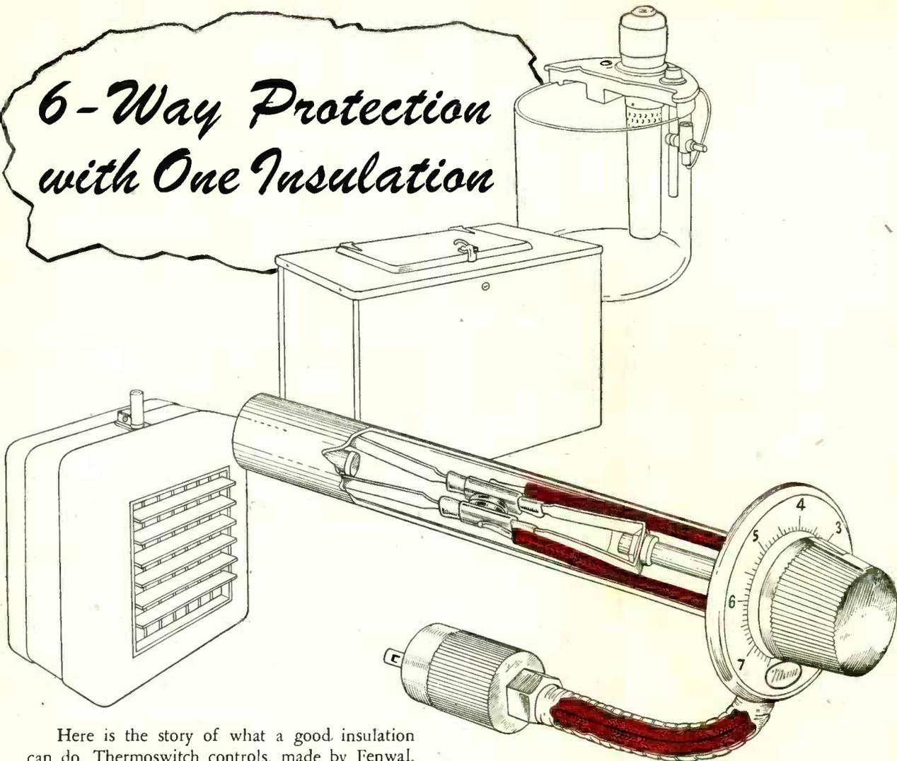
Here is the story of what a good insulation can do. Thermostats, made by Fenwal, Inc., are used in a wide variety of applications—unit heaters, home freezers, laboratory water baths, to mention only a few. The insulation is constantly subjected to (1) heat up to 700°F., (2) cold as low as -120°F., (3) extreme vibration, (4) friction, (5) bending, and (6) abrasion.
