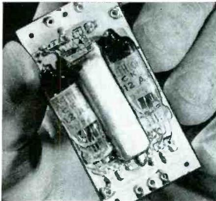
**4** Newest development of the "Printed Electronic Circuit", CRL's *Ampec* is a complete 3-stage audio amplifier. Get complete facts in Bulletin 973.
