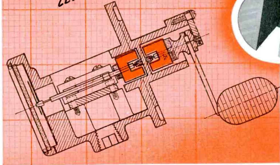
Here's another outstanding application for one of the many G-E permanent magnet materials — the magnetic liquid level gage manufactured by The Boston Auto Gage Company.
