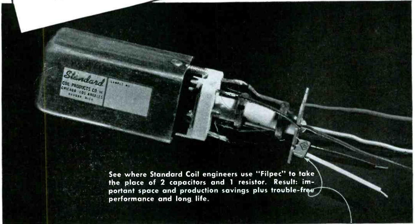
See where Standard Coil engineers use "Filpec" to take the place of 2 capacitors and 1 resistor. Result: important space and production savings plus trouble-free performance and long life.
