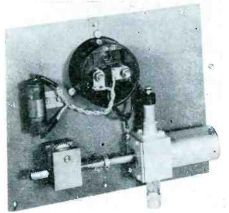
FIG. 1—A 5 to 30-cm searching wavemeter with finger contact to inner conductor
