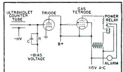
FIG. 3—Sensitive relay required in circuit of Fig. 2 is eliminated by use of thyratron
