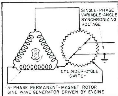
FIG. 1—Simplified circuit diagram of synchronizing voltage generator
