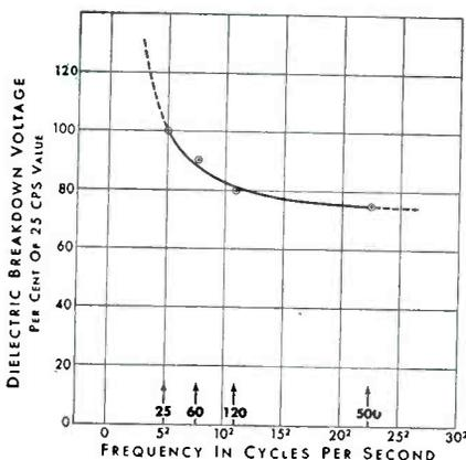
Figure 1: Effect of frequency on dielectric breakdown of transformer insulation. (Curve is based on findings of F. W. Peek)
