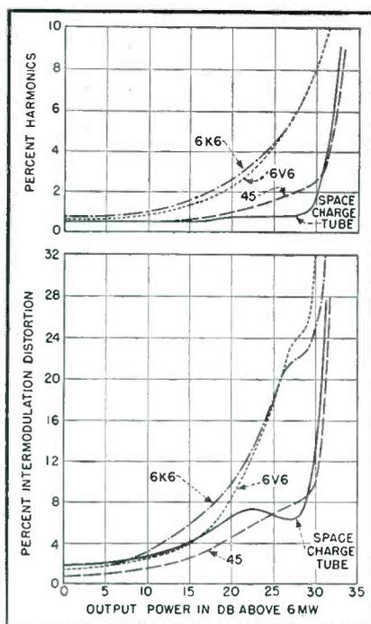
FIG. 1—Harmonic and intermodulation distortion versus output for resistive load
