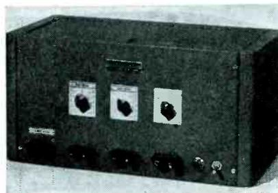
B supplies delivering from 0 to 300 volts at currents up to 120 milliamperes, one variable C supply delivering from - 50 to + 50 v at 5 ma, and one heater supply delivering 6.3 volts at 5 amperes.
