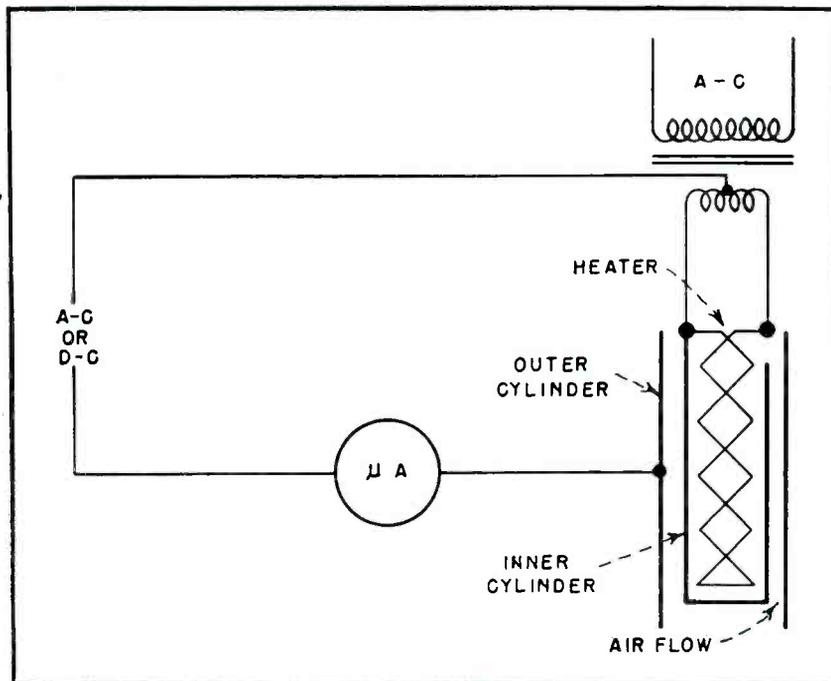
FIG. 1—Basic circuit of the new device
