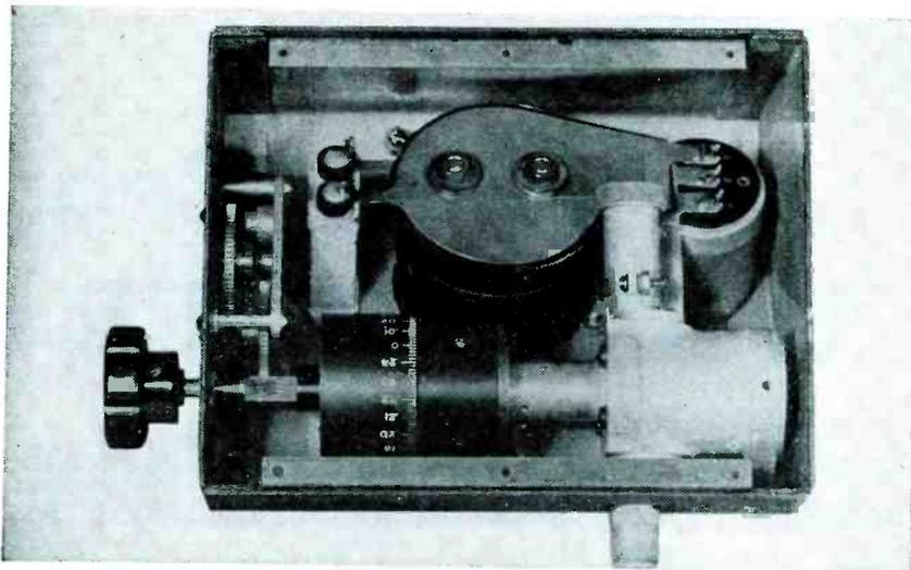
FIG. 4—Field type precision wavemeter. Indicating meter is at upper center
