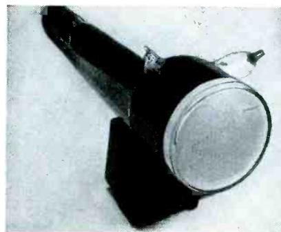
FIG. 4—Dark trace persistence is such that trace remains after tube is unplugged
