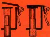
Above sketch shows the action of the Time Delay Tube, which prevents the breaker from opening on sudden inrush current, but allows it to open on sustained overloads. This is done by means of the plunger action in the liquid-filled tube. The speed with which the plunger is drawn toward the magnetized pole piece depends on the viscosity of the liquid. (At left—plunger in normal position. At right—after overload has attracted plunger to pole piece, opening contacts).
