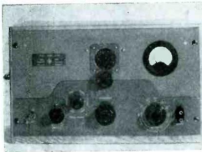
1 db from 10 cycles to 10 mc, and a voltage range of 0.00003 to 3 volts. Output impedance is 600 ohms or 6 ohms with output voltage divider.
