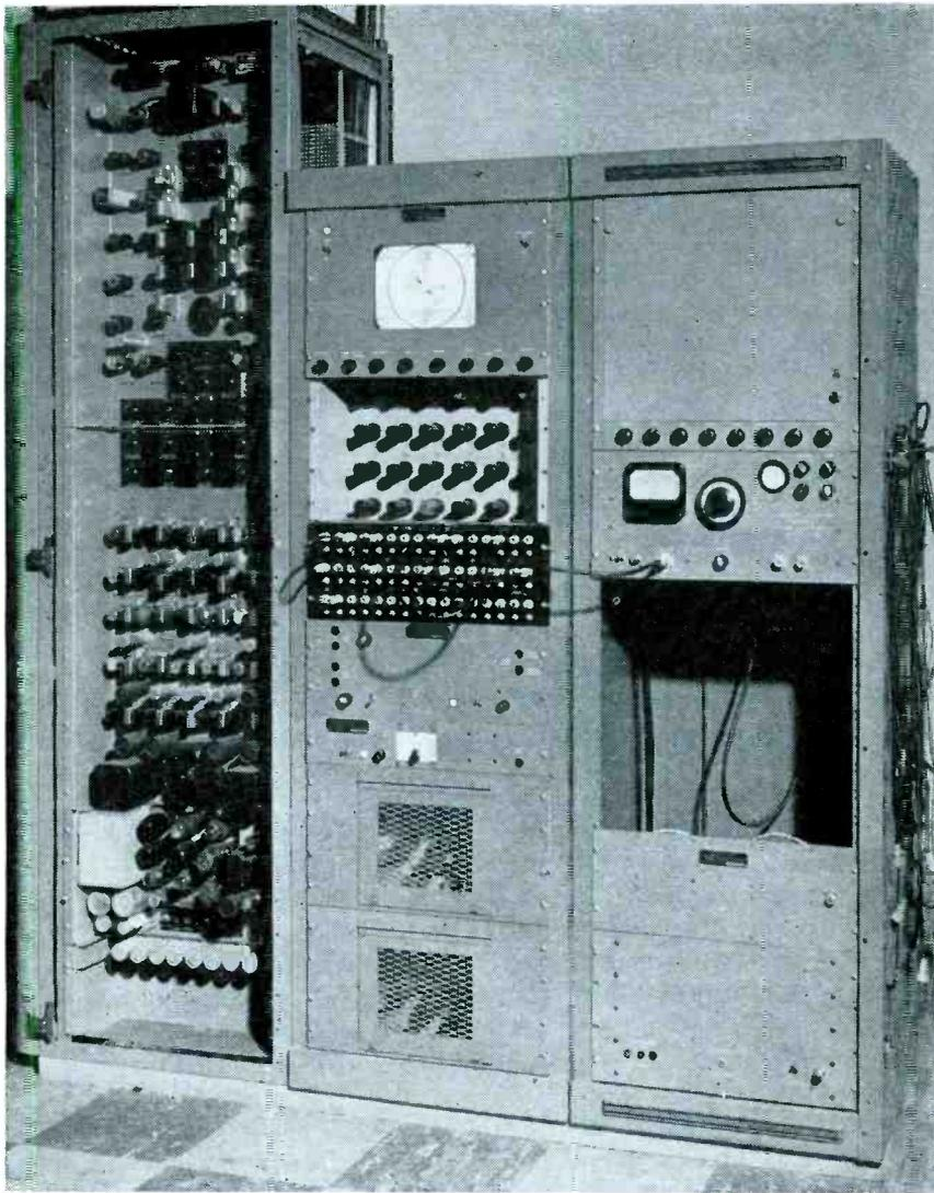
FIG. 2—Central receiver test equipment. The rack at left contains the sync generator. In the center rack are the laboratory picture monitor, distribution and line amplifiers, a linearity test generator, and picture monitor and monoscope camera power supplies. The right-hand rack mounts the monoscope, a transmitter, a noise generator, and line-isolation amplifier power supply
