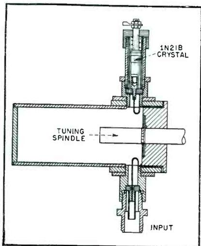
FIG. 2—Cross-section of 5 to 30-cm searching wavemeter
