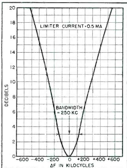
FIG. 3—Bandpass characteristic of the receiver i-f stages
