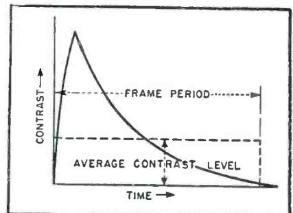
FIG. 1—Density-time characteristic of electron opacity phenomena
