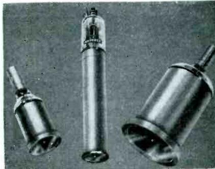
ized production the new series of Geiger tubes includes counter tubes for beta, gamma, and x-rays. Featured herein are direct bonds between mica and metal and mica and glass.
