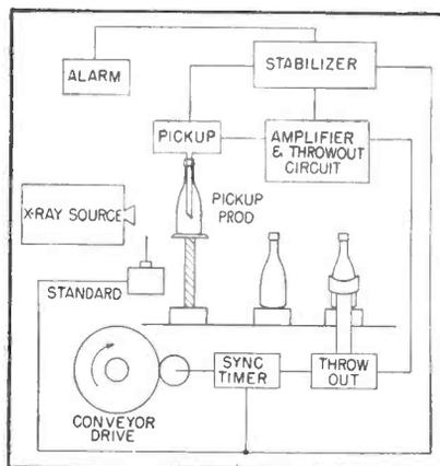
FIG. 2—A method of using the x-ray gage for measuring the thickness of a glass bottle
