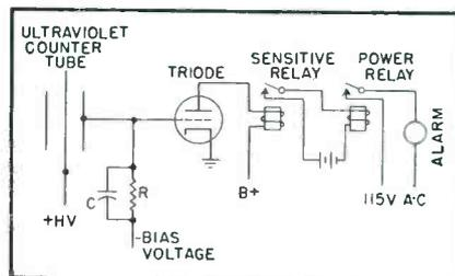
FIG. 2—Simple ultraviolet counter fire-alarm circuit
