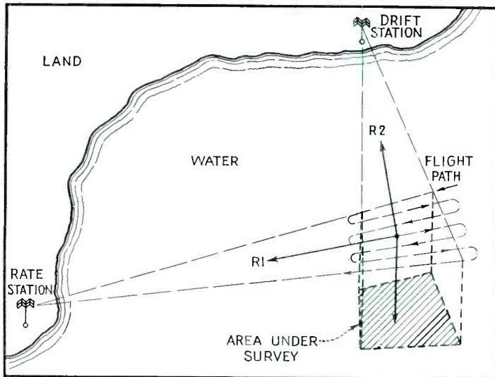
FIG. 1—Use of shoran for aerial photographic surveys. Indicator on aircraft shows airline distance to each ground station, and operator uses this data to determine deviation from desired flight path
