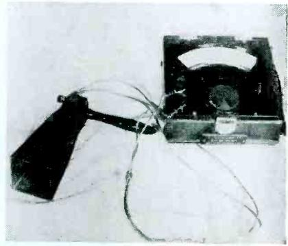
**FIG. 1—Thermopile in horn operates indicating meter**
