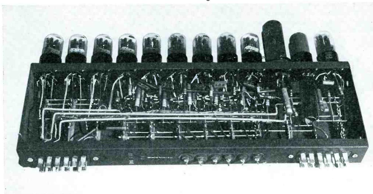
This stepping switch unit incorporates a six-stage counter. Three tubes at right are part of input pulse-forming circuit
