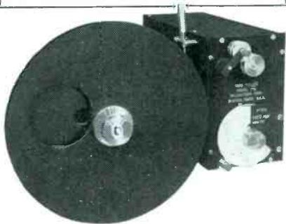
... a precision-built, highly accurate instrument for pulling tape or film at constant, pre-set speeds ranging from 6 to 148 feet per minute. Guaranteed accurate to within  $\pm 1\%$ .
