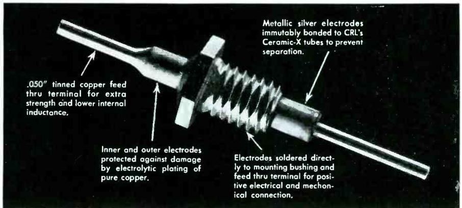
**5** Made with Ceramic-X, CRL's new Feed-thru and Bushing Mounted Capacitors eliminate structural and electrical damage during installation. Two special bonds are reason: 1) between inner feed-thru terminal and inside diameter of tube, and 2) between mounting bushing and outside diameter of tube. Send for bulletin 975.
