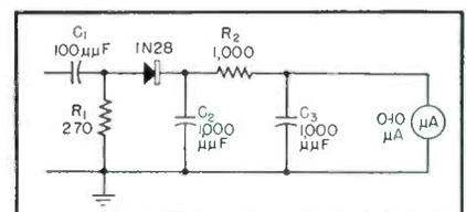
FIG. 1—Circuit diagram of crystal voltmeter
