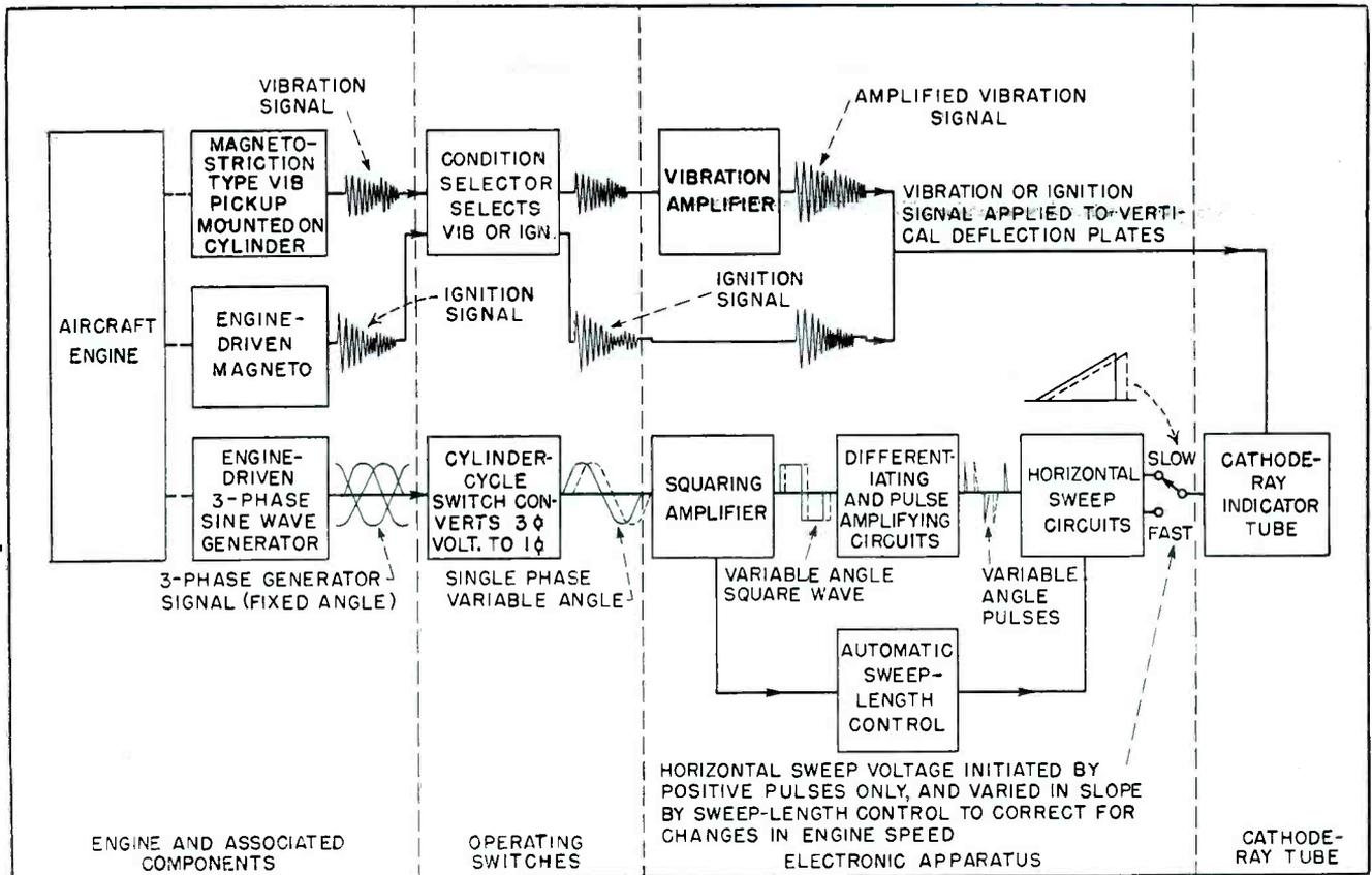
FIG. 2—Block diagram of engine analyzer
