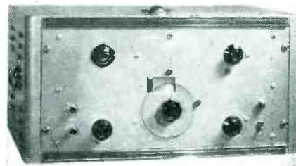
crofarads. Calibration charts allow the measurement of capacitance up to 20,000 micromicrofarads and of inductance up to 10,000 microhenrys.
