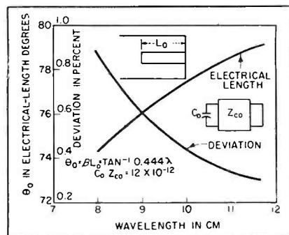
FIG. 7—Electrical length and deviation from the 4-to-1 slope in a finger-contact wavemeter
