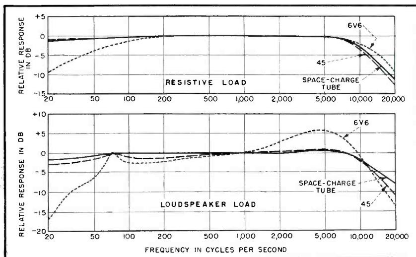
FIG. 3—These frequency response curves were obtained from amplifiers using three types of tubes with both resistive and loudspeaker loads
