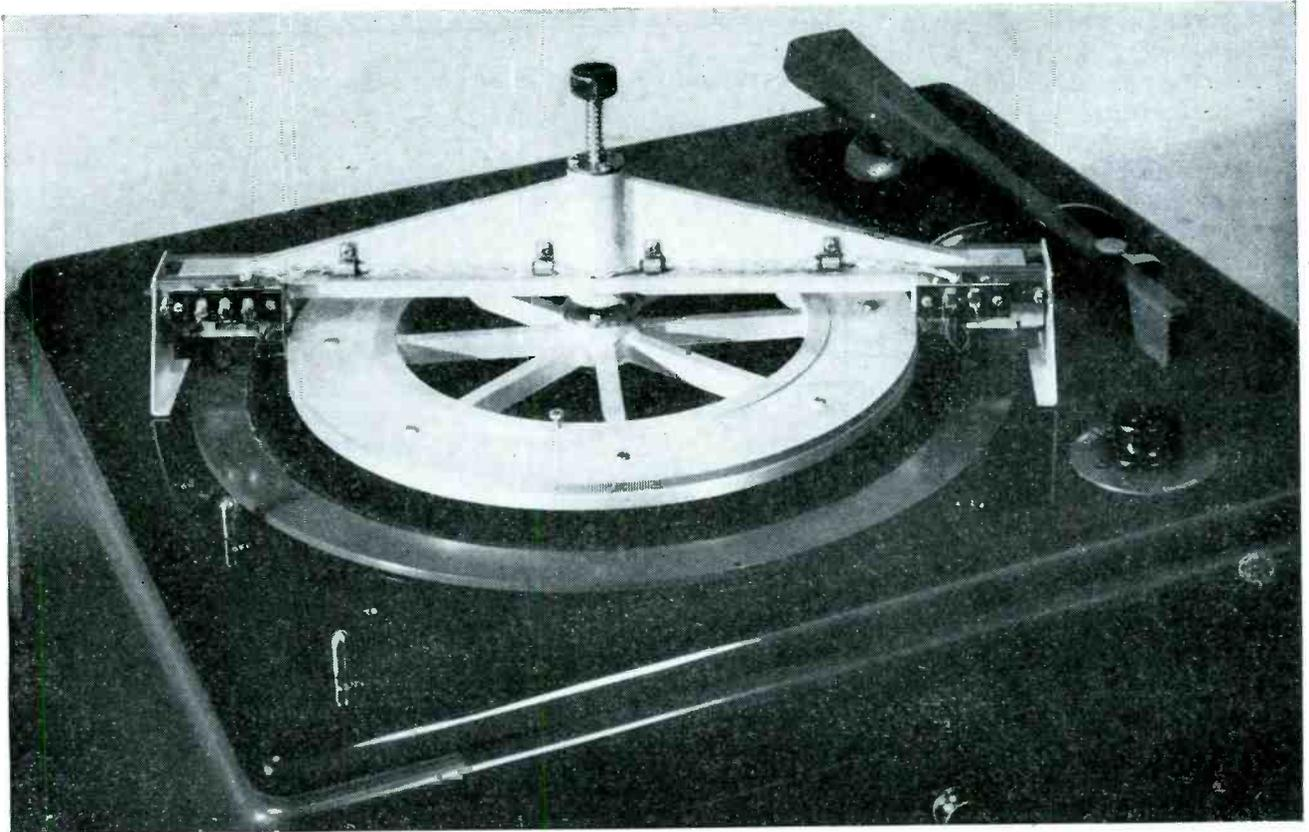
FIG. 1—Toothed-wheel tone generator centered on the turntable
