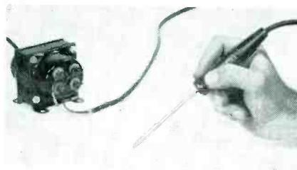
$\frac{1}{8}$  inch in diameter and weighs 1 $\frac{1}{2}$  ounce without the cord. It operates from 6 volts, consuming 25 watts and is illustrated with the step-down transformer used to adapt it to normal socket voltage.
