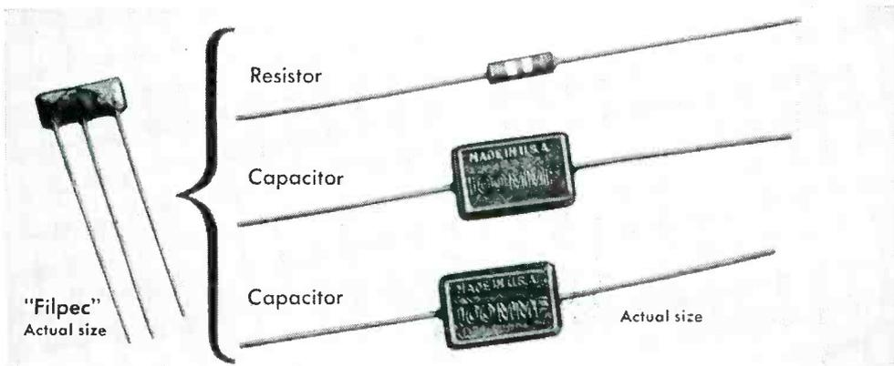
**3** Another application of the "Printed Electronic Circuit" is Centralab's *Filpec*! Designed for use as a balanced diode load filter, *Filpec* combines up to three major components into one tiny filter unit, lighter and smaller than one ordinary capacitor. Available for other applications. Send for Bulletin 976.
