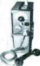
Model BC-322 Transceiver: simple, popular communications unit. Freq. range 52-65 mc. Uses only two tubes, types 33 and 30. Includes a 5 KC crystal in a crystal calibrator circuit. Range 5 to 150 miles, depending upon location and altitude. Operates from single battery block (not supplied) available from mfr., or other sources. Supplied with telescoping antenna and handset, almost new condition.
