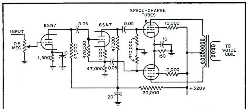
Simplicity and low cost are features of this high-quality space-charge tetrode amplifier
