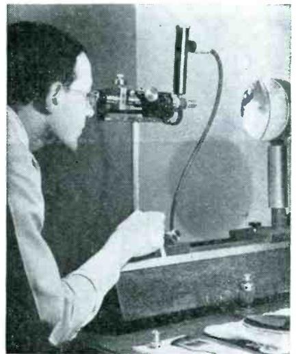
Optical laboratory instrument paves the way for production inspection of television projection mirrors
