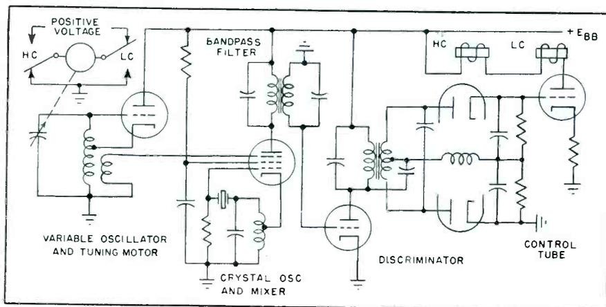
FIG. 3—Frequency stabilization is obtained by beating variable oscillator against crystal oscillator; compare with Fig. 2
