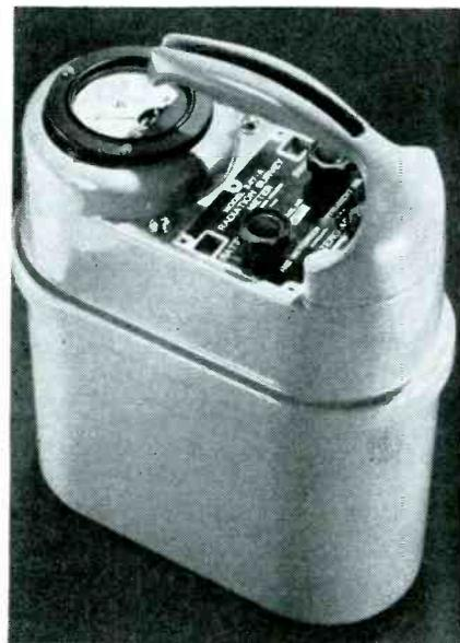
type that is hermetically sealed and watertight. Four ranges of sensitivity are provided to allow full-scale readings of 2.5, 25, 250, and 2,500 milliroentgens per hour. Total weight of the rugged instrument is 11 3/4 pounds.
