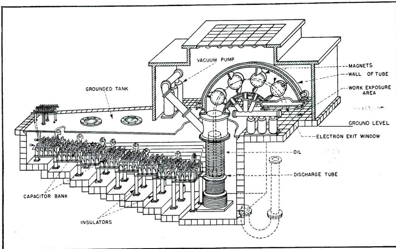
FIG. 3—Prototype of a commercial capacitron
