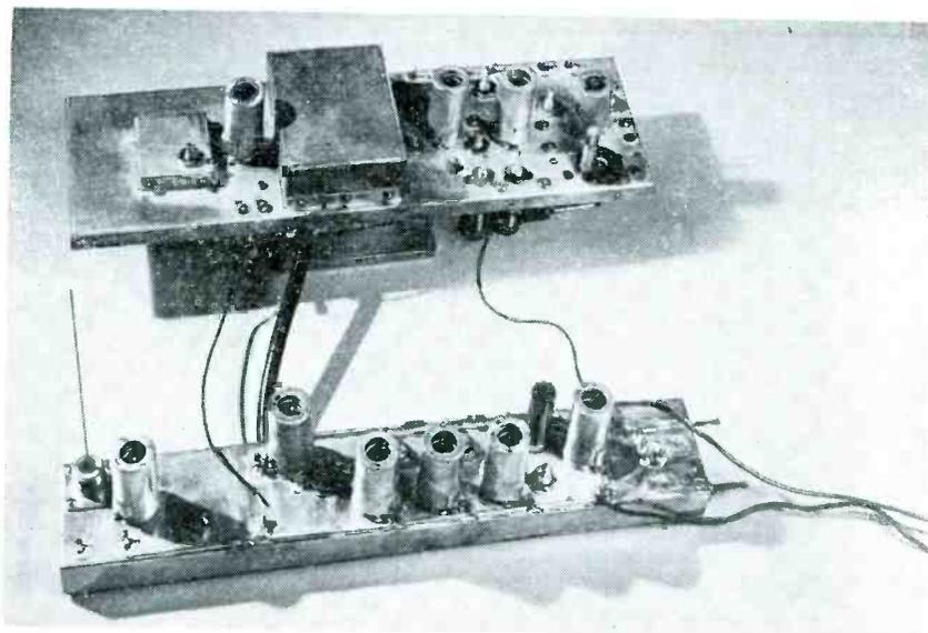
Transmitter and receiver for 465 megacycles. The quarter-wave receiving antenna is at the lower left. Local oscillator power for the receiver (bottom) is taken from the transmitter (top)
