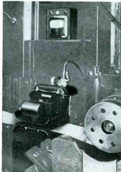
Setup of the x-ray thickness gage for checking copper strip in a cold reduction mill
