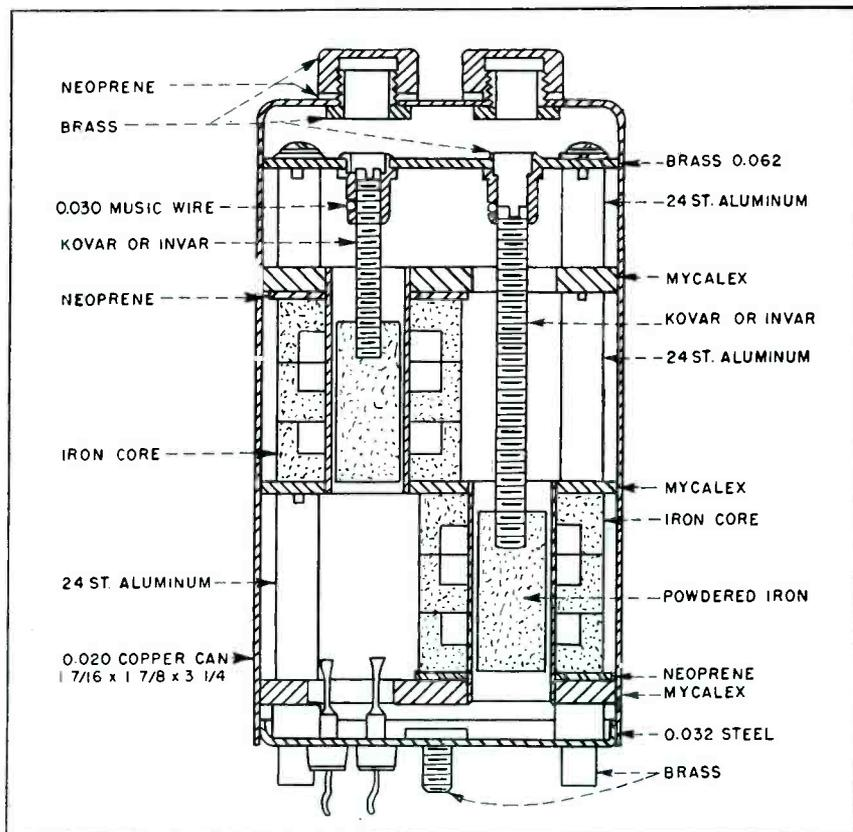
FIG. 4—Discriminator is constructed of compensating materials to insure stability
