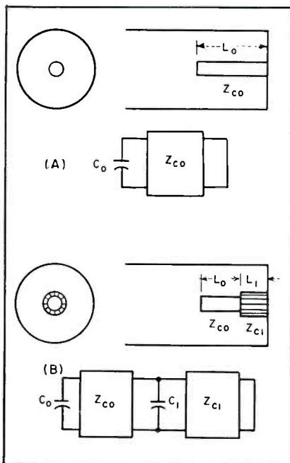
FIG. 6—Cross-section and equivalent circuit (A) of finger-contact type and (B) re-entrant type wavemeter
