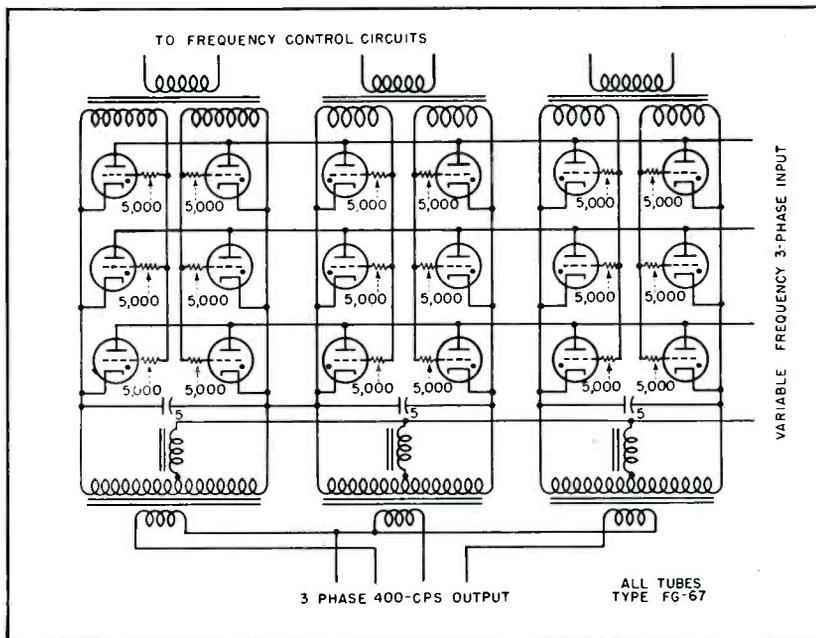
FIG. 2—Three-phase parallel-inverter shown here consists of three interconnected single-phase units with phase sequence determined by circuit of Fig. 4. Losses in transformers and chokes make this circuit less efficient than cycloconverter
