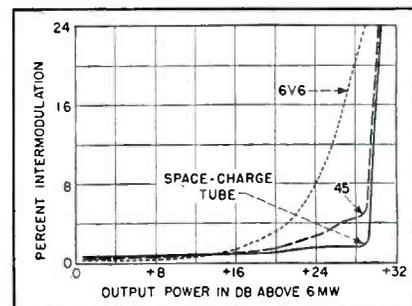
FIG. 4—Intermodulation distortion as a function of power output is shown for three amplifiers
