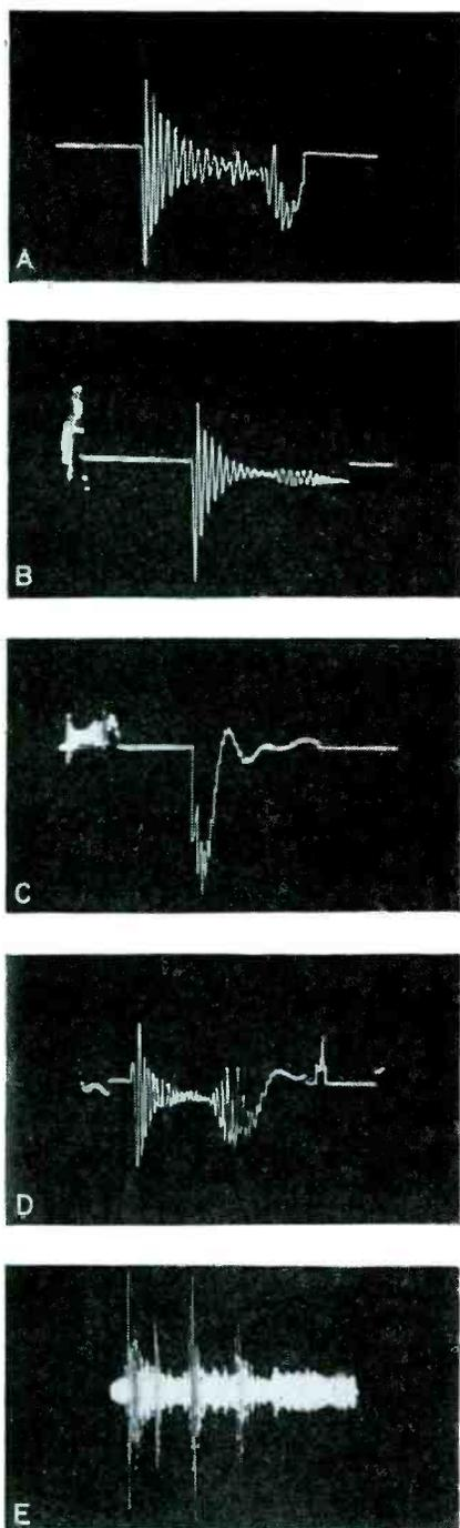
FIG. 4—Typical ignition patterns for (A) normal conditions, (B) fouled plug, (C) open secondary, (D) magneto breaker-point bounce, and (E) vibration pattern of a normal cylinder
