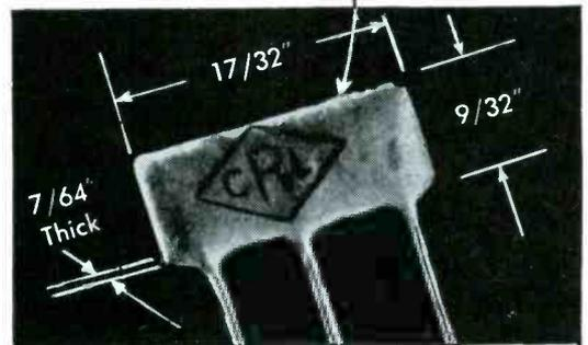
"Filpec" gives you integral construction! Made with high dielectric Ceramic-X, CRL's *Filpec* assures long life, low internal inductance, resistance to humidity and vibration. Note schematic diagram below, showing typical application.
