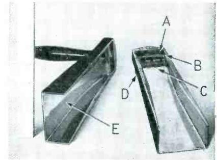
FIG. 2—Open horn shows internal shape and location of thermal junctions. There are 19 cold junctions (A) and 19 hot ones (C), the latter being blackened and located along the focus of the horn. The Thermopile is insulated (B) from the polished aluminum horn (E) and leads brought out to terminal posts (D). The equipment is available through Central Scientific Co., Chicago
