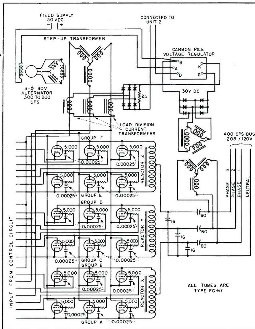
FIG. 1—In the cycloconverter, each phase of the step-up transformer secondary supplies voltage to three pairs of thyristors. Output frequency is held at 400 cycles by auxiliary control circuit that determines thyristor firing sequence
