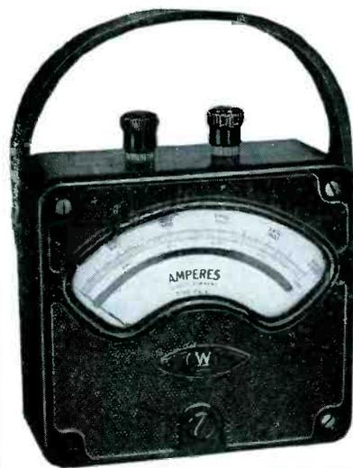
Westinghouse Type PX-4, accuracy within 1/2% of 1%; 3 1/2" long mirror scale with 100 scale divisions; Knife edge pointer; Moving coil D'Arsonval movement. Dimensions 4 1/2" x 4 1/2" x 2" @ . . . . . **\$17.50**
