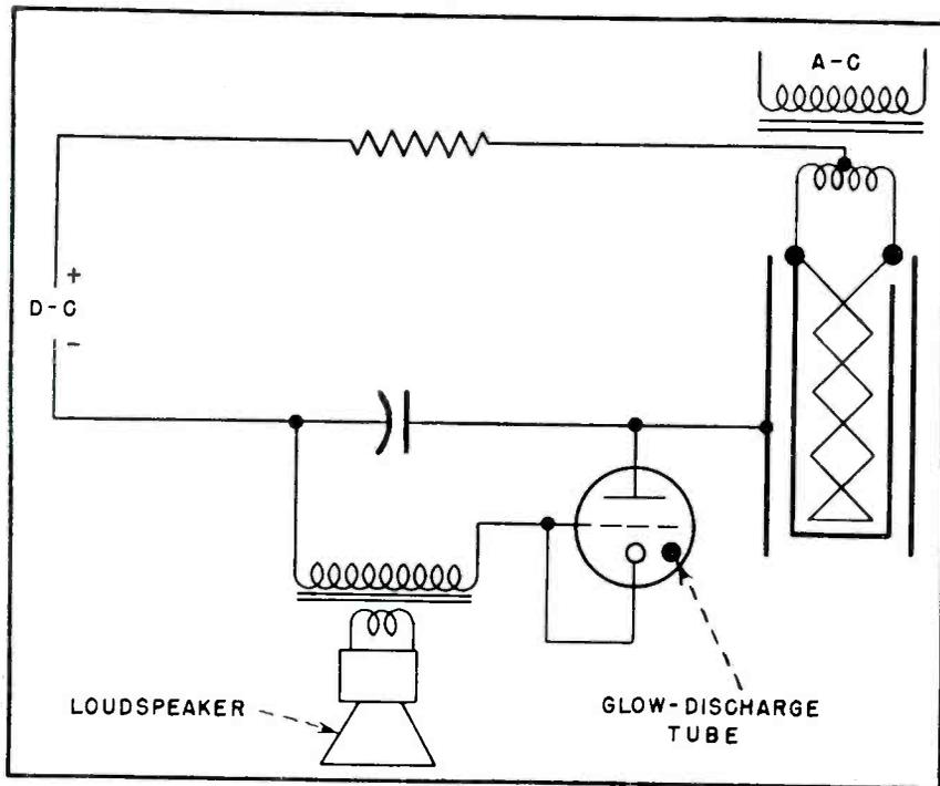
FIG. 2—Method of producing an audible response when the leak detector encounters halogen vapor compounds, or solid particles containing them, in the air
