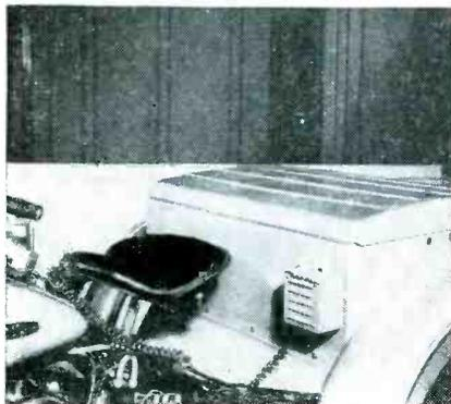
patcher unit is a compact mobile radiotelephone transmitter and receiver for motorcycle use with a power output of 7 to 10 watts. The crystal drift is held to less than  $\pm 0.002$  percent over a temperature range of  $-20$  to  $+80$ C.
