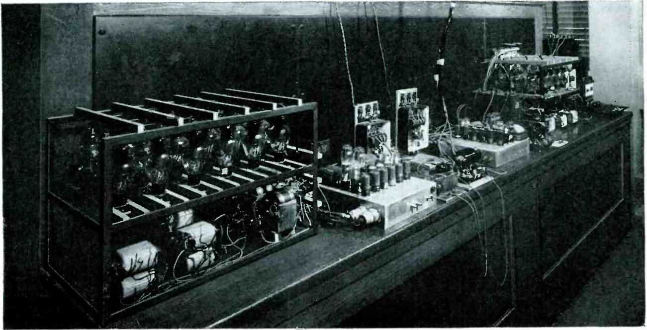
Frequency-changer power circuits include parallel-inverter type, left, and cycloconverter, extreme right. Frequency and phase control units are in the center. Connections between control circuits synchronize the two systems to permit parallel operation
