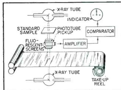
FIG. 1—Simplified schematic showing arrangement of units so that two x-ray beams strike the phototube pickup for comparison
