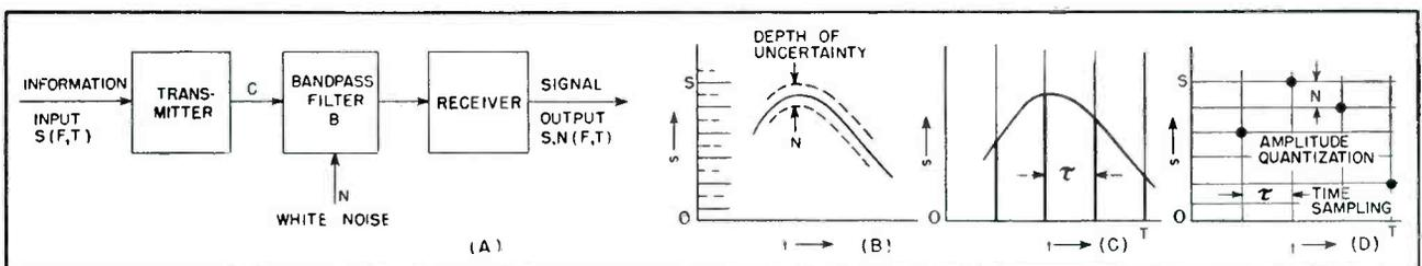
FIG. 1—Basic elements of simple communication system indicate that transmission can be by two-dimensional points
