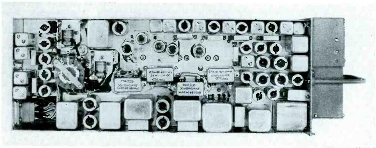
Omnidirectional range and communications receiver has the frequency monitoring circuit described in this article at the left of the chassis. The r-f and i-f circuits occupy the upper center and right, navigation circuits extend along the lower side of the chassis. Two crystal ovens are in cans on the underside of the chassis
