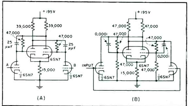
FIG. 2—Flip-flop (A) and scale-of-two (B) circuits used in ENIAC. Negative pulses are used to trip the flip-flop circuit; positive pulses trigger triodes which deliver negative pulses to plates of scale-of-two counter. This example illustrates the fact that trigger pulses of suitable shape can be applied to points other than the grids
