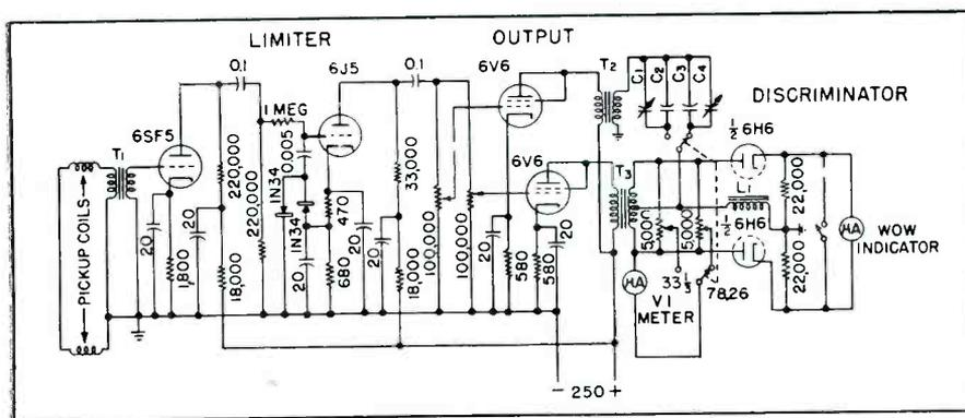
FIG. 3—Schematic circuit diagram of the wow meter. Shorting switch across the indicating meter prevents damage when turntable is started
