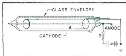
FIG. 1—Construction of basic Geiger-Muller counter tube. To sensitize tube to ultraviolet, surface of copper cathode is slightly oxidized and tube is filled with mixture of argon and alcohol vapor at low pressure. Quartz window in the glass envelope admits ultraviolet radiation
