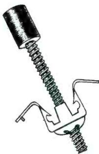
1. Provides required tension on iron core adjusting screw to maintain accurate setting, thru use of specially designed "Palnut" thread form.
