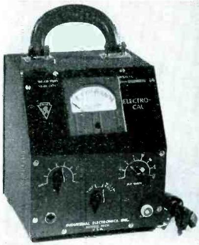
viding precision measured signal voltage for calibration purposes. Output signals in the form of 60-cycle sine waves up to 1,000 millivolts are available in eight ranges. An output signal of 0-5 volts can also be read directly on the meter.
