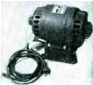
Mfd. By ESCO, Type R182, for marine use. Converts 115 V. DC to 115V. AC, very conservatively rated at 135 watts. Tests show that it is satisfactory for service up to 200 watts. Self-ventilated, semi-enclosed, wool-oiled bearing construction. Includes filter condensers and choke coils in base, as well as small condensers across each brushholder for filtering purposes. Provided with rubber connecting cords, and standard outlet receptacle.
