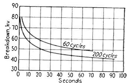
Figure 2: Effects of frequency and time. Press-board in oil at 25° C. (S. Whitehead)
