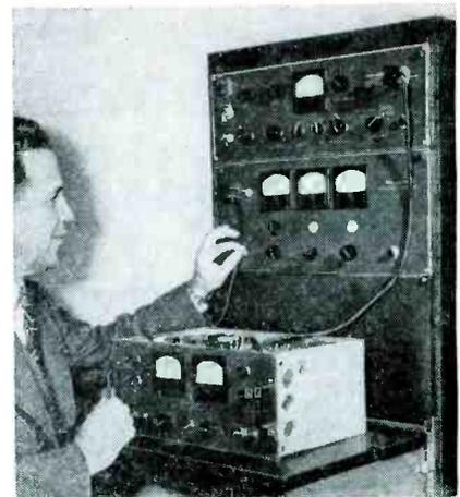
The signal generator and analyzer mounted on the rack form the two units of the Western Electric intermodulation test set for measuring audio-frequency distortion caused by intermodulation
