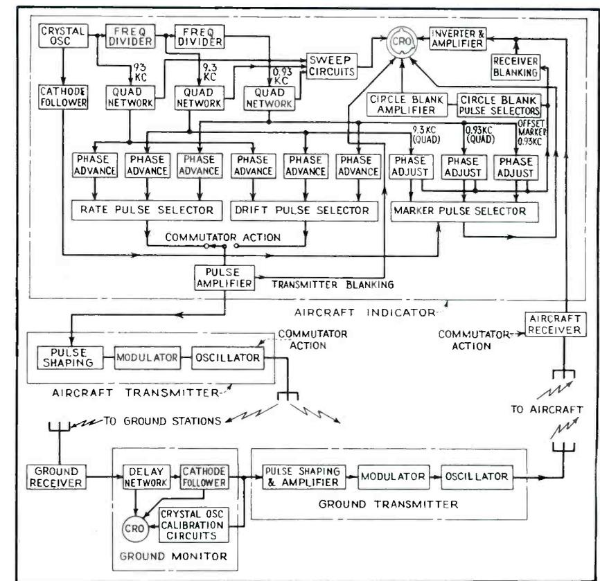
FIG. 2—Simplified block diagram of shoran system as used for aerial surveying
