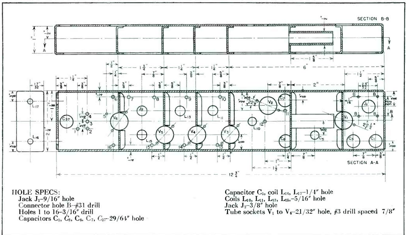
FIG. 6—Mechanical details of receiver chassis, including those of shield partitions. Section A-A at the right is the plate resonator of the r-f preamplifier stage
