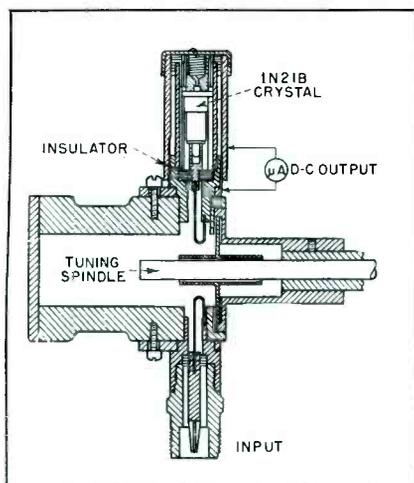
FIG. 5—Cross-section of re-entrant transmission line short circuit type
