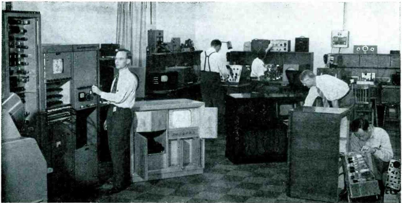
FIG. 1—In this view of the laboratory, the central test equipment racks illustrated in Fig. 2 appear at left. The line-isolation amplifiers are mounted on the walls
