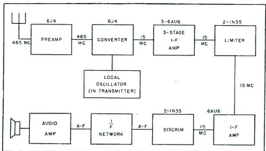
FIG. 1—Block diagram of the receiver. Power supply and a-f circuits are separate from the chassis illustrated in the accompanying photographs
