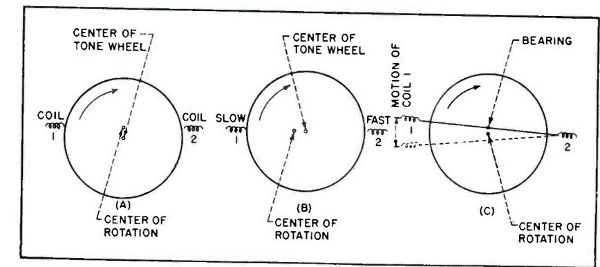
FIG. 2—Effect of wow on a single pickup coil (A and B) and upon a pair bearing on the center of the tone wheel (C)
