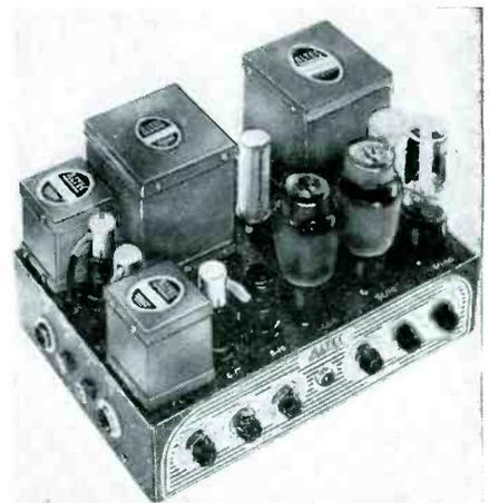
flat within 1 db from 20 to 20,000 cycles. Four inputs are provided, two low impedance with 95-db gain and the other two with 72-db gain at high impedance. Variable controls are available for both bass and treble.
