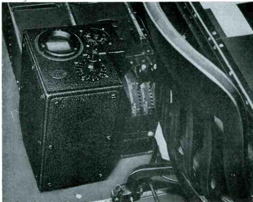
Engine analyzer installed in plane at rear of pilot's seat near flight engineer's desk
