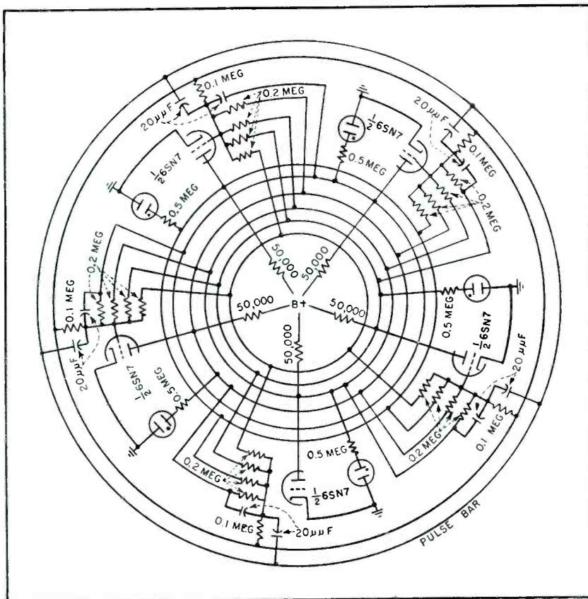
FIG. 3—Lewis five-stage ring counter. Successive pulses fed to pulse bar step the counter through five states; on sixth pulse the counter recycles
