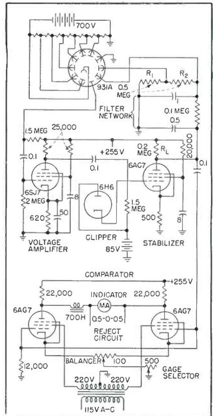
FIG. 3—Values of components and stages of the gaging circuit. The 6AC7 stabilizes the 931A photomultiplier
