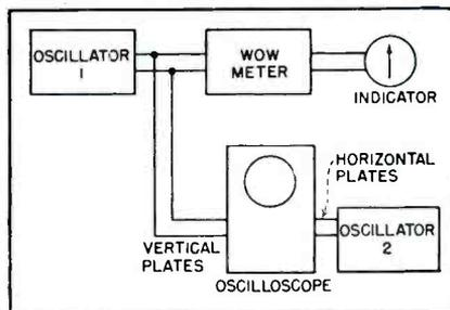
FIG. 4—Method of calibrating the meter by Lissajous figures
