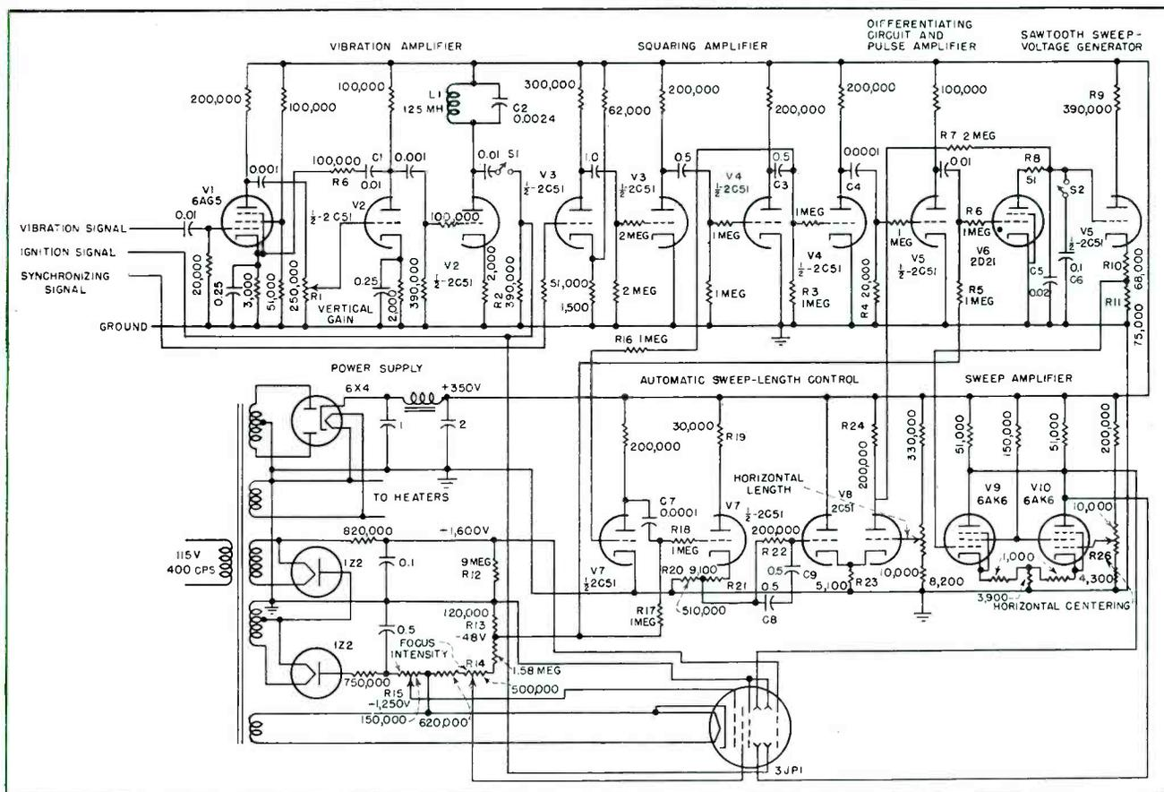
FIG. 3—Diagram of engine analyzer circuits. Value of capacitor C<sub>1</sub> is varied for different engines
