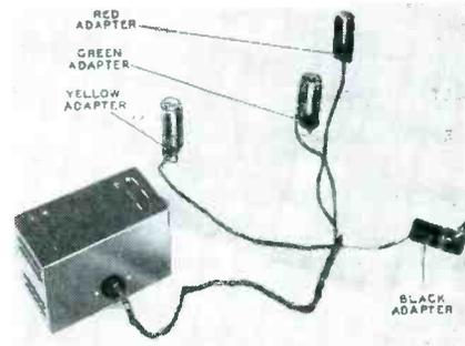
to check and adjust the linearity of a receiver's vertical and horizontal sweeps without depending on test charts from a television station. By means of an adapter harness the unit obtains required plate power, filament power and synchronizing voltages from the receiver itself.
