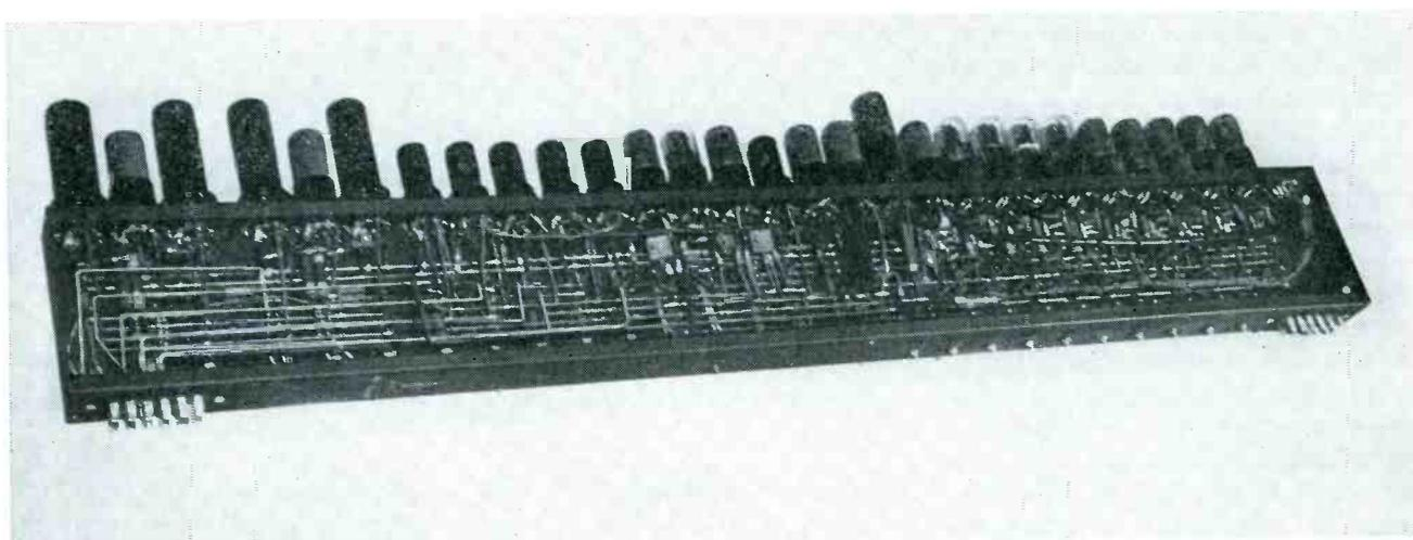
Ten stages at right form counter in this plug-in decade unit; other circuits are for carryover and transmission of count
