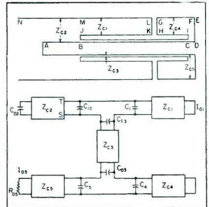
**FIG. 9—Equivalent circuit for re-entrant type wavemeter**
