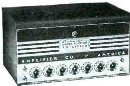
variable reluctance magnetic pickup without additional pre-amplification or equalized circuits, the model ACA-100GE direct-coupled amplifier develops 23 watts with less than one percent total distortion.
