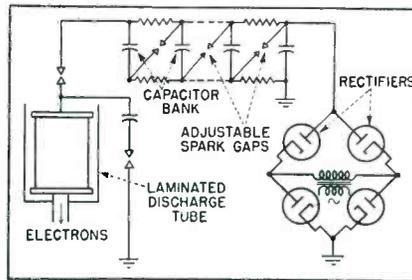
FIG. 1—Basic circuit of the electronic impulse generator
