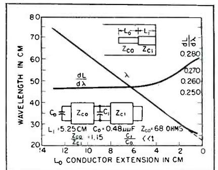
FIG. 8—Resonant wavelength versus conductor extension and slope for a re-entrant type wavemeter
