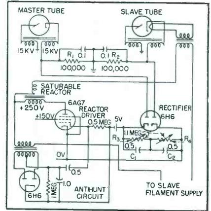
FIG. 4—In the x-ray tube stabilizer, the anode current of the master tube controls the filament current of the slave tube
