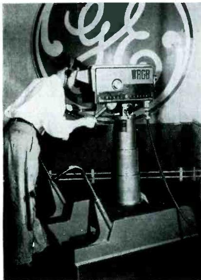
is mounted on a mobile dolly and may be operated with fingertip control. Acceptable pictures can be obtained at 50 foot-candles and f/3.5.
