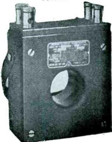
Weston Model 461 Type 4 (see illustration). This unit can be used with any precision 5 Amperes A.C. Meter to extend the ranges of the meter to 50, 100, 200, 250, 500 or 1000 Amperes A.C. Accuracy within 1/2% of 1%; Normal Secondary Capacity = 15 Va; Binding Posts for 50 Amperes tap; Inserted primary for 100, 200, 250, 500 and 1000 Amperes; insulated for use up to 2500 volts. List Price \$88.00. . . . . **NET fob, NY \$35.00**
