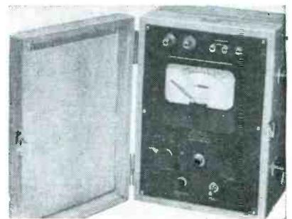
tribution of this direct-reading megohmmeter gives the same accuracy over the whole range of 1 to 100,000 megohms, covered by six decade steps. Range can also be extended to 1,000,000 megohms.
