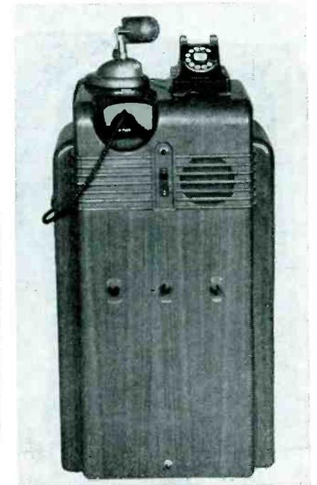
Jordaphone, a device which permits group telephone conversations without individual headsets. It consists of a regulation telephone, console cabinet and microphone. Impulses in the receiver are picked up by a coil in the console and amplified. In transmitting, the talker's voice is heard without amplification. A built-in receptacle cuts out all outside noises from both ends of the handset.
