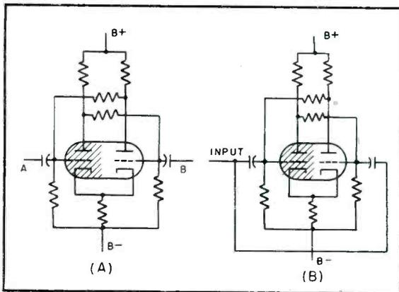
FIG. 1—Flip-flop circuit (A) is tripped by a negative pulse at input A and is reset by negative pulse at input B. Basic scale-of-two circuit (B) has two operating states, alternating from one to the other as successive negative pulses are fed to input
