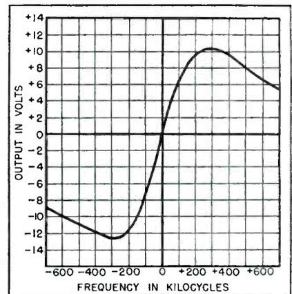
FIG. 5—Discriminator characteristic when limiter current is 0.5 milliampere
