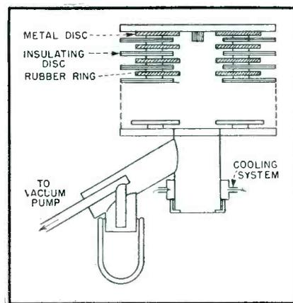
FIG. 2—Laminated discharge tube used in the system
