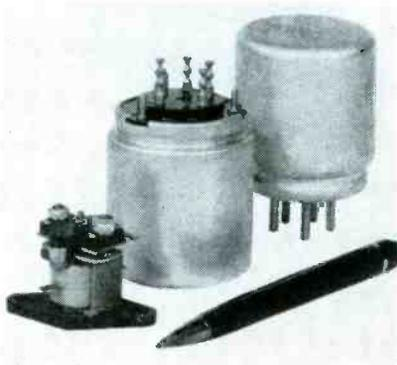
tive, d-c relays are announced. Input ratings range from 10 to 180 milliwatts, 0.47 to 1,470 milliamps, and 0.07 to 67,000 ohms. Additional information is given in GEA-3819D.
