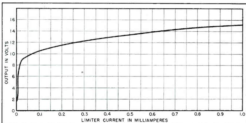
FIG. 4—Output voltage across  $R_2$  in the discriminator load circuit (Fig. 2) plotted against limiter current
