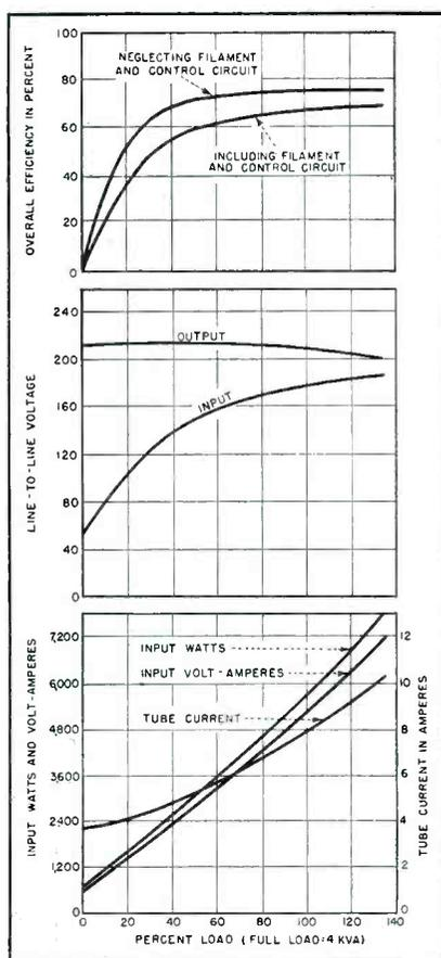
FIG. 3—Performance curves for cycloconverter power circuit
