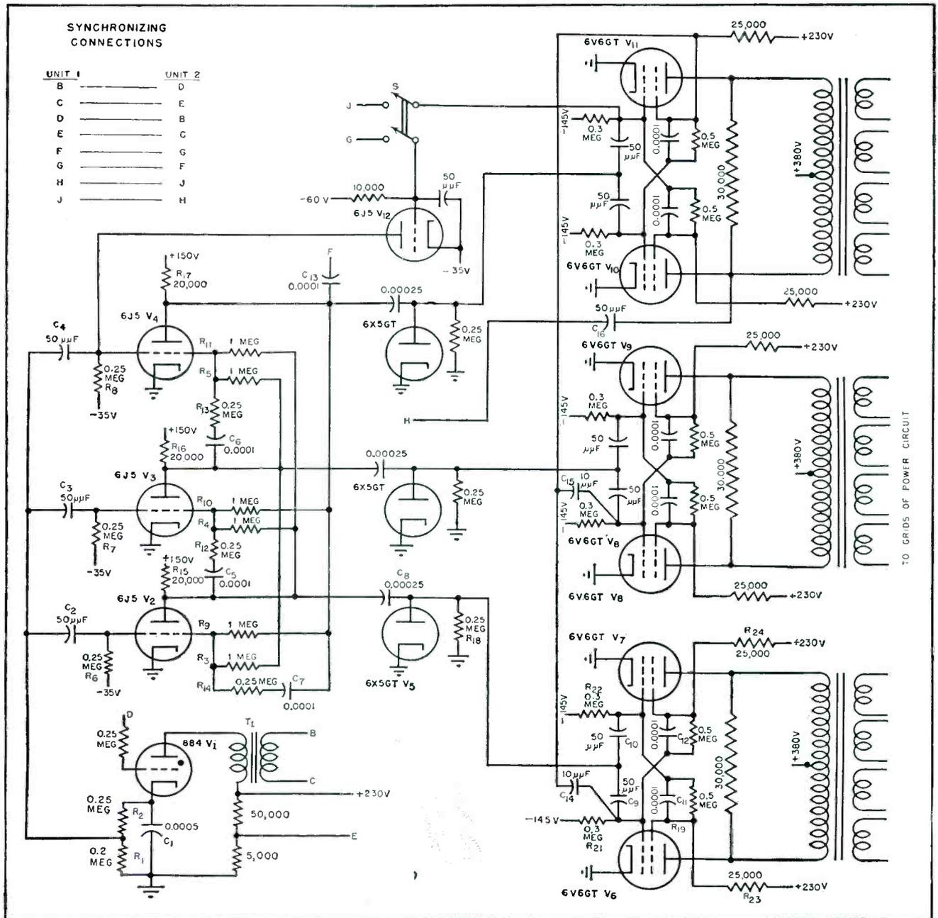
FIG. 4—In the control circuit, a 2,400-cycle relaxation oscillator drives a ring-of-three counter that develops three 800-cycle square-wave output voltages having 120-degree phase relationship. Each of these voltages drives a flip-flop circuit coupled to the thyatron
