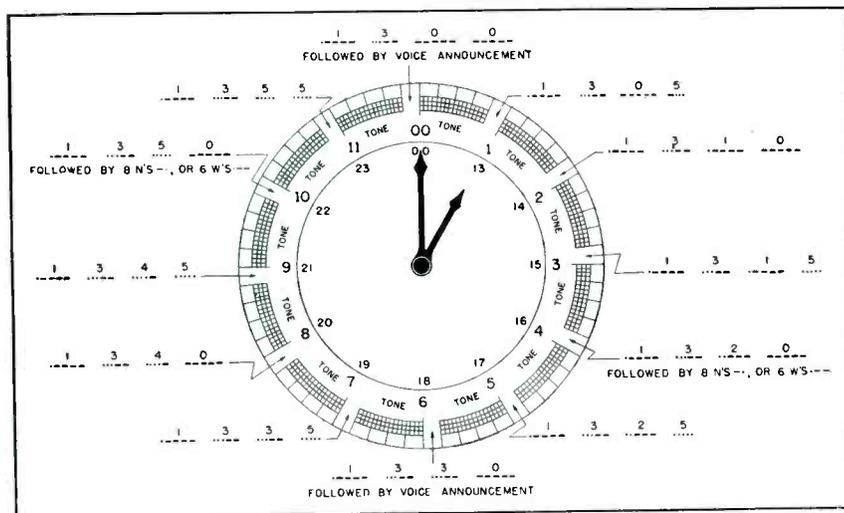
Example illustrating new schedule of time announcements by station WWV. Hour illustrated is 1 to 2 p. m., or 1300 to 1400 in 24-hour time for Eastern Standard Time
