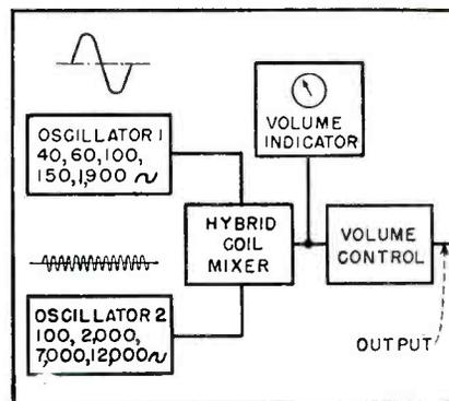
Essential stages of the system for measuring intermodulation distortion
