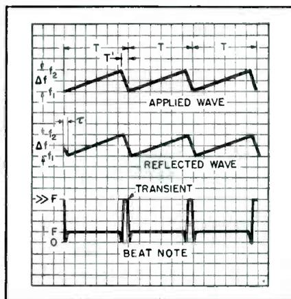
FIG. 3—Frequency vs time relationships existing at the beat-note detector
