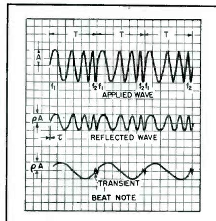
FIG. 4—Amplitude vs time relationships existing at the beat-note detector
