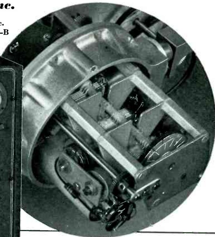
Shown above is an interior view of the 202-B Signal Generator RF assembly with shield cover removed. Heavy aluminum castings form the mounting base of this RF unit resulting in a compact and highly rigid structure. Girder type condenser frame construction, multiple rotor shaft grounding contacts, and welded interstage shield plates are but a few of the many design features of this unit which give added circuit stability.
