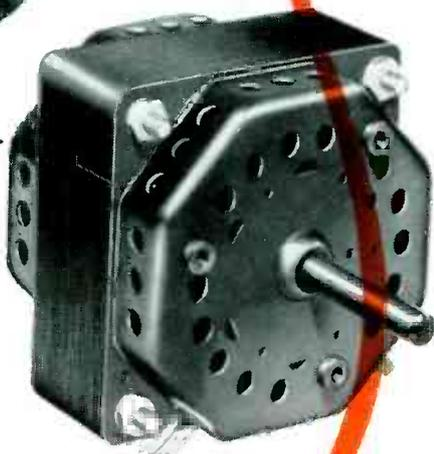
**MODEL B**—New type 4-pole shaded pole fan motor made in three standard lamination stack thicknesses. Power range is from 1/100th h.p. to 1/25th h.p. Size,  $3\frac{3}{8}$ " square. Especially adapted for fans, it will drive a wide variety of mechanical devices and is ideal for sound recorders. Full load speed 1550 R.P.M.—clockwise or counter clockwise rotation—not reversible. Made for 115 volts, 60 cycles—can be wound for 50 cycles and for other voltages.
