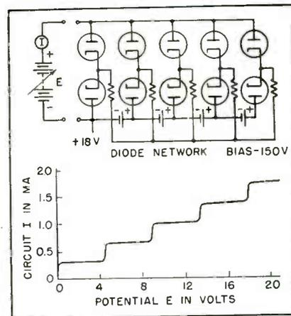
FIG. 1—Basic diode stepping circuit
