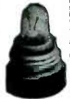
Photograph 3 times actual size. Soldering Iron removes lamp from base
