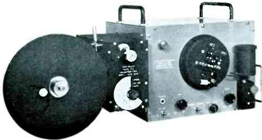
The model MA-126 series recorder represents a complete, self-contained high speed ink tape recording system. The Mecanitron recording head represents a new departure in moving coil design. A lightweight, rugged coil of eight ohms impedance is driven by a special polar, pulse amplifier.
