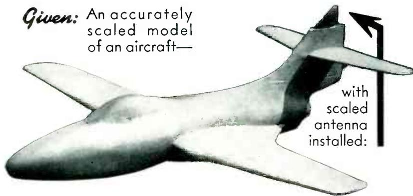
**Find:** The radiation pattern of that antenna on that aircraft in any plane and for either vertical or horizontal polarization.
