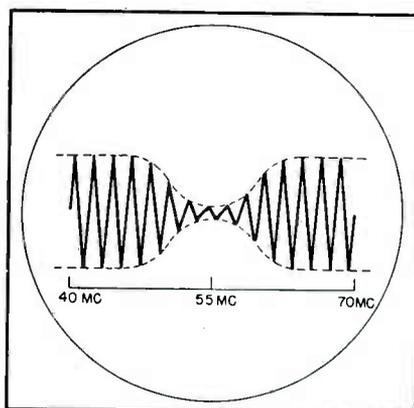
FIG. 6—Typical visual presentation of reflected energy on an oscilloscope screen
