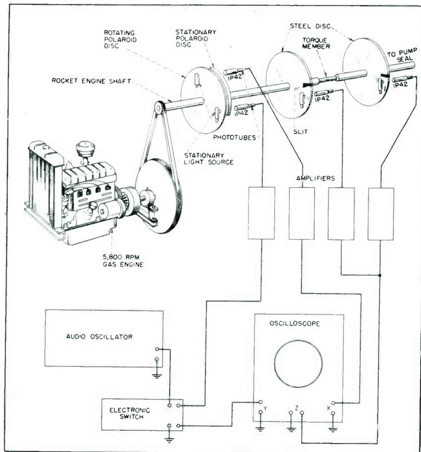
Block diagram of the rocket-engine pump-seal tester
