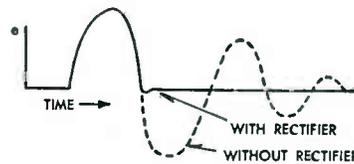
Unit damps out the oscillation after one-half cycle, producing a single pulse shaped similarly to half of a sine wave. This pulse may be clipped, provided clipper is isolated from pulse-producing tuned circuit to prevent damping out desired half cycle.
