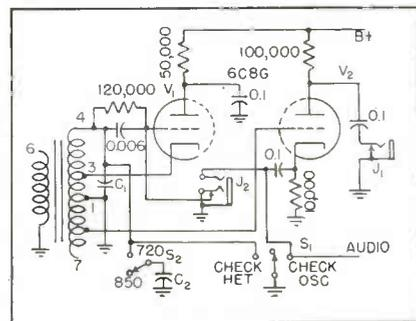
FIG. 2—Audio oscillator and mixer circuit. The center position of switch  $S_1$  is the normal position
