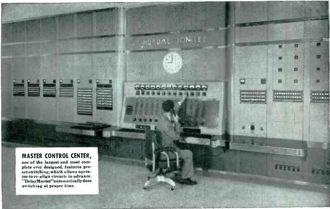
**MASTER CONTROL CENTER,** one of the largest and most complete ever designed, features pre-set switching, which allows operator to re-align circuits in advance. "DelayMaster" automatically does switching at proper time.
