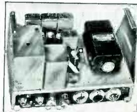
High frequency 160,000 kilocycle FM two-way Motorola radiotelephone equipment permits 100% radio coverage regardless of electrical interferences or steel enclosing structure. Sylvania Lock-Ins handle very high frequencies with ease. Have short, direct connections, fewer welded joints . . . no soldered joints—less loss; getter located on top; shorts eliminated by separation of getter material from leads! Cannot be dislodged from sockets no matter how rough the way.
