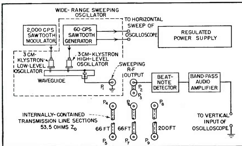
FIG. 5—Block diagram of the frequency-scanning vhf impedance meter showing lengths of transmission line available within the instrument
