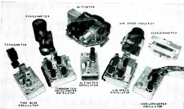
*Typical set of sensing instruments and oscillators for building into the magnetic recorder equipment. Sensing instruments can be designed and manufactured to order or standard elements can be adapted to individual requirements.*
