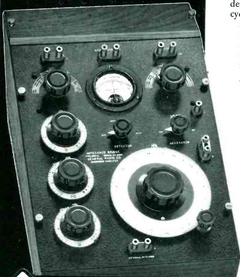
**C**OMPLETELY self-contained, portable and always set-up for immediate use, this impedance bridge is indispensable in any laboratory where electrical equipment is used. No hastily putting together a circuit, finding an oscillator and a detector and then a power supply . . . they are all here permanently assembled in an accurate instrument . . . always ready to use at any time.
