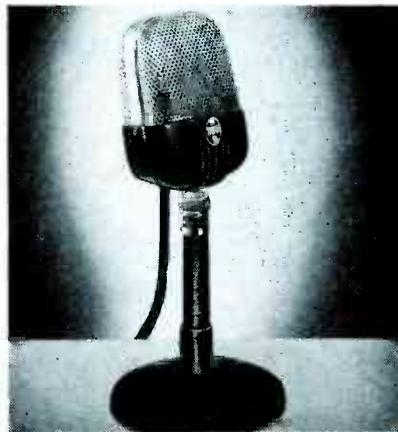
supported in an Alnico V magnet. Response is within plus or minus 5 db from 80 to 10,000 cycles. Level is 62 db below 1 volt per dyne per square centimeter at high impedance. A switch allows use into 50, 200, or 500 ohms.
