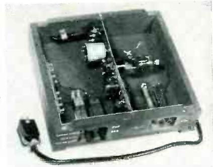
Constructed in this fashion, the carrier shift check meter fits under a BC-221 frequency meter
