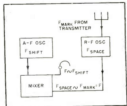
FIG. 1—Essential stages of a system for checking carrier shift
