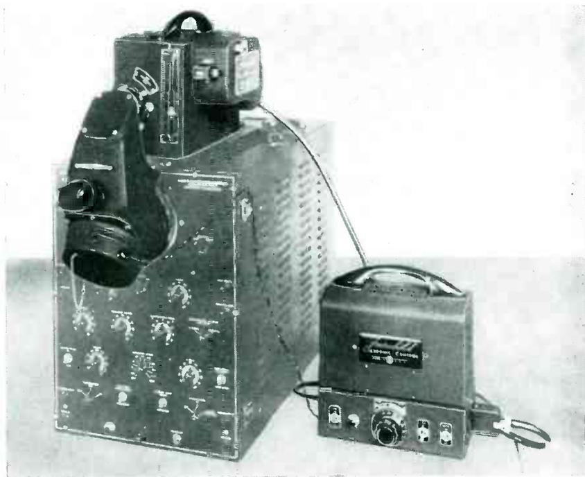
Camera mounted on oscilloscope, and electronic film-speed control unit
