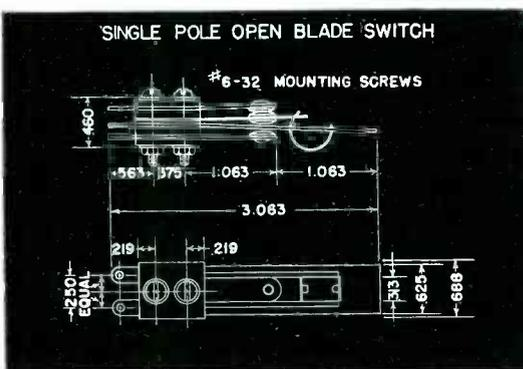
The larger single pole Open Blade Switch shown here, carries the same ratings as the small switch, but is of more rugged construction. Built with extra large contacts to assure extraordinary long life on applications where the continuous load is close to the rated load. Also built with the exclusive ACRO Rolling Spring principle for positive action and long, trouble-free life. Available with terminals at rear only, as illustrated.
