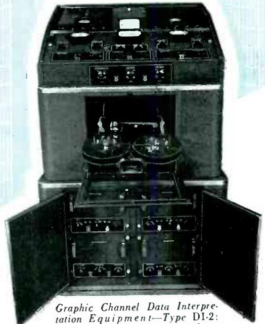
*Graphic Channel Data Interpretation Equipment—Type DI-2: showing front compartment doors open for tape loading and adjustment. Unit provides 1 time base and 2 information channels.*
