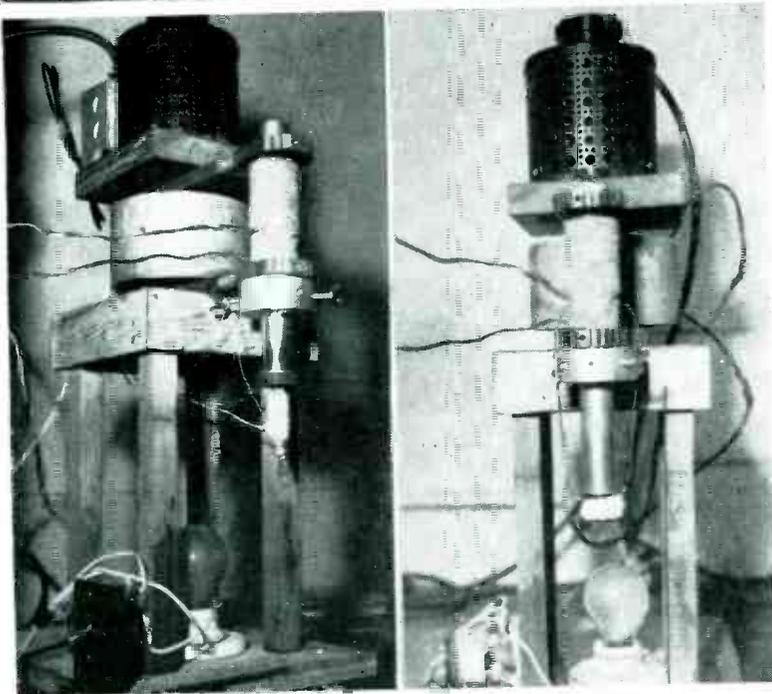
FIG. 2—Magnetostriction transducer with solid tinning tip and (right) with brush-type tip
