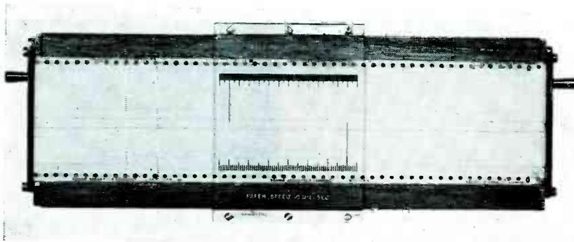
FIG. 7—Shot arrival time evaluator for two different recorder speeds. The long vertical line is placed over the maximum signal and tenths of seconds read off to the nearest chronometer time mark
