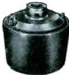
*Right*—NEW SPECIAL PM HORN UNIT, having Almico V magnet ring completely watertight, housed in a heavy aluminum spinning. Provides extremely high efficiency reproduction with minimum input. Handling capacity 35 watts continuous, 60 w. peak.
