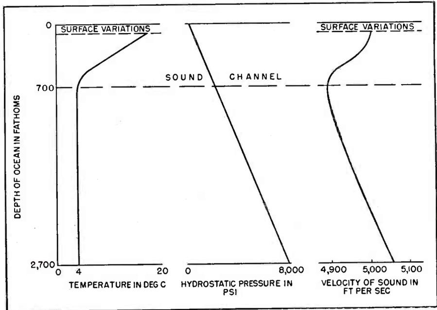
FIG. 1—Graphic explanation of the sound channel effect upon which the sofar system depends
