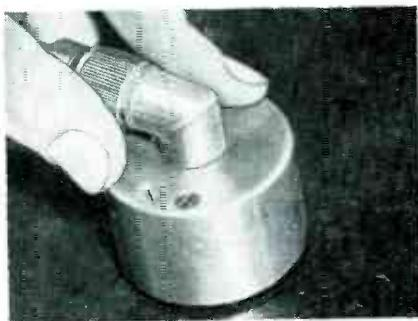
is used with the Supersonic Reflectoscope to inspect welds. The weld itself will not constitute a reflecting interface, but any voids or inclusions will reflect a part of the energy.
