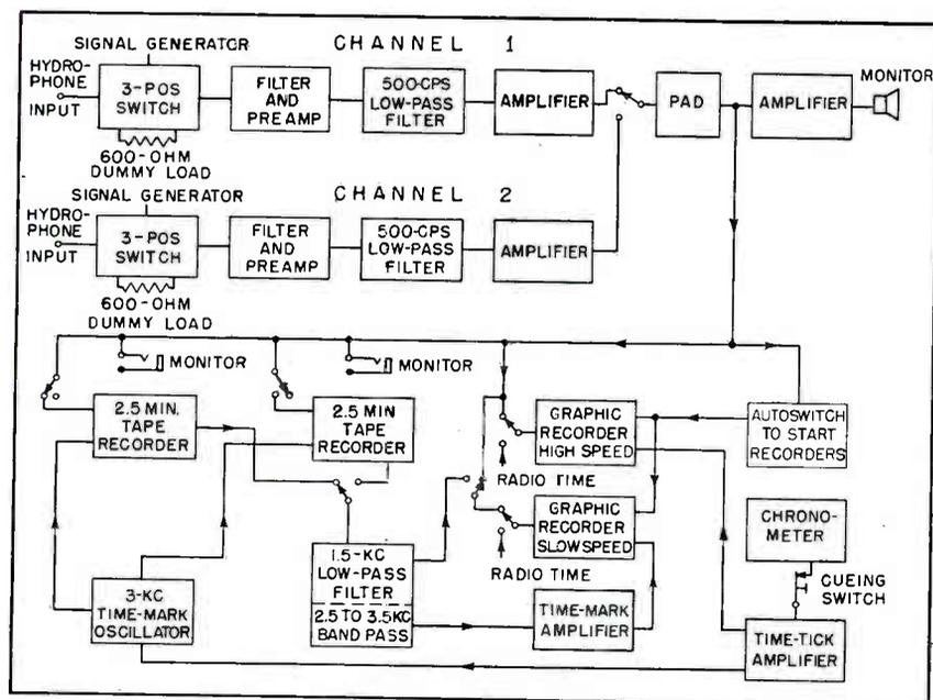
FIG. 3—Simplified block diagram of more important elements making up a complete monitoring station
