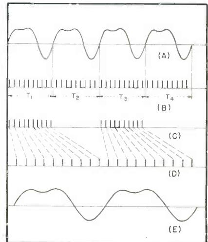
FIG. 1—Basic wave-expanding technique
