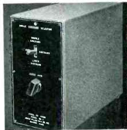
band reception on all signals rather than only to those with suppressed carrier. The unit is readily connected to any standard communications receiver.
