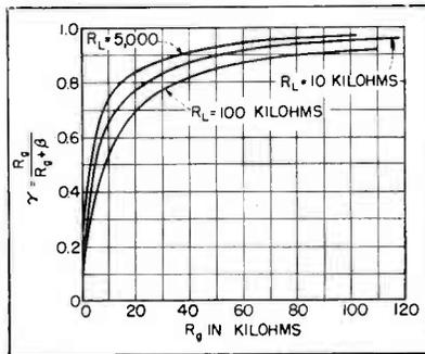
FIG. 6—Load resistance curves
