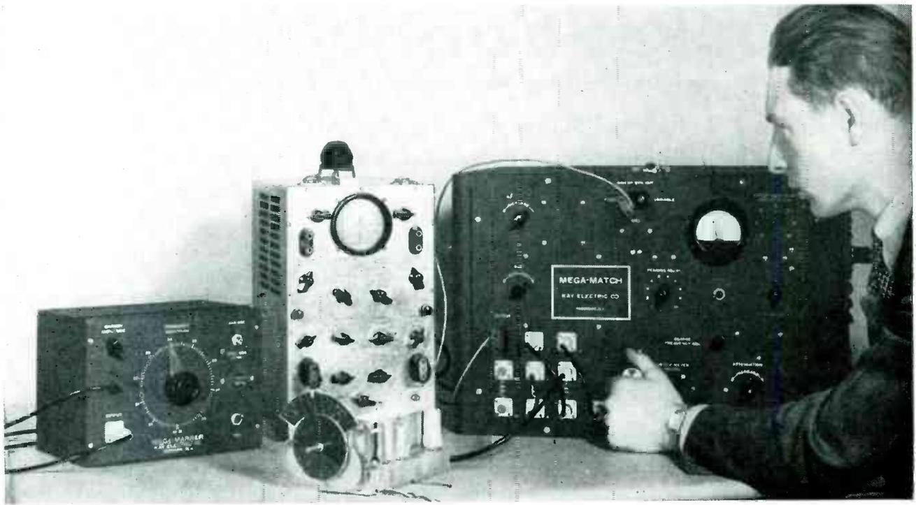
FIG. 1—Frequency-scanning vhf impedance meter in use, with conventional oscilloscope used as indicator
