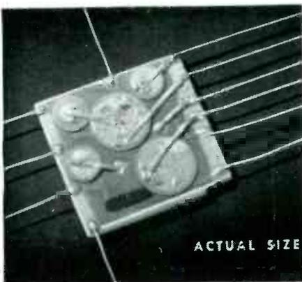
**2** Rear view of Beltone-CRL unit shows integral construction — ceramic disc capacitors, "printed" silver leads and resistors (black paths).
