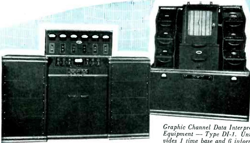
*Graphic Channel Data Interpretation Equipment — Type DI-1. Unit provides 1 time base and 6 information channels.*
