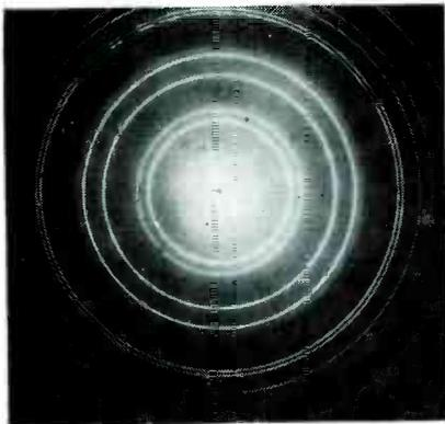
Although oxidation of a magnesium disc was not visible, this reflection electron pattern shows the surface presence of magnesium oxide
