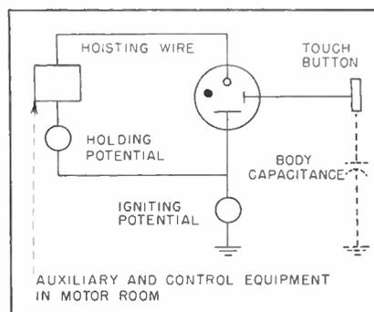
Basic circuit of electronic button; circuit values can be adjusted so that merely pointing at the button fires the tube
