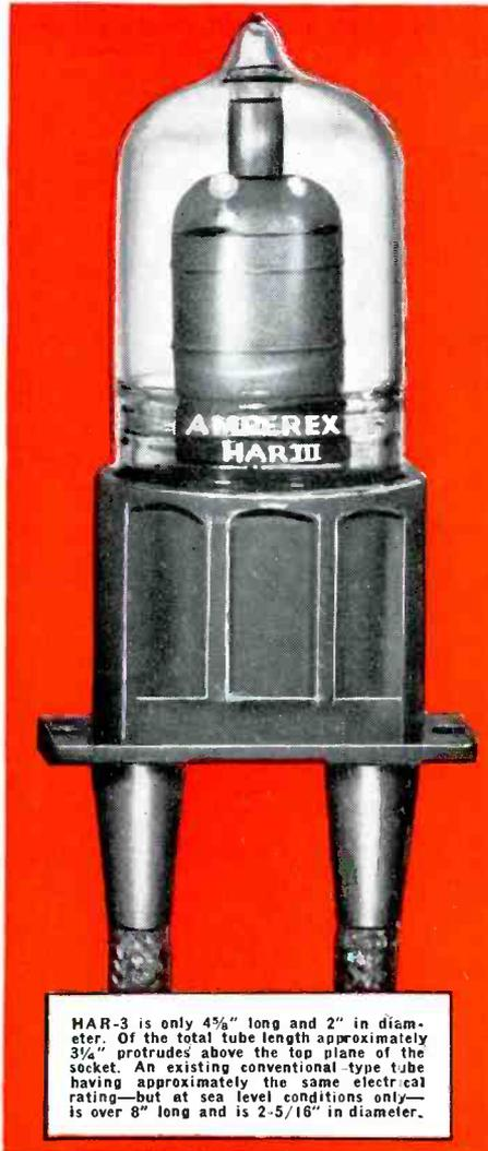
HAR-3 is only 4 1/4" long and 2" in diameter. Of the total tube length approximately 3/4" protrudes above the top plane of the socket. An existing conventional type tube having approximately the same electrical rating—but at sea level conditions only—is over 8" long and is 2-5/16" in diameter.
