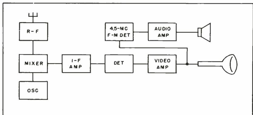
FIG. 1—Typical intercarrier receiver. The i-f, video detector and video amplifiers do double duty, handling picture and sound signals simultaneously
