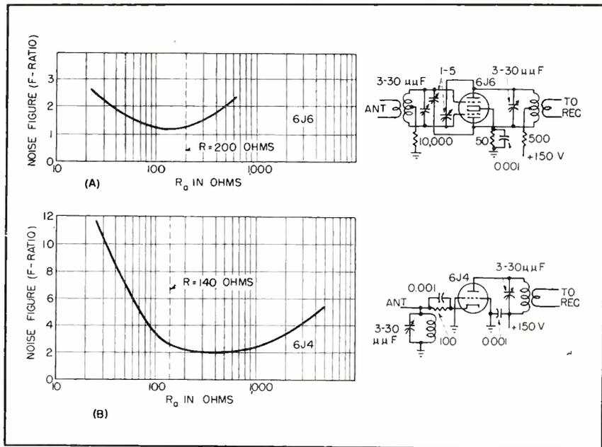
FIG. 4—Preamplifier circuits and measurements
