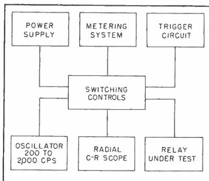
Fig. 1—Block diagram of the relay tester
