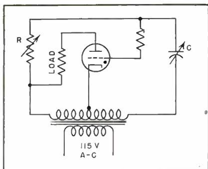
FIG. 1—Basic phase-control circuit using a single thyatron tube
