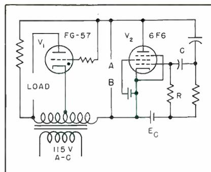
FIG. 3—Reactance-tube phase-control circuit that eliminates the transformer
