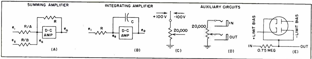
FIG. 1—Computer includes (A) summing and (B) integrating amplifiers, (C) initial condition and (D) multiplying pots, and (E) limiters
