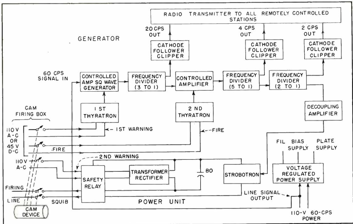
FIG. 2—Block diagram of the firing unit. Control signals are sent out by radio to receiving triangulation stations. Warning sirens at the firing grounds are actuated and the main firing line is open circuited until the safety sequence is complete
