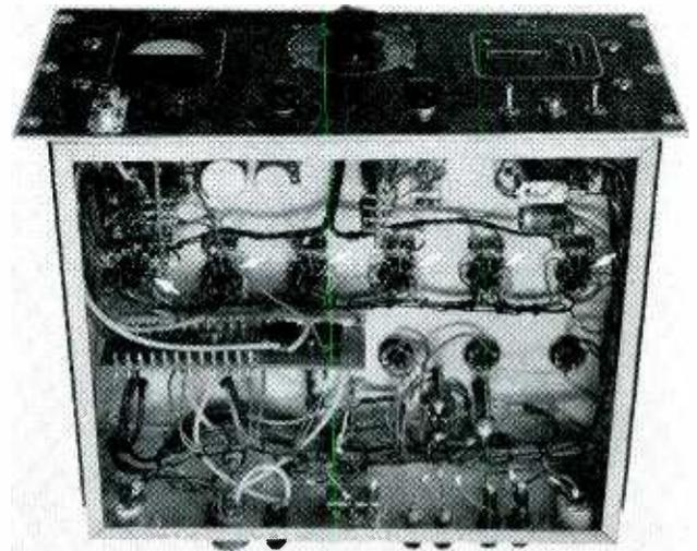
Bottom view of 64 scaler, showing simplicity of wiring. Arrows point to sockets of plug-in units
