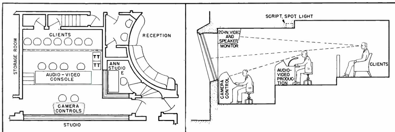
FIG. 3—Studio B control, showing location of technicians, directors, and clients. FIG. 4—Elevation view of a typical control room, showing sight lines for occupants. Video monitor indicates television action
