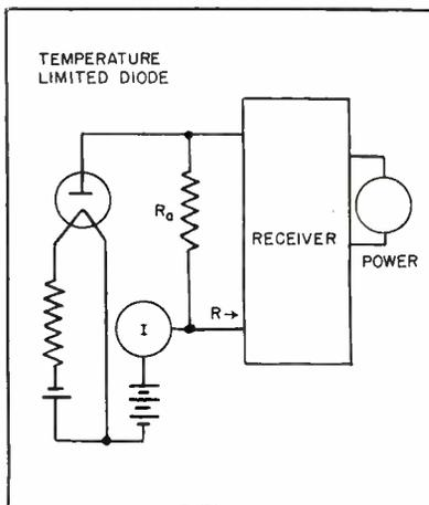
FIG. 1—Basic circuit for measurement of noise figure with a noise diode
