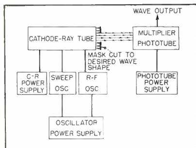
FIG. 1—Block diagram of system for generating stimulating current whose waveform is cut out from cardboard mask
