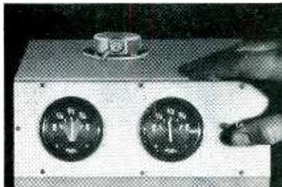
Silicone damping of gauge at right eliminates familiar fluttering of pointer shown in untreated automobile instrument at left.
