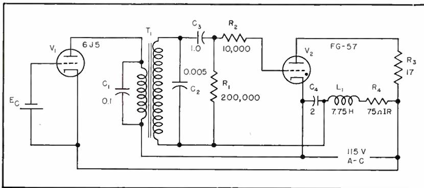
FIG. 6—Practical d-c phase control circuit using basic circuit of Fig. 5
