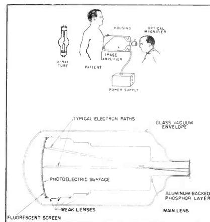
X-rays that have passed through the patient strike the fluorescent screen at left and produce light photons that eject electrons from the photoelectric surface. The electrons are electrostatically accelerated and focused to form an inverted smaller image on the phosphor at right. Optical magnification brings this image back to the original five-inch size
