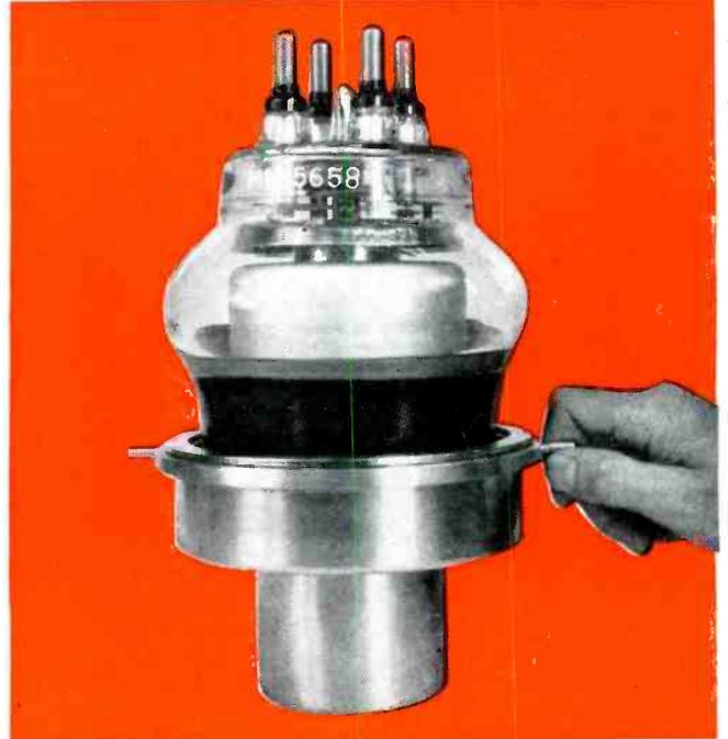
**MACHLETT AUTOMATIC SEAL WATER JACKET.\*** No tools are needed to open and close this new jacket. No worry about tube breakage or water leakage. Jacket cannot be opened unless water pressure is off, nor closed unless tube is properly seated. \*Pat. applied for
