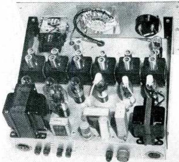
Top-of-chassis view of 64-count scaler using six scale-of-two plug-in units. Electromagnetic counter is at upper left
