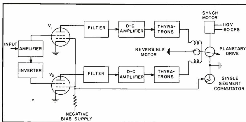
FIG. 3—Elements of the servoamplifier system used to synchronize cameras mounted on gun directors
