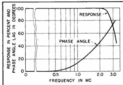
FIG. 3—Frequency response and phase angle of amplifier with link adjusted for 3-mc band
