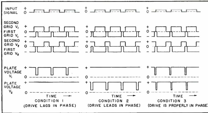
FIG. 4—Voltage patterns showing conditions that lead to automatic synchronism of tracking cameras
