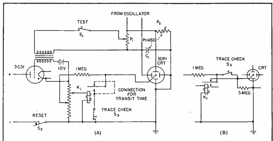
FIG.2—Circuit wiring for measuring operate time of normally-open relays (A), and opening time of normally-closed contacts (B). Transit time is measured by the dashed line modification of circuit A
