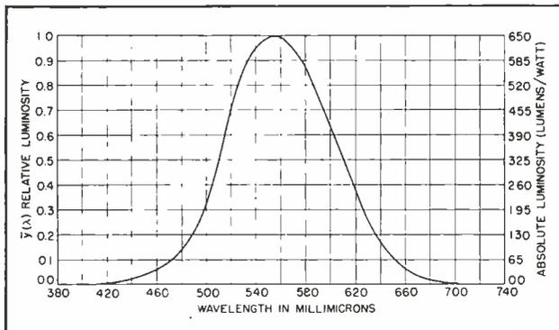
FIG. 1—Relative values (left) of luminosity curve apply to conditions met in television; absolute values (right) are used to determine luminous efficiency
