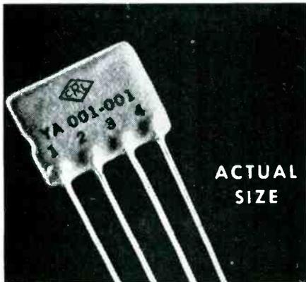
**2** CRL'S *Couplate* consists of a plate load resistor, grid resistor, plate by-pass capacitor and coupling capacitor. Write for Bulletin 943.
