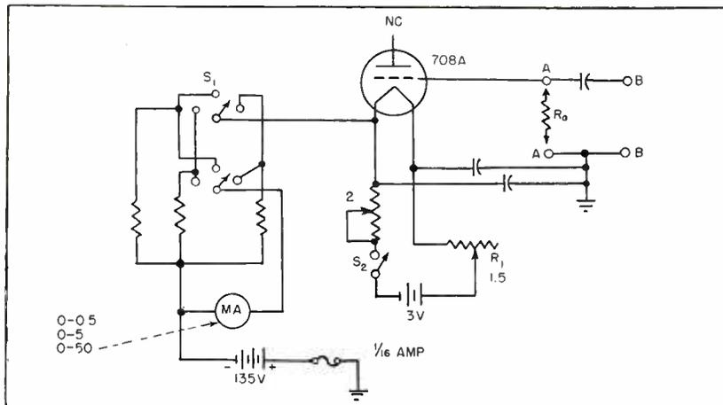
FIG. 2—Schematic diagram of the diode noise generator. The receiver connects to points A-A normally, to B-B if d-c isolation is required
