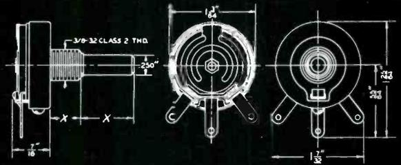
TYPE C IS A SMALL 2 WATT UNIT, USED AS A METER COMPENSATOR, MINIATURE MOTOR CONTROL AND LIGHT DIMMER.
