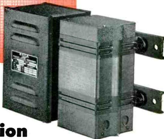
TYPE CVH, an important newcomer in a famous line—a SOLA CONSTANT VOLTAGE Transformer designed for use with equipment that requires a source of undistorted voltage. These new transformers, available in 250, 500 and 1,000 VA capacities, provide all of the voltage stabilizing characteristics of the standard SOLA Constant Voltage Transformer, with less than 3% harmonic distortion of the output voltage wave.
