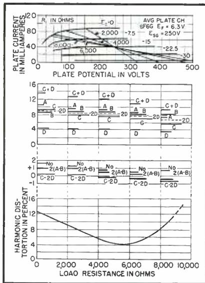
FIG. 1—Using currents from tube characteristic, combinations are plotted and differences and quadratic sums obtained giving quantities from which percent harmonic distortion is obtained
