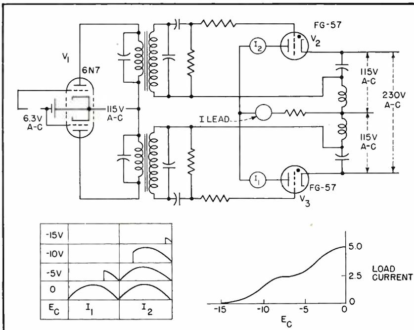
FIG. 7—Phase-control is provided over 360 degrees as illustrated by the waveforms
