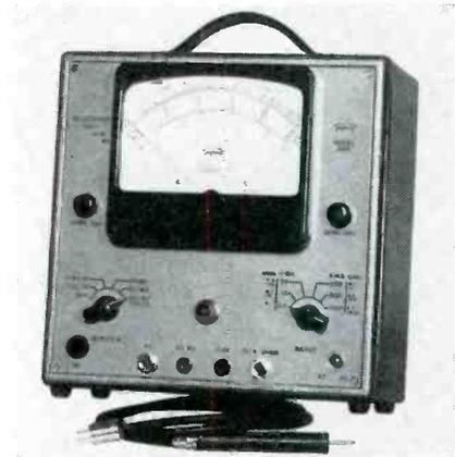
ation, broad test facilities and speed. It eliminates switching back and forth from one range to another to balance the circuit, and requires only zeroing the meter on the range to be used.
