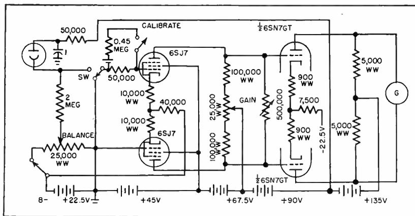
FIG. 4—Direct-coupled amplifier for driving recording galvanometer from phototube input
