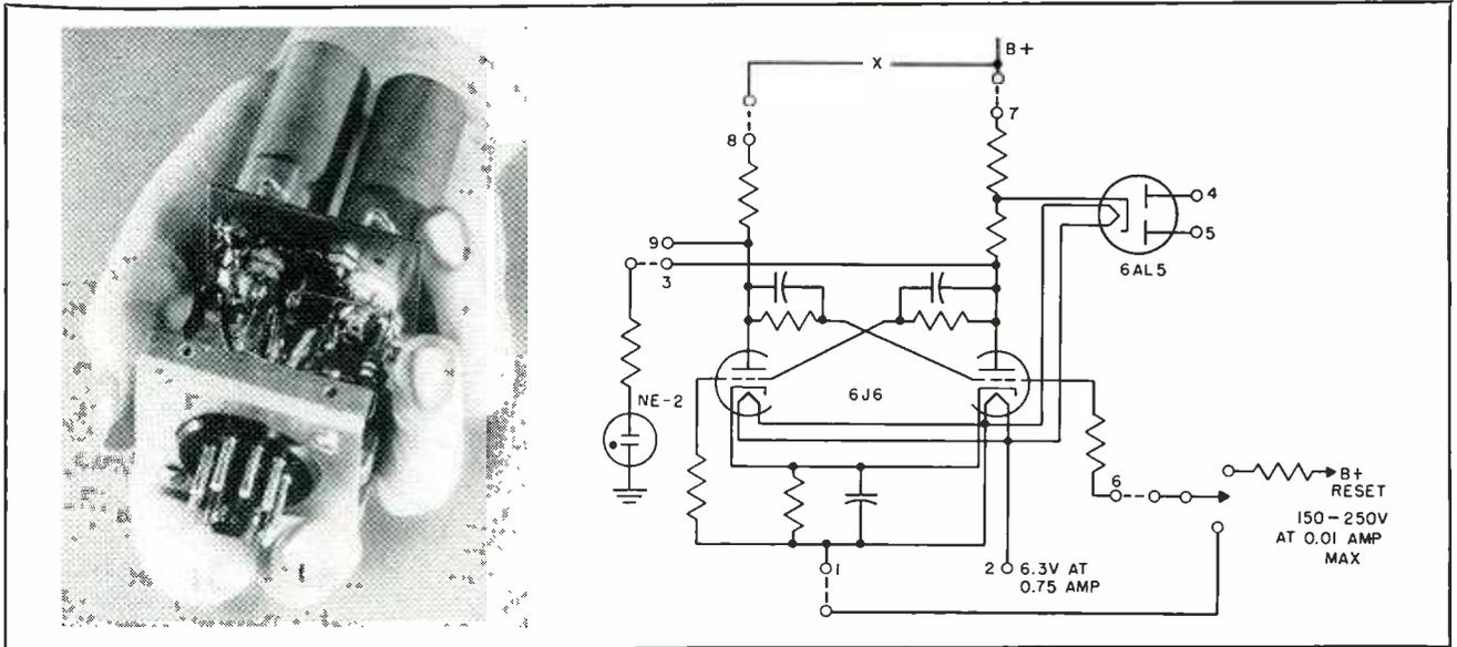
FIG. 1—Duoscale plug-in scale-of-two unit and schematic diagram. Numerals are pin connections for plug. Circuit is modified Eccles-Jordan trigger circuit using miniature tubes
