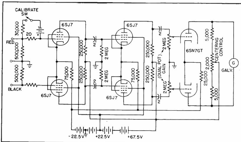
FIG. 5—Circuit of push-pull electrocardiograph amplifier adapted to work with Sanborn galvanometer
