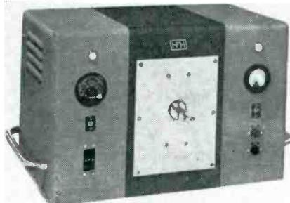
tronic power generator for production induction heating. Power output is 1,200 watts; frequency, 400 kc.
