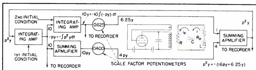
FIG. 3—Computer set up to solve equation of oscillator current
