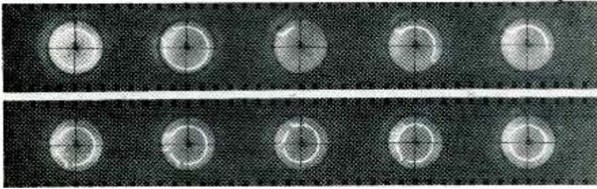
Upper oscillograms show closing time of normally-open contacts, opening time of normally-closed contacts, transit time of moving contact in operate direction, closing time of normally-closed contacts on drop out, and opening time of normally-open contacts on drop out. Lower strip shows various types of contact bounce
