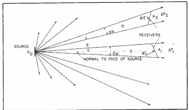
FIG. 2—Luminous intensity of the source is the flux emitted per solid angle. Illuminance of a receiver is the flux per unit area incident on its surface
