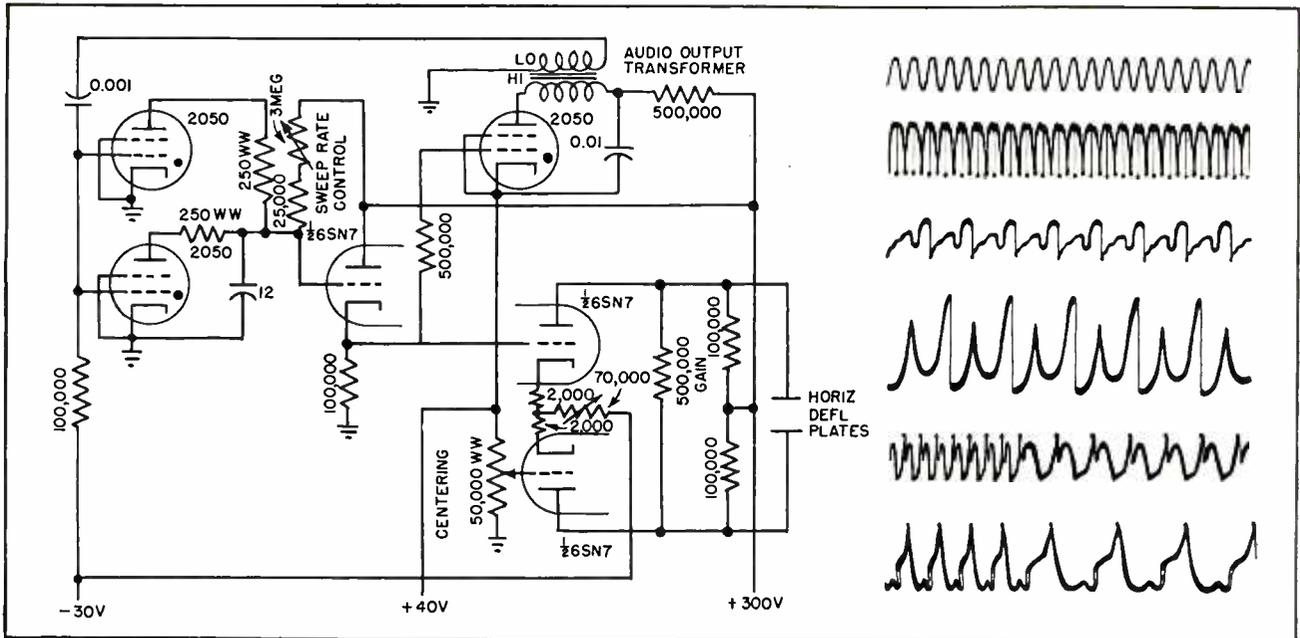
FIG. 2—Relaxation oscillator circuit used to sweep vertical-line trace across cut-out mask at desired frequency for generating medical stimulating current, and examples of waveforms generated. Lower two records show result of varying sweep rate
