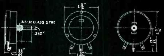
TYPE E, RATED AT 7 WATTS, IS WIDELY USED IN PRECISION INSTRUMENTS, RESISTANCE BRIDGES AND OTHER CIRCUITS REQUIRING ACCURATE SETTINGS.
