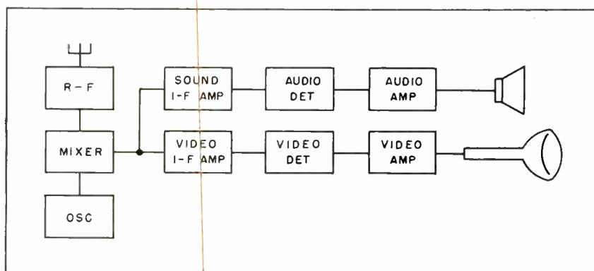
FIG. 2—Typical conventional television receiver. This type of receiver is more susceptible to faults in the local oscillator than is the intercarrier type
