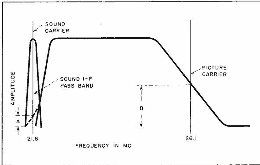
FIG. 3—Intermediate-frequency response characteristics of conventional (heavy solid line) and intercarrier (dashed-line extension) receivers
