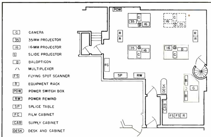
FIG. 6—Layout of equipment for telecine Studio C where motion pictures, transparencies, or opaque illustrations can be fed into the network
