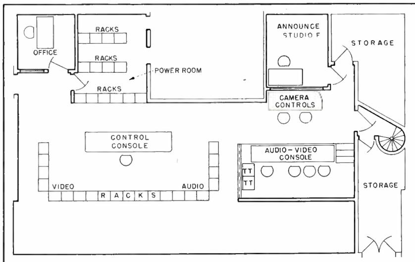
FIG. 7—WCBS-TV Master Control. Camera and associated controls are separated by curtains from main control activities at left
