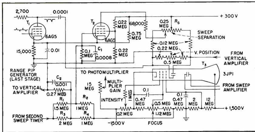
FIG. 4—Schematic diagram of gating circuits and cathode-ray tube
