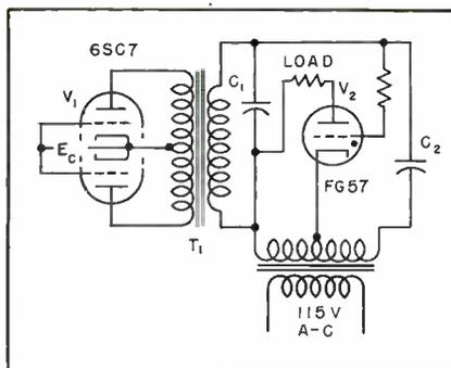
FIG. 2—Phase-control circuit with vacuum tubes as the variable parameter
