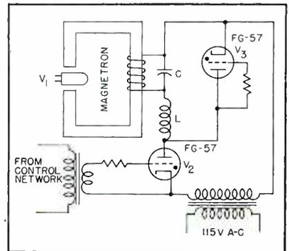
FIG. 8—Magnetron flux density is controlled by this circuit
