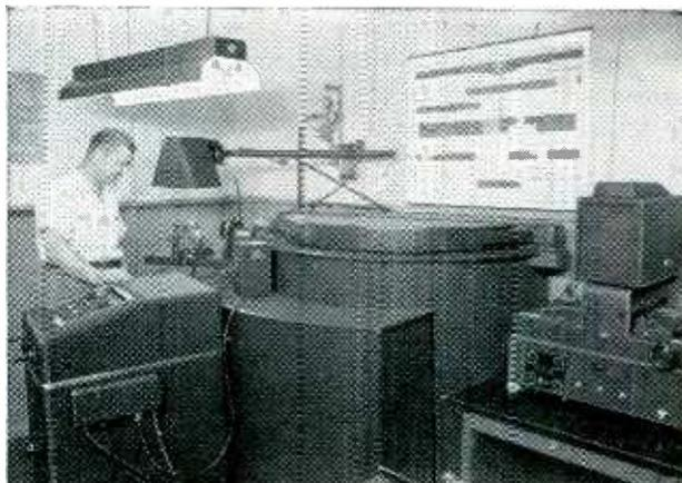
*This Mallory spectrograph determines the purity and composition of metals and alloys.*
