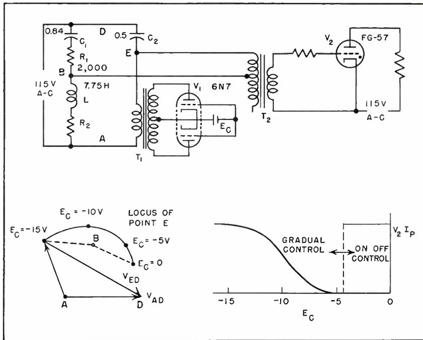
FIG. 4—Circuit for phase control with direct voltage. Transformer  $T_1$  is a Stancor A-63C, and  $T_2$  is a Thordarson T-33A91. Internal resistance  $R_2$  is 75 ohms. Vector relations and control characteristics are included
