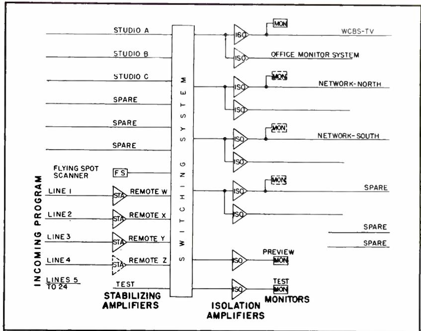
FIG. 8—Block diagram of Master Control video switching, showing mixing of studio and remote program for composite network output
