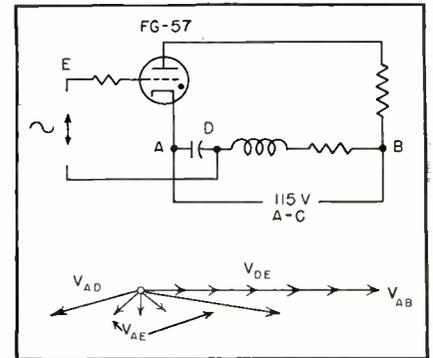
FIG. 5—Control is effected by changing the amplitude of an alternating voltage
