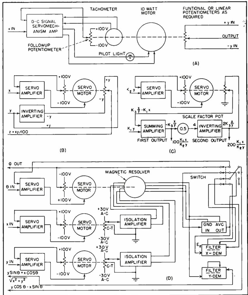
FIG. 4—Servomechanisms manipulate variables and vectors
