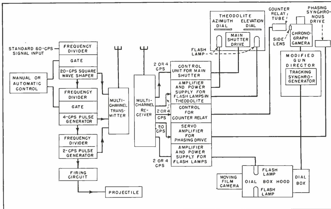
FIG. 1—Block diagram of the camera synchronizing system that is triggered when the projectile is fired. The camera station is common to two or more receiving locations. Position of the missile is recorded by the moving film camera by means of a linkage from the chronograph camera
