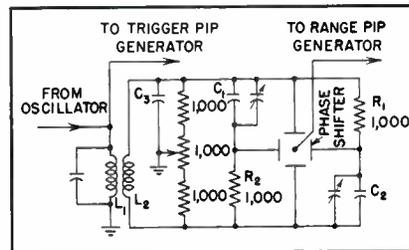
FIG. 5—Phase shifter and phase-splitting circuits
