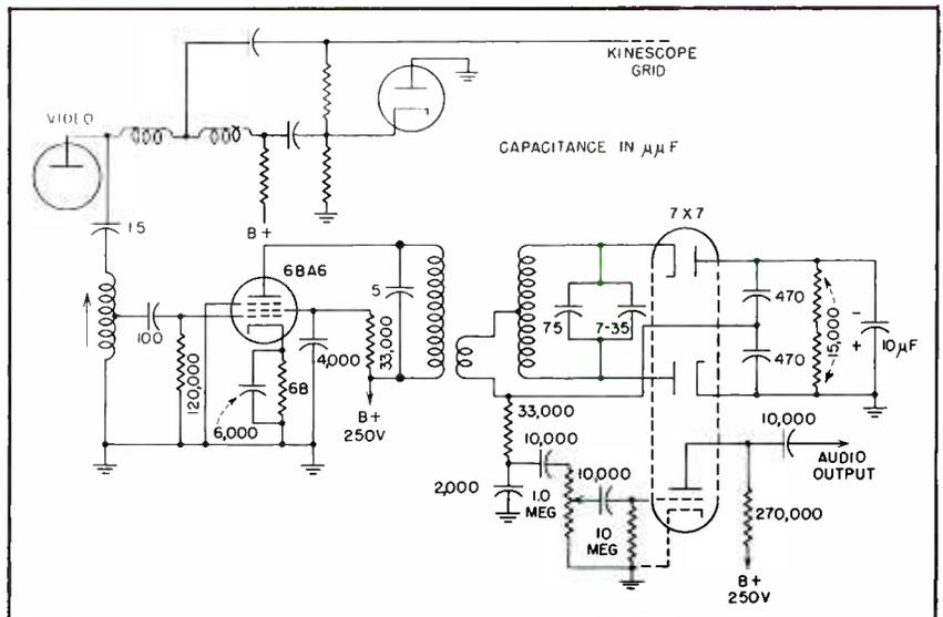
FIG. 5—Typical intercarrier sound circuit using a limiting amplifier and ratio detector for demodulation
