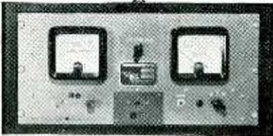
Calibrates crystal plate of unknown frequency against standard plate of desired frequency. Consists of standard and test oscillators whose outputs are mixed to produce an amplified beat note the frequency of which is shown on meter with ranges of 500, 5000, 50,000 cycles. In sturdy metal cabinet with hinged cover, 9"H x 13"W x 19"L. 4" square activity and frequency meters on front panel. Complete with tubes. New. Used but excellent condition **\$22.50**
