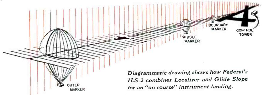
Diagrammatic drawing shows how Federal's ILS-2 combines Localizer and Glide Slope for an "on course" instrument landing.
