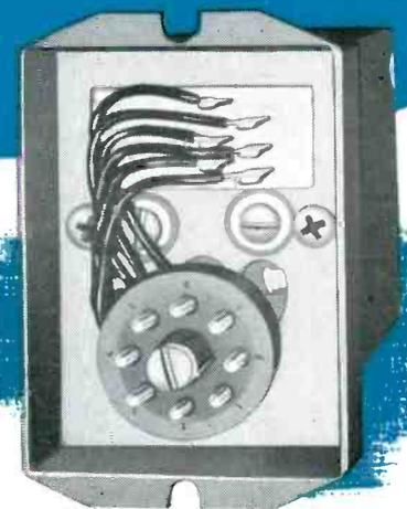
View of base assembly of dust-tight relay mounting showing terminals brought through Neoprene gasket. Note radio-type plug and flanges for securing to chassis.
