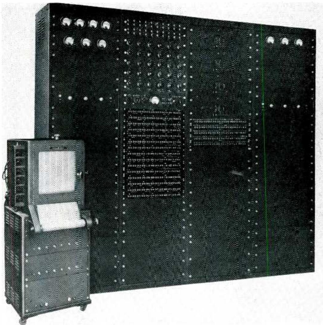
Elements of computer are interconnected by plugging into jacks at a common patch bay; recorder plots solution
