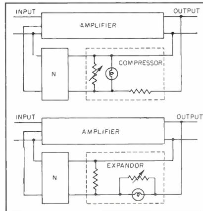
FIG. 2—Variable resistance controls the dynamic change that the lamp can produce
