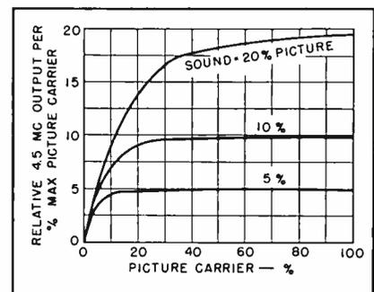
FIG. 4—Amplitude modulation of 4.5-mc beat note as a function of picture modulation, for various amplitudes of sound signal relative to picture signal
