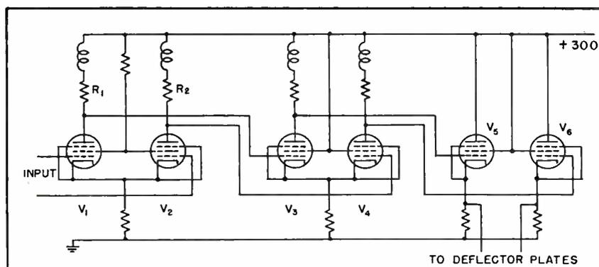
FIG. 1—Simplified schematic diagram of direct-coupled amplifier stages
