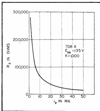
FIG. 3—Plate resistance versus plate current for the 708A tube
