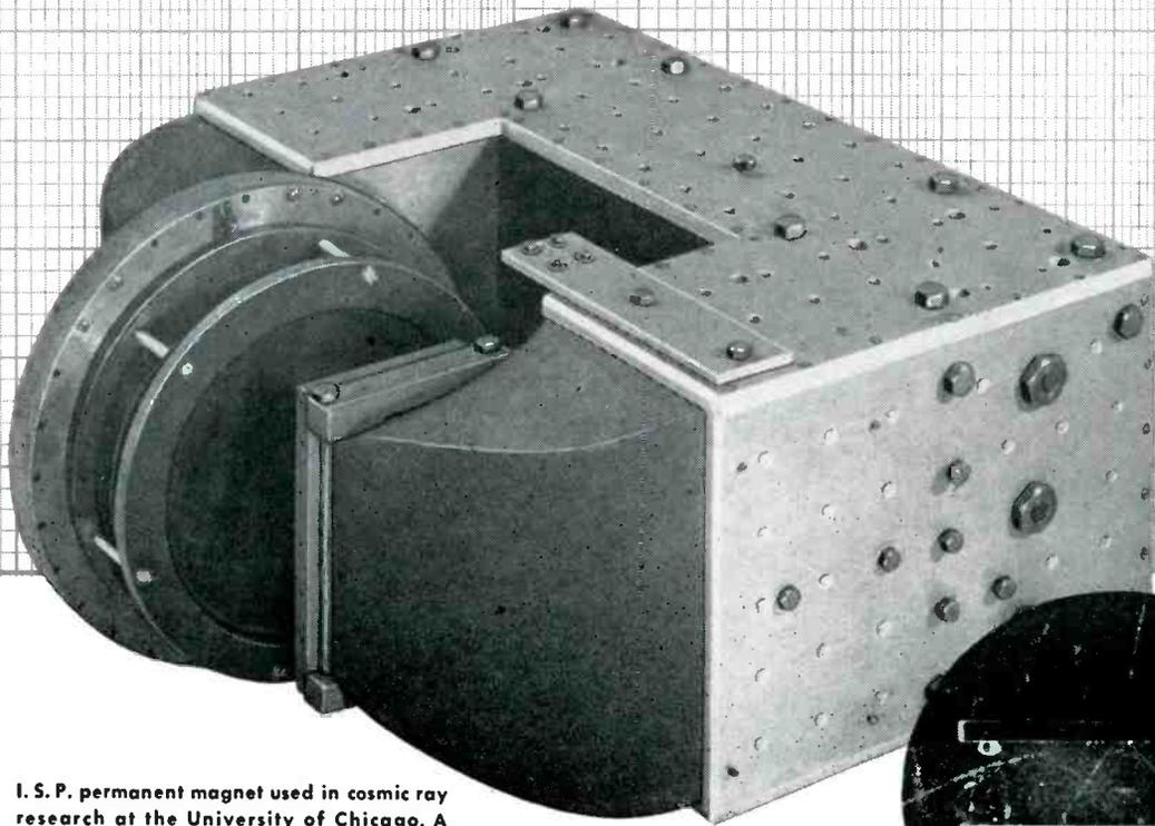
I. S. P. permanent magnet used in cosmic ray research at the University of Chicago. A "cloud chamber" is fastened rigidly within the air gap, so that cosmic rays entering the gas-filled chamber are deflected by the magnetic field. Physicists' calculations are based on the path made by the ray through the gas.
