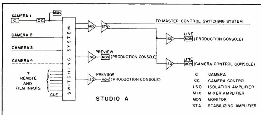
FIG. 5—Block diagram of video switching used in Studios A and B
