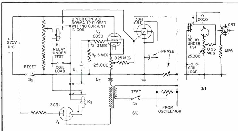
FIG. 3—Schematic circuit diagrams for measuring drop-out time of relays. Circuit A is for relays with normally-closed back contact, and modification B for opening time of normally-open contacts
