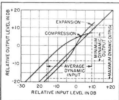
FIG. 4—Dynamic ranges obtainable from amplifier incorporating adjustable adc
