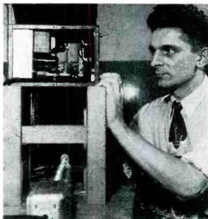
Spectral response at 1,850 and 2,537 Angstroms are measured in laboratory by placing photometer above lamps
