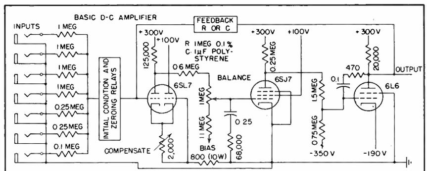
FIG. 2—Basic high-gain directly coupled amplifier used in computer
