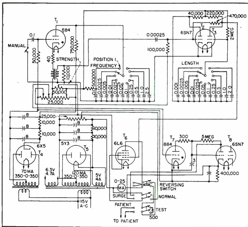
FIG. 3—Square-wave stimulator circuit providing separate adjustments for length and frequency of stimuli, along with constant preset current independent of resistance of patient
