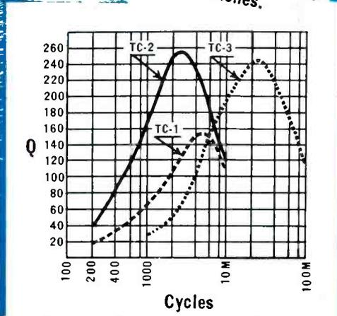
The big three out of 30 types of toroidal coils we are supplying.
