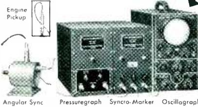
Angular Sync Pressuregraph Synchro-Marker Oscillograph
