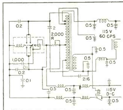
Adding potentiometer *R* to a vibrator power supply permits frequency adjustment
