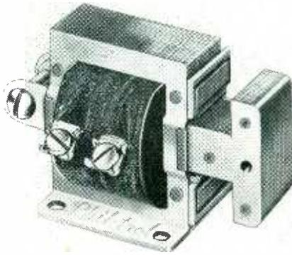
bonded silicon steel laminations and a T-shaped laminated plunger adaptable for both push and pull operations. It is available for continuous duty on 115 volts, 60 cycles, with a maximum stroke of one inch. Approximate pull is 2 pounds at  $\frac{3}{4}$  inch, 4.2 pounds at  $\frac{1}{4}$ -inch stroke.
