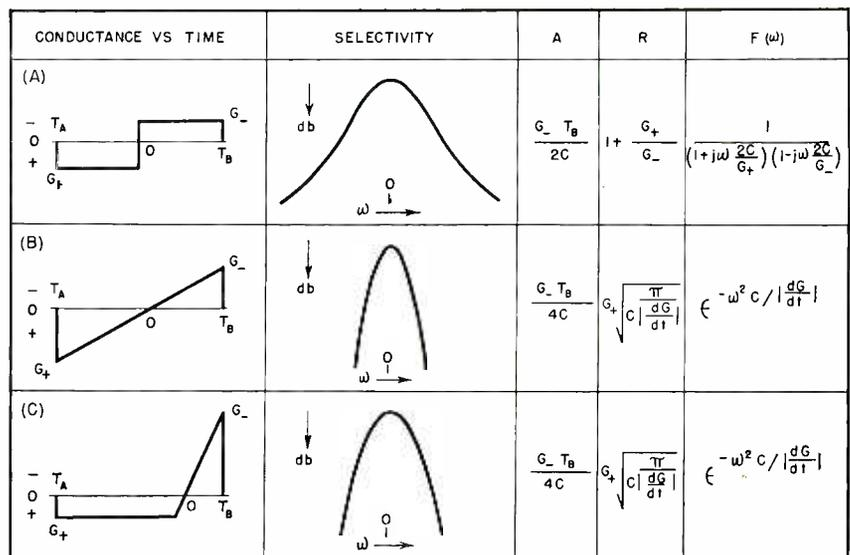
FIG. 3.—Conductance waveform controls selectivity, as these specific examples show
