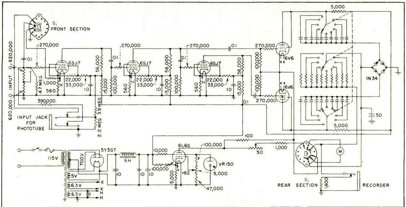
FIG. 3—Circuit of Hewlett-Packard frequency meter and tachometer used as a speed indicator for testing cabin superchargers
