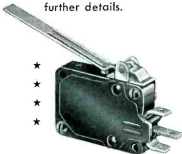
Model M fitted with No. A-18 Leaf Actuator Bracket. Also furnished with Roller Leaf, No. A-18M. Underwriters' Lab., Inc. Insp. 10 Amps, 125 V., 5 Amps, 250 V., A. C.
