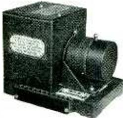
**AUTOMATIC KEYER** provides continuous or interrupted identification signals for beacon or aerophare service. Small, compact ( $6\frac{5}{8}'' \times 9'' \times 7''$ ) and fully enclosed, this keyer will give long trouble-free service. Two synchronized cams, which can be milled to your specifications, provide several keyer combinations. Motor -- 105/115 v-50/60 cy.
