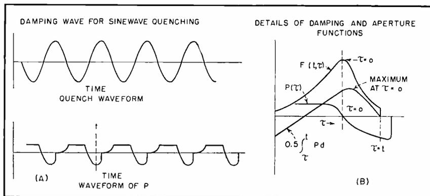
FIG. 2—Variation with time of the damping and aperture functions depends on the form of the quenching wave
