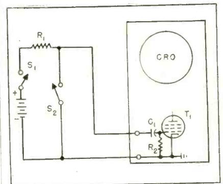
FIG. 1—Simplified circuit using battery to charge capacitor
