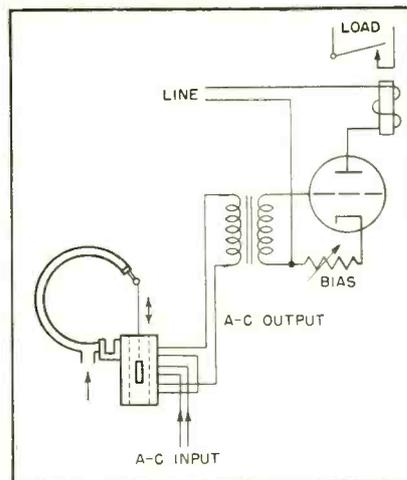
FIG. 5—Electronic phase and voltage-sensitive relay
