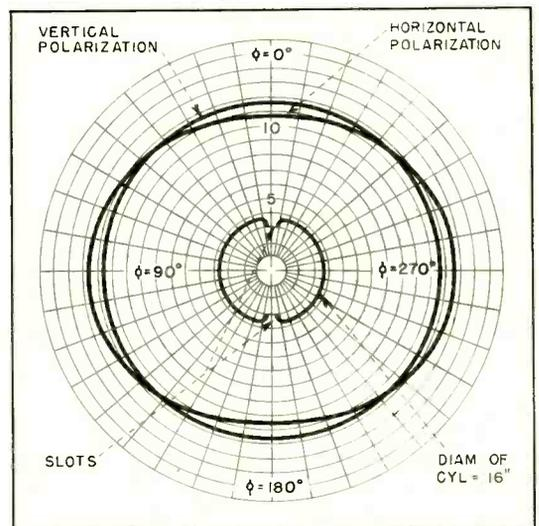
FIG. 9—Vertical and horizontal-polarization components of horizontal-plane pattern at 100 mc
