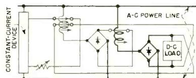
in opposition to the first carries the sensing current that is proportional to the load voltage. Because two transductors are used, the regulation is high. A rectifier of this type which can operate on both constant current and constant voltage is called an avostat. Avostat-regulated rectifiers can be built for all outputs for which metallic rectifiers can be used.
