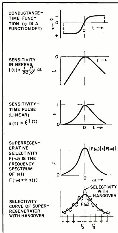
FIG. 2—Steps in the development of selectivity from waveform of conductance, as described in text, and, at bottom, effect of hangover on selectivity
