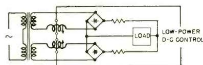
current. Power amplifications as high as a hundred million may be obtained from similar connections. If gain is sacrificed for stability, such transductor circuits are suitable for amplifying currents from photocells and thermocouples—
