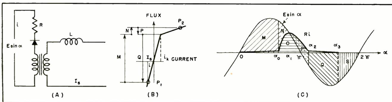
FIG. 4—Analysis similar to that of Fig. 3 but for imperfect core material
