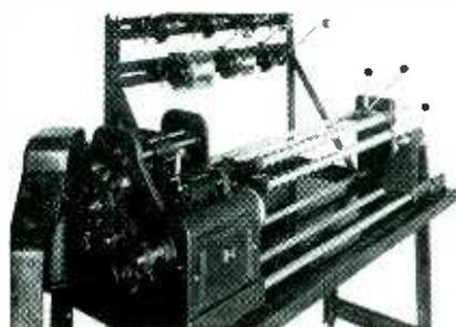
coil-winding machine that permits almost micrometer adjustment of guide roller travel through positive electric limit switches. The machine winds coils of all types in 16 gage to 42 gage wire. Maximum arbor space is 36 inches.
