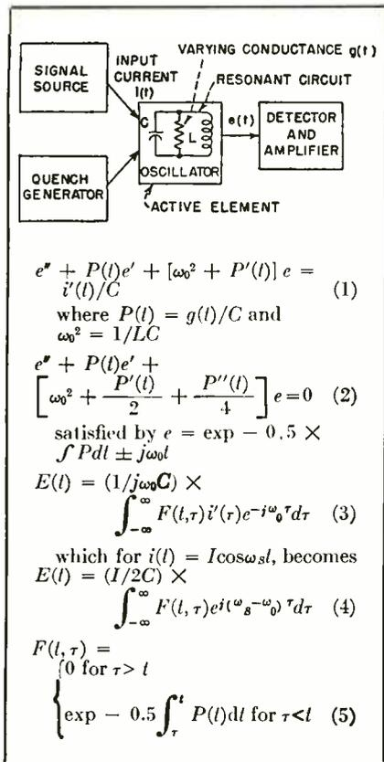
FIG. 1—Chief element of superregenerative detector is resonant circuit with varying damping; the equations describe it
