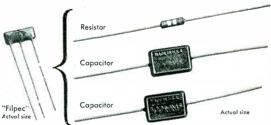
**3** Centralab's *Filpec* is for use as a balanced diode load filter. It combines up to three major components into one tiny filter unit, lighter and smaller than one ordinary capacitor. Also available for other applications. Write for complete information about *Filpec*, as well as other *Printed Electronic Circuits*.
