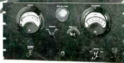
**RCA Model 66-A Modulation Monitor.** For rapid checking of percentage modulation. Neon peak flash lamp can be set to any predetermined threshold value. Readings can be made on either positive or negative modulation peaks. Measures also program levels, modulated carrier-shift, and average carrier value during modulation. Equipped with easy-reading meters, the 66-A is simple, accurate, foolproof.
