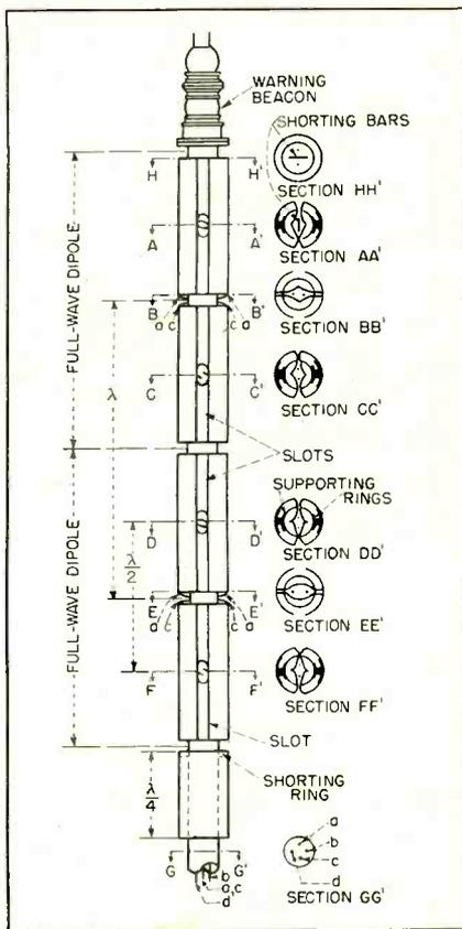
FIG. 10—Construction and feed details
