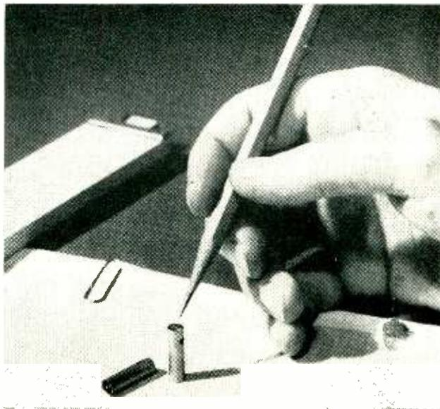
FIG. 1—Because of its simplicity the Transistor is even smaller than most subminiature vacuum tubes. The amplifier itself can be no larger than its associated coupling components
