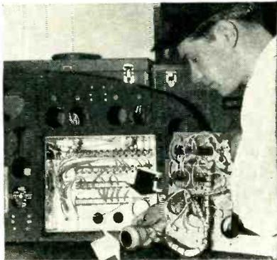
Mid Continent Airline mechanic, S. M. Fabac, holding a Cannon Electric Type "K" Plug about to be installed in the instrument panel of an MCA airliner. Upper black arrow points to K-32S Receptacle. "Major timesavers", say Mid-Continent Airlines of Cannon Plugs.
