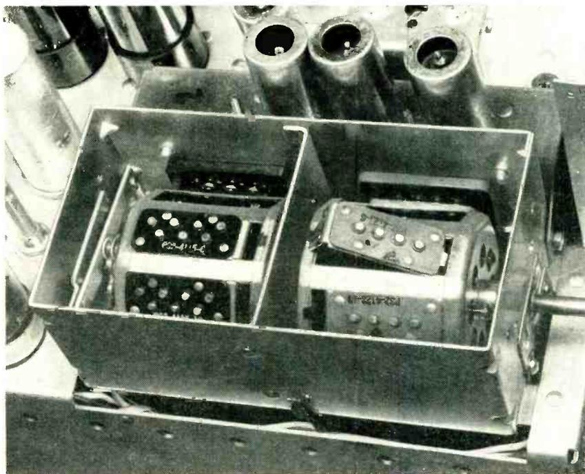
Philco rotary turret using replaceable coil assemblies
