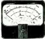
This is the exact meter utilized in the General Electric model YMW-1A Lab-Type Unimeter
