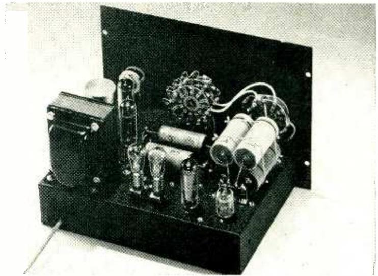
Top chassis view of the oscillator and conventional power supply. The two 6-watt lamps are in the feedback circuit
