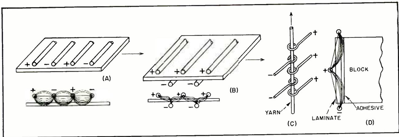
FIG. 2—Arranging electrodes of opposite polarity adjacent to each other along the film (A) or on opposite sides of it (B) minimizes the effect of air gap. The technique can be applied in various ways (C) and (D) depending on requirements
