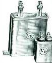
Plasticon A element; mineral oil impregnated in sturdy lead coated steel containers. Smaller, lighter and more economical than paper capacitors. Temperature range — 40° C to + 105° C. Type AOC rectangular; Type AOCO flattened oval.
