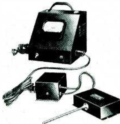
due to line voltage fluctuations. Readings are obtained merely by the operation of an on-off toggle switch, no previous current adjustments or calibration being required.
