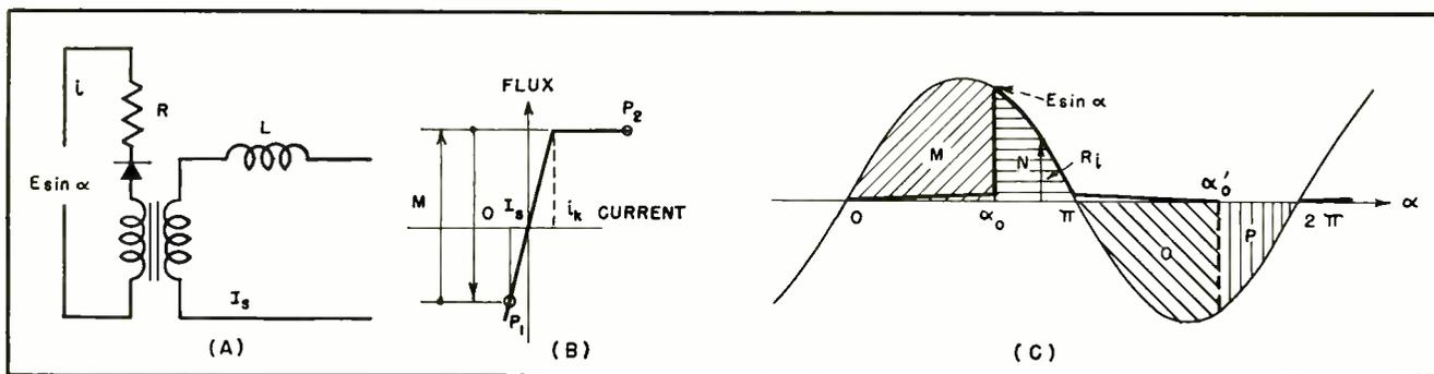
FIG. 3—Operation of a single element of a transducer with an ideal core
