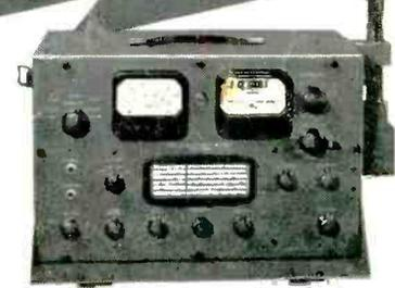
**RCA Model 308-A Field Intensity Meter.** *Direct Reading.* No calculations. Quick and accurate to use... light and easy to carry on field-intensity surveys. Covers 120 to 18,000 kc. Reads directly signal-strengths from 20 microvolts per meter to 10 volts per meter. Because it avoids time-wasting calculations for each of the hundreds of individual survey-points, the 308-A quickly pays for itself.
