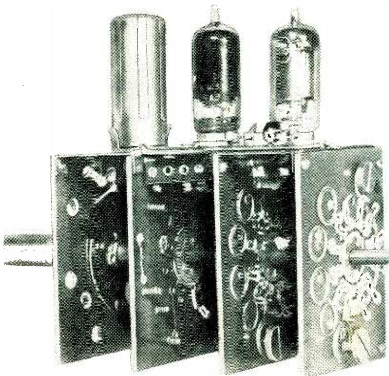
Franklin rotary-switch assembly with die-stamped transmission lines
