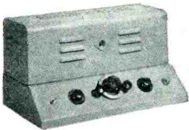
HS-5 alarm detects intrusion by change in antenna capacitance upon approach of a person. It also detects fire by means of a heat detector that operates at about 160 F. Slow capacitance changes owing to changing meteorological conditions will not affect the device.
