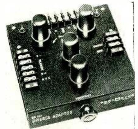
of two antennas for receiving the desired signal on as little as 0.05 volt of avc. It operates on 200 to 300 volts at 15 ma and filament supply of 6.3 volts a-c at 1.5 amperes.
