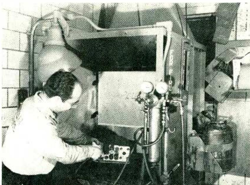
FIG. 3—Solvent spray booth for permanent installation in a factory, shop or laboratory. Fumes are vented to the outside air and additional equipment provided for control of air pressure, filtering and safety
