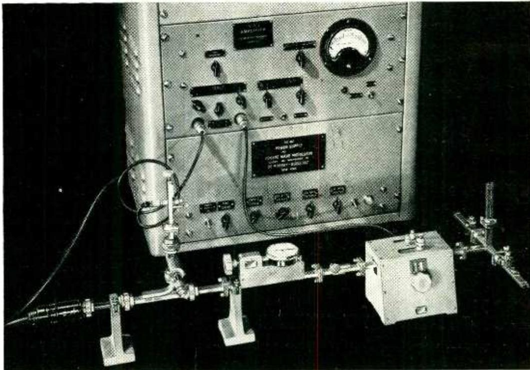
*A typical, K Band, bench test set-up with power supply and amplifier*
