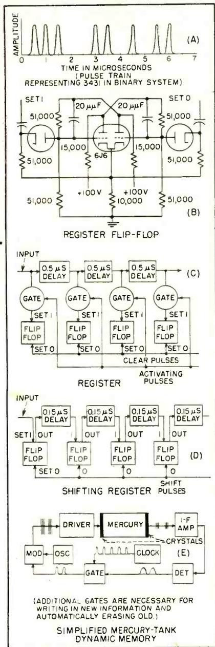
FIG. 1—Pulses are stored statically in flip-flops, dynamically in delay lines
