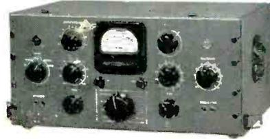
**RCA Type 69-B Distortion Meter.** With the Type 68-B Oscillator, the 69-B permits rapid determination of distortion, hum in amplifiers, noise, and frequency-response characteristics. Harmonic distortion can be measured at *any* audio frequency—not just at one “check frequency.”
