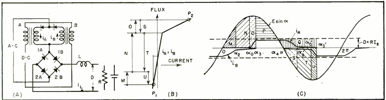
FIG. 5—Analysis like that of two-element transductor shows commutation of current from one element to the other
