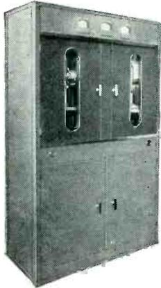
The Western Electric 33C Antenna Control Unit includes a branching circuit and two phase shifters, and permits adjustment of the current ratio and phase relation between the element currents of two towers. This unit handles up to 10 kw.
