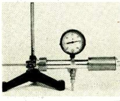
FIG. 2—Gas-filled cavity is acoustically resonant to modulation, electrically resonant to carrier frequency
