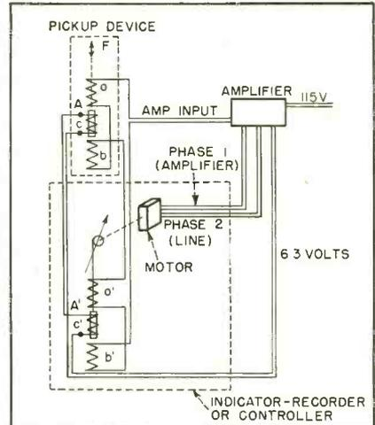
FIG. 4—Two Atcotrans in a balance circuit for remote indication or control
