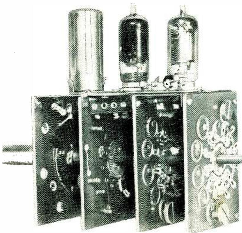
Franklin rotary-switch assembly with die-stamped transmission lines
