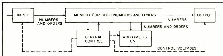
FIG. 3—Basic functional components of digital computer, and their interrelation
