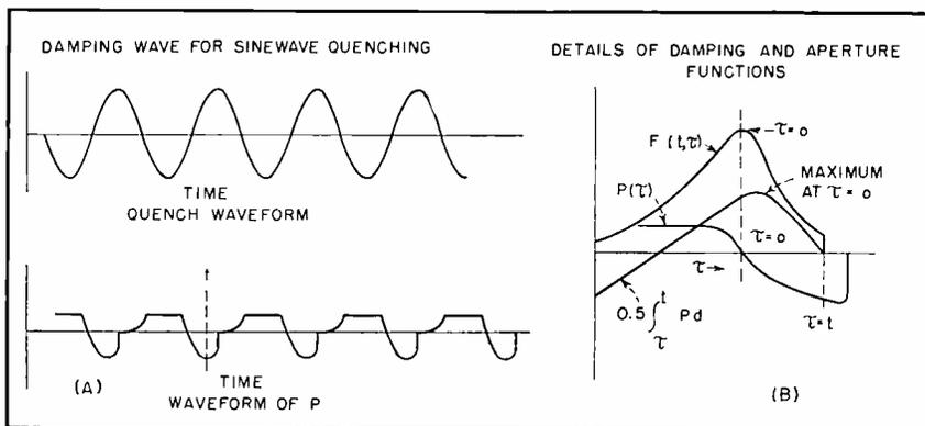
FIG. 2—Variation with time of the damping and aperture functions depends on the form of the quenching wave
