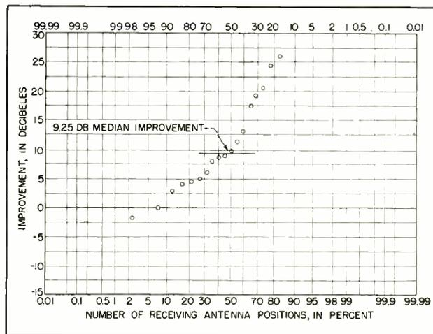
FIG. 6—Improvement of circular polarization over horizontal with vertical receiving antennas
