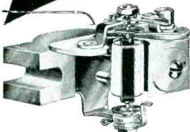
**BALANCE WEIGHTS** of helical type phosphor bronze, formed in a manner which eliminates slipping or shifting, are used to balance the moving element. All ranges AC and DC available in 2½", 3½", 4½" rectangular or round case styles and are guaranteed for one year against defects in workmanship or materials. Refer inquiries to Dept. F98.
