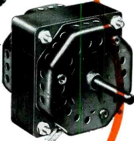
**MODEL B**—New type 4-pole shaded pole fan motor made in three standard lamination stack thicknesses. Power range is from 1/100th h.p. to 1/25th h.p. Size,  $3\frac{3}{4}$ " square. Especially adapted for fans, it will drive a wide variety of mechanical devices and is ideal for sound recorders. Full load speed 1550 R.P.M.—clockwise or counter clockwise rotation—not reversible. Made for 115 volts, 60 cycles—can be wound for 50 cycles and for other voltages.
