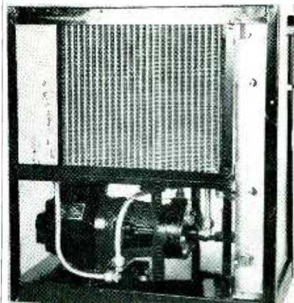
heated oven. The unit will dissipate 3,000 watts within a temperature rise of 40 F above ambient.
