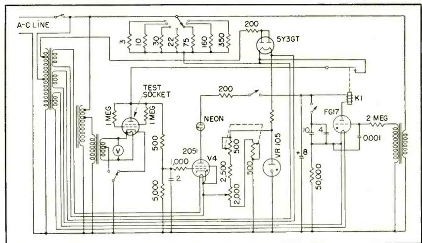
FIG. 1—Complete circuit of tube tester for phanotrons and thyatron
