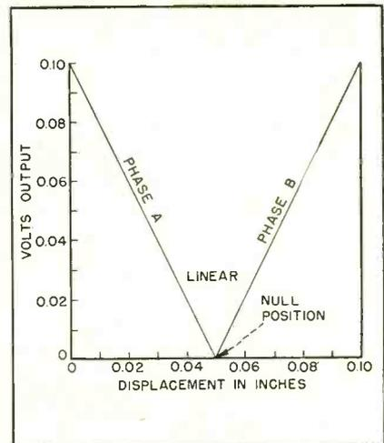
FIG. 2—Output voltage as a function of movement of the armature
