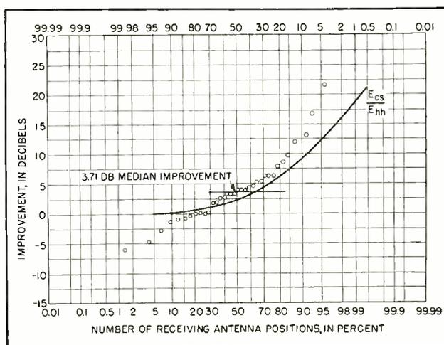
FIG. 4—Improvement of circular over horizontal polarization when receiving antennas are horizontal
