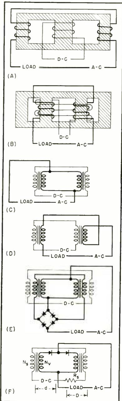
FIG. 1—Windings can be on one core (A) and (B), or on separate cores (C) to (F)
