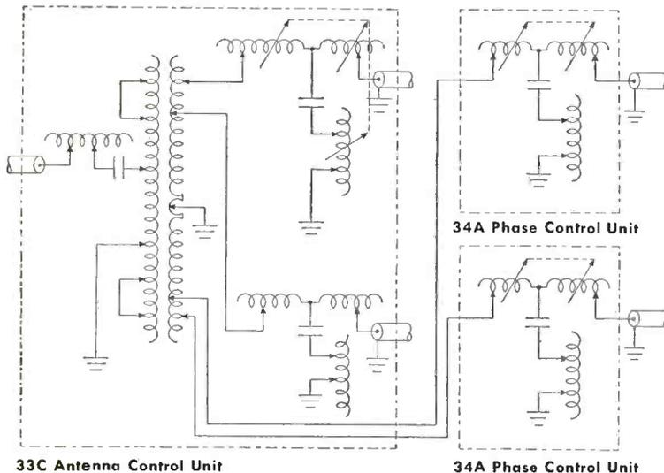
You can use Western Electric Antenna Control Equipment to good advantage in controlling current ratios and phase relationships. The master 33C Antenna Control Unit is styled to harmonize with cabinet design of Western Electric AM Transmitters. The 34A Phase Control Unit measures only 2' high, 3'7" wide, 2' deep, and requires no front-of-panel line-up space.
