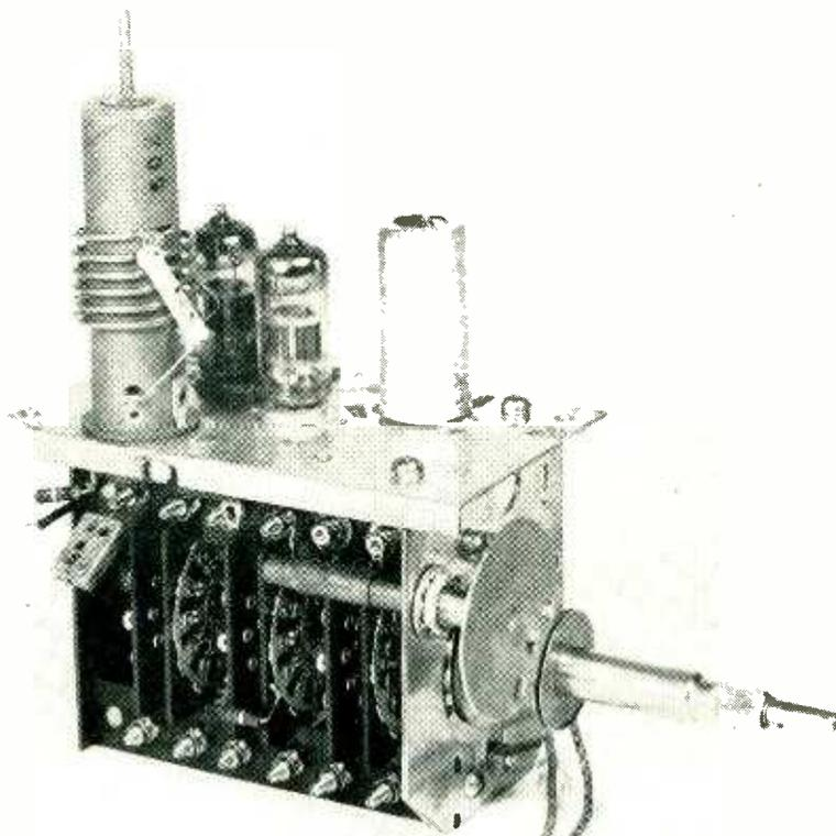
RCA rotary-switch type front end uses transmission lines and push-pull circuits
