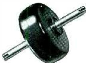
Hi-Q Disc Capacitors are high dielectric by-pass, blocking or coupling capacitors. Designed for application where its physical shape is more adaptable than tubular units. The placement of leads is such that close connections are easily made, thus reducing inductance to a minimum, a much desired feature in high frequency designs, such as television and FM. Available in three types: BPD-5: .005 MFD guar. min., BPD-10: .01 MFD guar. min. and BPD-1.5: .0015 MFD guar. min.
