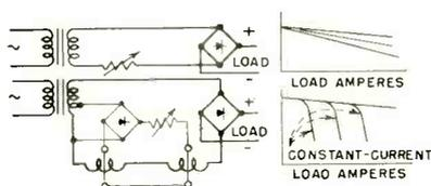
perfectly determined by transductor control current. Until limited by voltage, the current is independent of load resistance. Such circuits are extensively used in battery chargers for trucks and other cases where constant current is required. (For clarity the control portion of the circuit is drawn in lighter lines than the power portions.)
