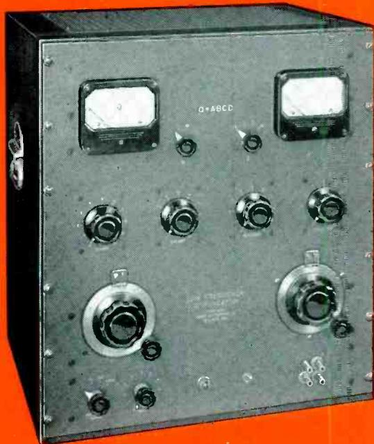
Frequency range from 20 cycles to 50 kilocycles. "Q" range from .5 to 500.
