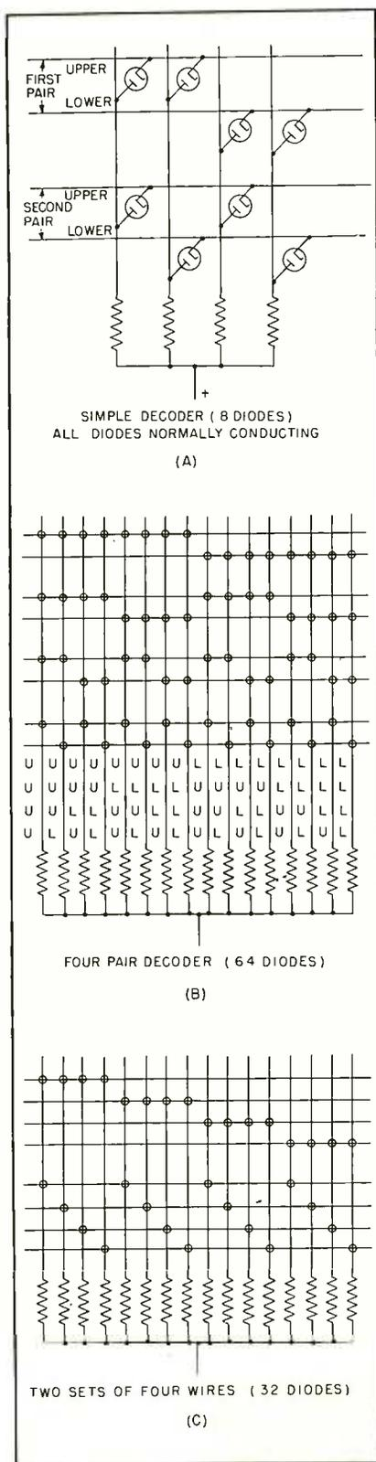
FIG. 4—Switching circuits use unidirectional conductance of diodes
