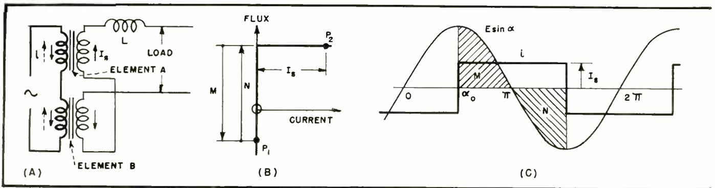
FIG. 2—Simple transductor connection (A) can be analyzed using portion of idealized magnetization curve (B). Voltage-time curves show action during operating cycle with zero
