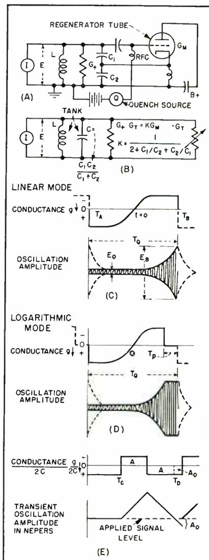
FIG. 1—Superregenerative circuit (A) and equivalent circuit (B) and relation of oscillation amplitude to waveshape of conductance (C), (D) and (E) under various conditions
