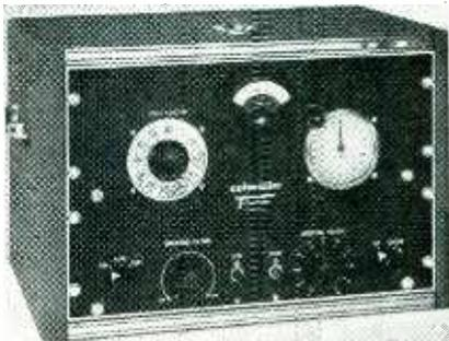
actuated by a pushbutton. Overall resolving time of the input amplifier and scaling circuit is about 5 microseconds. Pulse height sensitivity is approximately 250 millivolts.
