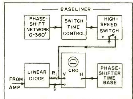
FIG. 3—Addition of the Baseline provides zero reference trace
