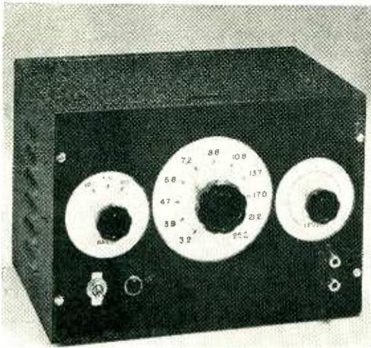
The low frequency oscillator showing range switch, step frequency selector, and level (gain) control
