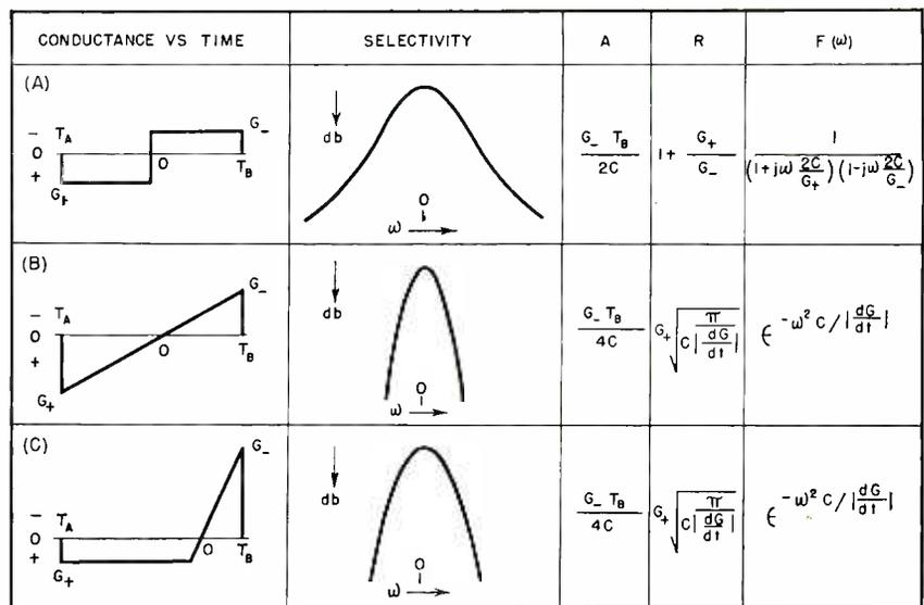
FIG. 3.—Conductance waveform controls selectivity, as these specific examples show
