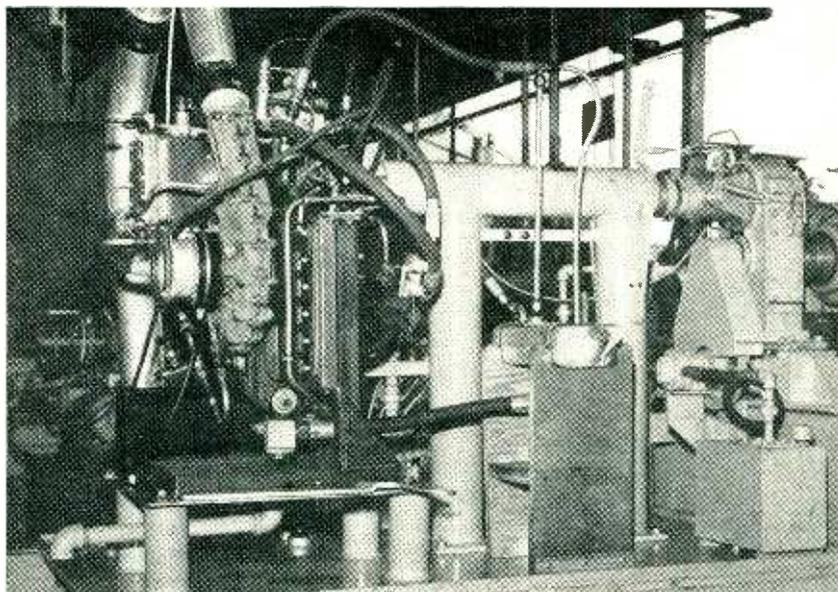
Test stand for an aircraft cabin supercharge:
