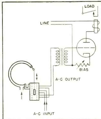
FIG. 5—Electronic phase and voltage-sensitive relay
