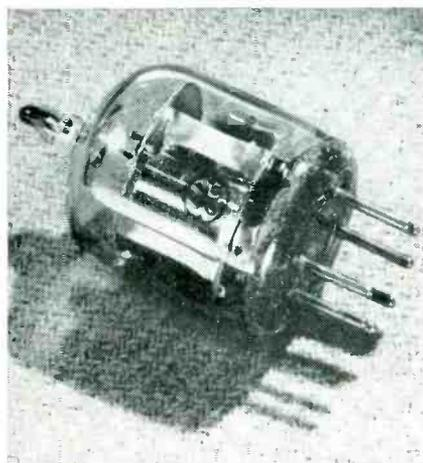
control grid and shield grid currents is inert-gas filled. Peak forward and inverse voltage ratings are 500 volts. Average anode current is 20 ma.
