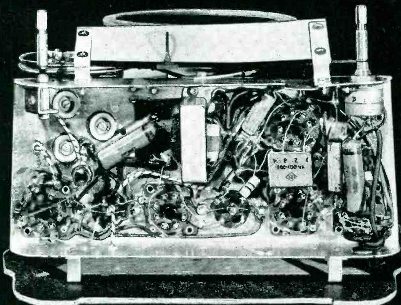
Sentinel Radio Corp. uses "Filpec" and "Couplate" for production savings on small receiver circuits.
