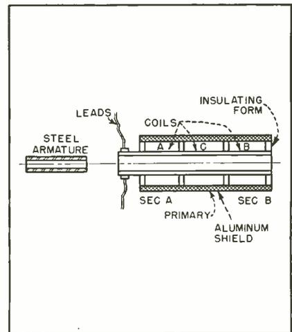
FIG. 1—Cross-section of coil assembly
