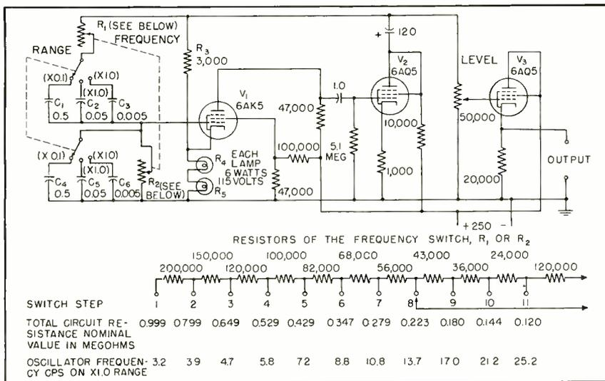
FIG. 1—Circuit diagram of the low-frequency oscillator. The stepped variable frequency control detail indicated
