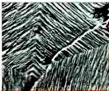
▲ An example of Electron Microscope's magnification 45,500X of chrome iron by replica and shadowing. Used by courtesy of Dr. Wyckoff and Dr. Williams.
