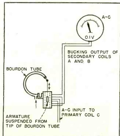
FIG. 3—Application of the pick-up unit to a Bourdon tube for pressure measurements
