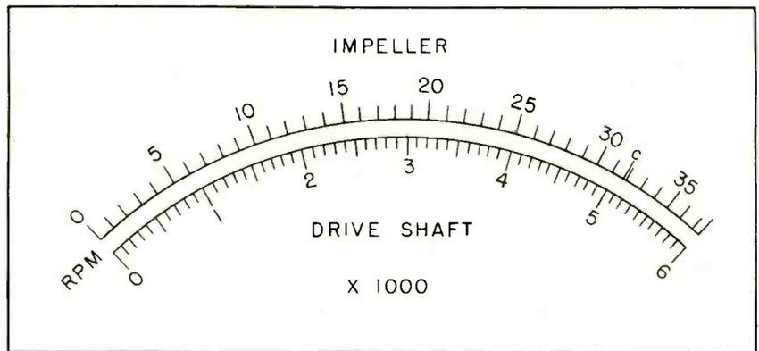
FIG. 4—Redrawn frequency-meter scale, giving rpm directly
