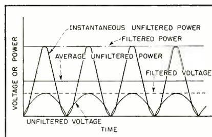
FIG. 3—Arcing at the applicator electrodes limits the peak voltage that can be applied. By filtering the power supply the effective rate of heating can be about doubled
