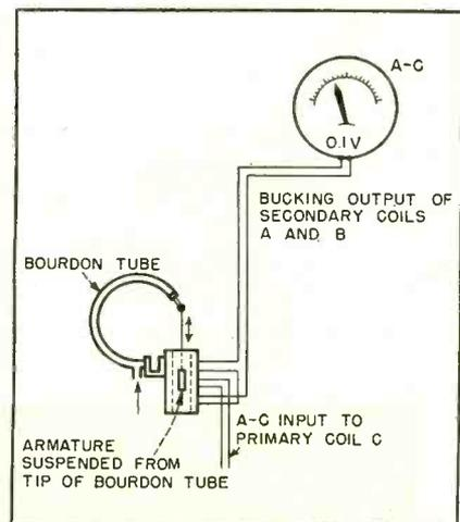
FIG. 3—Application of the pick-up unit to a Bourdon tube for pressure measurements
