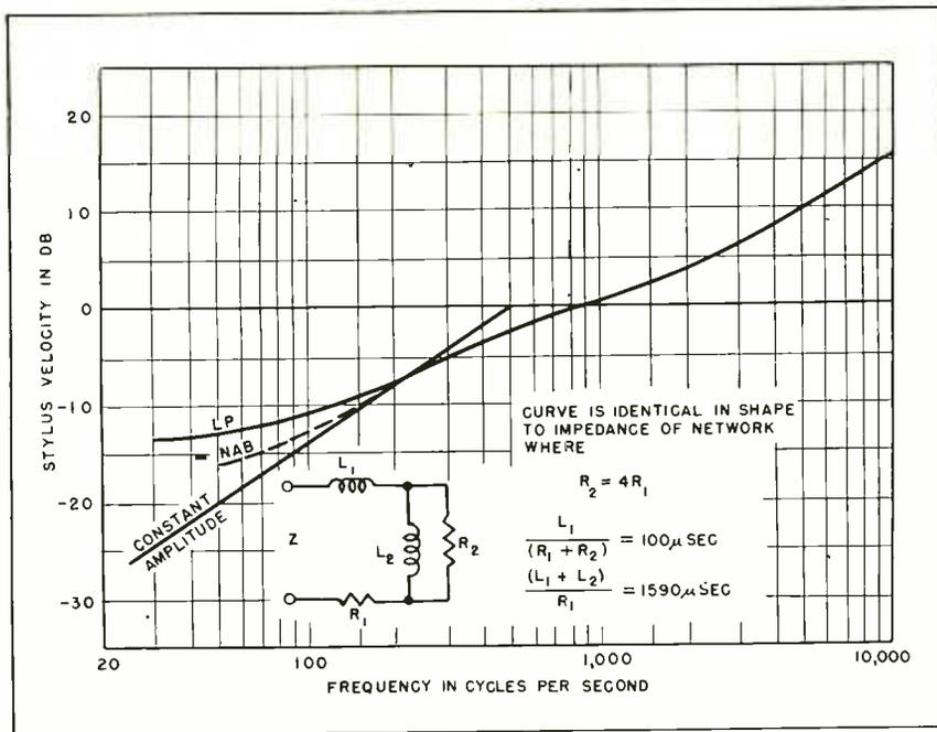
FIG. 1—Characteristics of new long-playing (LP) record, NAB transcription standard, and one having constant amplitude
