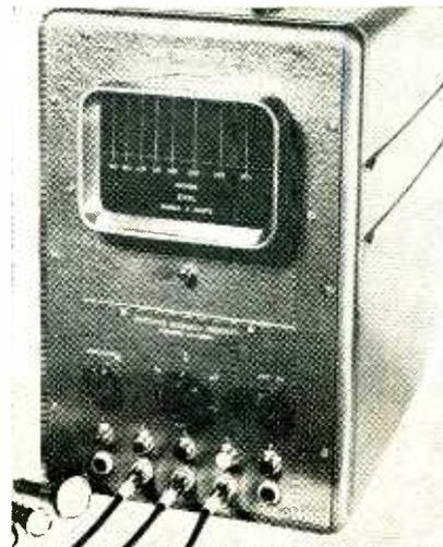
tions in these materials. Using ultrasonic frequencies, the device operates on the basis of thickness vibrations, and gives a cathode-ray presentation of its findings.
