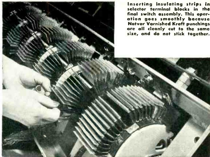
Inserting insulating strips in selector terminal blocks in the final switch assembly. This operation goes smoothly because Natvar Varnished Kraft punchings are all cleanly cut to the same size, and do not stick together.
