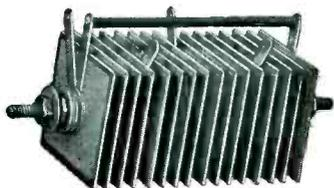
Bradley selenium power rectifiers are rugged and compact. Square plates afford maximum of rating to space factor. Conservatively rated up to thousands of amperes. Shown: SE11W20F, full-wave bridge, rated at 110 volts A.C., 5 amperes D.C.
