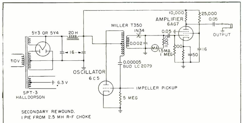
FIG. 2—The capacitance transducer. Plate series capacitor is variable
