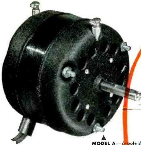
**MODEL A**—6-pole shaded pole induction motor • 60 and 50 cycles • Approx. 1000 R.P.M. full load speed • Size— $4\frac{1}{2}$ " O.D. • Length— $2\frac{3}{4}$ " to  $4\frac{3}{4}$ " depending on variable stack length • Rated at approx. 1/30th h.p. • Comes semi-open or fully enclosed with or without oilers.
