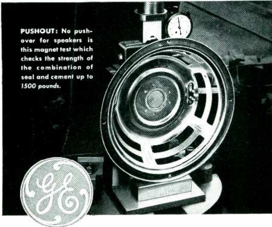
**PUSHOUT:** No push-over for speakers is this magnet test which checks the strength of the combination of seal and cement up to 1500 pounds.
