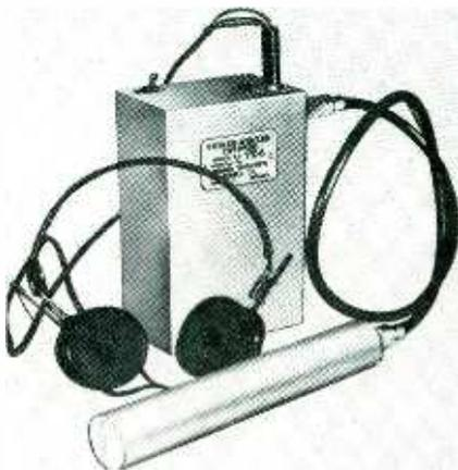
phones. The instrument is sensitive enough to detect radiation in a radium dial watch.
