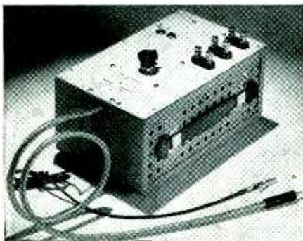
The Phantom Repeater bridges voltmeters and cathode ray oscilloscopes, which have inputs of 1 megohm and 30 mmf, onto signal circuits of 50,000 ohms and higher—such as a pentode amplifier stage with its high resistance plate load—without the loss of voltage and high frequency response which would result if the measur-
