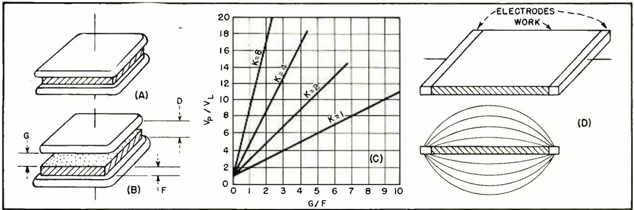
FIG. 1—Heating thin films by making them the dielectric of parallel plate capacitors (A) is difficult if there is an air gap (B) comparable to the thickness of the film, the ratio of applied voltage to load voltage is rising rapidly (C) with gap width. If it were not for excessive leakage (D) the electrodes could be placed at the edge of the film
