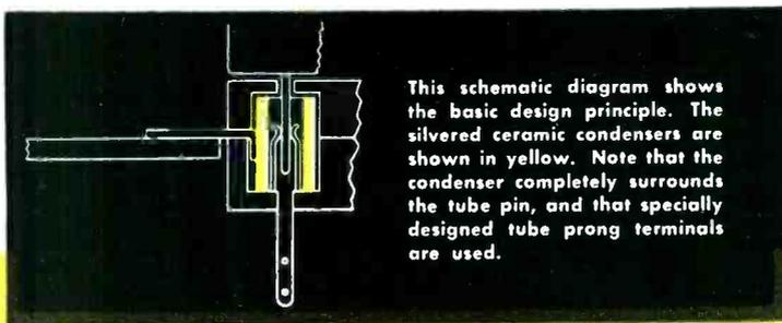
This schematic diagram shows the basic design principle. The silvered ceramic condensers are shown in yellow. Note that the condenser completely surrounds the tube pin, and that specially designed tube prong terminals are used.
