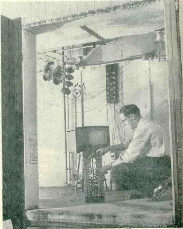
**HOT BOX**—Here receivers and components can be tested or operated for hours at temperatures up to 150 F and humidities up to 100 percent, to simulate ambient conditions encountered in any part of world where electronic equipment is used
