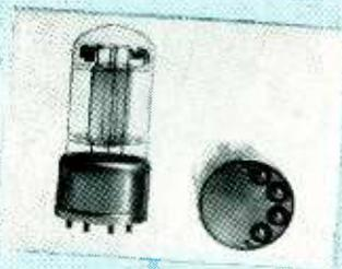
Key to the accuracy of the Western Electric Primary Frequency Standard is a GT-cut crystal, surpassing even the annular cut in the degree to which it nullifies the effect of temperature on frequency. The crystal is suspended by wires inside an evacuated glass envelope. The wire mounting results in an exceptionally rugged crystal unit, practically immune to shock.
