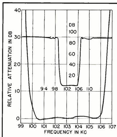
FIG. 15—Attenuation characteristic of a four-section crystal channel filter for 100.1-106 kc
