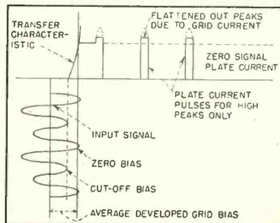
FIG. 5—Discriminator action allowing only input frequency of highest peaks to pass through amplifier
