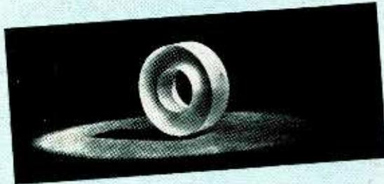
Heart of the crystal clock built 20 years ago at Bell Laboratories was this quartz ring, adjusted to a frequency of 100 kc. With the crystal cut to correct proportions in this annular
