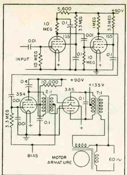
FIG. 7—Experimental circuit of amplifier for portable use
