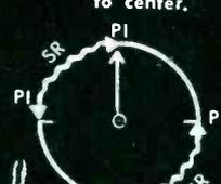
**10** Four position, two positive, spring return from clockwise, counter-clockwise.
