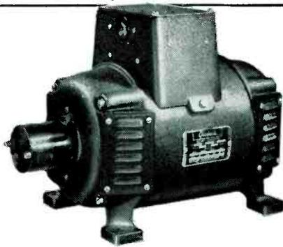
DC to AC Rotary Converters having Automatic Frequency Control are now being offered in all models. Input voltages from 6 to 230 V DC; output: 110 to 1000 VA at 60 cycles, 90 to 800 VA at 50 cycles.
