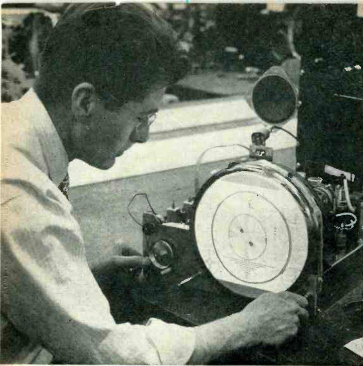
**IT WORKS**—Adjusting horizontal and vertical linearity controls of new table-model television receiver, using video signal and 400-cycle tone obtained from central signal source through coaxial lines. Picture tube is inserted only for alignment and test here, as sets are shipped without the tube
