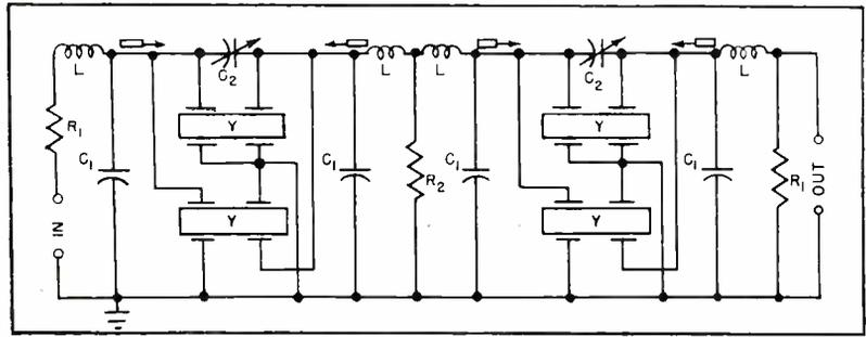
FIG. 12—A double-section 6-kc-channel crystal filter. Capacitors  $C_1$  permit fine adjustment of passband width,  $C_2$  fine adjustment of attenuation peaks,  $L$  are passband widening coils,  $R_1$  are terminating resistors,  $R_2$  are interstage impedance-matching resistors and  $Y$  are  $+5\text{-deg}$  X-cut crystals
