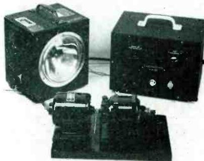
FIG. 2—The SynchroStrob is used with a tachometer and a Sirobotac to observe rotating machinery
