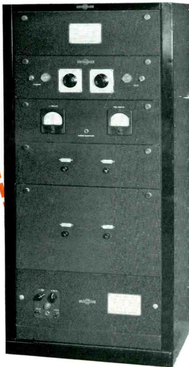
The 51M-2 is a fixed channel crystal controlled dual-superheterodyne receiver, and is highly sensitive and selective. It includes all modern circuit features, such as flat avc, noise limiter, and squelch. Write us for further information.
