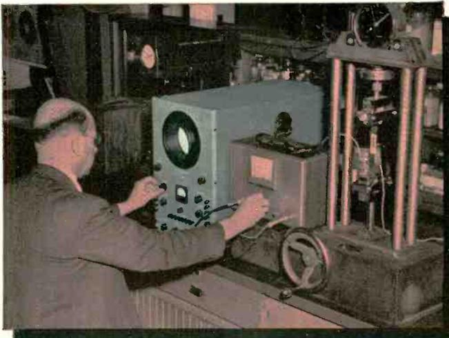
**D-c and low-frequency a-c (WO-27A)**—This oscilloscope also observes a-c and d-c simultaneously. *Frequency range:* 0 (d-c) to 100,000 cycles. Flat to zero cycles. Uses direct-coupled balanced amplifiers. *Timing range:* 1 to 30,000 cycles. Single-sweep and blanking circuits permit observation and photographic recording of one-time, high-speed transients. *Vertical amplifier sensitivity:* 0.084 volt (d-c) per inch. Shown in picture above measuring strain of test specimen in tension.
