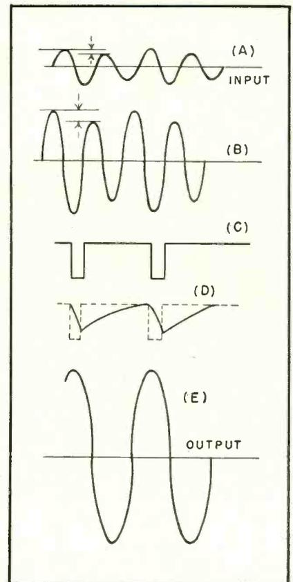
FIG. 3—Bridge signals of slight unbalance indication passing through the discriminator amplifier to be discriminated into a signal of complete unbalance
