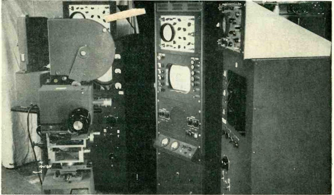
FIG. 1—General view of transcription equipment. Two units are used to provide uninterrupted recording of lengthy programs
