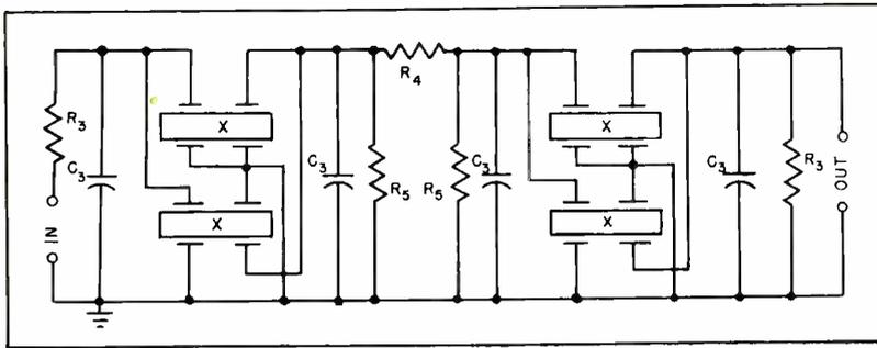
FIG. 13—A double-section 20-cycle crystal filter. Capacitors  $C_3$  control passband width,  $R_3$  are terminating resistors,  $R_4$  and  $R_5$  are interstage impedance-matching resistors and  $X$  are +5-deg X-cut crystals. These components are shown in the illustrations on this page
