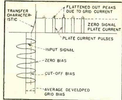
FIG. 4—Discriminator action allowing input frequency to pass through amplifier
