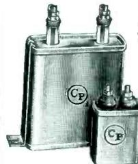
Plasticon A element, mineral oil impregnated in sturdy lead coated steel containers. Smaller, lighter and more economical than paper capacitors. Temperature range — 40° C to + 105° C. Type AOC rectangular; Type AOC6 flattened oval. Type ASC and ASCO (not listed) have Plasticon A element, silicone impregnated. Same dimensions as corresponding AO types. Temperature range — 60° C to + 125° C; greater capacitance stability. Prices on application.
