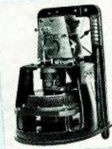
In the clock mechanism, a 1,000-cycle synchronous motor, driven by the output of the sub-multiple generators, was geared to the clock hands. Accuracy of this clock in 1928 was within 1 part in  $10^6$ . Accuracy of its present-day successor is of the order of 1 part in  $10^8$ —an advance made possible by continuing research.
