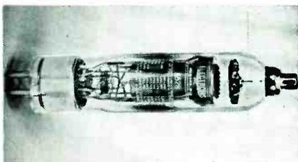
inverter applications which must operate at up to 800 cycles. It features 60 second heating time, a peak inverse voltage of 500 v, 6.4 amperes steady d-c current, and 77 amperes peak.
