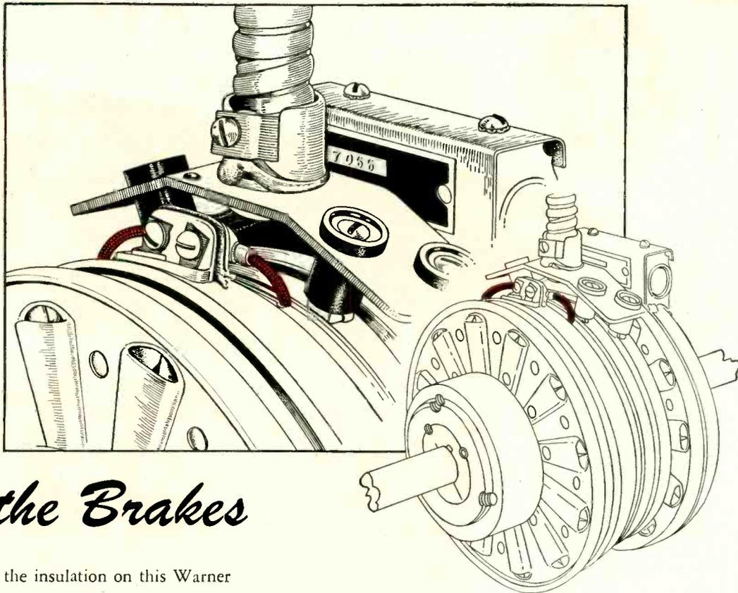
Take a close look at the insulation on this Warner "ICB" Electric Clutch-Brake. The wire that conveys the current from the collector ring to the magnet requires an insulation that is heat resistant to 300° F. at 110 v.
