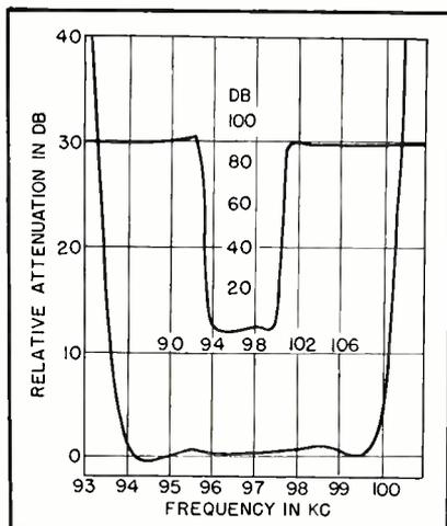
FIG. 14—Attenuation characteristic of a four-section crystal channel filter for 94-99.9 kc
