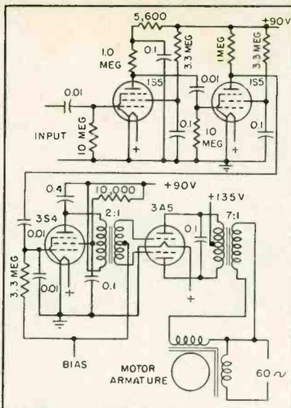
FIG. 7—Experimental circuit of amplifier for portable use
