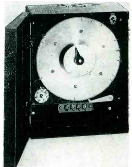
ing, can make a single circuit contact at any 5-minute interval in 24 hours and repeat each day. Model TS incorporates a holding circuit which it closes on the first impulse and opens on the succeeding impulse.
