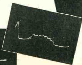
Trailing edge of horizontal synchronizing pulse.
