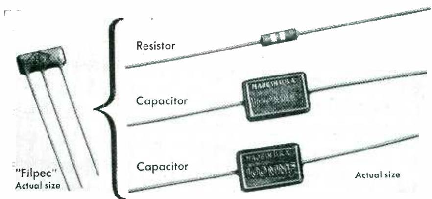
**4** Centralab's *Filpec* is designed for use as a balanced diode lead filter, combines up to three major components into one tiny filter unit, lighter and smaller than one ordinary capacitor. Capacitor values available from 50 to 200 mmf. Resistor values from 5 ohms to 5 megohms. For complete information write for Bulletin 976.
