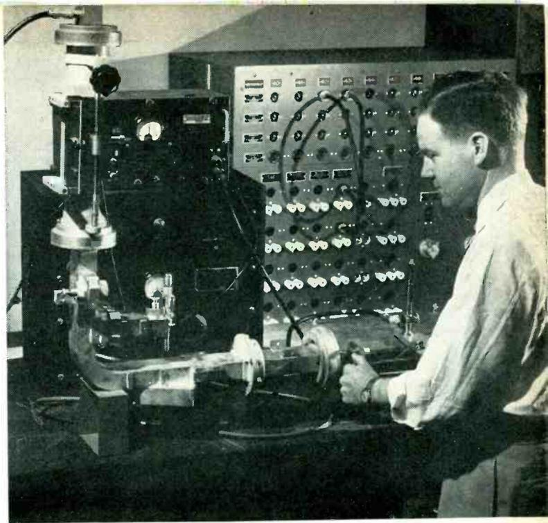
**PLAYING WITH PLUMBING**—Typical workbench scene in Government Division lab assigned to microwave development problems. Jumpers can be inserted in power panel at rear to feed any desired type of power to any particular bench
