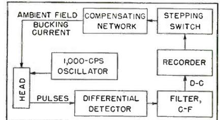
FIG. 2—Block diagram shows how pulses from sensing element are converted into direct current and fed to the recorder, and how a balancing current is obtained to restrict the range over with the head must operate
