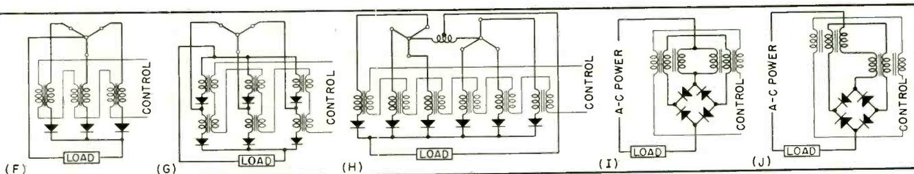
(D) or a full-wave circuit (E). These elements can be grouped (F), (G) and (H) for three-phase operation. Further elaboration of the single-phase circuits to obtain continuous rectified feedback current (I) and (J) results in the self-saturating magnetic amplifier
