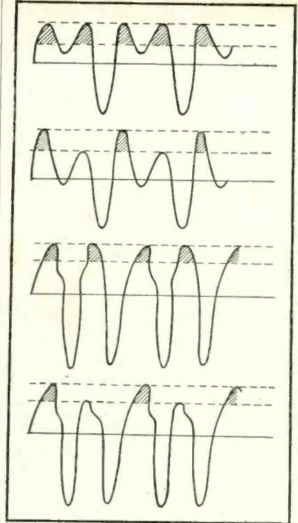
FIG. 6—Different waveforms react the same to discrimination producing almost identical pulses
