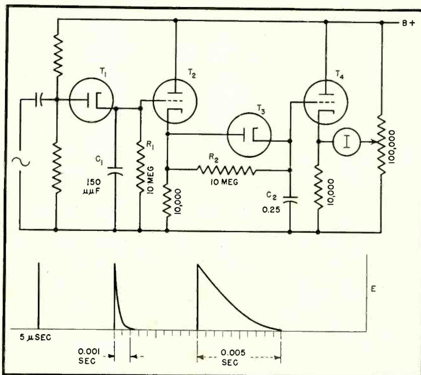
FIG. 1—Circuit and waveforms of pulse stretchers and impedance step-down repeaters
