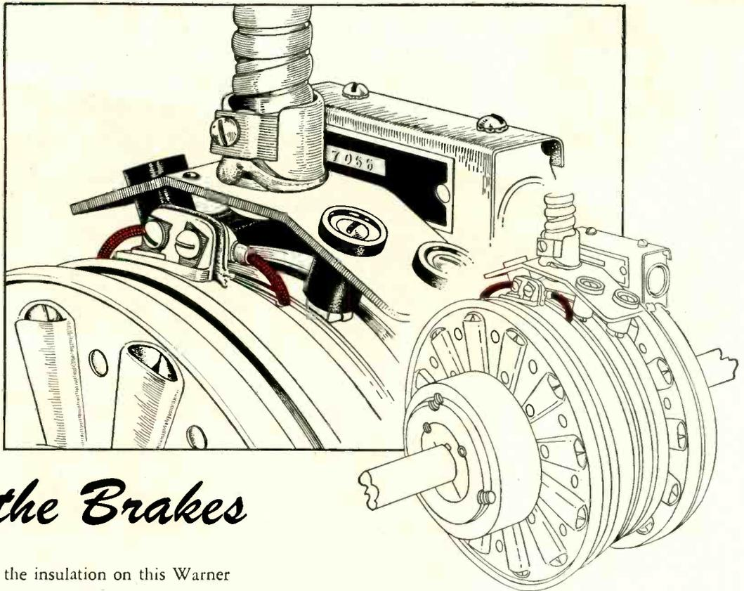
Take a close look at the insulation on this Warner "ICB" Electric Clutch-Brake. The wire that conveys the current from the collector ring to the magnet requires an insulation that is heat resistant to 300° F. at 110 v.
