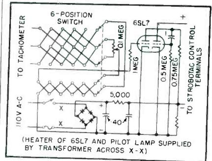
FIG. 1—Circuit diagram of synchronizer that provides phase adjustment throughout 360 degrees
