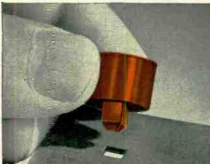
Square shank of nylon nut, molded as one unit but consisting of four separate prong-shaped legs, is inserted in square hole of supporting plate. Since nylon itself is an insulator, the nut does not require a grommet. And Du Pont nylon remains stable at temperatures ranging from  $-60^{\circ}\text{F.}$  to  $200^{\circ}\text{F.}$
