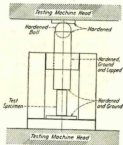
Figure 1 — Typical design of tool for making compressive strength tests.
