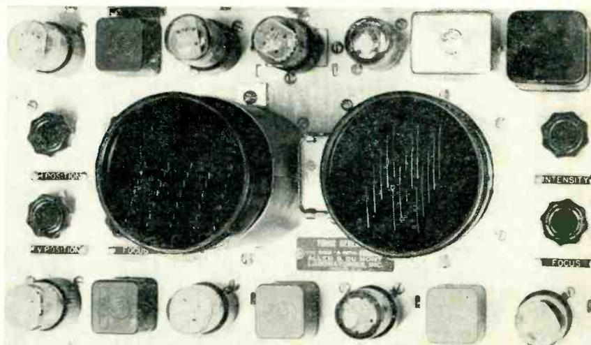
FIG. 3—Presentation of count-down frequencies on cathode-ray monitors
