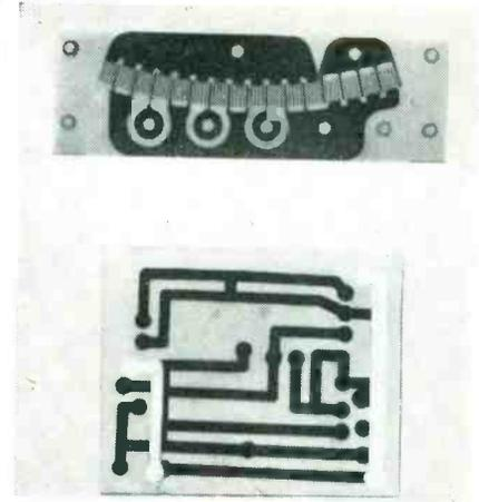
A commutator formed in ceramic and a circuit formed on top and bottom of a thin, transparent plastic sheet
