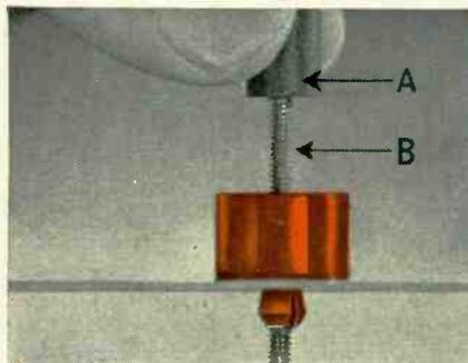
Tuning slug (A) and screw (B) are rotated, impressing thread shape of screw into nylon shank. Prong-shaped legs of shank flare outward, securing nut to plate. Nylon develops torque on screw thread to hold slug in adjusted position, despite vibration and variations in plate thickness and size of hole.
