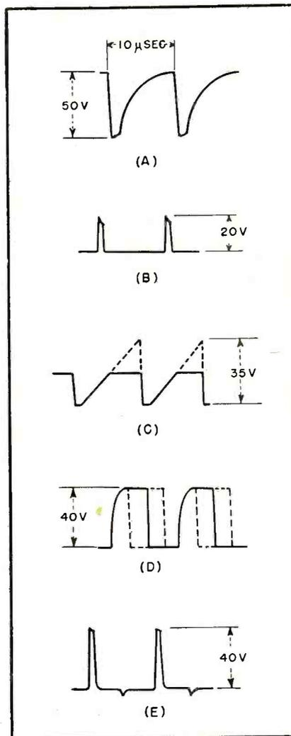
FIG. 2—Waveforms, oscillator to output
