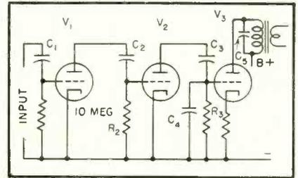
FIG. 2—Essential portions of amplitude discriminator amplifier showing cascaded discriminators and pulse reshap
