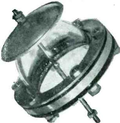
Clear glass, Corning Glass Works No. 67076. Type C Compromises flanged bowl 4<sup>3</sup>/<sub>8</sub>" h x 6-15/16 O.D. at base. Center lead-in pin 3/8" dia. x 1 1/2" long. Mounts by means of 5 studs through mounting flange. Overall dia. 8 3/4" S.C. Stock No. 3G-1830-67076.1 @ \$6.00
