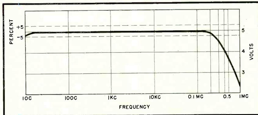
FIG. 3—Wide-band operation is indicated by voltage-versus-frequency characteristic
