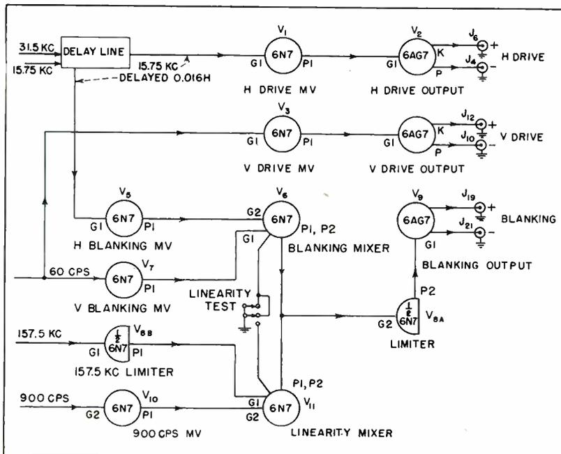
FIG. 7—Functions of stages in the blanking-driving unit
