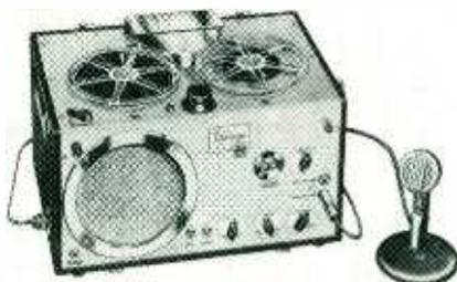
wind. It is equipped with an 8-inch speaker and an oversize motor with high inertia flywheel. Motor drive and capstan operate continuously so that tape starts and stops instantaneously.
