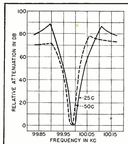
FIG. 16—Attenuation-frequency characteristic and effect of temperature change on the 100-kc 2-section carrier filter
