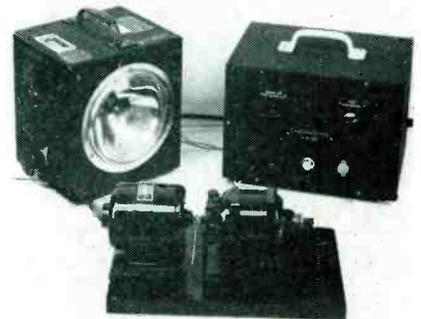
FIG. 2—The SynchroStrob is used with a tachometer and a Sirobotac to observe rotating machinery
