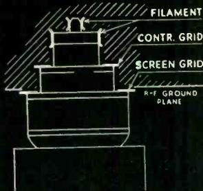
Sketch shows how easily the GL-7D21 can be plugged into a coaxial socket. Ring-seal design also provides ample contact surface for all terminals.
