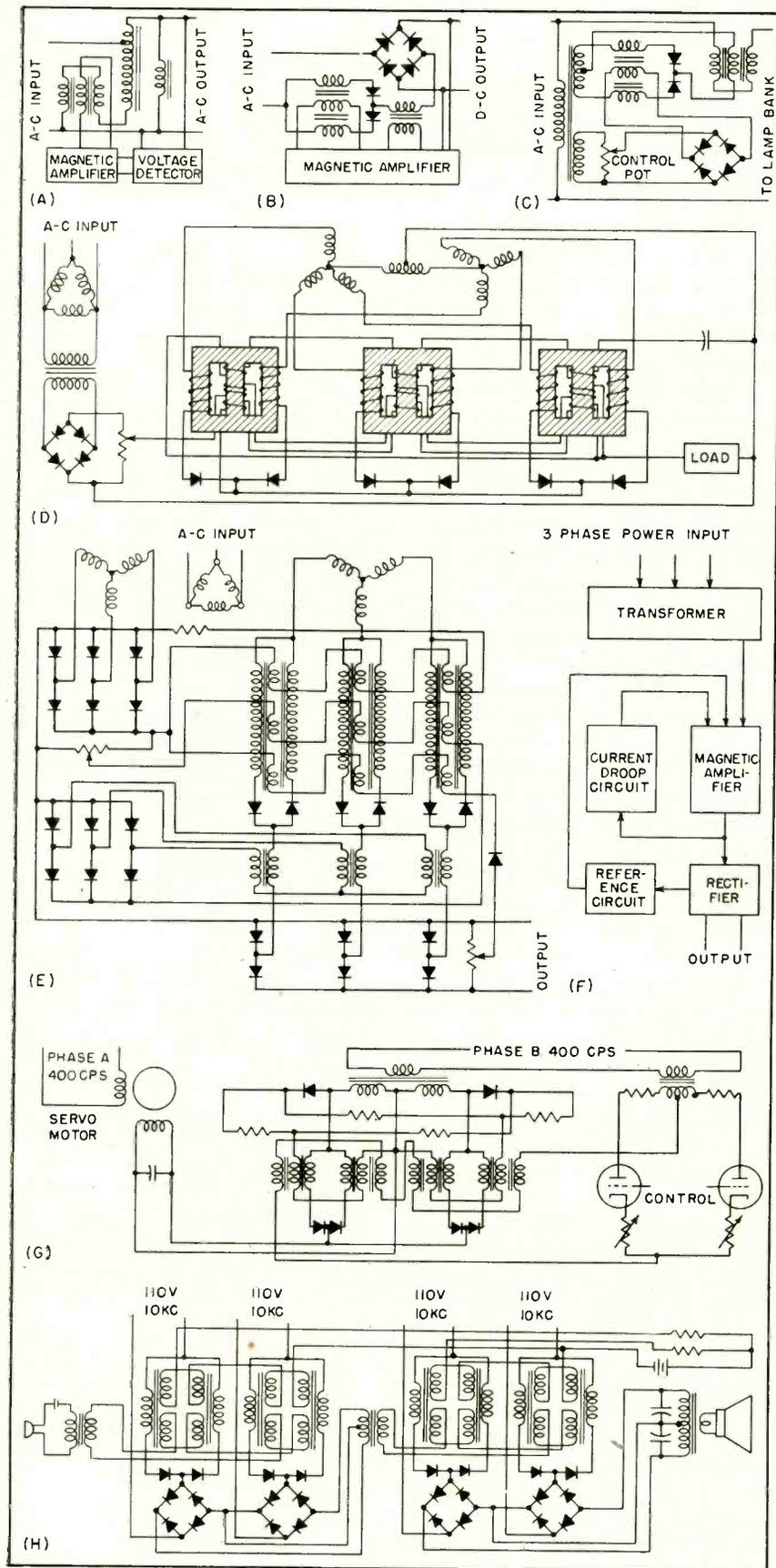
FIG. 4—Presaturated reactors and magnetic amplifiers have been used in various applications, as these simplified diagrams show: (A) line voltage regulator, (B) automatic battery charger, (C) theater lighting control, (D) constant potential rectifier, (E) welding rectifier, also shown in block form (F), (G) servo motor power amplifier, and (H) two-stage audio amplifier
