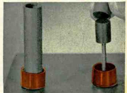
Coil form fits snugly in nylon nut... firmly gripped externally by six thin, flexible "fingers" on the inside wall of the support nut. The hollow tube is held securely in place by pressure of the nylon "fingers," although wall thicknesses of the tube may often vary as much as  $1/32$  of an inch.
