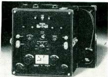
of the test voltage is 60 cycles. A feature of the bridge is the zero-compensating circuit that balances out the initial capacitance and dissipation factor at zero setting of the dials.
