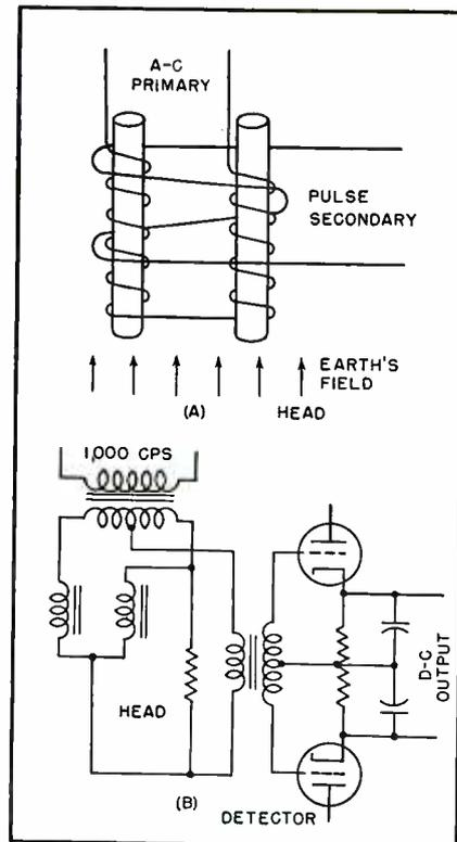
FIG. 1—Magnetometer head depends for its action on the change in inductance as the core becomes saturated (A). The pulses produced by the head are converted to direct current and combined to give a signal proportional to the magnetic field
