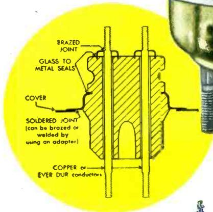
Can be welded, brazed, or soldered to case, forming a strong, permanent, hermetic seal that eliminates moisture problems and often permits more compact, light-weight design.
