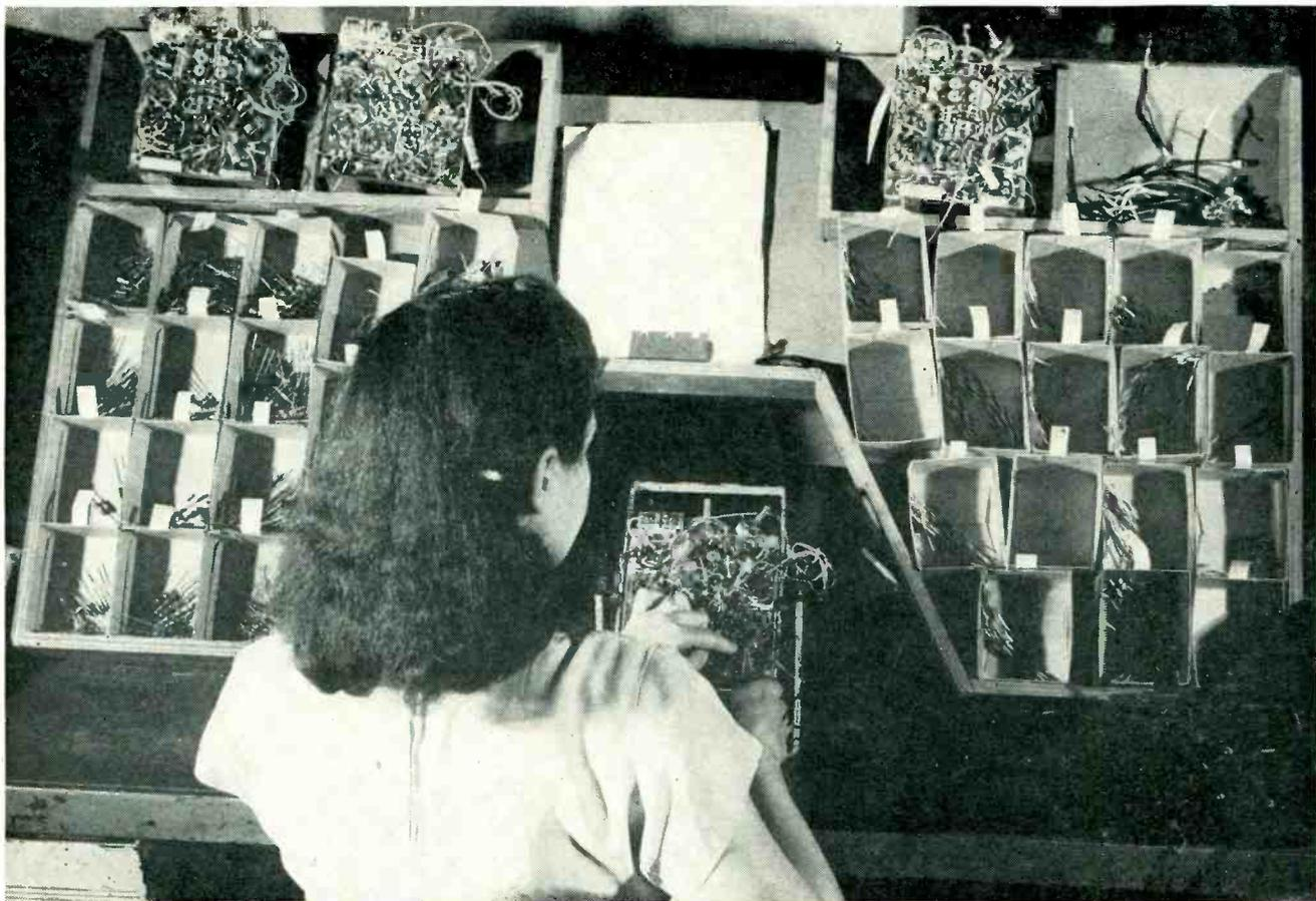
**ORGAN-TYPE CONSOLE**—For small production runs in Transmitter Building, long time cycles are most economical. Here one operator
