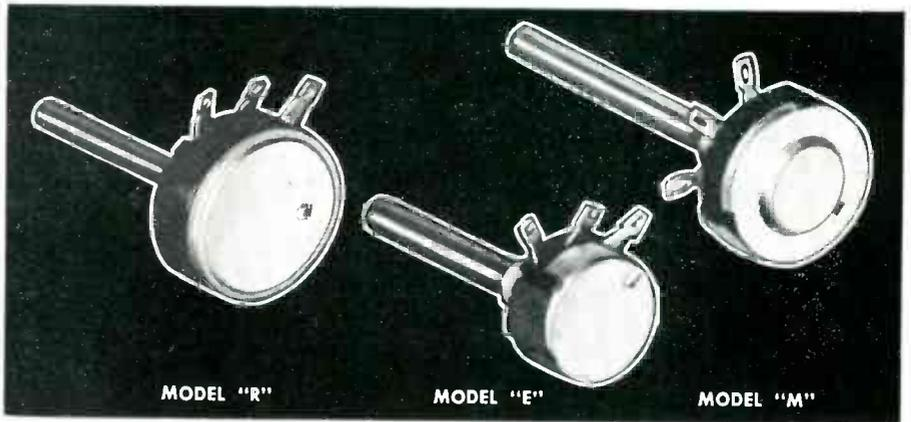
**5** Let Centralab's complete *Radiohm* line take care of your special needs. Wide range of variations: *Model "R"*—wire wound, 3 watts; or composition type, 1 watt. *Model "E"*—composition type, 1/4 watt. Direct contact, 6 resistance tapers. *Model "M"*—composition type, 1/2 watt. For complete information, write for Bulletin 697.
