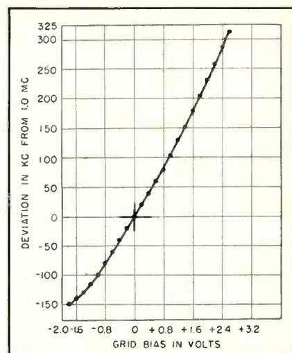
FIG. 11—Frequency deviation of the one-megacycle oscillator
