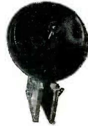
AS-217A/APG 15B. 12 Cin dipole and 13 inch Parabola housed in weatherproof Radome 16" diam. 24 v. DC spinner motor for conic scan. Stock #SA-95. Shipping wt. 70 lbs.
