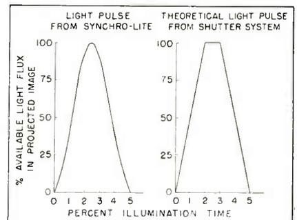
FIG. 6—Comparison of light pulse from Synchro-Lite with theoretical light pulse from shutter system having 2-percent opening and closing times
