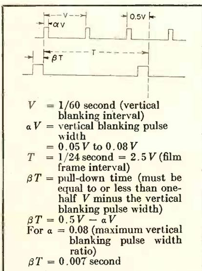
FIG. 1—Film pull-down and vertical blanking periods
