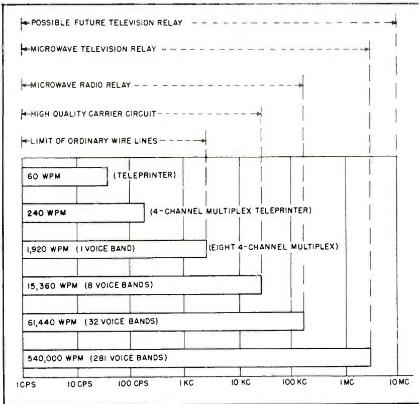
FIG. 2—Representative communications methods, showing their capacities and required bandwidths. Ultrafax demonstration system using 4-mc bandwidth shown at bottom
