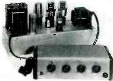
20,000 cycles. Intermodulation and harmonic distortion are negligible. A new circuit permits the amplifier to handle power peaks considerably higher than its 10-watt rating.
