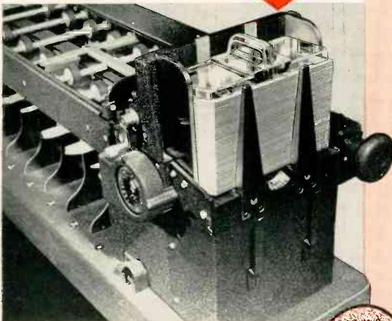
Above illustration shows an IBM Electric Punched Card Sorting Machine with cards stacked for automatic sorting. Note plastic Card Weight in its steadying position on top of stack.
