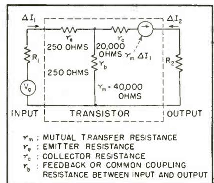
FIG. 2—The transistor can be represented by an equivalent resistance network at low frequencies. A typical input load would be 10,000 ohms, a typical input resistance is 500 ohms
