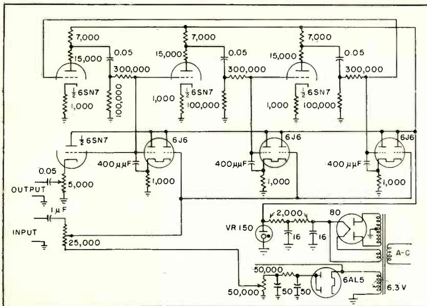
FIG. 12—Circuit of frequency-modulated audio oscillator
