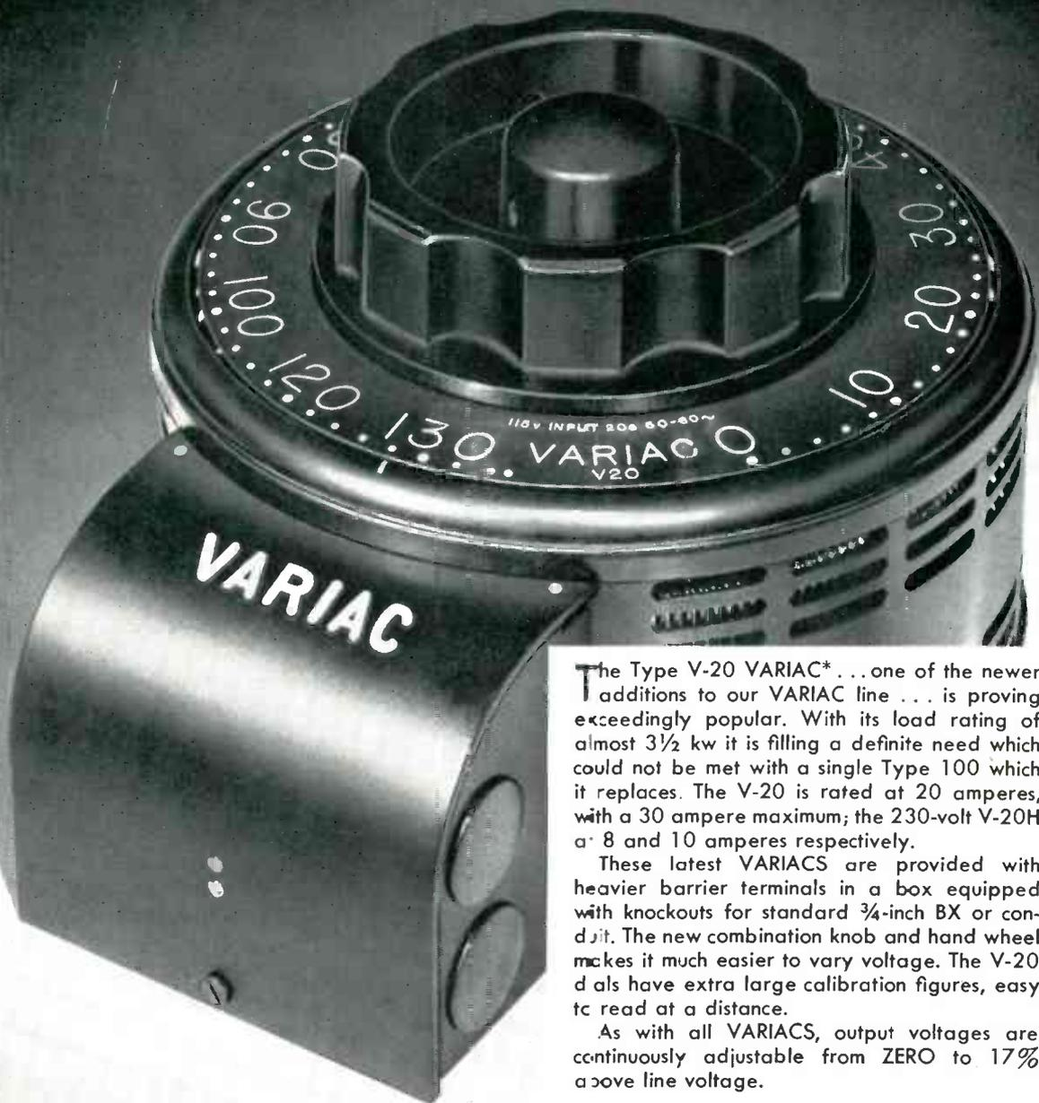
The Type V-20 VARIAC\* . . . one of the newer additions to our VARIAC line . . . is proving exceedingly popular. With its load rating of almost 3½ kw it is filling a definite need which could not be met with a single Type 100 which it replaces. The V-20 is rated at 20 amperes, with a 30 ampere maximum; the 230-volt V-20H at 8 and 10 amperes respectively.
