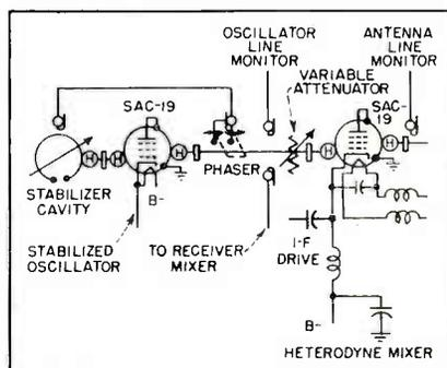
FIG. 4—Schematic of r-f head of Philco 6,000-mc television relay equipment
