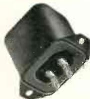
Two precision-built chokes with inductance values of .8 and 2.4 henrys respectively—accurate to within  $\pm 5\%$  with up to 15 ma d-c. Units have a minimum Q of 20. Exceptionally compact,  $1\frac{1}{16}'' \times 2\frac{3}{8}'' \times 1\frac{1}{16}''$ .
