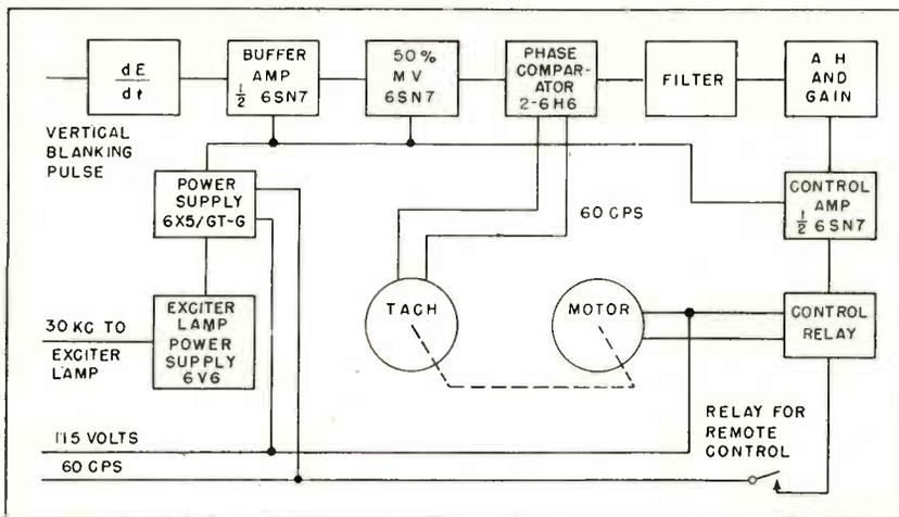
FIG. 3—Speed control amplifier for the projector
