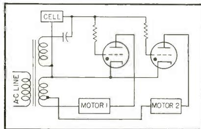
FIG. 3—Suggested circuit for operating a series of motors from different light levels
