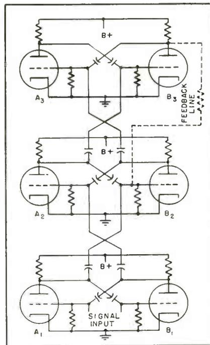
FIG. 2—Multivibrators in series. Dotted portion shows feedback network for non-integral frequency division
