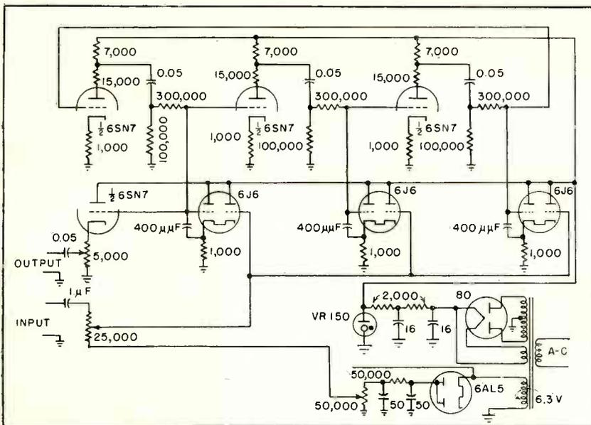
FIG. 12—Circuit of frequency-modulated audio oscillator
