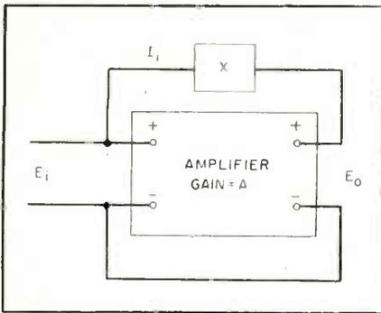
FIG. 1—Functional diagram of variable reactance
