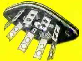
Laminated Noval (plain) with grip pin type contact, 1-1/8" mtg. center
