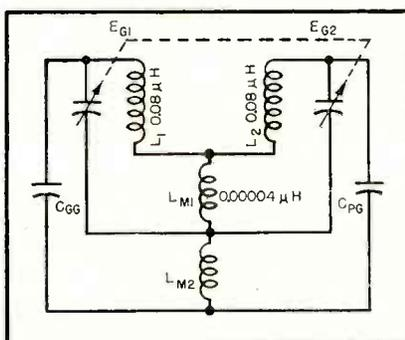
FIG. 8—Circuit to indicate capacitor-shaft coupling
