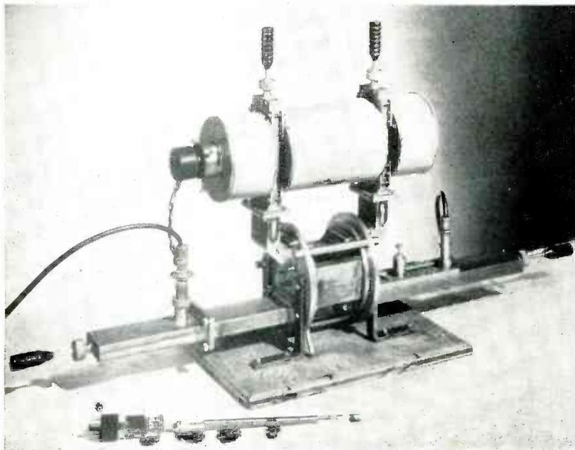
Traveling-wave amplifier tube in foreground is operated in waveguide circuit to give a gain from 20 to 30 db within plus or minus 1.5 db from 6.0 to 8.3 cm
