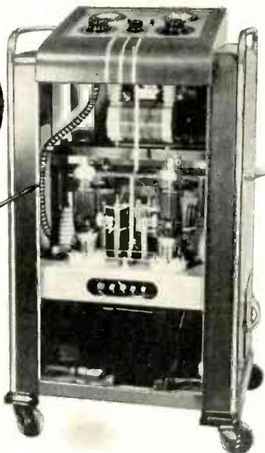
"This diathermy unit is a good example. A variable element in the circuit is mounted down in back. It had to be placed there to get optimum circuit efficiency and to simplify wiring. But that was no place for the control knob—which, of course, had to be up where it was easy to get at. Nothing to it. With an S.S.White remote control flexible shaft it was a simple matter to put the control where it was wanted.
