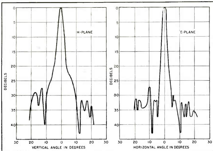
FIG. 2—Vertical and horizontal antenna patterns of 6,000-mc television relay antennas
