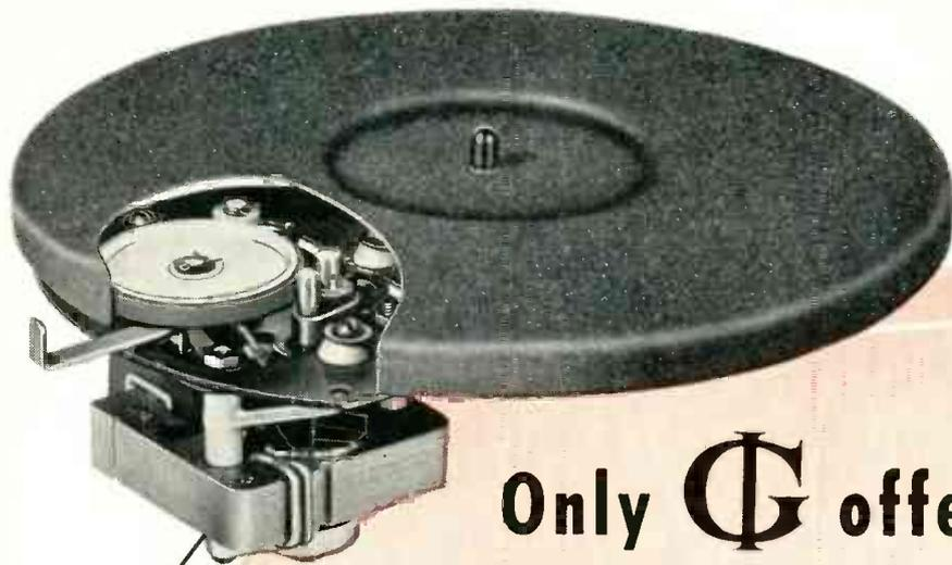
MODEL DM—Compact low cost 2 pole, shaded pole motor designed for portables, table models and other instruments in which space is an important factor. Simple speed change mechanism incorporates a special long-lasting molded neoprene belt.
