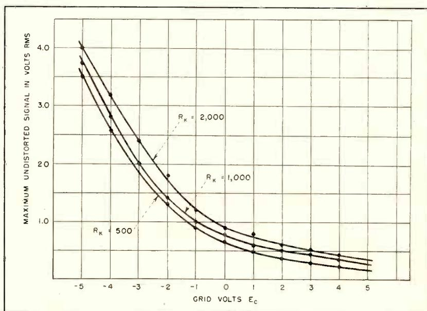
FIG. 8—Distortion level for the three values of cathode resistors
