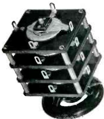
multipoint devices for commercial, industrial, and laboratory use. They are available from 2-contact single-deck types up to 24-point, six-deck models. Maximum load is about 40 amperes, and resistance is constant over long periods.
