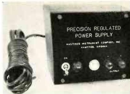
5 to 30 milliamperes. Regulation within plus or minus 0.1 percent for input line voltages from 75 to 135 volts a-c at frequencies from 50 to 400 cycles is obtainable. Output ripple is better than 0.01 percent.
