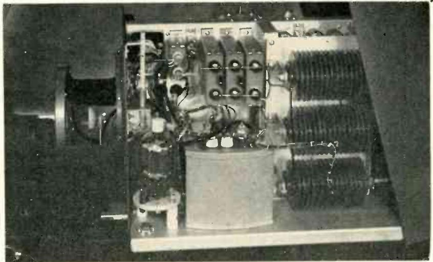
Internal view of Synchro-Lite chassis showing the high-voltage pulser and the selenium rectifiers
