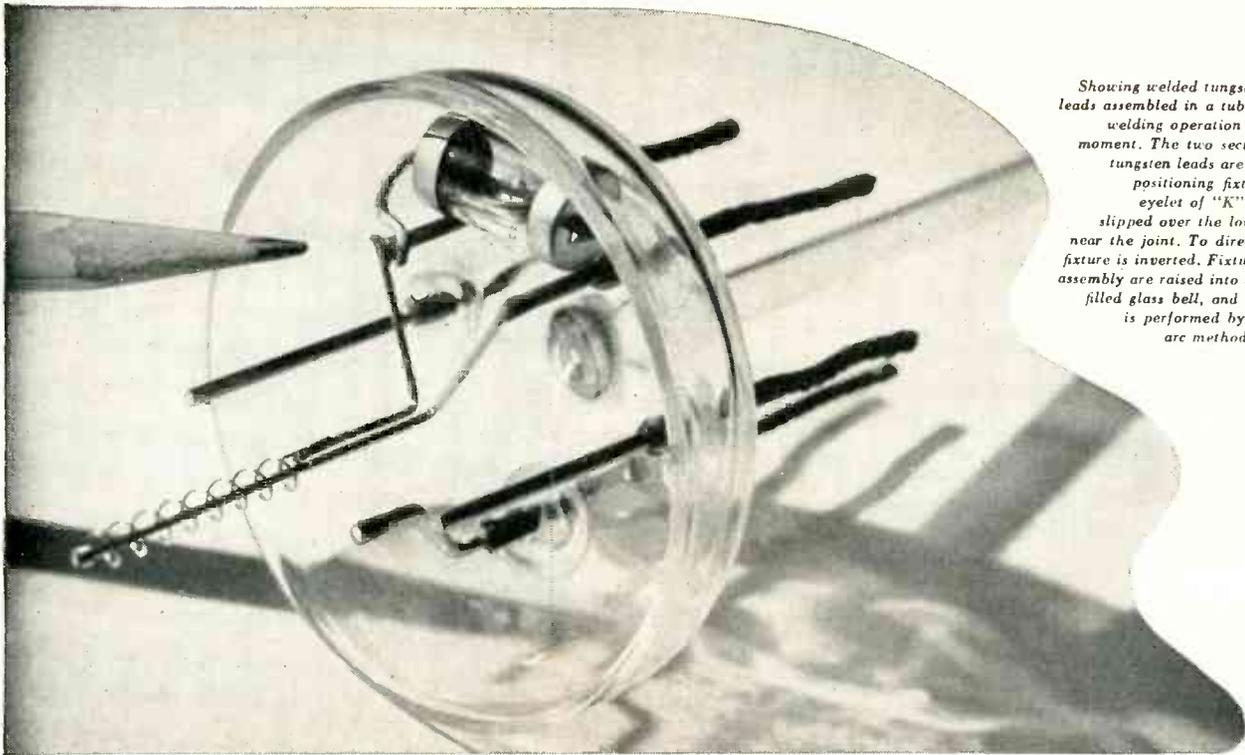
Showing welded tungsten filament leads assembled in a tube base. The welding operation takes but a moment. The two sections of the tungsten leads are placed in a positioning fixture. A tiny eyelet of "K" MONEL is slipped over the lower section, near the joint. To direct flow, the fixture and lead assembly are raised into a hydrogen-filled glass bell, and the welding is performed by the carbon arc method.
