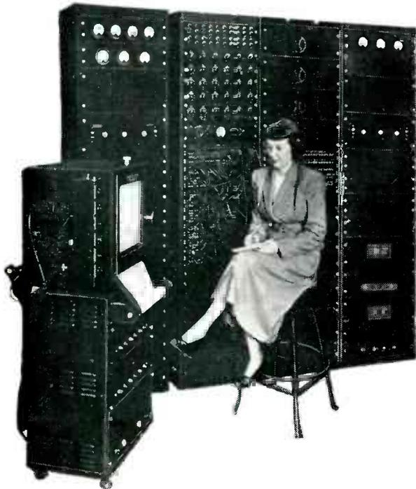
**The Reeves Electronic Analog Computer**, known in industry as REAC, is the first standard office size electronic "brain". This machine makes possible the rapid dynamic analysis of high order linear and non-linear differential equations, doing in a few hours computations formerly taking thousands of man-hours.
