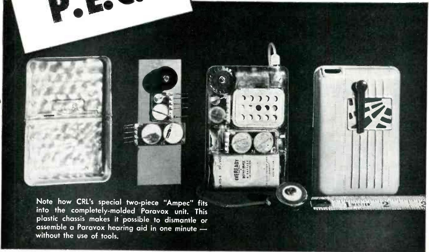
Note how CRL's special two-piece "Ampec" fits into the completely-molded Paravox unit. This plastic chassis makes it possible to dismantle or assemble a Paravox hearing aid in one minute — without the use of tools.
