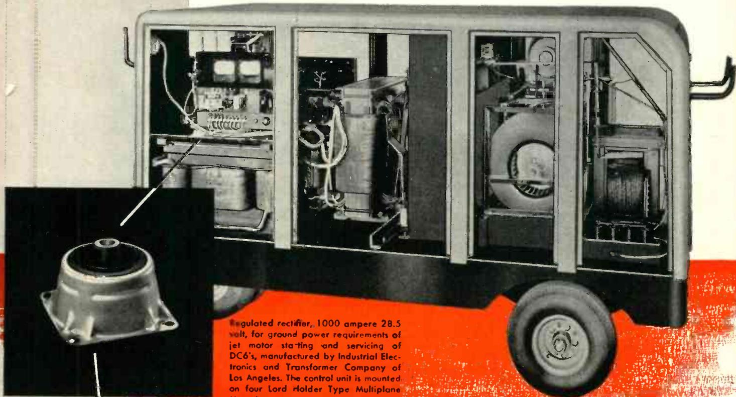
Regulated rectifier, 1000 ampere 28.5 volt, for ground power requirements of jet motor starting and servicing of DC's, manufactured by Industrial Electronics and Transformer Company of Los Angeles. The control unit is mounted on four Lord Holder Type Multiplane Mountings.
