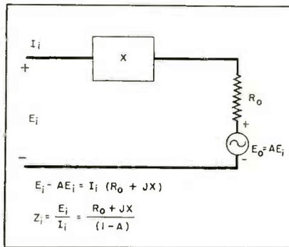
FIG. 2—Equivalent circuit of Fig. 1 for analysis
