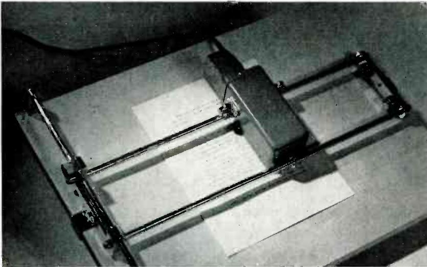
Photoelectric reading head analyzes letters into characteristic pulse patterns
