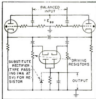
FIG. 2—By adjusting frequency meter circuit so that it has a constant-current output to a metallic rectifier, it is logarithmic
