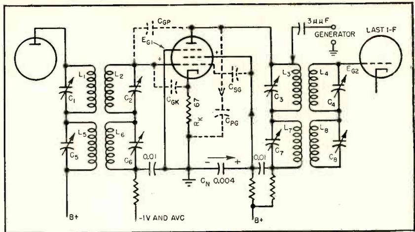
FIG. 5—Representative a-m and i-f intermediate-frequency stage with notations for discussion of regenerative effects
