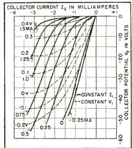
FIG. 1—Typical operating point on the static transfer characteristics of a transistor is at a few milliamperes reverse current in the collector and about one milliamperes forward current in the emitter
