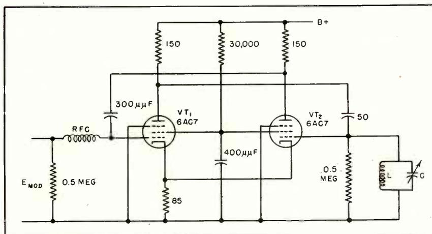
FIG. 10—One-megacycle f-m oscillator using a two-stage amplifier as a variable reactance
