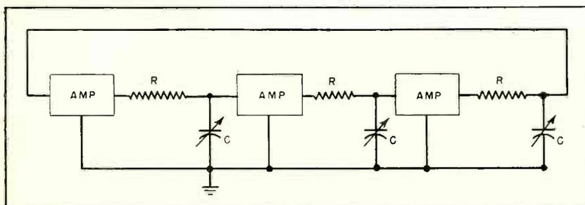
FIG. 13—Block diagram of f-m audio oscillator
