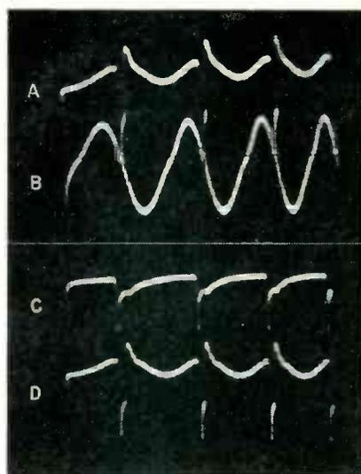
FIG. 5—Pulse transmission through the locked oscillator. Waveform A is the pulse input and oscillator voltage drop across the input resistor, showing  $i_{osc}$  in phase with the pulses. Waveform B is grid voltage lagging 90 degrees behind the pulse fundamental. Waveform C is the output from the discharge tube and D the signal input, showing that the discharge is ahead of the sync pulse thereby saving time for retrace
