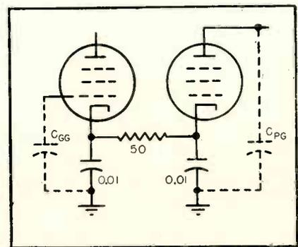
FIG. 6—B-minus decoupling circuit
