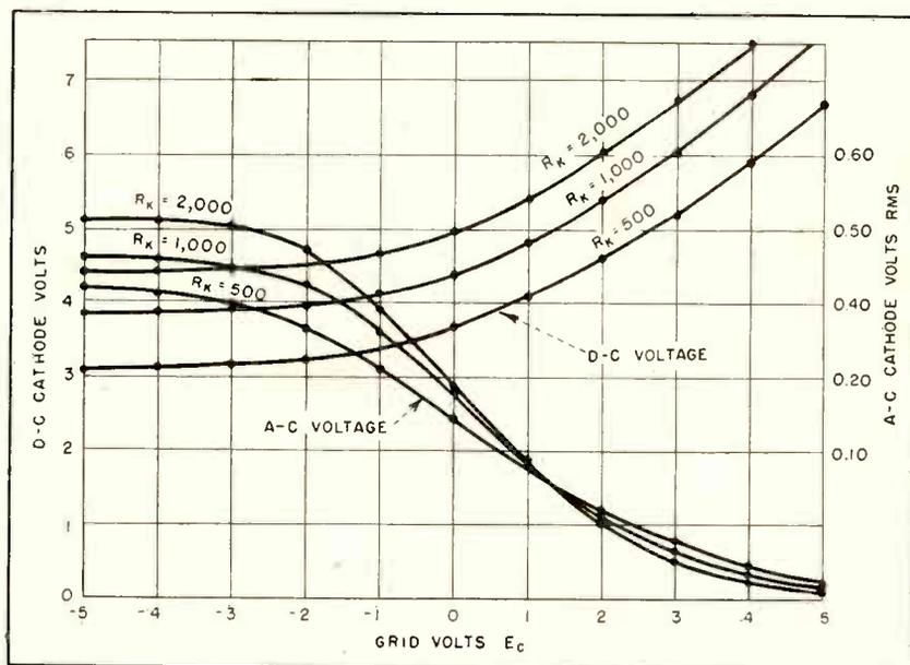
FIG. 7—Increasing the values of cathode resistor provides higher gain
