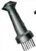
★ Star Miniature Socket Wiring Plugs for accurate alignment of miniature socket contacts during wiring. Precision cast of zinc base alloy—pins of stainless steel. #JE-9 (9 pin); #JE-10 (7 pin).
