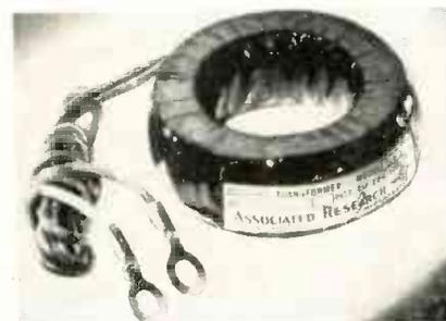
phase angle and ratio error. Designed for 5-volt-ampere burden they are provided with 2-foot secondary leads which may be connected directly to the instrument. The units are insulated for 4,500 volts a-c and can be used on 25 to 133 cycles.
