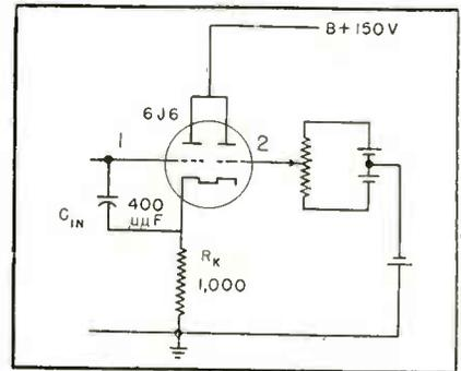
FIG. 3—Cathode-follower reactance-tube circuit
