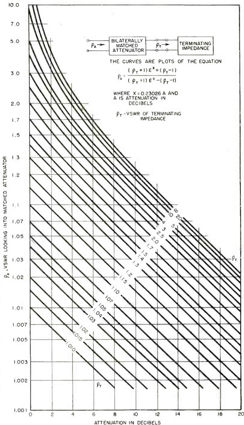
**A**TENUATORS are often used in circuits to isolate changes of impedance from impedance-sensitive devices such as klystron oscillators. Also, attenuators are occasionally used in transmission lines to reduce the voltage standing-wave ratio.
