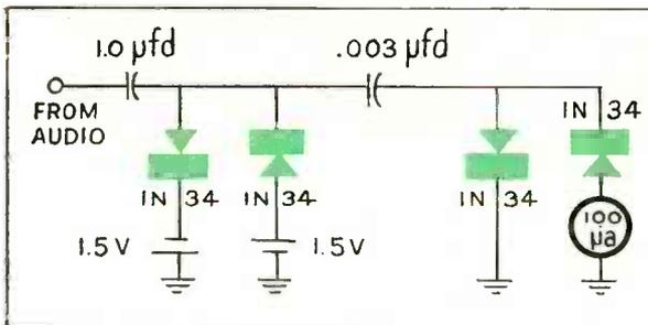
IN THIS PORTION OF THE CIRCUIT, the two 1N34's at the left are used as limiters. They are connected across the audio bus, but are biased so as to pass  $\pm 1.5$  volts of audio. Voltages above this level are clipped off by the action of the diodes. The two 1N34's at the right are used in a full wave counter circuit, and provide a d-c output proportional to the frequency input.
