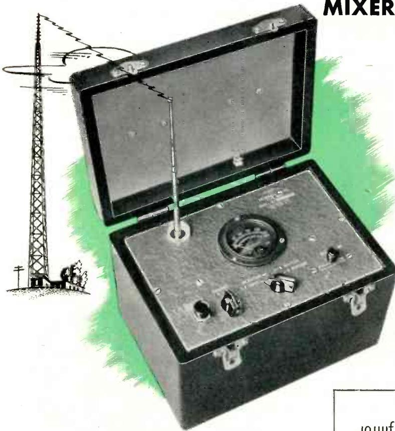
**5 Germanium Diodes make readings independent of battery voltage**
