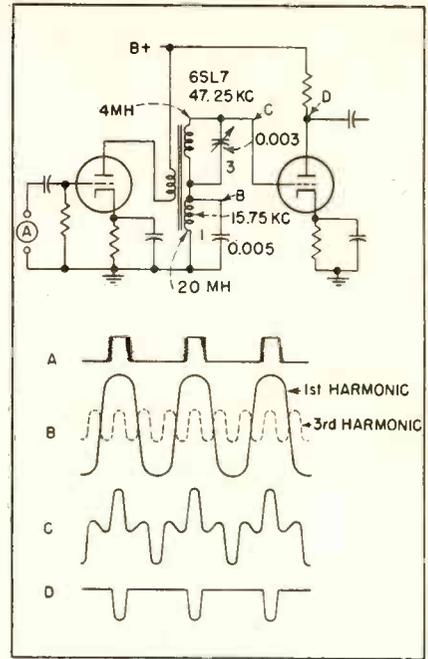
FIG. 2—Harmonic resonator circuit
