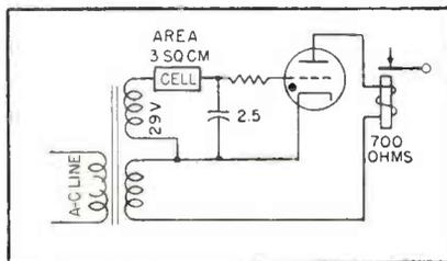
FIG. 1—Typical circuit for photocell and thyatron that supplies 88 milliwatts to operate the relay
