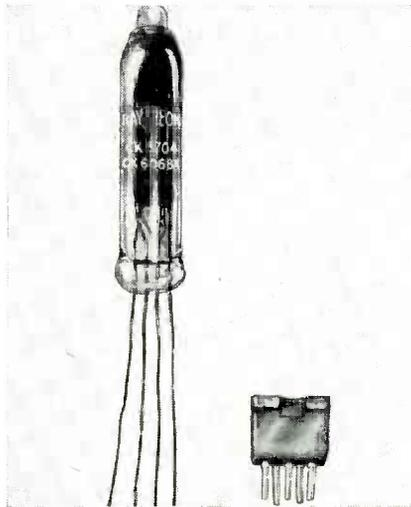
miniature diode with characteristics similar to those of one-half of a 6AL5. Resonant frequency is over 1,200 mc. The tube has a 6.3-volt 150-ma heater and is intended for applications up to a few hundred megacycles where very small size is important.
