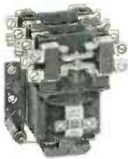
Bulletin 700 Universal Relays are available in 10-amp rating with 2, 4, 6, and 8 poles. Two contact banks permit quick changes from normally open to normally closed contacts. The double-break, silver-alloy contacts require no maintenance. There are no pins, pivots, bearings, or hinges to bind, stick, or corrode.
