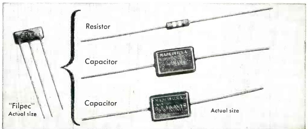
**3** Centralab's *Filpec* is designed for use as a balanced diode lead filter, combines up to three major components into one tiny unit, lighter and smaller than one ordinary capacitor. Capacitor values available from 50 to 200 mmf. Resistor values from 5 ohms to 5 megohms. For complete information, write for Bulletin 42-9.
