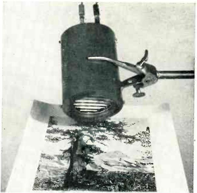
Printing industry setup for measuring amount of ink on a sheet of paper. As developed by Sun Chemical Corp., New York City, this technique involves adsorbing a small amount of a radioisotope on the ink pigment and using a Geiger counter to measure amount of activity that is present
