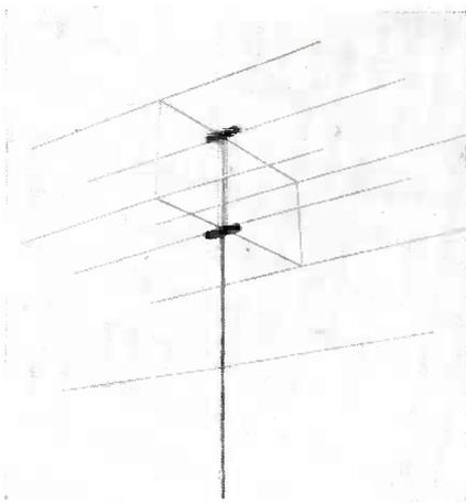
been designed to increase f-m and television reception in fringe areas. There are two antennas, two directors, and three reflectors that make up the array.
