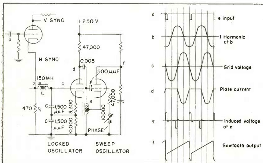
FIG. 4—Circuit and waveforms of locked oscillator
