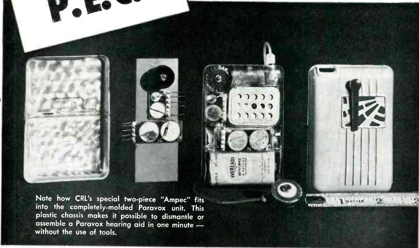
Note how CRL's special two-piece "Ampec" fits into the completely-molded Paravox unit. This plastic chassis makes it possible to dismantle or assemble a Paravox hearing aid in one minute — without the use of tools.
