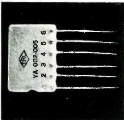
**2** Like all CRL *Couplates*, pentode (above) consists of plate lead and grid resistors, plate by-pass and coupling capacitors. See Bulletins 999, 42-6.
