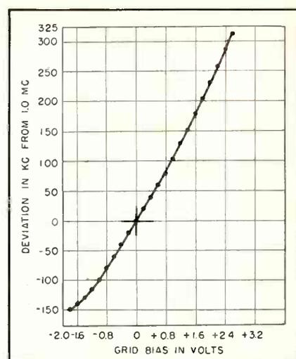
FIG. 11—Frequency deviation of the one-megacycle oscillator
