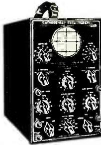
3" CRT operates at accelerating potential of 1100 V—brilliant well-defined trace. Vert amp voltage gain approx 43, horiz amp voltage gain approx 55, Freq. range vert. & hor. amp both uniform ±3 DB from 5-100,000 CPS Input impedance 1 megohm vert., .8 megohm hor. Operates 115 V, 40-60 cycles.
