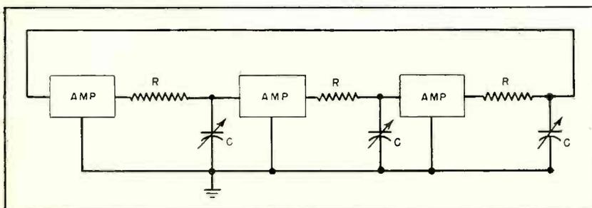
FIG. 13—Block diagram of f-m audio oscillator
