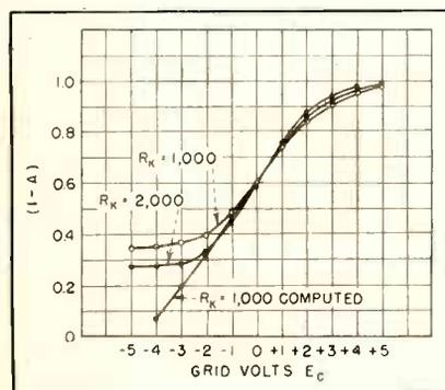
FIG. 6—Values of  $(1-A)$  for dual triode
