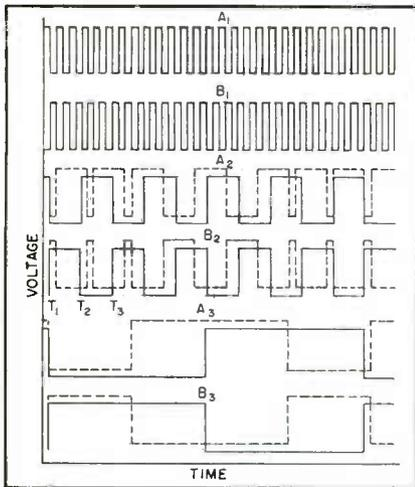
FIG. 3—Plate voltage waveforms for a three-stage multivibrator with and without feedback
