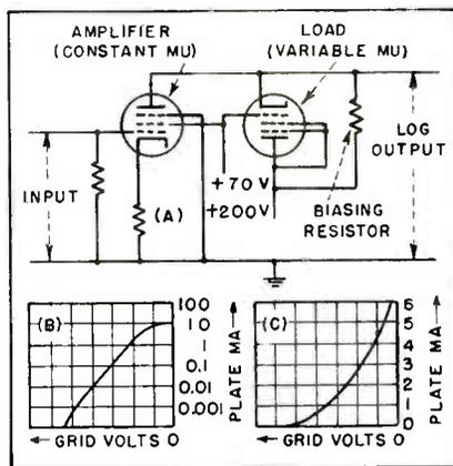
FIG. 1—Balancing voltage developed by variable-mu tube acting as load gives amplifier a logarithmic amplitude response
