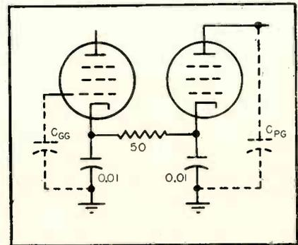
FIG. 6—B-minus decoupling circuit
