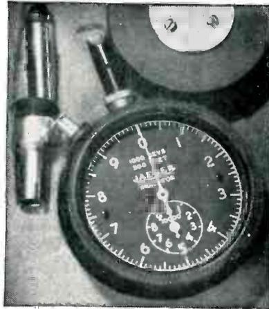
**PORTABLE (CHRONOMETRIC) TACHOMETER**
