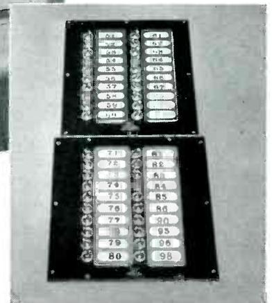
(Upper left) Cannon Annunciators (No. DRS-20) above radio transmitter used by Arkansas Power & Light Company, remote controlled from dispatcher's panels (Cannon No. DRC-20 above). Numbers flash the dispatch cars on air. Remote control panels at dispatcher's desk keep tab on cars checking in and out over radio.
