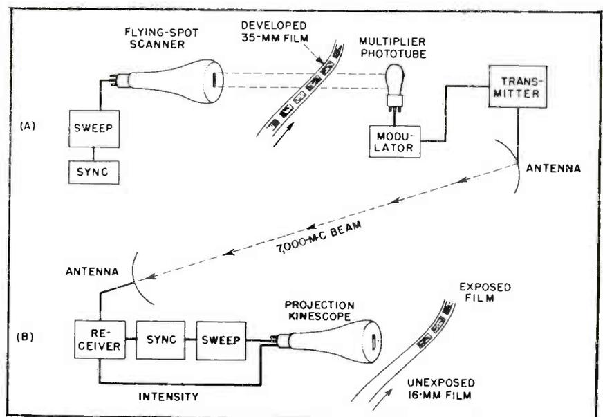
FIG. 1—Simplified block diagram of the system. Details of the photographic aspects are omitted
