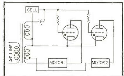
FIG. 3—Suggested circuit for operating a series of motors from different light levels
