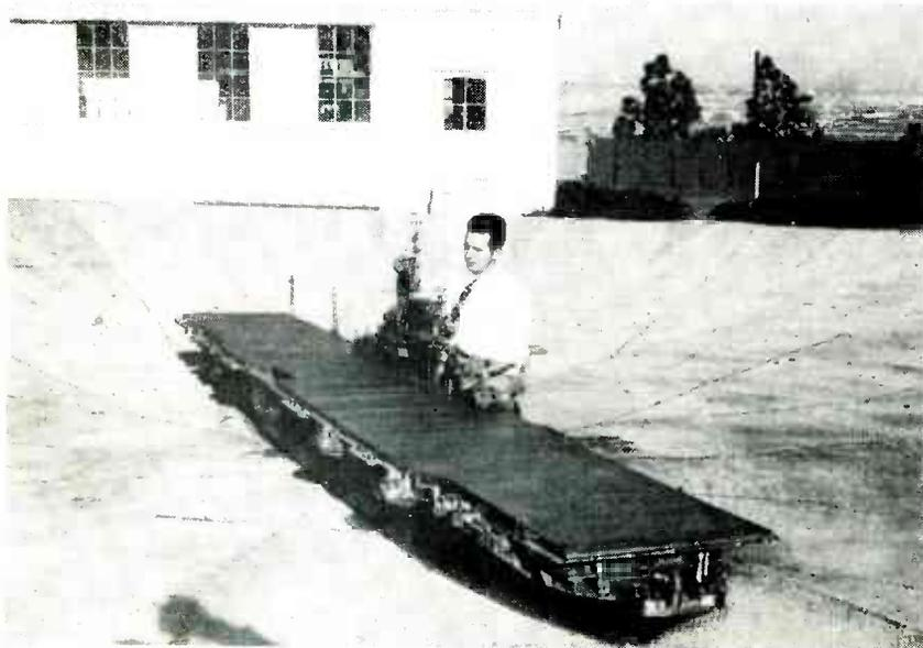
An 18-foot scale model Essex-type aircraft carrier is used to test equipment at the Navy's Electronics Laboratory, San Diego, Calif. While revolving on a turntable in the center of a wire-covered "ocean", the performances of the model's scaled-down radio and radar antennas are traced on plotting machines in the office at the rear
