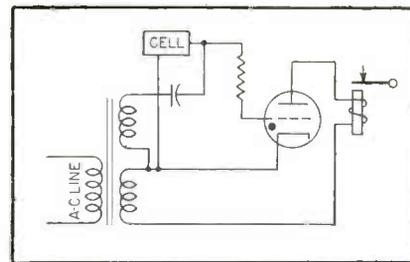
FIG. 2—The relay releases when illumination is removed from the photocell
