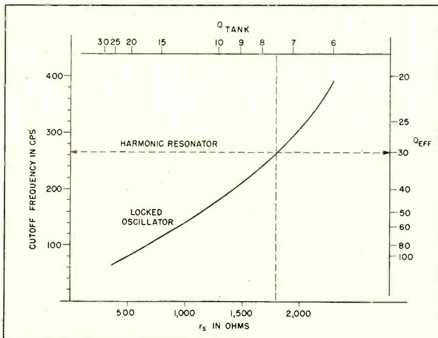
FIG. 10—Comparative measurements of oscillator and resonator performance
