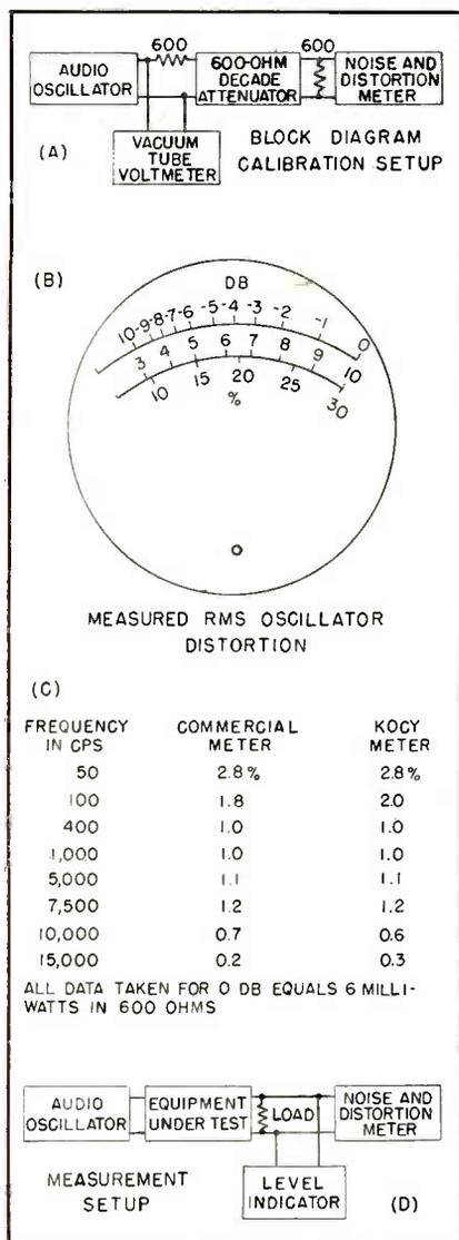
FIG. 2—(A) When the instrument is calibrated, the meter scale will appear as shown (B). Measurements made with the instrument (C) in a test setup (D) compare favorably with those made with a commercial meter
