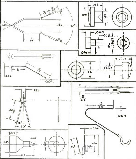
This simplified chart shows the form and overall dimensions of a few of the many types of contacts made from Ney Precious Metal Alloys with electrical and physical properties that have proved exceptionally satisfactory for brush or wiping contact applications. Full technical and test data are available on request. Other Ney Precious Metal Alloys have solved many special industrial application problems. Consult us freely without obligation.
