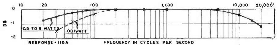
It may be noted that altho the permeability of magnetic materials drops at low flux densities, the **ADC** transformer has sufficient reserve inductance to allow for this even at low power levels. At 40 db below maximum power level it exceeds the response guarantee. Insertion loss at 1,000 cps was 0.75 db
