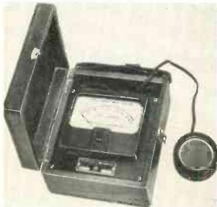
screens and c-r tubes. It is designed for laboratory tests, production control, installation and service. Range extends to 100 foot-lamberts.
