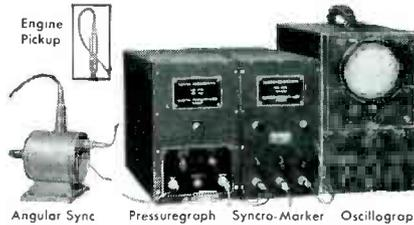
Engine Pickup Angular Sync Pressuregraph Syncro-Marker Oscillograph
