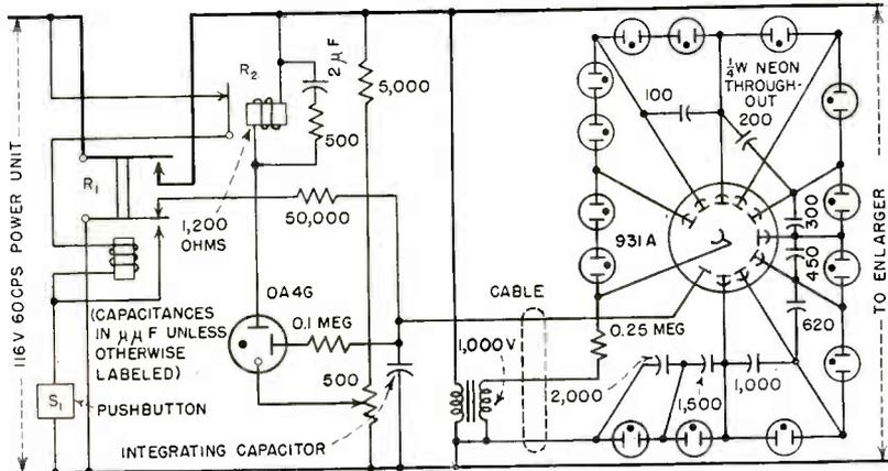
Circuit of timer shows parts built on chassis to left of cable and, at right, multiplier phototube and its neon-bulb regulator built in pickup head
