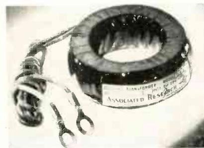
phase angle and ratio error. Designed for 5-volt-ampere burden they are provided with 2-foot secondary leads which may be connected directly to the instrument. The units are insulated for 4,500 volts a-c and can be used on 25 to 133 cycles.
