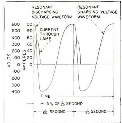
FIG. 5—Waveform of voltage across capacitor *C* of Fig. 4 and current through the lamp. The scale is distorted for illustration purposes
