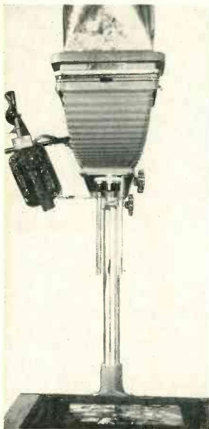
Pickup of timer (upper left) which scans printing easel (bottom) can be mounted on enlarger
