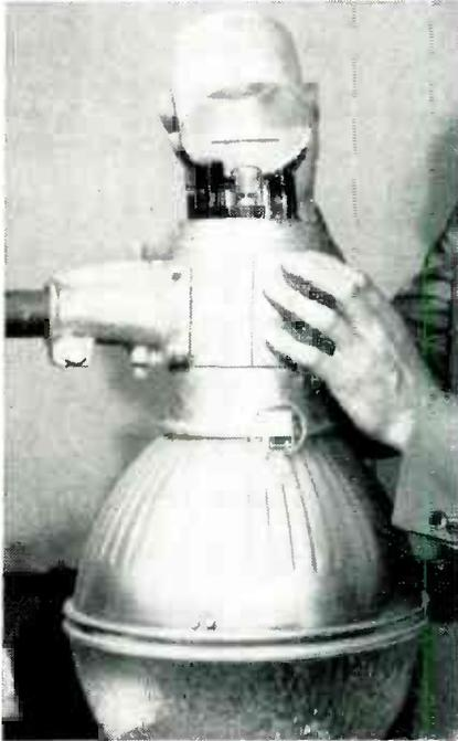
a red-sensitive gas-filled phototube, two amplifier tubes, a filament transformer, and a relay element.
