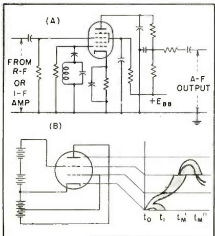
FIG. 1—(A) Phasitron circuit is a multigridded demodulator for f-m having the characteristic shown here. (B) Action of demodulator depends on the space charge coupling between two control grids
