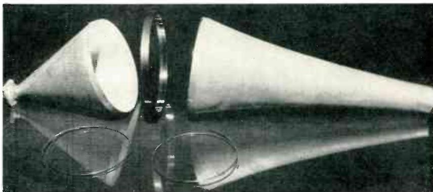
Parts for f-m dummy-antenna assembly. Silver-plated copper spinnings are simultaneously brazed to the brass support ring by induction heating
