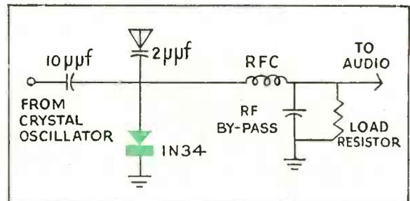
HERE A SYLVANIA GERMANIUM DIODE 1N34 is used as a high frequency mixer. RF signal from a crystal oscillator is impressed on the crystal, and mixed with RF signal from the antenna to produce an audio frequency beat note.
