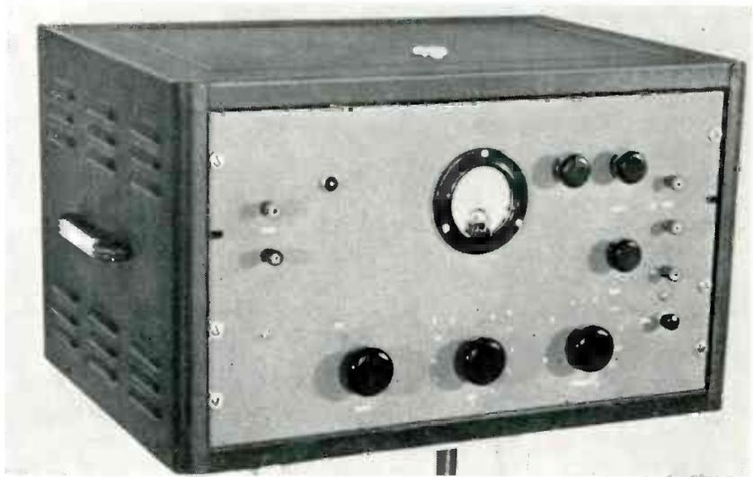
Test equipment, housed in cabinet, could equally well be mounted in rack. Upper lefthand terminals are for connecting oscilloscope; righthand terminals are for input. Three lower controls are, left to right, power switch, attenuator and frequency switch. Upper pair of controls are for bridge resistance, middle one is level control
