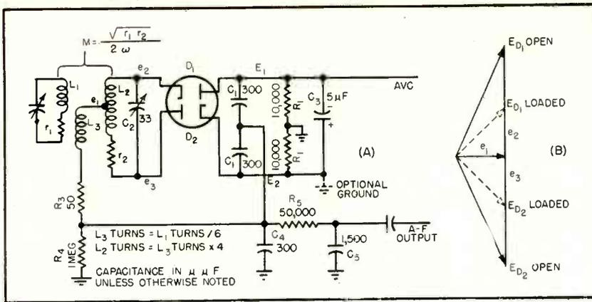
FIG. 2—Ratio detector for f-m. Transformer turns ratios are given and the vector diagram indicates optimum transformer performance
