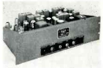
ing of channels may be necessary, the receiver is designed to have a selectivity of at least minus 80 db for 60 kc off resonance.
