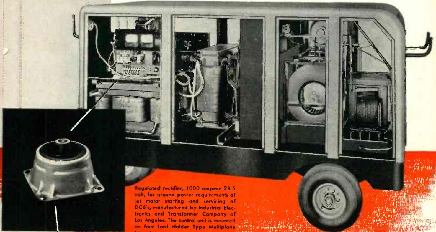
Regulated rectifier, 1000 ampere 28.5 volt, for ground power requirements of jet motor starting and servicing of DC's, manufactured by Industrial Electronics and Transformer Company of Los Angeles. The control unit is mounted on four Lord Holder Type Multiplane Mountings.
