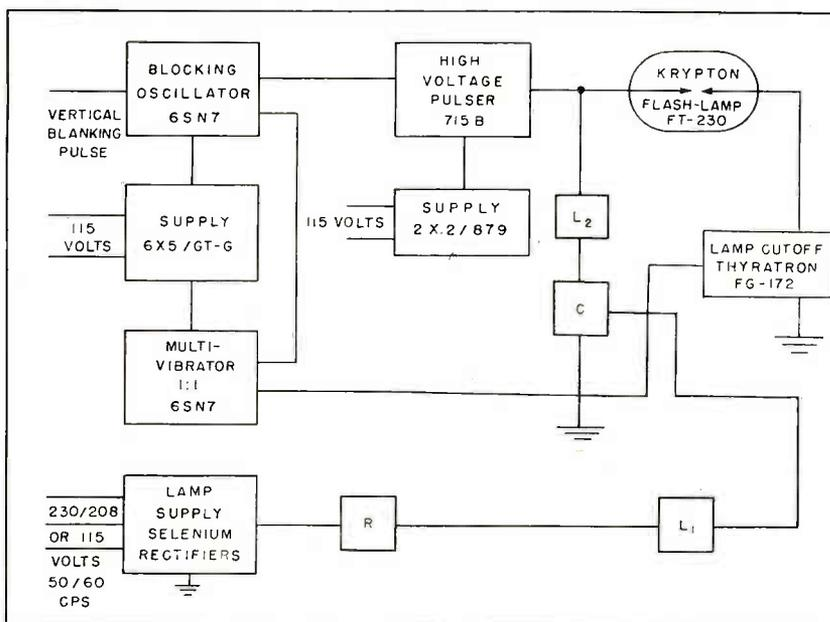
FIG. 4—Synchro-Lite block diagram
