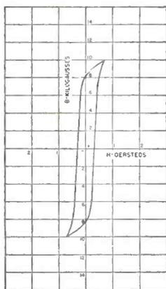
HYSTERESIS CURVES OF A SAMPLE OF 0.002" ARMCO THIN-GAGE ELECTRICAL STEEL
