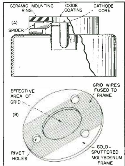
FIG. 2—Cutaway view of cathode sub-assembly (A) and grid structure (B)
