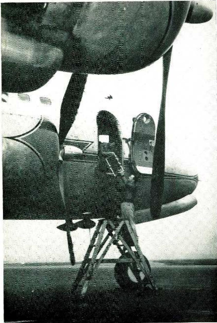
Line crew removing a typical piece of Collins equipment from a ship for overhaul
