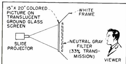
FIG. 3—Simple test setup used at CBS laboratories to determine effect of neutral density filters for typical observers
