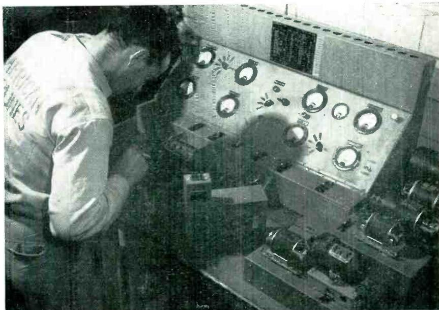
FIG. 11—A variety of adapter chassis permits testing dynamotors under load and for excessive noise
