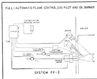
45JP1 electronic flame rod, type 45PH5 photoelectric scanner, and type 24PJ8 programming control. Relay contacts will directly handle a 1-h-p motor. Further details are given in bulletin CH4753.
