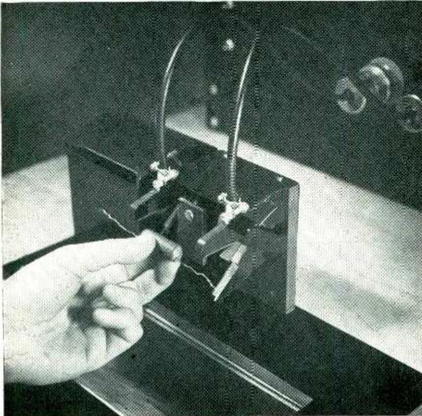
Universal jig for testing components with pigtails. Solenoid in box at left closes jaws when component touches ejector plate between jaws. Sorting chute opening is directly below jig
