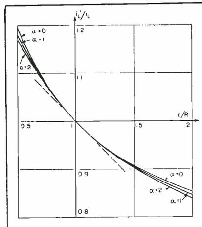
FIG. 2—Curves showing usefulness of match-test bridge circuit
