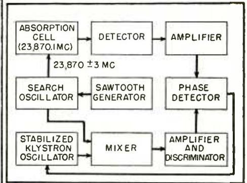
FIG. 2—Sampling stabilizer using a klystron oscillator
