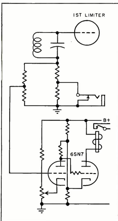
FIG. 3—Carrier-operated relay circuit for dial and ringdown operation
