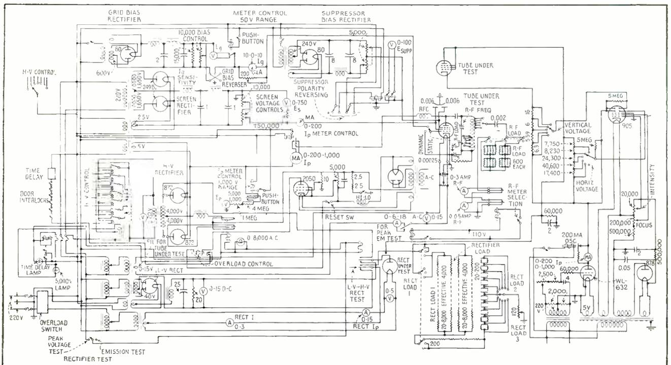
FIG. 8—Circuit of tube tester. A power tube is operated as an r-f oscillator under load conditions. The cathode-ray tube is used in an emission test
