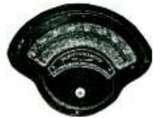
Another of the famous Weston fan shaped line. Very large scale 5.8" long. These meters were made by Weston to General Radio specifications, with special mirrored scale and knife edge pointer. Accuracy 1%.
