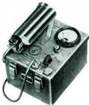
self-quenching with a Geiger threshold at 825 volts plus or minus 25 volts, and has a 200-volt plateau. The tube itself is mounted within a specially designed probe that enables differentiation between alpha, beta, and gamma radiations. Utilizing a plug-in circuit for easy servicing, the instrument has a battery life in excess of 400 hours. Price is \$289.50 delivered complete.
