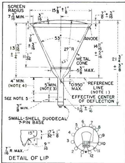
Dimensional specifications and basing diagram of type 16AP4 tube.
