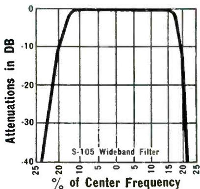
Wide band sharp cutoff band pass. Size:  $2 \times 3\frac{1}{2} \times 6\frac{5}{8}$ .
