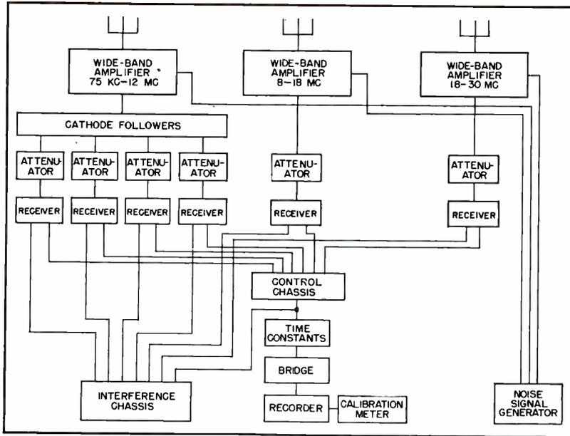
FIG. 1—Block diagram of the atmospheric noise-recording setup. Receivers are automatically switched
