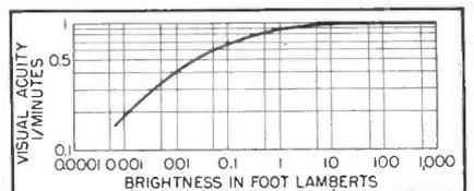
FIG. 1—Curves showing effect of increasing brightness on visual acuity
