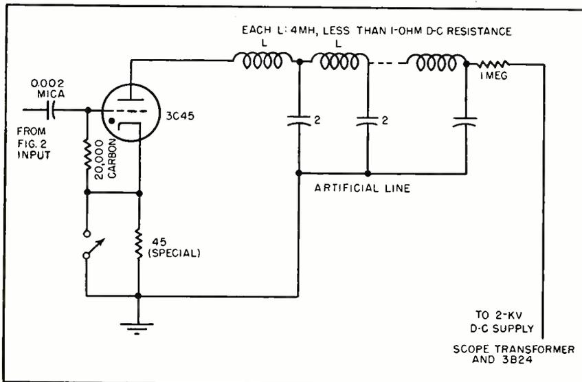
FIG. 5—Circuit of square-wave pulse generator
