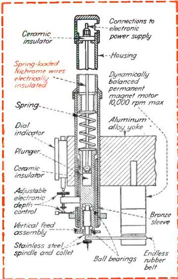
High coefficient of linear expansion of Nichrome V permits maximum vertical movement of spindle with shortest possible length of wire.
