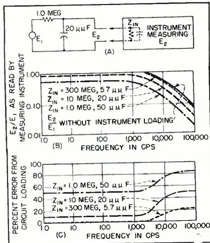
FIG. 3—Errors in high-impedance measurements due to circuit loading
