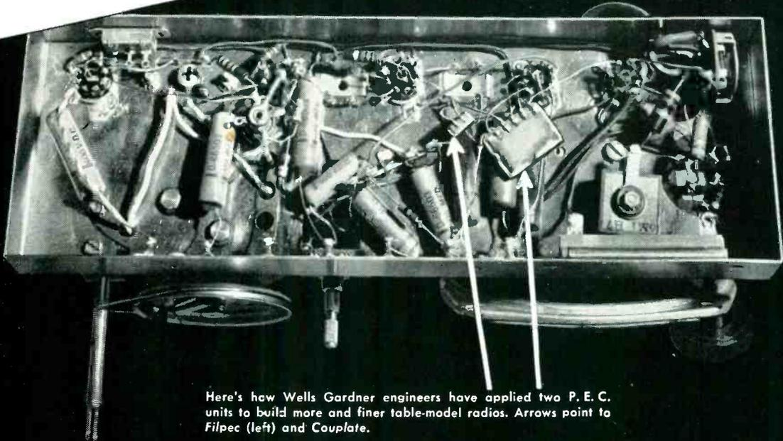
Here's how Wells Gardner engineers have applied two P. E. C. units to build more and finer table-model radios. Arrows point to *Filpec* (left) and *Couplate*.
