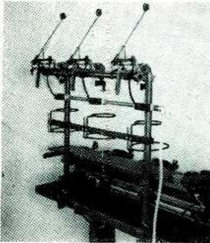
activated by the tension compensators. This lever is equipped with a splash type mercury switch that is connected to the counter solenoid. When the mercury switch is agitated, it operates the solenoid which in turn disengages the clutch in the winding head and stops the arbor.
