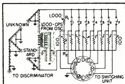
FIG. 2—Bridge circuit. Limit plugs in  $J_1$  through  $J_7$  determine range of tolerance groups into which components are sorted. Resistors  $R_1$  and  $R_2$  form 10-to-1 ratio arm which is connected when bridge is in rest position
