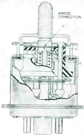
FIG. 3—Cutaway view of assembled triode, showing relative positions of elements
