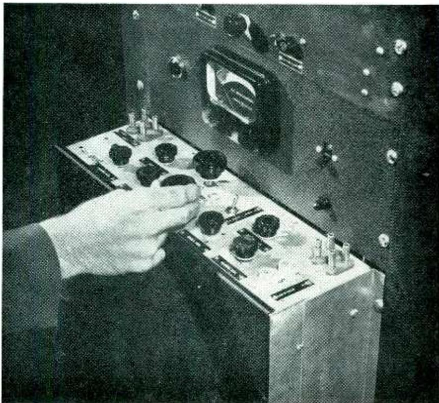
Rack-mounted version of low-distortion a-m signal generator
