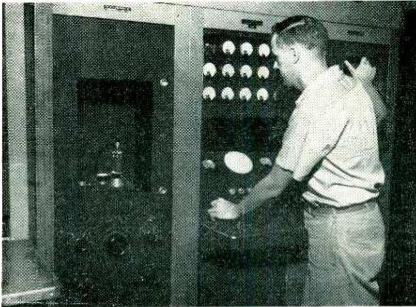
FIG. 7—Complete tube tester for transmitting and rectifier types is contained in these three racks and section above
