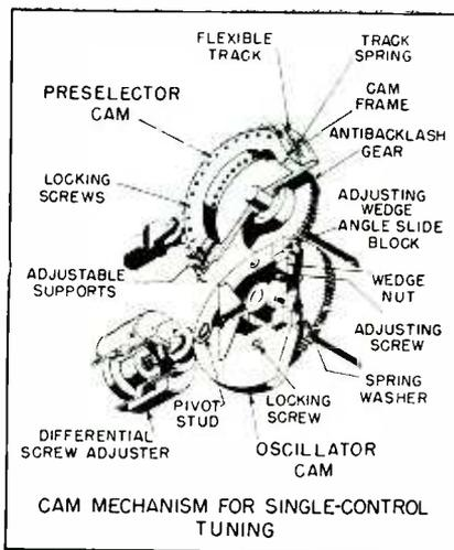
Adjustable cams relieve production tolerances and simplify tuning adjustments
