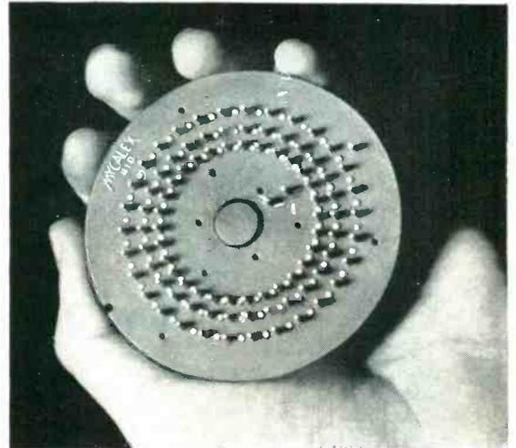
Illustrated are top and bottom views of the MYCALEX 410 molded insulation commutators manufactured to the specifications of Raymond Rosen Engineering Products, Inc., for Air Material Command and Navy telemetering projects. This commutator, with 180 contacts and 3 slip rings of coin silver, samples sixty channels of information such as air speed, altitude, angle-of-attack, temperature, pressure, voltage and other variables; and provides thirty synchronizing pulses.
