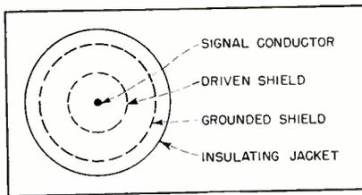
FIG. 2—Signal-probe cross section
