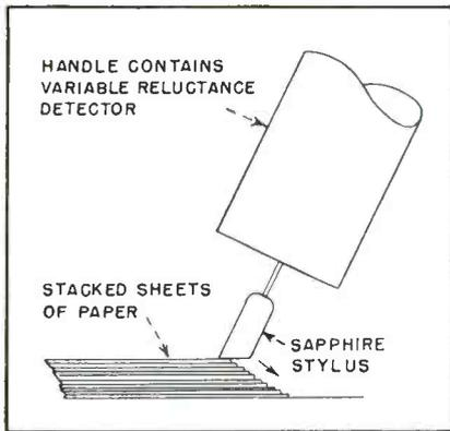
The number of sheets in a pile of paper is rapidly and accurately determined by brushing this sapphire stylus over serrated surface formed by riffling pile
