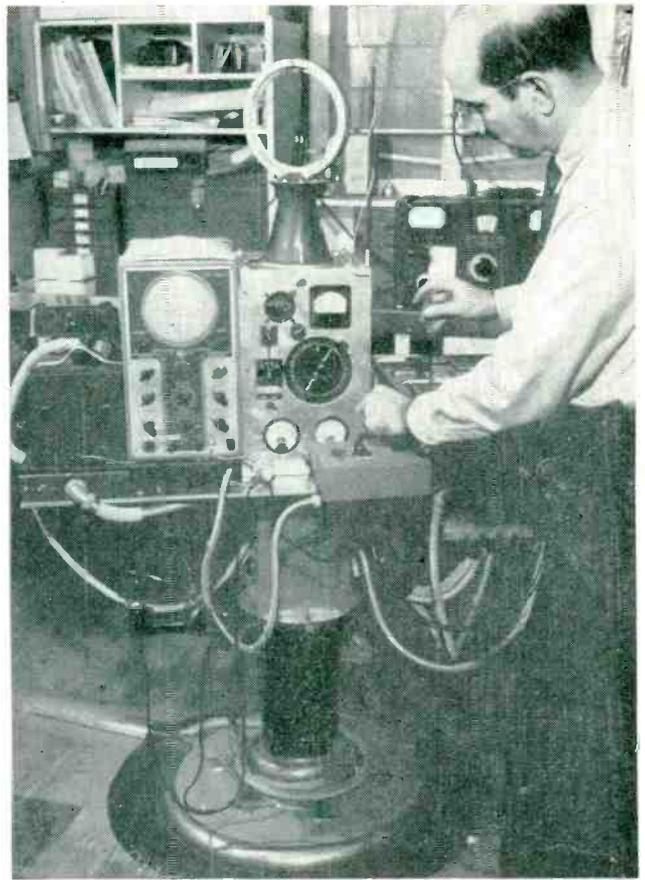
FIG. 2—A barber's chair provides a sturdy mount for rotating direction-finding equipment during final adjustment and performance check
