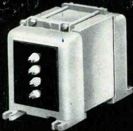
U.T.C. Commercial Grade components employ rugged, drawn steel cases for units from 1" diameter to 300 VA rating . . . vertical mounting, permanent mold, aluminum castings for power components up to 15 KVA. Units are conservatively designed . . . vacuum impregnated . . . sealed with special sealing compound to insure dependability under continuous commercial service.
