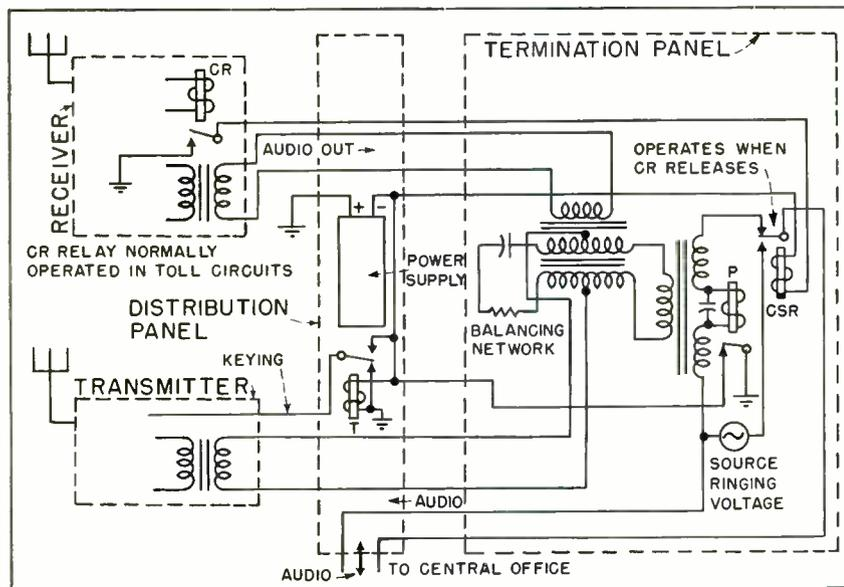
FIG. 2—Terminal equipment used to extend wire-telephone service by means of radio. It can be used in different ways, using optional interconnections
