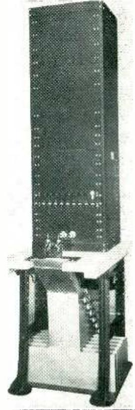
Front view of automatic bridge, showing jig, sorting chute and door-control solenoids, and bins
