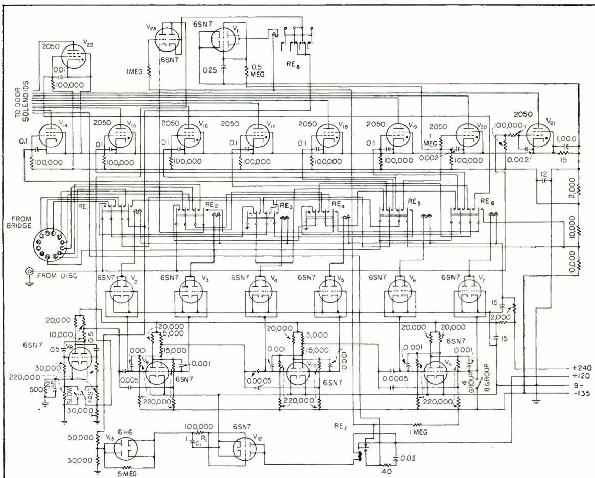
FIG. 5—Schematic diagram of switching and door-control circuits. Sequence of operation is explained in Table I. Frequency of free-running multivibrator is approximately 48 cps
