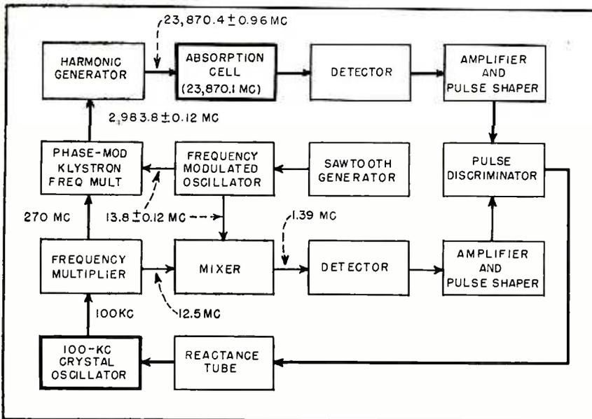
FIG. 3—Simplified block diagram of the NBS clock, based on 100-kc crystal driving a phase-modulated klystron multiplier
