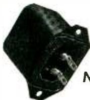
Two efficient filter reactors, inductance values .8 and 2.4 henrys respectively, are designed for noise suppression circuits, but can be used in any tuned circuit requiring the given inductances. Inductance values are accurate within  $\pm 5\%$  with up to 15 ma. d-c. Minimum Q of 20. Mounted in identical drawn steel cases  $1\frac{1}{16}'' \times 2\frac{3}{8}'' \times 1\frac{1}{16}''$ . Write for descriptive sheet including diagram of simplified dynamic circuit.
