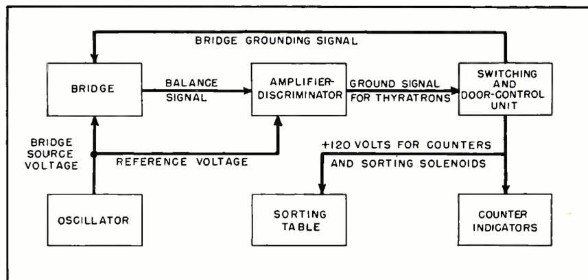
FIG. 1—Block diagram of Industrial Instrument's high-speed component tester and sorter
