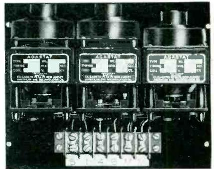
initial time delay of one minute. Time delay starts when the coil is energized. Once the timing cycle is complete the unit switches off. Restoration of power within 1 to 15 seconds instantaneously re-establishes the circuit. After 16 seconds, time delay is proportional to the length of time of the power failure.
