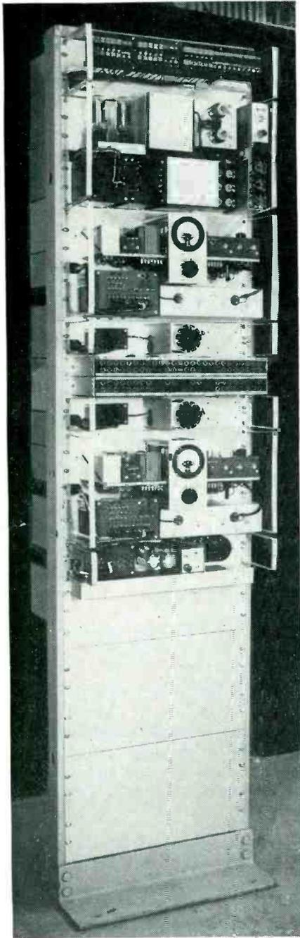
Complete Lenkurt type-32 three-channel carrier repeater
