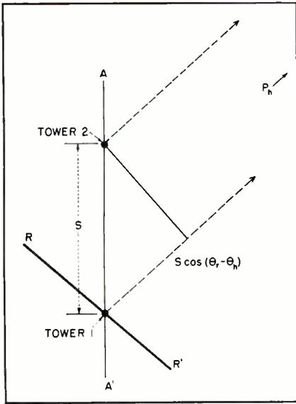
FIG. 1—Basic diagram of field created by a two-tower array
