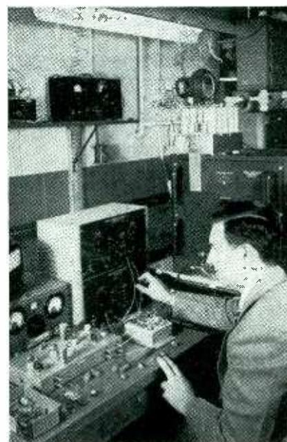
Checking performance of miniature tubes and special pulse transformers in NBS electronic lab prior to incorporation in new electronic digital computer that is scheduled to use a high-speed electrostatic cathode-ray memory storage device
