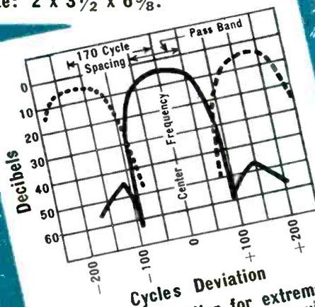
Tone channel filter for extremely high crossover attenuation requirement. Size:  $2\frac{1}{2} \times 2\frac{1}{2} \times 5$ .
