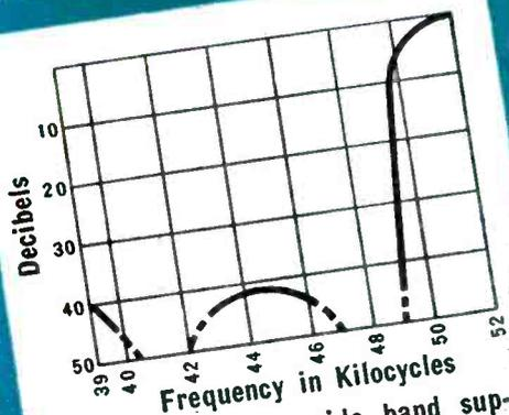
Extremely sharp side band suppression filter. Available in either low or high pass. Size:  $2\frac{1}{2} \times 4 \times 2\frac{1}{2}$ .
