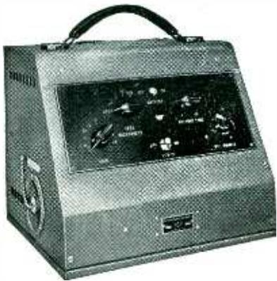
**An Electronic Replacement For Sensitive Galvanometer Systems**
