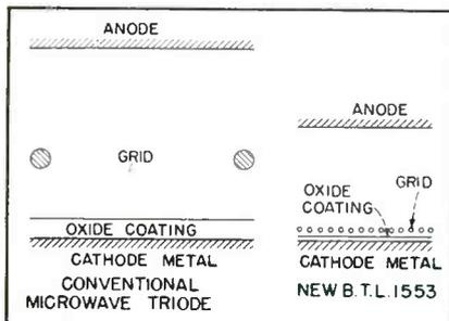
FIG. 1—Comparison of electrode spacing in ordinary microwave triode and the recently-developed BTL 1553
