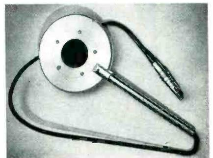
gages for measuring pressures of instantaneous nature from a few pounds to 30,000 psi. Their usefulness lies in their ability to measure shocks of high magnitude when transmitted through liquids, gases, and, at times, through solids.
