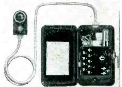
ing, conveyor control, short-range signal systems, motor or valve control, production inspection, machinery safeguards, and stop-motion control in the textile, paper, and wire industries. Designed for high-speed operation, the relay operates in 0.05 second. Operating range is 10 feet. A sensitivity adjustment provides for relay operation at any predetermined level of illumination within the range of 10 to 50 foot-candles. Maximum rating of the dpdt control relay is 10 amp, 115 v a-c.
