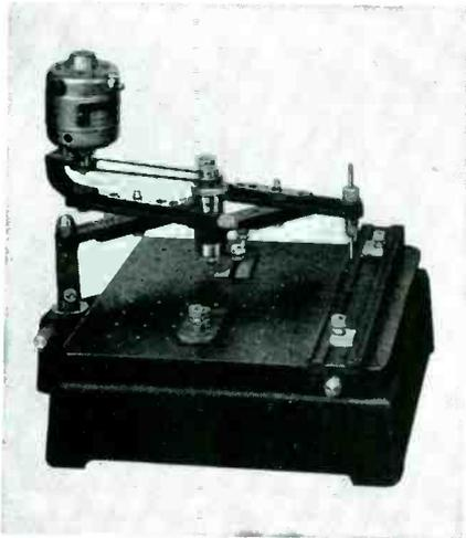
Used in making small molds and dies or engraving panels and nameplates of metal or plastic.
