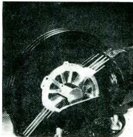
Anodes of magnetrons are made in quantity from stampings consolidated into a vacuum-tight whole by silver brazing. Alternate stampings have larger outside diameter to form cooling fins. Such techniques simplify production of complex shapes
