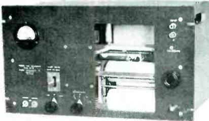
56 double-chart-speed combinations from 45 inches per minute to 0.5 inch per hour and for recording frequency ranges from 2 to 200,000 cycles. A calibration control is built in. Typical applications include the fields of acoustics, electro-acoustics, noise and vibration, loudness, strain and pressure, and field strength.
