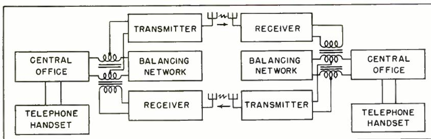
FIG. 1—Block diagram of a two-way radiotelephone circuit connected to conventional two-wire telephone system
