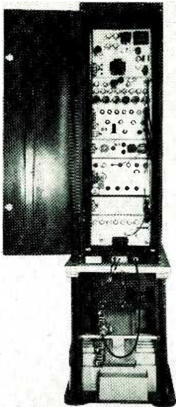
Rear view, showing unit construction for easy replacement. Limit plugs and standard may be seen on bottom chassis
