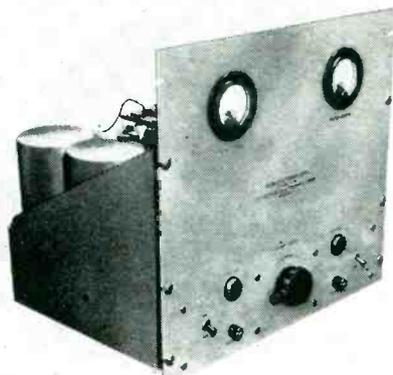
volts, 60 cycles, 750 watts. Output is variable from 160 to 1,500 volts, 125 ma d-c. Ripple is less than 0.05 volt peak-to-peak.
