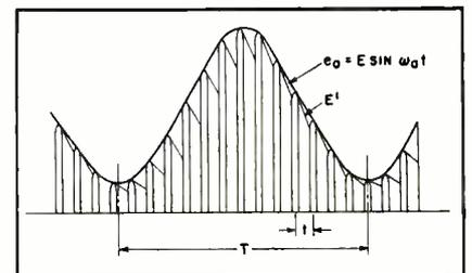
FIG. 3—Modulator cathode waveform showing the modulation envelope
