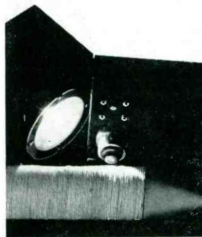
Closely-spaced small objects are accurately counted by this new narrow-beam count detector in conjunction with standard electronic counter
