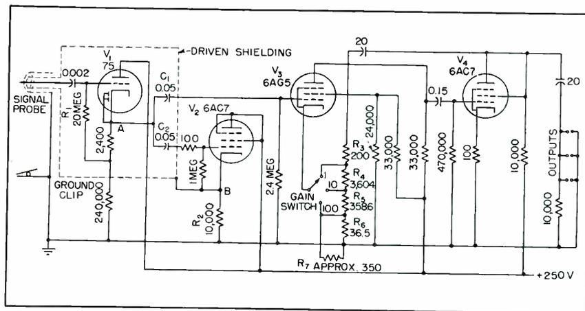
FIG. 1—Isolation amplifier circuit diagram. See text for resistor tolerances
