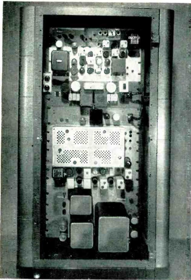
Complete terminal comprising transmitter, receiver, interconnecting equipment and power supply
