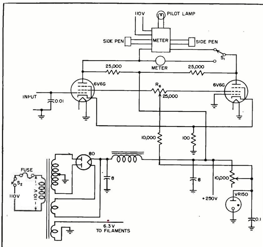
FIG. 3—Recording bridge circuit, balanced by adjustment of  $R_b$
