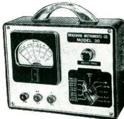
21 ranges; up to 1,250 v a-c, 1,000 v d-c, 100 ma d-c, 1 megohm, and from minus 10 to plus 57 db in five ranges. Sensitivity is 1,000 ohms per volt.
