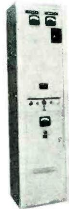
50,000 volts has a maximum current output of 1 milliamper. It has been designed for use in electron diffraction studies research on high-intensity cathode-ray screens, electron microscopy, and projection television experiments. High voltage is obtained by means of an r-f oscillator at 40 kc.
