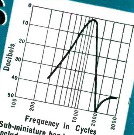
Sub-miniature band pass. Includes 3 coils and 4 condensers. Volume  $4\frac{1}{2}$  cubic inches.
