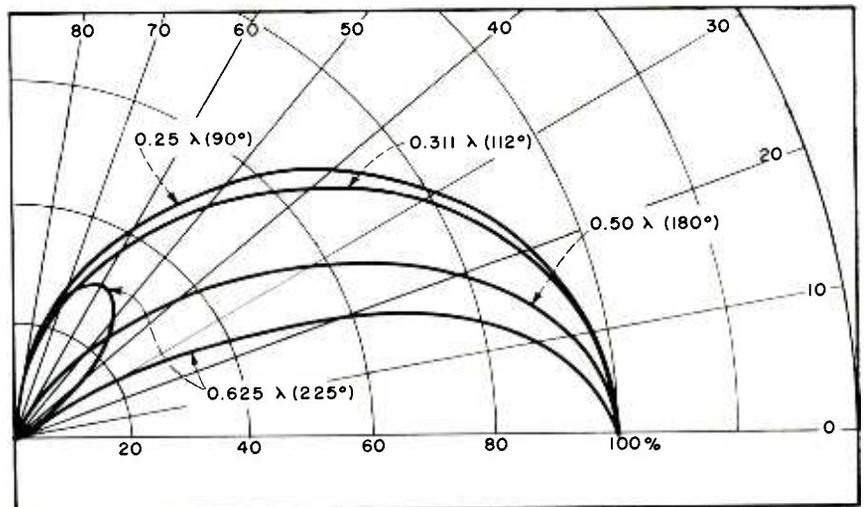
FIG. 2—Vertical radiation patterns of vertical antennas
