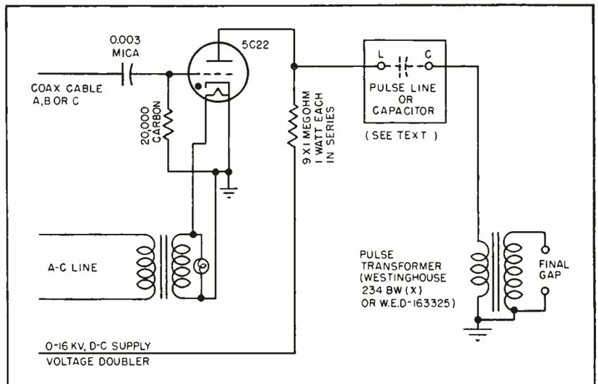
FIG. 3—Each high-level pulser employs a hydrogen thyratron
