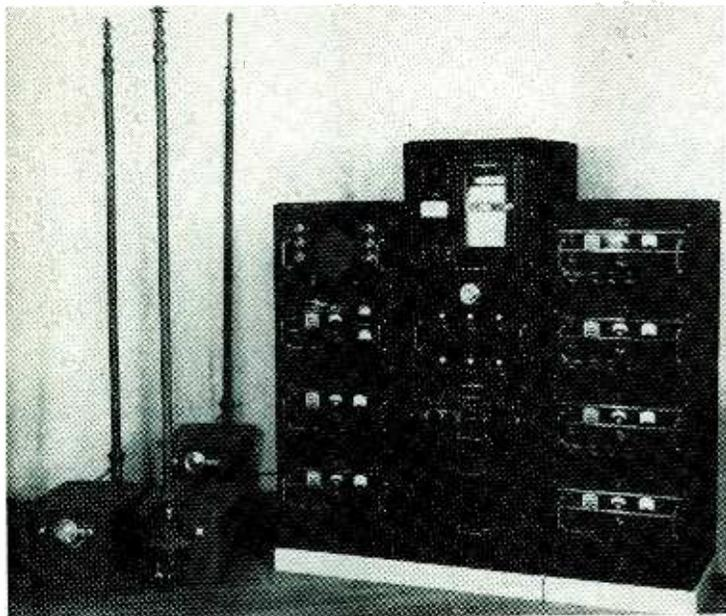
Loudspeaker monitor with noise generator and two receivers underneath in rack at left; control equipment and recorder in center rack; receivers at right
