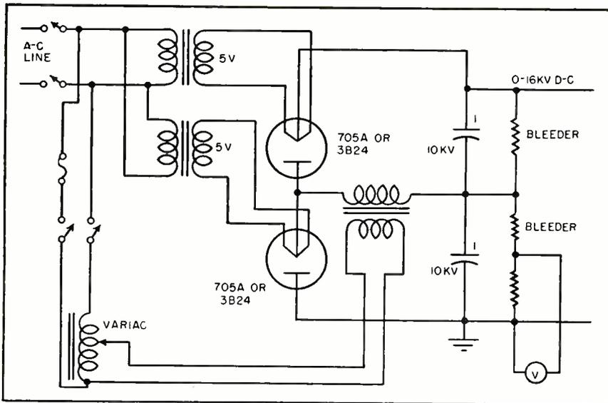
FIG. 4—Sixteen-thousand-volt power supply
