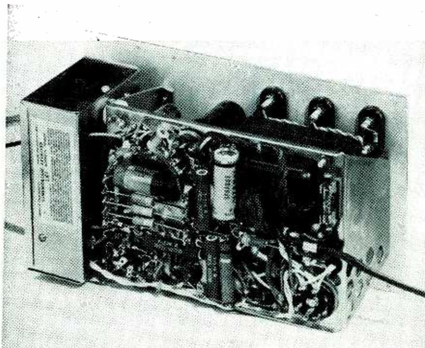
Under-chassis view. The type-75 tube is mounted inside the insulated shield box
