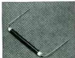
Bradley's new high voltage selenium rectifier—model SE8L—is low-priced for production requirements. Rated at 1.5 ma D. C. and up to 3,000 volts peak inverse. For higher voltage requirements, model SE8L can be used in series or multiplier circuits. Measures only 1/4-inch in diameter—up to 3 inches in length. Completely sealed.
