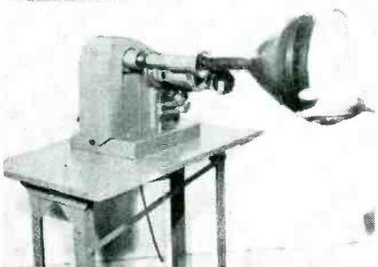
type number. The operator places the end of the tube into the fixture, depresses a foot treadle and the machine places the imprint on the tube.
