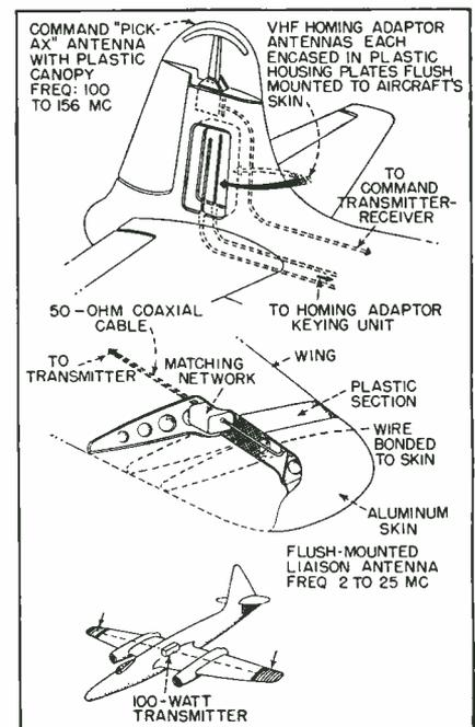
Flush mounted antennas for use in high-speed aircraft. Tests show them superior to exterior antennas in many ways
