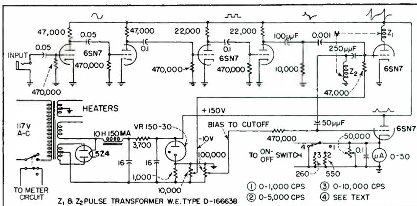
FIG. 1—Schematic circuit diagram of the audio-frequency meter
