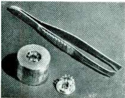
Tube parts can be machined from solid copper or built up and brazed together from smaller pieces
