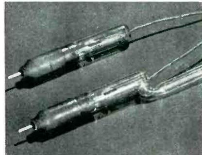
Two types of pipe seals: (above) coaxial press seals and (below) feather edge seals for magnetron filament leads
