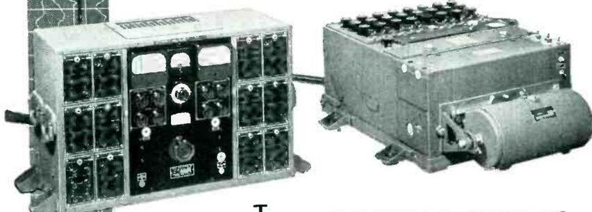
The type MRC-15 STRAIN GAGE CONTROL UNIT and the type S8-B OSCILLOGRAPH make up a complete strain recording laboratory. The MRC-15 contains complete equipment to power strain gages and to drive oscillograph galvanometers for recording from static strain to a frequency of 5000 cycles per second. It is complete with strain gage balancing controls, precision calibrating device, and power supply equipment.
