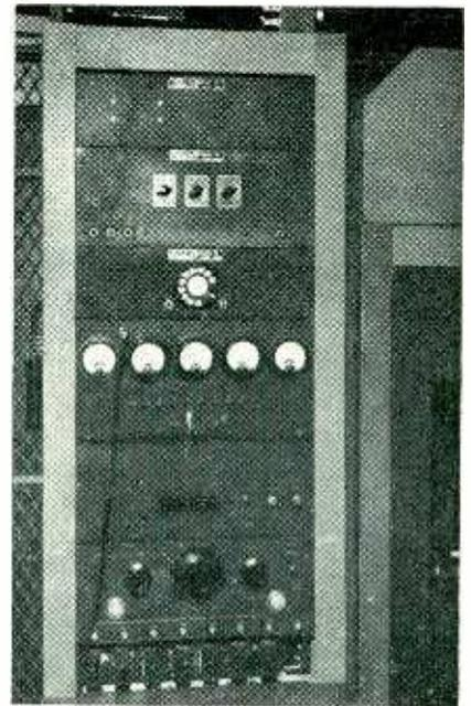
FIG. 6—Keying and dialing circuits are provided for testing ground transmitters
