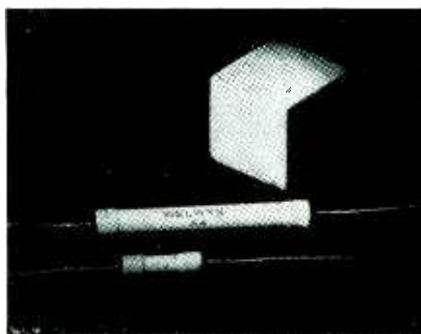
resistor element is a homogenous film of pure carbon deposited on a porcelain tube. After aging, fitted brass end caps are applied, into which the terminal leads are staked and soldered. The completed resistor is brought to the required resistance value by spiralling in automatic machinery.
