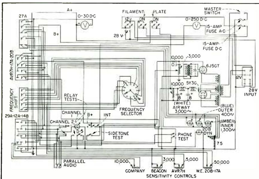
FIG. 4—Complete circuit of the special receiver test unit. Male plugs connect to cable sets for various receivers
