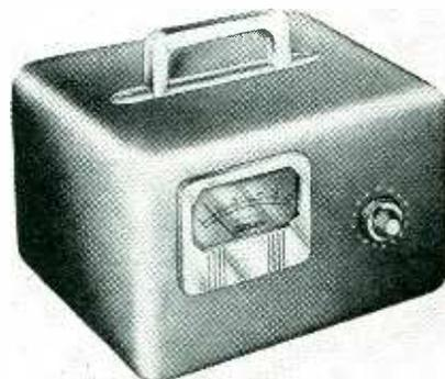
120 volts, 60 cycles. The unit is capable of measuring field strength from 50 to 50,000 microvolts at the 300-ohm input terminals.
