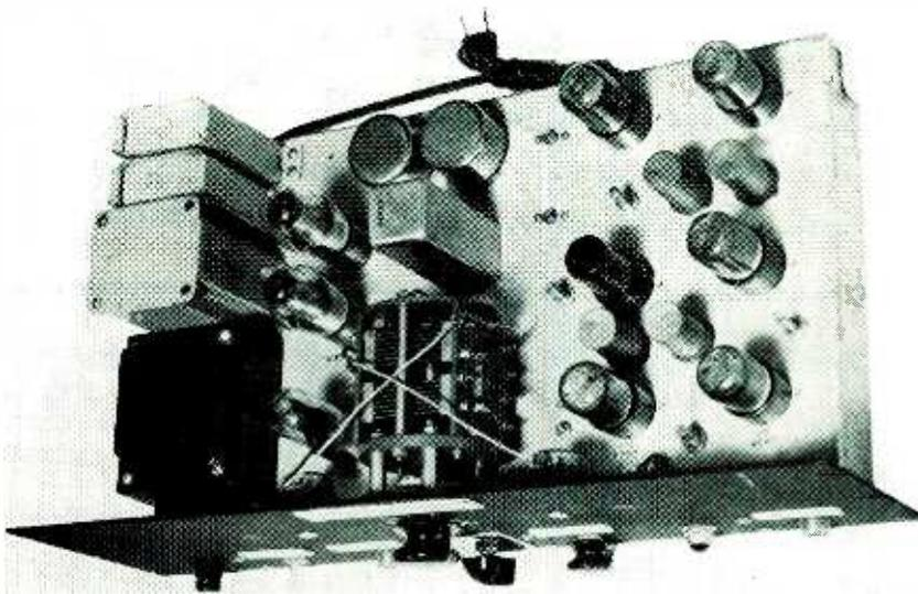
Production instrument for calibrating range ring pulses
