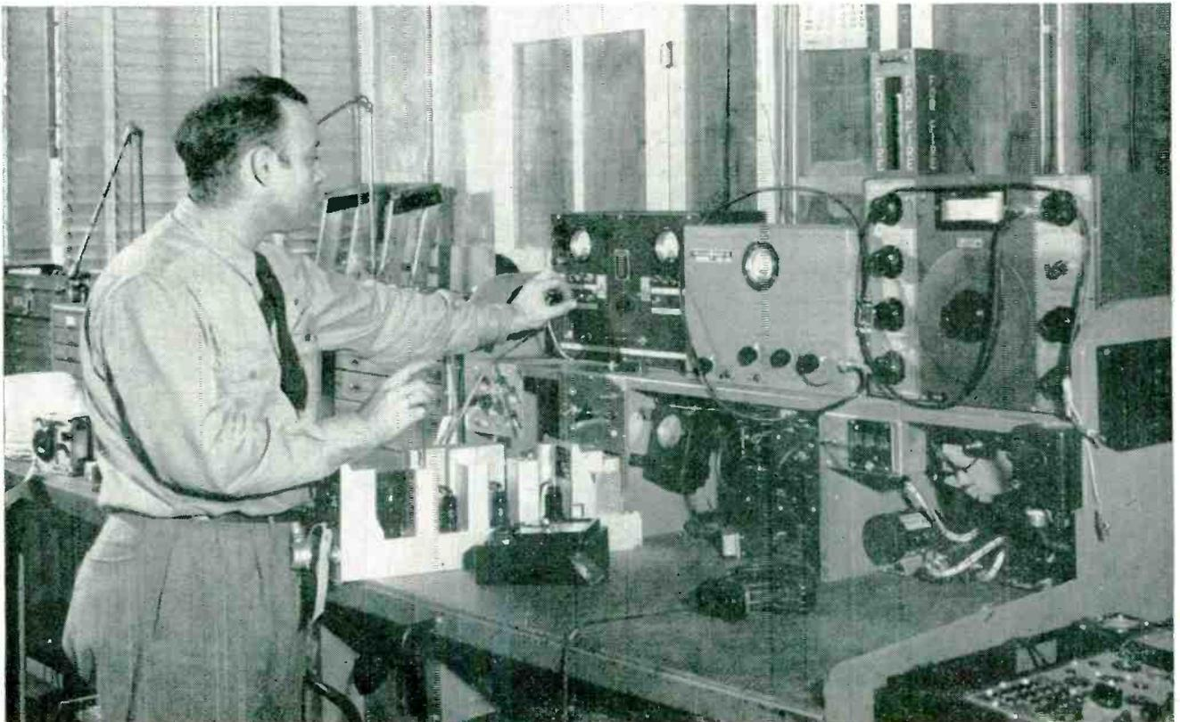
FIG. 3—Radio mechanic adjusts an AA-designed receiver test unit which simulates airplane wiring, controls and indicators
