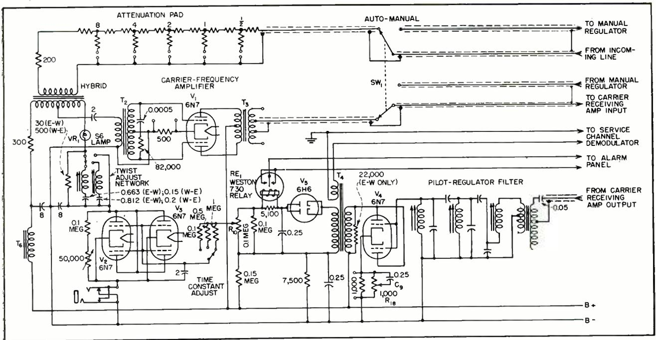
FIG. 3—Pilot regulator circuit. Reactance in the twist network in the right-hand arm of the hybrid bridge gives a frequency-discrimination factor that restores flat frequency characteristics
