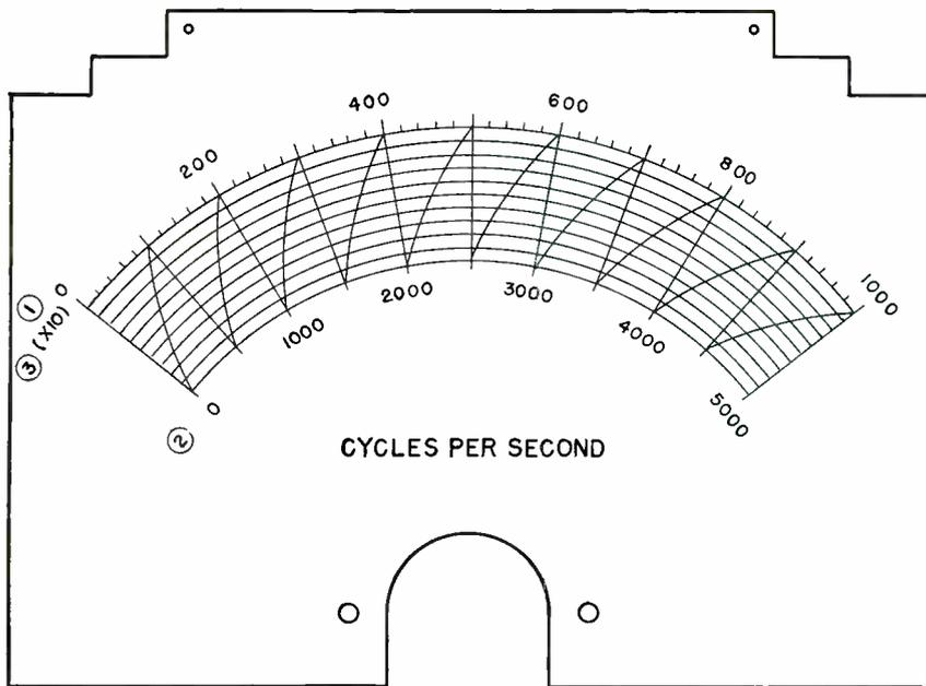
Meter scale used for three audio ranges
