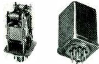
as well as other combinations up to 14,000 ohms in a single winding. The standard twin-150-ohm model operates satisfactorily on 5-ma reversals in one winding, and just trips at approximately 1 ma.
