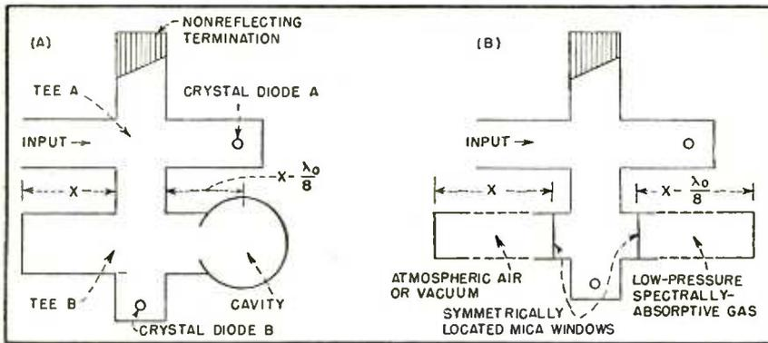
FIG. 1—Cavity-type discriminator (A) and similar spectrum-line discriminator (B) used for stabilizing frequency control
