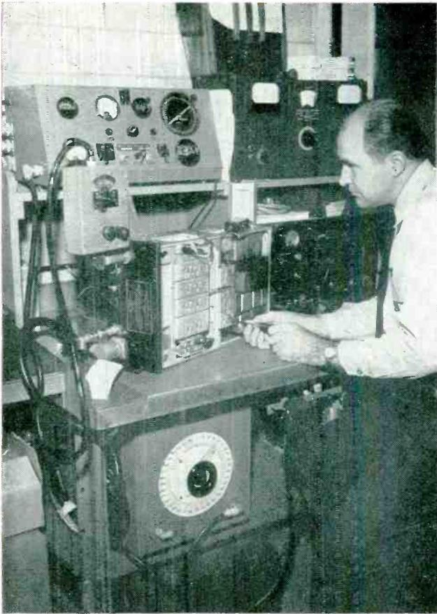
FIG. 1—Circuits of a Bendix adf receiver are completed by the accessories mounted in the cabinet at upper left. Operating conditions of the loop are simulated by the unit at lower left
