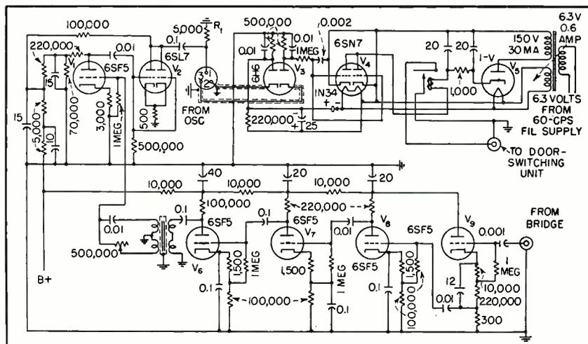
FIG. 4—Discriminator-amplifier circuit diagram. Crystal diode provides bias for discriminator by rectifying 6.3-volt filament supply
