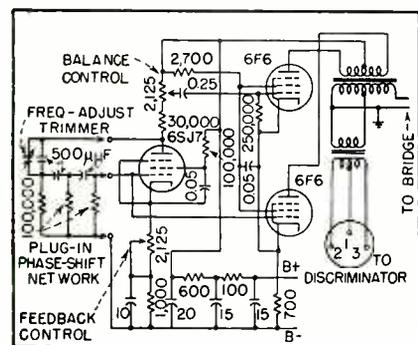
FIG. 3—Circuit diagram of Wien bridge oscillator which produces bridge voltage and discriminator reference voltage
