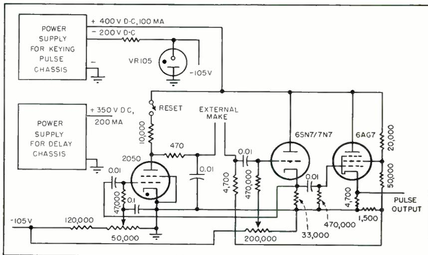
FIG. 1—Single pulses are generated with this circuit
