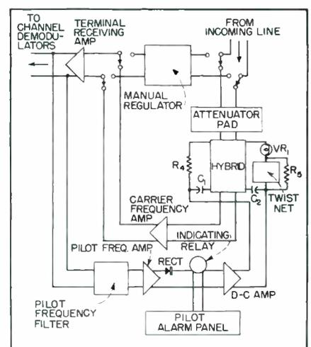
FIG. 2—Block diagram of pilot regulator. Control of attenuation is achieved in the hybrid transformer by the sampled pilot frequency derived from the carrier-frequency receiving amplifier
