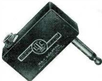
impedance microphones and pickups to high-impedance circuits. The unit matches any source from 50 to 500 ohms impedance to grid. Response is essentially flat from 50 to 10,000 cycles.
