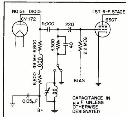
FIG. 4—Noise-initiating circuit for calibrating generator
