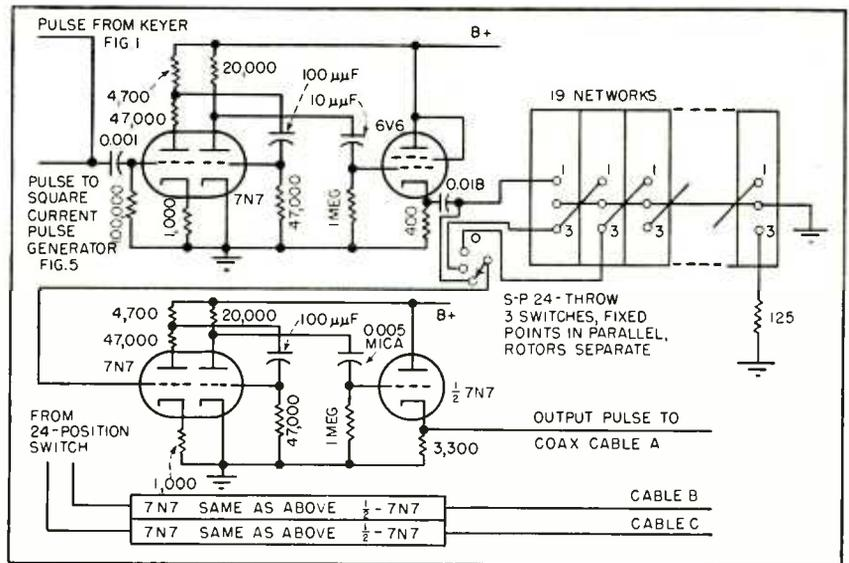
FIG. 2—This circuit provides a maximum delay of 26.6 microseconds
