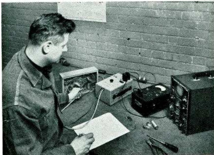
Amplifier being used for simultaneous voltage and waveshape observation
