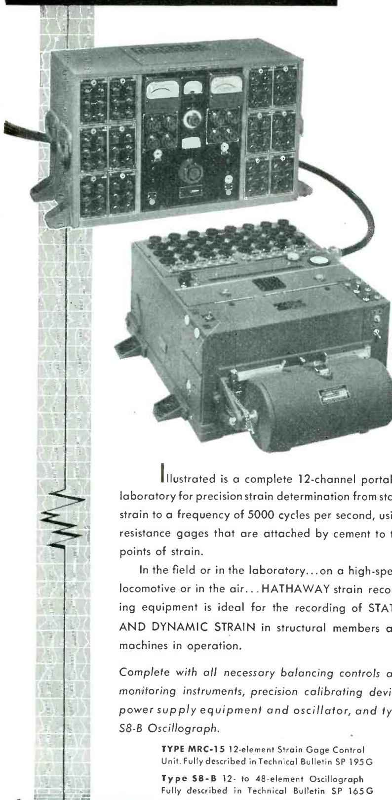
Illustrated is a complete 12-channel portable laboratory for precision strain determination from static strain to a frequency of 5000 cycles per second, using resistance gages that are attached by cement to the points of strain.
