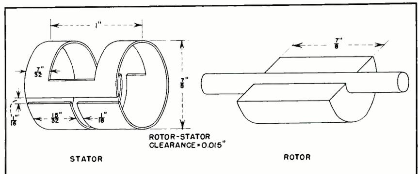
FIG. 6—Mechanical details of the rolled-up line
