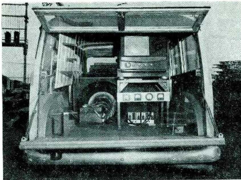
Interior view of the mobile setup used in the Washington field strength measurements. The four meters mounted below the receiver read 450-mc local oscillator injection current and plate current, the receiver afc voltage and the field strength
