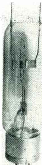
This GE type FH-11 split-anode magnetron was available commercially in 1930 but nobody wanted it
