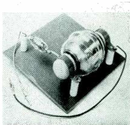
Photograph of a vacuum capacitor voltage divider. The values of the capacitors shown are 5 and 500  $\mu\mu\text{f}$  with 17,500-volt ratings—Official Photograph U. S. Navy
