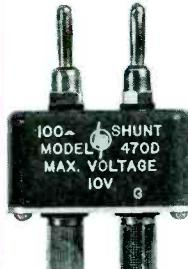
For -hp- 400A or 400C Voltmeters, to measure currents as small as 1  $\mu\text{A}$  full scale. Accuracy,  $\pm 1\%$  to 100 kc,  $\pm 5\%$  to 2 mc. Max. power dissipation 1 watt.
