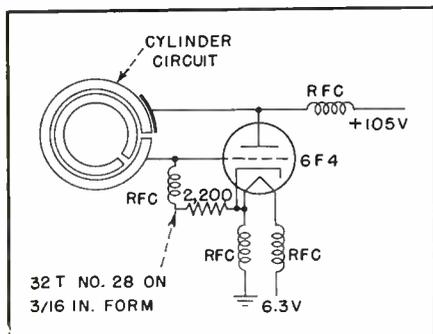
FIG. 2—Circuit of the cylinder oscillator
