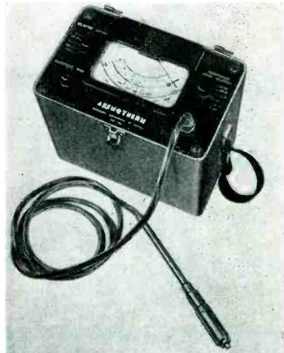
and 0.05 to 4 negative. The unit is useful for adjusting and testing equipment used for heating, ventilating and air conditioning.
