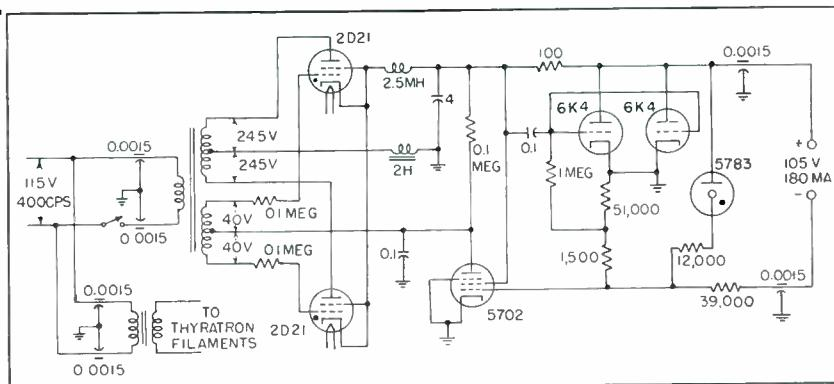
FIG. 1—Example of miniature thyatron regulated power supply circuit used with potted subassemblies to decrease size, weight and heating. Thorough shielding is necessary to avoid radiated noise from thyatrons. All 0.0015- $\mu$  capacitors are ceramic feed-through units to prevent conducted noise
