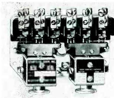
175KXX contactor comprises two 3-pole solenoids for forward and reverse operation mounted on a common frame and mechanically interlocked to prevent simultaneous closure. Designed particularly for service in the control of single horsepower motors, the use of the contactor is completely described in bulletin 7100.
