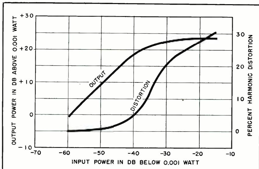
FIG. 3—Output and distortion curves of the clipping amplifier
