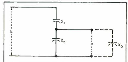
FIG. 1—Vacuum capacitor voltage dividers can be used to extend the range of vacuum-tube voltmeters, and similar indicating devices, without destroying their high-impedance characteristics
