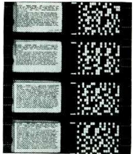
Sample of coded master 35-mm film. Wide dashes in middle are for frame sync, and first vertical row of squares to the right is for line sync to identify the horizontal rows to be paired in searching for a blackout. Each pair of rows is a subject code number, hence six pairs permit coding each abstract under up to six different subject headings
