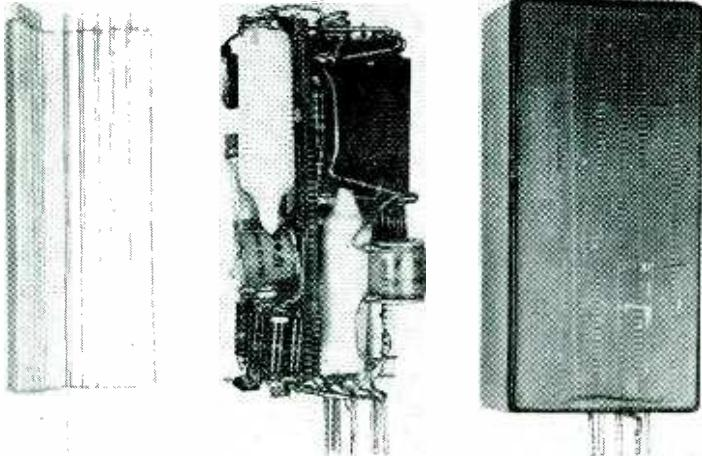
Steps in potting a three-tube strain gage amplifier. Left—casting-resin chassis with imbedded silver-clad beryllium-copper wires serving as stiffeners, tie points, plug prongs and lead wires. Center—assembled chassis with built-in limiter and voltage gain of 20,000, adjusted in production so all units have same gain within 1 percent. Right—complete plug-in unit as potted in casting resin. Other examples of potted plug-in units are shown in color on the front cover of this issue
