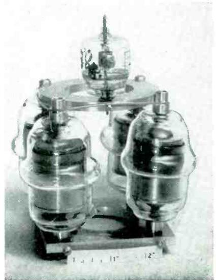
Vacuum capacitor voltage divider using tube plate-to-filament capacitance in series with four 50- $\mu\text{mf}$  vacuum capacitors connected in parallel—Official Photograph U. S. Navy
