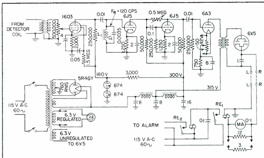
FIG. 4—Schematic diagram of metal detector amplifier and null detector
