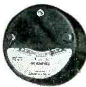
SENSITIVE RELAYS a line of sensitive relays including the Model 705 which provides positive control at levels as low as  $\frac{1}{2}$  microampere. Non-chattering magnetic contacts handle up to 10 watts at 120 volts.
