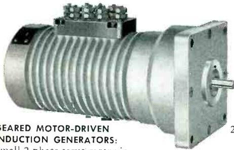
**GEARED MOTOR-DRIVEN INDUCTION GENERATORS:** Small 2-phase servo motor in combination with a compact gear-reducer and a low residual induction generator. Motor has high torque/inertia ratio and develops maximum torque at stall. Gear-reducer permits a maximum torque output of 25 oz. in. and is available in ratios from 5:1 to 75,000:1.
