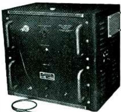
This unit is designed for use as an oscilloscope deflection amplifier for the measurement and viewing of pulses of extremely short duration and rise time, and contains the Video Amplifier Unit, Power Unit and a low Capacity Probe.
