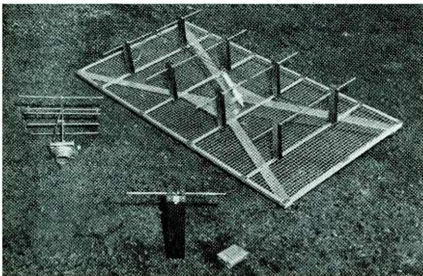
The three types of receiving antennas used in the Washington, D. C. uhf television field strength measurements are shown above. They are the half-wave dipole, a 4-element Yagi and an 8-element array
