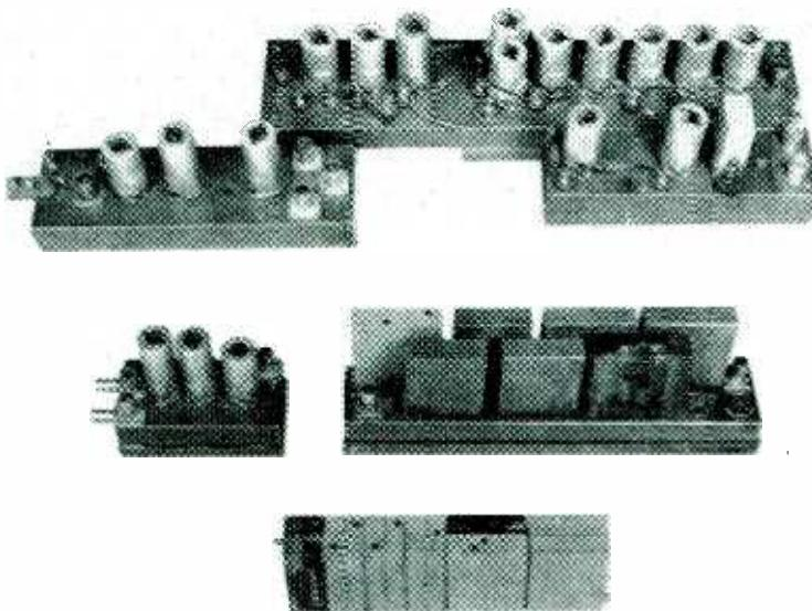
Top—conventional construction of 14-tube wide-band i-f and video amplifier with afc and agc, for input frequency of 100 mc. Center—first step in miniaturization, using potted subassemblies but retaining the chassis and a conventional low-noise preamplifier. Bottom—final miniaturized assembly complete with preamplifier, with each unit plugging into its neighbor to eliminate the chassis. Most of the subassemblies are coated with silver shielding paint
