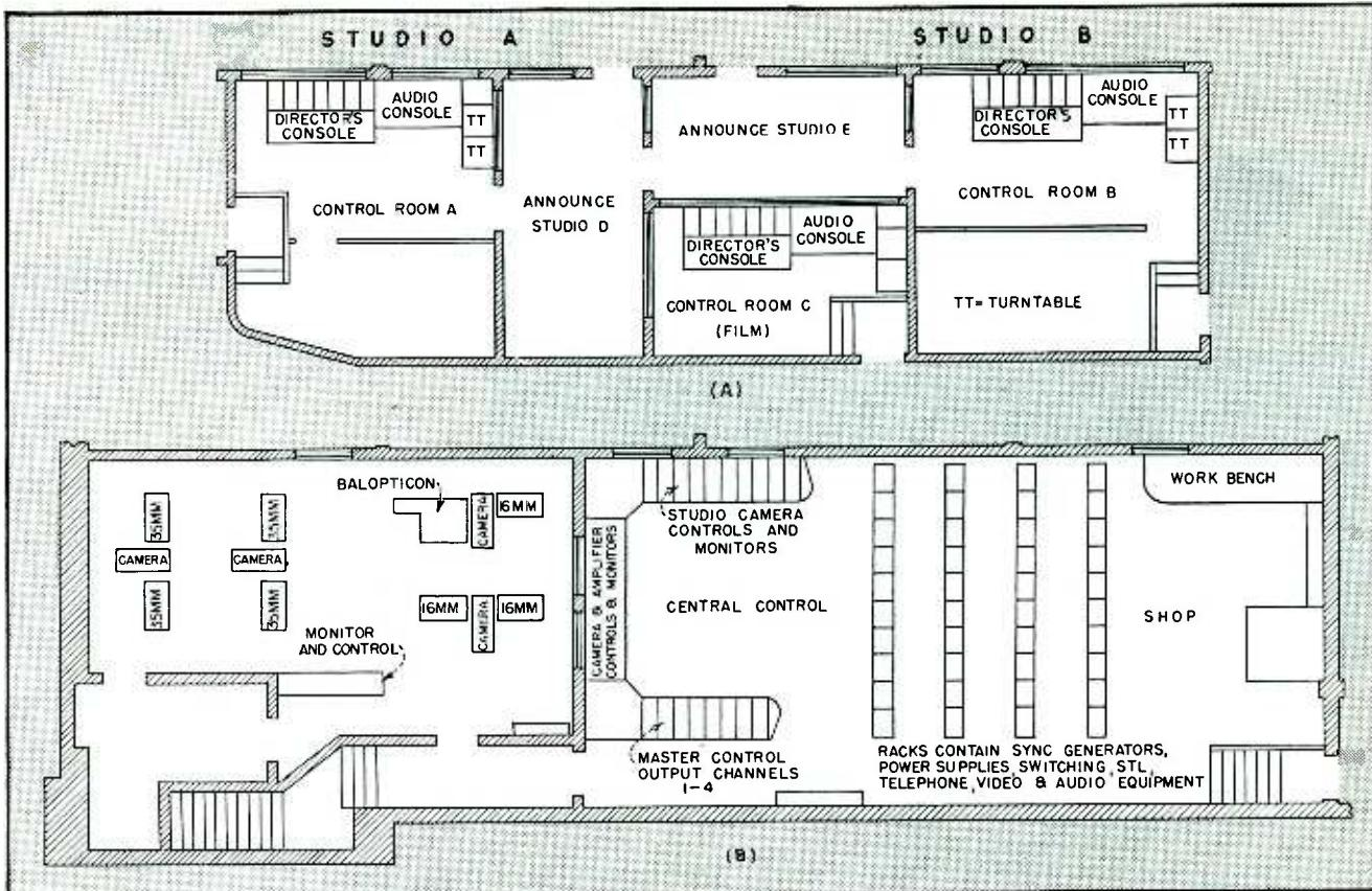
FIG. 9—Control areas in the studios. Program control rooms (A) are located at approximately studio floor level. Camera control and equipment (B) are located on floor above looking out over studios
