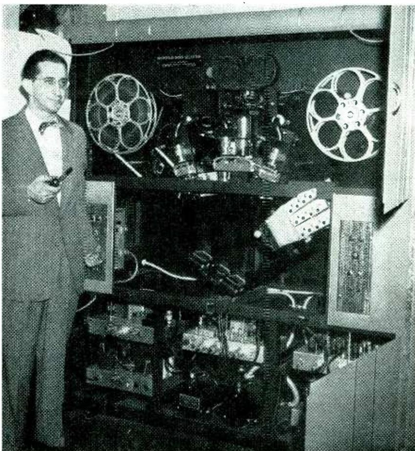
Microfilm Rapid Selector as developed and constructed by Engineering Research Associates, Inc., St. Paul, under the supervision of Ralph R. Shaw (left), librarian of the Department of Agriculture. Film on reels is scanned by phototube system while running through optical system at 300 feet per minute. The twelve phototubes used are in the bright metal housing set at 45 degrees under right-hand film reel
