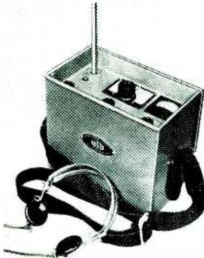
spot checks at 50 and 150 mc. Interference intensity is indicated in headphones and on a dual-scale meter having 0 to 100 and decibel graduations.
