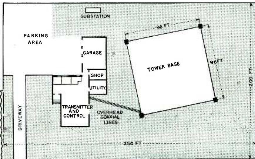
FIG. 2—Ground plan of the North Bergen property showing relation of the tower, transmitter building and power substation
