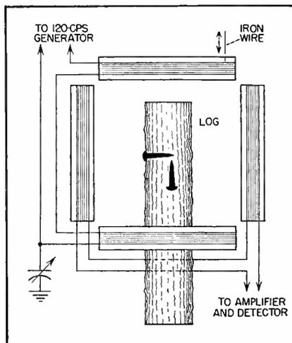
FIG. 2—Improved metal detection coil system which detects nails driven radially into a log as well as axially oriented objects
