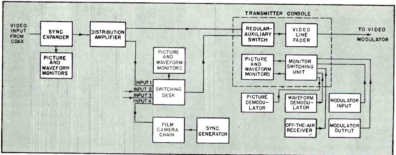
FIG. 8—Video signal switching and check points at the transmitter plant
