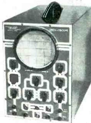
it has a horizontal sweep circuit of 15 to 30,000 cps. Frequency response of horizontal and vertical amplifiers is 50 cycles to 50 kc. It has an input impedance of 1 meg-ohm and 50  $\mu$ uf, and a deflection sensitivity of 0.30 volt per inch full gain.
