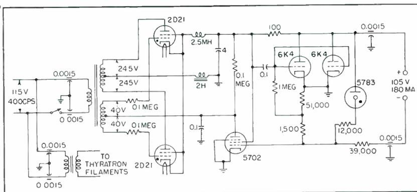
**FIG. 1**—Example of miniature thyatron regulated power supply circuit used with potted subassemblies to decrease size, weight and heating. Thorough shielding is necessary to avoid radiated noise from thyatrons. All 0.0015- $\mu$ f capacitors are ceramic feed-through units to prevent conducted noise
