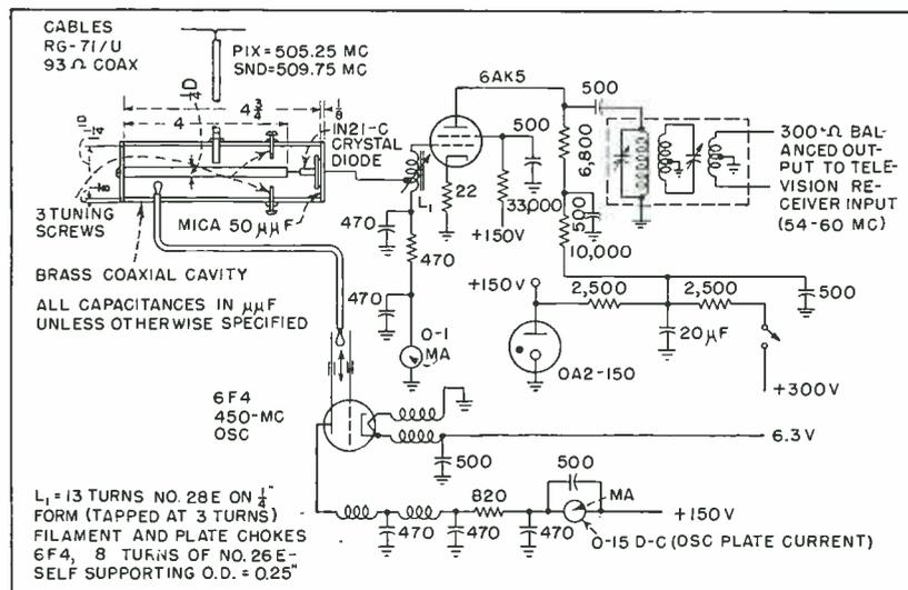
FIG. 1—Circuit diagram of the cavity-tuned 500-mc uhf television converter. The output is fed into a standard television receiver with 300-ohm balanced line
