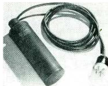
810 counts per minute from 5 micrograms of radium filtered through  $\frac{1}{2}$  in. of lead 12 inches from the end; has a maximum recovery time of 800 microseconds; a maximum dead time of 100 microseconds; is suitable for an input circuit impedance of 5 megohms; and has an ambient temperature rating of +40 to -70 C.
