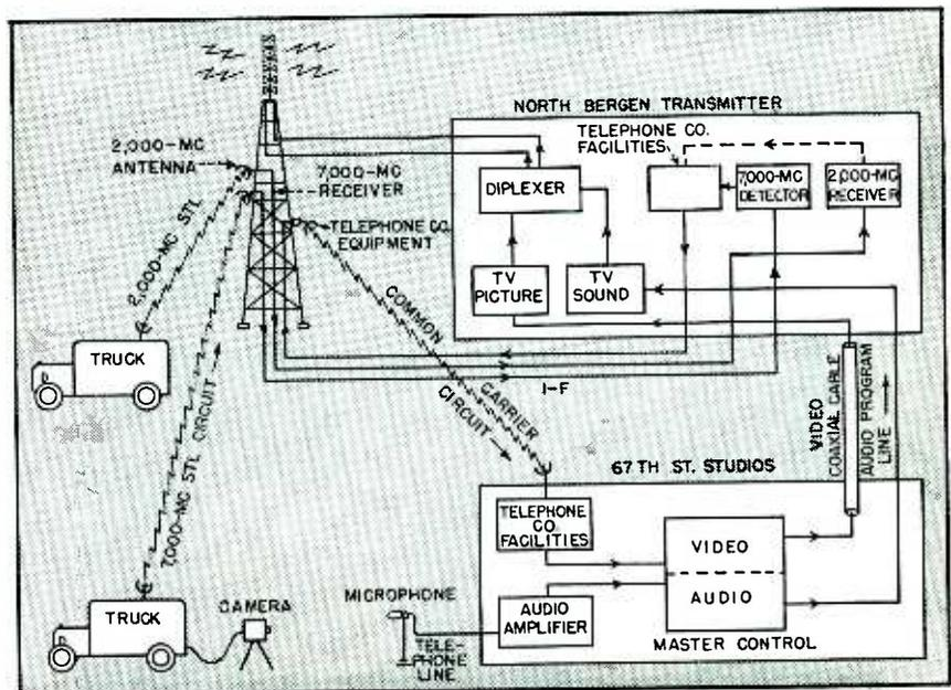
FIG. 7—Facilities are provided for carrying one remote while setting up for another simultaneously. Switching is done at studios and desired program fed back to transmitter
