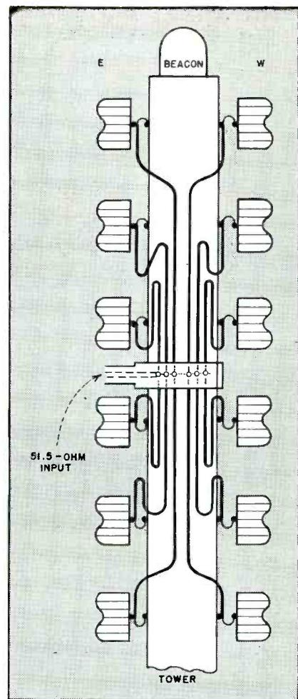
FIG. 3—Detail of the East-West feeder system to the television supertturnstile. The North-South feeders are identical
