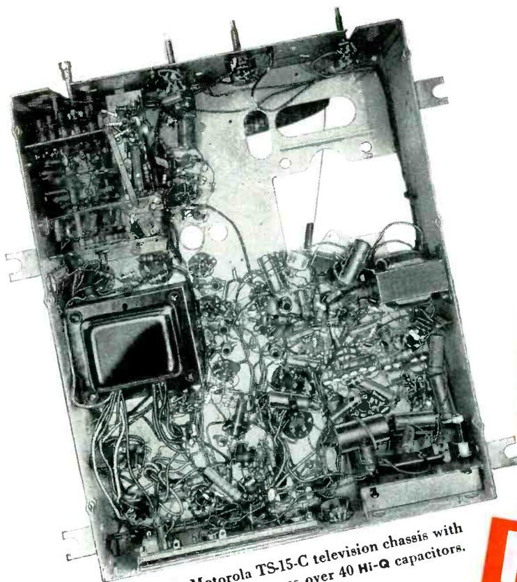
This Motorola TS-15-C television chassis with 12" picture tube uses over 40 Hi-Q capacitors.
