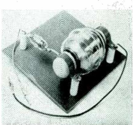
Photograph of a vacuum capacitor voltage divider. The values of the capacitors shown are 5 and 500  $\mu\text{f}$  with 17,500-volt ratings—Official Photograph U. S. Navy
