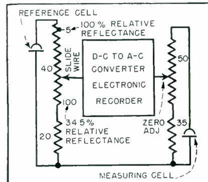
FIG. 4—Slide-wire photometer bridge circuit
