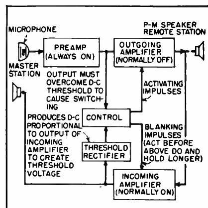
FIG. 2—Simplified block diagram of voice-controlled intercommunication system
