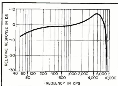
FIG. 2—Gain characteristic of the amplifier. At 1,000 cycles for 50 db the noise is 67 db below a milliwatt
