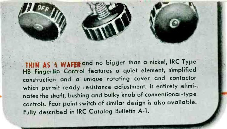
**THIN AS A WAFER** and no bigger than a nickel, IRC Type HB Fingertip Control features a quiet element, simplified construction and a unique rotating cover and contactor which permit ready resistance adjustment. It entirely eliminates the shaft, bushing and bulky knob of conventional-type controls. Four point switch of similar design is also available. Fully described in IRC Catalog Bulletin A-1.
