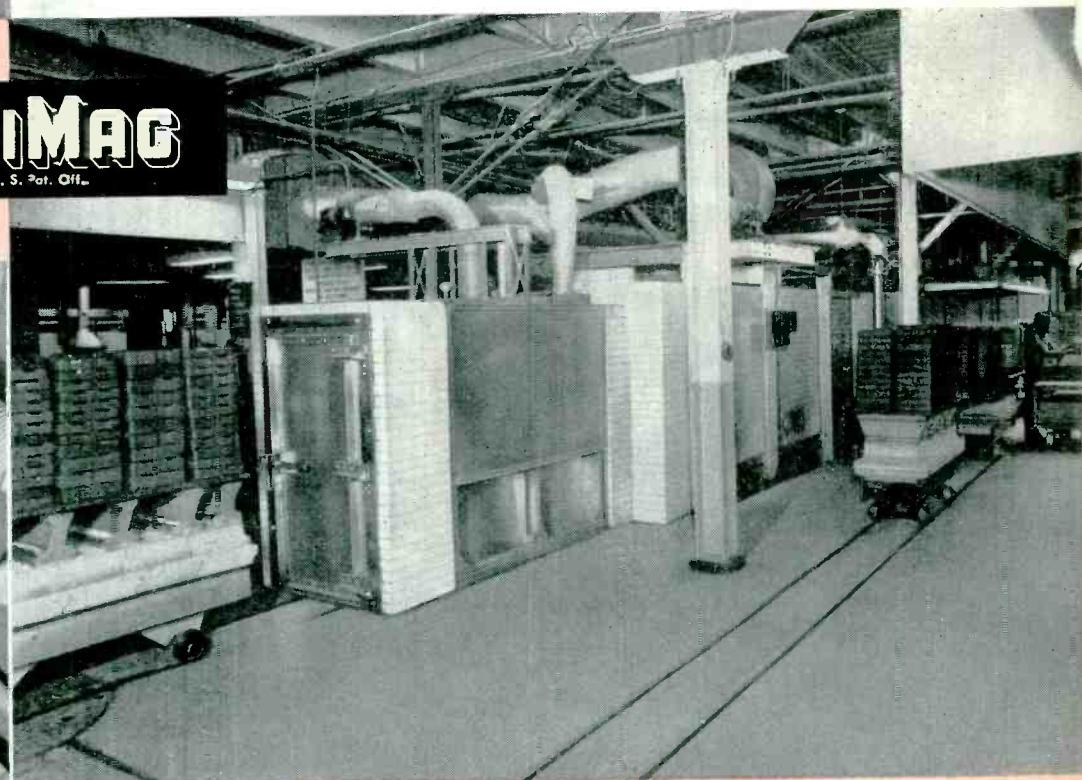
Side view of one of AlSiMag's tunnel kilns. All kilns, both circular and tunnel, are handled from one centralized control panel.
