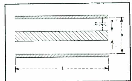
FIG. 1—Basic concept of coaxial line used to develop wavemeter
