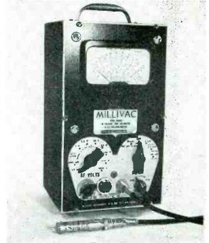
200 mc flat within 10 percent. The unit can also be used with a calibration chart for frequencies as high as 2,500 mc, with 10 mv being the lowest readable voltage.
