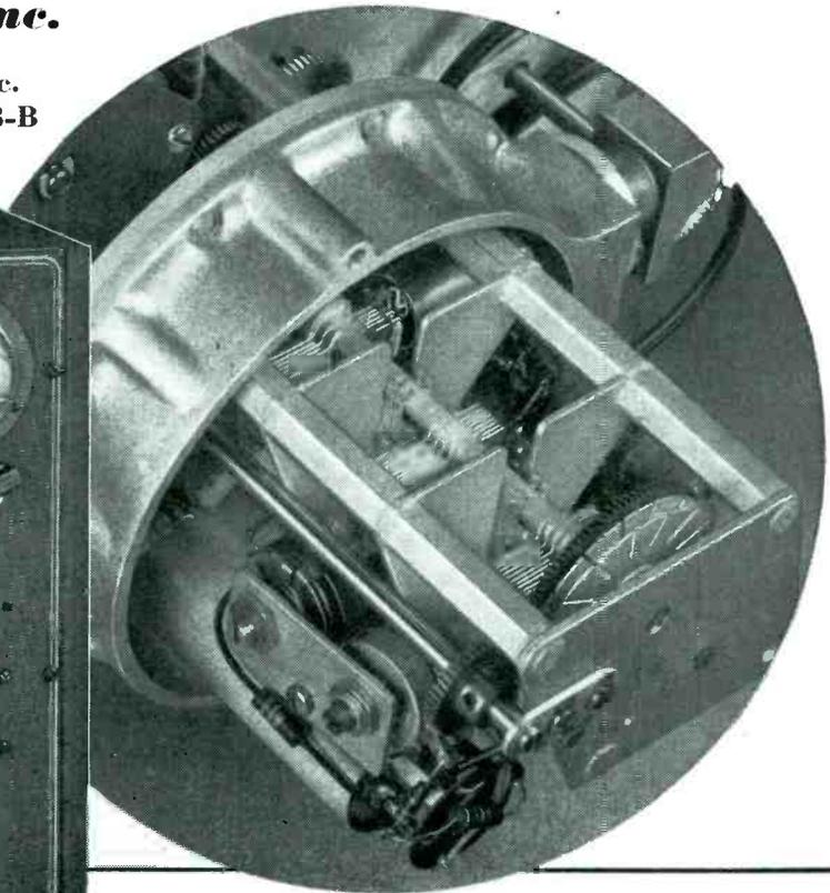
Shown above is an interior view of the 202-B Signal Generator RF assembly with shield cover removed. Heavy aluminum castings form the mounting base of this RF unit resulting in a compact and highly rigid structure. Girder type condenser frame construction, multiple rotor shaft grounding contacts, and welded interstage shield plates are but a few of the many design features of this unit which give added circuit stability.
