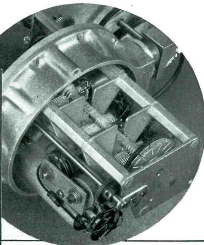
Shown above is an interior view of the 202-B Signal Generator RF assembly with shield cover removed. Heavy aluminum castings form the mounting base of this RF unit resulting in a compact and highly rigid structure. Girder type condenser frame construction, multiple rotor shaft grounding contacts, and welded interstage shield plates are but a few of the many design features of this unit which give added circuit stability.
