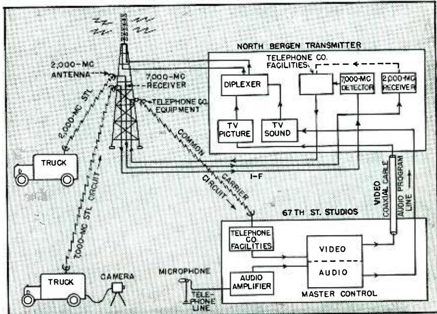
FIG. 7—Facilities are provided for carrying one remote while setting up for another simultaneously. Switching is done at studios and desired program fed back to transmitter
