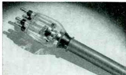
This tube is designed to supersede type 892 in R. F. Heating equipments and directly replaces it without equipment modifications. The ML-5606 incorporates all of the features of the ML-5668 except that it is provided with a standard type 892 anode to fit existing 892 sockets.
