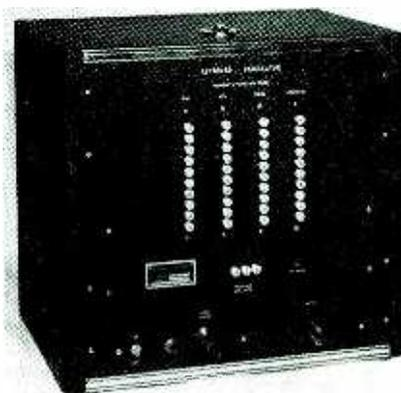
board oscillator covering a range from 0.3 cycle to 100 kc with decades of pushbuttons. Frequency accuracy for the lower ranges up to 10,000 cycles is 0.1 percent plus 0.1 cycle. If there is no abnormal change in room temperature, frequency drift after a short warmup period is less than 0.02 percent per hour.
