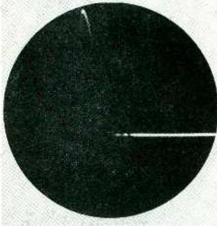
▶ At low operating voltages the cathode-ray tube will respond to a high-speed transient signal, but—only at high voltages is the light output sufficient to SEE and RECORD it.
