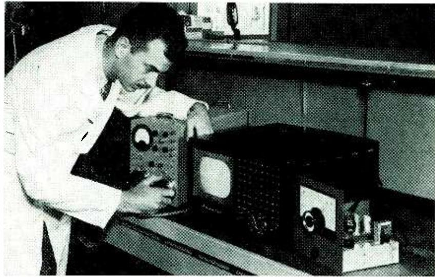
Fixed-tuned converter being tested in conjunction with a standard television receiver.
