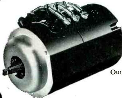
**SYNCHRONOUS DIFFERENTIAL UNITS:** electro-mechanical error detectors with mechanical output for use in position or speed control servo systems. These torque-producing half-speed synchros are composed of two variable frequency synchronous motors and a smoothly operating system of differential gearing
