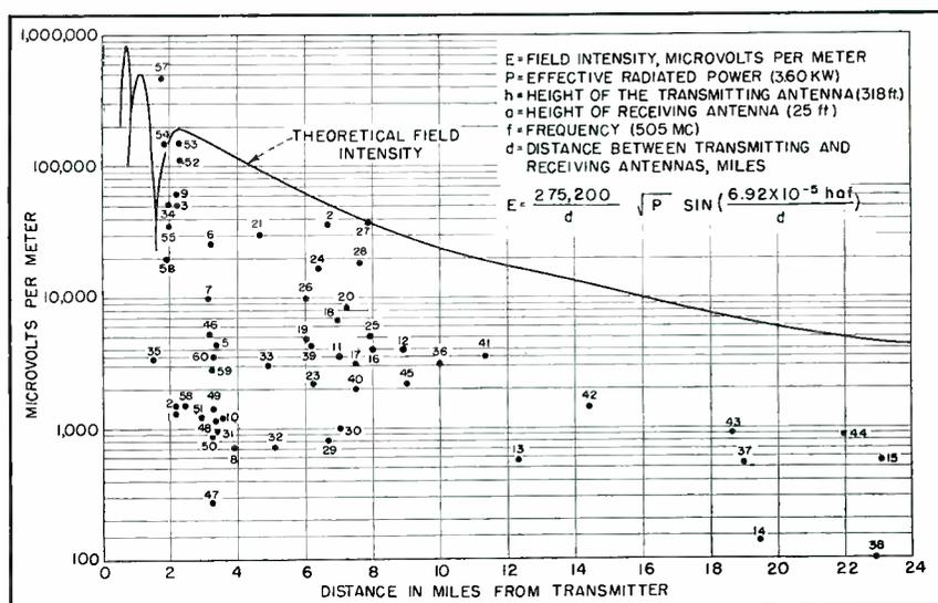
FIG. 4—Curve showing theoretical field strength (assuming flat earth) and typical measured values
