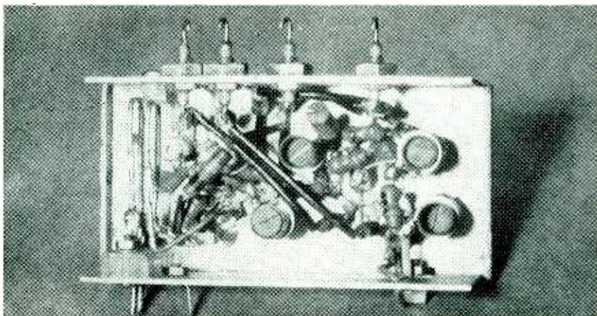
FIG. 9—Bottom view of 205-mc i-f amplifier. Chassis is approximately 2 inches wide and 4½ inches long
