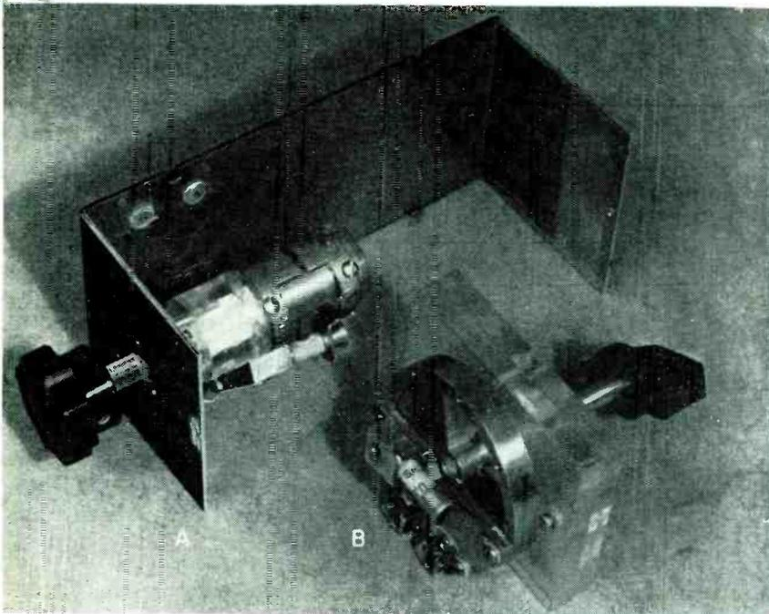
FIG. 4—A rolled-up line mixer is shown at A and a semi-butterfly mixer at B
