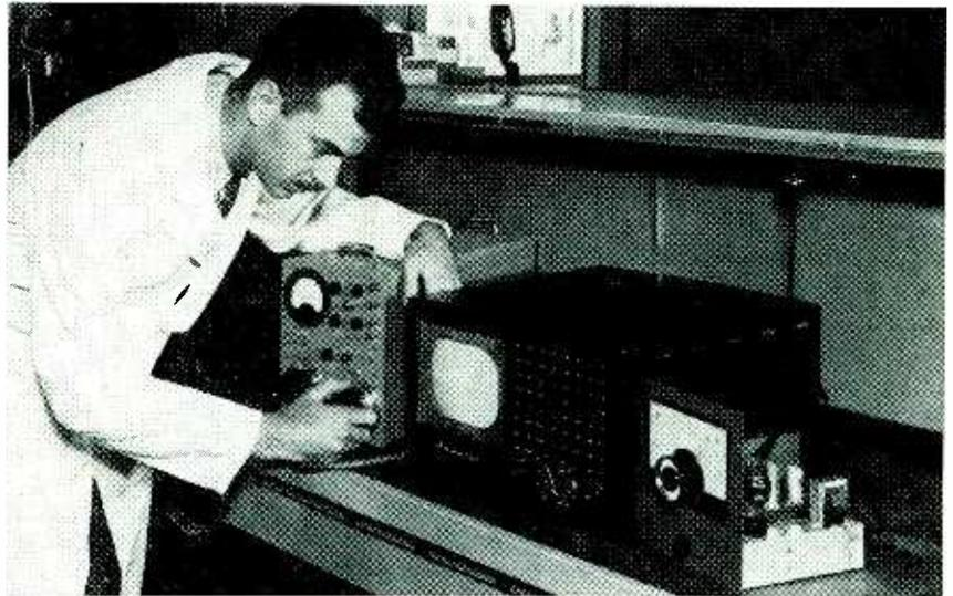
Fixed-tuned converter being tested in conjunction with a standard television receiver. Vernier tuning of the local oscillator is provided
