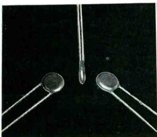
**6** For by-pass or coupling applications, check Centralab's original line of ceramic disc Hi-Kaps. Disc Hi-Kaps are smaller than a dime!
