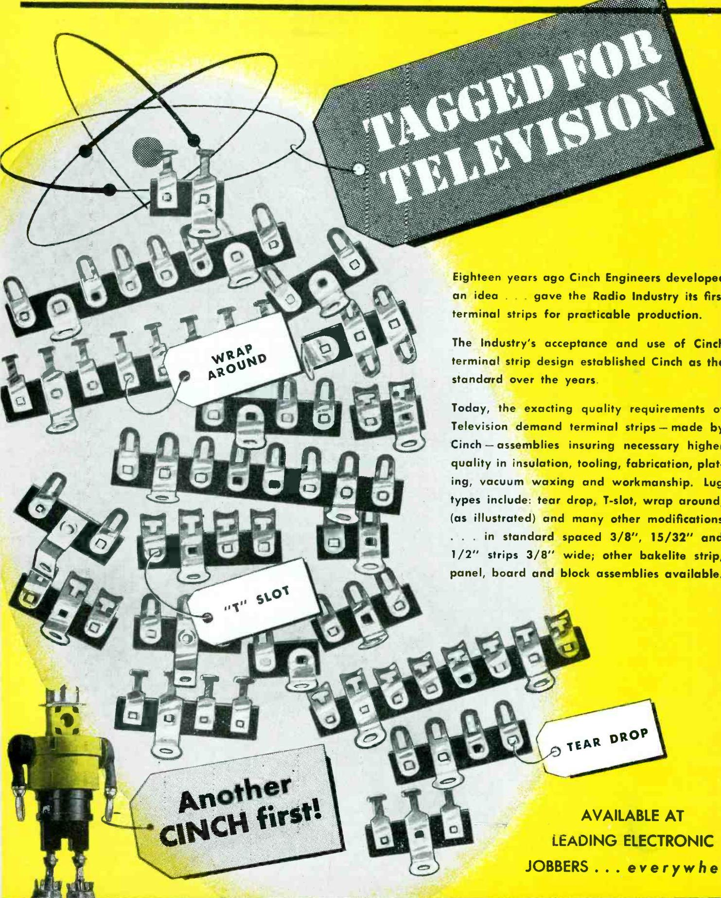
Eighteen years ago Cinch Engineers developed an idea . . . gave the Radio Industry its first terminal strips for practicable production.
