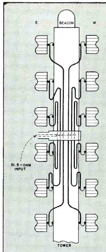
FIG. 3—Detail of the East-West feeder system to the television superturnstile. The North-South feeders are identical
