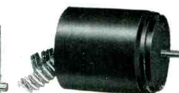
**INDUCTION MOTORS:** miniature 2-phase motors of the squirrel cage type. Designed specifically to provide fast response to applied control signals and maximum torque at zero r.p.m. Unit shown weighs 6.1 oz. and has stalled torque of 2.5 oz. in.
