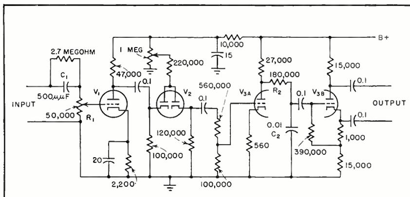
FIG. 3—Fixed station instantaneous deviation control circuit
