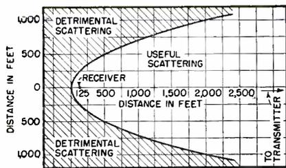
FIG. 3—Plan view of receiver vicinity showing areas of useful and detrimental scattering
