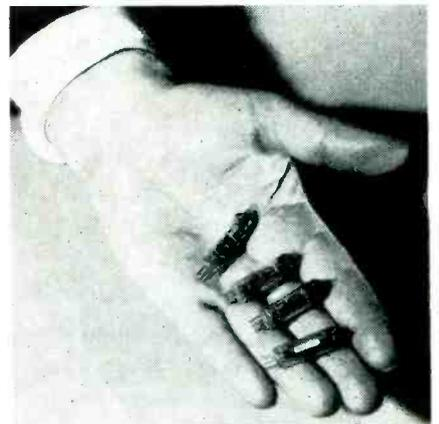
at 1.25 v and 40 ma d-c. Plate voltage ranges from 30 to 67.5 volts, and plate currents, from 0.30 ma to 2.0 ma.
