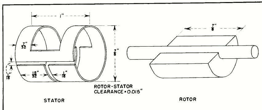
FIG. 6—Mechanical details of the rolled-up line
