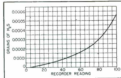
FIG. 3—Basic calibration of the analyzer
