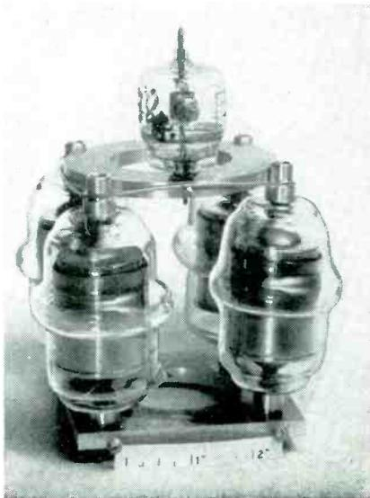
Vacuum capacitor voltage divider using tube plate-to-filament capacitance in series with four  $50-\mu\text{f}$  vacuum capacitors connected in parallel—Official Photograph U. S. Navy
