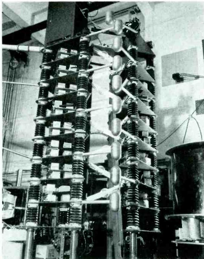
An 8 stage capacitor-rectifier multiplier. This unit is used in the "Racetrack" Synchrotron of the University of Michigan
