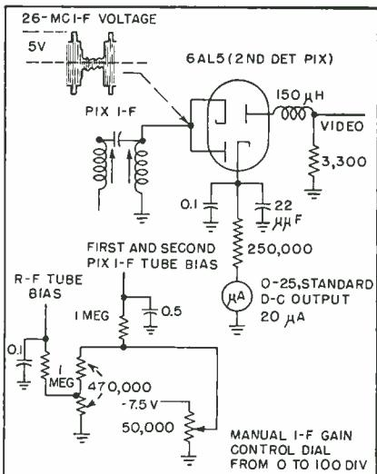
FIG. 2—Schematic diagram of special vtvM and manual gain control circuits
