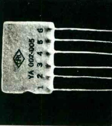
**1** Pentode Couplate consists of plate lead and grid resistors, plate by-pass and coupling capacitors. Minimum soldered connections speed production.
