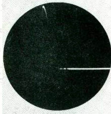
At low operating voltages the cathode-ray tube will respond to a high-speed transient signal, but—only at high voltages is the light output sufficient to SEE and RECORD it.
