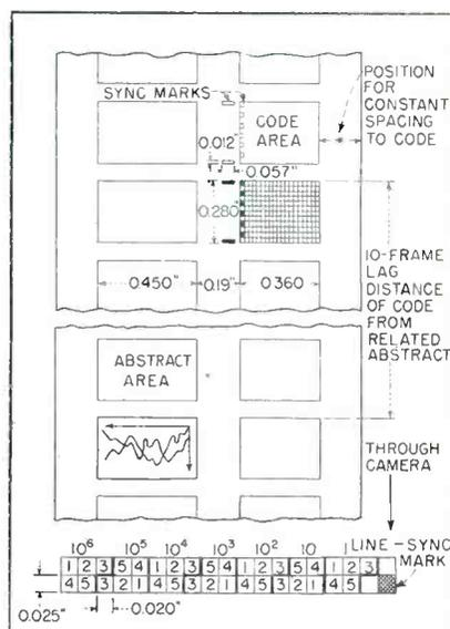
FIG. 1—Arrangement of abstract and code areas on master film, and method of assigning code numbers to squares to accommodate 10,000,000 different subjects
