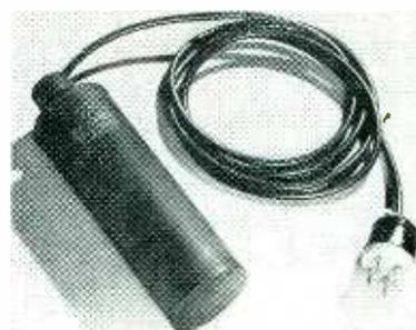
810 counts per minute from 5 micrograms of radium filtered through  $\frac{1}{8}$  in. of lead 12 inches from the end; has a maximum recovery time of 800 microseconds; a maximum dead time of 100 microseconds; is suitable for an input circuit impedance of 5 megohms; and has an ambient temperature rating of +40 to -70 C.
