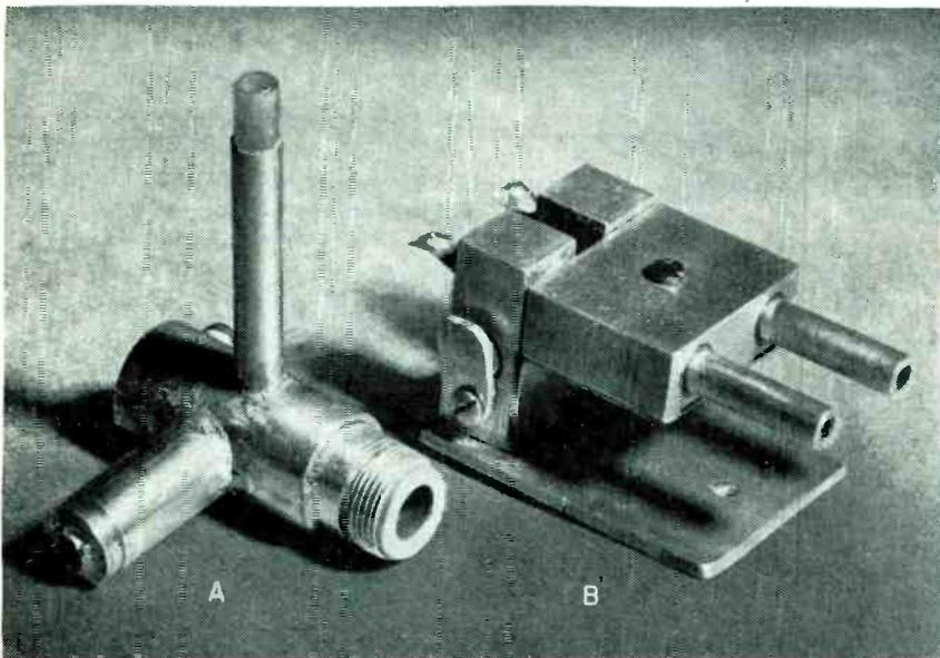
FIG. 5—A coaxial form of mixer is shown at A and a parallel-line mixer at B
