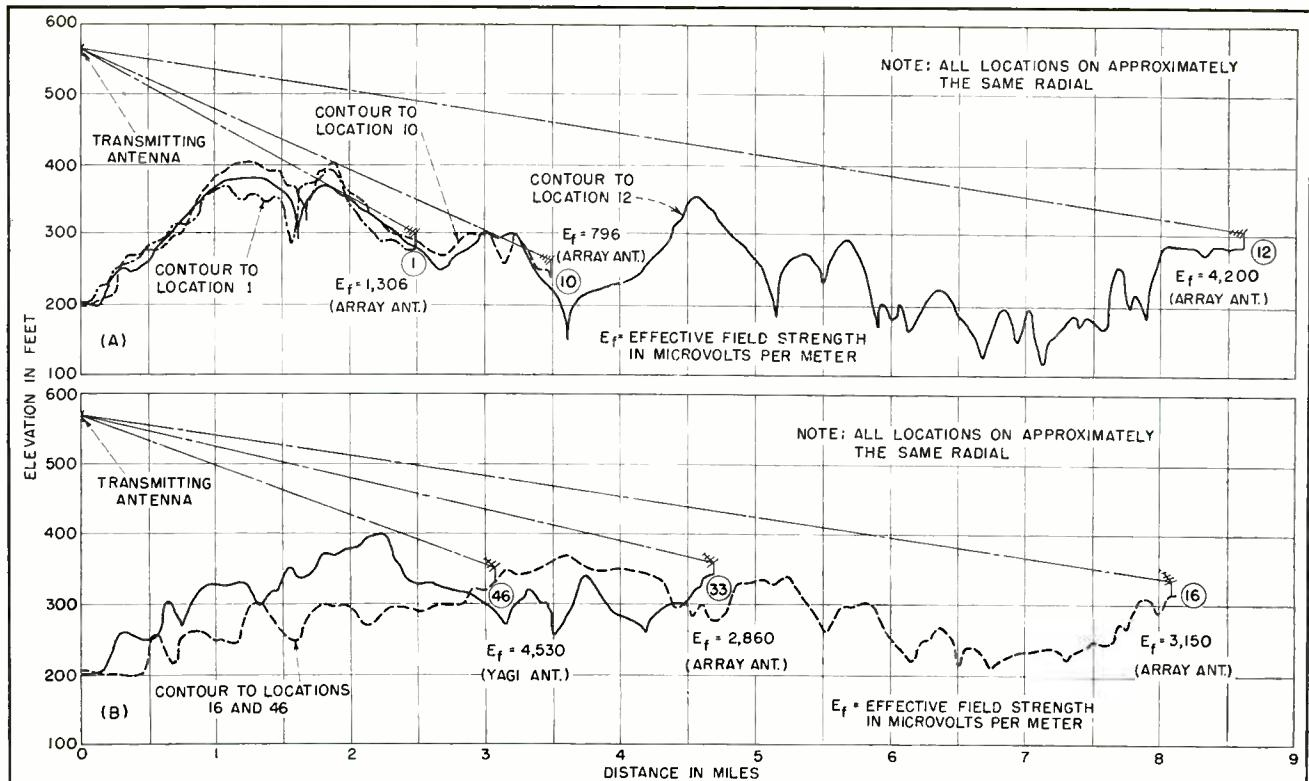
FIG. 5—Ground contours for radials containing typical measuring locations. It may be seen that the field strength at any location is highly affected by the existence of obstructions between transmitter and receiver.
