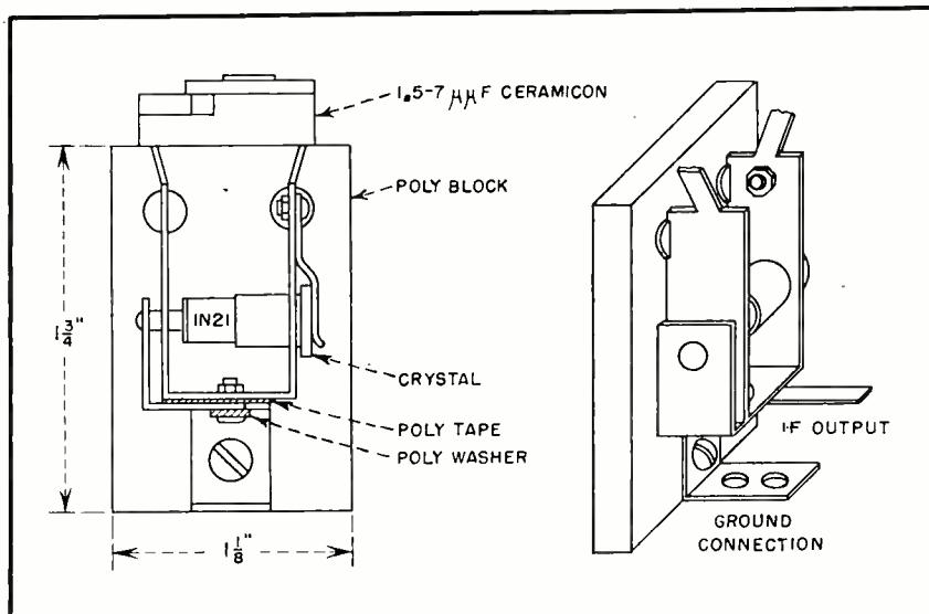
FIG. 7—Simple fixed-tuned mixer for 530 mc
