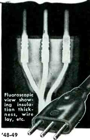
Fluoroscopic view showing insulation thickness, wire lay, etc.
