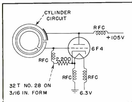
FIG. 2—Circuit of the cylinder oscillator
