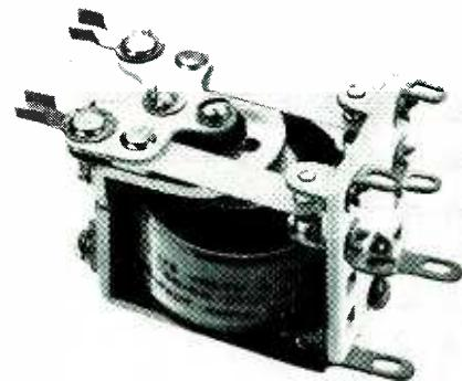
ture and stationary contact assemblies. Coil data: a-c coils, consuming approximately 4 volt-amperes, available up to 220 volts; d-c coils, consuming 1 to 2 watts, available up to 110 volts. Overall dimensions are 15/16 x 1 7/8 x 1 9/16 inches.
