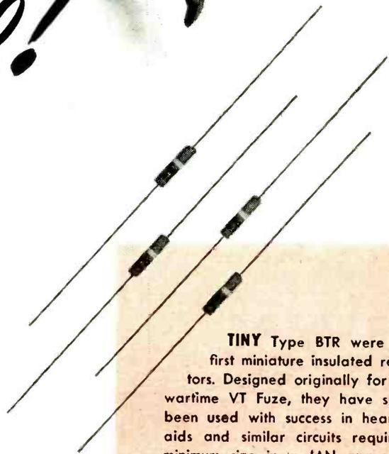
**TINY** Type BTR were the first miniature insulated resistors. Designed originally for the wartime VT Fuze, they have since been used with success in hearing aids and similar circuits requiring minimum size in a JAN approved resistor.  $\frac{1}{3}$  watt rating ranges up to 220 ohms. Convenient coupling.
