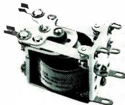
ture and stationary contact assemblies. Coil data: a-c coils, consuming approximately 4 volt-amperes, available up to 220 volts; d-c coils, consuming 1 to 2 watts, available up to 110 volts. Overall dimensions are 15/16 x 1 $\frac{1}{8}$  x 1 $\frac{9}{16}$  inches.
