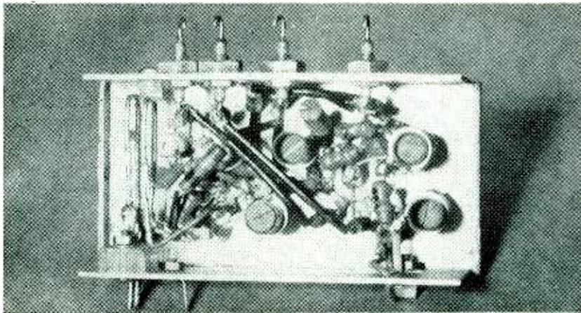
FIG. 9—Bottom view of 205-mc i-f amplifier. Chassis is approximately 2 inches wide and 4 3/4 inches long
