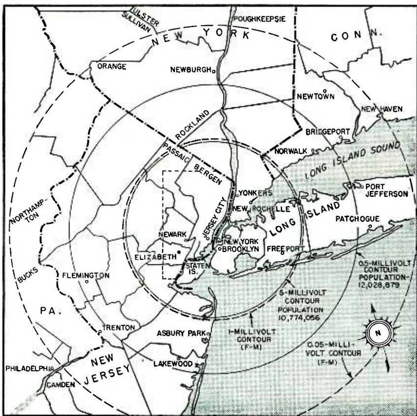
FIG. 1—Service areas for WOR-TV (solid lines) and WOR-FM (dashed lines). Note that the contours for tv and f-m are not directly comparable
