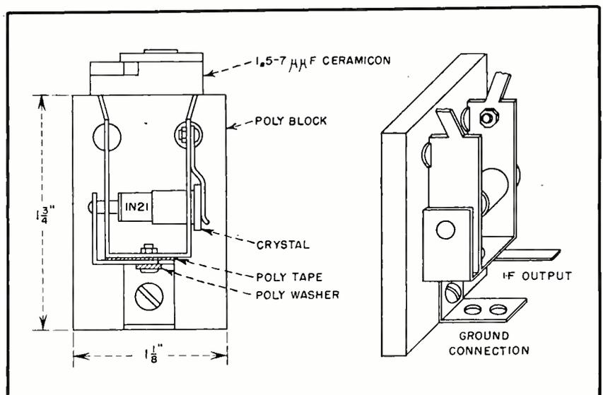
FIG. 7—Simple fixed-tuned mixer for 530 mc
