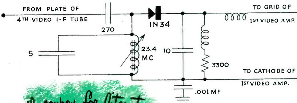
Portion of diagram of the Magnavox Embassy, showing the 1N34 used as the video detector.
