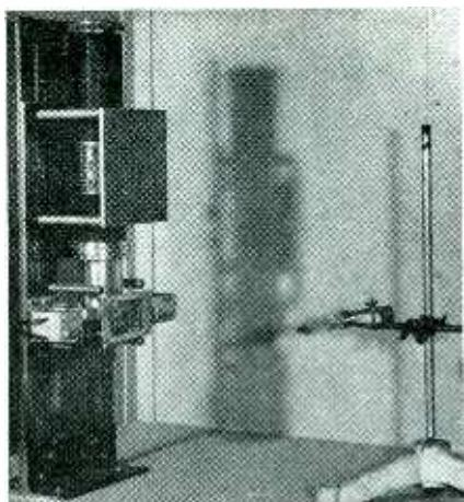
Experimental arrangement used at National Bureau of Standards to expose a nylon thimble chamber to x-rays from a beryllium-window x-ray tube mounted behind a solenoid shutter control which admits definite amounts of radiation to the thimble ionization chamber
