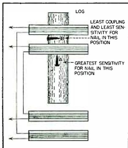
FIG. 1—Top view of two mutual inductance coils arranged in the regular way for use with the Felici mutual inductance bridge
