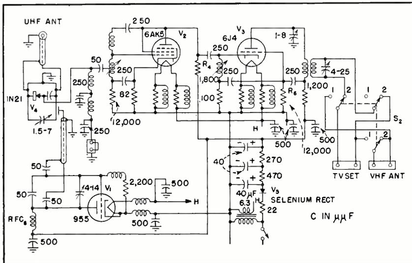
FIG. 8—Complete circuit of a converter with output on channel 12
