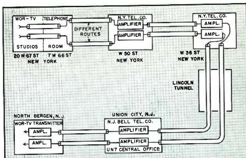
FIG. 6—Simplified diagram of the coaxial cable circuits between studios and transmitter
