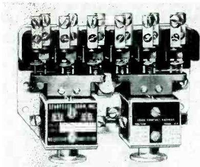
175KXX contactor comprises two 3-pole solenoids for forward and reverse operation mounted on a common frame and mechanically interlocked to prevent simultaneous closure. Designed particularly for service in the control of single horsepower motors, the use of the contactor is completely described in bulletin 7100.
