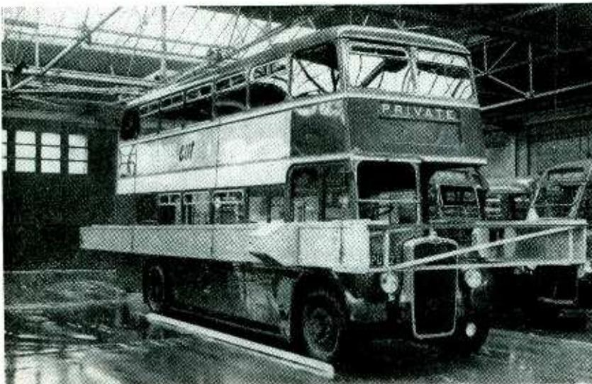
Both sides of the bus are embraced simultaneously by the trough while being washed
