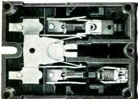
Showing the sure-contact spring in switch assembly.
