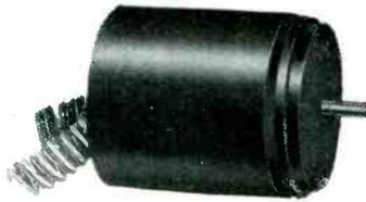
**INDUCTION MOTORS:** miniature 2-phase motors of the squirrel cage type. Designed specifically to provide fast response to applied control signals and maximum torque at zero r.p.m. Unit shown weighs 6.1 oz. and has stalled torque of 2.5 oz. in.
