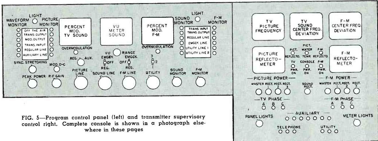
FIG. 5—Program control panel (left) and transmitter supervisory control right. Complete console is shown in a photograph elsewhere in these pages
