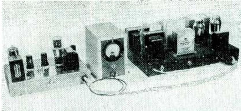
Metal detector chassis, power supply and meter which is used to zero the instrument and to give an indication for extremely small metallic objects where the relay would not normally be operated
