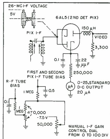
FIG. 2—Schematic diagram of special vtm and manual gain control circuits
