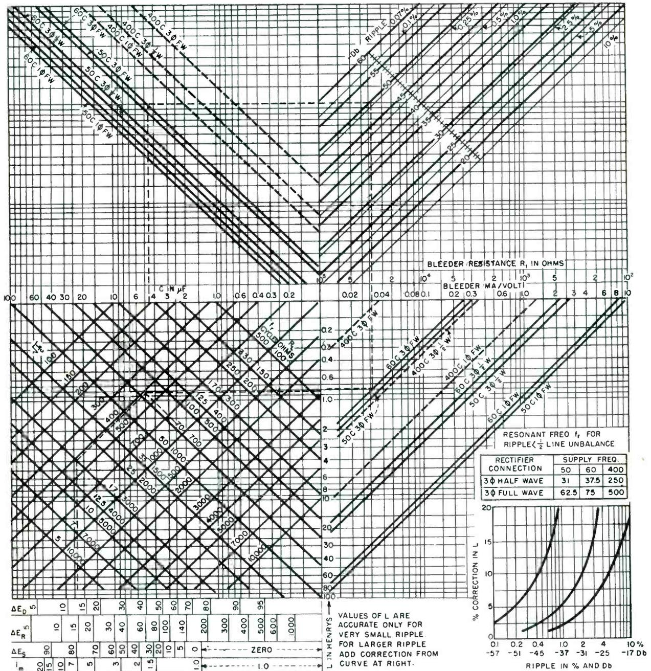
1. Assume suitable value of bleeder resistance or bleeder current  $I_1$  in ma per volt of  $E_{d-c}$ . This is also steady-state peak ripple current in ma.
