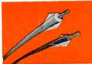
**HEAT-RESISTANT** nylon-jacketed wire, made by Gavitt Manufacturing Co., Brookfield, Mass., in two types: 1/64" wall thickness with 300-volt rating, and 1/32" wall thickness with 600-volt rating—both with 5-mil extruded nylon jackets.
