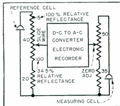
FIG. 4—Slide-wire photometer bridge circuit
