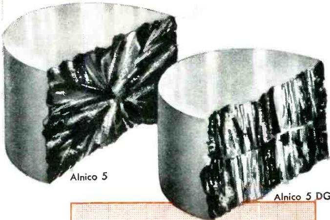
Here is the Alnico 5 DG compared with Alnico 5. Note the directional grain structure that imparts a greater energy potential. Note the reduction of size in Alnico 5 DG.
