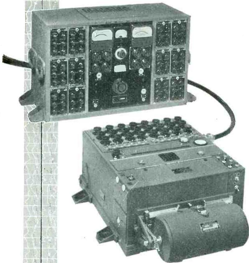
Illustrated is a complete 12-channel portable laboratory for precision strain determination from static strain to a frequency of 5000 cycles per second, using resistance gages that are attached by cement to the points of strain.
