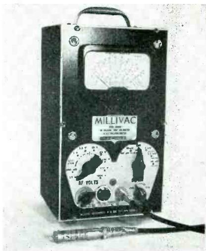
200 mc flat within 10 percent. The unit can also be used with a calibration chart for frequencies as high as 2,500 mc, with 10 mv being the lowest readable voltage.
