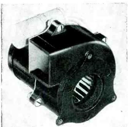
Jamaica 1, N. Y. Model 805J is a small centrifugal blower designed for electronic tube cooling and for ventilating small enclosed areas. Performance data are as follows: voltage, 115, 60-cycles a-c; current, 0.150 amp; speed, 3,599 rpm; input, 15 watts, power factor, 85 percent; capacitor required, 0.5  $\mu$ f, 300 volts a-c. Weight is 24 ounces.
