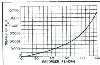
FIG. 3—Basic calibration of the analyzer
