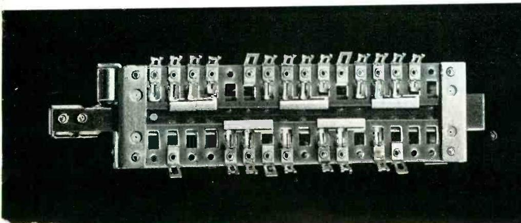
Centralab's development of a revolutionary, new Slide Switch gives you improved and FM response! Flat, horizontal design saves valuable space, allows short connection to coils, reduced lead inductances for increased efficiency and frequency response. CRL Slide Switches are rugged and dependable.
