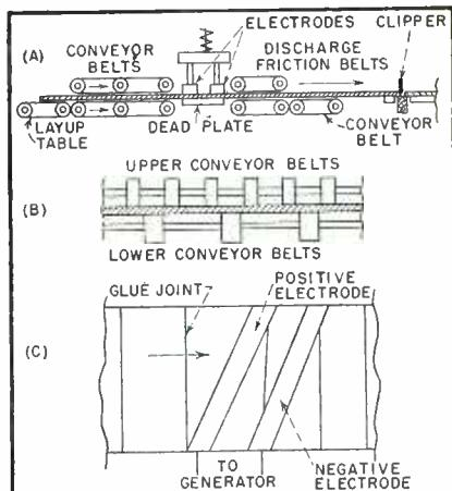
FIG. 1—Setup for r-f wood veneering machine
