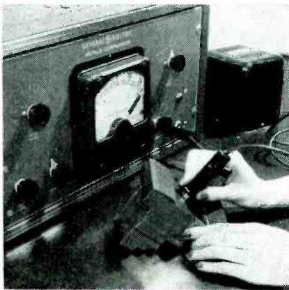
ring separated from a concentric core by an air gap, thereby forming a radial magnetic path across which the test piece is placed. Three inches long, it can be supplied in various face diameters depending upon the application.
