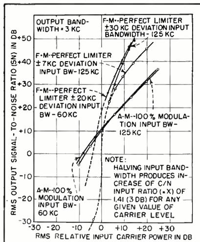
Comparison of theoretical a-m and f-m range performance with decrease of input bandwidth and different frequency deviations
