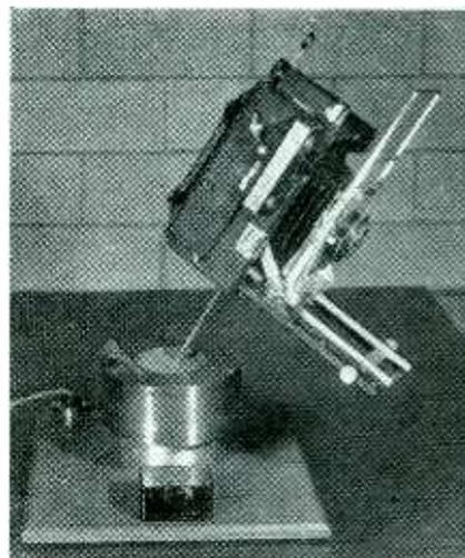
Demonstration of use of magnetic fluid as universal positioning device for heavy camera. Fluid in nonferrous metal cup solidifies around camera support rod when coil surrounding cup is energized with d.c. Current is interrupted with switch in foreground whenever camera needs repositioning
