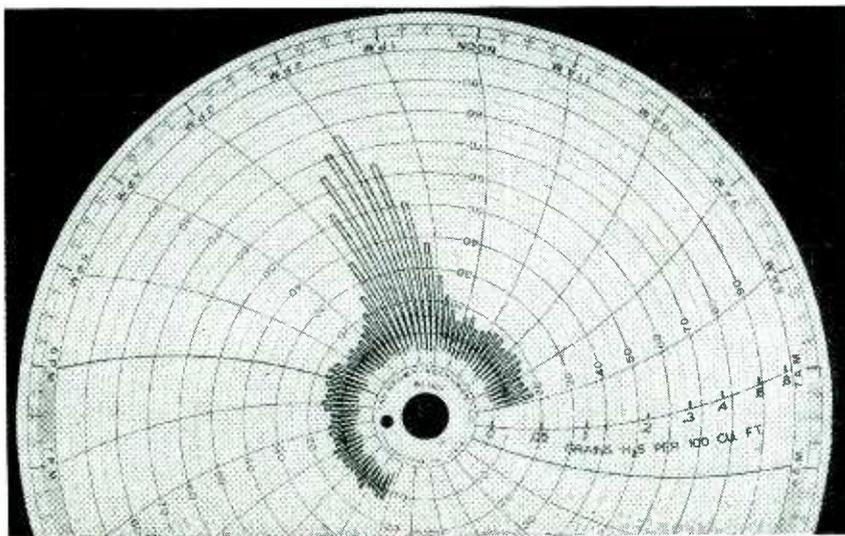
FIG. 2—Portion of a typical hydrogen sulfide analyzer record covering several hours showing a 10-minute test period in each 15-minute cycling period
