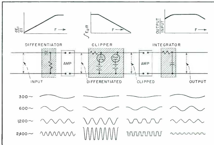
FIG. 1—Basic circuits illustrating the fundamental principle
