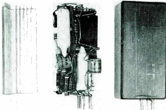
Steps in potting a three-tube strain gage amplifier. Left—casting-resin chassis with imbedded silver-clad beryllium-copper wires serving as stiffeners, tie points, plug prongs and lead wires. Center— assembled chassis with built-in limiter and voltage gain of 20,000, adjusted in production so all units have same gain within 1 percent. Right—complete plug-in unit as potted in casting resin. Other examples of potted plug-in units are shown in color on the front cover of this issue
