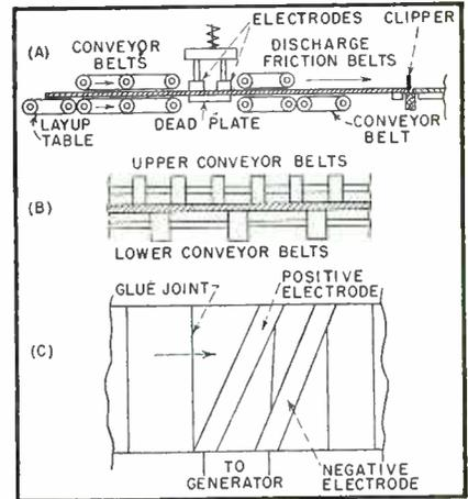
FIG. 1—Setup for r-f wood veneering machine
