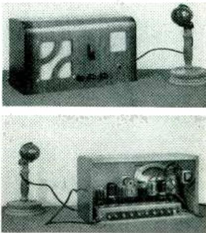
FIG. 3—Front and rear views of typical master station
