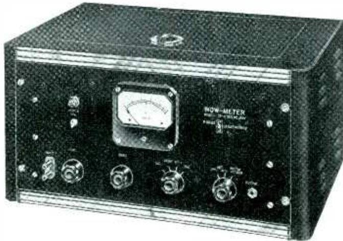
Newly developed direct-reading instrument simplifies measurements of wow and flutter in speed of phonograph turntables, wire recorders, motion picture projectors and similar recording or reproducing mechanisms. It is the only meter in existence giving direct steady indication of meter pointer on scale.
