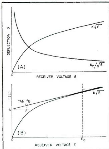
FIG. 1—Curves for determining the ratio of p-m to e-m magnetic field for combination focus compensation of television receivers
