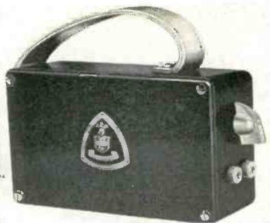
ard flashlight batteries power the unit through a vibrator power supply which furnishes the high voltage for the Geiger tube. Practically any magnetic type single or double phones having 1,000 to 24,000 ohms impedance can be used with the instrument. Further details may be found in bulletin E-5.
