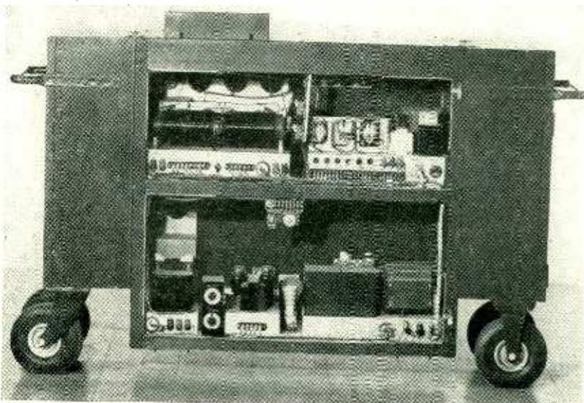
The entire transmitter is contained in a portable dolly so that it can be moved rapidly from one set to another
