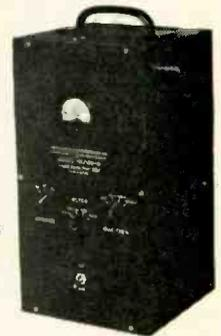
**TS/170-C GLIDE PATH TEST SET**... Battery operated portable test oscillator which provides a crystal-controlled signal at 332.6, 333.8 or 335 mcs., which may be 30% modulated from an internal source at 90, 150, 1000 cps. or unmodulated as desired, for glide path channels GX, GY, and GZ.
