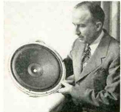
drives the small cone section to produce the high frequencies; and a 2-inch voice coil drives the large cone section to produce the lower frequencies. The unit employs a 2-pound Alnico V magnet.
