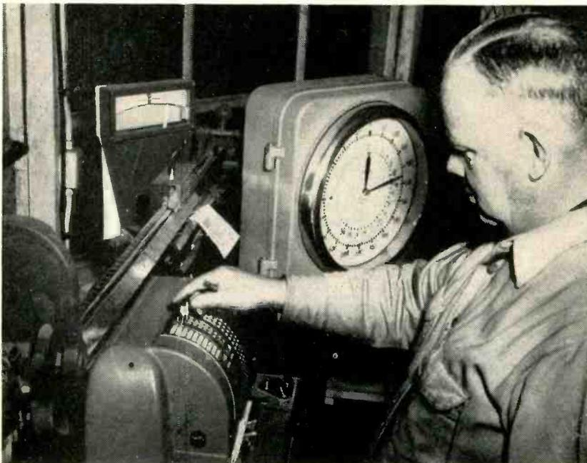
Operator sets up information to be printed, along with weight of cattle, by electronic live stock weighing instrument. Old beam-type scale may be seen in background. Scale is calibrated from zero to 50,000 pounds.
