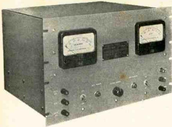
**Left: MODEL PSR-100**... 30 to 500 volts D.C. at 0 to 300 ma. 6.3 volts A.C. center-tapped at 6 amp; 1/2% or better regulation under any conditions of operation within ratings. 10 MV. or less peak-to-peak ripple voltage. Output impedance effectively zero. High voltage continuously variable from 0 to 500 volts.
