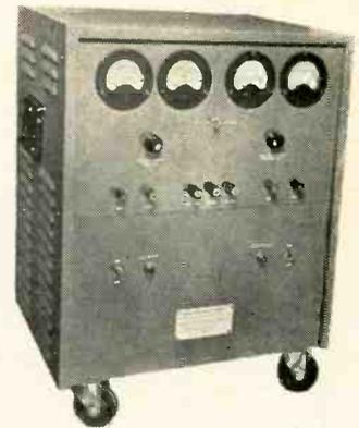
**Above, right: MODEL PSR-105**... 200 to 400 volts D.C. at 0 to 200 ma. from each of two separately controlled outputs, or 200 to 400 volts D.C. at 0 to 400 ma. 6.3 volts A.C. center-tapped at 10 amp; 1/2% or better regulation under any conditions of operation within ratings. 10 MV or less peak-to-peak ripple voltage. Output impedance effectively zero. Output voltages continuously variable. NET PRICE F.O.B. FACTORY.....\$695.00
