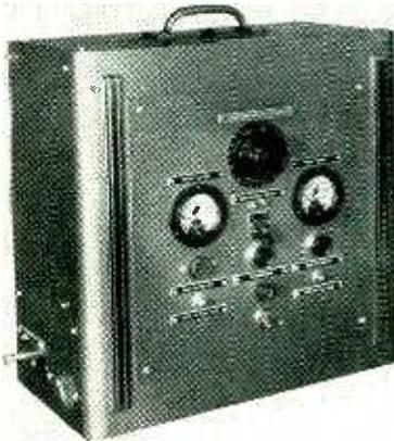
power supply operates on an input of 117 volts, 50 or 60 cycles, 225 volt-amperes maximum. Output voltage is continuously variable from 0 to 30 kv d-c; output current, 2 ma maximum, approximately 300  $\mu$ a at 30 kv.
