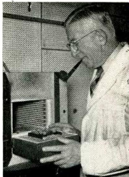
Oven used in initial trials of new Signal Corps process for eliminating aging characteristics of finished quartz crystal blanks. Development of process is credited to David G. McCaa (above), Arthur G. Prichard and Maurice A. A. Druesne, all Signal Corps physicists
