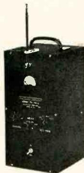
**TS/173-C LOCALIZER TEST SET**—Left... Battery operated portable test oscillator which provides a crystal controlled signal at 108.3, 108.7, 109.1, 109.5, 109.9, or 110.3 mcs., which may be 30% modulated from an internal source at 90, 150, 1000 cps. or unmodulated as desired, for localizer channels U, V, W, X, Y and Z.
