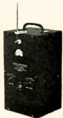
**MB-2 MARKER BEACON TEST UNIT**—Right... A crystal controlled, portable, 75-megacycle transmitter whose output may be tone-modulated at 400, 1300 or 3000 cycles per second, as desired.
