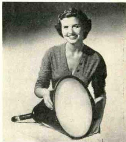
rect view television tube, is supplied with a heater rated at 6.3 volts, a-c or d-c and 0.6 ampere for unipotential cathode. Magnetic deflection, focusing and ion trap auxiliaries are required. Operating voltage of the high-voltage anode is 12,000 volts; of the focusing anode, 300 volts; and of the control grid, -33 to -77 volts. Overall length of the tube is 22½ in.
