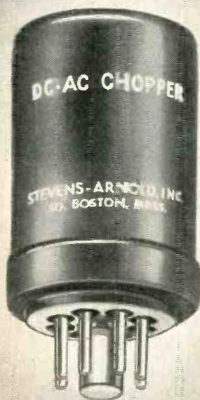
These Choppers convert low level DC into pulsating DC or AC so that servo-mechanism error voltages and the output of thermocouples and strain gauges, may be amplified by means of an AC rather than a DC amplifier.
