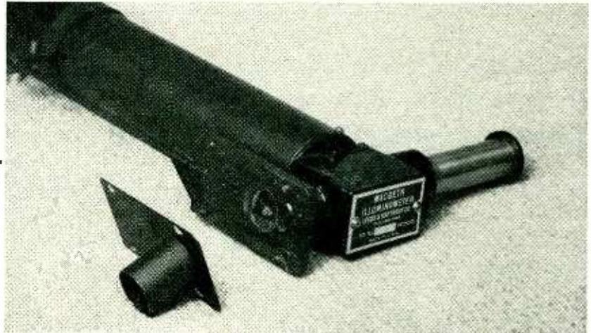
FIG. 5—Measuring unit employs microscope cover glasses for the neutral filter
