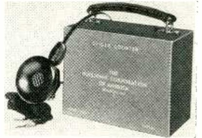
counter for prospectors. Two pounds in weight, the instrument may be clipped to the belt, allowing freedom of both hands. Clicks in an earphone and a flashing light indicate the presence of radioactive ore.
