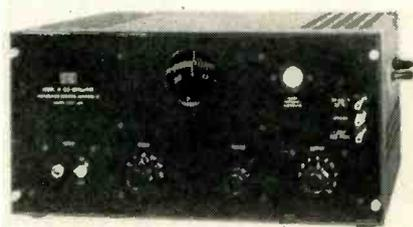
liver 20 volts across 1,000 ohms or 20 ma rms, and the other has a constant internal resistance of 250 ohms and an open circuit voltage of 1 volt. Power supply noise is less than 0.01 percent of the output signal. Harmonic distortion is less than 0.2 percent from 20 to 15,000 cps.
