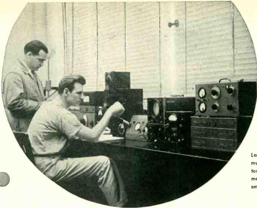
*Laboratory Controlled*—Every batch of CIP must be put through very extensive laboratory tests to keep quality high. Test cores are made from every batch at the lab. Above, a small section of the test equipment.
