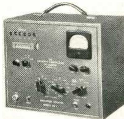
binates the functions of a scaling unit, a radiation survey meter, a count-rate meter and a contamination detector. Some of its features are: continuous 24 hour per day stable operation without overheating; bi-
