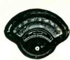
Another of the famous Weston fan shaped line. Very large scale 5.3" long. These meters were made by Weston to General Radio specifications, with special mirrored scale and knife edge pointer. Accuracy 1%.
