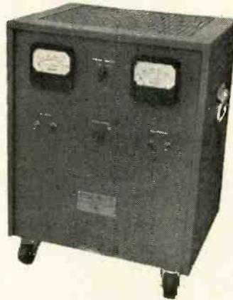
**Right: MODEL PSR-102**... 200 to 1000 volts D.C. at 0 to 500 ma. 6.3 volts A.C. center-tapped at 10 amp; 1/2% or better regulation under any conditions of operation within ratings. 20 MV. or less peak-to-peak ripple voltage. Output impedance effectively zero. High voltage continuously variable from 0 to 1000 volts.
