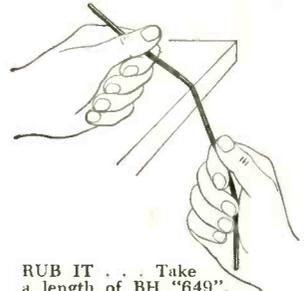
**RUB IT . . .** Take a length of BH "649". Hold the ends firmly. Then rub the sample up and down briskly in a sawing motion against the edge of a desk or chair. See how difficult it is to damage the coating.
