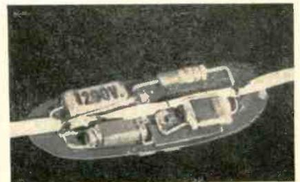
Actual-size view of receiver with protective cover removed
