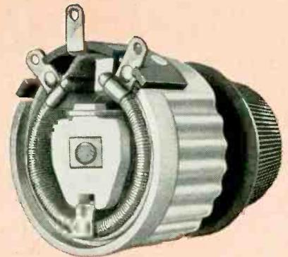
**VARIABLE POWER** requirements within 25 and 50 watt ratings are well handled by IRC Type PR Power Rheostats. All-metal corrugated construction gives maximum heat dissipation. PR Rheostats can be operated at full power in as little as 25% of rotation without appreciable temperature rise. Direct contact between housing and mounting panel increases ability to disperse heat. Bulletin E-2 details specifications; send for your copy.
