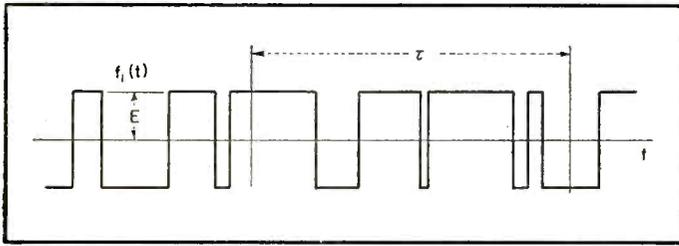
FIG. 3—Time function having random zero crossings following the Poisson distribution law
