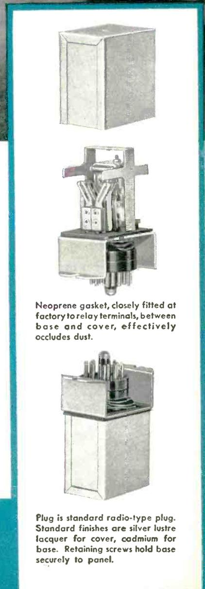
Neoprene gasket, closely fitted at factory to relay terminals, between base and cover, effectively occludes dust.
