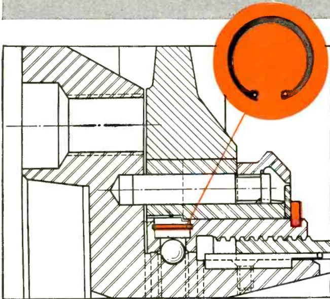
**INTERNAL RING:** Used instead of a shoulder screw, Truarc internal ring #5000-37 locks disc over ball loading hole. Saves 1/8 inch in overall diameter. Eliminates tapping. Withstands machine vibration and vibration from impact device within chuck. Used with Truarc pliers, it facilitates assembly and disassembly.
