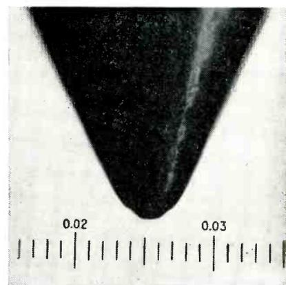
FIG. 7—Photograph of a 2-mil osmium all-purpose needle after 21 hours of wear on fine-groove records
