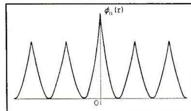
FIG. 7—Autocorrelation function for duration-modulated pulses
