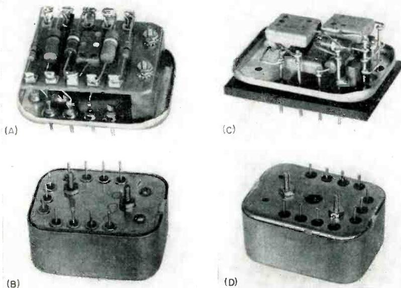
FIG. 3—Old and new techniques employed in assembling an industrial instrument subassembly, the former shown at (A) and (B) and the latter at (C) and (D)
