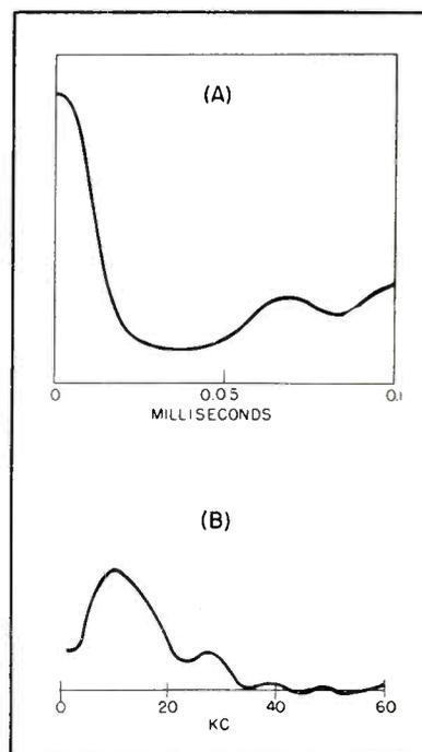
FIG. 12—Correlation function (A) for noise from a type 884 gas tube, as obtained with electronic correlator, and corresponding power spectrum obtained by making cosine transformation of function with an electronic differential analyzer
