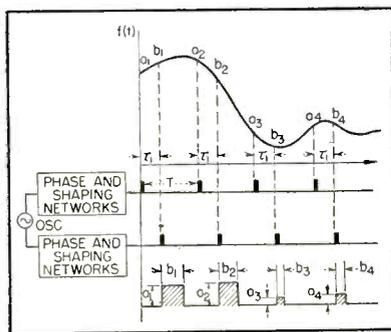
FIG. 9—Method of sampling a random function at regular intervals with an electronic correlator
