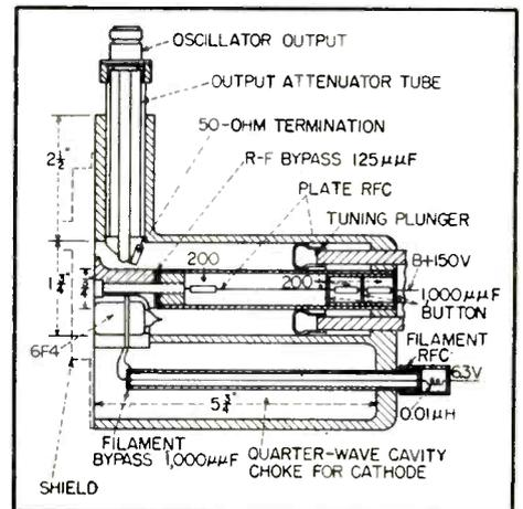
Fig. 2—Physical construction of coaxial-line oscillator
