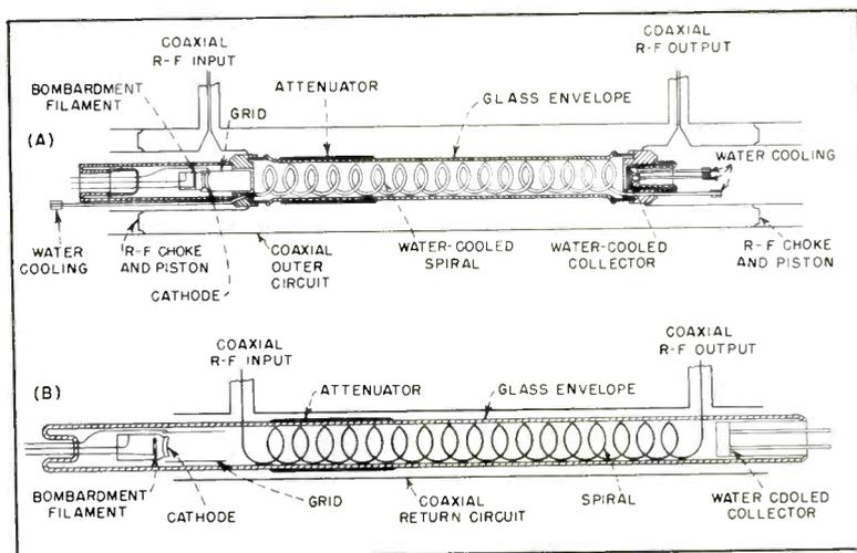
FIG. 1—Construction details of both types of traveling-wave tubes
