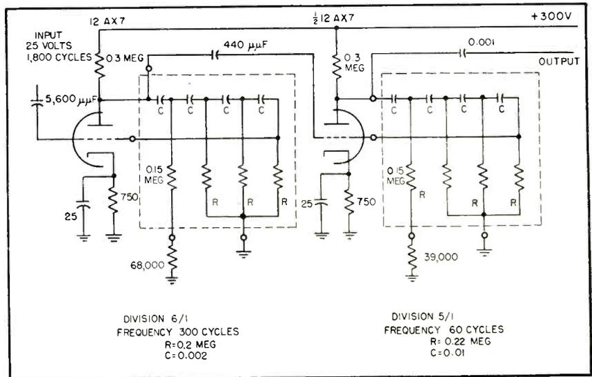
FIG. 4—Synchronous motor-control giving frequency division of 30
