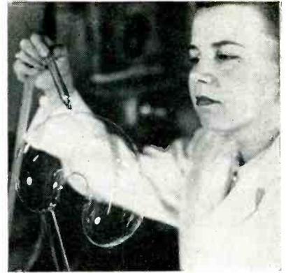
FIG. 5—The glass target section is cut from a carefully-blown glass bubble
