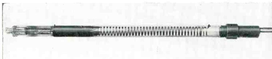
Radiation-cooled-spiral tube, capable of 500 watts output at 450 mc
