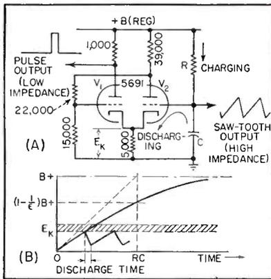
FIG. 5—Basic oscillator-counter operates at twice horizontal scanning frequency
