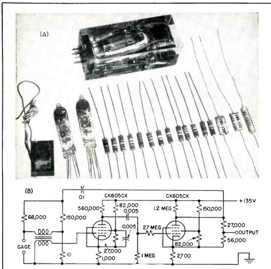
FIG. 1—(A) Plug-in oscillator for vibrating-wire-type pressure gage used for guided-missile telemetering application and, in foreground, the component parts embedded therein. (B) Circuit of the oscillator
