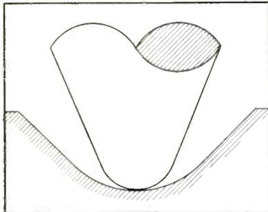
FIG. 5—Profile of 1-mil needle placed in a 78-rpm groove
