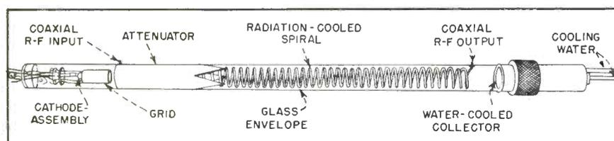
Input and output connections are brought out radially from the spiral
