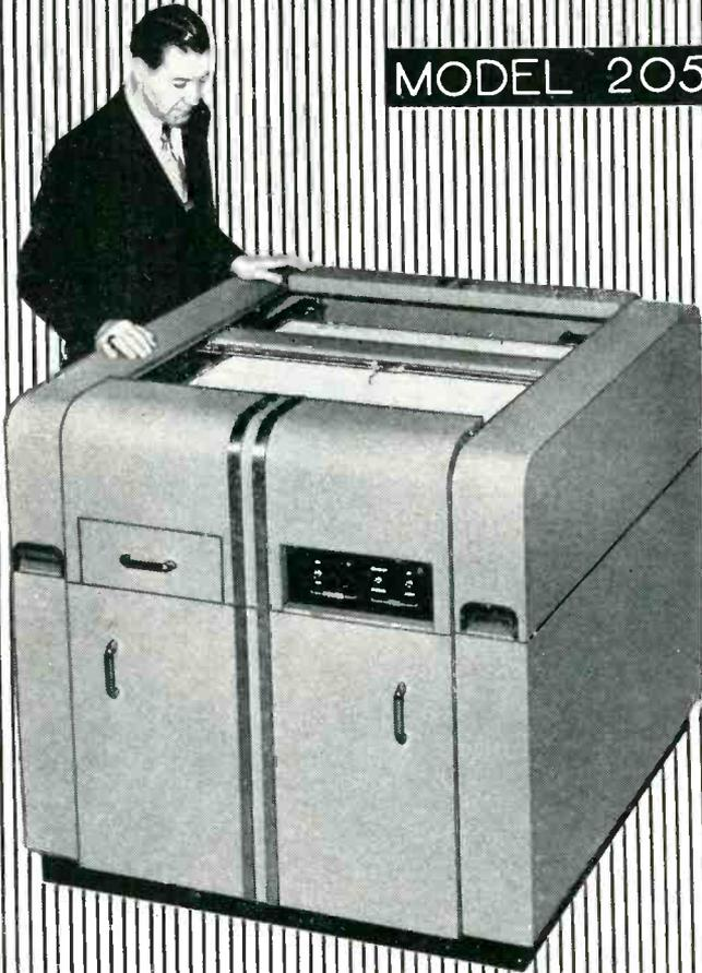
The Model 205 Variplotter, highlighting accuracy, speed, and versatility, brings to industry and laboratory a new tool with a wide field of application. This instrument will present on a 30-inch square plotting surface a precise graphic representation of one variable as a function of another variable, requiring only that the variables be expressed by d-c voltages.
