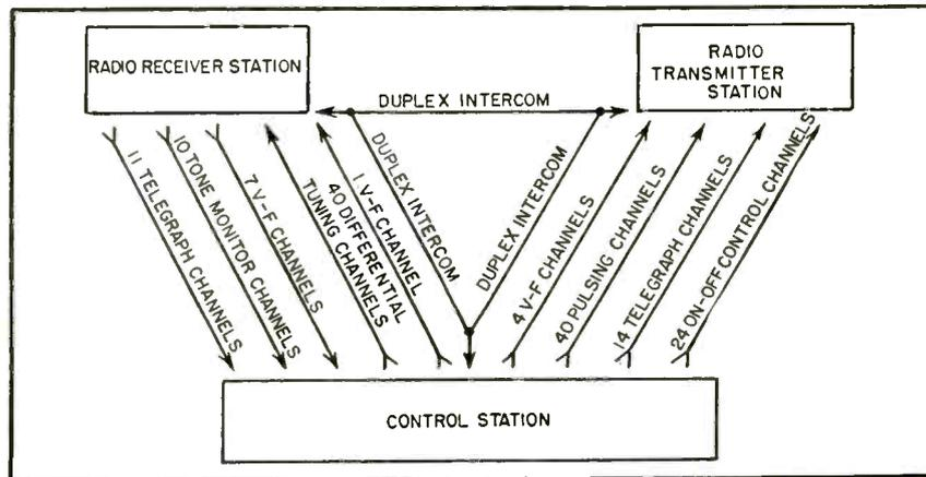
FIG. 1—Each arrow represents one of the vhf links used in lieu of wire lines between control station at airport and the two remotely located antenna sites. Numbers and types of carrier-derived channels provided by each link are indicated
