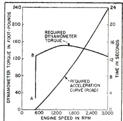
FIG. 1—Acceleration curve of 1941 Chevrolet going from 10 mph to 70 mph in high gear at full throttle on a level highway, and torque curve that electronic control system must produce to simulate this acceleration in laboratory
