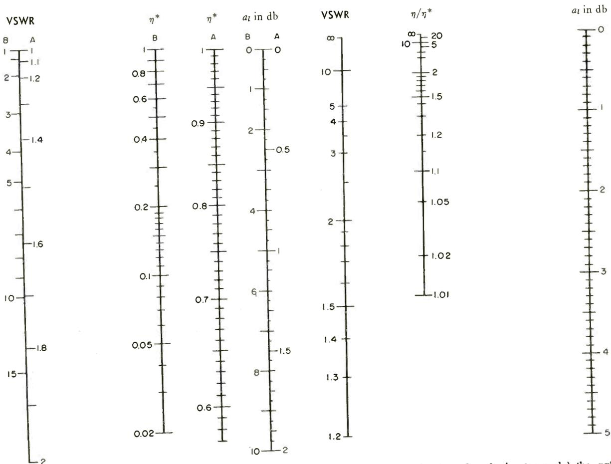
FIG. 1—Combination two-range nomograph for finding third value when any two are known. Use all three scales marked A together for lower ranges of attenuation  $a$  and vswr; use scales marked B together similarly for higher ranges
