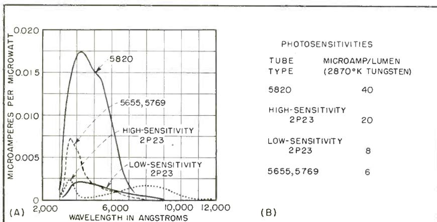
FIG. 1—Comparative spectral responses and overall sensitivities of the four types of image orthicons
