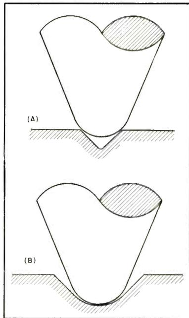
FIG. 6—(A) Profile of 2-mil radius needle in a fine groove. (B) Profile of needle in 78-rpm groove
