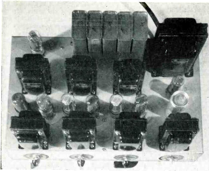
Electronic control unit used between tachometer generator and dynamometer amplifier
