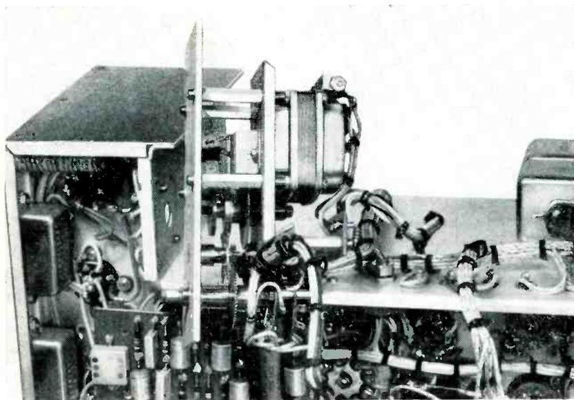
Motor, gear train and Geneva gear used in the scale-changer, showing interconnection with electronic equipment
