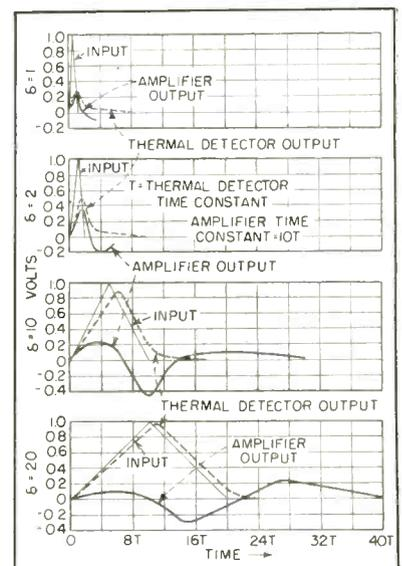
FIG. 3—Curves of pulses in relative time domain for detector and amplifier
