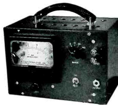
THIS instrument is designed to replace high-sensitivity galvanometers in many applications. Due to its ruggedness, freedom from burnout, and relative insensitivity to shock, it is an ideal instrument for use in balancing resistance bridges, measuring crystal rectifier output, photo-cell, strain-gage, thermocouple, and lead-sulphide cell currents, etc. The instrument may also be used as a DC pre-amplifier for recorders. When used in this manner, current amplification of 1,000 is available.
