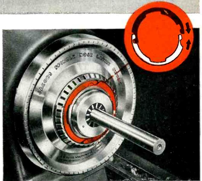
**INTERLOCKING RING:** Used instead of a locknut, Truarc interlocking ring #5107-343 locks handwheel assembly securely on impact sleeve of Jacobs chuck. Saves 7/32 inch in overall length. Eliminates tapping. Chuck's top speed: 5000 RPM; Truarc ring is dynamically balanced to withstand 50,000 RPM's. Services easily with a screwdriver.
