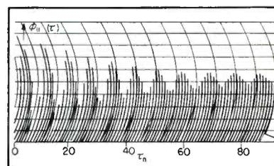
FIG. 11—Example of autocorrelation function for filtered noise, as recorded by correlator
