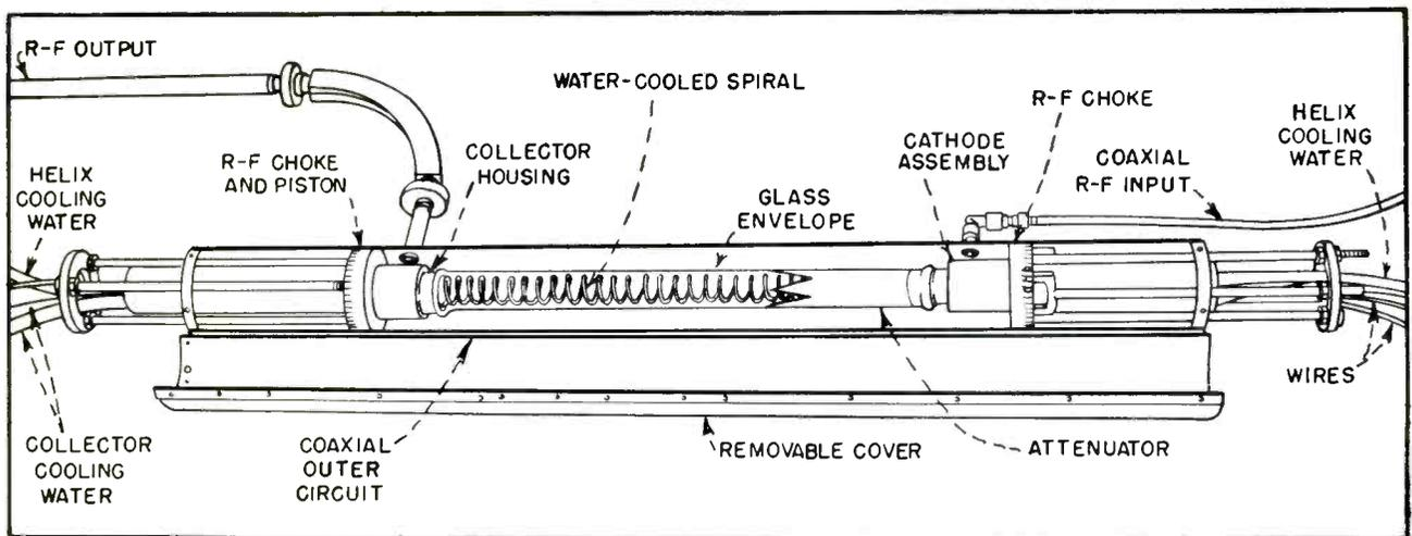
In the 1,000-watt tube, both the spiral and collector are cooled by a continuous flow of water
