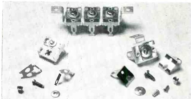
Padder condenser is shown on left and trimmer condenser and parts on right. Ganging, as shown at top right, may include any number of individual condensers. Courtesy Electro Motive Manufacturing Co., Willimantic, Conn.
