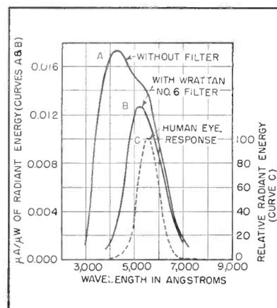
FIG. 2—Comparison of 5820 spectral response with that of human eye
