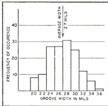
FIG. 3—Distribution of groove widths of 147 fine-groove records
