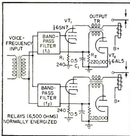
FIG. 4—Double receiver used for on-off control over a radio link
