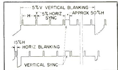
FIG. 7—Composite waveform for the industrial television system
