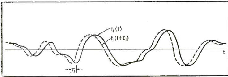
FIG. 1—Time functions used for determining the autocorrelation function of a stationary random process
