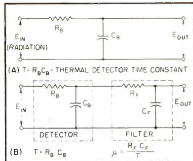
FIG. 1—Equivalent circuits for thermal detector A and for detector with low-pass filter B
