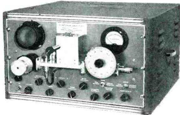
**X BAND SPECTRUM ANALYZER 8500-9600 Mc.**, calibrated linear below cut-off attenuator, calibrated frequency meter, tuned mixer, 4 i.f. stages, 3 video stages overall gain 125 db., regulated power supply.
