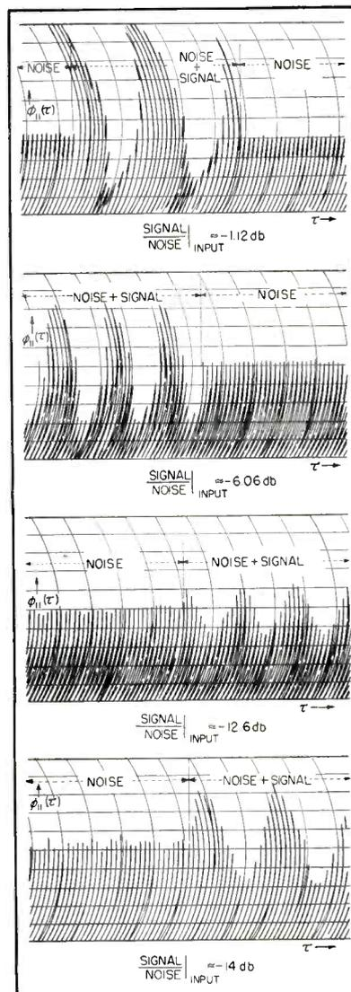
FIG. 14—Experimental results obtained by using electronic correlator to detect pure 8-kc sine-wave signal at four different levels below that of random noise. Sinusoidal output is clearly evident in each case
