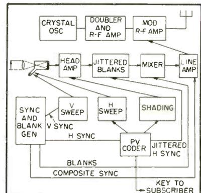
FIG. 1—Block diagram of typical Phonevision transmitter
