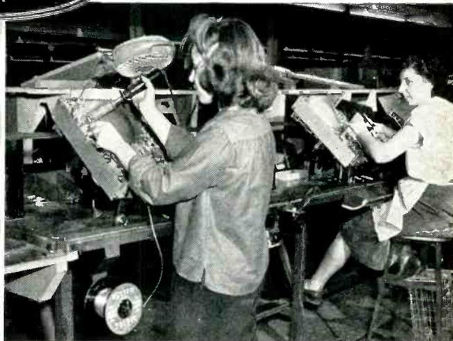
Using Kester Flux-Core Solders, Plastic-Rosin and "Resin-Five" Core Solders, will keep your solderers satisfied. Kester flows better—handles easier—faster to use. Kester Solders are made only from newly mined grade A tin and virgin lead.
