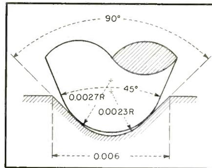
FIG. 1—Profile of typical 78-rpm groove and standard 2.7-mil radius needle
