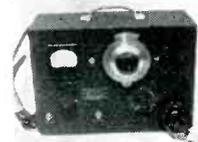
**FERRIS TEST EQUIP. 18B (I-136):** VHF Signal generator, 20-150 MC, mod 400 cps. 115V, 60 cy input. \$80.00
