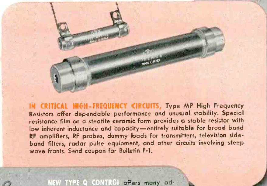
**IN CRITICAL HIGH-FREQUENCY CIRCUITS**, Type MP High Frequency Resistors offer dependable performance and unusual stability. Special resistance film on a steatite ceramic form provides a stable resistor with low inherent inductance and capacity—entirely suitable for broad band RF amplifiers, RF probes, dummy loads for transmitters, television side-band filters, radar pulse equipment, and other circuits involving steep wave fronts. Send coupon for Bulletin F-1.
