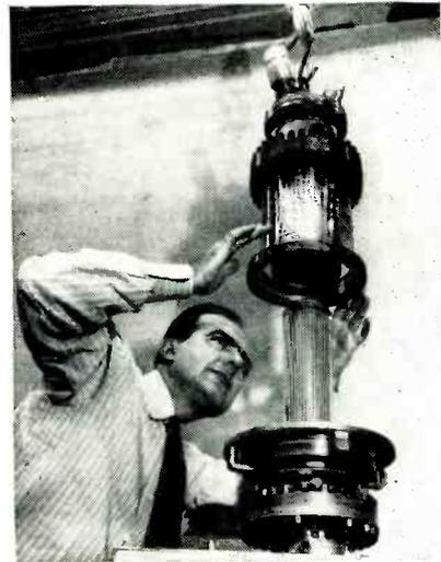
Individual filament and grid elements of the unit triodes in the array are tungsten rods 8 inches long, supported at both ends by means of knife-edge V-notch arrangements. A pantographic mounting device has flexible spring-loaded fingers to which the filament rods are hooked. This makes each filament strand and grid rod mechanically independent, and allows vertical movement without disturbing the precise alignments and spacings essential to effective electron optics.
