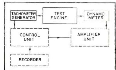
FIG. 2—Closed-servo electronic control system used with laboratory dynamometer to place controlled loads on auto engine
