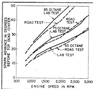
FIG. 6—Correlation of knock-rating curves obtained on road and with electronic control system in laboratory
