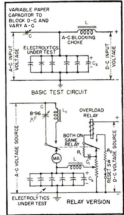
FIG. 2—Basic circuit used for life-testing electrolytics
