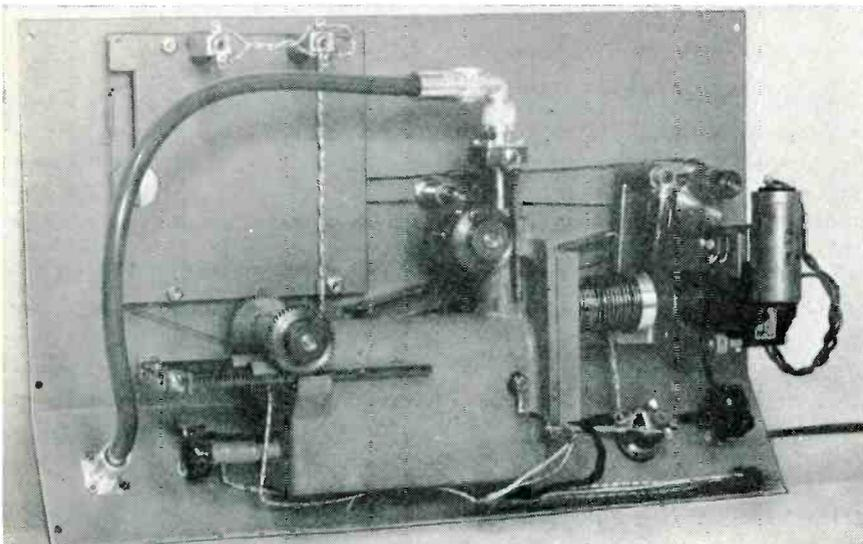
A standard rack-and-pinion drive is used on both tuning plunger and attenuator
