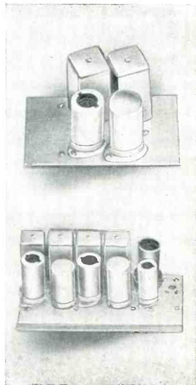
Two of the frequency dividers described. The upper one is based on 1,800 cycles and the lower upon 90.72 kc
