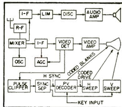
FIG. 3—A decoder is added to a normal receiver
