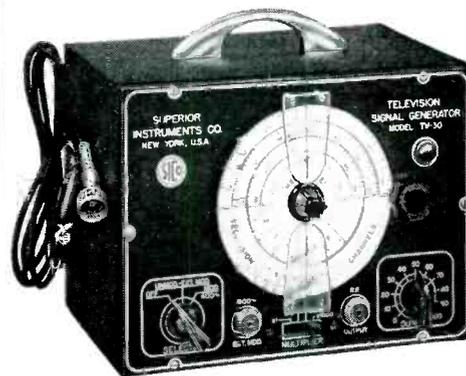
Enables alignment of television I. F. and FRONT ENDS without the use of an oscilloscope.
