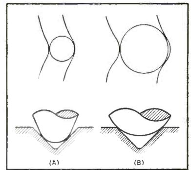
FIG. 4—(A) 1-mil radius needle in a modulated fine-groove. (B) 2-mil needle
