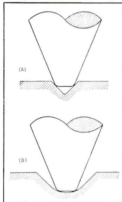
FIG. 9—(A) Profile of Unipoint needle in a fine groove. (B) Profile of needle in a 78-rpm groove.
