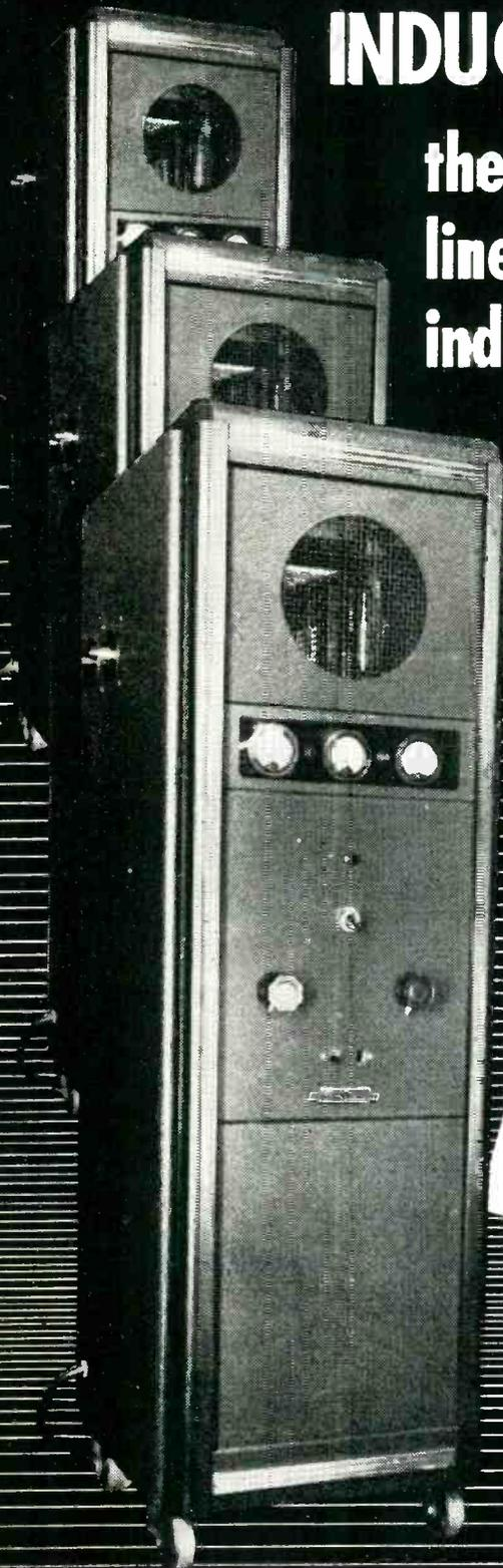
HAYDU BROTHERS' answer to your problem in brazing, annealing and hardening — where localized heating is important — can be solved with these machines of infinite uses. One of its important functions is the heat treatment of internal metal parts of electron tubes.
