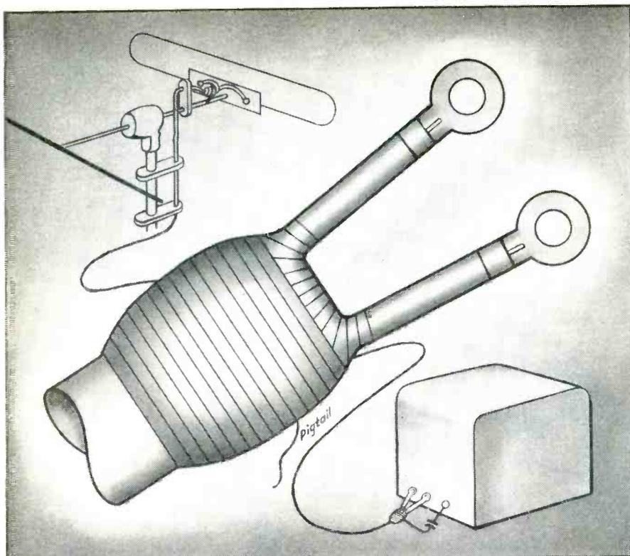
FEDERAL TELEPHONE AND RADIO CORPORATION'S shielded balanced 300-OHM Lead-in, lap-wrapped with "SCOTCH"
