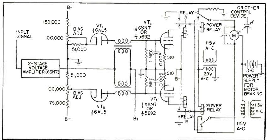
FIG. 5—Differential signal receiver circuit used to control reversible motor over radio link between airport station and remote station
