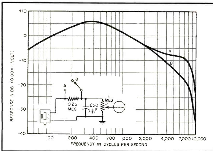
FIG. 11—Switching circuit for selecting (A) extended frequency range, or (B) early cutoff when using a pickup with a Unipoint needle on fine-groove records and 78-rpm records respectively. Response-frequency characteristic measured on RCA 12-5-31-record
