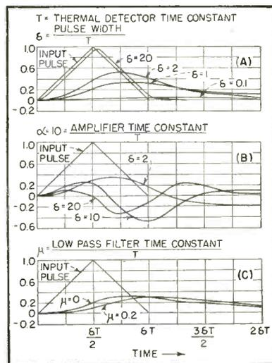
FIG. 2—Curves show response of thermal detector and five-stage amplifier to symmetrical triangular input pulses
