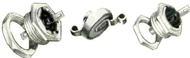
Sangamo Silvered Mica Button Capacitors are available in a wide variety of sizes and styles in capacitance ranges from 10 mmfd. to 7000 mmfd. and meet all requirements of component capacitors for V. H. F. and U. H. F. applications. Sangamo Button Capacitors are fabricated with silvered mica to provide high conductivity. They are completely sealed against humidity, and have a very low temperature coefficient.
