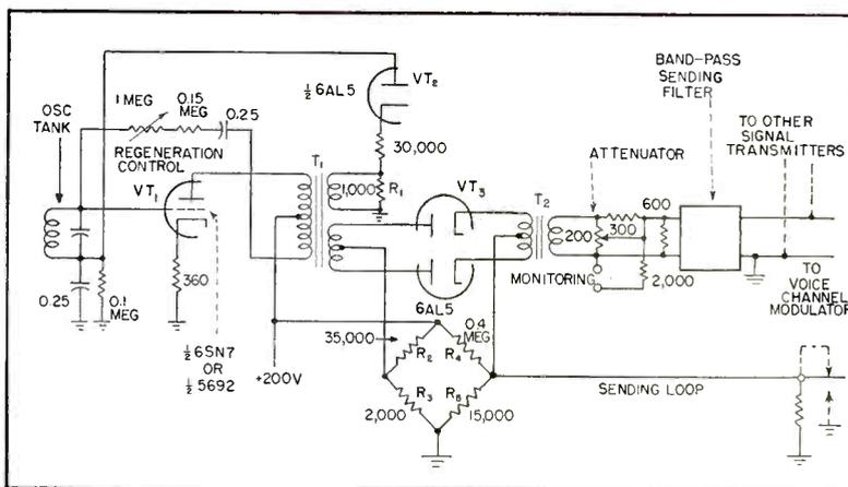
FIG. 3—Typical universal signal transmitter circuit. In use these are paired to utilize the other sections of the first two tubes
