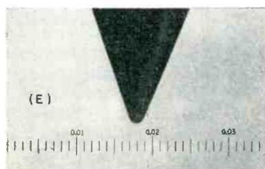
Contours of five types of needles in use today. (A) Standard 2.7-mil radius needle for 78-rpm discs. (B) All-purpose needle with 2-mil tip radius. (C) All-purpose Unipoint. (D) All-purpose wide-angle needle. (E) Standard 1-mil radius needle for fine-groove records
