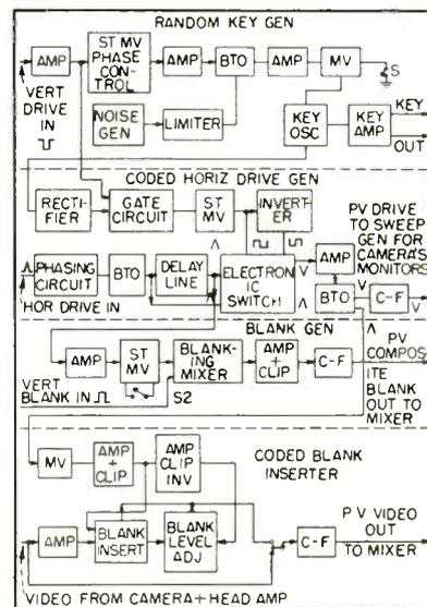
FIG. 2—Setup of stages in the four main sections of the coder unit for the transmitter
