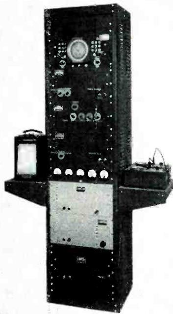
FIG. 10—Electronic correlator built at MIT for obtaining complete autocorrelation curve of a random function automatically on recorder at left
