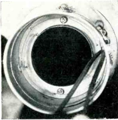
FIG. 3—Image section of the 5820. Evaporators are being welded in place
