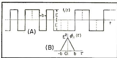
FIG. 5—Random distribution of equal-length positive and negative pulses, corresponding to tossing a coin heads or tails, and triangular autocorrelation function obtained
