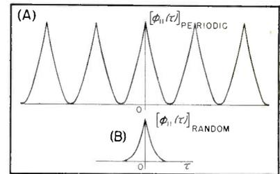
FIG. 8—Periodic and random components of autocorrelation function for duration-modulated pulses
