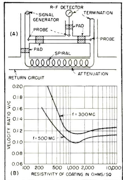
FIG. 3—Setup for determining velocity of waves on spiral is shown in (A). Curves in (B) show results obtained
