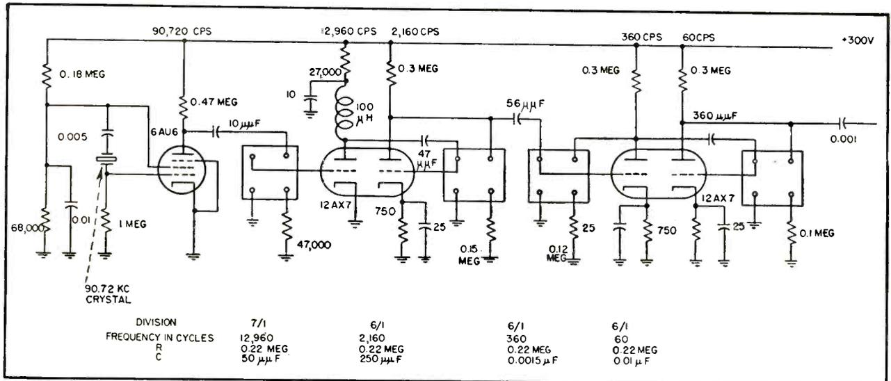
FIG. 5—Divider system using a 90.72-kc crystal gives highly accurate 60-cycle output
