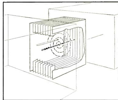
Cutaway drawing of the heart of the omegatron. Difference between applied r-f field and particle cyclotron frequency is inversely proportional to particle rotations before collision with central collector
