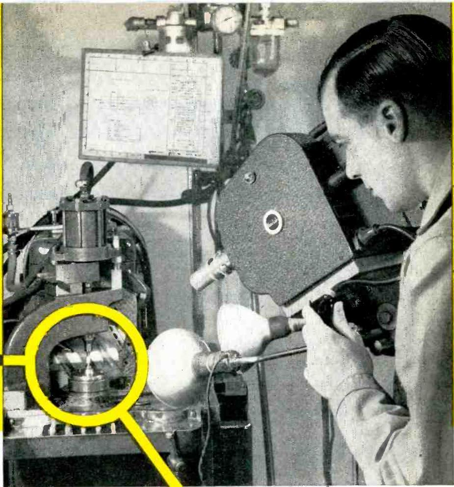
Fast-moving machines are hard to study under actual working conditions. But with high speed movies you can slow down fast action to a pace the eye can follow.
