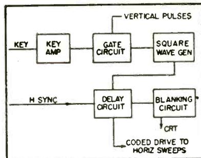
FIG. 4—Stages of the decoder unit at the receiver.
