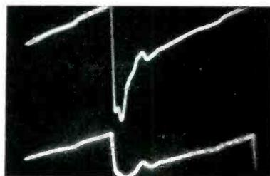
TV horizontal output tube waveform
