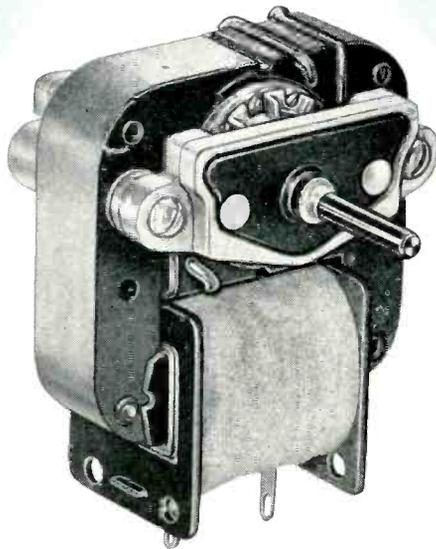
Type 230 Shaded 2-Pole Motor. For continuous duty without fan cooling. 1/200 to 1/50 hp at 3200 rpm. Flat Speed Torque Curve and High Starting and Pull Up Torque are characteristic of all Type 230 Raytheon motors. Efficiency is almost double the value ordinarily obtained in shaded two-pole motors of this type. Write for Data Bulletin 1000.
