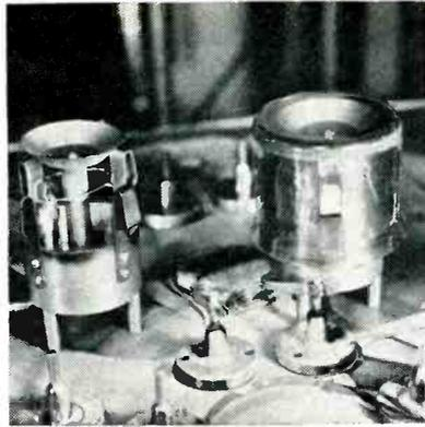
FIG. 4—Image-section glass caps are aluminized in an evaporating system
