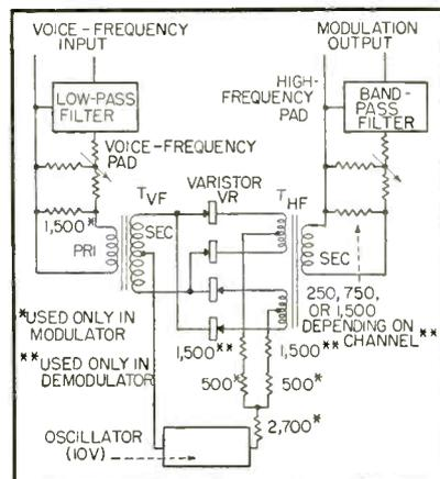
FIG. 2—Basic modem circuit that can be used either as a modulator for producing sidebands or as a demodulator
