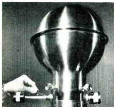
Specimens can be placed in the permanent-magnet electron microscope without disturbing the vacuum
