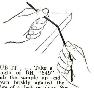
**RUB IT . . .** Take a length of BH "649". Rub the sample up and down briskly against the edge of a desk or chair. See how difficult it is to damage the coating.
