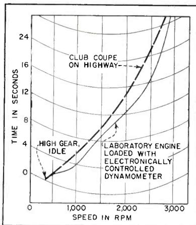
FIG. 7—Correlation of acceleration curves obtained for 1941 Chevrolet club coupe on road and with engine alone in laboratory
