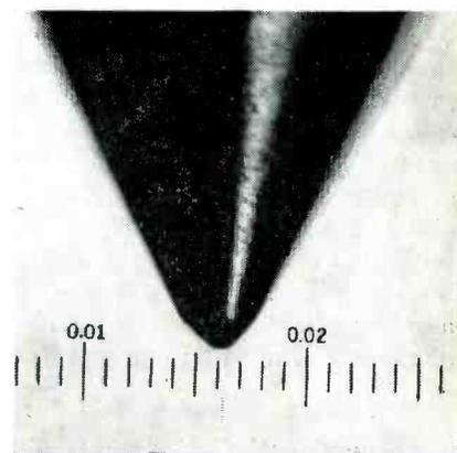
FIG. 10—Photograph of osmium Unipoint needle after 43 hours of wear on fine-groove records
