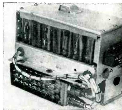
FIG. 2—Missile-borne telemetering system employing the technique
