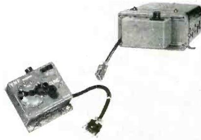
**Remotely Controlled VHF Receiver**
