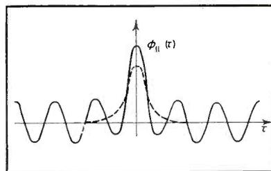
FIG. 13—Autocorrelation function of additive mixture of random noise and sine wave
