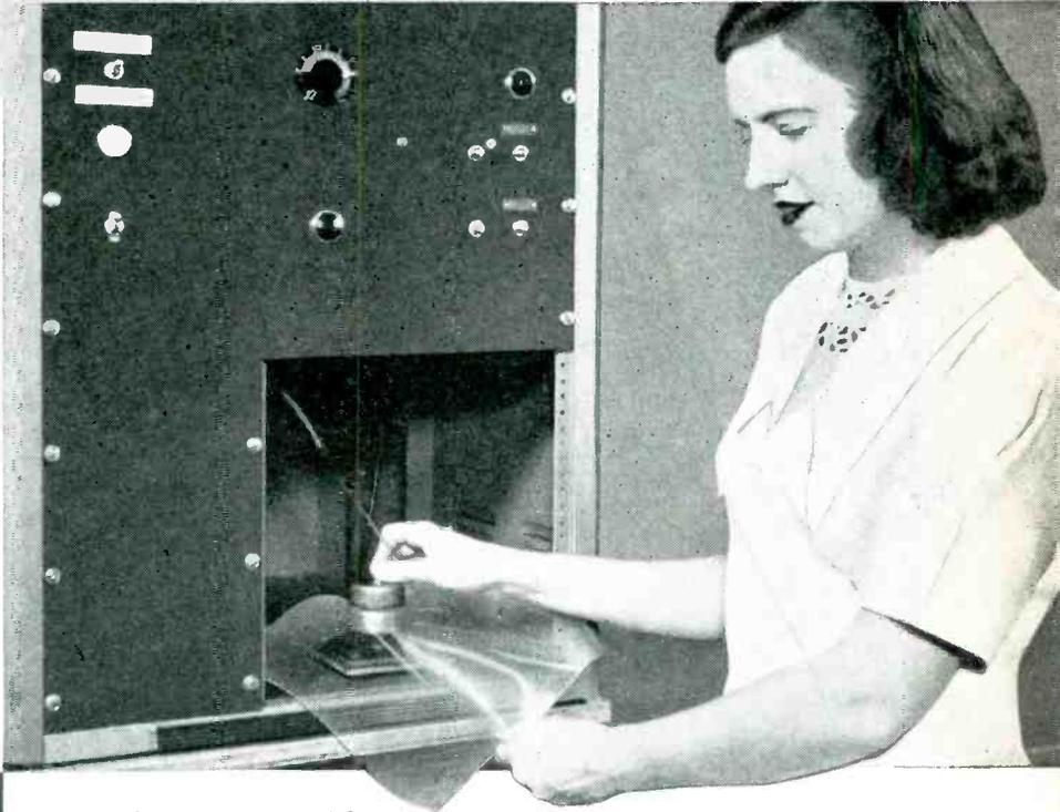
Inserting a sample preparatory to a voltage breakdown test on Kodapak Sheet.
