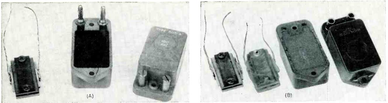
FIG. 4—Precision capacitor made by two methods, the case filled with silica gel, ground cork, paper and wax at (A), and dipped in wax and embedded in plastic within the case at (B)
