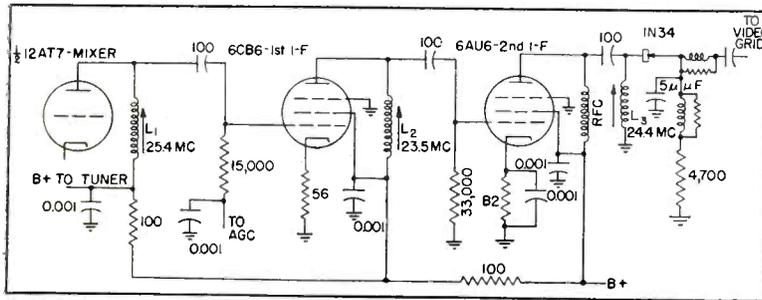
FIG. 3—Circuit of conventional single-tuned staggered stages
