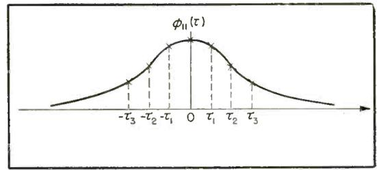
FIG. 2—Autocorrelation function of random time function that can represent a voltage or current
