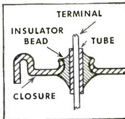
thermostats have a tight, permanent seal that prevents deterioration or sulphiding of contacts. They can also be sealed in helium or other inert gas atmosphere. Terminals are sweat-soldered into inert alloy tubes interfused with inorganic glass insulator bead.
