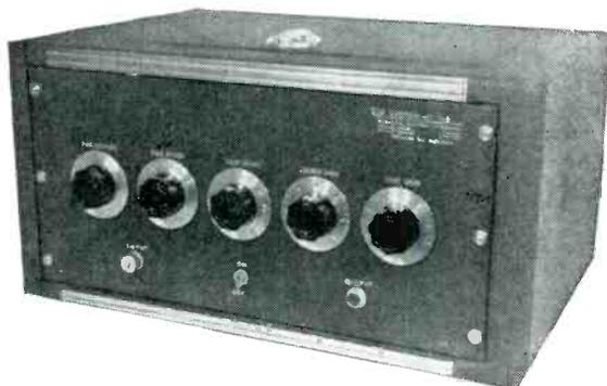
1. This new and improved DC amplifier of the General Motors breaker type offers many advantages in the measurement of DC and low frequency AC voltages in the micro-volt and fractional microvolt regions. It is useful for the amplification of low level thermocouple voltages, infra red detectors, photovoltaic cells and the like. It can be used to replace suspension galvanometer systems.
