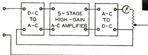
Voltage-balance feedback (above) and current-balance feedback stabilize gain . . . provide virtual null balance.
