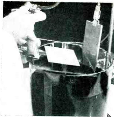
FIG. 7—Completed 500-mesh screen and master being removed from bath
