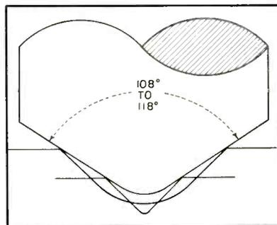
FIG. 12—Wide-angle needle shown with the outlines of a 78-rpm groove and a fine groove
