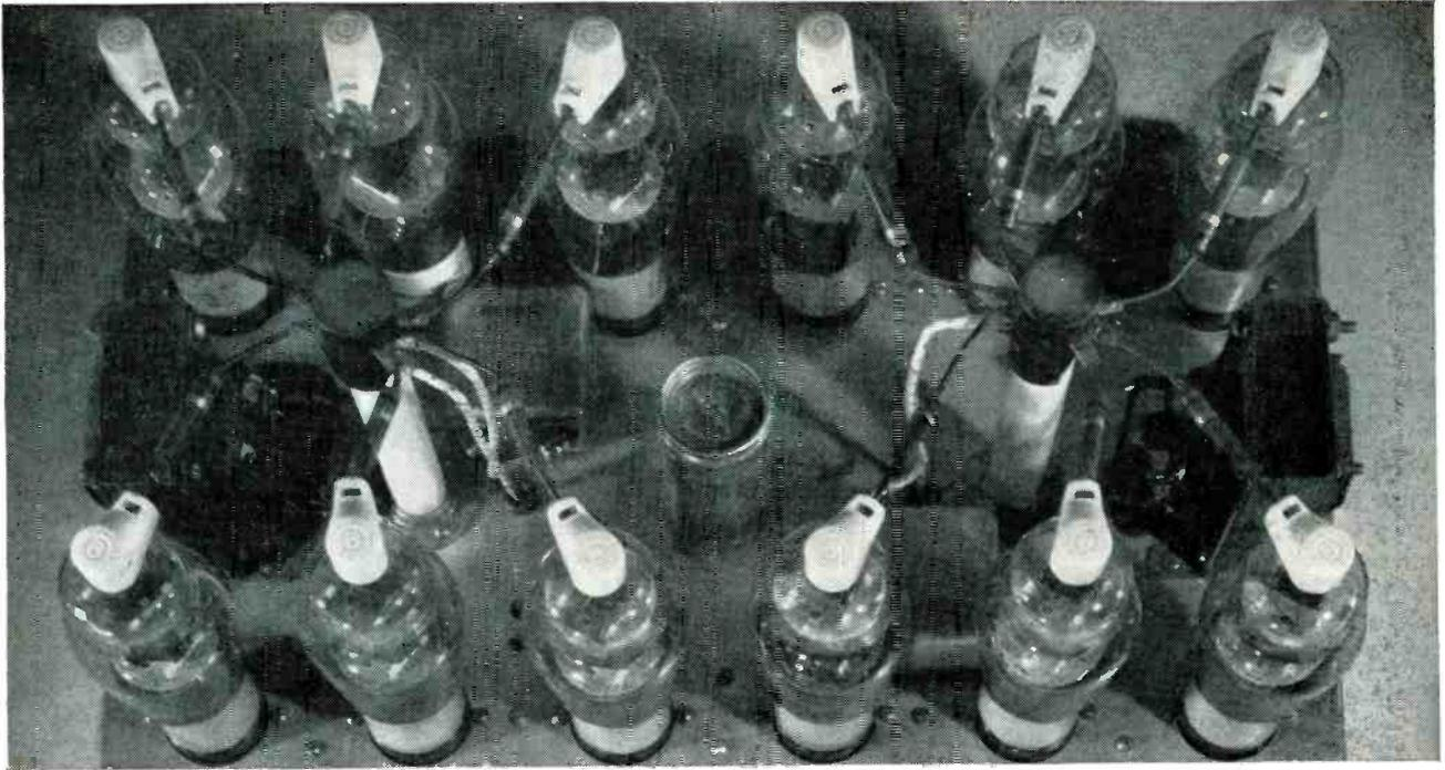
Amplifier used to provide controlled field current for dynamometer, employing twelve 807's in parallel
