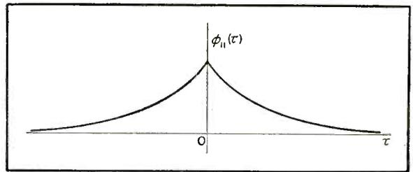
FIG. 4—Autocorrelation graph for random-width pulses of Fig. 3
