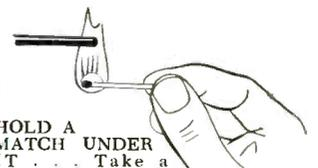
**HOLD A MATCH UNDER IT . . .** Take a length of BH "649". Hold a lighted match under it. BH "649" will not support combustion.
