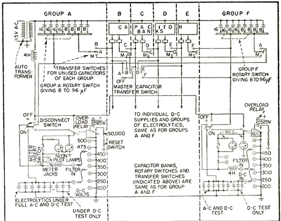
FIG. 1—Test set for making life test runs of up to six groups of electrolytic capacitors, each at different values of a-c ripple current and d-c polarizing voltage that are set up on a jack panel. Temperature oven is used for electrolytic capacitors under test. Paper capacitor banks at top provide various ripple currents needed
