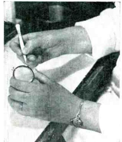
FIG. 9—Complete mesh-target system ready for insertion in the tube structure
