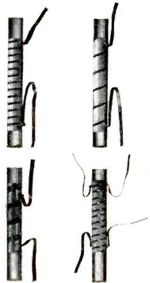
Corning Metallized Inductances are superior in every way for high frequency applications. Their electrical characteristics include low temperature coefficients, high Q and high stability. The smooth glass wall insures noiseless tuning and fine adjusting screws permit rapid and accurate alignment.
