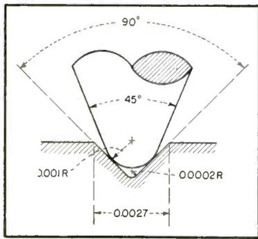
FIG. 2—Profile of typical fine-groove and standard 1-mil radius needle
