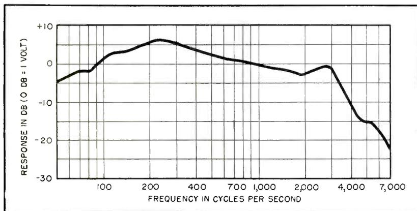
FIG. 8—Response-frequency characteristic of Shure P81 pickup cartridge terminated with 1 megohm, with all-purpose 2-mil radius needle on Audiotone record. High-frequency response is attenuated by means of an internal mechanical filter
