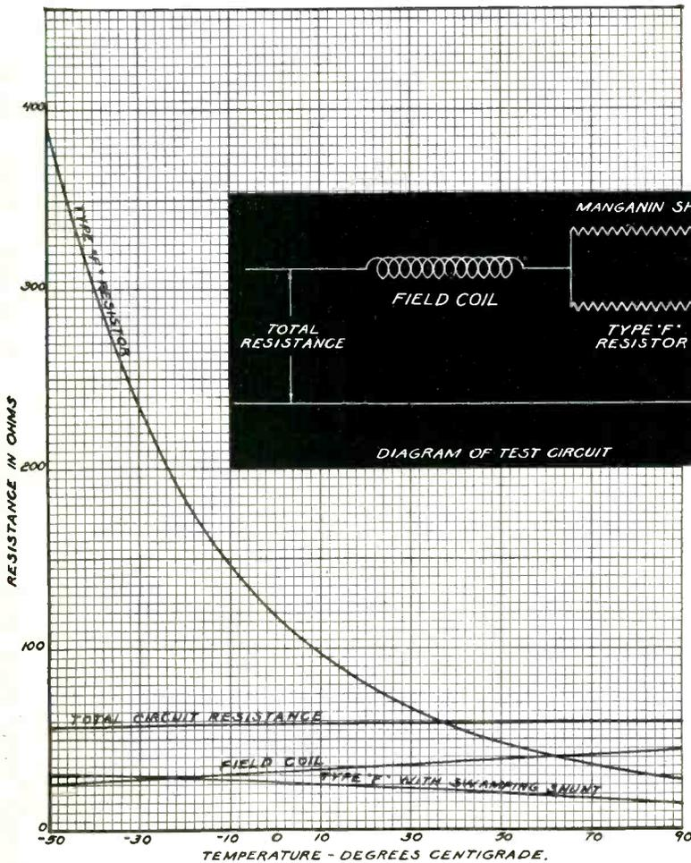
GLOBAR brand type F resistors can often provide the answer when extremes of temperature present an engineering problem. A typical example is shown by the curves plotted here. In this important control system, a GLOBAR type F resistor is used to compensate for resistance changes due to temperature variations in coils such as generator and motor fields, measuring and control circuits.
