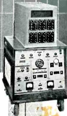
The Hathaway SC-16A Six Element Recording Cathode-Ray Oscillograph, designed for recording fast transients and continuous phenomena, brings you new highs in resolution because of its unusually high frequency response and high chart speed. Note these unusual features:
