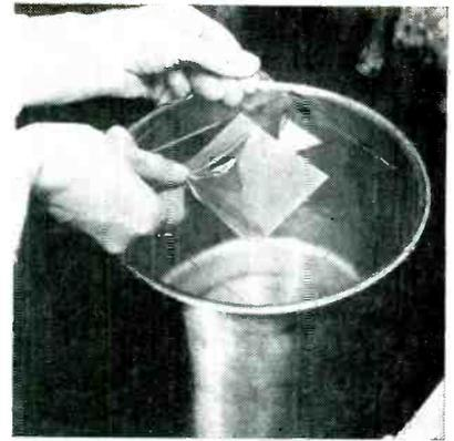
FIG. 8—Copper mesh is carefully removed from master and then inspected
