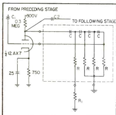
FIG. 1—Basic divider circuit illustrates importance of couplings
