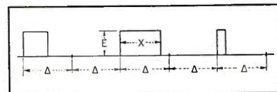
FIG. 6—Duration-modulated pulses, characterized by equally-spaced leading edges
