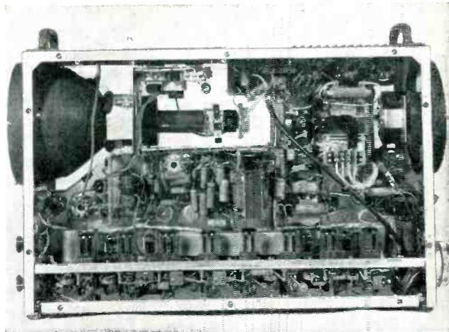
FIG 4—Right-side view shows frequency-division chain and high-voltage circuits
