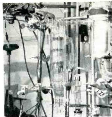
Close-up of a completed three-stage nonmagnetic mass spectrometer tube
