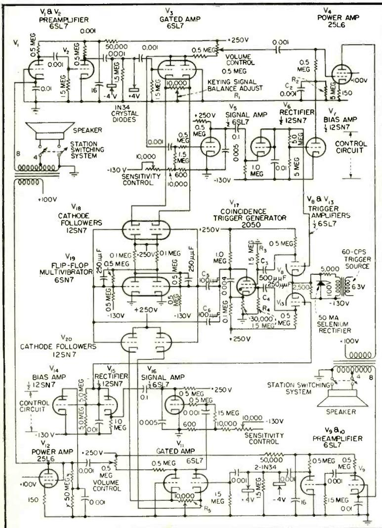
FIG. 2—Amplifiers and control circuits. Power supplies and station-switching arrangements are conventional hence not shown
