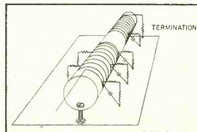
FIG. 2—Distributed-constant resistor approximate a lossy distortionless line
