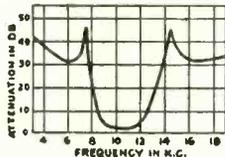
Specialized design and complete production facilities for your filter requirements. Where space is critical, miniature filters with wedding ring toroids and special capacitors. Supplied in standard units, or designed to your specification. A miniature band pass filter and curve are shown.
