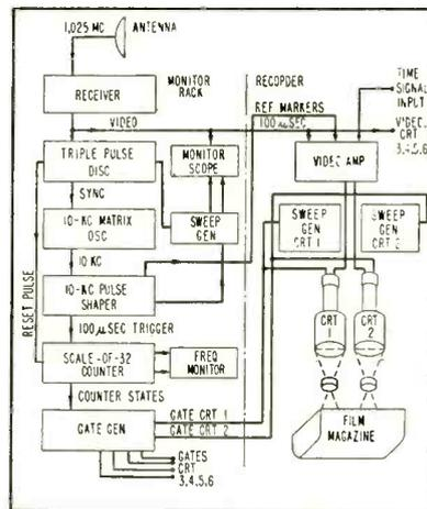
FIG. 5—Matrix receiving equipment must be kept in both frequency and phase synchronism with transmitter timing oscillator
