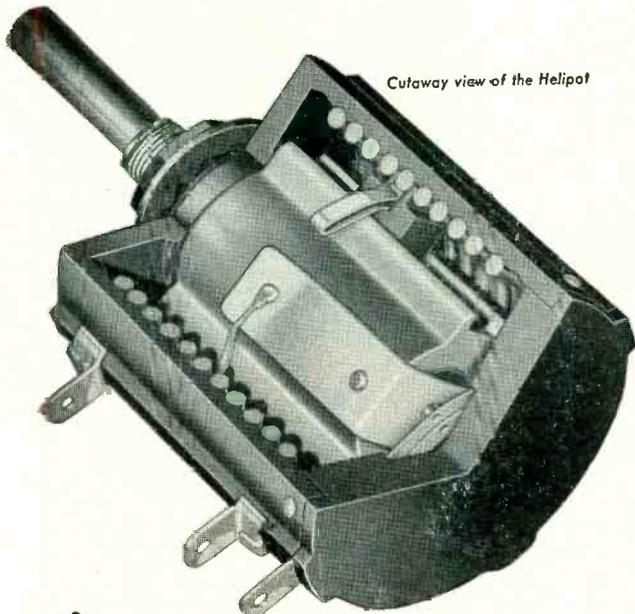
Cutaway view of the Helipot
