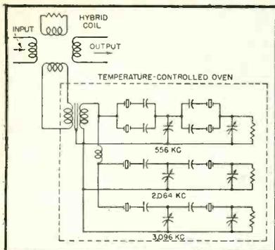
FIG. 3—Filter for elimination of pilot tones at three frequencies
