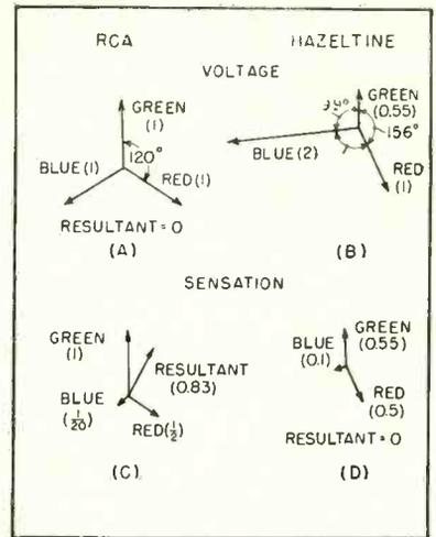
FIG. 1—Vector relations of voltage and visual sensation for the two systems. Angle blue-red is 105 degrees
