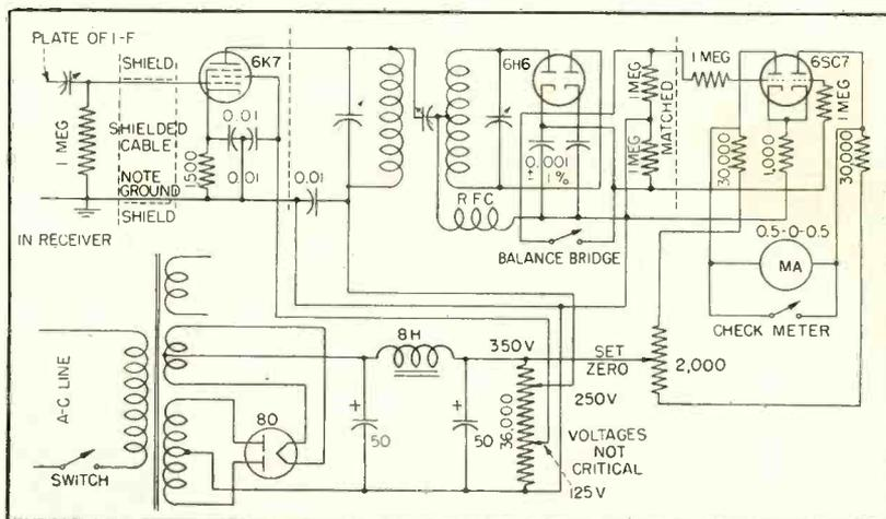
FIG. 1—Circuit of tuning indicator forms a complete unit that can be added to any standard superheterodyne receiver
