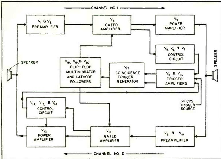
FIG. 1—Twenty stages, some using halves of dual-function tubes, keep either channel open as long as voice signals are present and permit other channel to take over quickly at end of message
