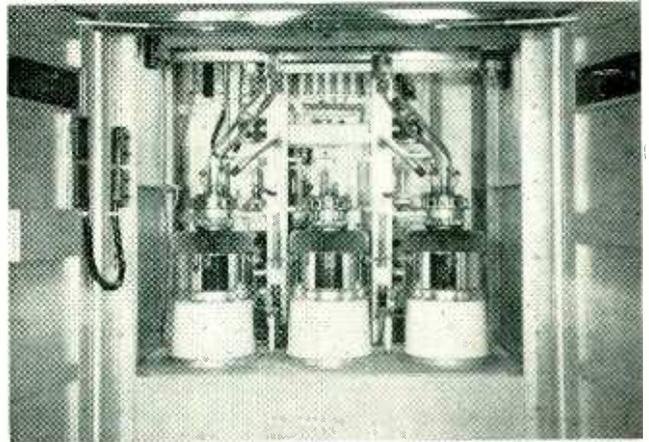
Tube end of system using ducts to radiators and to filament connections
