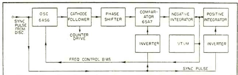
FIG. 6—Block diagram of receiving station matrix oscillator
