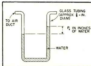
FIG. 6—Simple U-tube manometer, useful for system tests
