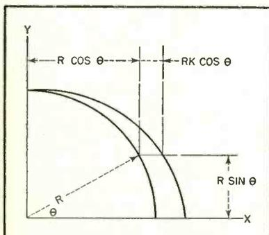
FIG. 1—Geometry of potential theory on which the yoke design is based
