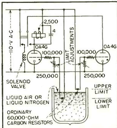
FIG. 1—Circuit diagram of low-temperature liquid level control
