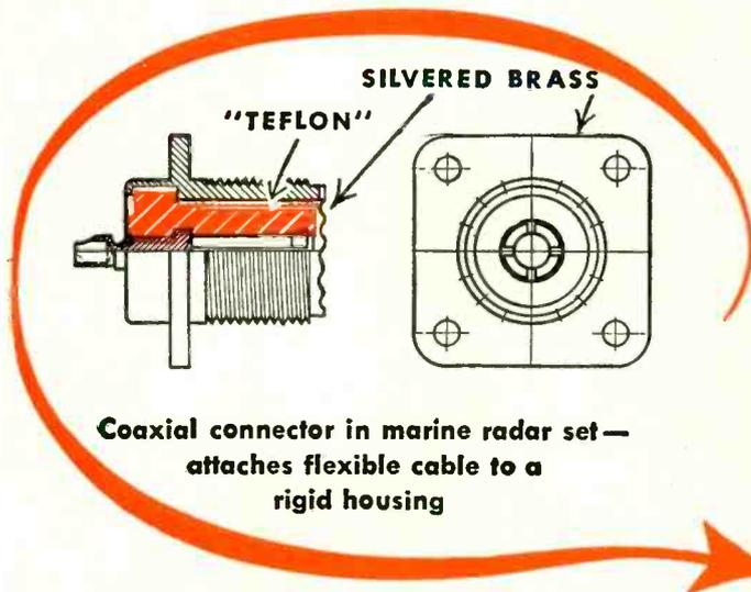
**Coaxial connector in marine radar set—
