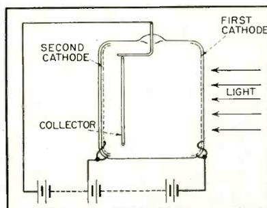
idea. The first cathode is a pervious layer of the Sb-Cs type, which lets pass the red component of the light. The second cathode is a red-sensitive cathode (Ag-Cs<sub>2</sub>O-Cs) at a positive potential with respect to the first cathode. The electrons emitted from the first cathode and the red light strike this second cathode. If the field between the cathodes is sufficiently high, some of the electrons emitted from the first cathode will release secondary electrons.
