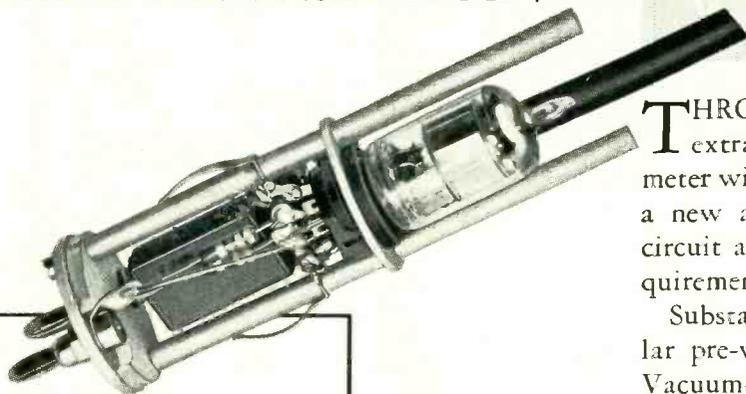
Probe with completely shielded case removed. Twin diode tube in the probe has an inactive section connected to the grid of one triode in the V-2 amplifier while the active section is connected to the grid of the other triode, both sections of the amplifier being used in a balanced circuit. The balanced amplifier insures very little zero shift when the line voltage varies.
