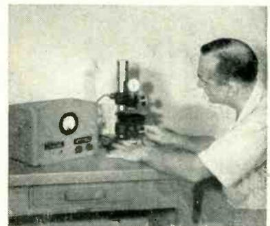
FIG. 1—Ceramic thickness gage gives direct, nondestructive measurements of thickness of nonconducting coatings on nonmagnetic metals
