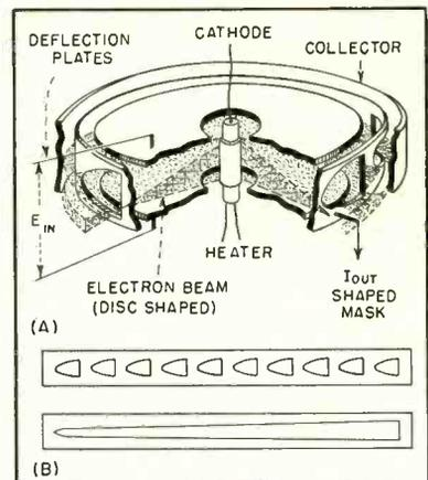
FIG. 3—Cutaway view of beam-deflection tube and equivalent mask shapes
