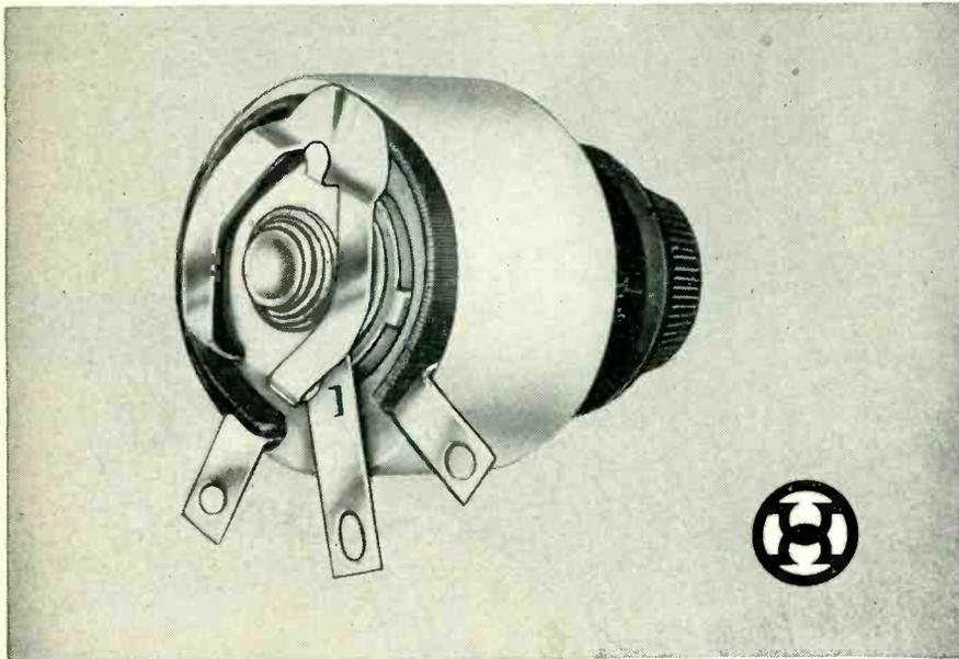
**T**HIS COMPACT, rugged type M 25 watt rheostat offers exceptional heat dissipation. An exclusive Hardwick, Hindle feature is the lock tab which prevents deformation of the contact arm due to rough handling. Its steel stop pin will withstand over 40 inch pounds torque.
