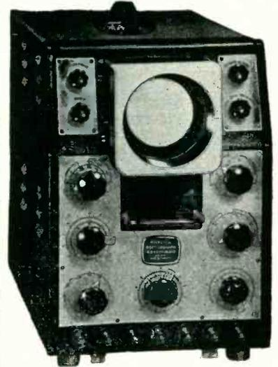
MODEL 1035 Provides FAST SWEEPS, from 150 Millisec. to 5 Microsec., and Video Frequency Amplifiers, Stepped -VE Feedback Type, with Gain of 3 at 7 Mc. Bandwidth to Gain of 3000 at 60 Kc. Bandwidth,  $\pm 1.5$  DB., PLUS Triggered Sweeps, Suppressed Flyback,  $\pm$  VE Sync.
