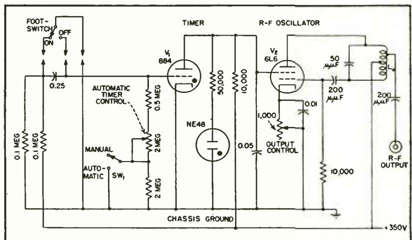
FIG. 3—Schematic of oscillator and automatic pulse timer which resembles those used in electronic exposure controls for photography
