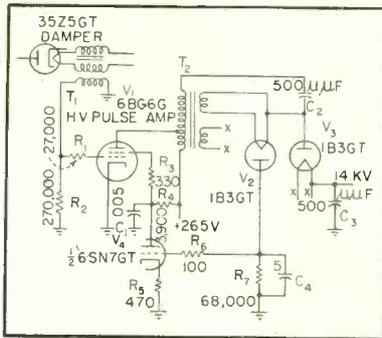
Regulated high-voltage power supply utilizes ringing current in primary of  $T_1$ .
