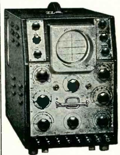
MODEL 1049 Provides SLOW SWEEPS from 1.5 Sec. to 50 Microsec., and D.C. Amplifiers Completely Stabilized Throughout, Response 0-100 Kc.,  $\pm 1.5$  DB., Gain 900, PLUS Beam Blanking Circuits, Triggered Sweeps,  $\pm$  VE Sync.
