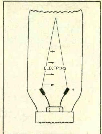
FIG. 1—Edison effect in an incandescent lamp with V-shaped filament
