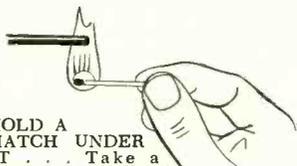
**HOLD A MATCH UNDER IT . . .** Take a length of BH "649". Hold a lighted match under it. BH "649" will not support combustion.
