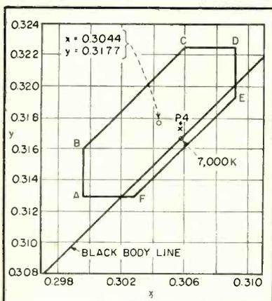
FIG. 4—JETEC specification for neutral filter face-plate glass
