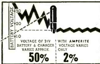
Amperite REGULATORS are the simplest, lightest,
