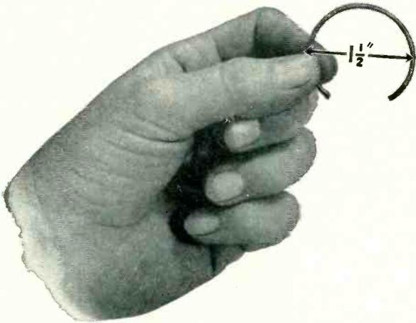
**CONVENTIONAL POTENTIOMETERS** have a coil diameter of approximately 1 1/2" and provide only 4" (about 300°) of potentiometer slide wire control.
