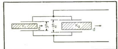
FIG. 1—Basic idea of adjustable temperature coefficient capacitor
