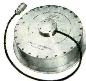
A new series of unbonded strain gage angular accelerometer is available to detect and measure angular acceleration in ranges from  $\pm 3$  to  $\pm 400$  radians/sec/sec. The design of these instruments permits close balance against linear acceleration effects and excellent resolution while providing greatly increased resistance to destruction by linear acceleration. In these instruments, the suspended mass weighs but a few grams.
