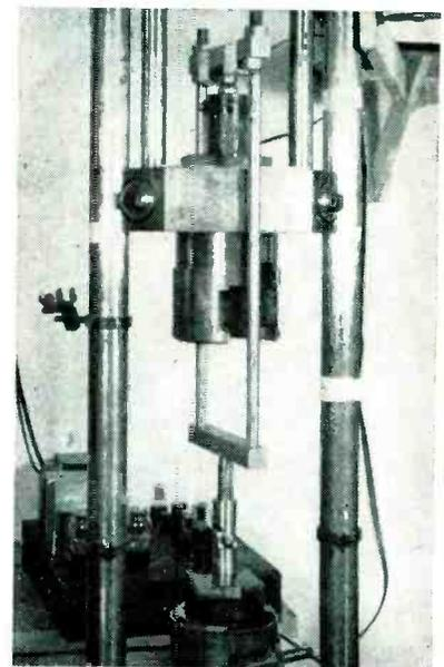
Modified Wagner viscometer with timer chassis in background. Cup and ball are shown at top. Conventional yoke and loading press are at center
