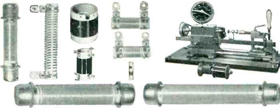
**SPACE WINDING MACHINE, MODEL 30**, winds resistors and space wound coils up to 6" long. Winds wire from No. 40 to 18. For smaller wire sizes, Model 92-6 De-Reeler is recommended instead of the bench type spool holder illustrated.
