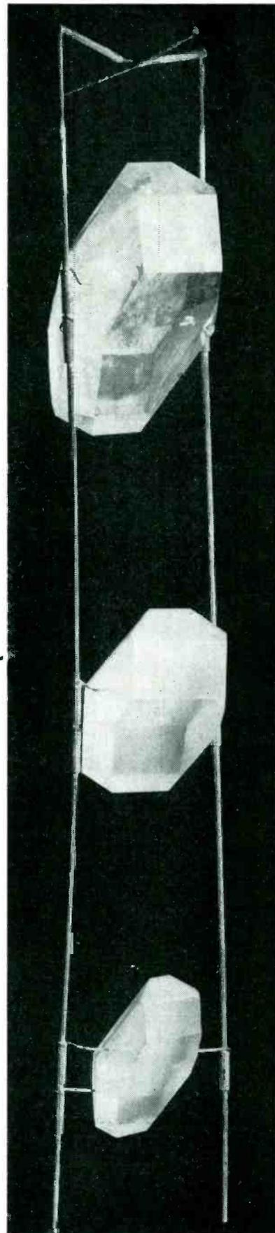
Examples of large quartz crystals grown by autoclave technique in 32 days. Weights, from top to bottom, are 321 grams, 143 grams and 71 grams
