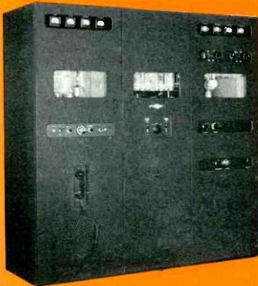
Collins 231D high frequency Autotune<sup>®</sup> transmitter. The power output is 2.5 to 5 kilowatts, depending on frequency and type of emission.
