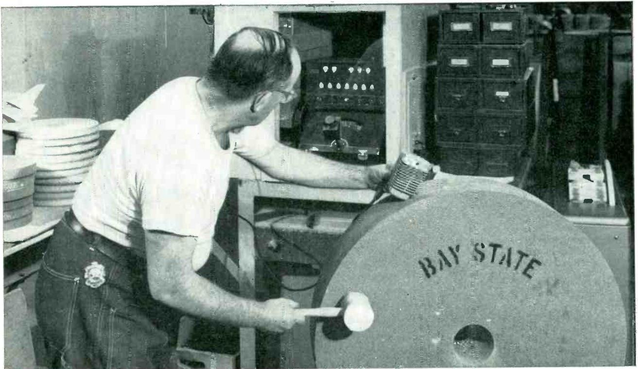
Grinding wheel being tested for flaws by measuring its ringing frequency with a stroboscopic frequency meter. Instrument is enclosed in a temperature-controlled and dust-free compartment, cover of which is open here
