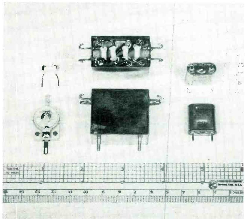
Components making up the filter are familiar. Zero-temperature-coefficient capacitors are used. High-grade variable capacitors can be used to determine parameters
