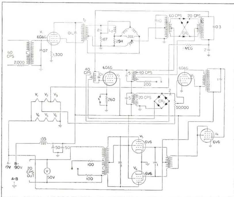
FIG. 3—Schematic of the chronograph power amplifier, with phasing-control selsyn in upper center
