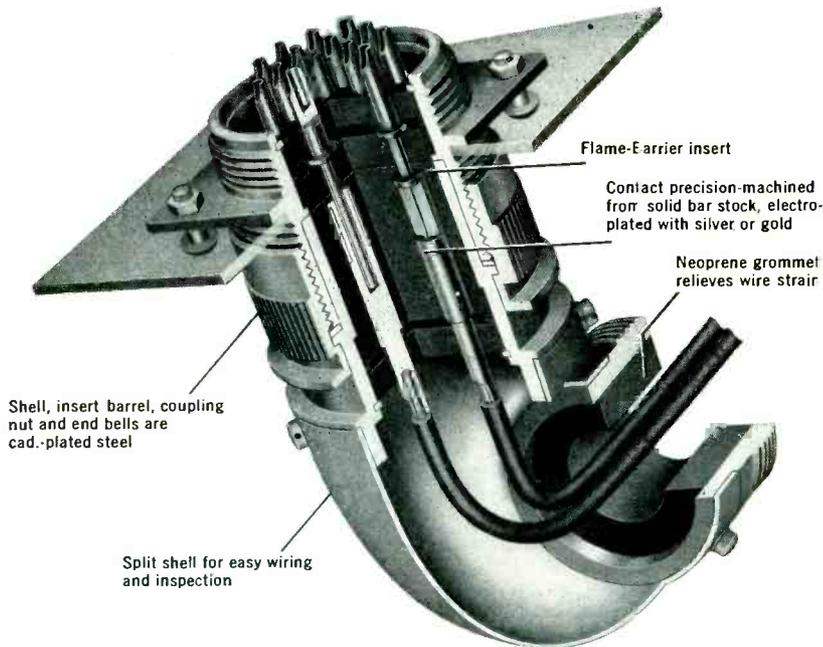
Here is another example of the care Cannon Electric takes in developing a connector for specialized use. This is the Firewall Connector to prevent the spread of a possible aircraft engine fire through the bulkhead into wing sections.
