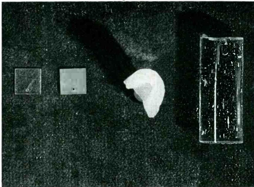
FIG. 1—Quartz crystals grown by Nacken process. Transparent quartz plate at left was grown from seed plate next to it. Rod of clear Vitreosil (amorphous silica) is at right, and partially recrystallized section of this rod is next to it
