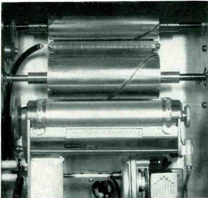
FIG. 1—Remodeled chart recorder for use as a spark chronograph. Special waxed recording paper has been removed to show details
