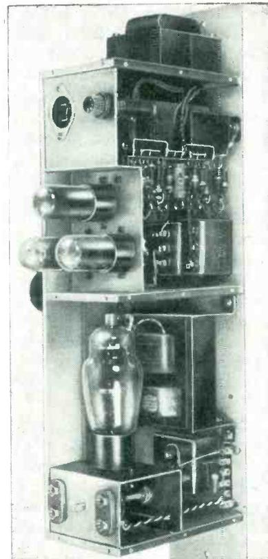
Rear view of spark generator with shield covers removed
