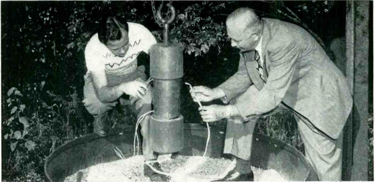
Harvesting of an autoclave in which quartz crystals have been grown at high temperature and pressure. Operators are removing thermocouples that measured temperature differential along length of steel container. Wire frame in bomb supports wafer-thin quartz seed plates on which crystals grow
