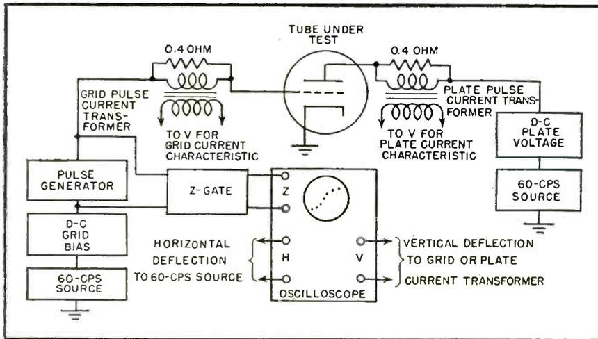
FIG. 1—Plate voltage is swept over desired range by 60-cycle a-c voltage superimposed on d-c voltage, while grid is driven by pulses riding on top of 60-cycle grid voltage. Resulting dots on oscilloscope screen trace out the desired characteristic
