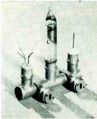
FIG. 1—Special BTL tube for amplification at 48,000 mc
