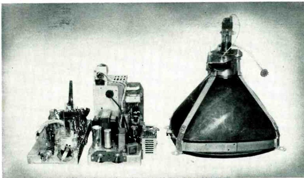
NEW PHILCO TV SET using electrostatically focused picture tube weighs 27-pounds 8-ounces
