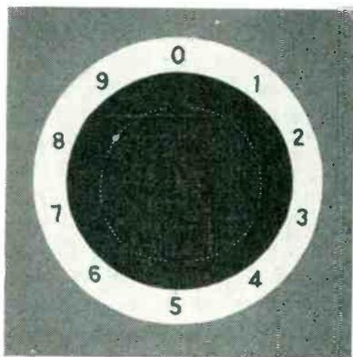
Typical pattern display on cathode-ray chronoscope tube. Small dots are 0.1 millisecond apart, with every tenth dot blanked out to facilitate counting dots clockwise from zero to enlarged dot representing time difference
