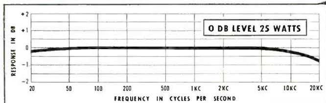
Curve represents an average response of the ten transformers in this series. Units used for this test were drawn at random from current Stancor stock.
