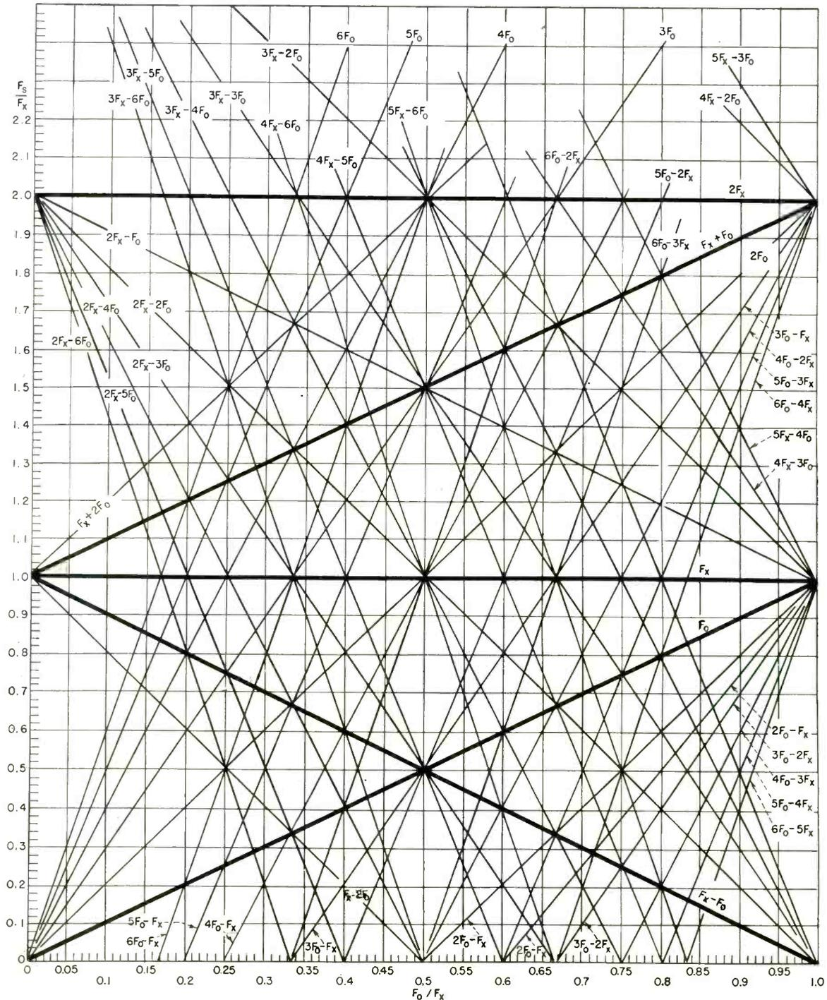
Mixer chart, with  $F_o$  and  $F_x$  as mixer input frequencies (with  $F_x$  the higher) and  $F_s$  as desired output frequency. Lines intersected when tracing straight up from value of  $F_o/F_x$  represent combination frequencies, values of which can be found either from labels on lines or from scale of ordinates. Only intersections near desired combination (sum or difference) need be considered. When  $F_x$  is fixed, ordinate scale can be marked to give frequency directly.
