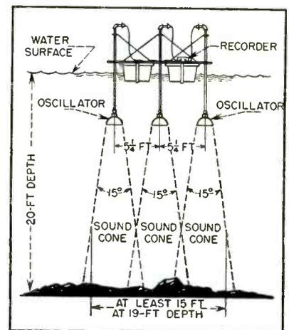
FIG. 1—Sweeping system employing three ultrasonic oscillators connected in parallel
