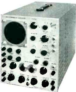
The advantages of the direct coupled oscilloscope are now available in the region of 10 mc. Not only is it possible to measure the duration and amplitude of a waveform, but also the D.C. level at which it occurs.
