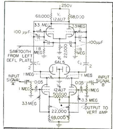
FIG. 1—Circuit of electronic switch used to obtain two simultaneous and independent traces on an oscilloscope
