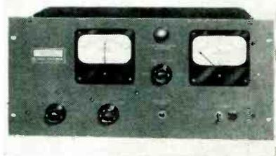
and an audio output for aural monitoring. Frequencies from 30 mc to 175 mc may be monitored, and the instrument is sensitive enough to monitor mobile units some distance away.
