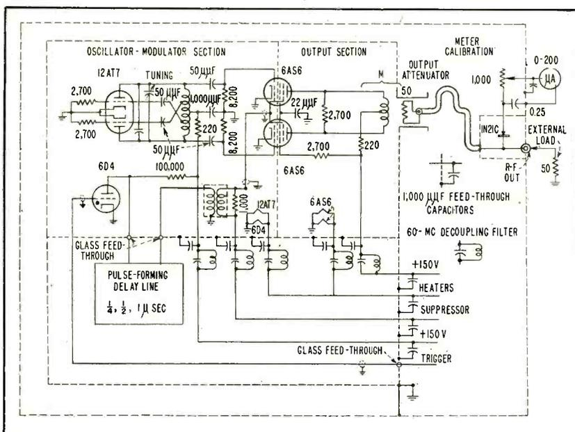
FIG. 2—Schematic diagram of the r-f section of the radar test generator
