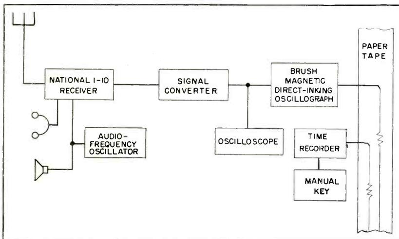
FIG. 5—Receiving and recording setup used on the ground
