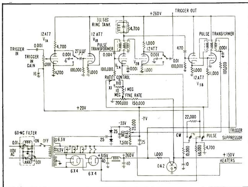
FIG. 4—Schematic diagram of the power supply and trigger chassis for the generator
