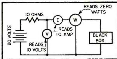
The apparent power dissipation in the black box is 10 watts according to the voltmeter and ammeter, but the zero wattmeter indication is a contradiction of this. What is in the little "black box?"
