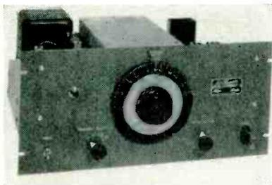
age conditions; no electrolytic capacitors used; all capacitors are hermetically sealed in oil or mica. Its chief uses are: amplifier testing, broadcast transmitter audio response, loudspeaker resonance tests, signal generator modulation, and ultrasonic voltage source.
