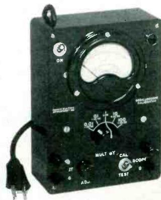
scope it enables the operator to make measurements of voltages within this range. It has the added feature of being calibrated directly in peak to peak volts and decibels as well as rms volts. Price is \$24.95 complete with tube and instructions.
