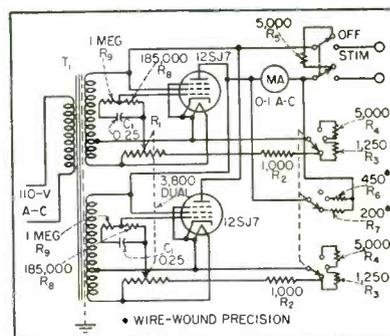
FIG. 2—Circuit diagram of the constant-current stimulator
