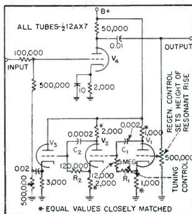
FIG. 1—Selective amplifier tunable with approximately constant absolute bandwidth and constant gain between 300 and 6,000 cycles per second
