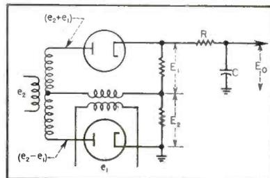
consider the phase detectors to be square law, then the d-c voltages appearing across the load resistors will be, respectively
