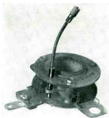
is varied by a sliding steel collar controlled by a lead screw at the output end of the flexible shaft. The shaft is formed of high-strength bronze, and is sometimes enclosed within an insulating plastic or braided cotton sleeve. While normally controlled from the rear of the set, some units are designed to operate from the front panel.
