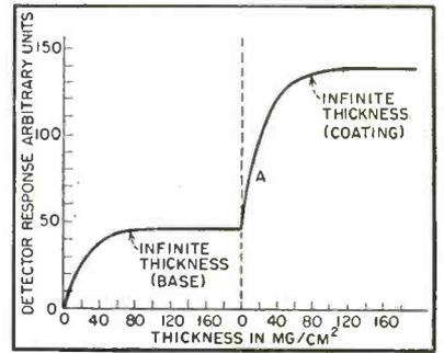
FIG. 2—In making coating-thickness measurements, only linear portion of curve (A) is used
