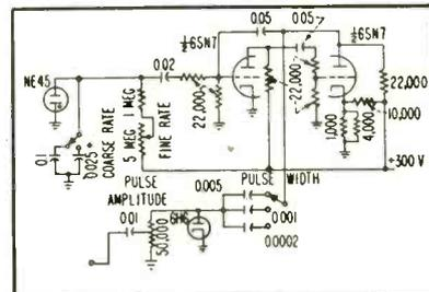
FIG. 1—Circuit of the test generator for simulating Geiger-counter pulses
