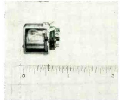
the dynamically balanced armature provides the 1001 with high resistance to vibration and shock and sudden changes in acceleration and direction. It is a spdt 28-volt d-c relay with contacts rated at one ampere noninductive load.
