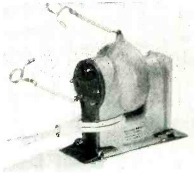
trated has transformer, coil and core entirely encased in a molded plastic form. The high dielectric strength of the plastic provides greater protection against corona discharge and the resultant fire hazards. Reduction of acoustical radiation is another important feature. When used in a high-efficiency 66 to 70-deg circuit, it will provide full deflection and up to 14-kv anode potential.
