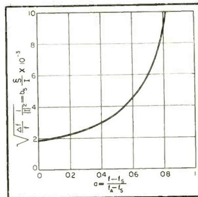
FIG. 1—Ratio of amplitude to current for ammonium dihydrogen phosphate crystal cut (zxw) 45 deg, thickness shear mode
