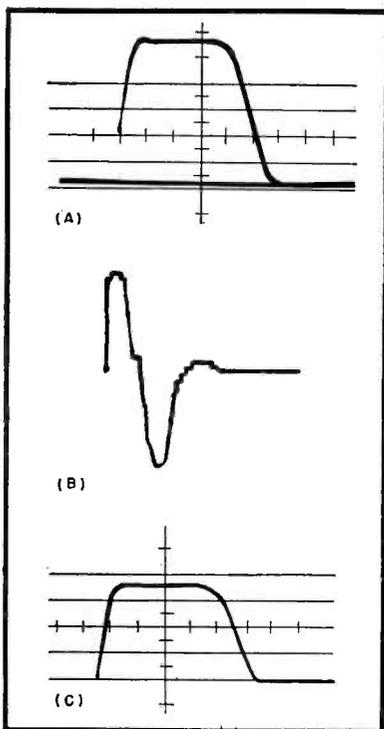
FIG. 3—Voltage waveforms at output of pulse-forming network (A), at Z-output of gate (B), and at secondary of pulse transformer (C)
