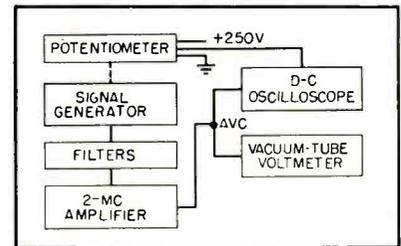
FIG. 4—Test equipment used to adjust the filter. The potentiometer and signal generator are driven simultaneously by hand
