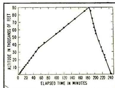
FIG. 4—Time-altitude record of a typical flight
