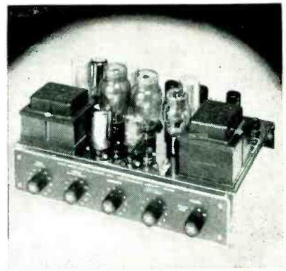
amplifier has a frequency response flat from 12 to 22,000 cycles; harmonic distortion less than 0.5 percent at full 20-watt output; first-order difference-tone intermodulation less than 0.1 percent at full output; and hum level of 84 db or more below full output. It also features a noise suppressor which virtually eliminates record scratch and rumble without affecting the music response.
