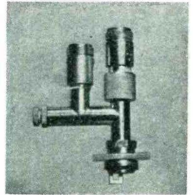
S Band Crystal Mixer, variable oscillator injection, illustrated .....\$17.50
