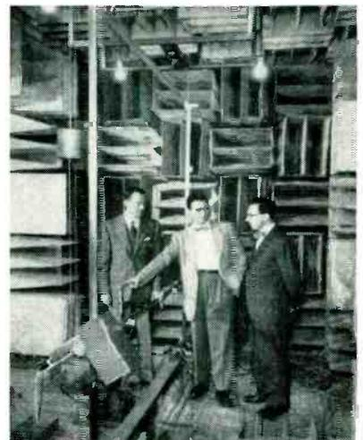
In the acoustics laboratory at the Massachusetts Institute of Technology, studies are being made to find methods for producing quieter, more restful homes and offices with the aid of the sound-mapping equipment shown. Room shown above contains 256 loudspeakers capable of duplicating the noise made by a field-artillery battallion. Sensitive microphone moves back and forth to cover space in test room, and equipment below plots a sound contour map showing sound levels at different positions
