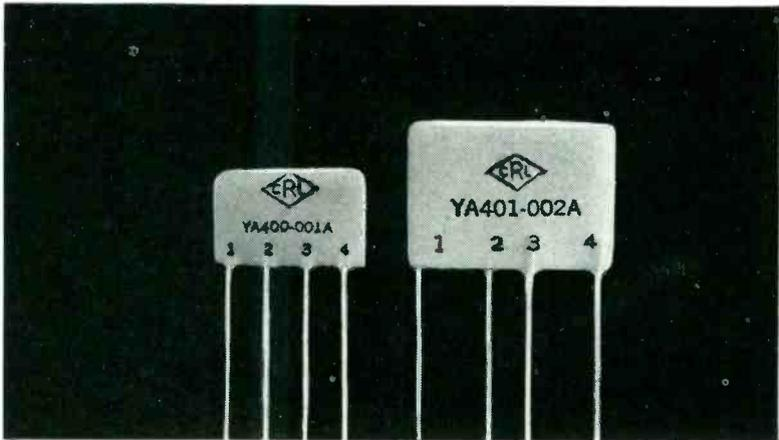
Centralab Triode Couplates save space and weight, replacing 5 components normally used in audio circuits. They consist of 3 capacitors and 2 resistors bonded to a dielectric ceramic plate. Available in variety of resistor and capacitor values. For complete data, check coupon No. 42-6 — Couplate, and No. 42-27 — Model 2 Couplate.
