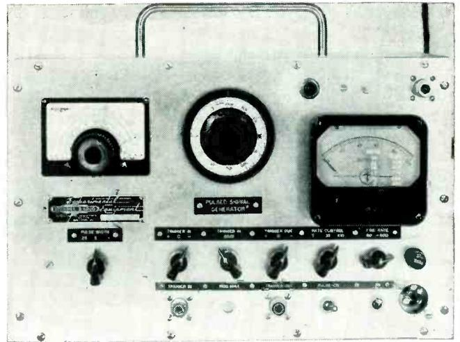
Front-panel view of the pulsed-signal radar test generator
