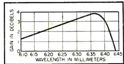
FIG. 4—Curves show the gain of the new tube as a function of wavelength
