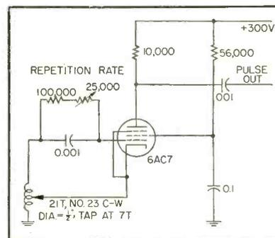
FIG. 1—Schematic diagram of simple blocking-oscillator trigger generator
