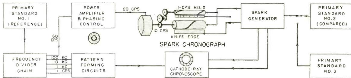
Any crystal clock at CRPL (like No. 1) can be used to drive the spark recorder through a frequency-divider chain and power amplifier. The phasing control allows adjustment of the starting point. A waxed-paper chart, calibrated in 0.002-sec strips, is drawn at three inches a day between the lower knife-edge and the spiral helix that rotates ten times a second.
