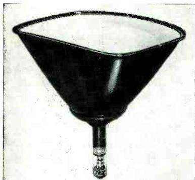
Seventeen-inch rectangular metal 17GP4, incorporating new electrostatic-focus gun. The electron gun is readily adaptable to all current glass or metal picture tubes. No change is needed in either the deflecting yoke or ion-trap magnet
