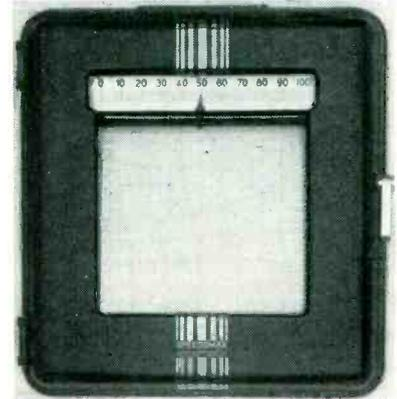
urements with thermocouples, and speed measurements. Calibrated d-c millivolt range is adjustable from a minimum across-chart span of 1.1 mv to a maximum range span of 22 mv. Uncalibrated coarse and fine rheostats provide maximum zero suppression of -50 or +50 mv, continuously adjustable between these limits.
