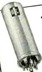
**Type UMP** An old favorite now completely Hermetically Sealed if desired or necessary. For use in all TV, radio and rectified DC circuits. Twist-prong mounted, available in single, dual, triple and quadruple units. Wide range of capacities in working voltages from 3 to 600 VDC. Heavily tinned soldering lugs, seamless drawn aluminum cans.
