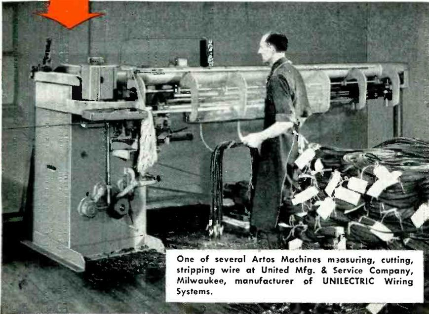
One of several Artos Machines measuring, cutting, stripping wire at United Mfg. & Service Company, Milwaukee, manufacturer of UNILECTRIC Wiring Systems.
