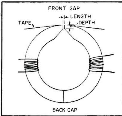
Typical magnetic recording head showing how the front gap is reduced in depth
