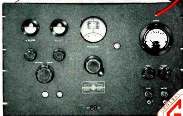
**Type 1107-A Interpolation Oscillator** is used to measure the difference between the unknown frequency and a known harmonic of the Standard. The direct-reading linear scales of 0 to 5,000 and 5,000 to 10,000 cycles make possible the rapid evaluation of the frequency difference *by addition only*. The actual frequency range is 0 to 5,000 cycles.
