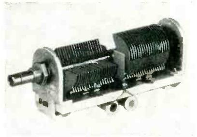
**FIG. 3—**As the capacitance of one section increases, that of the other decreases, but the total capacitance remains fixed. The fixed positive and negative temperature coefficient capacitors are mounted under the modified two-section variable
