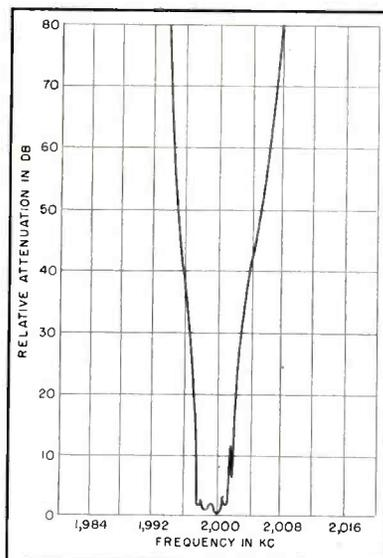
FIG. 5—Selectivity curve for a typical crystal filter
