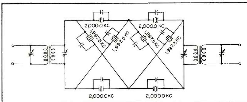
FIG. 1—Circuit for the 2-mc filter using eight crystals
