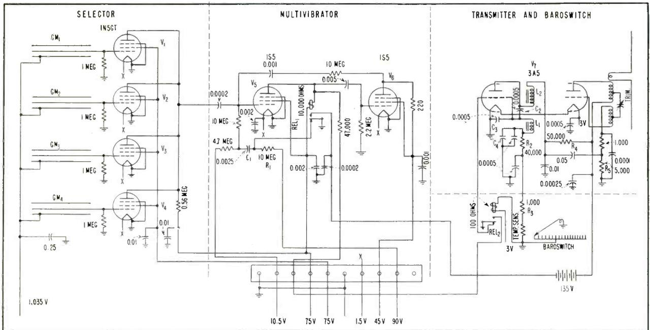
FIG. 2—The complete balloon-borne unit, with dashed lines indicating sub-assemblies
