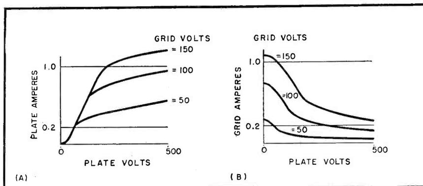
FIG. 5—Examples of families of plate-voltage characteristic curves obtained for type 6C4 miniature tube
