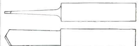
Solid sintered carbide flat drill used in automatic machines on phosphor bronze. (6444)
