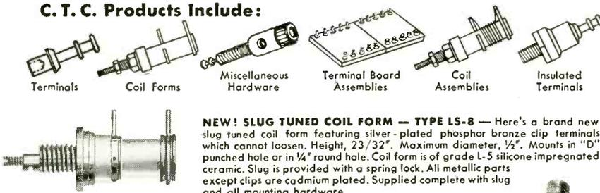
**NEW! SLUG TUNED COIL FORM — TYPE LS-8** — Here's a brand new slug tuned coil form featuring silver-plated phosphor bronze clip terminals which cannot loosen. Height, 23/32". Maximum diameter, 1/2". Mounts in "D" punched hole or in 1/4" round hole. Coil form is of grade L-5 silicone impregnated ceramic. Slug is provided with a spring lock. All metallic parts except clips are cadmium plated. Supplied complete with slug and all mounting hardware.
