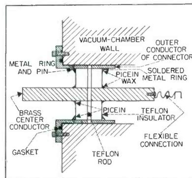
FIG. 4—Cross section of the coaxial connector, part of which is visible in Fig. 3
