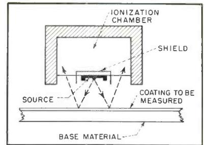
FIG. 1—Thickness of thin coatings can be measured by measuring amount of radiation reflected by a surface
