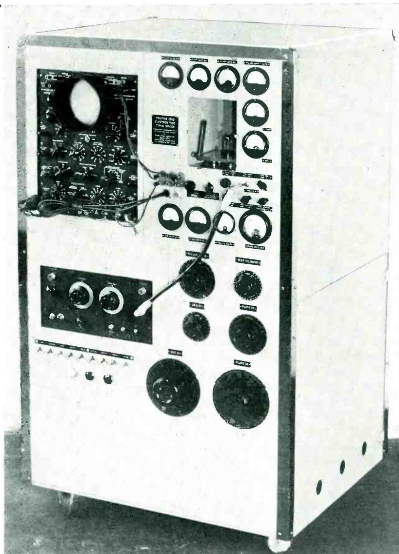
Electron-tube curve tracer using pulse techniques for displaying on cathode-ray screen the characteristics up to high peak power levels in the positive grid region. Tube being tested is in recess at upper right
