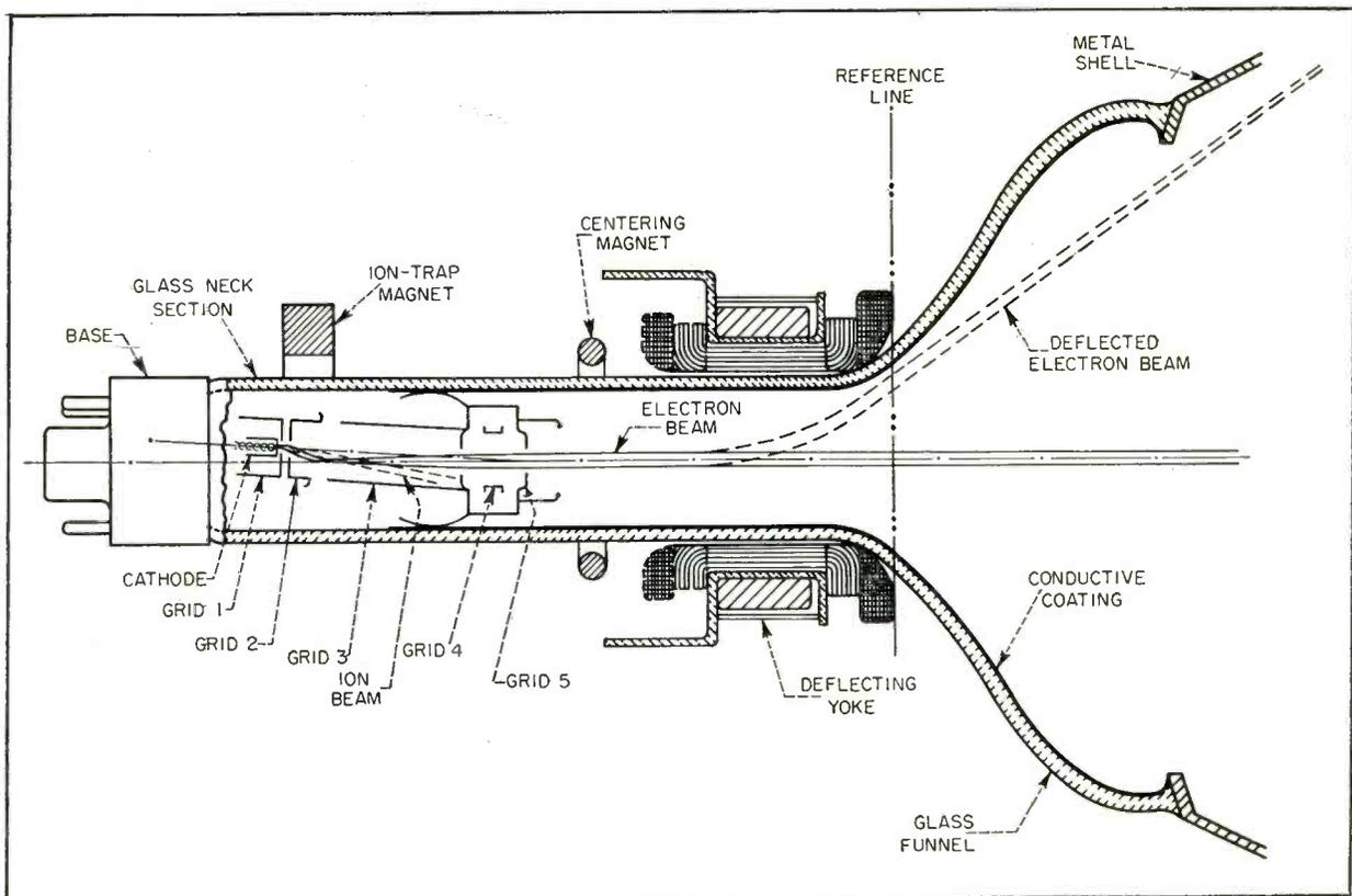
FIG. 1—Cross-section of new electrostatic-focus gun, showing path of electron beam and location of centering magnet
