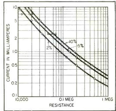
FIG. 1—Curves showing the limits of regulation. For all resistance lines which intersect the desired current line below the 2-percent curve, the current will change less than 2-percent from the present value. Similar manipulation applies to the 5 and 10-percent curves
