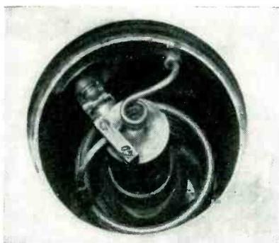
FIG. 3—Looking down into the vacuum chamber, showing the small water-cooled work coil, the larger resonant-circuit coil with its tuning capacitor and, at the upper left, the coaxial connector
