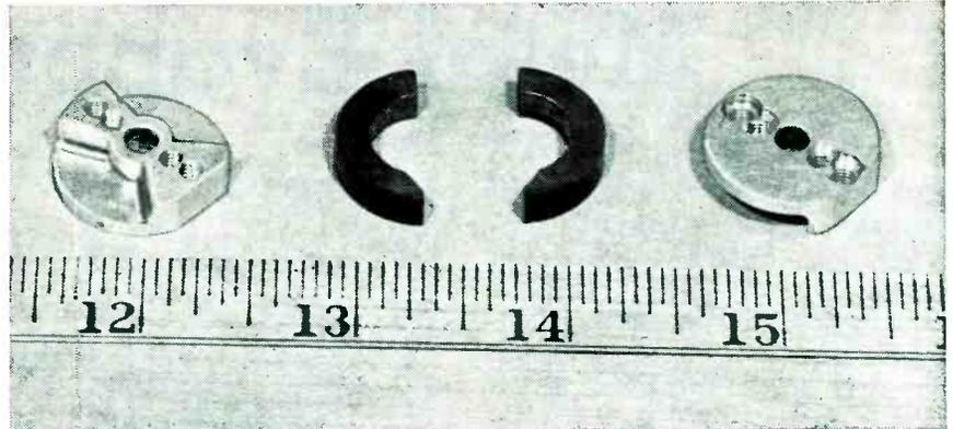
FIG. 1—Components of an experimental magnetic recording head using a core made of Ferramic E or Ferramic G. Core was obtained by cutting a toroid of  $\frac{1}{8}$ -in. outer diameter in half and then reducing one gap in depth
