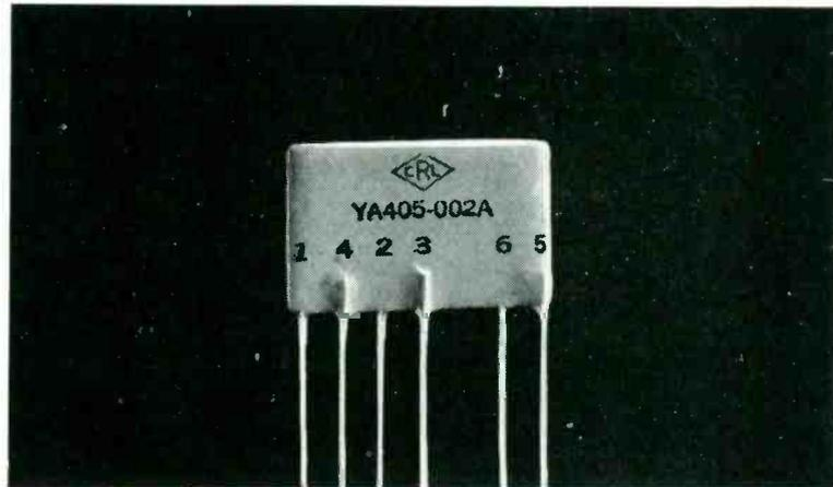
Pentode couplers are complete interstage coupling circuits consisting of 3 capacitors and 3 resistors on a small 6 lead ceramic plate. Compared with old-style audio circuits, they reduce soldered connections 50% — wiring errors accordingly. Big saving in space and weight. For complete data, check coupon No. 999 — Pentode Couplate.
