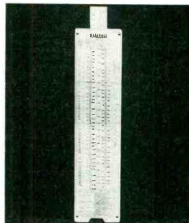
slide rule, the Datarule, illustrated above. In making any type of change in the coils or winding—whether in the form of frequency, voltage, number of turns, connection, speed or size of wire—or in testing or determining the effect of such a change in existing design, the Datarule indicates the effects of such change on the other related factors in coil or winding design.
