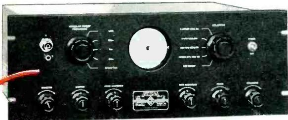
**Type 1106-A Frequency Transfer Units**, of which there are three, contain a heterodyne frequency meter and heterodyne detector, with direct-reading scales. The ranges of the three units are: 100 kc to 2,000 kc; 1 Mc to 10 Mc and 10 Mc to 100 Mc. Harmonic output of the frequency meter can be used at frequencies considerably higher than those covered by the dial ranges.
