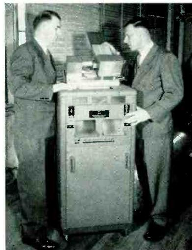
Electronic currency counter to be used by Treasury Department. Packets of lower halves of bills enter machine in trough at top right. Left chute on front of machine is for rejected packets and right chute is for correct ones
