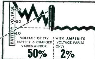
Amperite REGULATORS are the simplest, lightest, cheapest, and most compact method of obtaining current or voltage regulation . . . For currents of .060 to 6 Amps. . . Hermetically sealed; not affected by altitude, ambient temperature, humidity.
