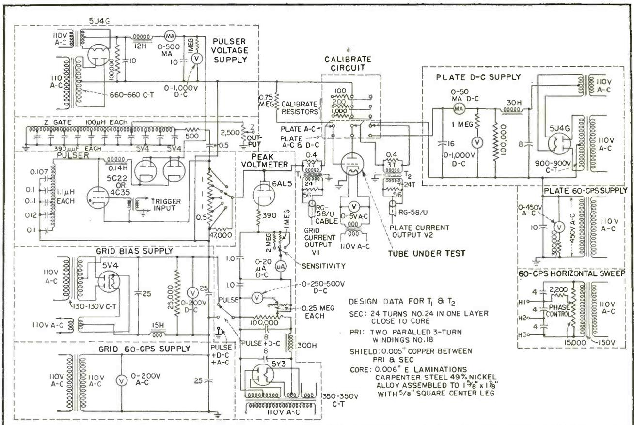
FIG. 2—Complete circuit diagram, including all power supplies since they play a major part in the operation of the tracer
