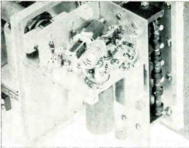
FIG. 1—The r-f section with the shield removed
