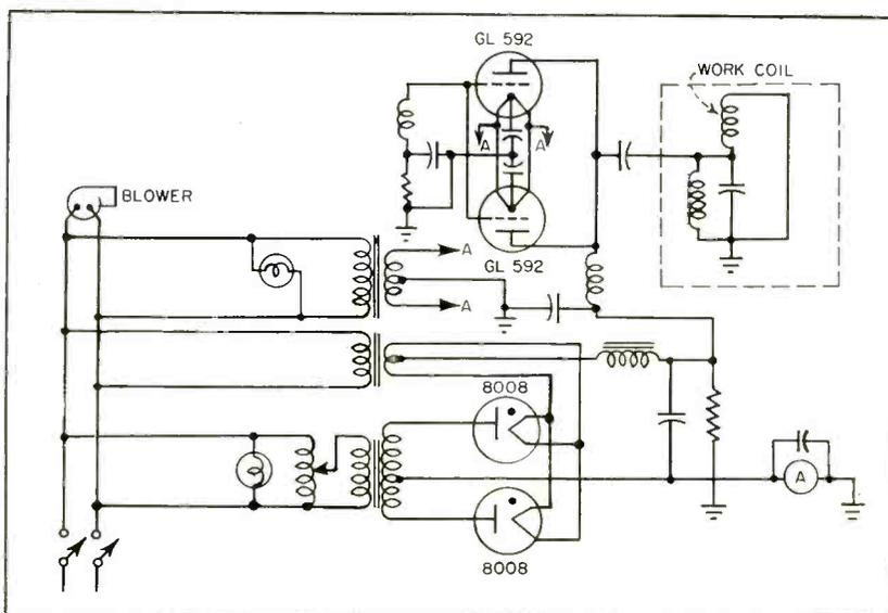
FIG. 1—Circuit of the high-frequency metal evaporator. Protective contactors are not shown
