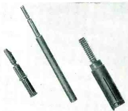
Phosphor bronze terminals for micro-wave equipment turned in Swiss screw machines.
