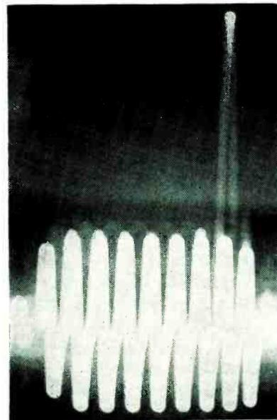
FIG. 6—Oscilloscope trace of voltage applied to grid of the chronoscope. Every tenth wave is attenuated. A 10-pps time signal is at right
