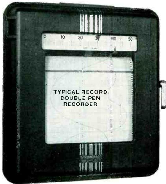
To save the researcher from tedious curve plotting, here are 4 new Speedomax Recorders. There's a double-pen recorder to put two continuous curves on one chart . . . there's a recorder for "X-Y" curves . . . there's an adjustable range—adjustable zero recorder for narrow ranges at high levels . . . and there's a recorder for photomultiplier tubes.
