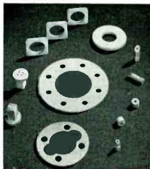
Teflon's loss factor is less than 0.0005; its dielectric constant only 2.0—at all frequencies measured to date. Teflon is serviceable throughout the entire temperature range of  $-110^{\circ}$  F. to  $575^{\circ}$  F. with negligible change in critical electrical characteristics. Teflon is tough, somewhat resilient, weather-proof, has zero water absorption and is absolutely non-corroding.
