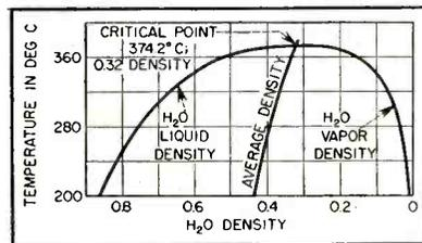
FIG. 2—Liquid-vapor density relations of water near its critical temperature at which density of liquid and vapor are equal
