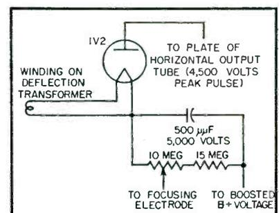
FIG. 3—Rectifier circuit for providing focusing voltage
