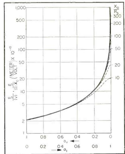
FIG. 2—Amplitude-to-voltage and amplitude-to-current ratios as functions of  $a$  for AT and BT cut quartz crystals
