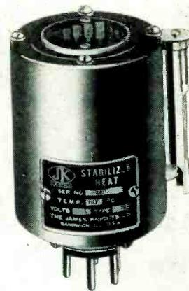
in frequency) in that the variable electrode only moves up and down in guides like a piston. Frequency range is from 400 kc to 1,750 kc. Nominal temperature is 60 deg  $\pm$  1 deg. Adjustable frequency is  $\pm$  0.01 percent. It features a 6.3-volt, 1-ampere heater. The unit can be supplied with octal base with or without thermometer, and can be factory set for operation at specific temperatures.
