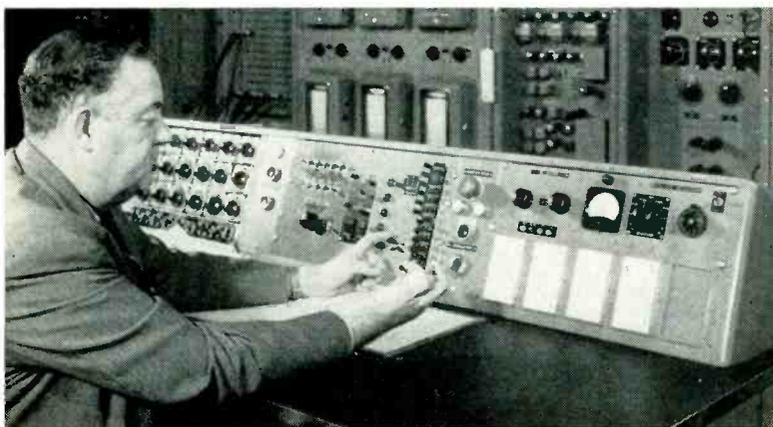
**T**HE COVER PHOTOGRAPH this month dramatizes one important application of the 4,000-tube Project-Typhoon electronic analog computer—determining the optimum trajectory of a radar-controlled, rocket-propelled guided missile for interception of an attacking bomber target with minimum waste of time and fuel. The models identify the paths traced by the inking pens on the elevation plotting board that shows results. If the two pens hit each other, interception is possible.
