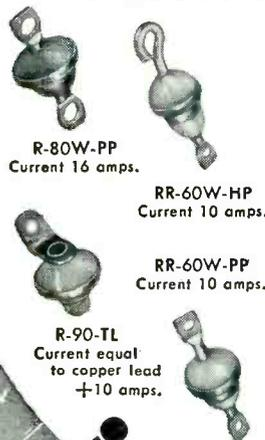
A completely new line of double barrel terminals that provide added protection against flashover without any appreciable increase in terminal size. The double barrel results in a longer leakage path on both ends of the terminal while the upper barrel increases the mechanical strength of the terminal and facilitates soldering. For information call or write today.
