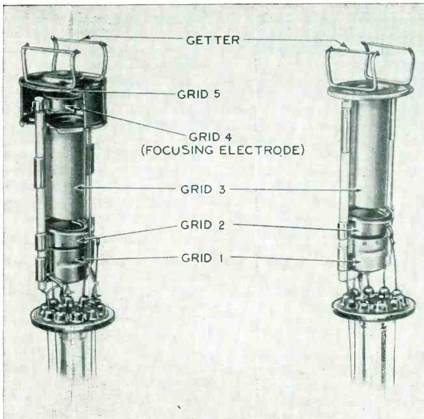
FIG. 2—Structure of electrostatic-focus gun compared with magnetic-focus gun
