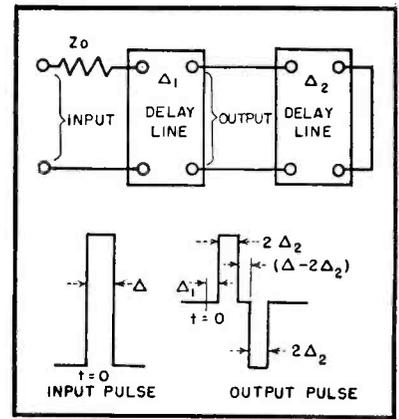
FIG. 4—Transmission line shorted at far end serves as gate that brightens trace during flat-top portion of grid pulse
