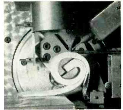
Package of half-notes firmly locked in jaws of spindle (center). Combined action of friction band (curled around outer contour of packet) and air jet (air hose, center) cause each note to break light beam of phototube (left)
