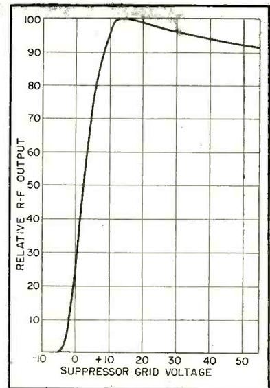
FIG. 3—Characteristic curve of 6AS6 class-C r-f amplifier with constant control-grid excitation
