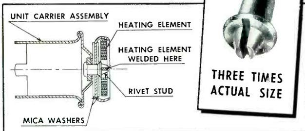
Small enough to put under your fingernail, this rivet is made by Progressive for The Cuno Engineering Corporation. Used in an automotive cigarette lighter, it serves as a post to which the center of the heating coil is spot welded and as a rivet for fastening the burner cup to the lighter shell.
