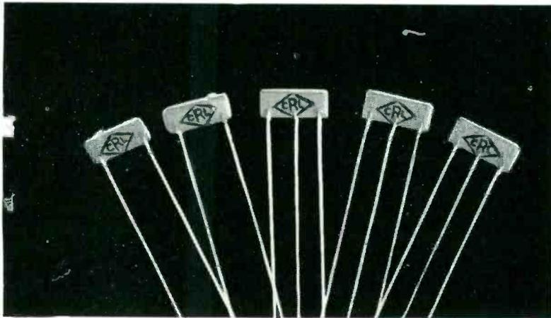
Actual size photo of plate capacitor, resistor, and resistor-capacitor units. Because of size and ease of installation, they easily fit miniature and portable electronic equipment — overcome crowded conditions in TV, AM, FM, and record-player chassis. For complete data, check coupon No. 42-24 — Ceramic Plate Components.
