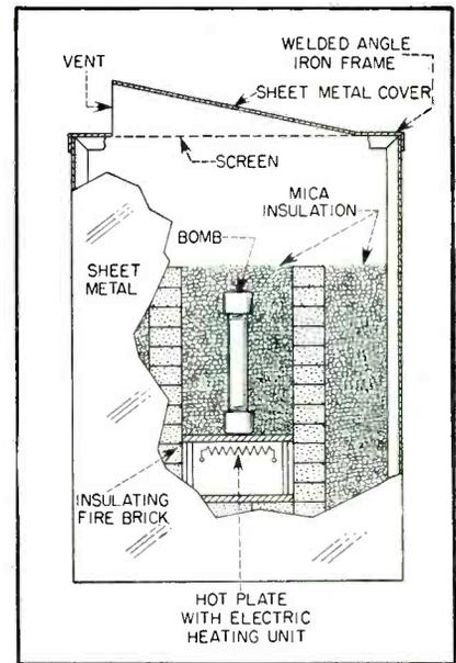
FIG. 4—Cross-section of furnace in which bomb is kept at 400 C
