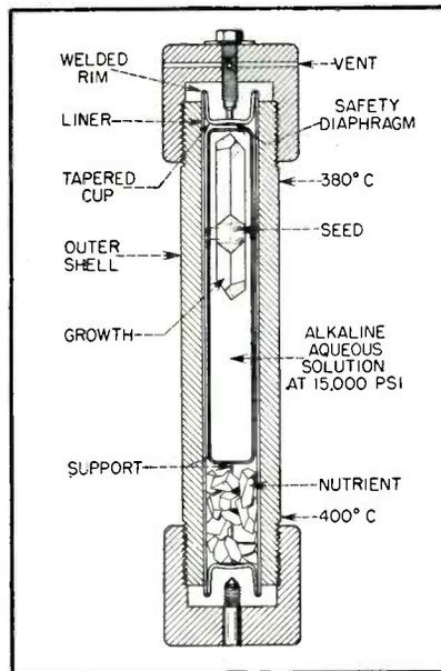
FIG. 3—Cross-section of steel bomb in which quartz crystals are grown
