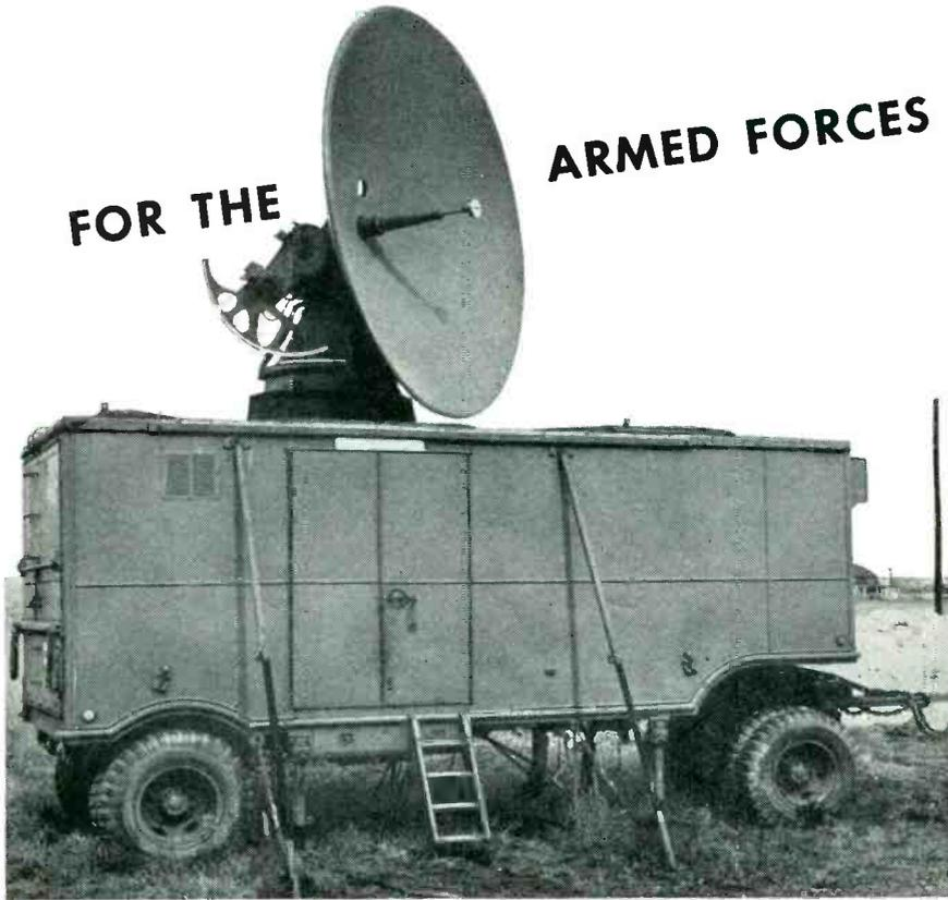
This radar field unit for high speed missile tracking is equipped with a Workshop 10-foot parabolic antenna system. The principal problem in its development was to provide a good primary pattern on the feed, with an accurately predictable "crossover." Through the use of a slotted cavity feed, Workshop engineers were able to achieve the "crossover" and gain desired.
