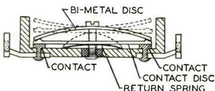
Action of new Type M thermostat is extremely precise because bi-metal element is electrically independent. Bi-metal disc rests on top of rigid Monel-backed contact disc, which carries current on its silver side because of minimum electrical resistance. Since bi-metal carries no current, artificial cycling and life-shortening "jitters" are eliminated.
