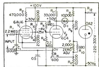
FIG. 1—Circuit diagram for d-c vtvm with feedback over two stages
