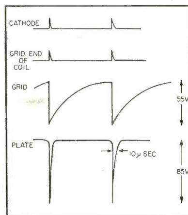
FIG. 2—Typical waveforms of blocking oscillator for component values given in Fig. 1
