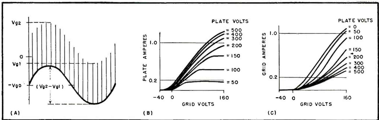
FIG. 6—Method of superimposing pulses on a-c grid voltage, and examples of families of grid-voltage characteristic curves obtained for type 6C4 miniature tube
