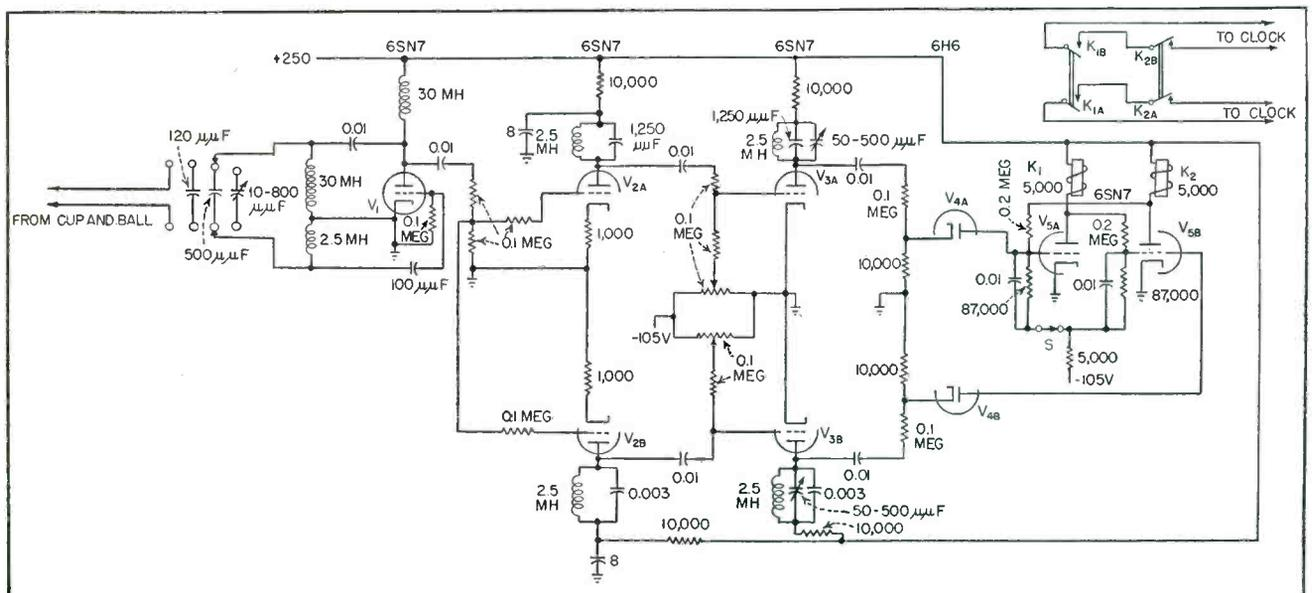
FIG. 1—Complete circuit diagram of the capacitance-change timer
