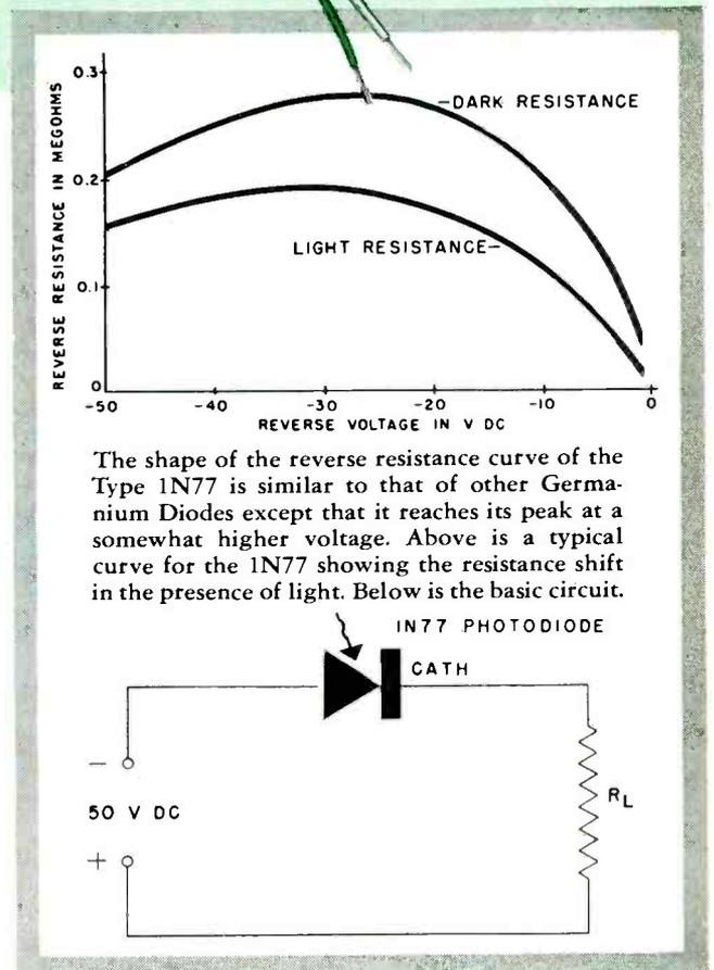
The shape of the reverse resistance curve of the Type 1N77 is similar to that of other Germanium Diodes except that it reaches its peak at a somewhat higher voltage. Above is a typical curve for the 1N77 showing the resistance shift in the presence of light. Below is the basic circuit.
