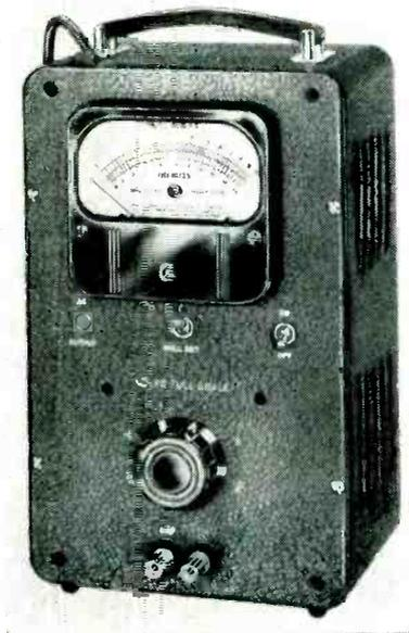
ance is 2 megohms shunted by 8  $\mu$ mf on the two most sensitive ranges, and by 15  $\mu$ mf on the other ranges. The amplifier section of the voltmeter may be used separately as amplifier flat within 1/2 db up to 2 mc with a maximum gain of 60 db and an output impedance of 500 ohms.
