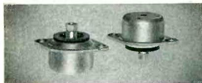
Upright and inverted types are available for two-hole or four-hole mounting. Unit mountings are one inch in diameter and 1-1/32 inches high under maximum rated load. Load ratings are 0.1 to 3.0 pounds per mount. The mountings weigh only 5/16 ounce each.
