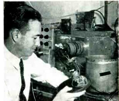
Operating multiplier phototube at 4,000 volts for short periods of time, instead of 1,000 volts prescribed, extends range of scintillation counter
