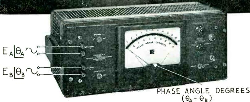
TIC's New 320-A Phase Meter is the first commercially available instrument for the direct measurement of the phase difference between two recurrent mechanical motions or two electrical signals independent of amplitude, frequency, and wave shape.
