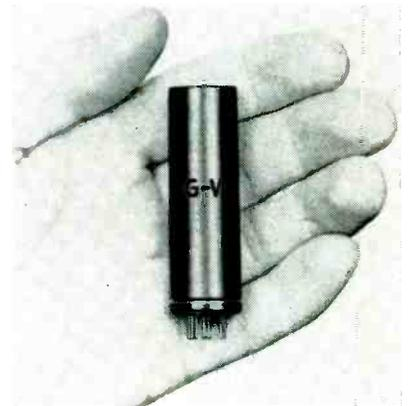
screw located outside the sealed space. This screw permits the timing to be changed over a 5 to 1 range. The miniature size, 3/4 in. in diameter and 2 3/8 in. seated height, fits a 7-pin miniature tube socket. Contacts are single pole, rated at 6 amperes. Relays are available for any energizing voltage up to 125 and operate interchangeably on a-c and d-c.
