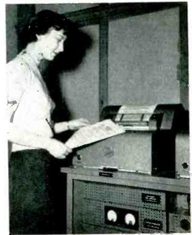
FIG. 2—Transmitted copy feeding from the recorder at a speed of  $\frac{1}{4}$  inch per second
