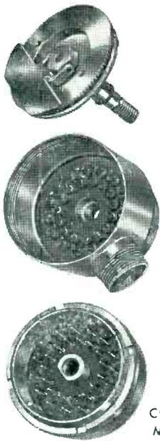
Our Series "R" Connectors were designed by us for the United States Signal Corps to provide water-tight and pressure-tight plugs and receptacles. They had to be compact and exceptionally strong. The special double lead center lock screw (with bale), which facilitates both engagement and disengagement, eliminates accidental disconnection. Cable entry can be oriented in any desired position.
