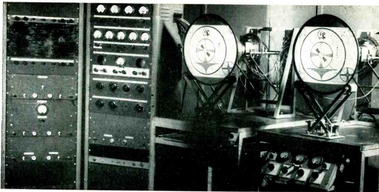
Dual magnetic-deflection test setup for side-by-side comparison of picture-tube resolution
