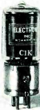
peak anode current, 8 amperes; maximum peak inverse voltage, 1,250 v; maximum peak forward voltage, 1,000 v. Grid shielding results in a grid-anode capacitance of only 1  $\mu\text{pF}$  with a grid-cathode capacitance of 10  $\mu\text{pF}$ . Critical grid current is less than 5  $\mu\text{a}$ .
