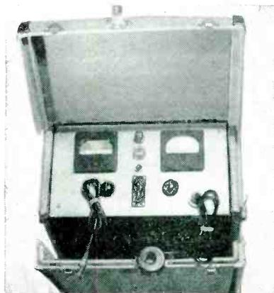
house or laboratory. An adaptation of the JAN gas ratio formulas uses standard, stabilized, regulated circuits for utilizing the c-r gun as its own ionization gage. A 3-in. meter reading 0.2 at midscale measures all electromagnetic types.
