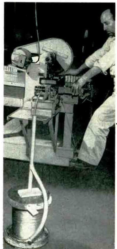
Spiral pipe whips around to unreele cable faster than from conventional rack, with no need to lift spool
