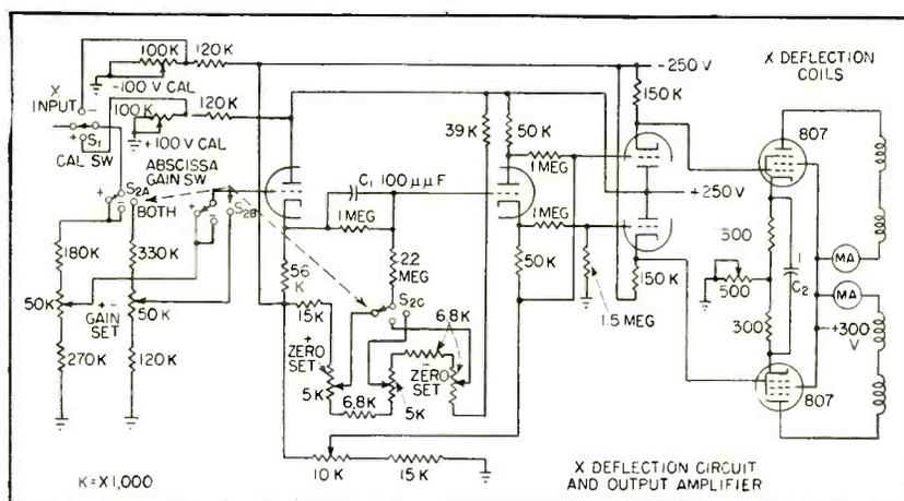
FIG. 4—Circuit for X-axis deflection must provide currents in phase with input voltage
