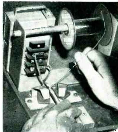
Setup for fast tinning of working face of soldering iron tip after grinding
