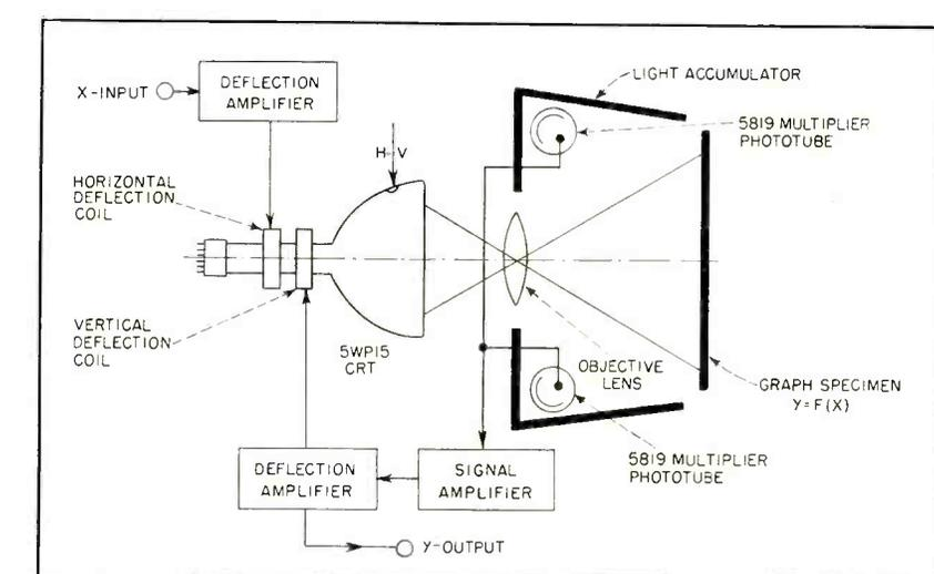
FIG. 1—Block diagram illustrates how phototube feedback loop forces crt trace to follow drawn curve of desired function
