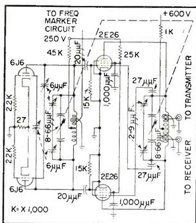
FIG. 4—Push-pull mopa variable-frequency oscillator is temperature controlled
