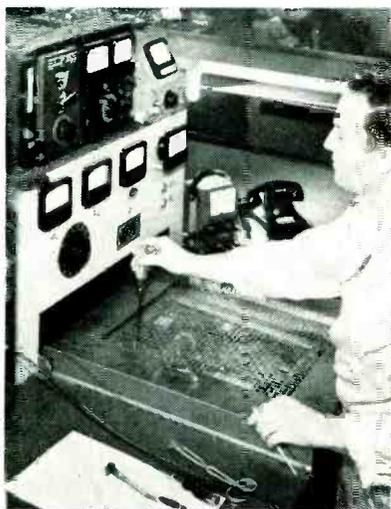
Close-up of new test bench, showing how alignment adjustments can be made through screen of shielded compartment
