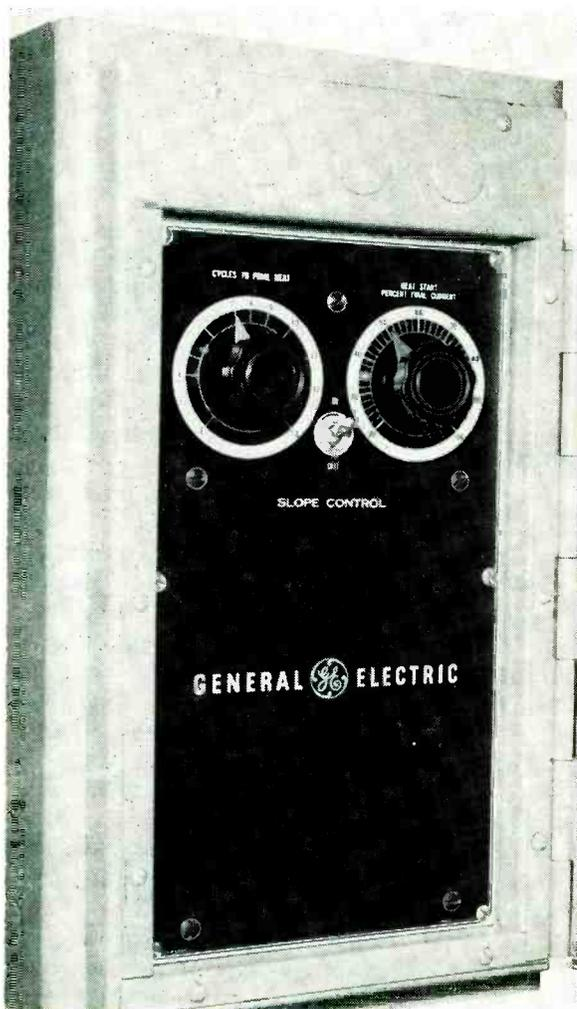
Slope control panel has three adjustments, labeled **CYCLES TO FINAL HEAT**, **IN-OUT** and **HEAT START—PERCENT FINAL CURRENT**
