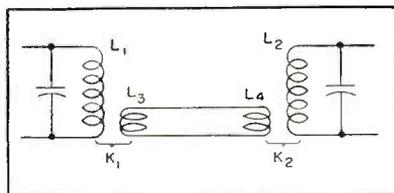
FIG. 6—Basic circuit of link-coupled tuned circuits. Maximum effective coefficient of coupling is realized when two links have same inductance
