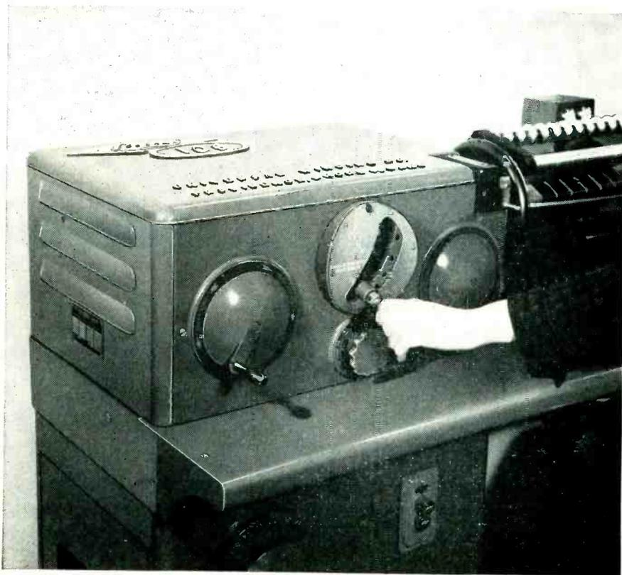
**LEESONA NO. 108 COIL WINDER**, award winner in the 11th Annual Product Design Competition sponsored by "Electrical Manufacturing," meets the demand for a modern manual paper feed machine for winding paper insulated coils in multiple or "stick" form. It winds coils from #20 to #44 (A.W.G.) in coil lengths from 1/4 in. to 3 3/8 in., in diameters, up to 5 in. round or square.
