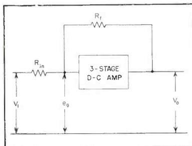
FIG. 1—Basic circuit showing how  $e_g$  tends towards zero voltage
