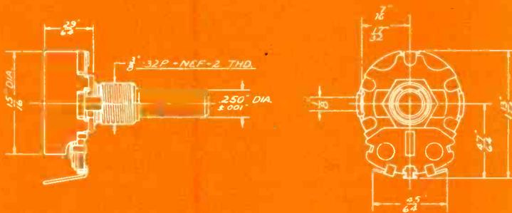
1 watt 70°C, 1 1/16" diameter variable composition resistor. Attached Switch can be supplied.
