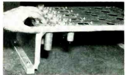
Use of temporary wood strips and masking tape to protect baked enamel finish of chassis during assembly
