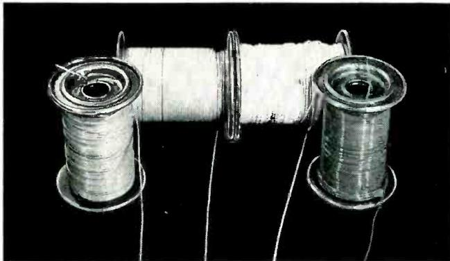
**3. This electronic hookup wire** is Kel-F insulated, capitalizing on the plastic's high temperature and high electrical resistance. In the production of this wire, Kel-F is extruded onto copper wire in conventional equipment. Commercially available from several sources, the wire comes in an assortment of keying colors.
