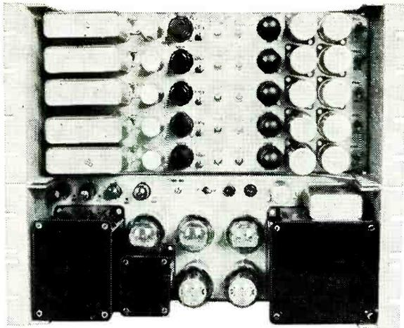
TYPE 1311 Video Distribution Amplifier is specifically designed to distribute video or synchronizing signals to several outlets. Thus, five separate equipments can be fed from a single synchronizing signal generator and monoscope combination.
