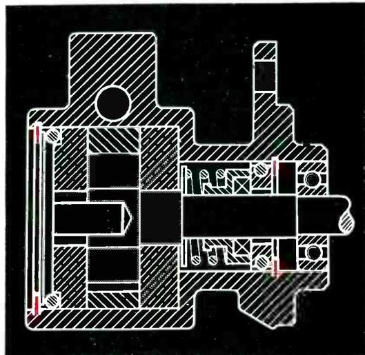
Using 2 Waldes Truarc Retaining Rings in their new Pump, saved the Procon Pump & Engineering Co., Detroit, \$1.48 per unit! With Truarc Rings, assembly is speedy, simple. Skilled-labor threading operations...stripped threads...maintenance are eliminated. Parts are firmly held together for life of unit!
