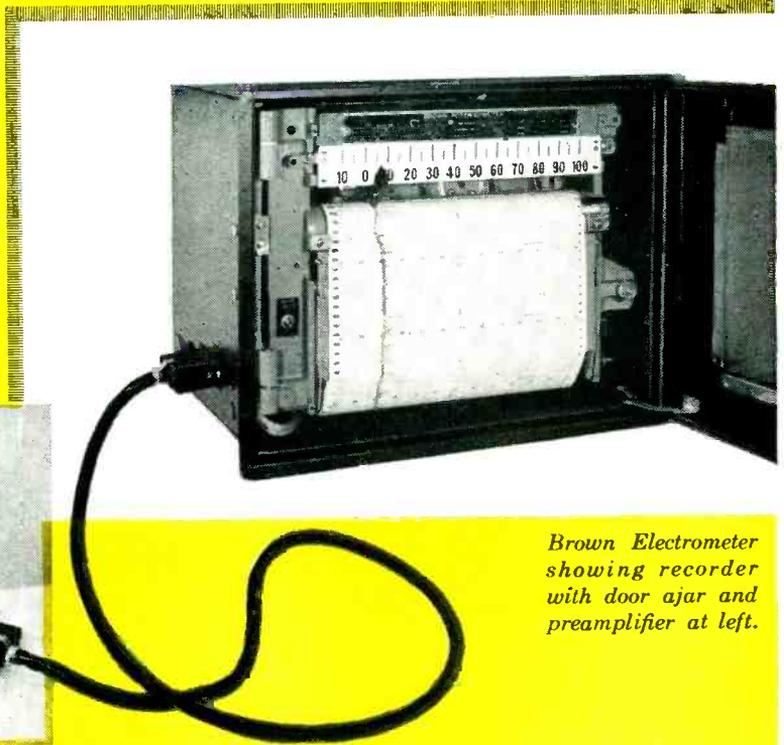
*Brown Electrometer showing recorder with door ajar and preamplifier at left.*
