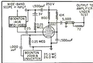
FIG. 6—Mixer used to modulate i-f with video
