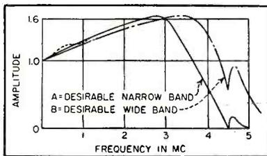
FIG. 3—Detector characteristics in terms of normalized amplitude vs frequency
