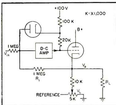
FIG. 8—Change of limit potential can be provided
