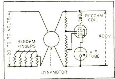
FIG. 2—Power amplifying and impedance watching abilities of stepped-resistance controller in a Motorola design
