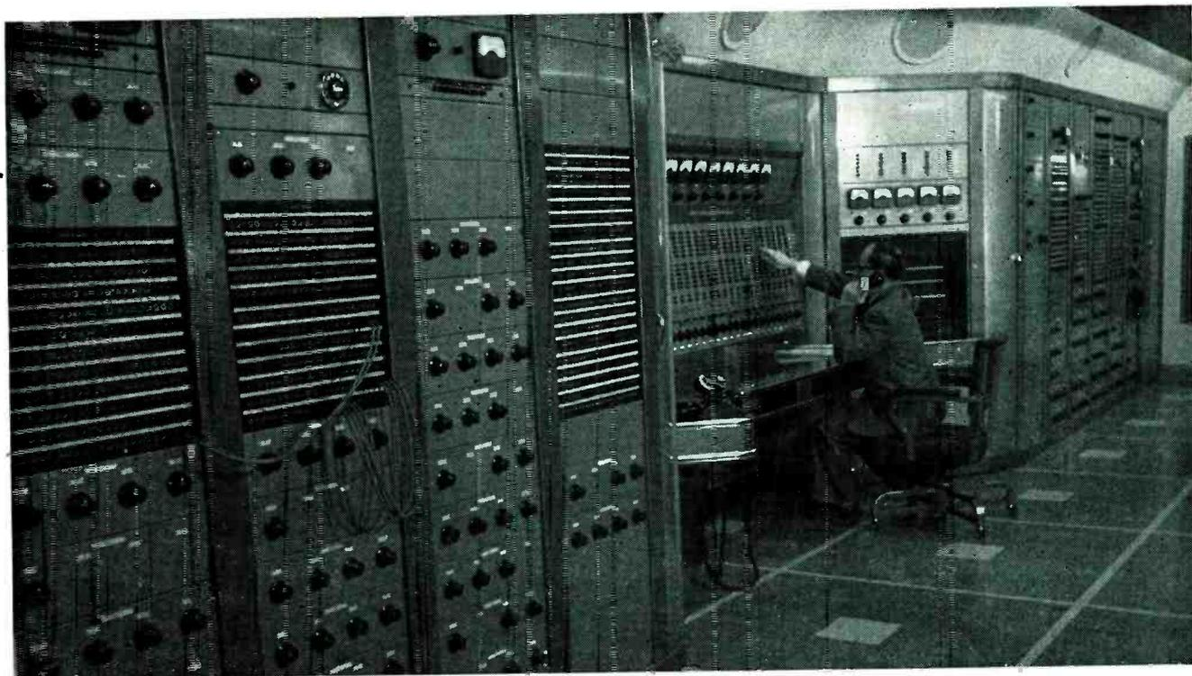
Master control board stretches the width of the room, but the most important switching circuits are under the direct control of a single operator who sits or stands before v-i monitors at center
