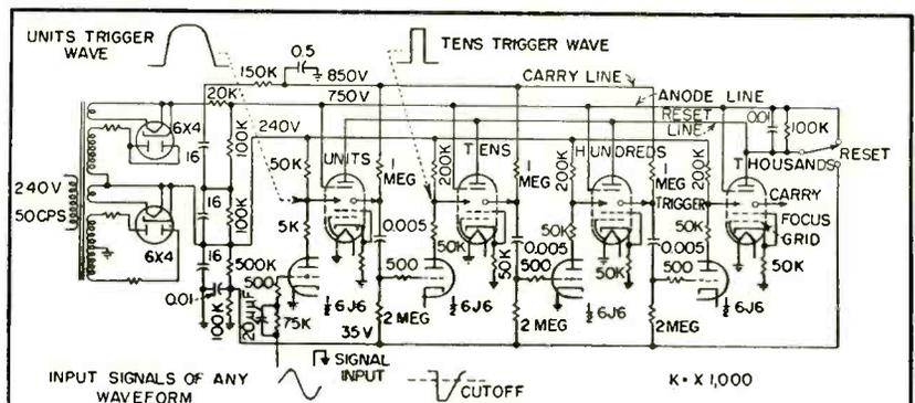
Circuit diagram and check-point waveforms of a complete counter having four scale-of-ten stages
