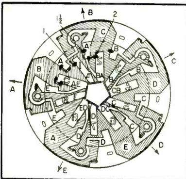
FIG. 2—Front collector plates showing the stable positions of the beam
