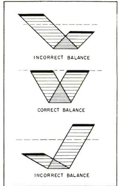
FIG. 2—Calibration patterns for correct and incorrect balance-control adjustments
