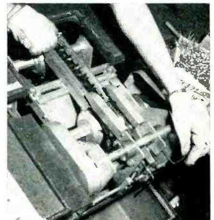
Method of changing position of cutter wheel with Allen wrench on lead-cutting machine at Emerson plant. Sample parts are taped to cardboard alongside machine, with correct chain and cutter settings for each marked alongside
