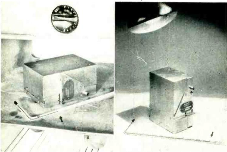
Thermometer reads  $-30^{\circ}$  centigrade as the *Permakay* selectivity reading remains same as before this extreme cold test was started
