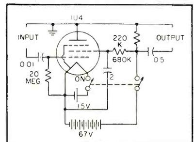
FIG. 2—Grounded-plate pentode cathode-follower circuit. Gain is 0.98
