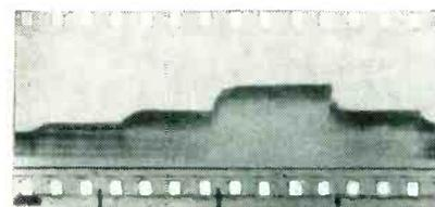
FIG. 3—Oscillogram shows response to 1, 2 and 5-mv steps
