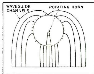
FIG. 1—Source motion produced by feed-horn rotation
