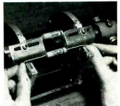
Sample capacitor is placed on adjustable guides of CBS-Columbia machine to show operator correct position of outer-foil end when leads are cut to unequal lengths
