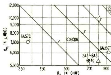
FIG. 1—Some typical tube types compared under varying conditions
