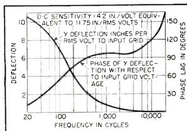
FIG. 3—Sensitivity and phase characteristics of Y-axis open loop deflection
