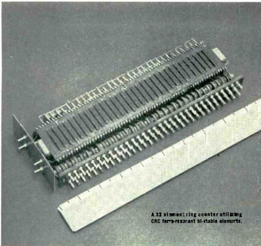
A 32 element ring counter utilizing CRC ferro-resonant bi-stable elements.
