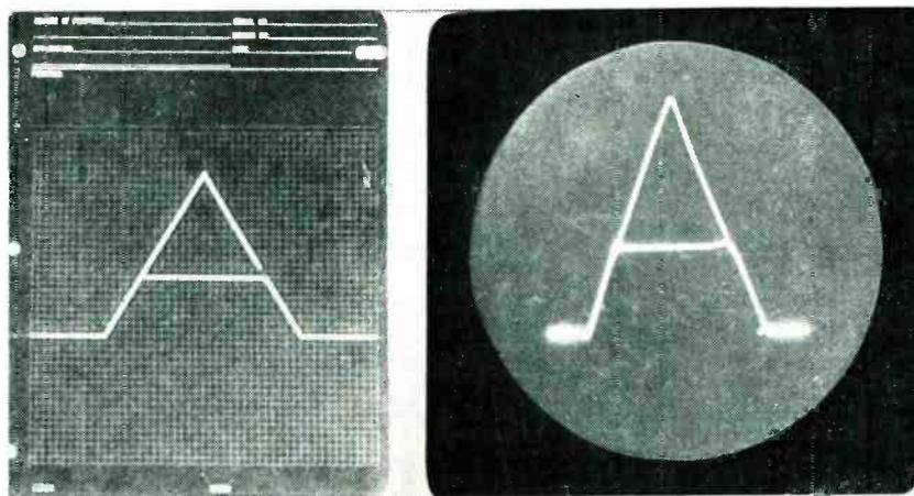
Multivalued functions may be handled by generator. Graph input of desired function at left may be compared with generator output as displayed at right on externally-connected oscilloscope
