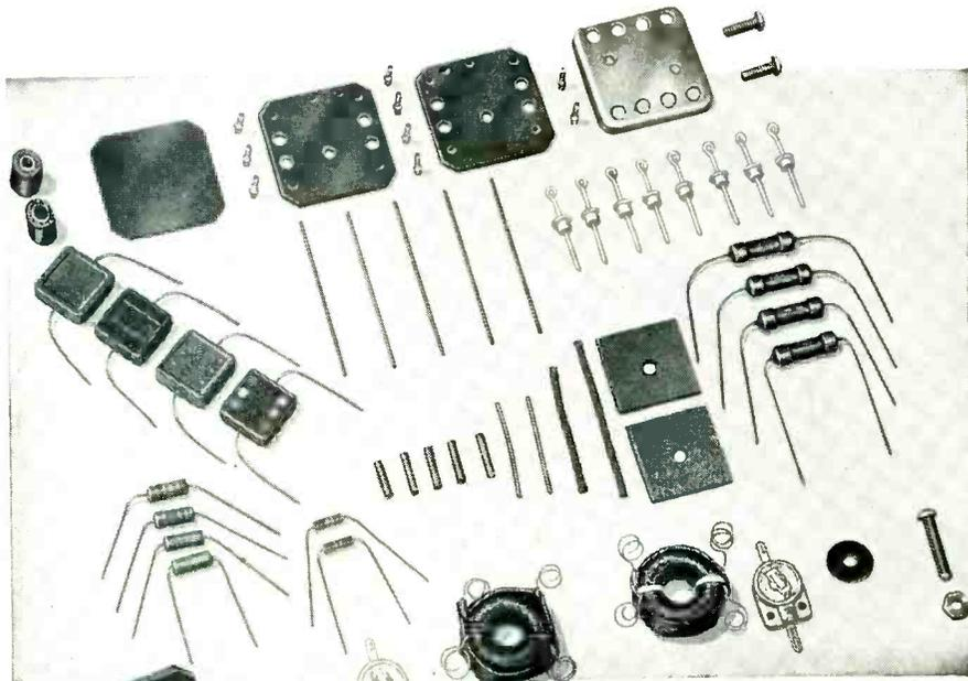
All of these 66 parts are from a single B&W Toroidal-coil type discriminator only 1 $\frac{3}{4}$ " square by 3 $\frac{1}{2}$ " long exclusive of terminals!
