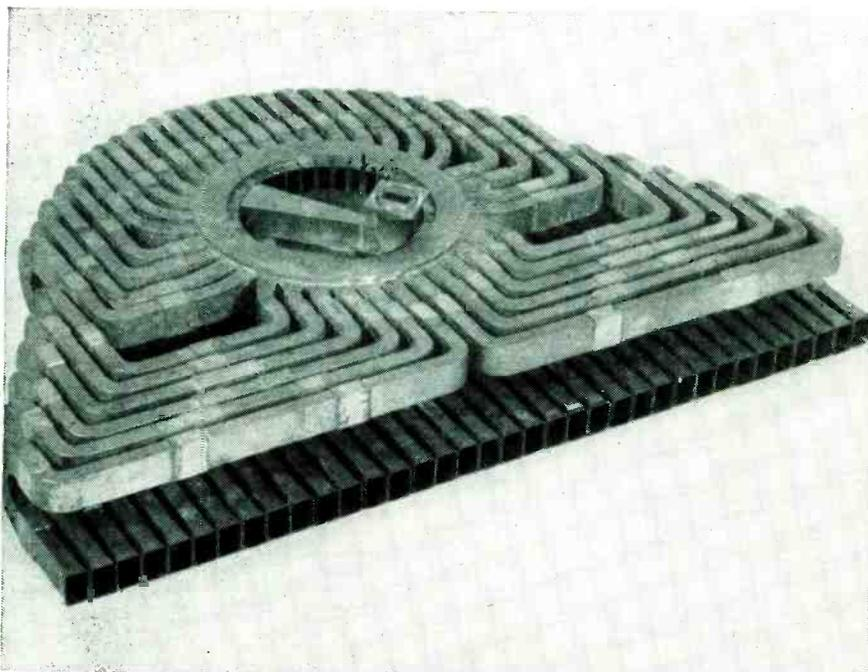
Experimental model of the organ-pipe scanner
