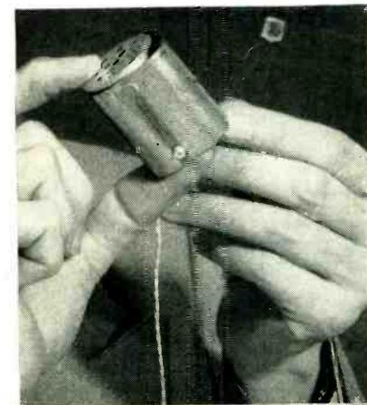
Experimental radio transmitter built at General Electric. It uses germanium transistor (right) and has broadcasting range of several hundred feet
