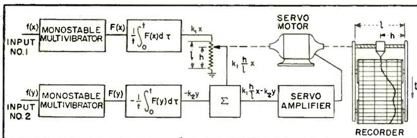
FIG. 1—Block diagram shows setup for determining ratio between recurrent rates of pulses from two different sources
