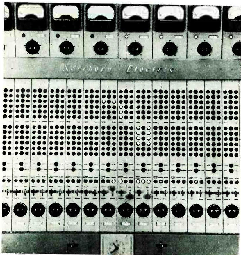
Portion of the main switching system for Radio Canada. System permits selection of inputs from which program is connected to one or more outputs. Novel push-button-relay arrangement allows presetting connections and control to network either by master or studio
