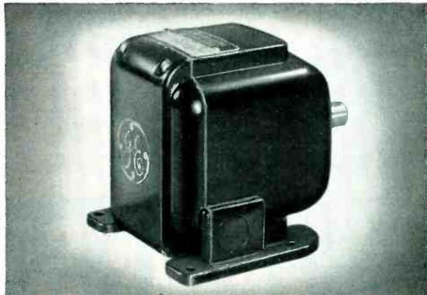
**CONTROLS**—A new plugging control for brakeless stopping of polyphase induction motors features a Carboloy permanent magnet. An eddy current disk, rotating in the magnetic assembly, creates a torque. As the motor's speed nears zero with the power reversed, the torque decrease interrupts the circuit and quickly stops the motor.
