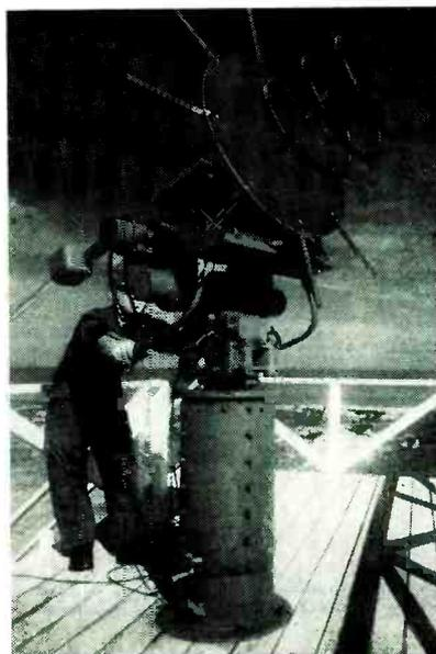
Helical antennas used at ground receiving stations provide good reception despite missile roll
