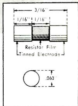
**TYPE R RESISTORS** employ noble metal film deposits on specially selected heat resistant glass. The resistance films are not spiral and have a minimum self-inductance; are only 1/20 wavelength long at 10,000 mc. Ideal for applications from DC to well above X-Band.
