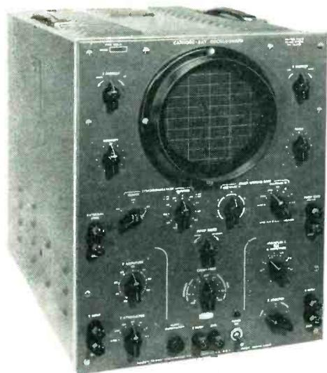
**HIGH SWEEP SPEEDS** . . . Sweep speeds considerably in excess of the rated 10"/ $\mu$ sec are available as shown by Figure 4 where a single cycle of 10 MC timing signal covers 2" on screen . . . above 10"/ $\mu$ sec, some sacrifice in positioning range and sweep linearity is experienced but measurements are still made accurately by time-calibration substitution.
