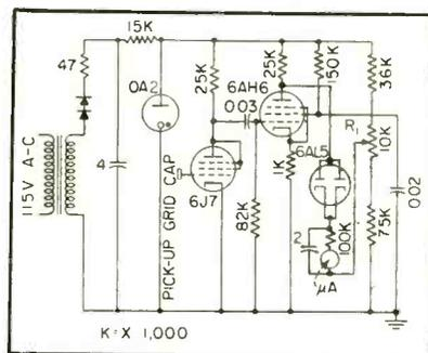
FIG. 1—Floating-grid amplifier picks up static charge. Diode meter furnishes indication of total charge and rate of decay
