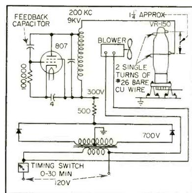
FIG. 1—Schematic and mechanical set-up for the ozone generator
