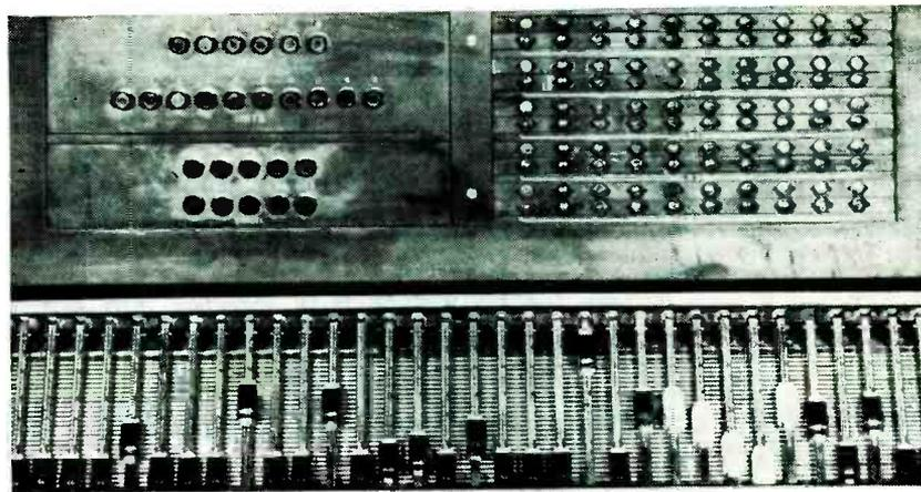
FIG. 2—Crossbar switches actuated by pushbuttons (upper left) dial up monitor speakers or volume indicators for any one of sixty program sources. Slides at bottom are cue selectors as explained in text
