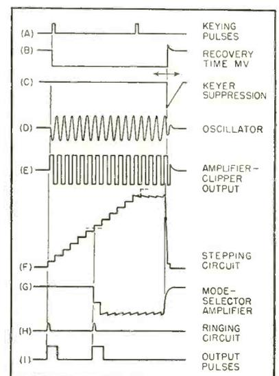
FIG. 1—Double-pulse generator waveforms
