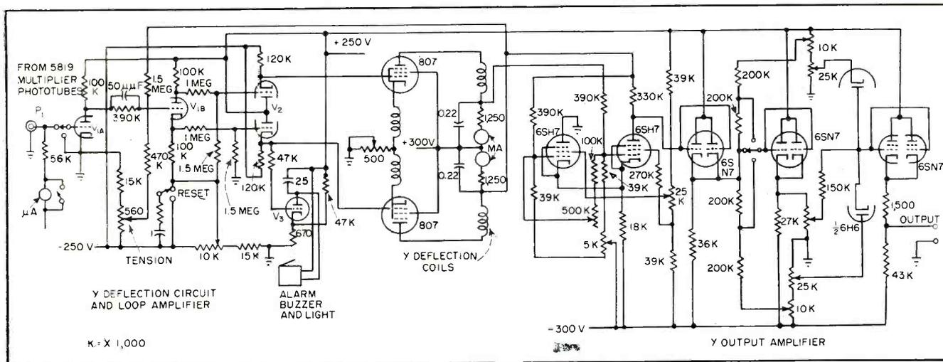
FIG. 2—Phototube transducers supply error signal to Y-feedback loop. Waveform taken from Y-deflection coils through output amplifier corresponds to desired function
