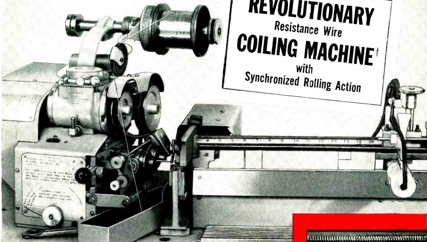
As producers of the world famous "Nichrome"\* and other outstanding electric heating and resistance alloys, Driver-Harris engineers are interested in obtaining application results commensurate with the exceptional advantages their alloys afford. Therefore they have developed a new coiling machine which eliminates wire coiling faults—especially coil irregularity due to work-hardened areas produced during coil formation.
