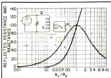
FIG. 2—Resistance and reactance reflected into tank coil are shown as percent of maximum possible reflected resistance for various values of pick-up coil reactance to load resistance ratio
