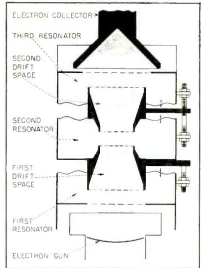
FIG. 1—Cross section of tube showing shape of cavities, drift tubes, gaps, cathode and beam
