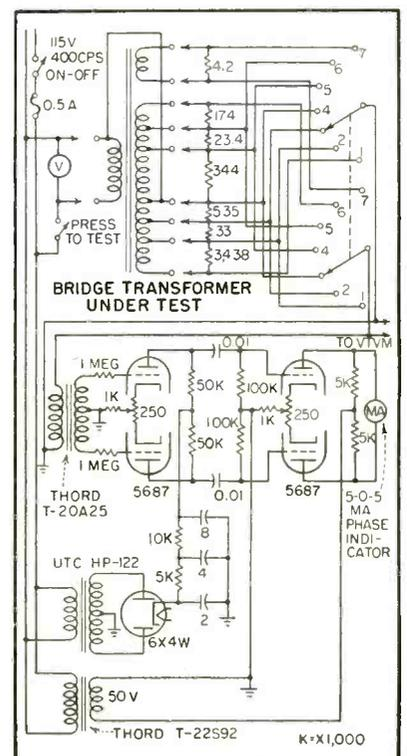
Complete circuit of bridge transformer tester. First tube is push-pull voltage amplifier, feeding second tube which serves as phase detector
