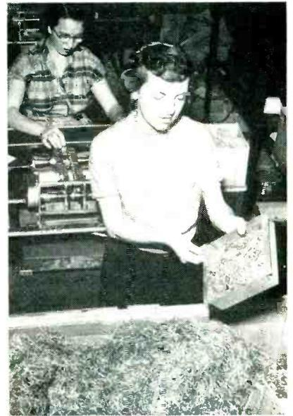
Scrap from lead-cutting machine is saved for salvage at DuMont television plant. The DuMont-developed machine in background is being used for trimming leads of mica capacitors
