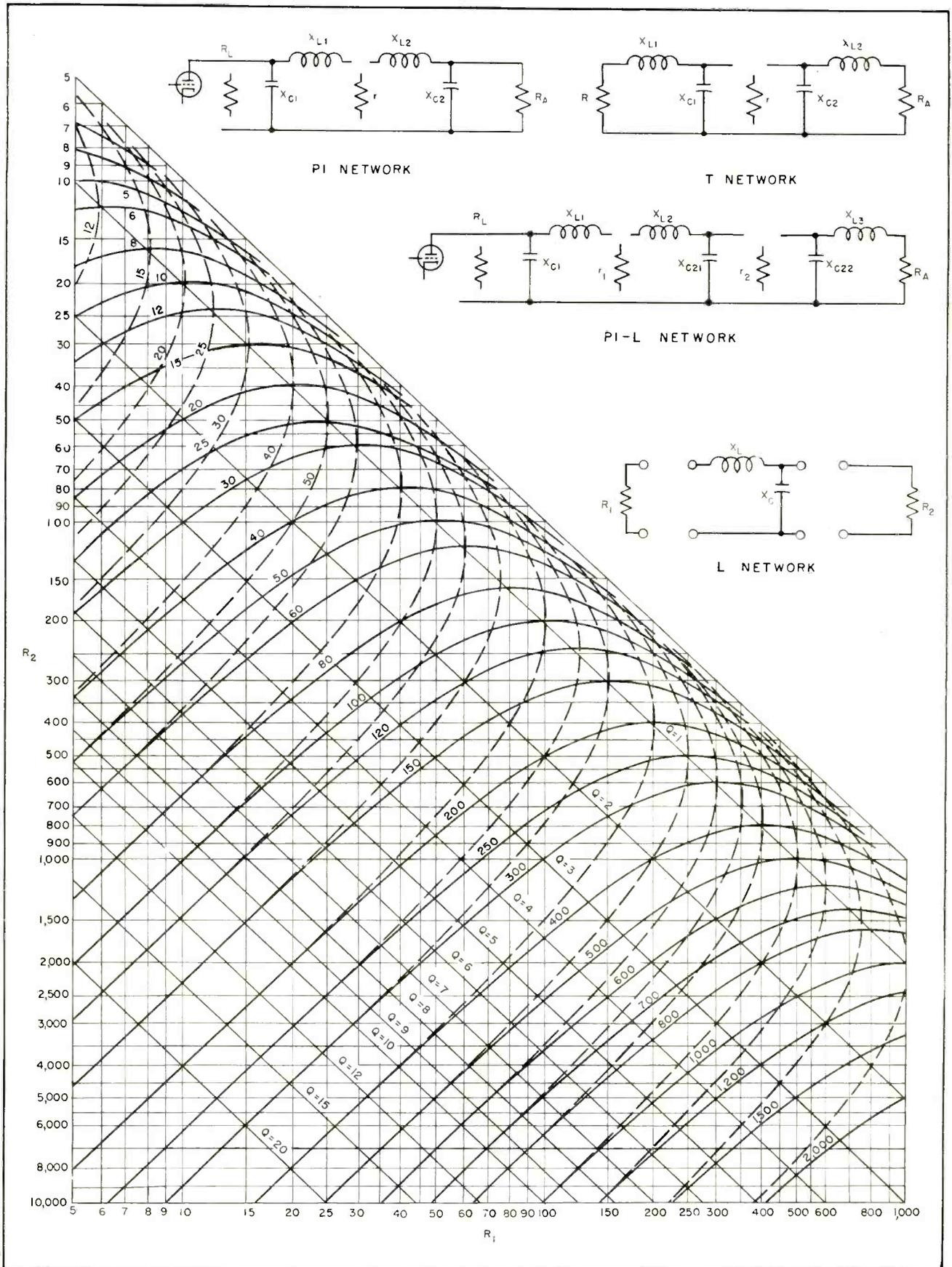
FIG. 8—Design chart for determining optimum component values for L, T, pi and pi-L networks. Inductive-reactance curves are shown solid. Capacitive-reactance curves are dashed. Use of chart is explained in text
