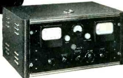
When used for different bands, plug-in type antenna coils provided. Crystal accuracy guaranteed to be  $\pm .0015\%$  over range of 15° to 50° C. Meets or exceeds FCC requirements.
