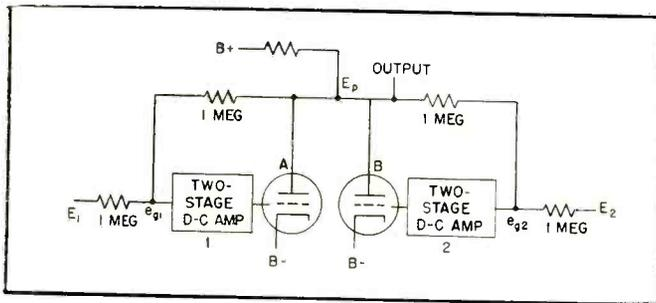
FIG. 3—If  $E_1$  is more positive than  $E_2$ ,  $E_1$  controls  $E_p$
