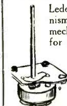
Ledex D.C. Impulse operated mechanisms rotate in 30° steps. Ratchet mechanism has 1/4" shaft with flats for standard switch wafers.
