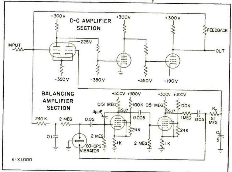
FIG. 6—A zero-drift balancing amplifier is used for greater precision
