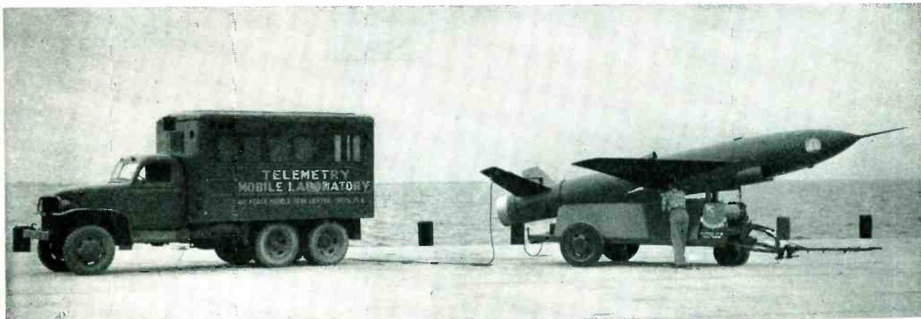
Missiles are checked out prior to launching by mobile test laboratory that indicates last-minute adjustments of instruments
