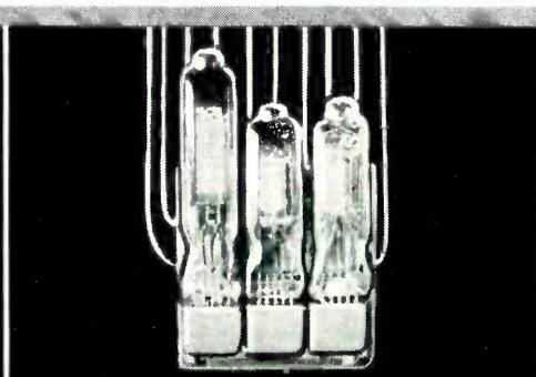
**New Sub-miniature Model III Ampec** — a full three-stage speech amplifier of remarkably small dimensions — approximately 1 1/2" x 1 5/8" x 1 1/2" (barely larger than a postage stamp!). Excellent for microphone preamplifiers and similar applications. Check No. 42-130 on coupon for complete information.
