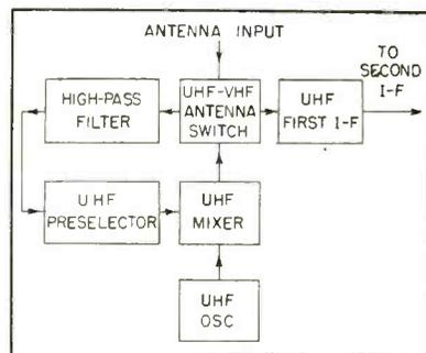
FIG. 1—Block diagram of the vhf-uhf tuner
