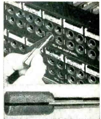
Removing dummy plug from jack after using it to speed insertion of the flat burnishing strip between the jack contacts
