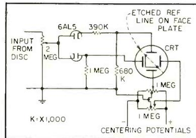
FIG. 1—Basic circuit of L-pattern tuning indicator
