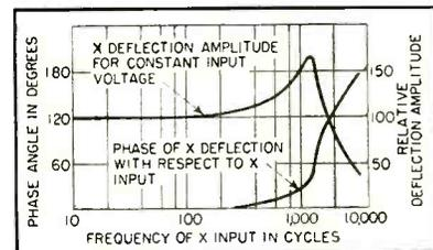
FIG. 5—Amplitude and phase of X-axis deflection as functions of input frequency
