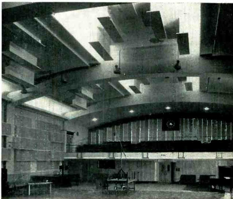
New BBC orchestral studio uses roofing-felt membrane absorbers
