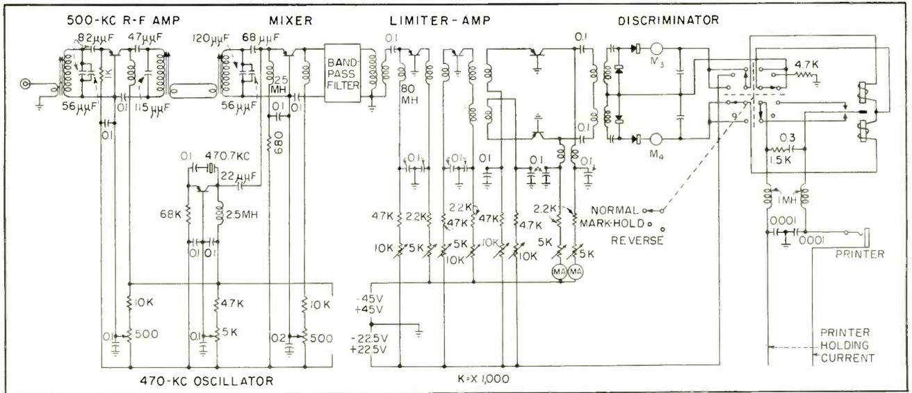
Schematic drawing of the complete frequency-shift teletypewriter converter using all transistors and no vacuum tubes
