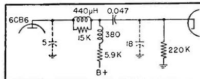
FIG. 8—Calculated constant-k filter
