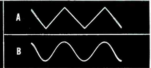
**Figure 2.** Oscilloscope of (a) triangular wave applied to shaping circuit and (b) resulting sine wave.
