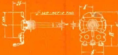
1/2 watt 70°C, 1/4" diameter miniaturized variable composition resistor.
