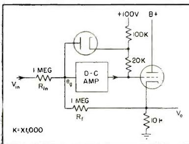
FIG. 7—Cathode follower avoids long-time discharge of  $C_1$
