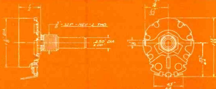
2 watt 70°C, 1 1/8" diameter variable composition resistor. Also available with other special military features not covered by JAN-R-94. Attached Switch can be supplied.
