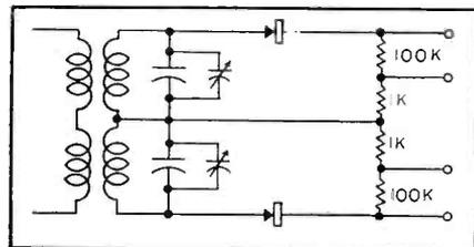
FIG. 4—Circuit of the discriminator in the original converter
