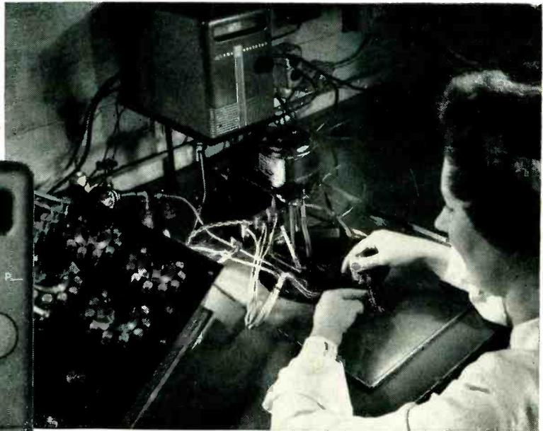
Calibrating the reference junction coils for potentiometers is typical of the measurements in which we use the compact Type E Galvanometer in our own plant. This routine measurement formerly required a wall-type galvanometer with separate lamp and scale.
