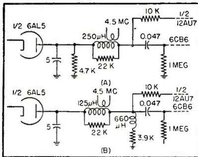
FIG. 4—Preferred wide-band peaking networks for best phase response
