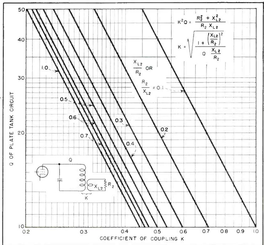
FIG. 3—Relation of  $k$  to  $Q$  for untuned coupling coil
