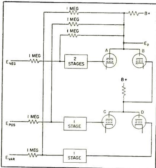
FIG. 5—Combined positive and negative limiting
