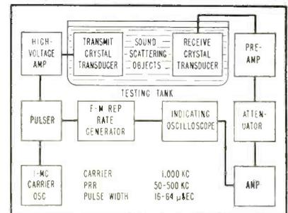
FIG. 1—Block diagram of sound-scattering investigation equipment
