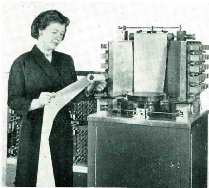
"Flying Typewriter" produces typewritten copy at speeds up to 900 lines per minute from digital computers or binary-coded communications circuits
