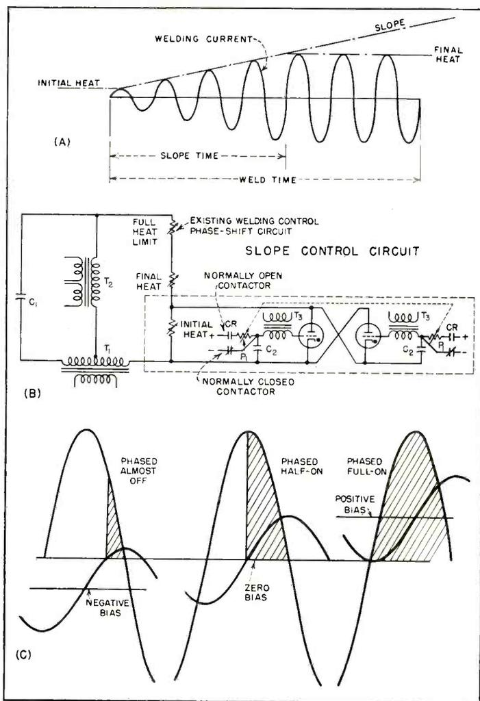
FIG. 1—Waveforms and circuit of new accessory control for standard synchronous and nonsynchronous electronic controls for resistance welding of difficult or heretofore impossible jobs
