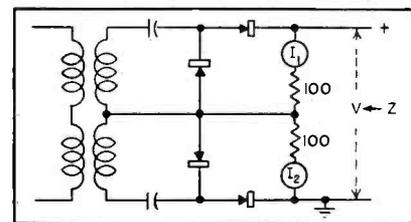
FIG. 5—New discriminator circuit using series-resonant circuits
