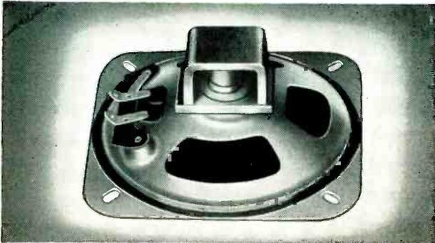
**SPEAKERS**—Many radio and TV speakers now use Carboloy permanent magnets to replace other electrical fixtures in the voice coil. Current passing through this uniform magnetic field causes the voice coil and attached cone to vibrate in proportion to the applied voltage . . . producing truer tone. These Carboloy magnets will never fail, never need maintenance. Permanent magnets are also used in television focusing assemblies.
