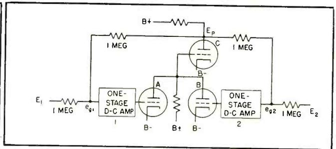
FIG. 4—If  $E_1$  is more positive than  $E_2$ ,  $E_2$  controls  $E_p$
