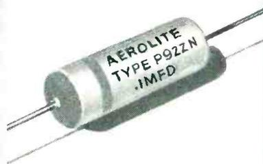
Series P92ZN Aerolene-impregnated metallized-paper capacitors are modified plastic-tubular duranite-end-sealed units in paper cases. Operating temperatures of  $-30^{\circ}\text{C}$ . to  $+100^{\circ}\text{C}$ . 200, 400 and 600 V. D. C. 0.01 to 2.0 mfd.
