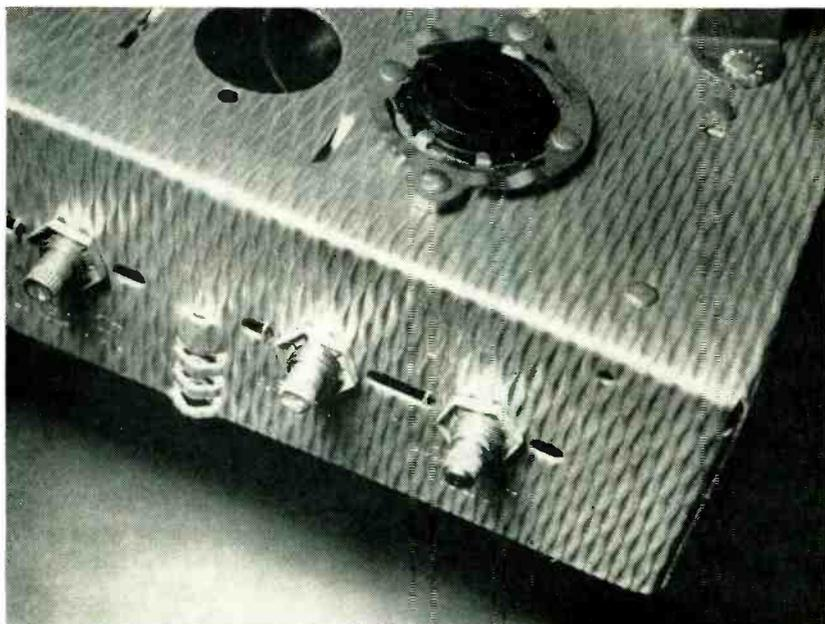
Example of television-receiver chassis made from rigidized steel, showing feasibility of conventional punching, forming, stamping and riveting operations
