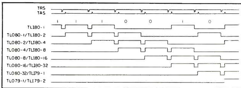
FIG. 3—Timing diagram shows spacing and duration of pulses in a typical section of control circuit
