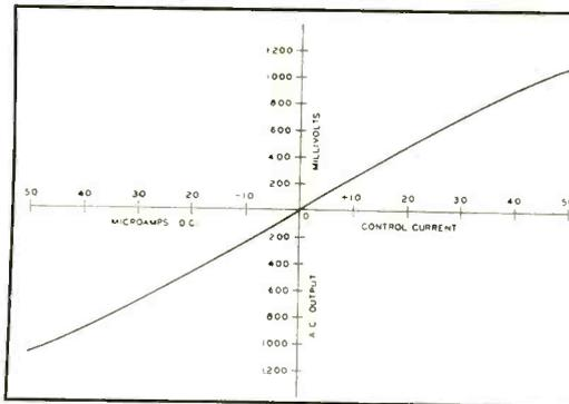
For conversion of a D. C. signal into a modulated carrier, where long life and reliability are important, as in power and instrument servos. Modulator output may be amplified to drive the control phase of a two phase servo motor.
