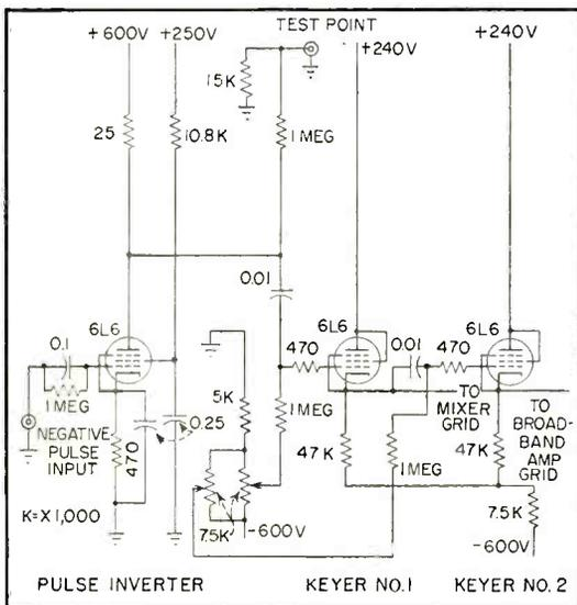
FIG. 2—Circuit of typical pulse inverter and cascade cathode-follower keyers used in Fig. 1
