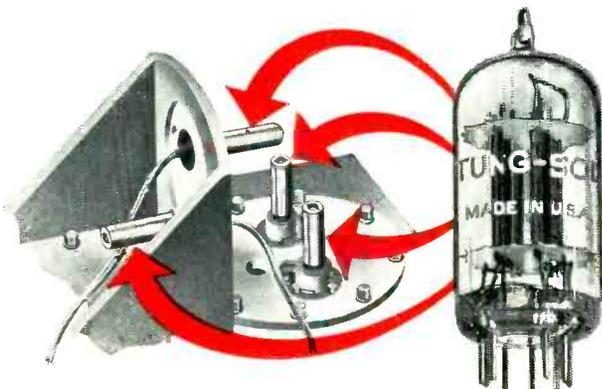
The four tubes are mounted in different positions to determine stability in all directions. Each tube is wired to a control panel where any electrical damage is recorded by indicator lights.
