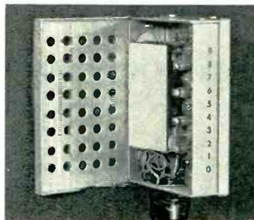
A 10 stage ring counter using 20 kc Ferro-Resonant Flip Flops
