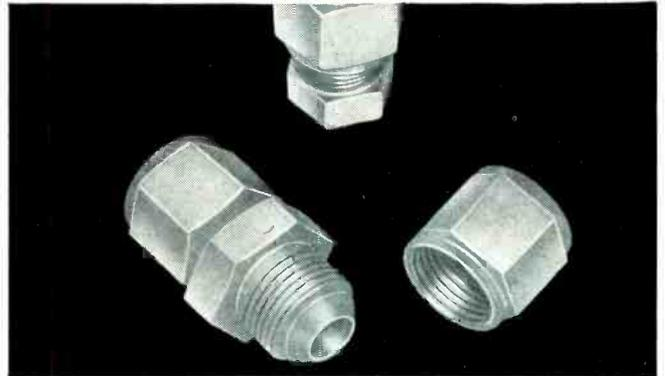
**4. Fittings for chemical equipment** are excellent examples of the design values found in five of the principal properties of Kel-F: high chemical resistance; a wide temperature range; non-wetability; plus ease of molding and machining. These commercial fittings are made from extruded rod which is conventionally machined to final, close tolerance.
