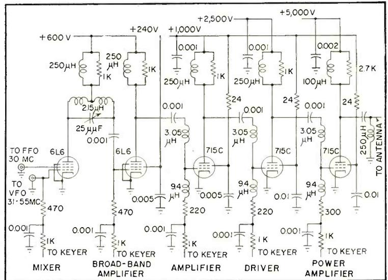
FIG. 3—Broad-band amplifiers used over the range 1 to 25 mc without band switching
