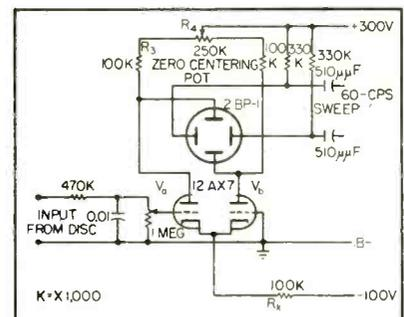
FIG. 4—Basic indicator circuit utilizing modified cathode-coupled amplifier
