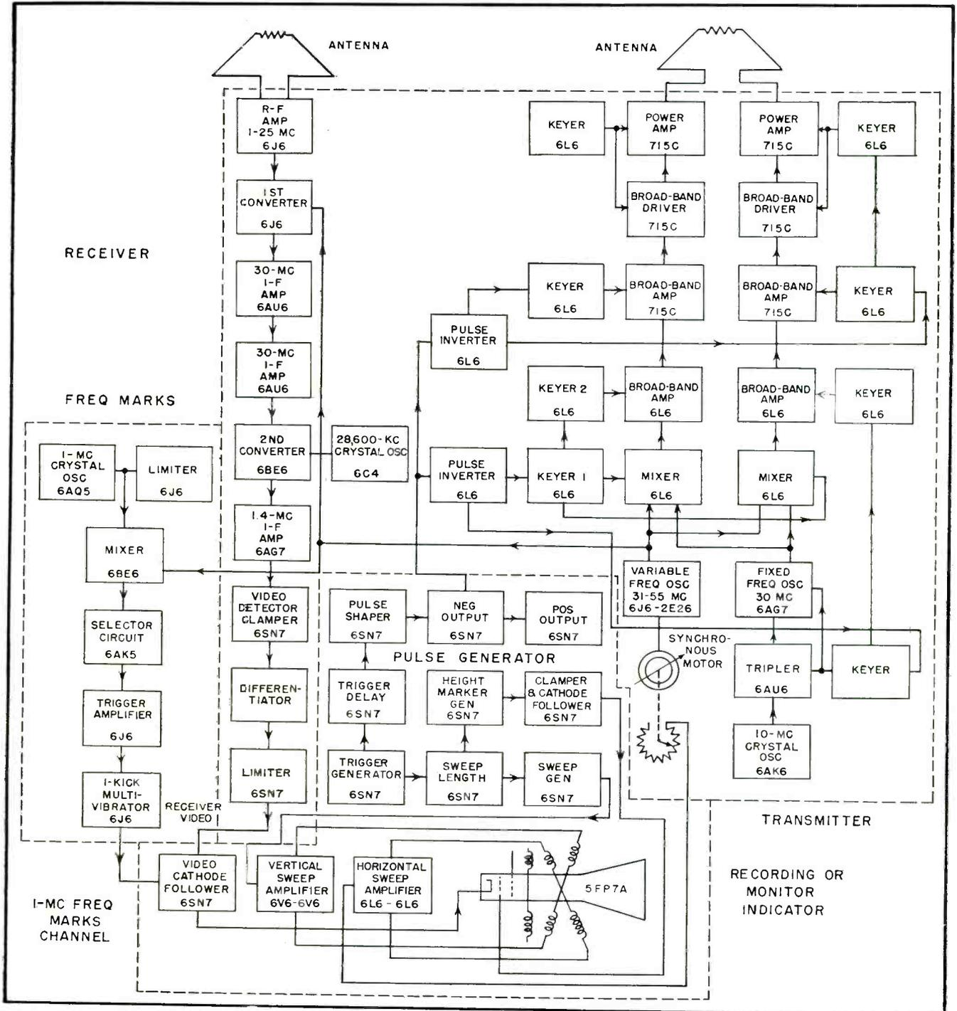
FIG. 1—Pulse generator, transmitter, receiver and recorder elements that make up the complete ionosphere recorder
