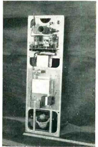
Main equipment panel of the weather station. Transmitter and keying oscillator are located at top and compass for indicating wind direction on bottom
