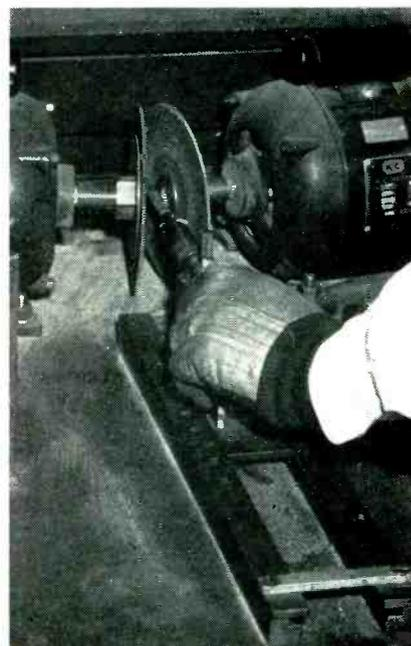
Pushing fixture in for rough grinding of soldering-iron tip. Metal protective cover, normally over grinding wheels, has been removed to show operation more clearly
