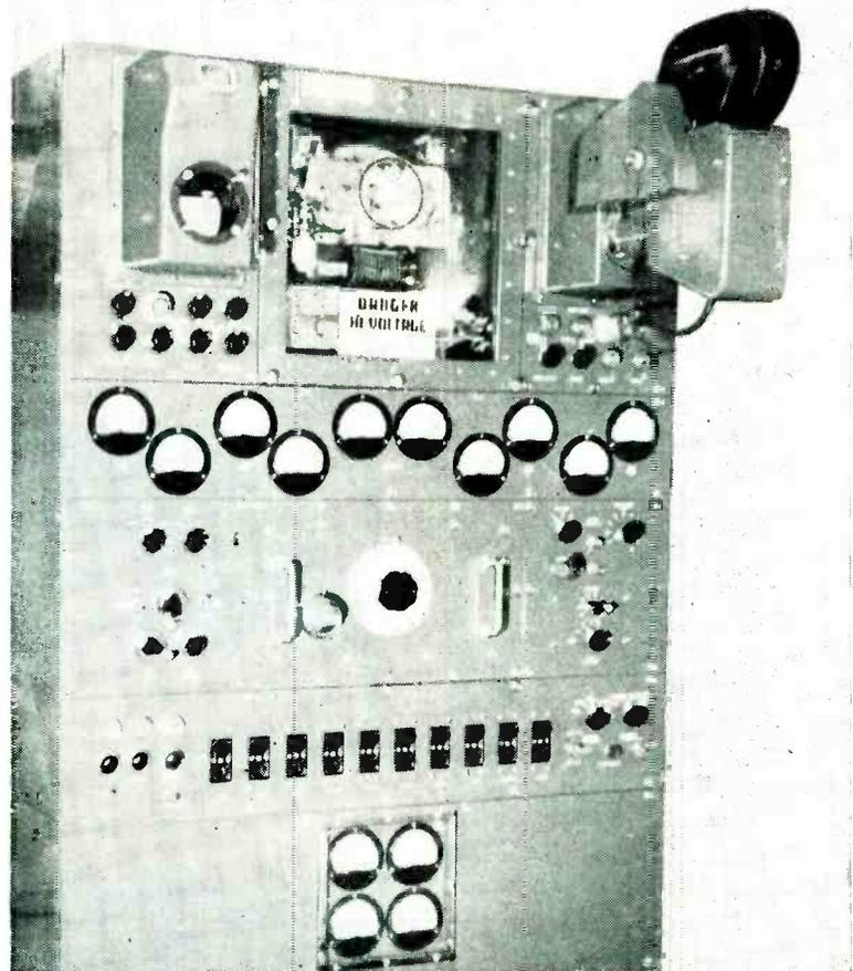
Complete transmission-recorder with 35-mm camera in use at upper right
