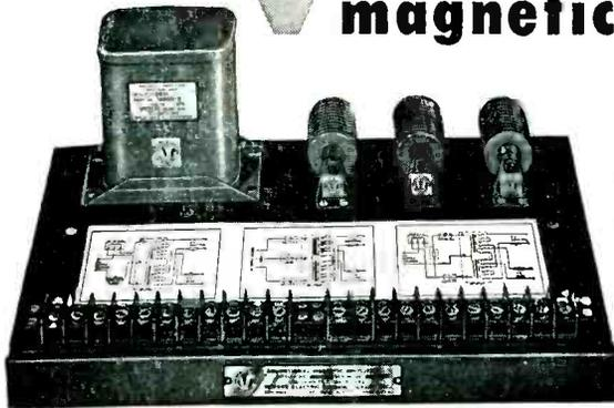
Permits study of all three basic single phase self-saturating circuits
