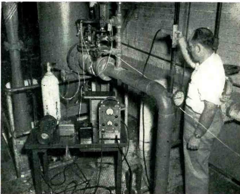
Operator is shown inserting a General-Electric leak detector in the exhaust pipe of a deodorization process in a food plant. Freon gas is sprayed over the system and a leak will suck the gas into the system and convey it to the detector. The detector records the leak (center) and sounds a horn (left). Position of the Freon sprayer determines the leak location
