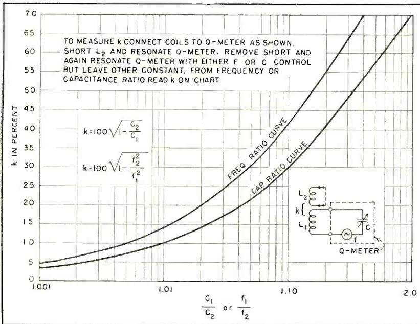
FIG. 4—Chart explains method for determining coupling coefficient using Q meter
