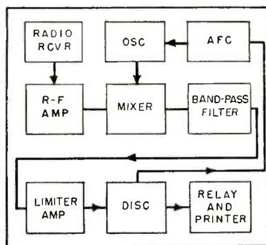
FIG. 1—Block diagram of the original vacuum-tube converter
