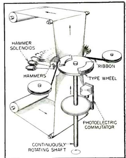
FIG. 1—Artist's drawing of printer shows positions of type wheel and printing hammers. Photoelectric pulse generator disk is beneath type wheel
