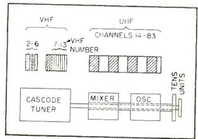
FIG. 2—Division of the television frequency spectrum
