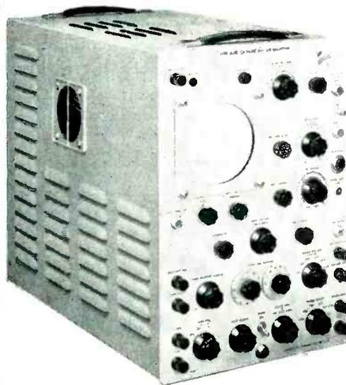
Twelve kilovolts of accelerating potential provide the light intensity necessary for photographic recording of single high speed sweeps, or visual observation of pulses of low duty cycle. Signals producing 0.5 cm or greater deflection will trigger the sweep. Trigger pulses may be as short as 0.05 usec. Distributed amplifier technique provides a 0.025 usec risetime with a vertical sensitivity of 0.03
