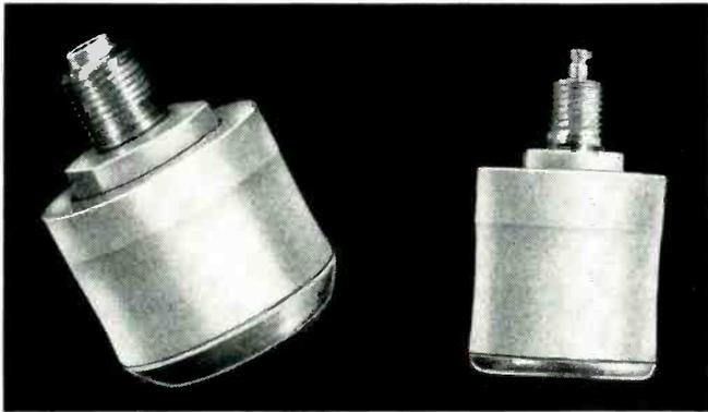
**1. For these antenna bases,** Kel-F's properties of zero moisture absorption and high electrical resistance immediately suggested it as a desirable material. However, its final selection was deemed mandatory because Kel-F could be injection molded around a metal insert, thus providing a completely hermetical seal.
