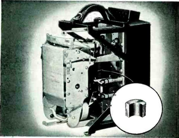
**METERS**—Here, a Carboloy concentric magnet element is the measuring mechanism of this new-type portable current recorder. The permanent magnet cut down fabrication costs by eliminating other power-supplying parts. It also reduced the recorder's weight by 10 pounds and greatly contributed to the sensitivity and accuracy of the instrument. A typical case of modernization through magnets.
