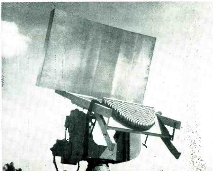
Scanner with six-foot cylindrical reflector
