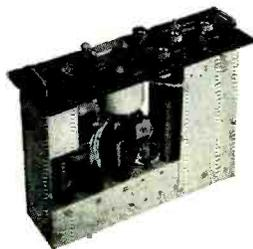
**GENERAL PURPOSE**— AC operated driver amplifiers; comprising three direct coupled push-pull stages.
