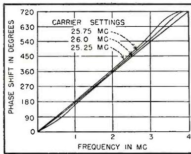
FIG. 5—Phase-frequency response of an i-f amplifier (Fig. 1) and detector (Fig. 4A)
