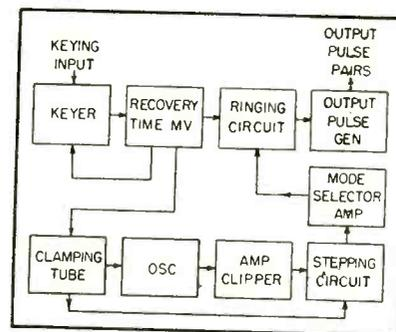
FIG. 2—Block diagram of the double-pulse generator
