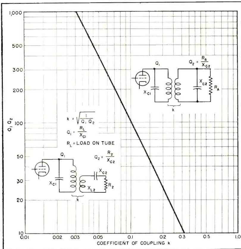
FIG. 5—Relation of  $k$  and  $Q$  for tuned coupling circuits
