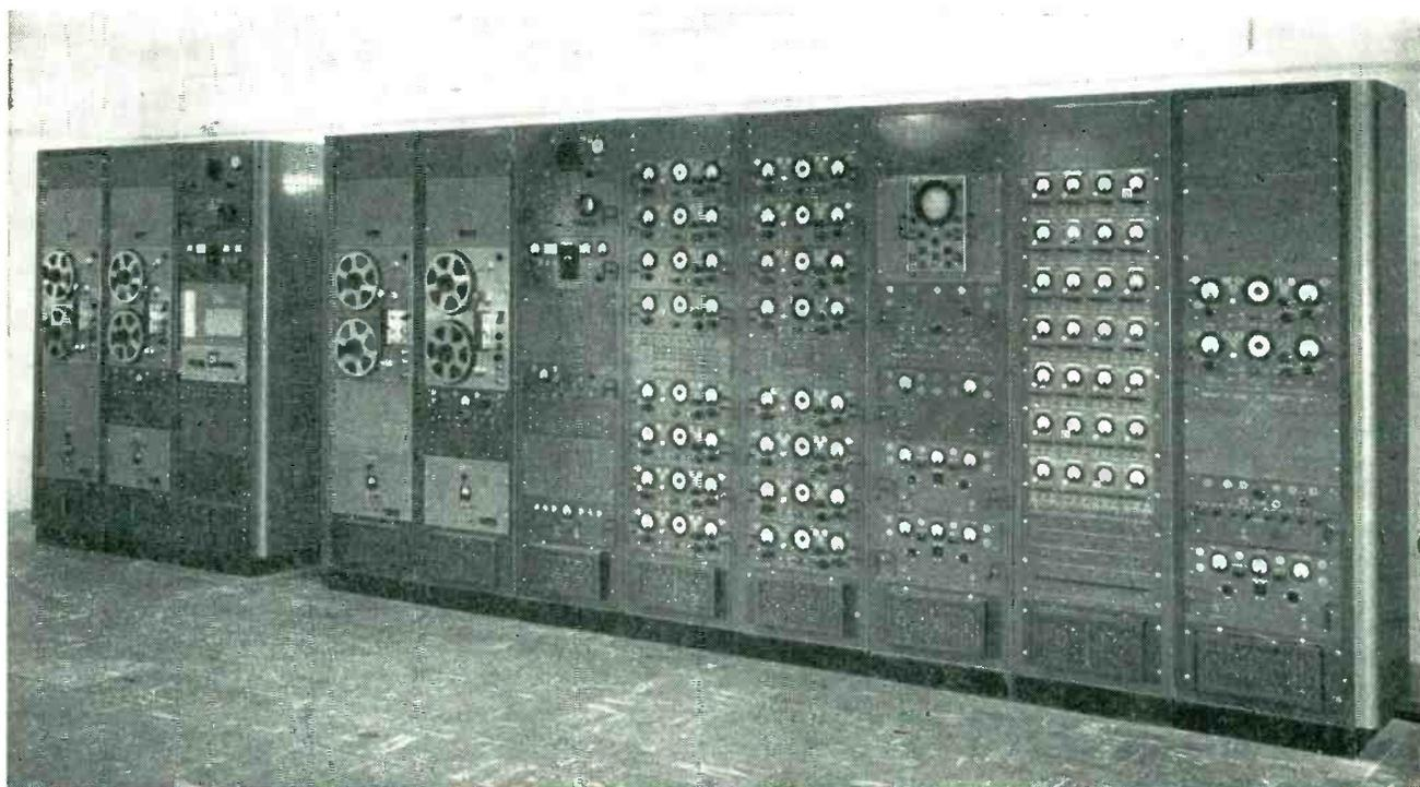
Inside view of permanent telemetry station. Eight racks at right comprise complete station, while three at left suffice for along-the-route substation
