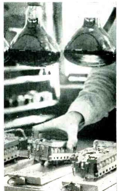
Switch arrangement for turning baking lamps on and off automatically
