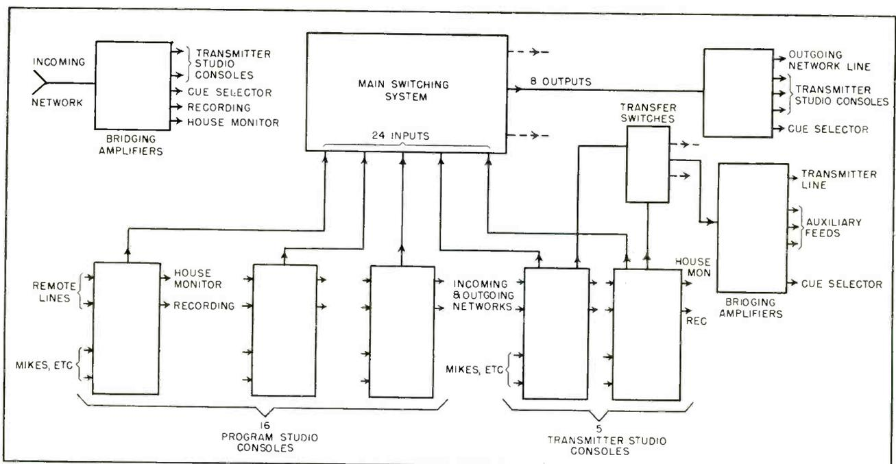
FIG. 1—Elemental layout of the main program circuits and switching systems employed at Radio Canada master control
