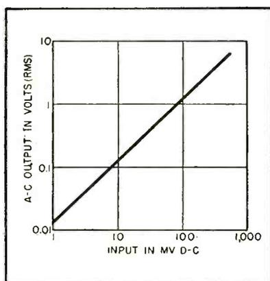
FIG. 2—Curve shows excellent linearity between d-c input and a-c output
