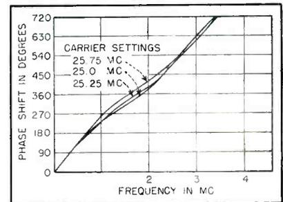
FIG. 10—Phase vs frequency of unmodified set for overall i-f and video. Three carrier settings are shown
