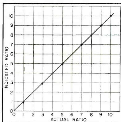
FIG. 3—Performance of ratio computer is illustrated by close adherence of ideal straight line and actual measured points
