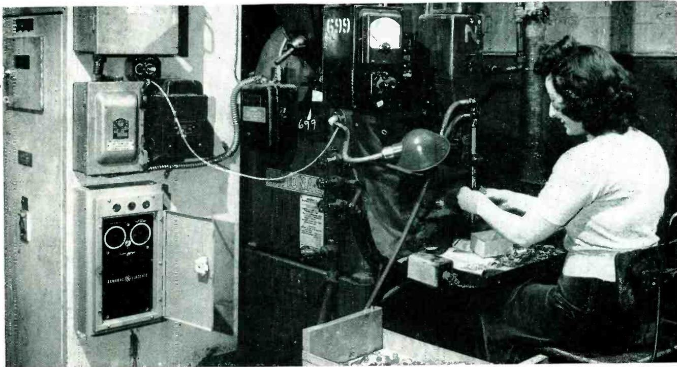
Slope control unit at lower left, incorporated in welding control cabinet, here permits welding chrome-plated beryllium-copper spring strip to steel-backed silver contact, meeting Navy specifications that the chrome plating be undisturbed by welding. This installation is in the Schenectady plant of the G-E Control Divisions
