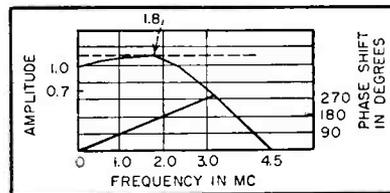
FIG. 7—Recommended amplitude-versus-frequency response of the video amplifier
