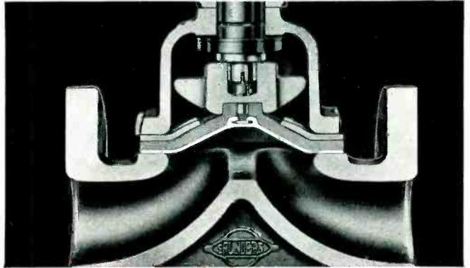
**2. Diaphragm valves for acid handling** dramatize several of Kel-F's basic values. Its use in this commercial valve points up Kel-F's properties of low cold flow (good memory); chemical inertness; flexibility; and wide temperature range. Again however, the fact the Kel-F could readily be compression molded around an insert was a determining factor in its use.
