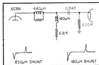
FIG. 9—Practical video circuit for cathode feed. Differentiated square-wave response for two different values of shunt
