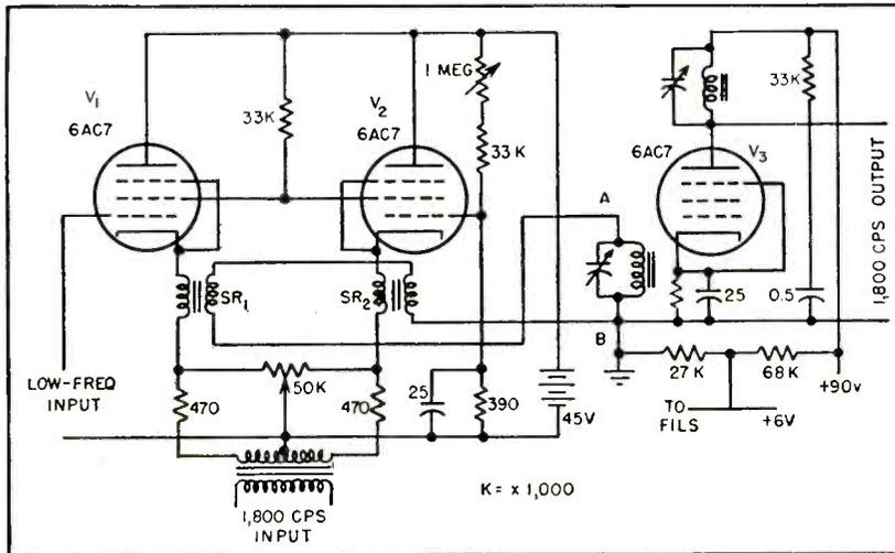
FIG. 1.—Saturable reactors are used in cathode-follower circuits to obtain high stability and good low-frequency response with high input impedance
