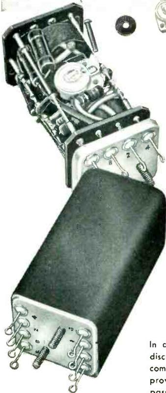
unit before and after spraying for tropicalizing and fungiproofing.
