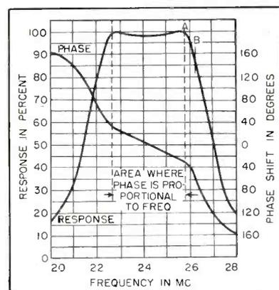
FIG. 2—Overcoupled video i-f amplitude and phase response vs frequency
