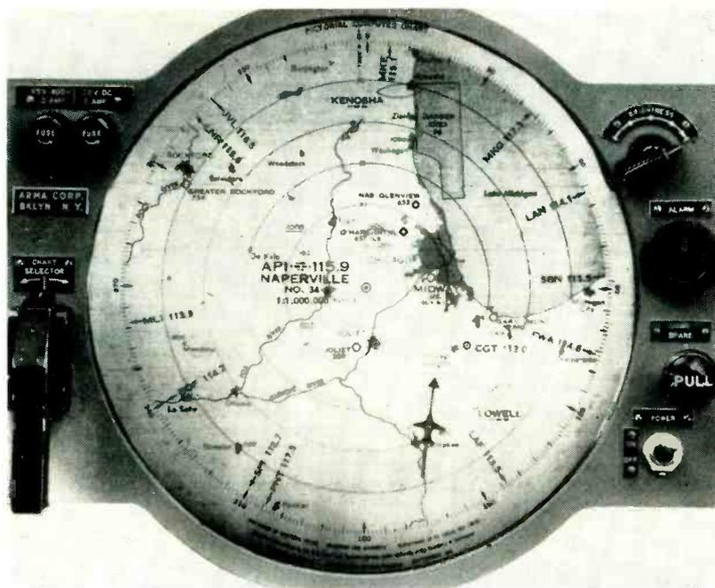
Pictorial computer gives continuous indication of plane's position and heading on charts projected on ten-inch screen on instrument panel
