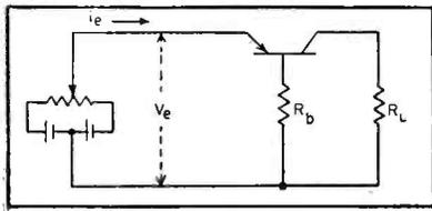
FIG. 2—Transistor circuit connection for driving a relay
