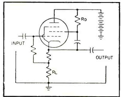
FIG. 1—Conventional cathode-follower circuit using a pentode
