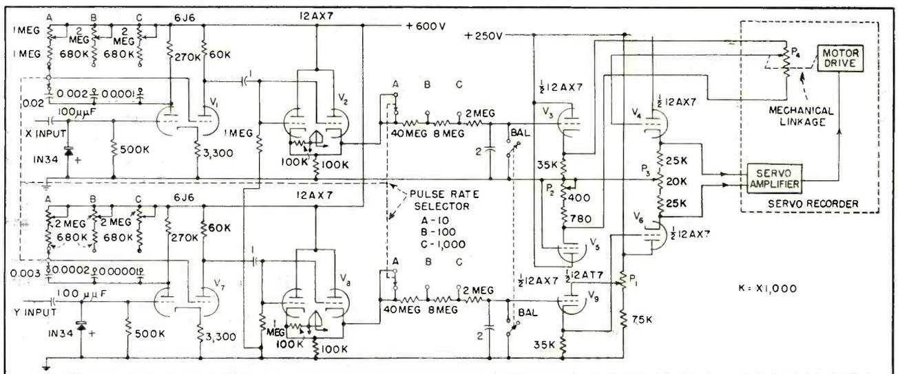
FIG. 2—Ratios between pulse rates from ten to ten thousand per minute are determined in three ranges. Note unconventional use of recorder
