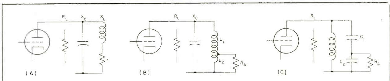
FIG. 1—Basic circuits for matching high-impedance plate to low-impedance load
