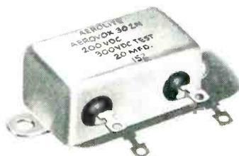
Series P30ZN Aerolene-impregnated metallized-paper capacitors housed in "bathtub" metal cases with vitrified or glass terminal seals. Operating temperature range of  $-55^{\circ}\text{C}$ . to  $+100^{\circ}\text{C}$ . at full rating; to  $+125^{\circ}\text{C}$ . at 75% of voltage rating. Capacitances available from 0.1 mfd. up to 15.0 mfd. at 150 V. D.C., and up to 3.0 mfd. at 600 V. D.C.
