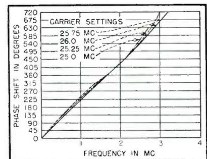
FIG. 11—Phase vs frequency characteristic for receiver with modified i-f and video circuits
