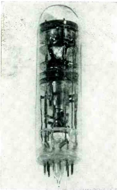
FIG. 3—Scale-of-ten counter tube. The tube is approximately four-in. long and  $1\frac{3}{16}$  in. in diameter
