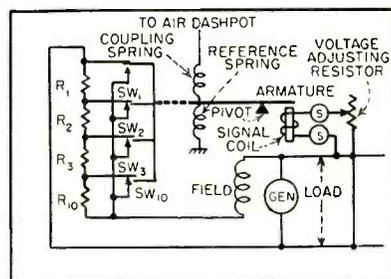
**FIG. 1**—Schematic-mechanical drawing showing operating principle of the controller
