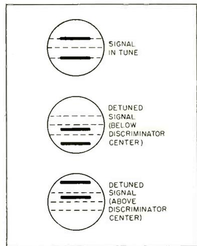
FIG. 3—Patterns obtained with two-line tuning indicator
