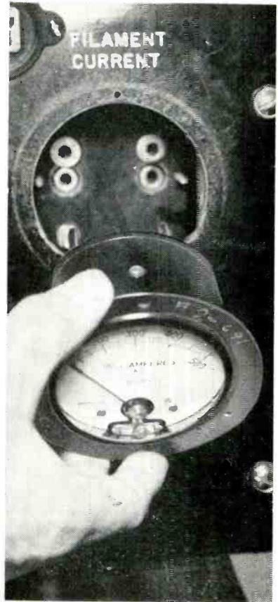
Plugging meter into test set
