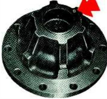
**AS A DOWEL . . .** Rollpin is used here to prevent rotation of a thrust bearing. No reaming, no special locking. Easily removed. Lowest possible dowel pin cost.
