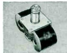
Type 4J78—High-power X-band magnetron
