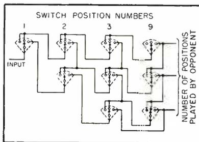
FIG. 3—Switching arrangements for the counter circuit
