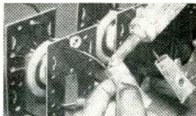
Heating open end of polystyrene sleeve
