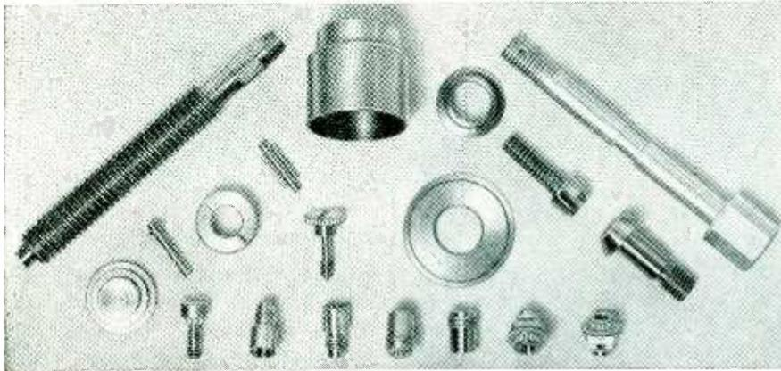
Precision-made automatic screw machine products—
