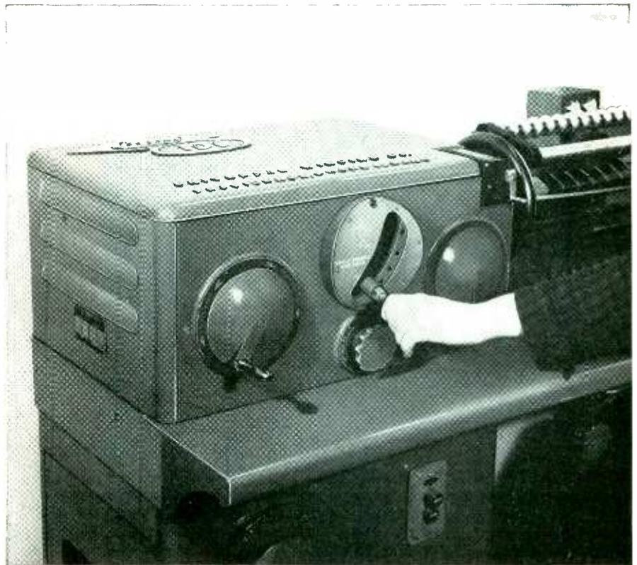
**LEESONA NO. 108 COIL WINDER**, award winner in the 11th Annual Product Design Competition sponsored by "Electrical Manufacturing," meets the demand for a modern manual paper feed machine for winding paper insulated coils in multiple or "stick" form. It winds coils from #20 to #44 (A.W.G.) in coil lengths from 1/4 in. to 3 5/8 in., in diameters, up to 5 in. round or square.
