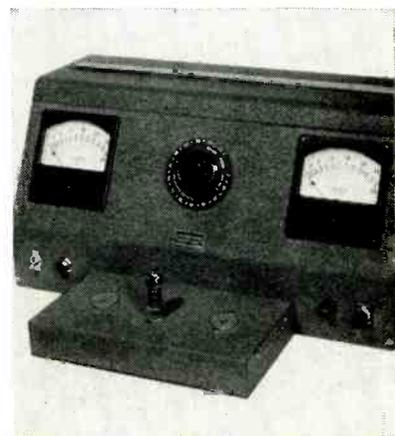
Tube test setup using circuit of Fig. 2
