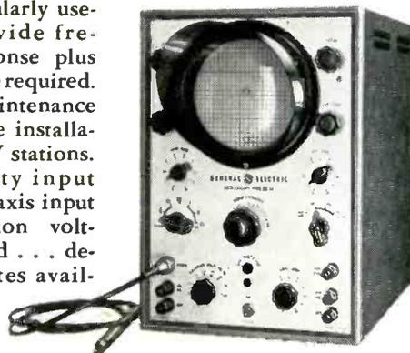
**Type ST-2A**—For general purpose use in laboratories. Excellent wide frequency response for TV receiver circuit work and industrial testing. Special features include a DC vertical amplifier to adapt the equipment to a wide range of applications. Deflection pattern can be expanded to several times the diameter of 5-inch tube.
