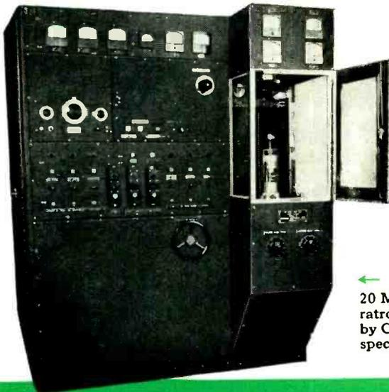
← 20 Megawatt Hydrogen Thyatron Test Equipment built by CHATHAM to customers' specifications.
