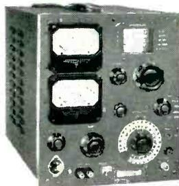
**-hp- 608A VHF Signal Generator** provides output ranging from 0.1  $\mu$ v to 1.0 v into 50 ohms. Accuracy is  $\pm 1$  db. Direct reading frequency and output calibration; no charts or interpolation required. Pulsed, cw or amplitude modulated output (50 cps to 1 mc). Resettability better than 1 mc. Has master oscillator-power amplifier for widest modulation capabilities. Constant internal impedance. Maximum VSWR 1.2. \$850.00
