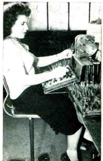
Automatic dipping machine set up for applying plastic coating to peaking coils. The same machine is also used for adding a plastic corona bead to flyback coils
