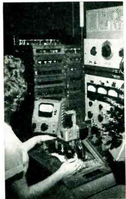
Vibration test set using magnetron magnets for 100-percent production testing of subminiature tubes
