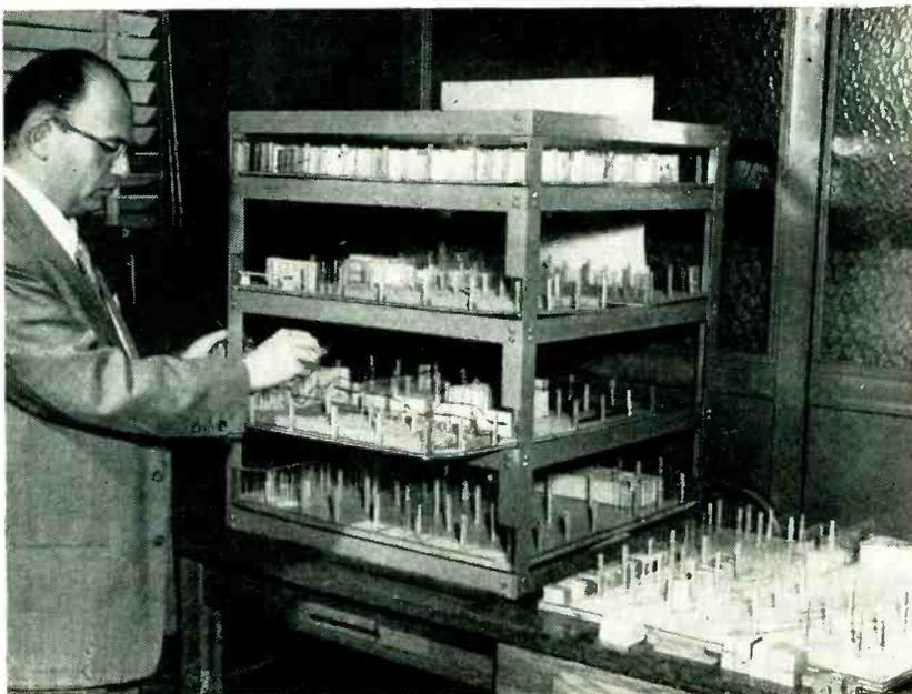
B. Bordiga, director of manufacturing at Olympic, tries out an idea for rearranging benches on second floor of his plant simply by sliding out plywood floor of model and shifting accurately scaled wood blocks. When the best setup for a new production problem is found, a draftsman is called in to take measurements and notes from which new floor plans can be drawn
