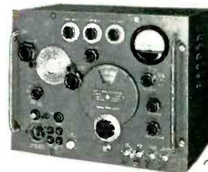
**-hp- 614A UHF Signal Generator** provides output ranging from 0.1  $\mu$ v to 0.223 v (1 mw) into 50 ohms. Accuracy  $\pm 1$  db. Has single dial, direct reading frequency and output, no charts or interpolation. Offers cw, fm or pulsed output. Widely variable pulsing, synchronizing, delay and triggering features. Extremely fast rise/decay time of 0.1  $\mu$ sec. Constant internal impedance. Maximum VSWR 1.6. \$1,950.00
