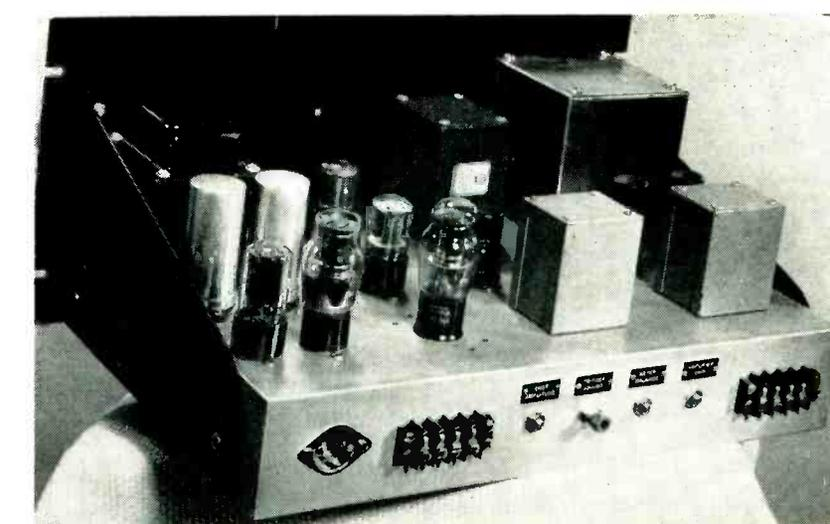
Rear of generator, showing the four preset controls for shot amplitude, trigger adjust, keyer balance and amplifier gain
