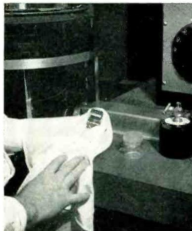
Method of handling baked-out parts with a lint-free cloth. Glass container is used for storage before baking, and container at right is used after bake out
