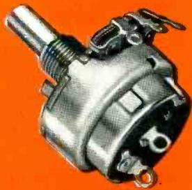
TYPE GC-35, 1 1/8" diameter variable composition resistor. Wattage rating: 3/4 watt for resistances through 10,000 ohms, 2/3 watt for resistances over 10,000 ohms through 25,000 ohms, 1/2 watt with 500 volts maximum across end terminals for resistances over 25,000 ohms. Available with or without illustrated attached switch and in concentric shaft tandem construction C2-35 as shown above.
