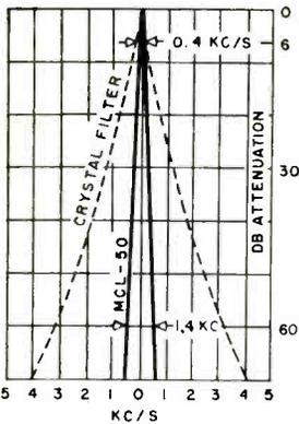
**MINIMUM:** The MCL-50 has 5 times more CW selectivity without "ringing" than 455 kc/s crystal-filter.
