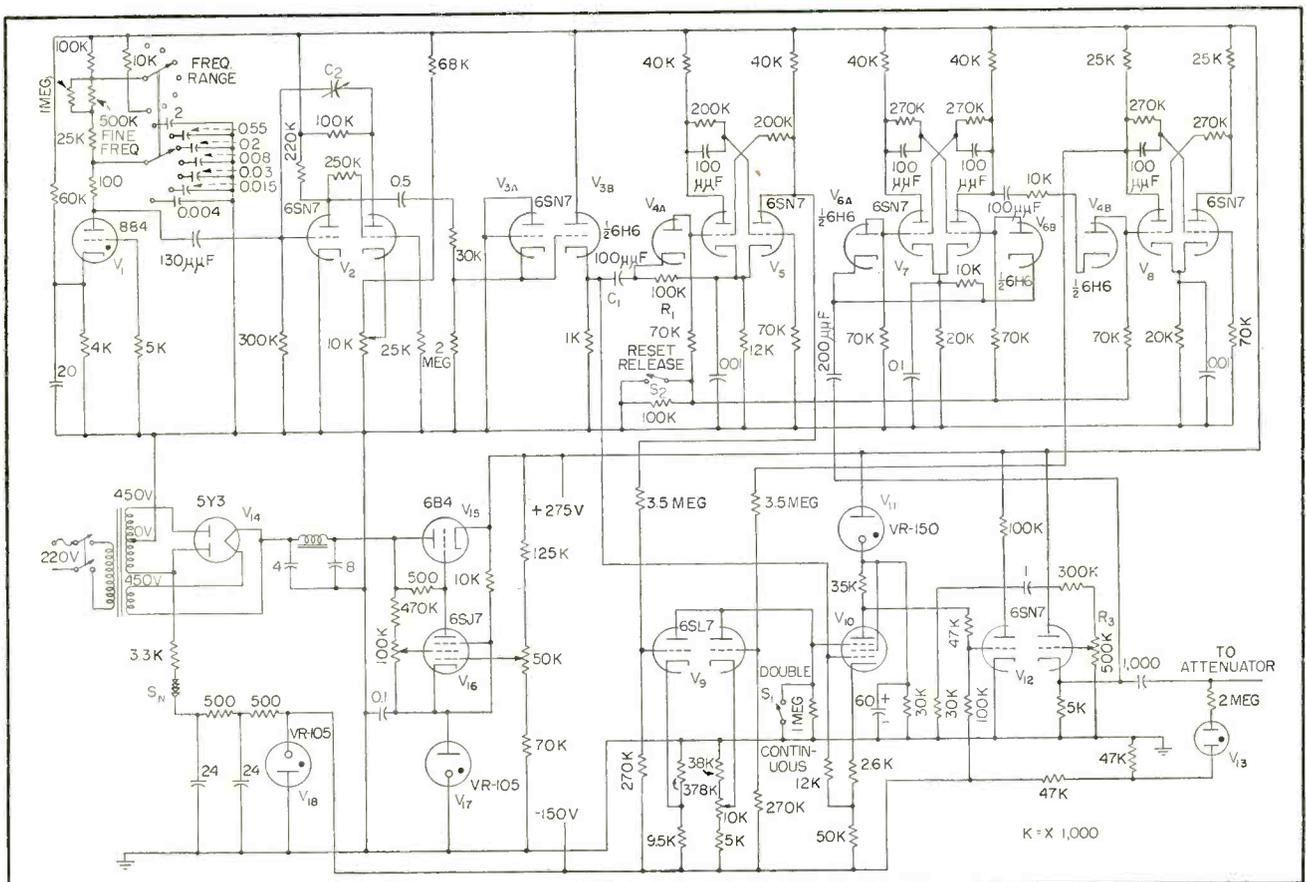
FIG. 1—Schematic diagram of the rectangular-pulse stimulus generator
