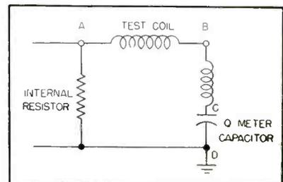
FIG. 1—Output circuit of Q meter
