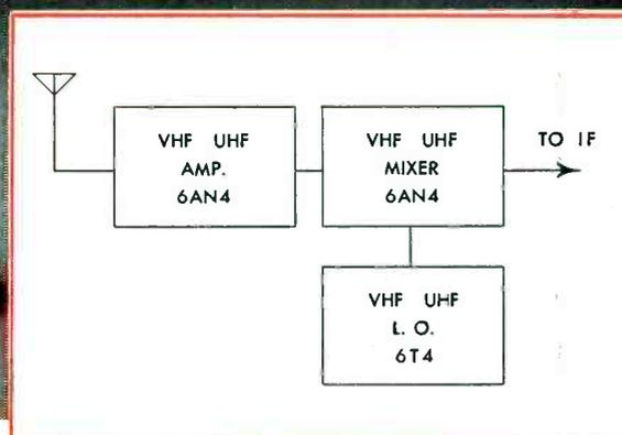
Equipment Manufacturers! Simplify design of combination VHF-UHF tuners, UHF converters for TV! Two new Sylvania-developed tubes permit adaptation of conventional amplifier-mixer-local oscillator circuit to the new frequency bands—completely eliminate complicated switching arrangements or stage duplication. Leading Tuner Manufacturers have adopted these types for current tuner production.
