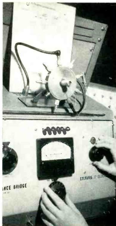
Tube is plugged into holes in center of adapter on top of bridge, and metal shield is pushed over tube as shown, for sampling inspection check of inter-electrode capacitance. Chart behind adapter gives approximate values and bridge connections
