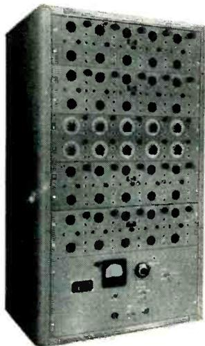
**SIMPLICITY:** Plug in pre-matched components, patch the "blocks" together, and compute.
