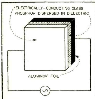
FIG. 1—Electroluminescent screen resembles ordinary capacitor
