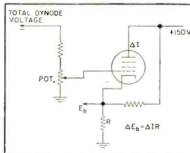
FIG. 5—Basic correcting circuit for high-intensity response
