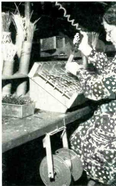
Fixture for holding three-potentiometer strips. Soldering iron is plugged into overhead outlet, and rests in horizontal holder at back of bench when not in use. Solder reel holder is screwed to bottom of bench
