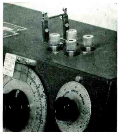
Calibrating bar in place on Q meter
