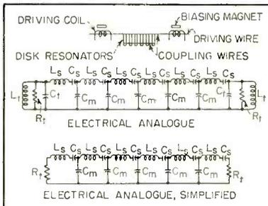
FIG. 5—Six-disk filter and electrical analogue
