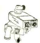
**Emerson Electric**—Part ET35300 (shown with and without housing). Used to transfer voltages between stationary and moving parts as in turrets or revolving displays. Full 360° rotation up to 15 RPM. Rating 12 conductors ten 10 amp and two 100 amp at 28 VDC. Adaptable to higher voltages. Also has swivel plumbing designed to transfer oxygen at 15 P.S.I. Size 9x6x10". Wt. 10 lbs. Price complete NEW...\$8.50
