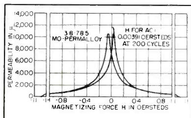
FIG. 1—Butterfly curves of one magnetic sample show typical peaks due to residual magnetism
