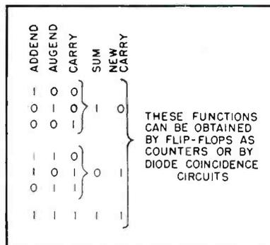
FIG. 6—Three-terminal binary adder
